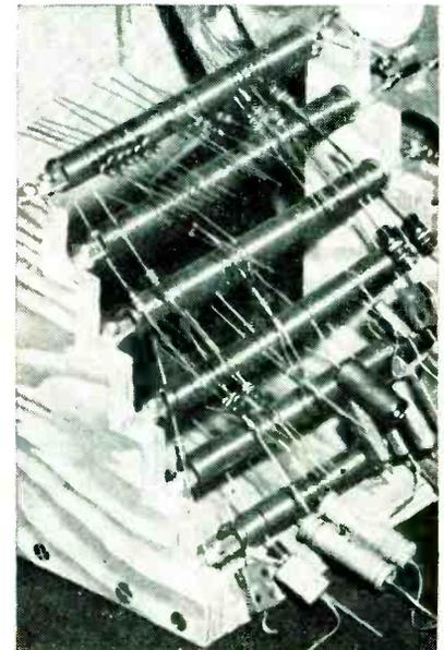
Stand made from springs, metal strips and plywood here holds parts needed for three terminal board subassemblies. Operator keeps original sample in front of her to serve as guide, supplementing prints mounted above sample
