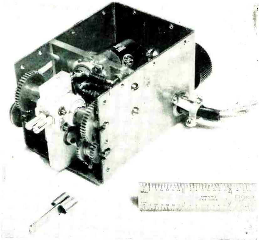
Experimental model using ceramic capacitors covers the frequency range from 430 to 975 mc continuously
