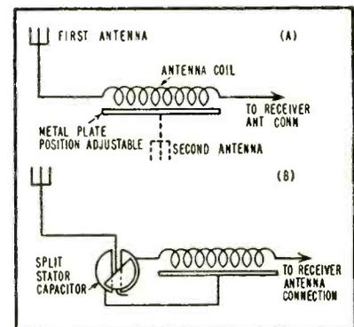
FIG. 2—Two methods of coupling opposing interference signals
