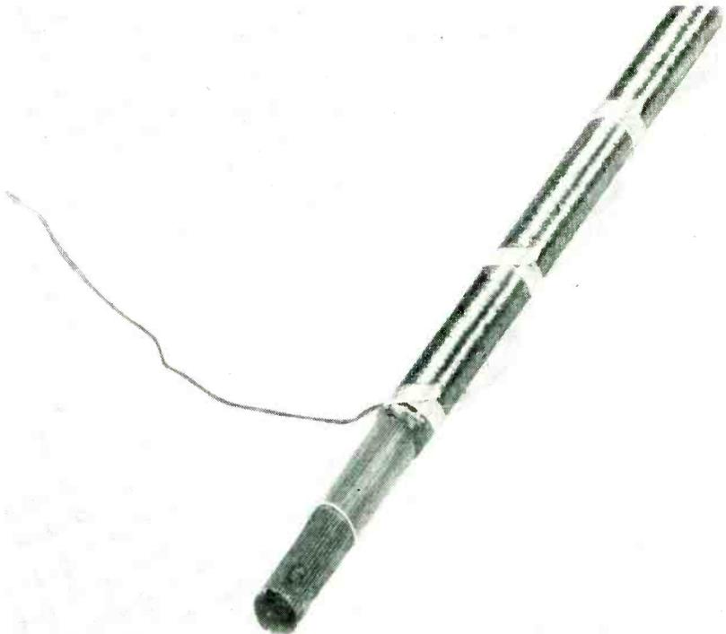
Enlarged view of end of wound delay line shows core details, dielectric and winding
