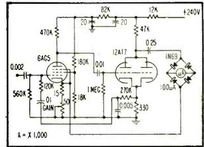
FIG. 9—One kilocycle millivoltmeter for production testing
