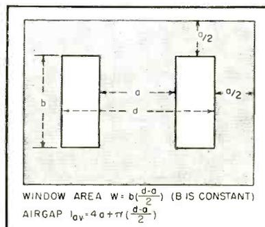
FIG. 1—Lamination shape and dimensions for standard square-stack core
