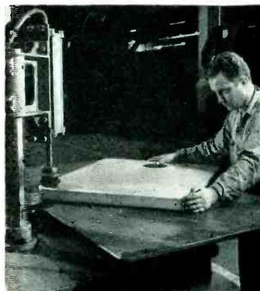
Trimming excess metal from edge of formed shell for electronic equipment housing. Rollers on bottom of pressure arm permit sidewise movement while maintaining downward pressure
