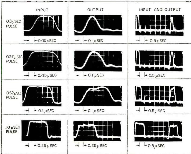
FIG. 5—Pulse response of 5,600-ohm line wound with No. 46 wire
