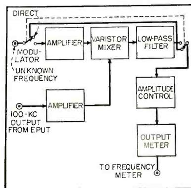
FIG. 5—Block diagram of Eput modulator
