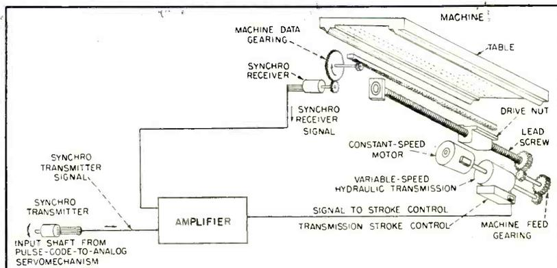
FIG. 2—Power servomechanism controlling table motion consists of synchrocontrolled hydraulic rotary transmission driving lead screw. Identical units control head and cross slide
