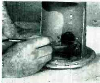
Cutting a piece of hard, brittle metal manually by means of the "Airbrasive" process.
