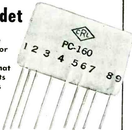
Talk about compactness — this new Pendet has it! You get 4 resistors and 5 capacitors screened and fired to a *single* Ceramic-X plate. It replaces 9 conventional components. Only 9 connections are required instead of the usual 18.
