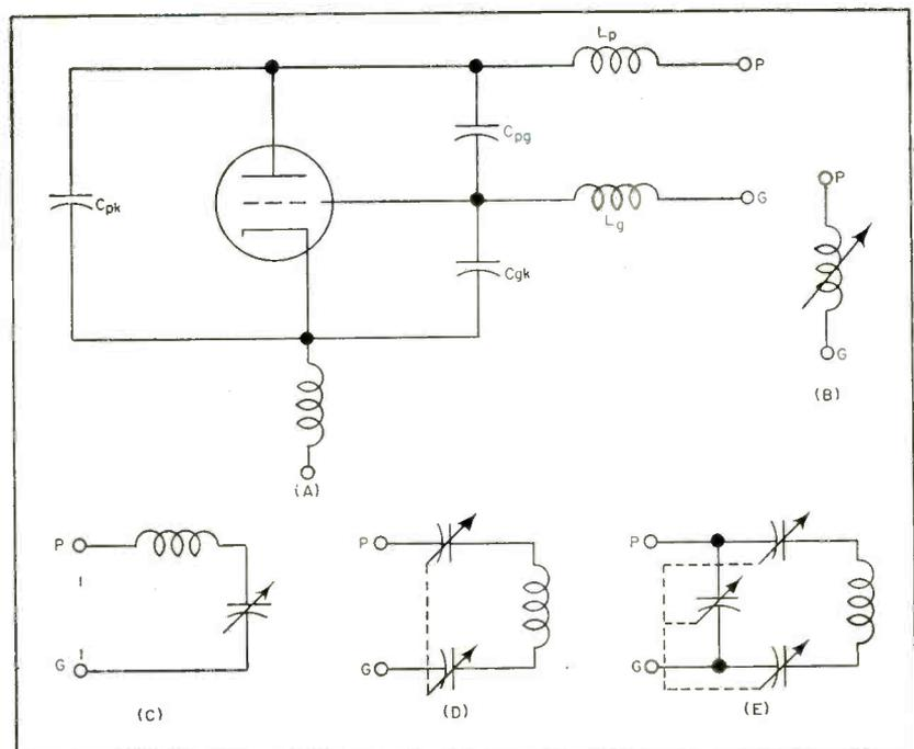
FIG. 1—Several methods of tuning a uhf oscillator
