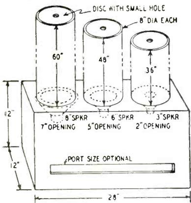
FIG. 518—Unusual three-speaker baffle (from Clifford—Radio & TV Hints)
