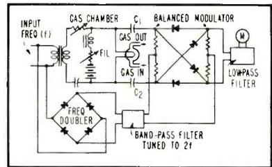
FIG. 12—Analyzer for combustible gases
