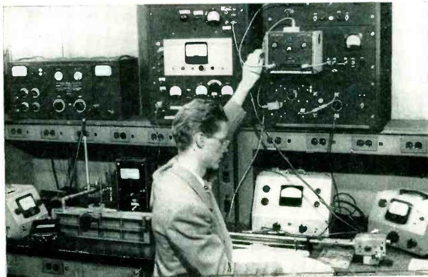
Laboratory setup of equipment used to measure characteristics of 1N72 mixer crystals
