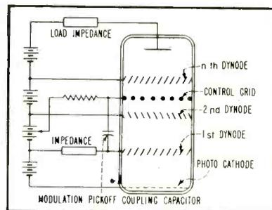
FIG. 11—Electron multiplying device applicable to television
