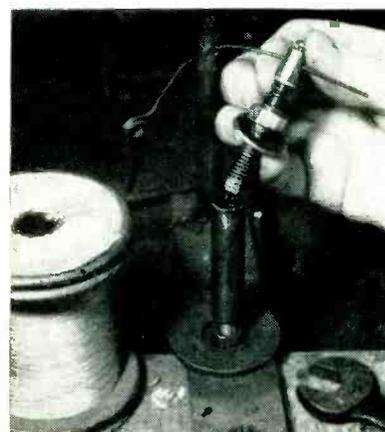
Construction of dereeler. Mounting bolt has drilled hole; dereeler bolt fits loosely in this and has two lock nuts at its bottom end so it can turn freely against slight spring friction without getting loose. Dereelers reduce wire tension and make it more constant, since heavy spool does not turn
