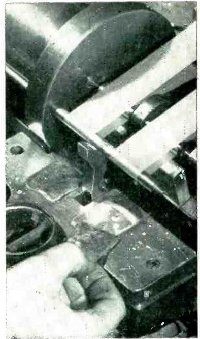
Closeup of glue pump, with pad removed to show hole through which glue is squirted up through pad each time round bar strikes lever, as shown here, during indexing of head
