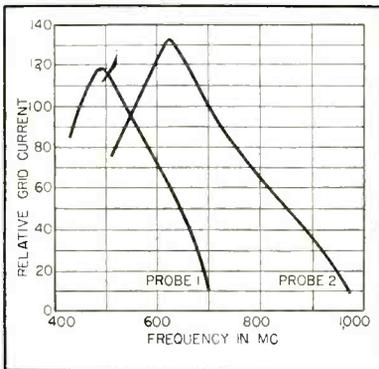
FIG. 4—Variation of grid current with frequency for developmental uhf grid-dip meter
