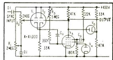
FIG. 1—The modified Miller transitron circuit
