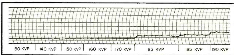
FIG. 7—Effect of x-ray voltage variation on gage output with projectile in position and stationary shows voltage change from 120 to 170 kvp produced output change no greater than change in steel thickness of 0.005 in 0.025 inch
