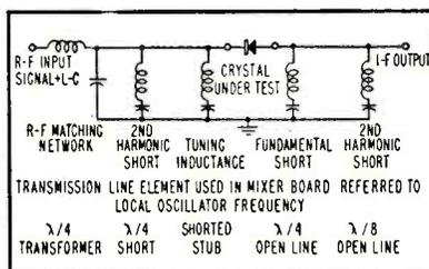
FIG. 2—Equivalent circuit of mixer test board
