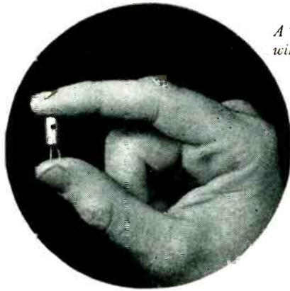
*A Transistor of point-contact type. Two hair-thin wires control current flow in germanium metal.*
