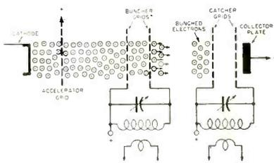
FIG. 7-36—Electrodes in a klystron tube (from Lytel—"UHF Practices and Principles")
