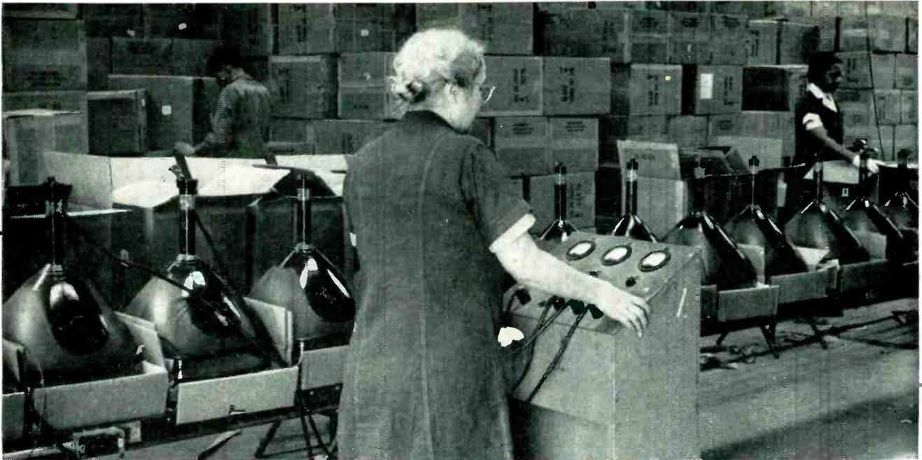
Gas-buggy test unit used at Electronics Park plant to check for gas in tube and leakage between elements, at rate of one tube per minute. Four tubes are connected at a time so that three are being preheated while the fourth is checked. Tubes are aged for several days in storage before this final checkup
