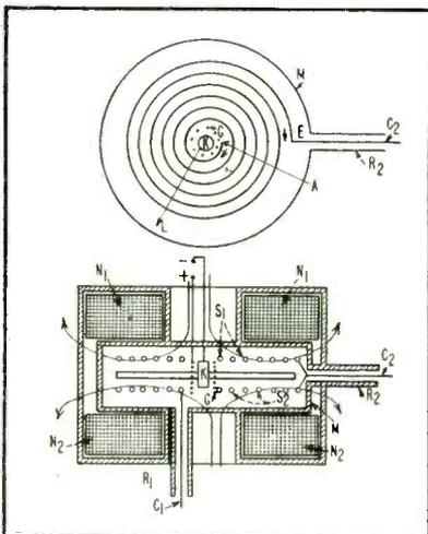
FIG. 4—Spiral traveling-wave tube elements
