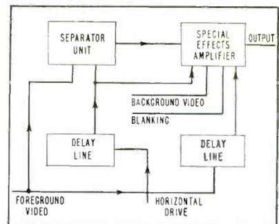
FIG. 2—Special interconnections, including delay cables, are used to insure proper register of composite video signal
