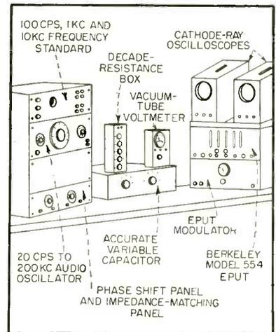
FIG. 2—Filter test station using new method
