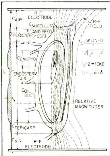
FIG. 1—Course of r-f lines of force longitudinally through a carrot seed
