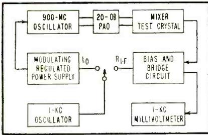
FIG. 6—Production test equipment arrangement
