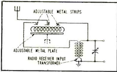
FIG. 3—Interference eliminator coupled to receiver input
