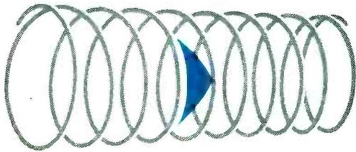
With the development of the original HELIPOT—the first multi-turn potentiometer—an entirely new principle of potentiometer design was introduced to the electronic industry. It made possible variable resistors combining high resolution and high precision in panel space no greater than that required for conventional single-turn potentiometers.
