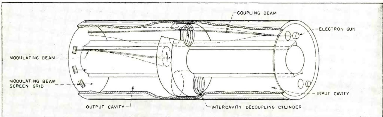
Electron coupler is 18 in. long by 5½ in. in diameter. Details shown in cutaway include the two coupling-beam electron guns and three of the five modulating beams. Coupling loops are not shown
