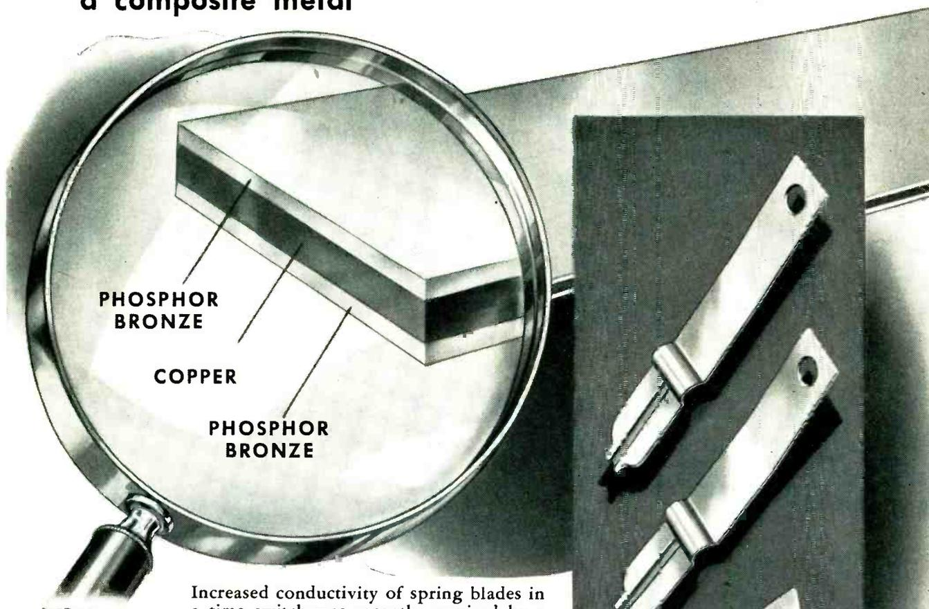
Increased conductivity of spring blades in a time switch was recently required by a manufacturer of demand meters. Operating requisites were high conductivity, excellent spring properties and small cross-sectional area.
