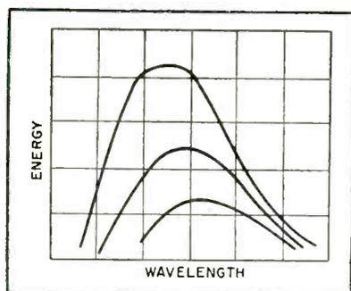
FIG. 1—Black-body radiation curves, showing variation of energy with wavelength. Energy increases with absolute temperature, and the peaks shift toward the shorter wavelengths
