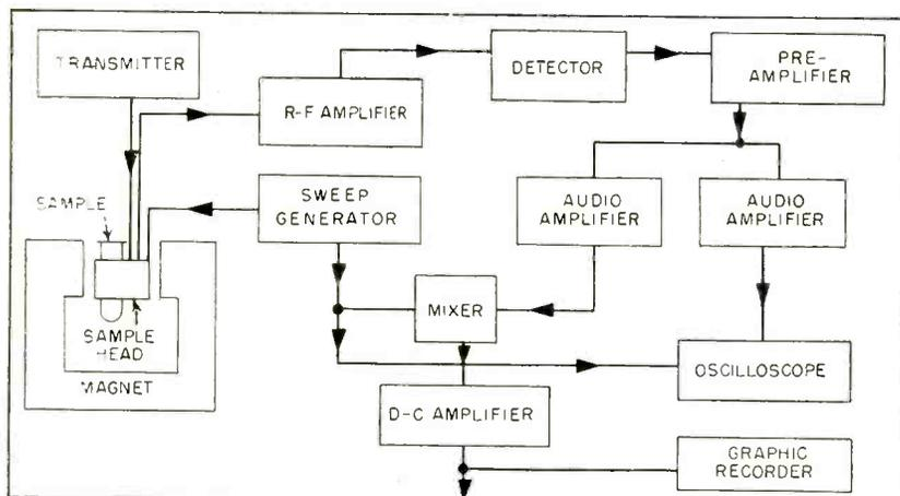
FIG. 1—Block diagram shows use of r-f transmitter, receiver and associated equipment
