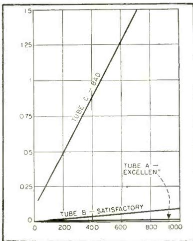
FIG. 2—Gas ratio for any given tube is a constant regardless of emission when gas current in  $\mu\text{a}$  is plotted vertically against cathode current in  $\mu\text{a}$
