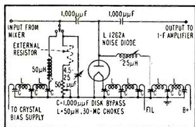
FIG. 4—Contents of Y-factor box used in noise temperature test
