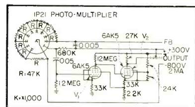
FIG. 8—Preamplifier and phototube circuits used in each pickup head. Miniature 6AK5 tubes operate in starved pentode circuit
