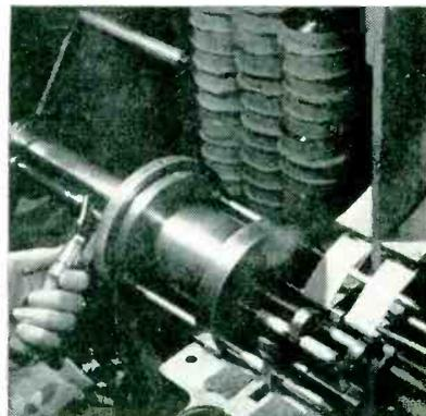
Left hand of operator is holding forked tool used to push out first half of split arbor preparatory to releasing finished units. Winding is already under way here on the next two units
