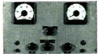
Front panel of semiautomatic gas ratio indicator
