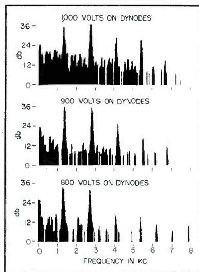
FIG. 10—Output spectra of 1P21 tube at various accelerating voltages indicate better signal-to-noise ratio at lower dynode voltages.
