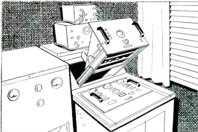
3 **Grant Industrial Slides** were used. With them, units may be withdrawn and locked in a fully extended position in a matter of *seconds*, with no more effort than opening a filing cabinet.
