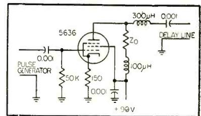
FIG. 4—Video amplifier circuit diagram
