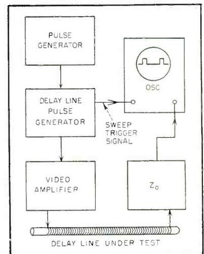
FIG. 3—Simplified block diagram of setup for testing distributed-constant lines
