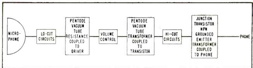
FIG. 1—Block diagram of tube-transistor hearing aid using two subminiature tubes and one npn junction transistor
