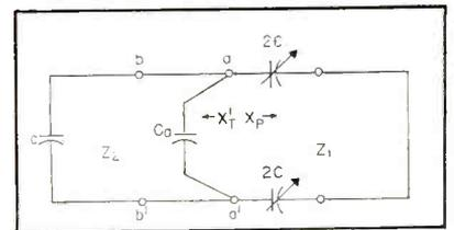
FIG. 5—Equivalent circuit for series-shunt capacitance tuning
