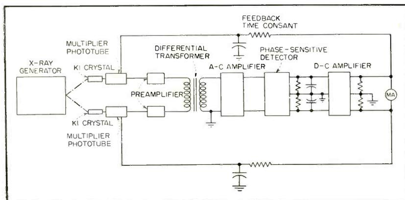
FIG. 1—Block diagram shows self-balancing bridge arrangement of differential x-ray gage whose output is independent of line voltage variations
