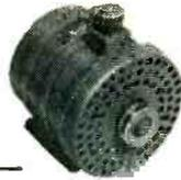
● REVERSIBLE DUAL SPEED D-C MOTOR — John Oster Type, DESTU-2-IR Western Electric #KS-15170-LOI. 26 volts @ 1.3/2.3 amps. 4500/10,000 rpm. @ 2 oz.-in. torque. 4" long x 2 1/4" diam. 3/16" shaft extends 3/8". Weighs 2 lb. SA-228 ..... \$8.75
