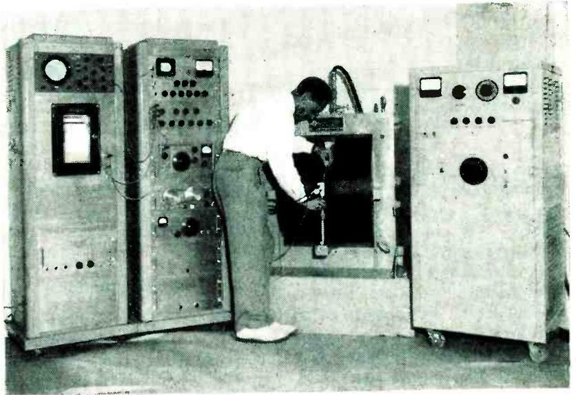
Sample of material being tested (usually liquid) is placed in test tube and inserted between jaws of large magnet where analysis process is accomplished
