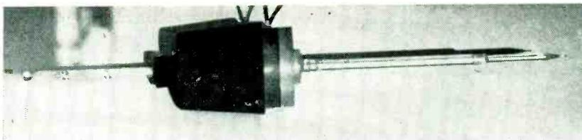
Immersion thermocouple comprises cold junction thermometer, cold-water chamber and hollow needle point containing hot junction, left to right
