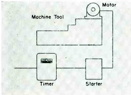
General Electric Electronic Timers assure precise timing of repetitive operations. One manufacturer reports the use of G-E timers on bearing grinding machines where they control cutting time and drift time. Here, G-E timers perform over 500 repetitive time cycles per hour. Where you require a uniform product turned out at high speed, put the accuracy of the General Electric Electronic Timer to work for you.
