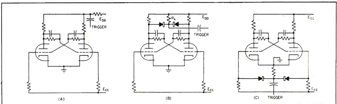
FIG. 6—Flip-flop with triggering network designed for large-amplitude negative pulses or steps (A); for smaller negative pulses (B); and for still smaller negative pulses of short duration (C)
