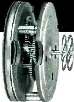
Rotor unit of H-3 motor
