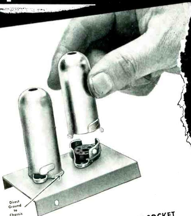
Recent addition to METHODE line of TUBE SOCKET ACCESSORIES is this new "Twist-On" type of tube shield and base, mounted in combination with molded sockets, as illustrated. Projecting lugs on shields provide direct ground to chassis under screw pressure and a reliable shock and vibration proof mount.
