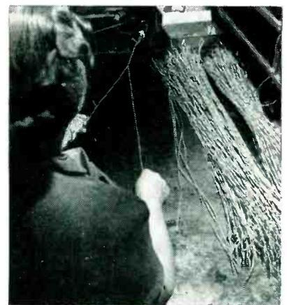
Method of using air gun to twist filament leads together after they have been cut and stripped on an Artos machine
