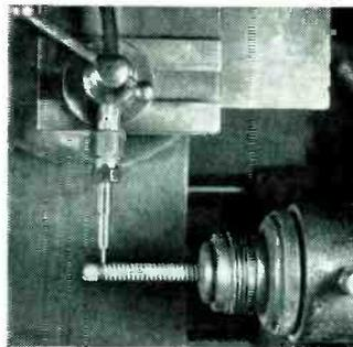
Automatic set-up on a lathe for cutting spiral bands on a deposited carbon resistor.
