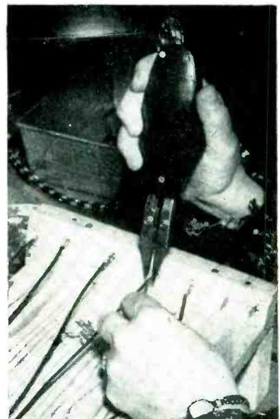
Using soldering tweezers to get heat exactly where it is needed on a joint
