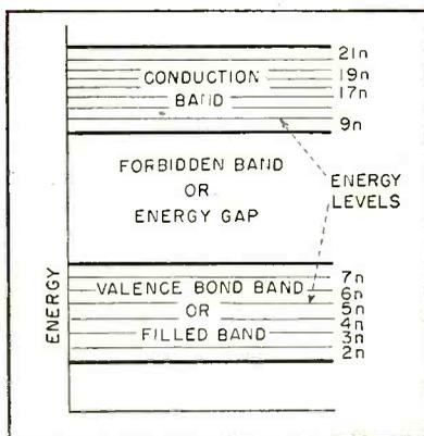
FIG. 2—Energy of a quantized particle, such as an electron. Only the ordinate is to scale. Figure shows how energy, according to quantum mechanics, can change in discrete amounts only, and often in large jumps
