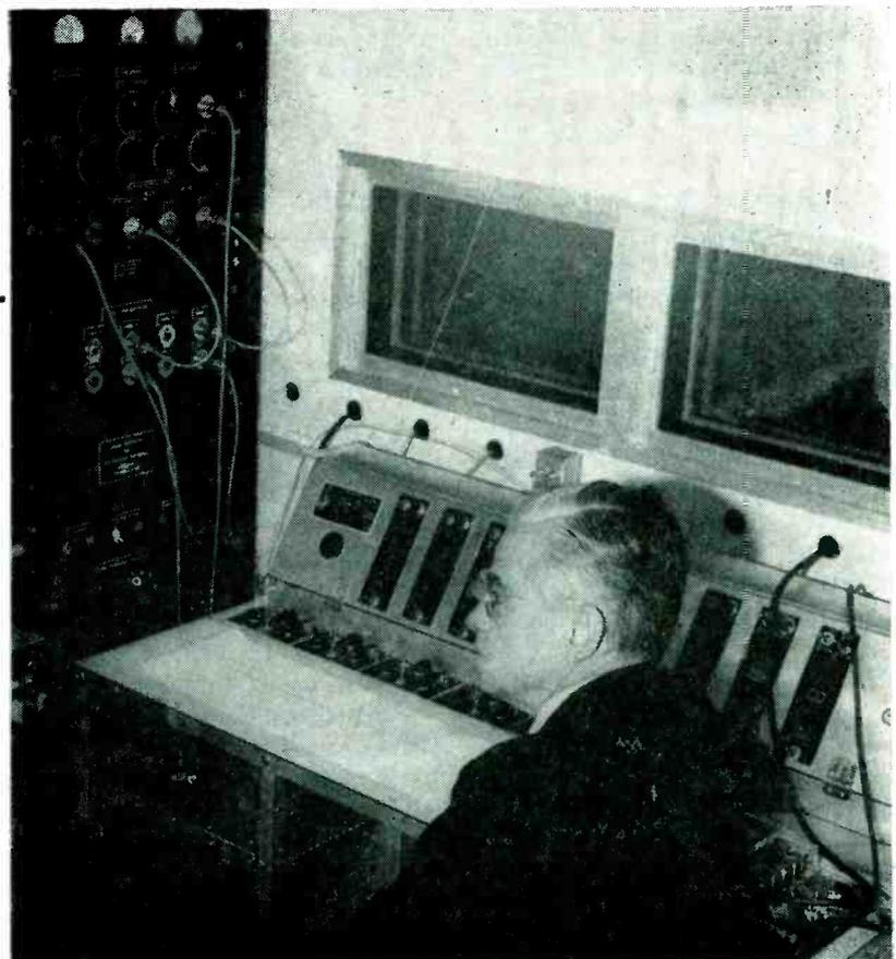
Bioelectric integrator outside shielded room quantifies potentials taken from subject. Electroencephalograph at right makes continuous paper tracing
