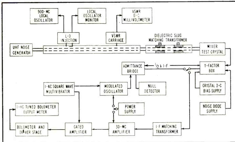
FIG. 1—Measuring equipment for uhf germanium mixer crystals is used in the laboratory to obtain parameters
