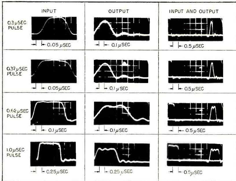
FIG. 6—Pulse response of 5,600-ohm line wound with No. 44 wire
