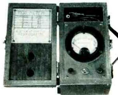
Compact test meter for audio signal level and recorder bias. A 100  $\mu$ a movement is used
