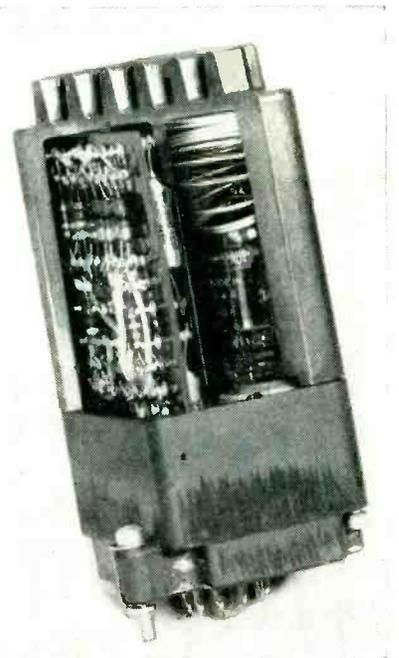
FIG. 1—Navy Electronics Laboratory packaged replacement unit with section cut away to show placement of components
