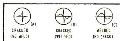
FIG. 9—Typical patterns for (A) cracked, (B) cracked and welded, (C) welded metal
