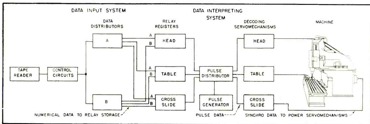
FIG. 1—Tape reader and digital-to-analog converter supply synchro data to power servomechanisms. Orthogonal motions of table, head and cross slide can produce any desired cut
