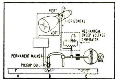
FIG. 8—Induced-voltage flaw detector
