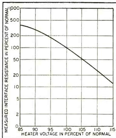
FIG. 1—Measured values of cathode interface resistance plotted as a function of heater voltage
