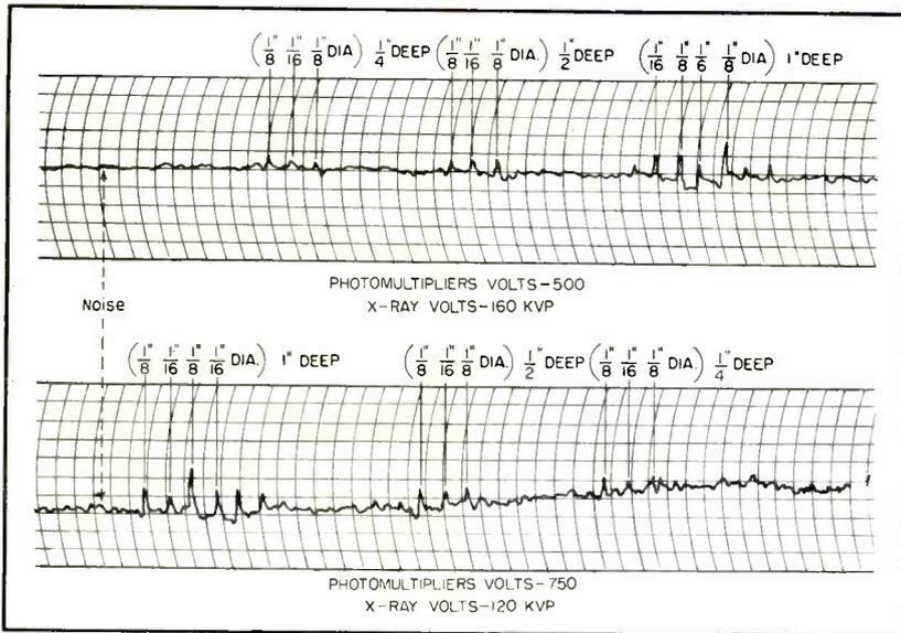
FIG. 6—Typical projectile test record with pulses corresponding to varied depths in filler. Reducing phototube voltage improves signal-to-noise ratio
