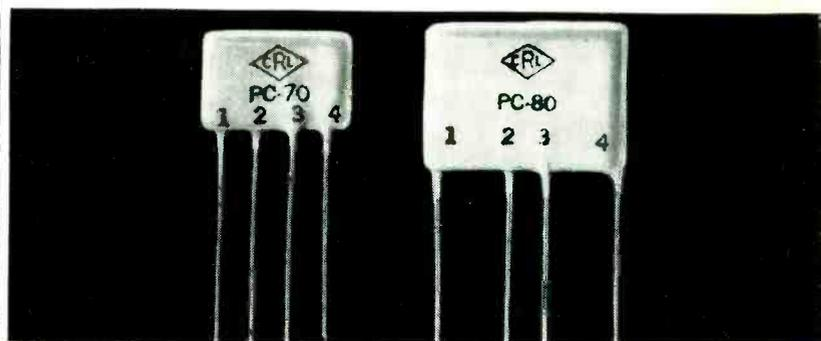
**CENTRALAB TRIODE COUPLATES** replace 5 components normally used in audio circuits. Triode Couplates are complete assemblies of 3 capacitors and 2 resistors bonded to a dielectric ceramic plate. Available in a variety of resistor and capacitor values. Technical Bulletin 42-127.
