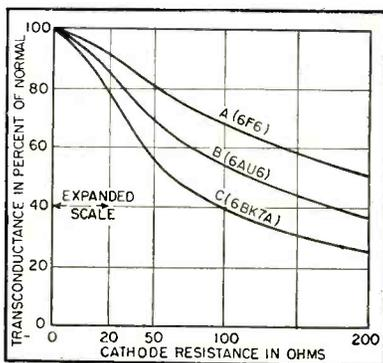
FIG. 2—Loss of transconductance with increasing cathode resistance illustrates effect of cathode interface. Curve A shows low- $\mu$ , low  $g_m$  6F6, triode connected; B shows medium- $\mu$  medium  $g_m$  6AU6, triode connected; and C, high- $\mu$ , high- $g_m$  6BK7A
