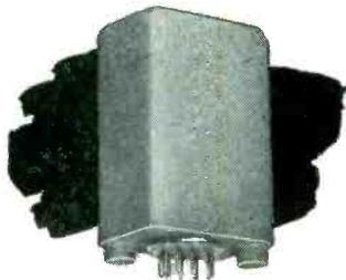
**R 94 SERIES**—Hermetically sealed small telephone type relay with pin hinge construction for long life. Available in D.C. only with contact springs up to 4 pole double-throw. In 1 amp., 3 amp., or 5 amp. capacity. Plug-in or solder terminals. Overall size 1-5/8 x 1-1/32 x 2-1/4 D.
