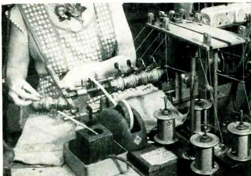
Winding flyback coils in multiples of four on keyed mandrel. Dereelers are on tops of wire spools at lower right. Tape for anchoring leads is in heavy dispenser, with end of tape anchored over tailstock so pieces can be cut easily with scissors that are always in operator's right hand. While winding is in progress, operator cuts the adhesive tape into strips and sticks them on her left hand, ready for instant use
