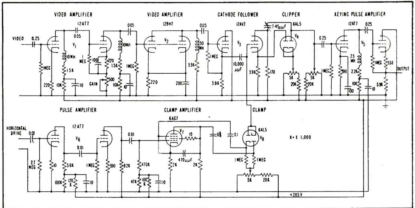
FIG. 3—Circuit diagram of the NBC keying separator amplifier
