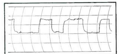
FIG. 5—Output of absorption gauge for 0.002-inch change in 0.5-inch steel equivalent, obtained with 180-kvp x-rays, 4-ma beam current
