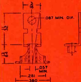
**HERMETIC** has designed a complete series of hermetic seals with attached lugs as an associated line of the self-lug tubing seals. This series is characterized by innovations of particular interest to design engineers:
