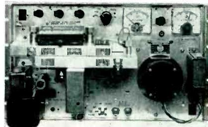
In this equipment the meter in conjunction with a germanium diode suitably coupled, monitors the r-f output and serves as a tuning indicator. The low limit contact is set at some predetermined scale point. If the power fails the CMR contacts close circuits sending alarms or energizing standby equipment.
