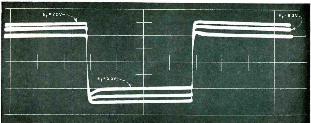
FIG. 3—Plate-voltage waveform for 6AH6 with 50-kc square-wave excitation. Overshoots due to cathode interface resistance are noted as heater voltage is reduced
