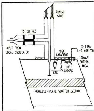
FIG. 3—Local oscillator injection and monitor probes
