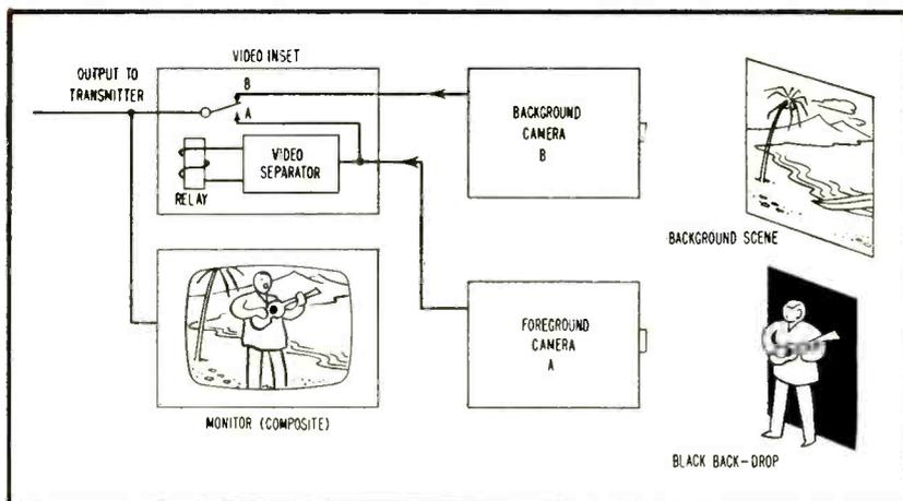
FIG. 1—Elements of the video inset system show a simplified camera relay
