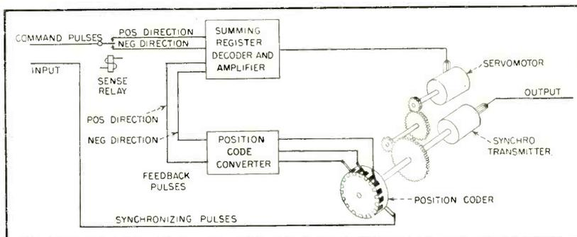
FIG. 3—Digital-to-analog converter changes input pulse data to equivalent shaft rotation. Commutator-type coder wheel generates feedback pulses for checking
