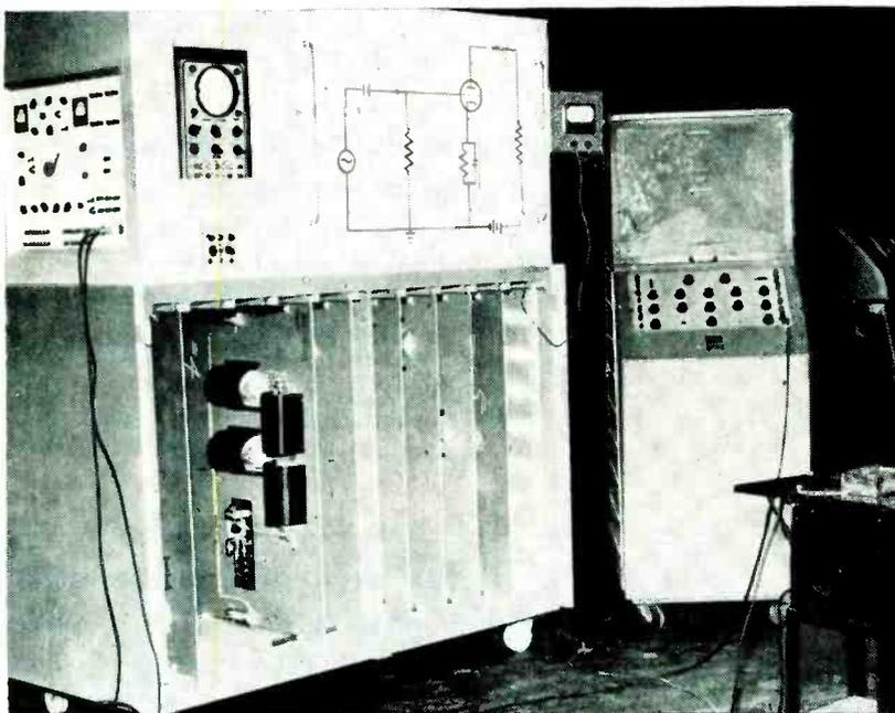
FIG. 1—Classroom demonstration board allows nine different circuits to be demonstrated to a large group. Projection oscilloscope at right makes it possible to show what is happening at various points in the circuit
