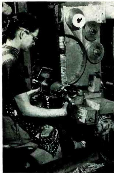
Tandem high-speed machine for winding paper capacitors two at a time. Operation is almost completely automatic.
