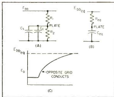
FIG. 4—Effect of coupling capacitor on switch-over
