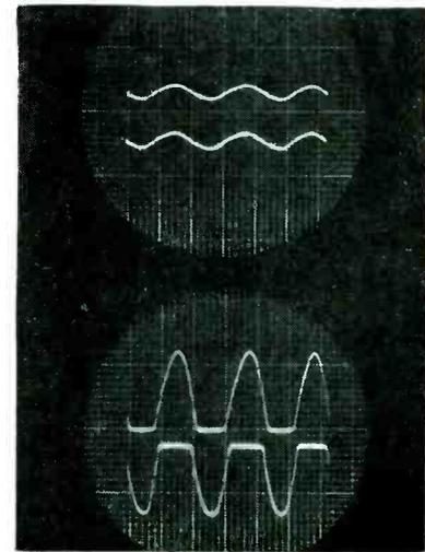
Circuit (top) and output waveforms for pnp-npn transistor amplifier
