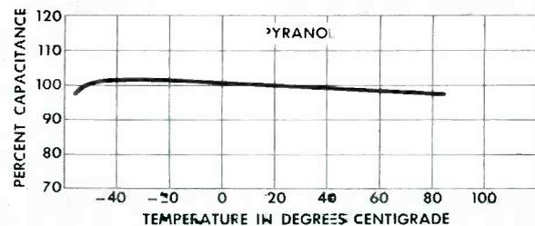
Capacitance vs. Temperature is shown by this typical curve. G-E Pyranol subminiature metal-clad capacitors have only a small capacitance change through the entire range from  $-55^{\circ}\text{C}$  to  $+85^{\circ}\text{C}$ .
