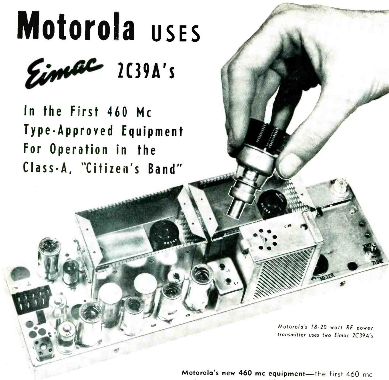
*Motorola's 18-20 watt RF power transmitter uses two Eimac 2C39A's*
