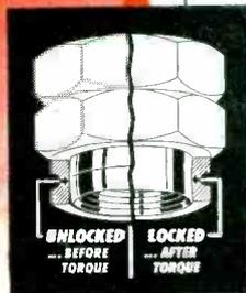
Reasons are many why Klincher is getting first call on more and more of the really tough fastening jobs in the Electronics industry. For instance, on critically vital thermocouples Klincher Locknut permits use of desired torques without causing stud failure or unnecessary wear of stud threads.
