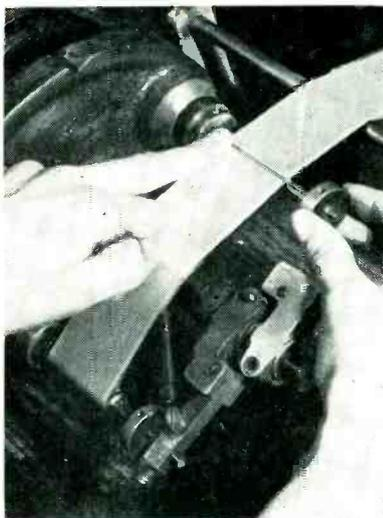
Inserting arbor pin to lock start of next winding after indexing head to bring newly-finished capacitor forward
