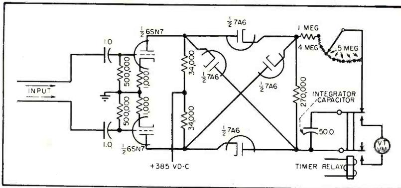
FIG. 2—Schematic shows one channel of four-channel bioelectric integrator. Additional R-C amplifier may be switched in when dealing with low potentials
