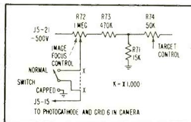
FIG. 1—Effective lens capping for a camera in the TK-10A chain is accomplished by insertion of a toggle switch as shown
