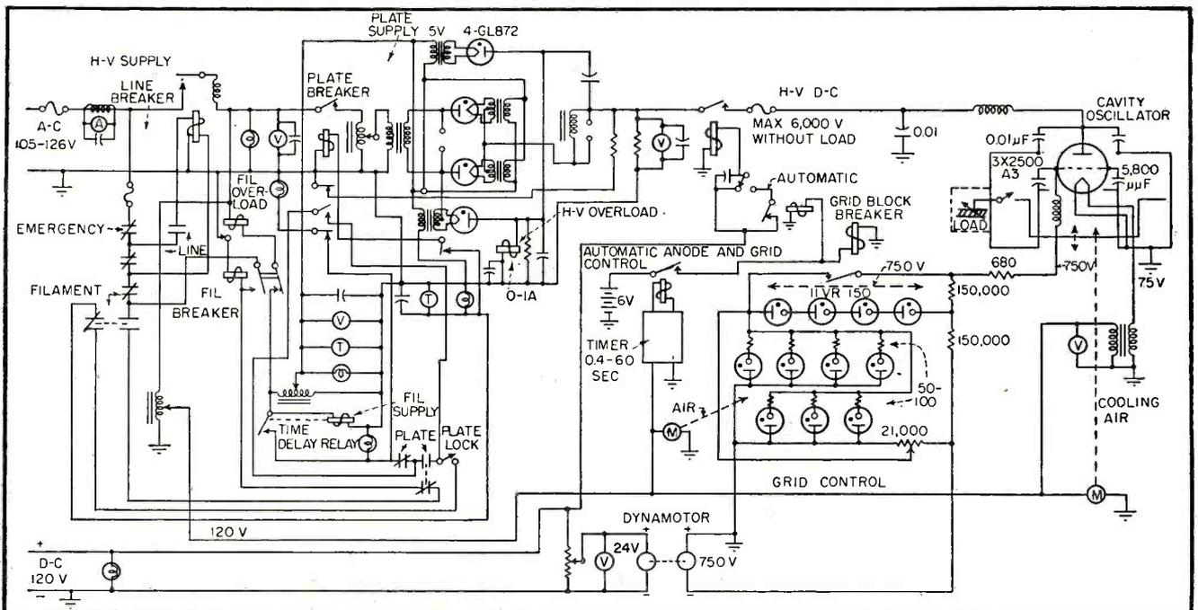
Circuit diagram of the radiation equipment includes timer for accurate dosage and safety controls for nontechnical personnel
