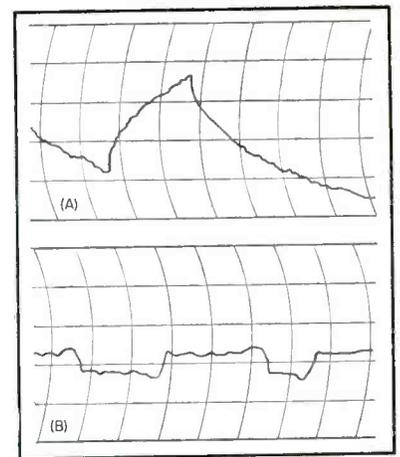
FIG. 3—Pulses with regeneration (A) and negative feedback (B)
