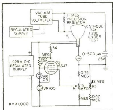
FIG. 3—Production-type gas ratio test
