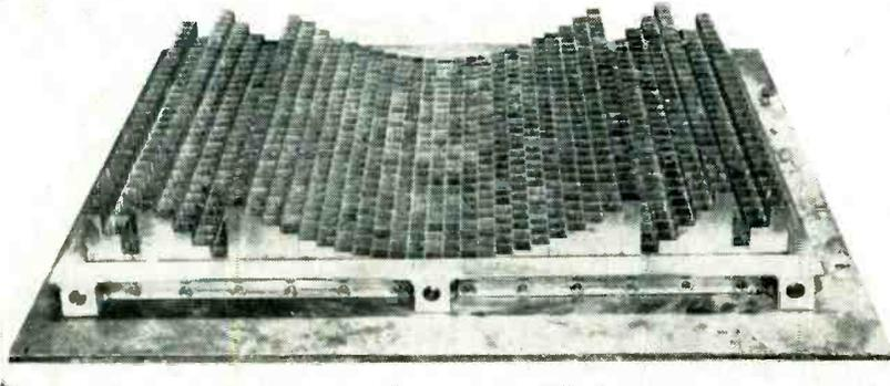
Experimental radar lens made of square Monel tubing, as it appeared after furnace brazing and removal of solder
