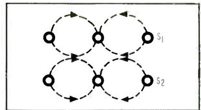
FIG. 5—Radial electric field between successive turns of same spiral
