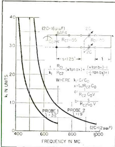
FIG. 3—Variation of  $k_1$  with frequency for grid-dip meter using series tuning
