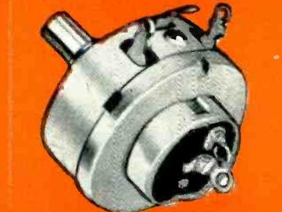
TYPE GC-45, 15/16" diameter variable composition resistor. Wattage rating: 1/2 watt for resistances through 10,000 ohms, 1/3 watt for resistances over 10,000 ohms through 100,000 ohms, 1/4 watt with 500 volts maximum across end terminals for resistances over 100,000 ohms. Available with or without illustrated attached switch and in concentric shaft tandem construction C2-45 as shown above.
