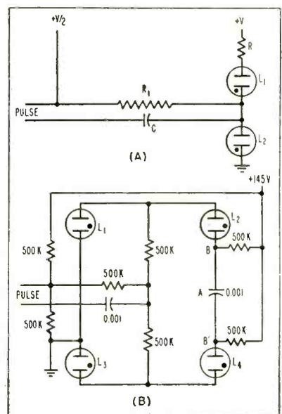
FIG. 1—Basic circuit (A) used in flip-flop and binary counter. Flip-flop (B) uses NE-2 neon lamps
