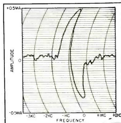
FIG. 4—Record of blip showing abundance of oxygen 17 in water. Nuclear resonance is at point where curve crosses centerline
