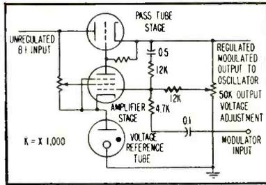
FIG. 7—Small-percentage modulation circuit
