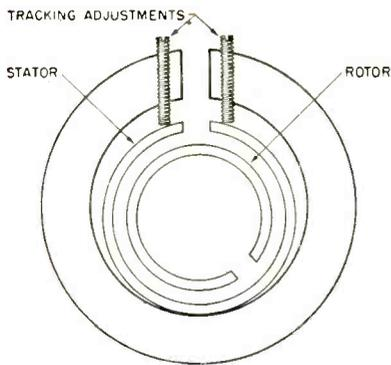
FIG. 8-14—Side view of cylindrical tuner (from Lytel—"UHF Practices and Principles")
