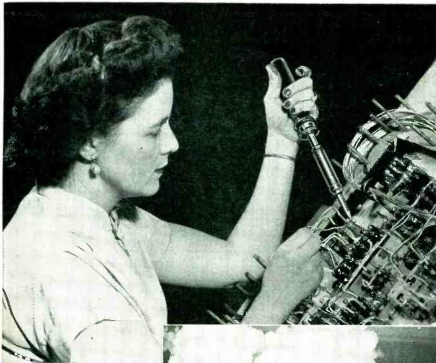
At the Glenn L. Martin Co., Baltimore, Md., American Beauty Soldering Irons are used to fasten parts to an overhead switch control panel for the pilot's compartment of Martin 4-0-4 twin-engine commercial transports.
