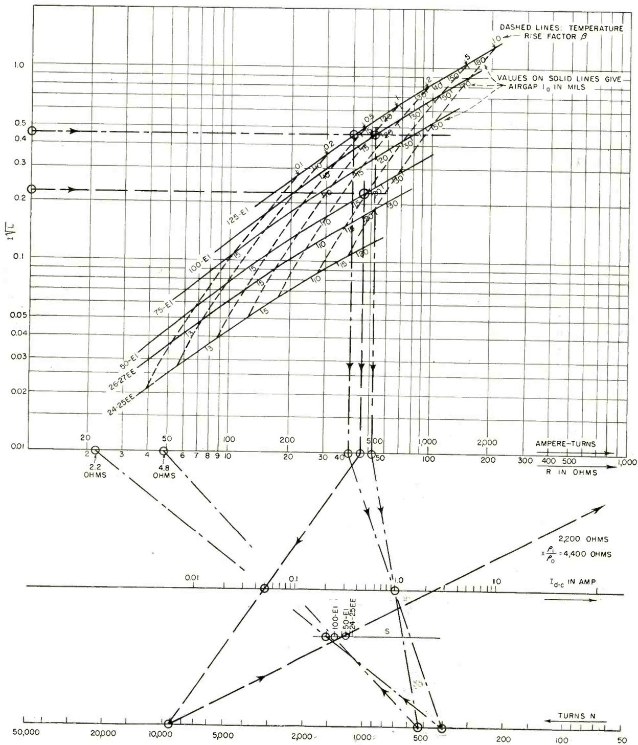
FIG. 3—Calculation chart for chokes using 7-mil laminations of 4-percent silicon steel with square stack. Dash-dotted lines show solution worked out for Example 1, and long dashed lines apply to Example 2
