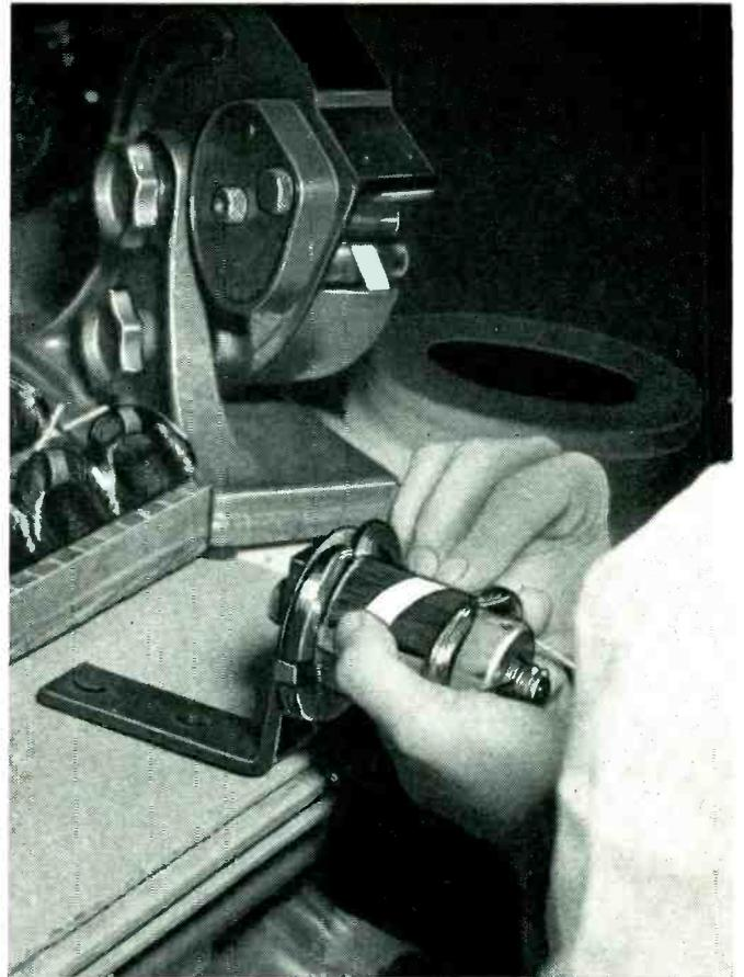
**TOUGHNESS AND CONFORMABILITY** of "Scotch" Yellow Crepe Paper Tape No. 38 with Thermo-setting Adhesive means dependable, compact TV deflection coils.
