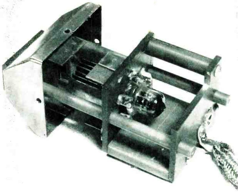
Final version uses 6F4. Tube and circuits are mounted on movable carriage
