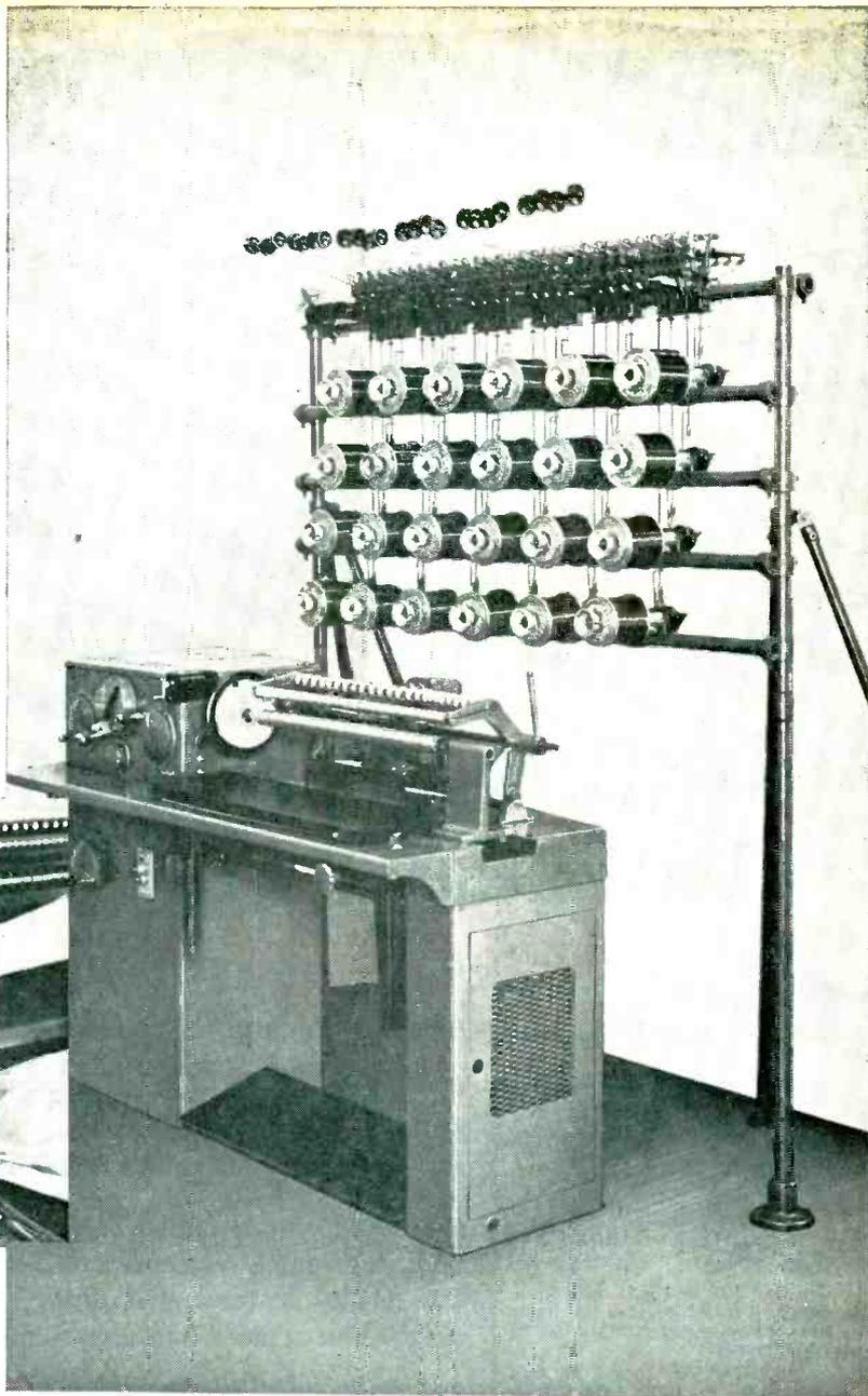
*Leesona® No. 108 Coil Winder for high accuracy, top production and lowest costs in shops where change-overs are frequent. Takes long or short runs; easy to set up; no cams or gears to remove when making set-up changes; all controls are within easy reach of the operator even when seated.*
