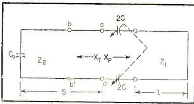
FIG. 2—Equivalent circuit for series capacitance tuning
