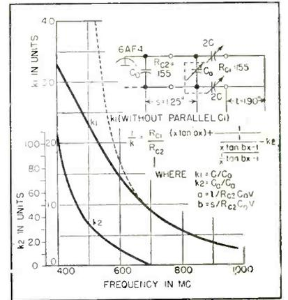
FIG. 6—Variations of  $k_1$  with frequency for grid-dip meter using shunt and series tuning
