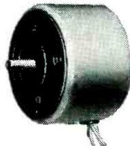
Type F4H92H-1CC **400 CYCLE—RING MOUNTED** Propeller Fan. 115 volt, 400 cycle, 130 C.F.M. at .5" S.P., single phase.
