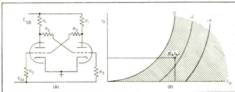
FIG. 2—Rudimentary circuit for steady-state design (A) and tube characteristic (B) showing operating point
