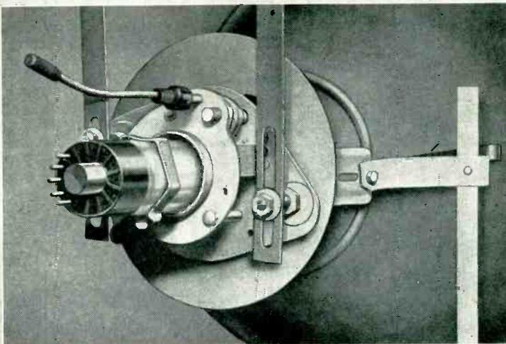
● The external ion-trap magnet on this standard tube, is an extra cost item for the TV manufacturer and requires special adjustment. The focus coil and complicated mounting also mean extra cost. They take up space, add weight, consume assembly and adjustment time. Get rid of all three parts with G. E.'s new *i-m-f* tube!
