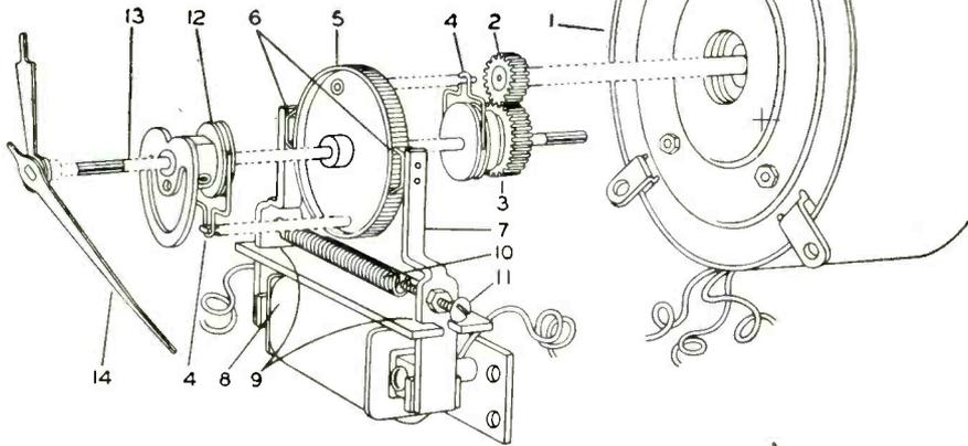
**Formula S-1: Expensive high torque, ball bearing motor, low inertia of moving parts, high proportion of precision and ground parts, no thrust bearings as found in ordinary clutches.**
