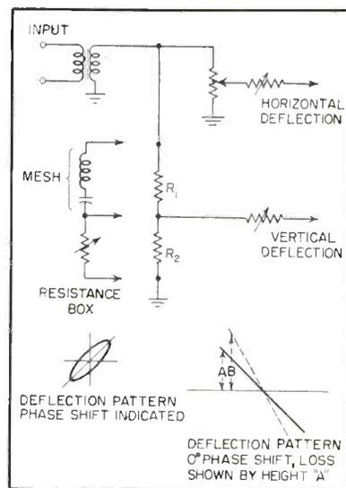
FIG. 4—Method of using resistance decade box to determine effective a-c resistance of a mesh
