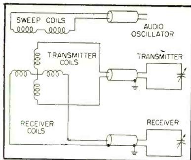
FIG. 2—Probe contains three sets of coils
