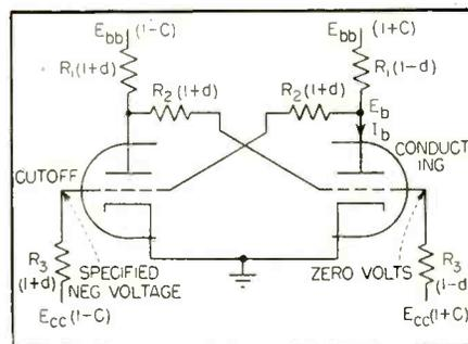
FIG. 3—Circuit showing conditions under which d-c stability is most difficult
