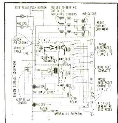
FIG. 1—Well-logging system uses combination of a-c and ground potential
