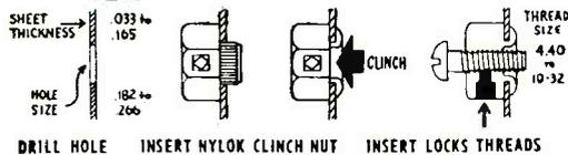
No fastening problem with NYLOK Self-Locking Clinch Nuts. Simply press in nut... clinch, insert screw and run it down. Resilient nylon insert assures positive lock. Assemble either end, speed up assembly. No damage to nut in removing. Can be used again and again, with no loss of locking feature. Available in steel and aluminum, standard sizes # 4 to # 10, or others to specifications. Write for complete information today.
