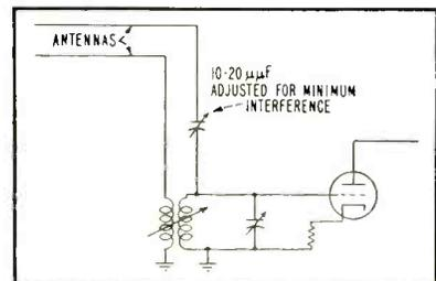
FIG. 7—Simple system claimed to eliminate static and interference
