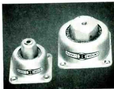
The new Type 7630 and Type 7640 ALL-METL Barrymounts have been specifically designed to eliminate loss of efficiency due to damper packing. Previous wire-mesh unit vibration isolators exhibited a definite loss of damping efficiency after a period in actual service, because the wire-mesh damper tended to pack. These new unit Barrymounts have eliminated this difficulty, because load-bearing spring returns damper to normal position on every cycle.
