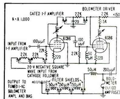
FIG. 5—Measurement of relative output noise power is obtained with this circuit
