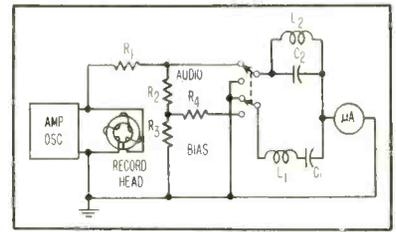
FIG. 1—Circuit of bias and audio level meter shown connected to the recorder head
