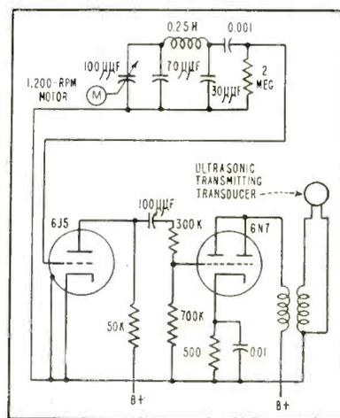
FIG. 1—Diagram of ultrasonic oscillator used in tire inspection unit
