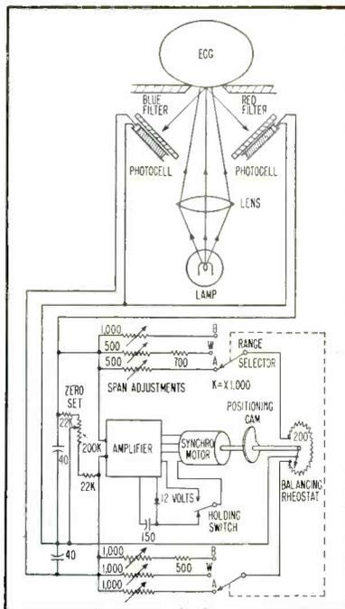
FIG. 1—Shell-color determinator utilizes light reflected from egg shell through red and blue filters to photocells
