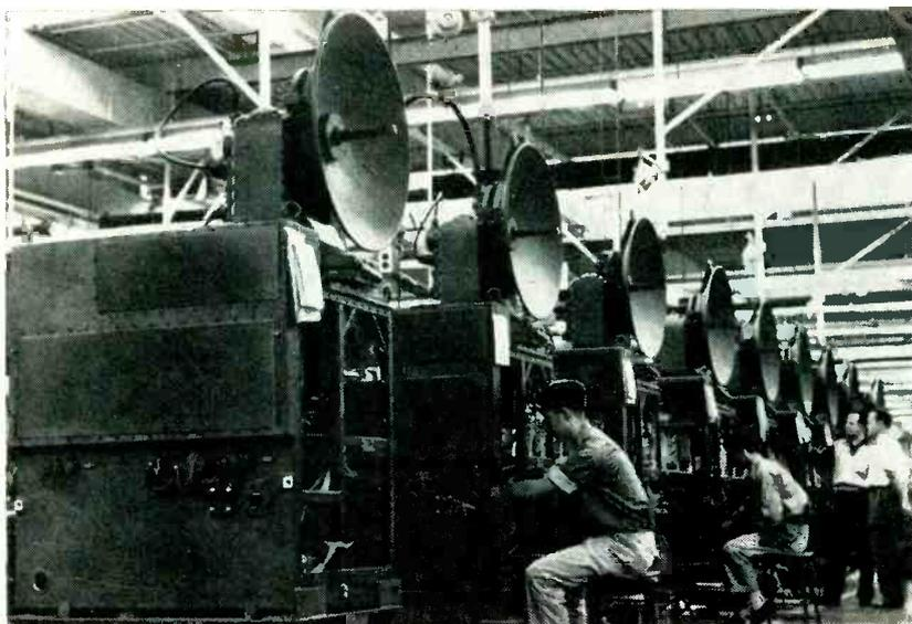
Production lineup of radar trackers for the Skysweeper
