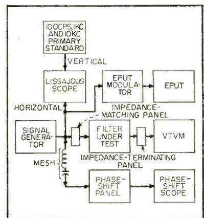
FIG. 3—Block diagram illustrating new method employing an Eput (events-per-unit-time) meter to indicate frequency
