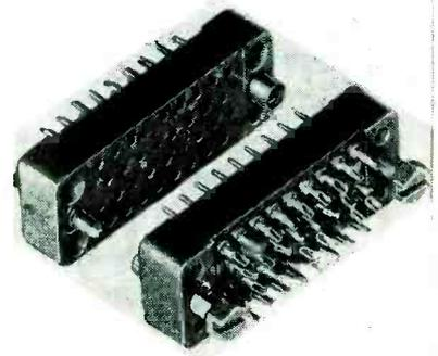
**Connector Guide Pin and Socket**
