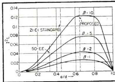
FIG. 2.—Curves for silicon steel, showing that optimum core shape is obtained at a dimension ratio  $a/d$  of about 0.65
