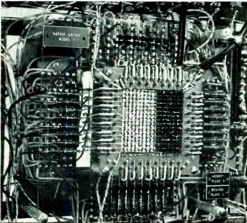
An experimental coincident-current memory containing two 15-by-16 arrays. This unit is driven by a magnetic matrix switch
