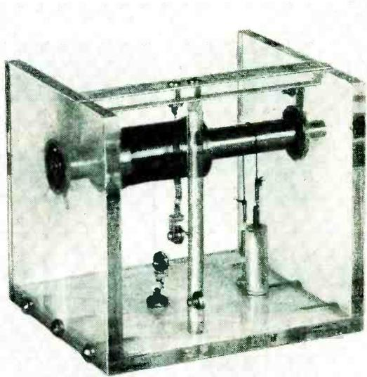
Constant tension wire feeder permits use of wire as small as No. 48 in delay lines
