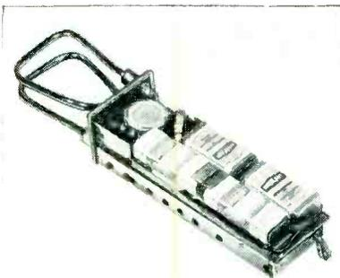
This 25-milliwatt f-m transmitter was designed by Motorola engineers to extend the range of the microphone used with a loudspeaker system in railroad yards. It operates in the 152-to-174 mc band, produces a 15-kc deviation and measures approximately 2 x 3 x 7 inches
