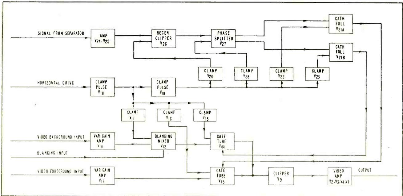
FIG. 4—Block diagram of the special effects amplifier showing tube designations is explained in text with reference to Fig. 5
