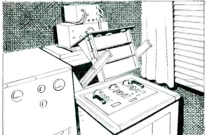
4 **A full 90° tilt** brings the wiring under the chassis into full view for repair. Unit locks at this and other angles, and may continue to operate in any of these positions.
