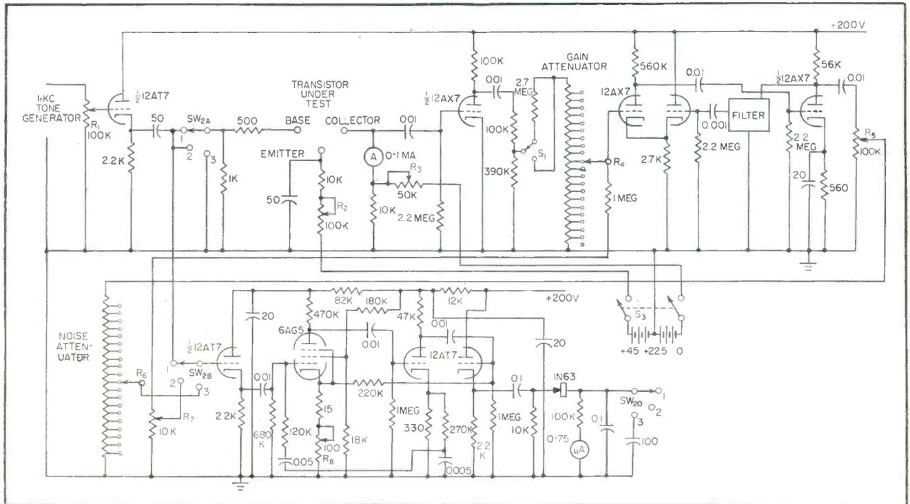
FIG. 4—Complete schematic of noise analyzer
