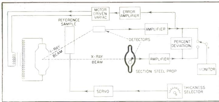
FIG. 2—Block diagram shows arrangement of system components for comparison measurements
