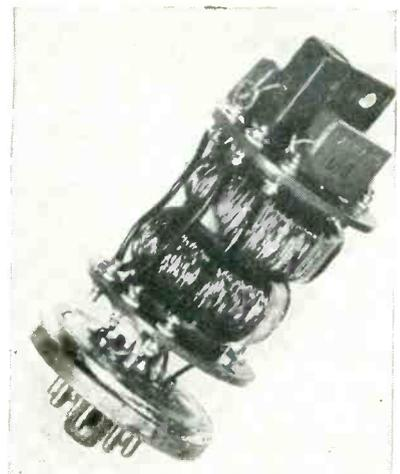
Complete oscillator assembly showing placement of toroids under investigation
