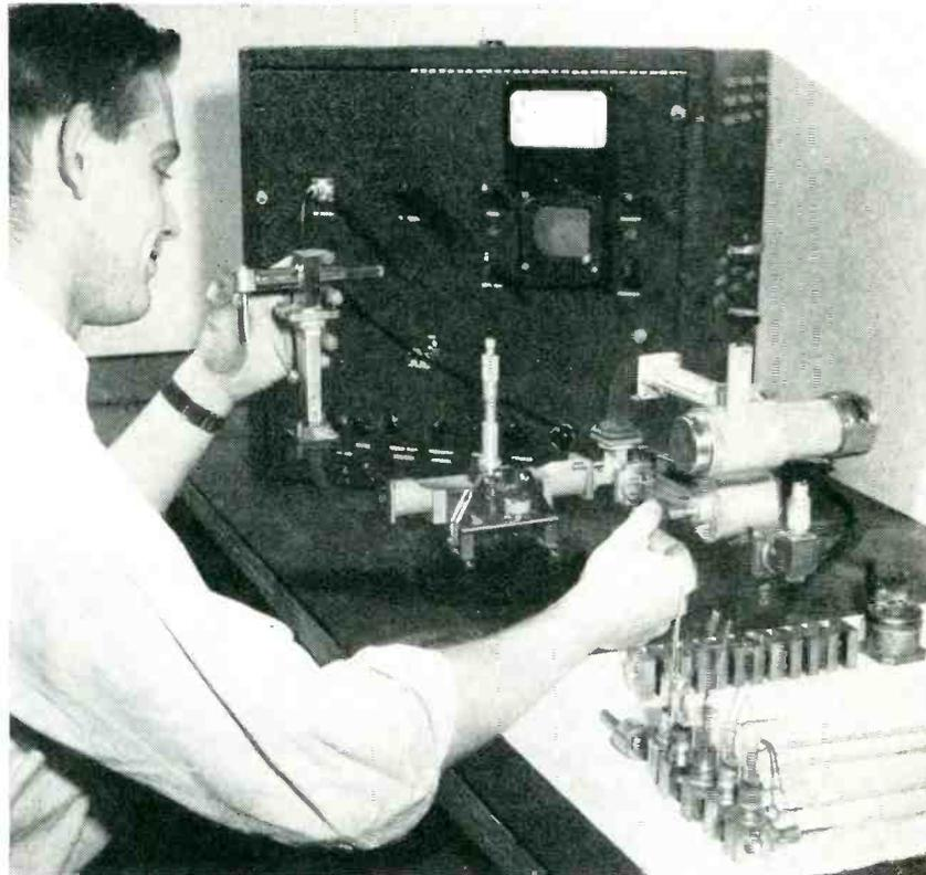
Production setup for cold-testing anode blocks of type 2J55 magnetrons. Blocks for 2J48 and 4J52 tubes are on bench also, awaiting test. Cabinet contains klystron power supply and oscilloscope circuits. Operator is adjusting klystron oscillator with right hand
