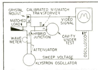
FIG. 1—Setup for testing microwave cavity resonators before assembly in magnetrons
