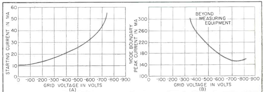
FIG. 3—Oscillator starting current and mode-boundary current versus magnetron grid voltage
