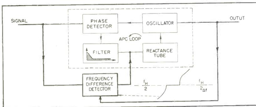
FIG. 8—More elaborate circuit adds frequency difference detector to Fig. 7, improves pull-in time after interruption to about 0.1 second
