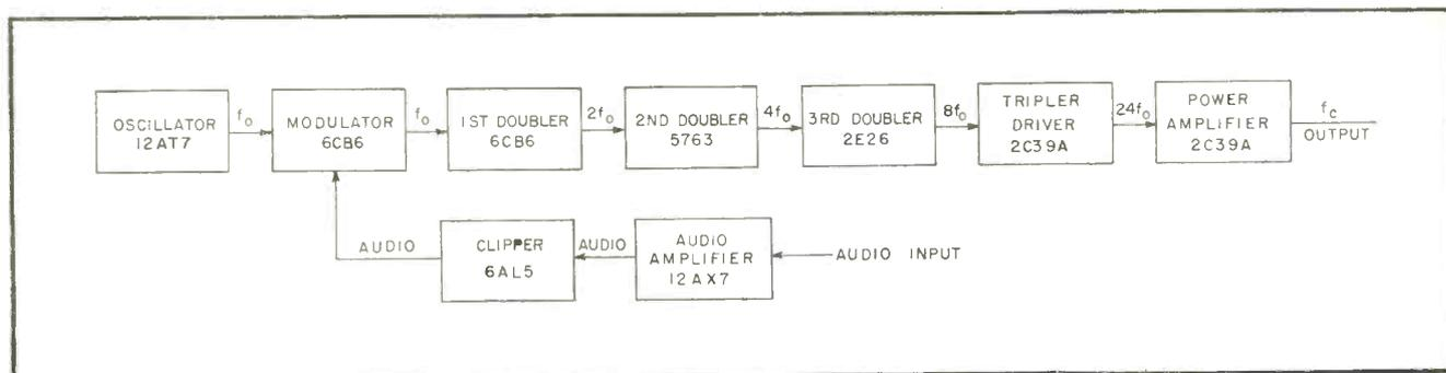
A simplified block diagram of the 450 to 470-mc transmitter
