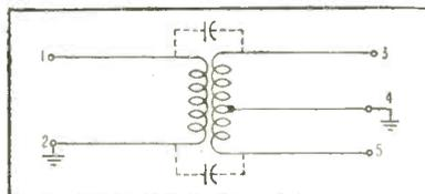
FIG. 1—Coupling circuit showing effective primary-to-secondary capacitance
