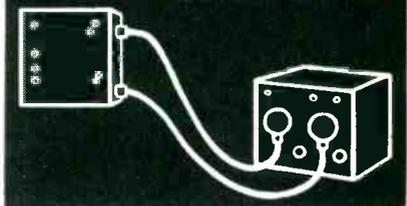
If you have to control a piece of equipment from a remote point, an S.S.White flexible shaft is the simple, low-cost way to do it. The shaft can be run along any desired path, can be installed with a minimum of difficulty, requires no alignment or adjustment. In fact, no other mechanical control set-up offers the same economy and ease of application.
