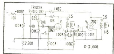
FIG. 3—Trigger circuit with time delay energizes circuit of Fig. 2
