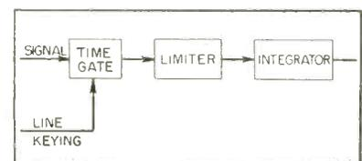
FIG. 5—Meeting phase error specification of five degrees is done by basic arrangement shown above
