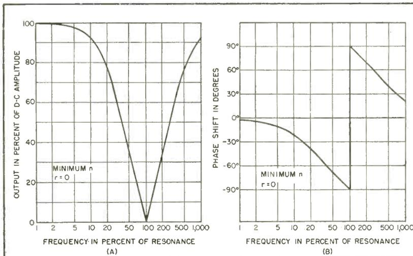
FIG. 3—Amplitude and phase response for infinite-notch, minimum-width, parallel-T network
