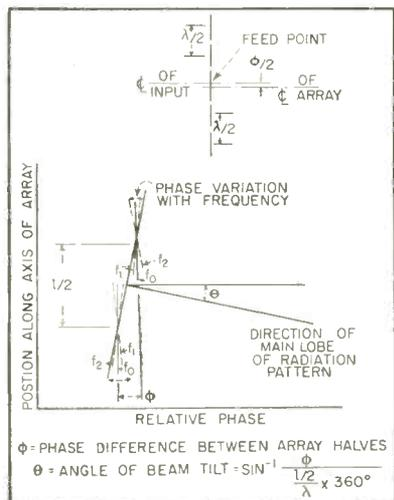
FIG. 4—Relation of beam tilt to displacement of feedpoint from center
