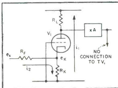
FIG. 3—Circuit in which feedback and cathode current subtract
