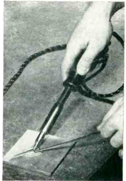
Demonstration showing ease of soldering directly to aluminum sheet having a chemically deposited nickel coating
