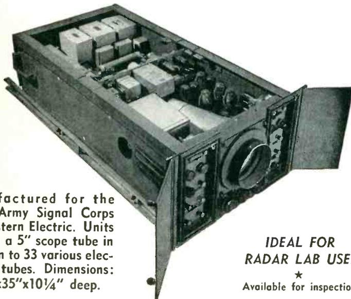
Manufactured for the U. S. Army Signal Corps by Western Electric. Units contain a 5" scope tube in addition to 33 various electronics tubes. Dimensions: 17 1/4" x 35" x 10 1/4" deep.
