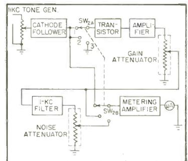
FIG. 3—Direct-reading noise analyzer
