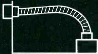
A single S.S.White flexible shaft will bring control to any point regardless of intervening obstacles or distance. Its basic simplicity, adaptability and ease of installation insures lower costs by eliminating unnecessary control parts and by making it easier to meet wiring, servicing and space requirements.
