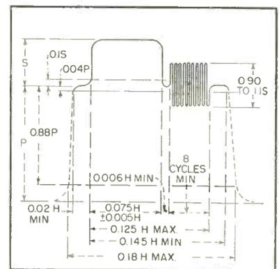
FIG. 4—Simultaneous compatible system employs as color sync signal a burst of sine wave at subcarrier frequency, imposed on each horizontal sync pulse
