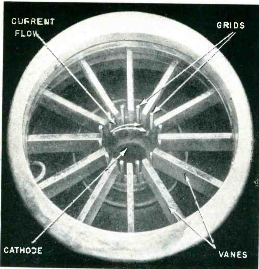
Top view of tube's anode section shows placement of vanes and grids; also tangential beam-current flow near vane tips
