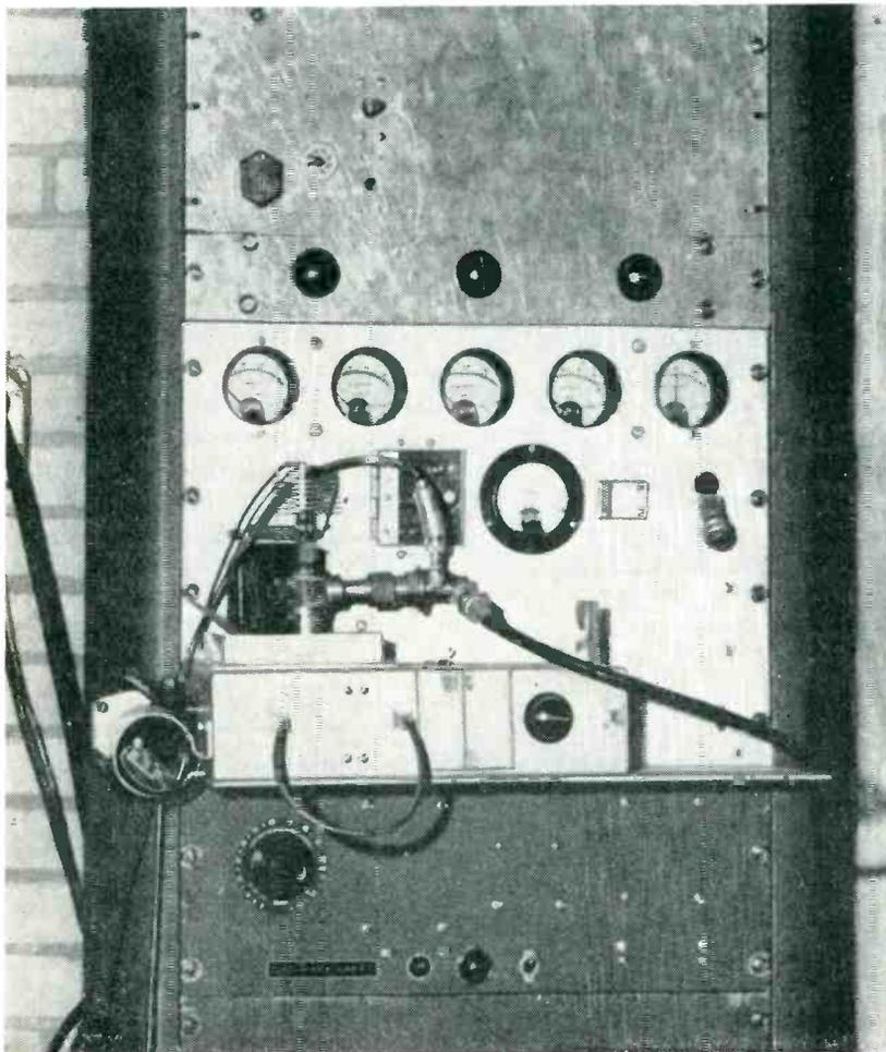
Video-modulated grid magnetron used in experimental television relay
