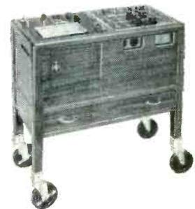
One channel Model 128/141 above and two-channel Model 60 at right both incorporate Sanborn recording advantages which include interchangeability of amplifiers and (with Model 60) preamplifiers.
