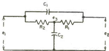
Capacitor-Shunt Bridged-T Network
