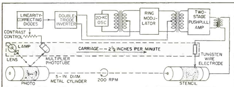
FIG 1—Operating principle of electronic stencil-cutter capable of transferring photos to stencils, with 500-line resolution of detail
