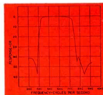
This band pass filter is designed for sharp cut-off at both ends of the range... 10,000 ohms... case dimensions 1 5/8" x 2 1/2" x 3 1/4".
