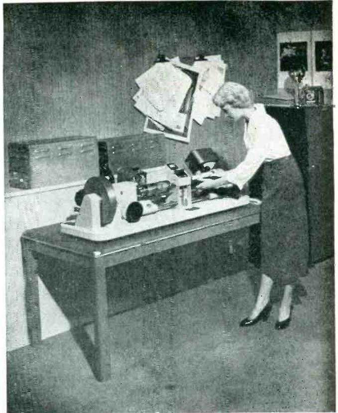
Tabletop model of photoelectric engraver, known as Fairchild Scan-a-graver Cadet, produces 85-screen four-column halftone in 24 minutes after photo is loaded as shown. Amplifiers and tone-correcting circuits are in separate housing on shelf at rear
