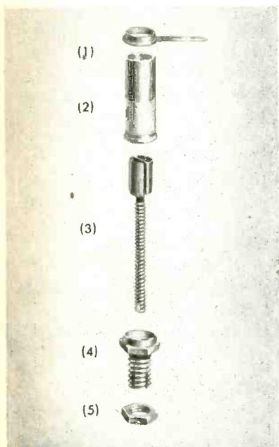
Exploded view of the CST-50 capacitor shows: (1) ring terminal with two soldering spaces; (2) metallized ceramic form; (3) spring-type S-shaped tuning sleeve\*; (4) split mounting stud; (5) locking nut.
