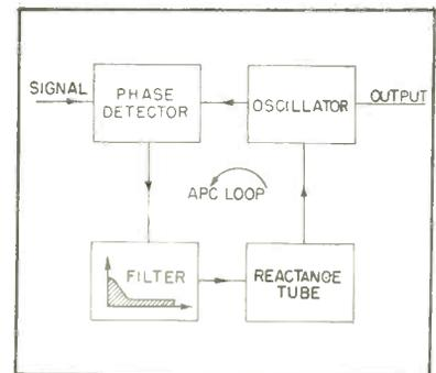
FIG. 7—Automatic phase control compares burst signal with oscillator
