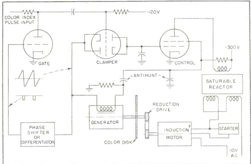
FIG. 1—Color synchronization in the field sequential system commonly employs a filter disk driven at 1,440 rpm. Disk is 23 inches in diameter and may weigh several pounds
