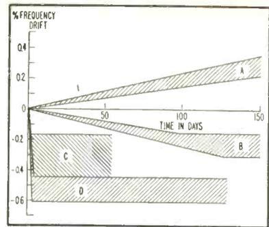
FIG. 1—Frequency drift in oscillators with powdered core toroids that have been (A) open and undried, (B) Vacuum dried and (C) (D) heat dried. Oscillators in (D) had lower frequency range than those in (C)
