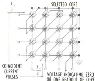
4-BY-4 COINCIDENT-CURRENT MEMORY ARRAY SHOWING PATH OF PULSE STORED IN SELECTED TOROID
