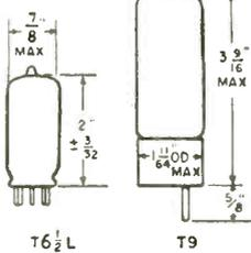
Maximum Wattage Dissipation: T6 1/2 L—5W. T9—10W.
