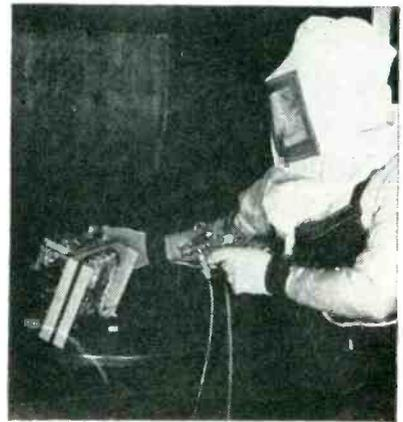
Example of application requiring masking of certain regions during spraying for tropicalizing. The electronic unit here is a Philco-built radar set, being given a special varnish to inhibit moisture absorption and fungus growth in tropical climates
