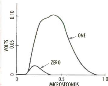
CHART SHOWS VOLTAGES OBSERVED READING ONE OR ZERO FROM A SELECTED TOROID. RESPONSE TIME 0.5 MICROSECOND
