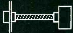
Short lengths of S.S.White flexible shafting make ideal, low-cost couplings. They make accurate alignment unnecessary, thereby saving assembly time and costs—and unlike solid connections, will not transmit vibration.
