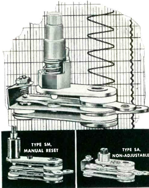
If your product requires sensitive, snap-action control characteristics, better check Stevens Type SA thermostats *first*. For these small, snap-acting thermostats can be used with differentials as wide as 100°F . . . or as narrow as 10°F. Furthermore, standard models are available in adjustable, non-adjustable, manual reset, or single-pole double-throw styles.
