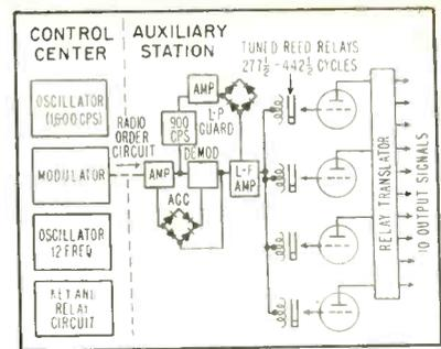
FIG. 1—Block diagram of the remote control system for microwave relay stations
