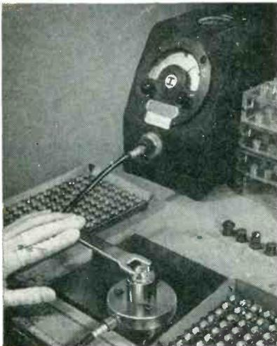
Setup for using air stream to measure electrode spacings on a production basis
