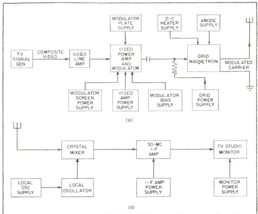
FIG. 4—Grid-magnetron video transmitter and microwave receiver used in television transmission test
