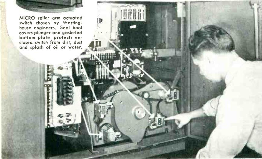
So speedy and efficient is this Westinghouse INDUCTALL gear hardening machine that a battery of five of them is capable of heat-treating up to 300 gears an hour.
