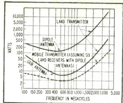
FIG. 1—Transmitter power into antenna required for urban and suburban coverage
