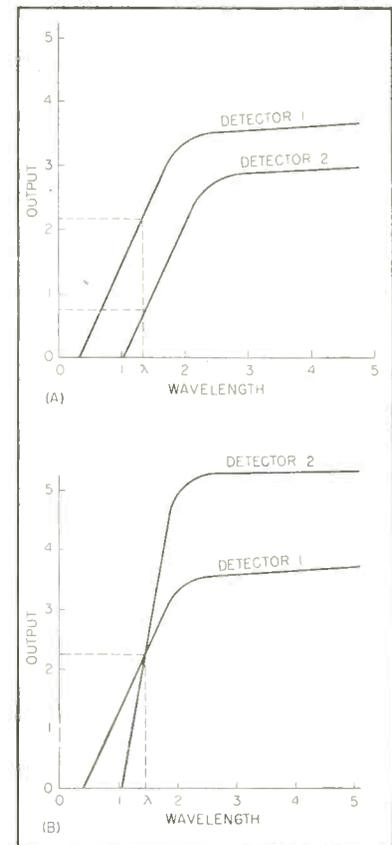
FIG. 4—Output vs wavelength curves for unmatched detectors (A) and curves showing result of attempt to match detectors by sensitivity control only
