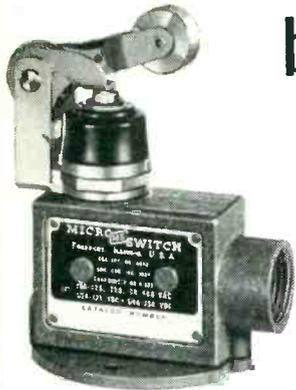
MICRO roller arm actuated switch chosen by Westinghouse engineers. Seal boot covers plunger and gasketed bottom plate protects enclosed switch from dirt, dust and splash of oil or water.
