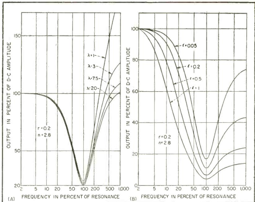
FIG. 4—Effect of output and input loading on bridged-T amplitude response
