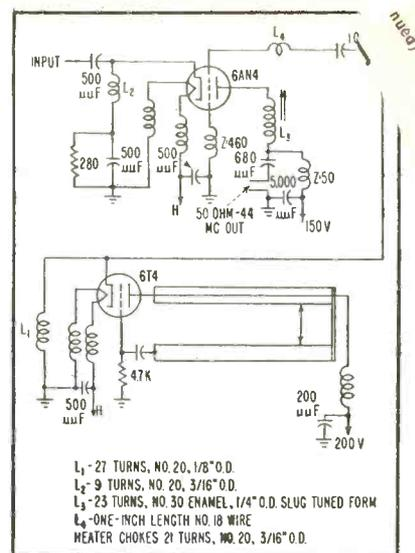
FIG. 2—6AN4 used as mixer with 6T4 oscillator
