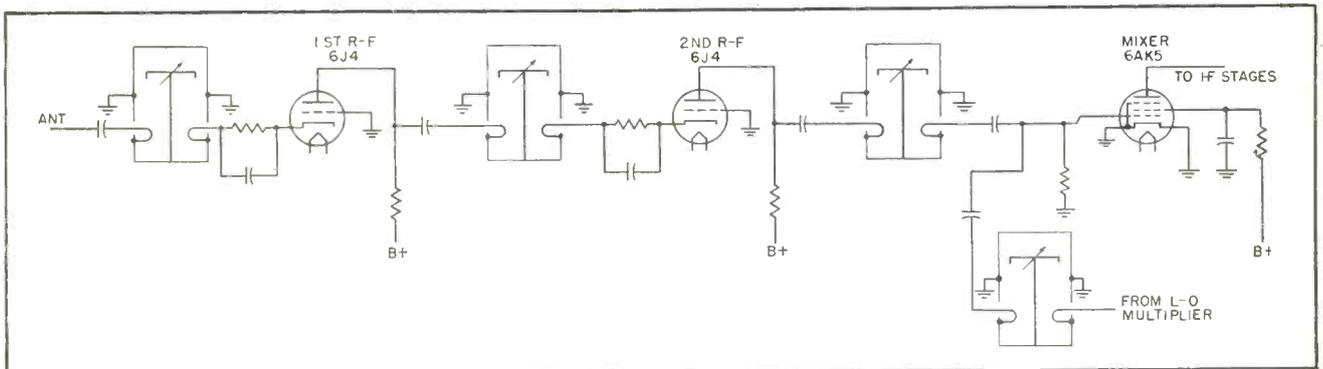
Circuit diagram of the receiver r-f deck
