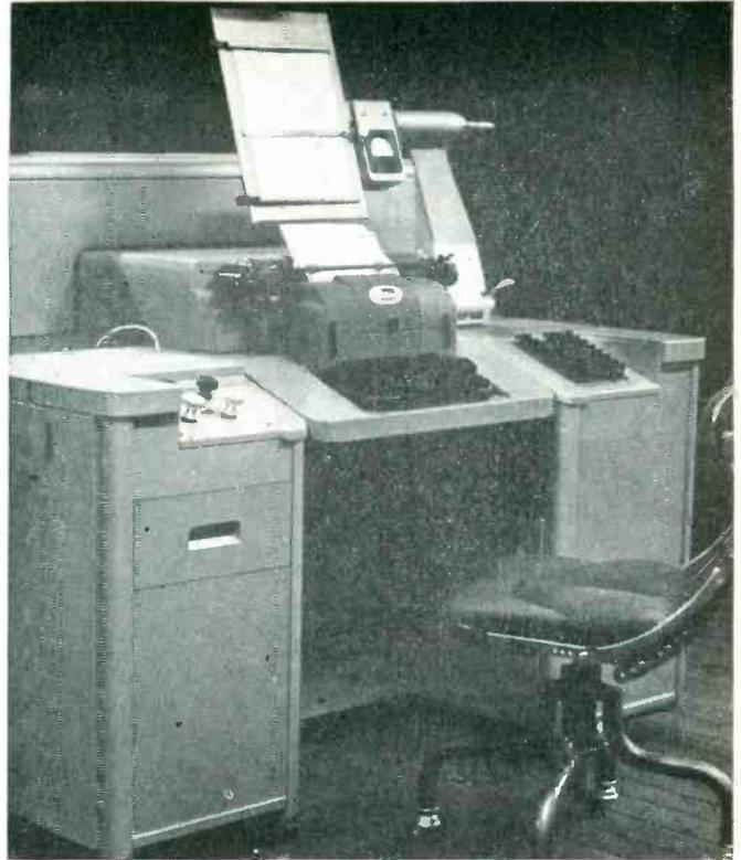
First commercial production model of Photon typesetter. Negative-exposing unit is at rear. Choice of type size and style is made on keyboard at right of electric typewriter. Machine delivers strip of exposed film, resembling galley proofs.
