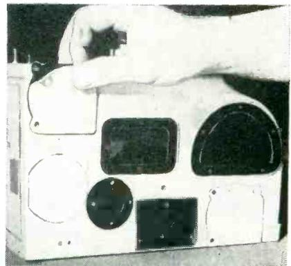
Method of applying precut pressure-sensitive mask to irregular area requiring protection during spraying of electronic equipment housing
