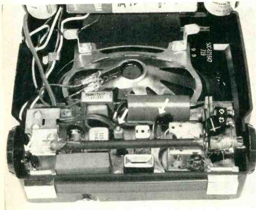
Transistors aren't the only way to cut battery drain. Note subminiature tubes (arrows) used in this new Motorola clock portable. It operates from two 1½-volt A batteries and a 67½-volt B or from 117 volts a-c/d-c. Magnet and associated components are within cone of loudspeaker, saving still more space
