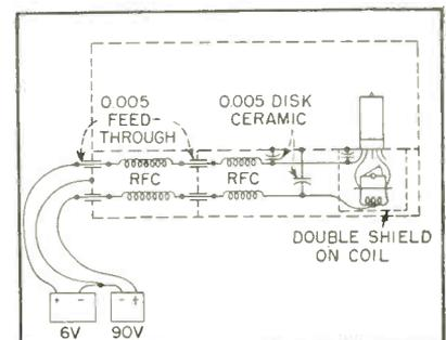
**FIG. 6—Coil shield and second filter section are added**
