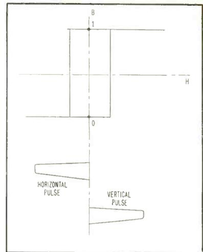
FIG. 2—Cores have square hysteresis loop. Vertical pulse will move core from 0 to 1 position
