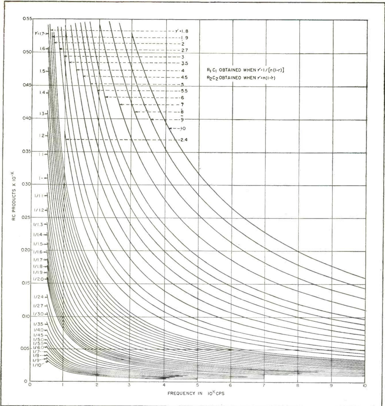
FIG. 6—Nomograph for finding R-C products for bridged and parallel-T networks
