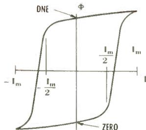
DIAGRAM ILLUSTRATES FLUX-CURRENT CHARACTERISTIC OF FERRITE TOROID WITH NEARLY RECTANGULAR HYSTERESIS LOOP
