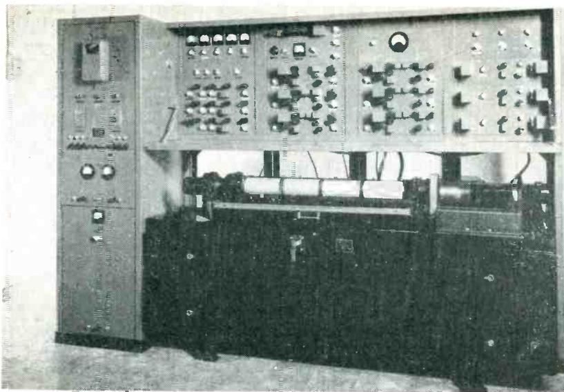
Time-Life color scanner, with light-tight housings swung forward to show the four cylinders on which corrected negatives are exposed
