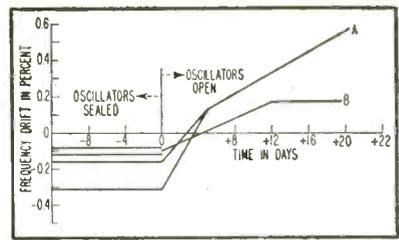
FIG. 2—Chart showing the effect of sealing oscillators. Units maintained in moist atmosphere (A) showed greater drift than those exposed to normal atmosphere (B)
