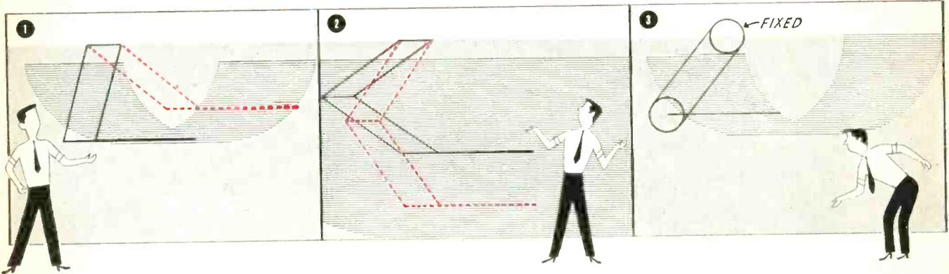
Start with a parallelogram somewhat like this. Visualize one of its short sides anchored to the top of a drawing board parallel to your base line, and let the remaining three sides be free to move together. Add a projecting straightedge to the bottom side as shown, and it will theoretically stay parallel to the base line. Parallel lines could be drawn anywhere within the shaded area above. But clearly, that field of action is too limited.
