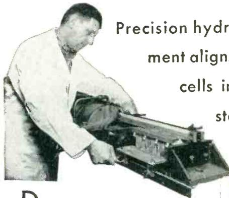
Precision hydraulic equipment aligns and compresses cells into "stacks". Special steel studs keep stacks tight and true.
