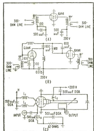
FIG. 1—Two booster circuits (A, B) used to obtain performance characteristics of tubes at vhf. Performance at vhf was obtained from tuned-line amplifier (C)
