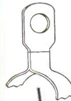
Terminal lugs are tinned for ease in soldering to connecting wires. Resistance wire is welded or brazed to the lug, assuring perfect electrical connection.
