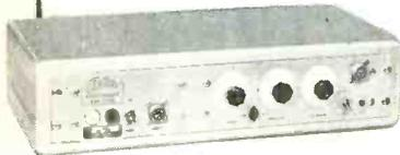
Four stage amplifier for study of steady state and varying phenomena. Amplifies signals from .25 mv to 100 volts. Linear response from DC to 2500 cps. with extended range to 10,000 cps. Low drift, low impedance output. Designed especially to drive Edin recording galvanometers.
