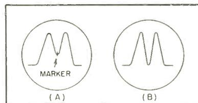
FIG. 2—Resonance absorption patterns seen on cathode-ray screen, for cavity resonance with wavemeter marker at  $f_0$  (left) and for match at  $f_0$
