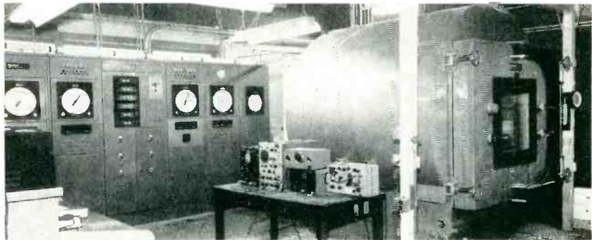
Stratosphere chamber made for Bendix by Bemco Inc., using Square D equipment for power control and Honeywell recorders on the control racks at the rear
