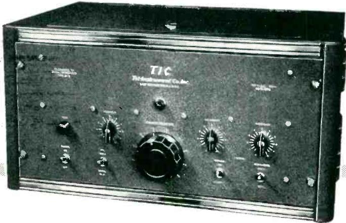
The Type 2113, 12 Channel Picture Signal Generator has been specifically designed for production line testing of TV receivers. Used in conjunction with the equipment listed below, the manufacturer can produce his own "Indian Head" test pattern and is no longer dependent on local transmissions. This signal generator has also received wide acceptance for dealer demonstrations of TV receivers in areas where transmitting facilities are not yet available.
