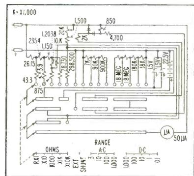
Fig.1—Complete diagram of the printed circuit multimeter
