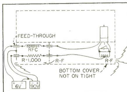
**FIG. 5—Cracks in shielding permit r-f to leak out**
