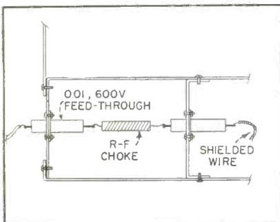
FIG. 7—Recommended construction of shielding for filter section
