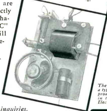
The illustrated, a typical "GTC" product, is used in the Parmak Electric Fencer...
