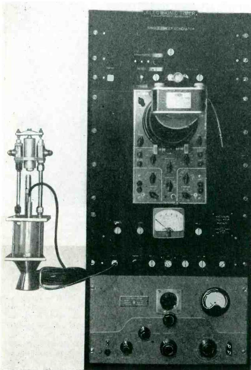
Pressure test cell at left is used to test the recorder built into table-mounting rack. Single-sweep oscillator at top provides timing marks
