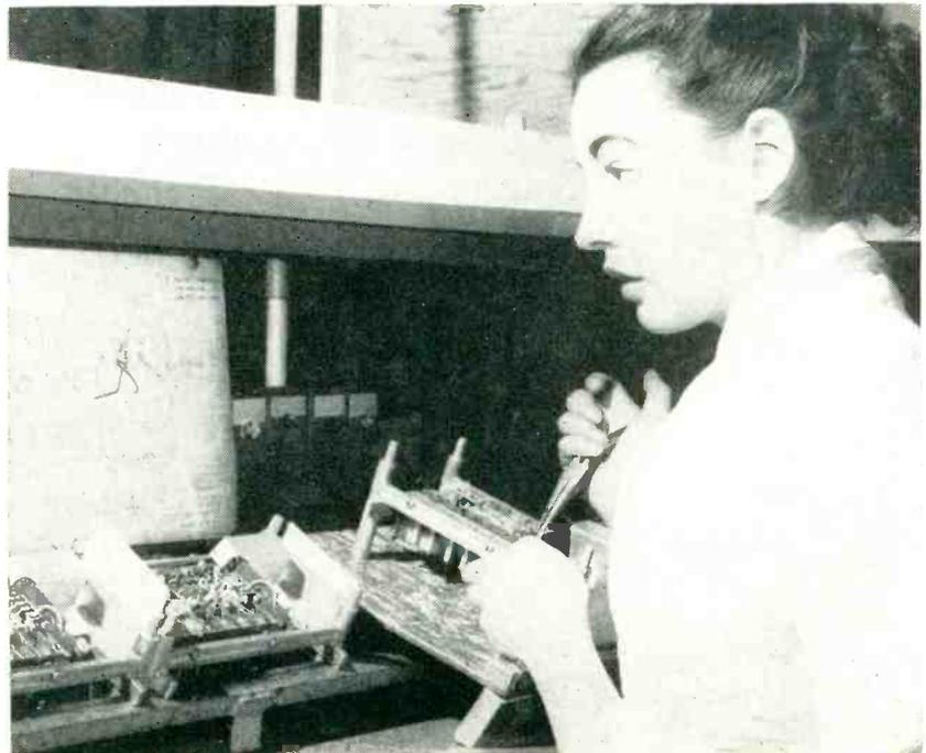
Use of self-stacking die-cast carriers on pass-along assembly line
