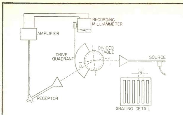
FIG. 1—Diffraction grating spectrometer
