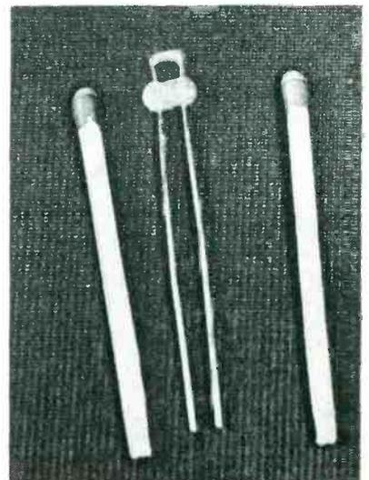
Comparison of CdS detector with ordinary match shows small size
