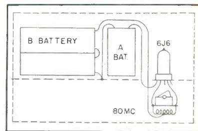
FIG. 2—Complete shielding of batteries, leads and oscillator proved most effective in tvf elimination
