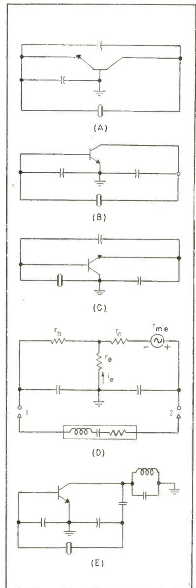
FIG. 1—Simple junction-transistor crystal oscillators
