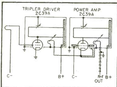
Circuit diagram of the r-f deck used in the transmitter
