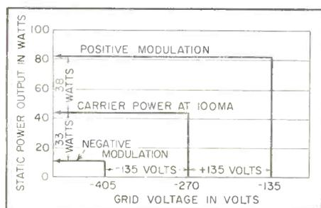
FIG. 1—Magnetron power output versus control-grid voltage
