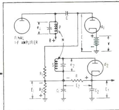
FIG. 1—Trigger voltage circuit
