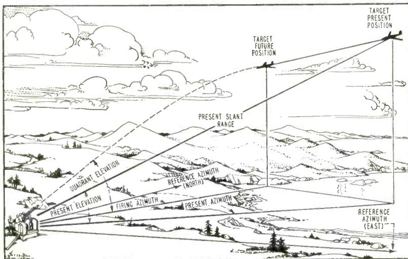
FIG. 1—Pictorial representation of fire-control problem
