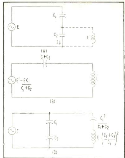
FIG. 1—Circuit simplification for shunt impedance calculations
