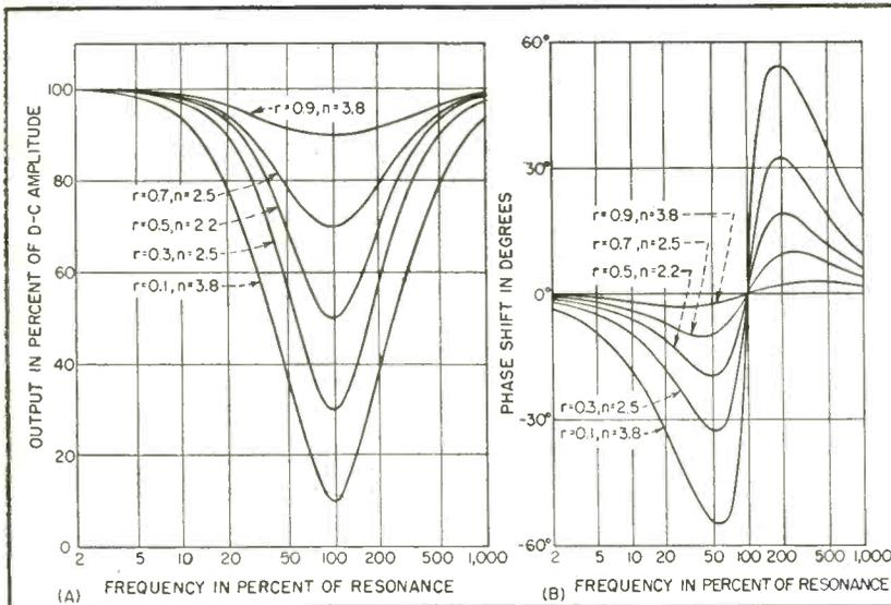
FIG. 1—Amplitude and phase response of bridged-T network as notch ratio,  $r$ , is varied. Minimum notch width,  $n$ , is chosen for each value of  $r$
