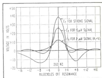
FIG. 3—Selectivity curves for the circuit described in text
