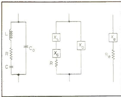
FIG. 1—Equivalent electrical circuits of crystal unit
