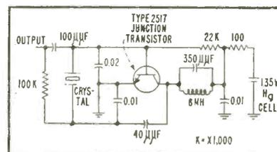
FIG. 2—Experimental transistor crystal oscillator
