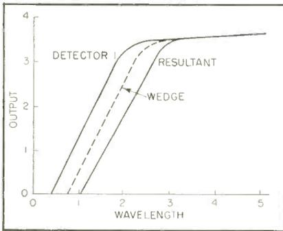
FIG. 5—Detector output vs wavelength response shifted by addition of absorbing material
