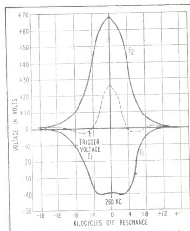
FIG. 2—Selectivity voltage of Fig. 1 circuit
