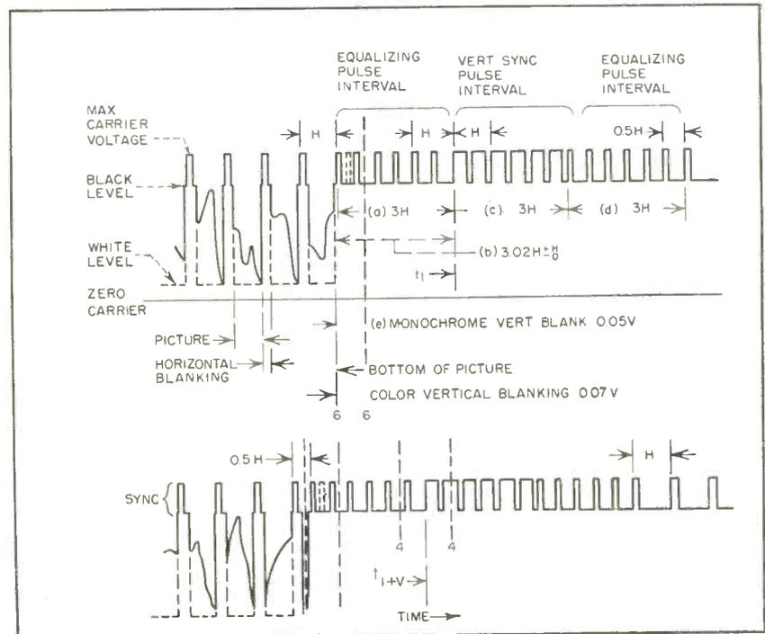
FIG. 2—Color-index pulse in FCC field sequential system has frequency of 48 cps, time rise of about 0.24 microsecond and provides automatic correction of color-index-errors
