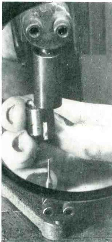
Use of permanent magnet to place grid over flaring tube, as viewed through illuminated magnifying glass
