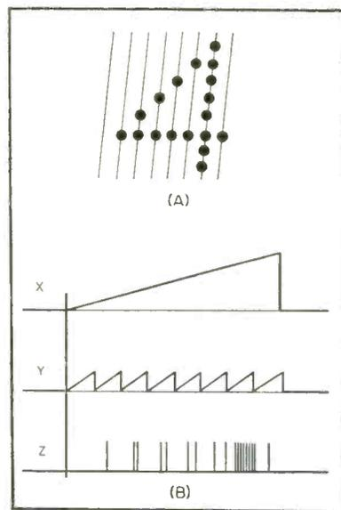
FIG. 1—Number produced (A) by intensifying crt scanning beam. Three waveforms (B) are required
