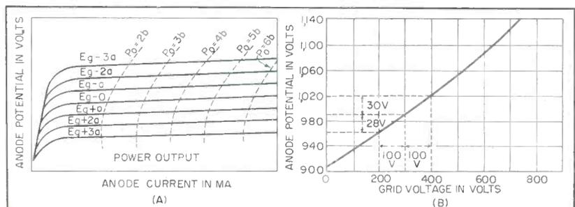
FIG. 2—Plate characteristic and grid-to-plate transfer characteristic for grid-controlled magnetron
