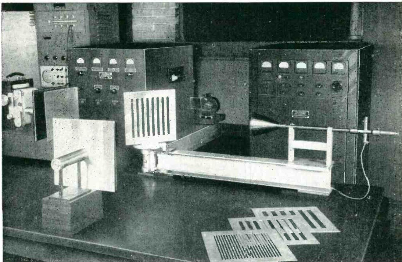
Michelson interferometer arrangement of equipment for determining frequency with a 1.25-cm magnetron. These components can be rearranged for Boltzmann interferometer measurements or as a diffraction grating spectrometer
