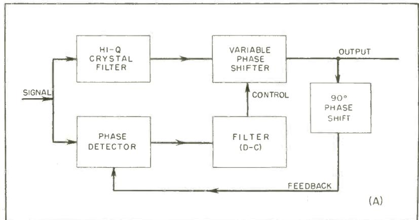
FIG. 6—Passive integrator circuit employs high-Q quartz crystal filter at subcarrier frequency, with 3-db bandwidth in order of 100 cycles. Circuit is sensitive to mistuning
