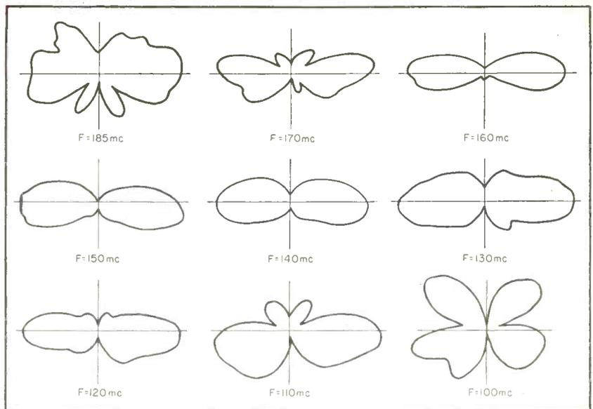
FIG. 5—Radiation patterns of three-element array at various frequencies
