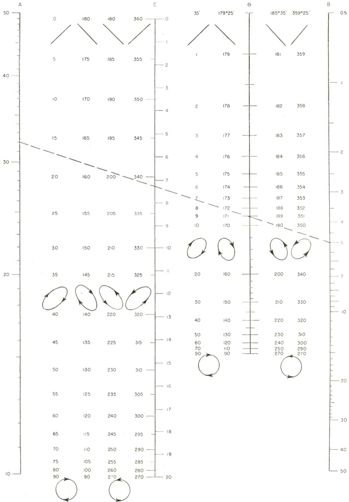
FIG. 2—Nomograms convert intercept-to-maximum ratios into phase angles as explained in text
