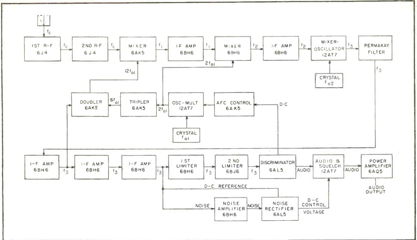
Block diagram of the 450 to 470-mc receiver
