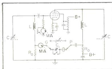
FIG. 4—Simplified circuit of crystal impedance meter
