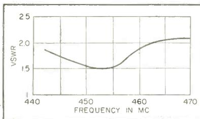
FIG. 3—Graph of vswr versus frequency for a seven-element antenna
