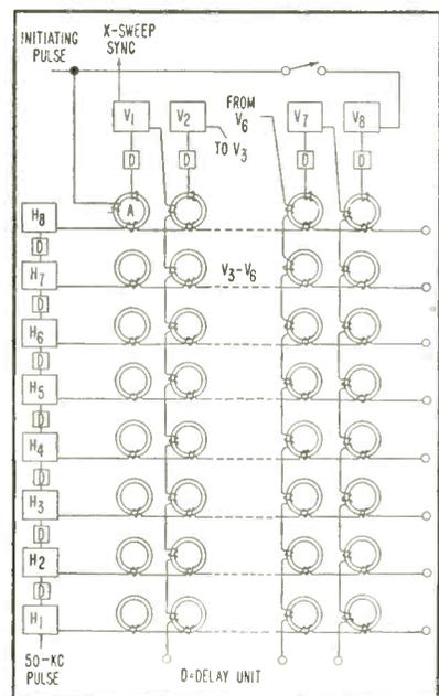
FIG. 3—Eight-by-eight magnetic matrix used in number generator
