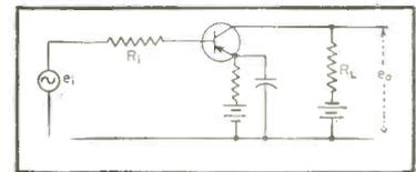
FIG. 1—Grounded-emitter transistor
