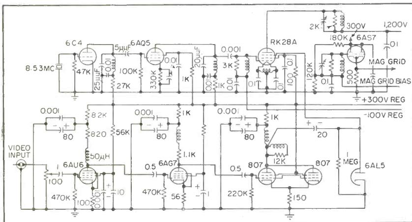
FIG. 7—Frequency generator, video amplifier and modulator for subcarrier system. Amplified composite video is applied to suppressor grid of RK28A pentode. Magnetron grid drive is taken off cathode follower
