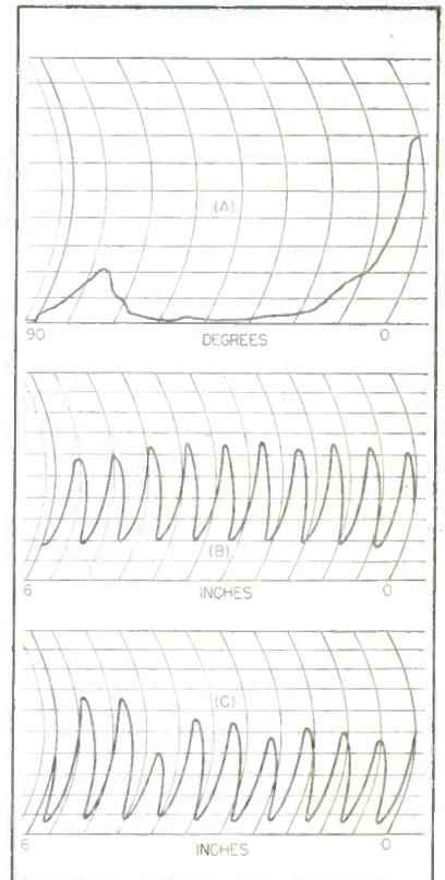
Typical recordings from grating spectrometer (A), Boltzmann interferometer (B) and Michelson interferometer (C)
