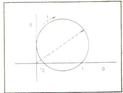
FIG. 3—Admittance diagram of crystal unit
