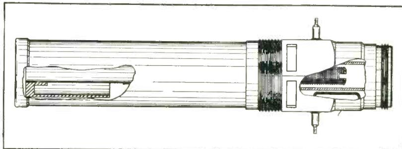
Receiver tuned cavity has input and output probes and loading drum
