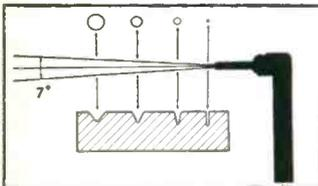
The diameter and form of the "Airbrasive" cut is determined by the distance of the nozzle from the work, as shown in this illustration. The depth and speed of cut can be varied by varying the angle of impingement and the richness of the "Airbrasive" mixture.
