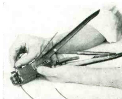
Inserting stripped wire into connector. Cartridge-holding magazine is under thumb of left hand
