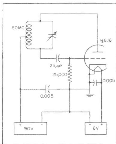
FIG. 1—Circuit of low-power oscillator used to simulate local oscillator of a tv receiver
