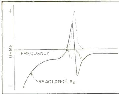
FIG. 2—Impedance characteristic of crystal unit
