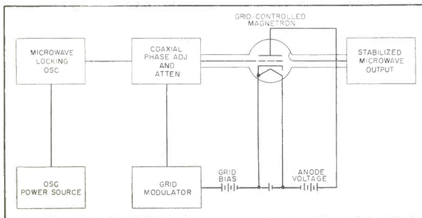
FIG. 8—Frequency-stabilization system for grid-controlled magnetron
