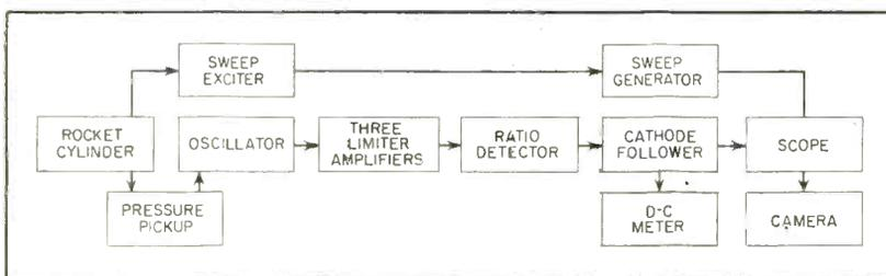
FIG. 1—Block diagram of the rocket pressure recorder. The instrument gives a graph showing pressure variations and time
