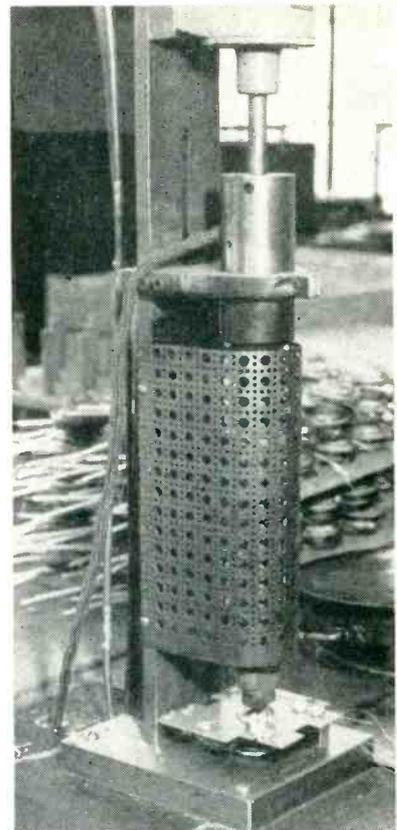
Coil form and terminal board in position ready for heat-and-pressure flaring operation
