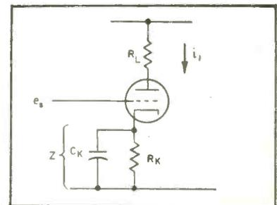
FIG. 1—Simple amplifier circuit illustrates bypassing situation discussed in letter
