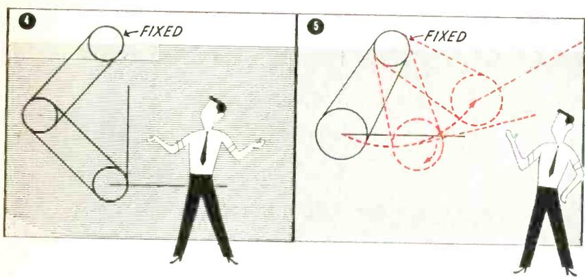
The band-and-drum machine, with all three drums of precisely equal diameters and with bands which will not slip, will draw absolutely parallel lines over the entire working area. But if the drum diameters are not equal, the parallelogram principle is violated and the machine cannot draw parallel lines. The greater the difference in diameter the more the lines will be out of parallel.
