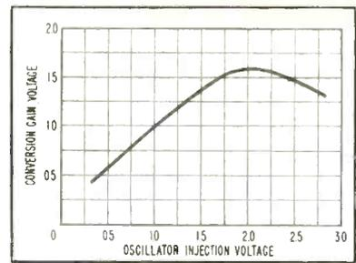
FIG. 3—Conversion gain characteristics of 6AN4
