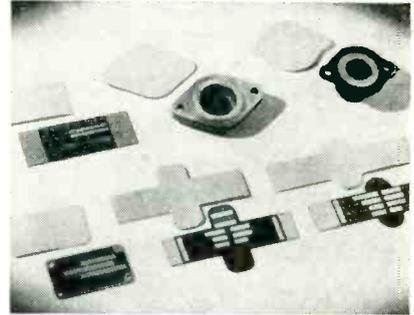
Examples of precut masks used for protecting name plates and openings during spraying
