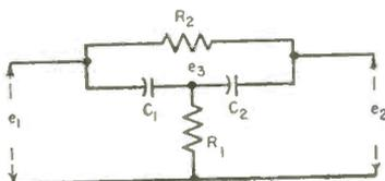
Resistor-Shunt Bridged-T Network
