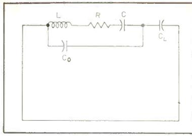
FIG. 7—Crystal unit connected to its load impedance
