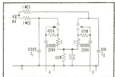
FIG. 2—Flash circuit provides double spark from main and delayed trigger
