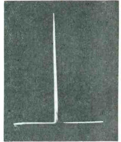
unlocked carrier and sidebands as external signal is tuned continuously, coming closer and closer to unlocked carrier. Finally the grid magnetron's output locks in frequency with the external signal and sidebands disappear
