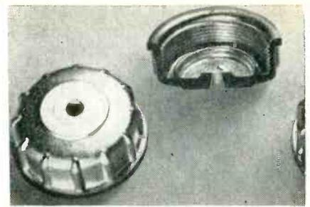
Example and cross-section of plastic knob on which a hard coating of nickel has been deposited chemically with a new process having 100-percent throwing power
