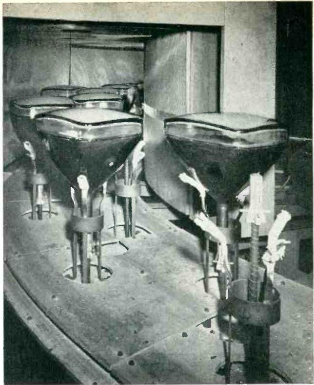
The Inconel "X" spring seen in the foreground supports the television tube on the "spider" during a 45-50 minute baking and cooling cycle that reaches 750° F. The oven for which this spring problem was solved is one designed and made for a famous electronic equipment manufacturer by TRUTNER & BOUMANS, INC., Hillside, N. J.
