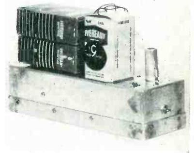
Test oscillator with top cover removed to show batteries and leads
