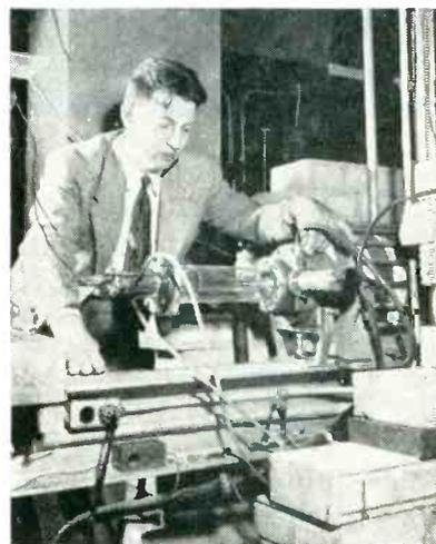
Linear accelerator used in nuclear research uses the firing chamber shown in the photograph. Edward L. Ginzton, Director of Stanford University's microwave laboratory is shown aiming electron bullets shot down the 200-foot gun. They attain a speed 99.9 percent that of light in the first foot traveled
