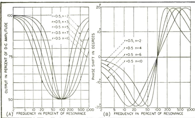
FIG. 2—Amplitude and phase response of bridged-T network as notch width is varied with notch ratio held constant
