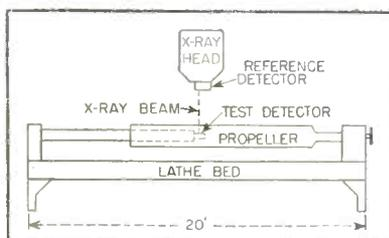
FIG. 1—Cadmium sulphide detector is drawn through spinning propeller
