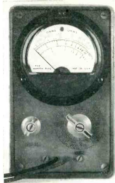
Meter dial and controls of multimeter. Note nonlinearity of meter scales
