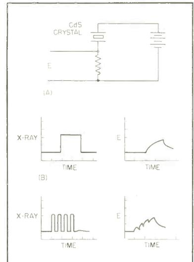
FIG. 3—Connection of CdS crystal and typical response curves
