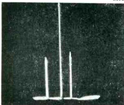
Spectrum-analyzer view of magnetron output with one-mc modulation
