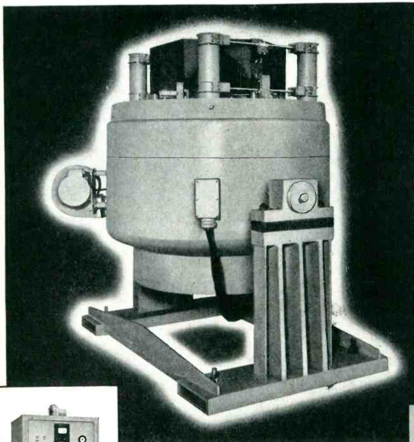
HERE'S the latest—and the largest—vibration exciter ever built for shake testing. Developed by MB vibration specialists, this unit incorporates all the advances made in the last seven years for assuring dependable operation, pure table motion, and absence of resonances. These include specially designed table flexures, forced air cooling, built in protection against overtravel of the table and against misoperation of the equipment.
