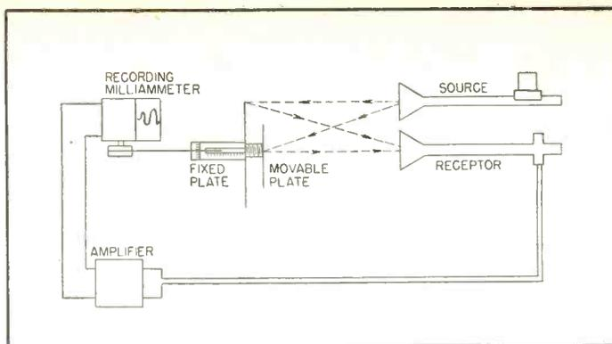
FIG. 2—Boltzmann interferometer
