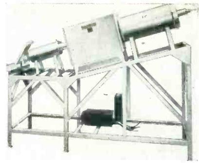
New germanium production furnace made by Hevi Duty Electric Co., Milwaukee, Wisconsin. Crank at upper left on machine is used to pull the boats of germanium oxide through the various stages of the furnace. Square center section is 1,000-deg C second-stage furnace
