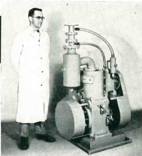
*NRC Rotary Gas Ballast Pump —
