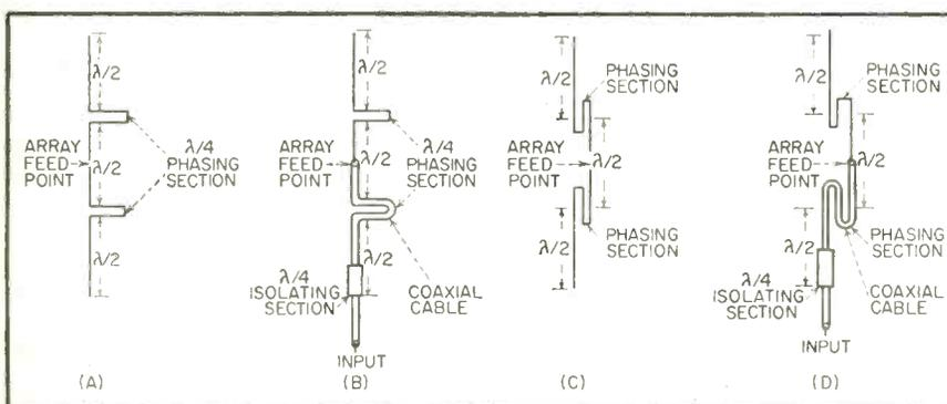
FIG. 1—Development of antenna system from two arrangements of the Franklin colinear array (A and C). The portion of the antenna above the feedpoint, in B and D, is an extension of the center conductor of the coaxial cable. Outer shield of cable is used as lower portion of radiator. A quarter-wave isolating sleeve terminates lower radiator in this type of arrangement.
