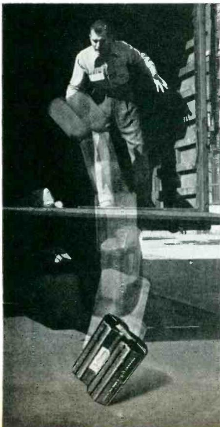
**3. New Molded Shipper** has a soft lining to cradle wire spools gently. Top half rests in bottom... and stores in one-third the space required by wood empties.
