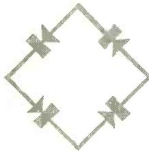
**For Carrier Communications, IN71 VARISTOR.** The IN71 consists of 4 matched low impedance diodes each of which, with +1 volt impressed, will pass a current of 1 ma. of the average current of the four.
