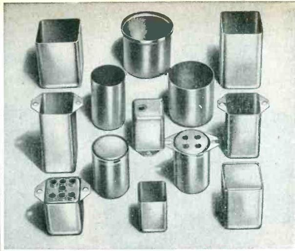
hot tin dipped . . . fabricated terminal and vent holes . . . smooth, one-piece construction using cold rolled steel . . . draw depths up to 2½" . . . inside fit covers for easy hermetic sealing in all sizes . . . available as stock sizes and as special fabrications.
