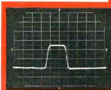
37.5 Mv., 0.2  $\mu$  sec width, 1  $\mu$  sec sweep full scale
