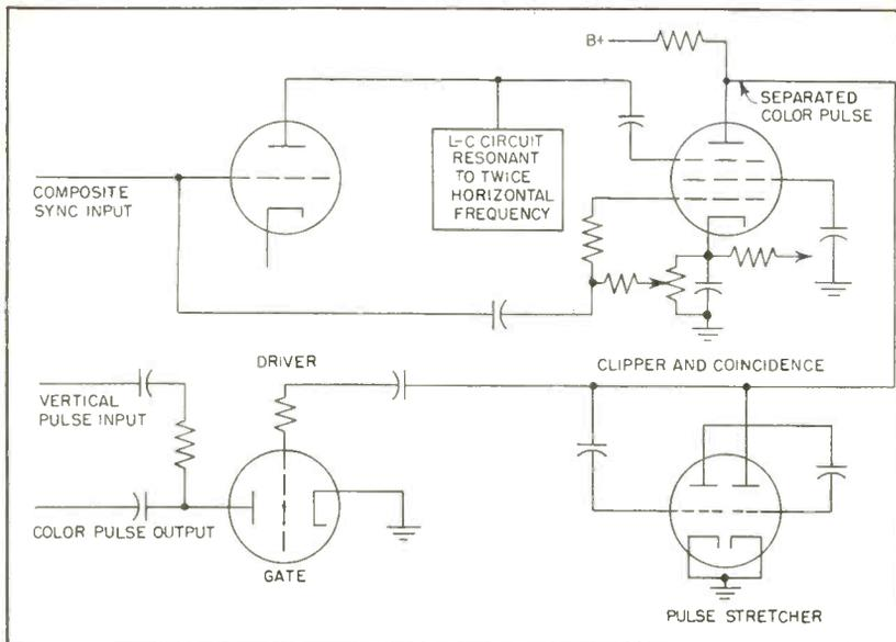
FIG. 3—Typical receiver circuit separates color-index pulse from horizontal and equalizing pulses in a coincidence amplifier and uses color pulses to index color disk to proper position
