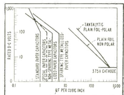
FIG. 1—Volume comparison of tantalum-foil and paper capacitors
