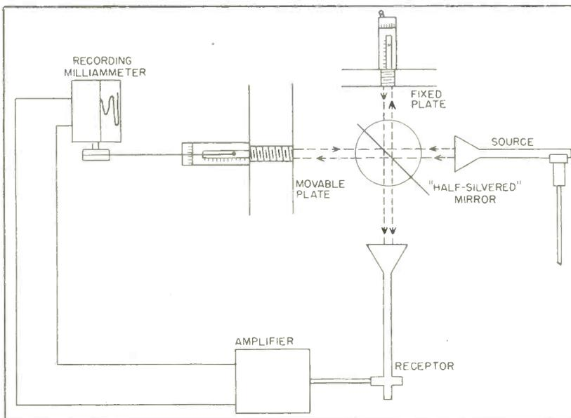
FIG. 3—Michelson interferometer
