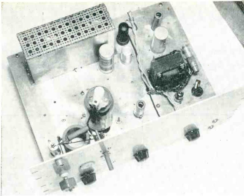
Type RK28A subcarrier final is suppressor modulated by video signal
