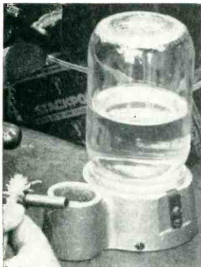
Crosley-designed cement dispenser being used with small brush to apply household cement to a finished coil
