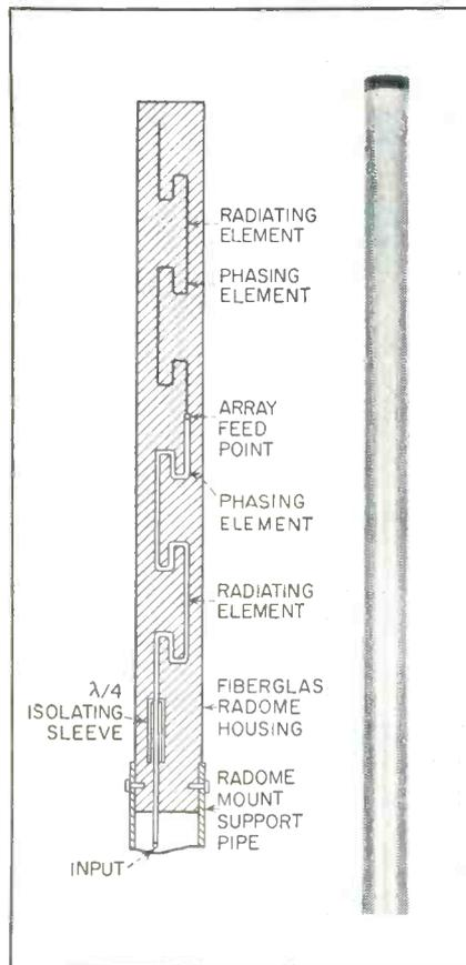
Seven-element array and cross section showing coaxial element imbedded in Fiberglass tube
