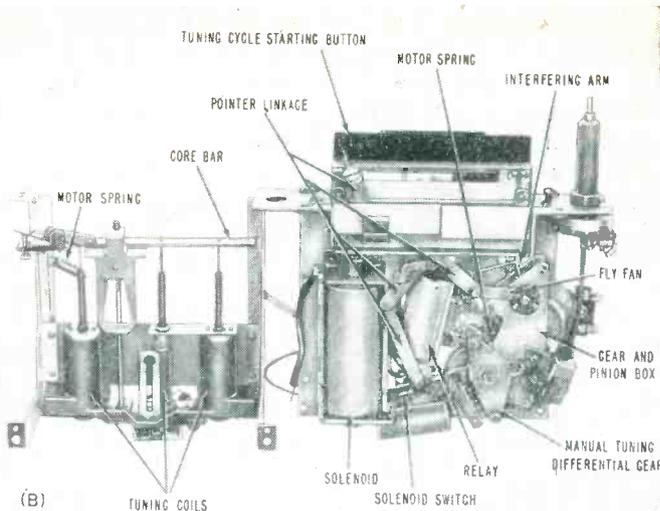
FIG. 5—Simplified tuning mechanism (left) and side view (right) of actual mechanism used in Oldsmobile car radio
