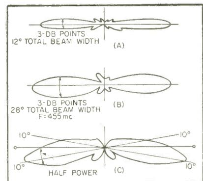
FIG. 2—Radiation patterns of three arrays. Pattern of seven-element unit is shown at A and a three-element unit in B. Pattern C is produced by a five-element array with 8-deg beam tilt
