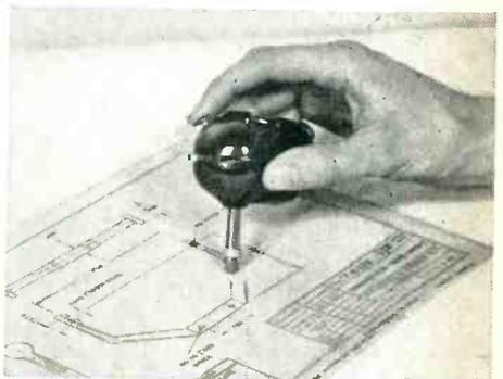
After you've once used a K&E MOTO-RASER,† you'd no more go back to hand erasing than you'd take to drawing with your gloves on. With MOTORASER you can either pin-point your objective, or cover a larger area without damage to the drawing surface. Runs on 110 volt 60 cycle AC, or DC with an inexpensive adapter.
