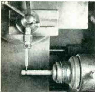
One of the many applications on which the S.S. White "Airbrasive" Unit has been successfully used — cutting spiral bands on a deposited carbon resistor. Successful applications are also to be found in printed circuit work.
