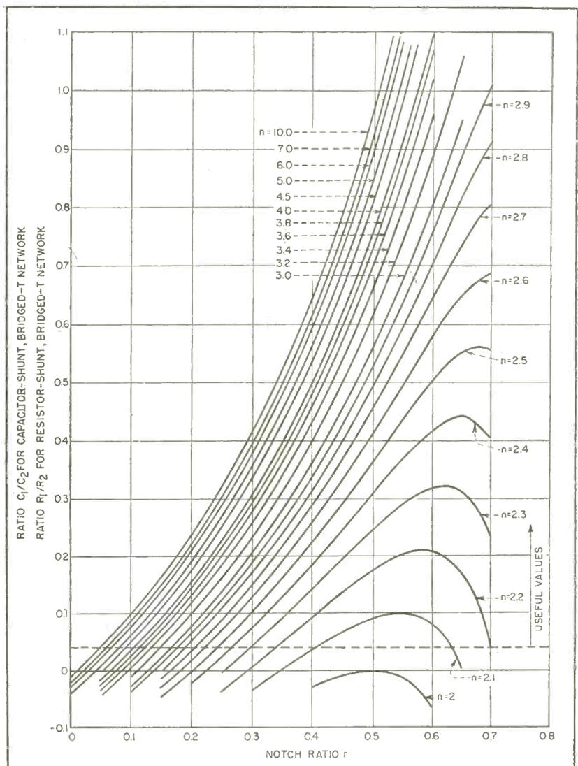
FIG. 5—Nomograph for finding  $C_1/C_2$  or  $R_1/R_2$  ratio for bridged-T network
