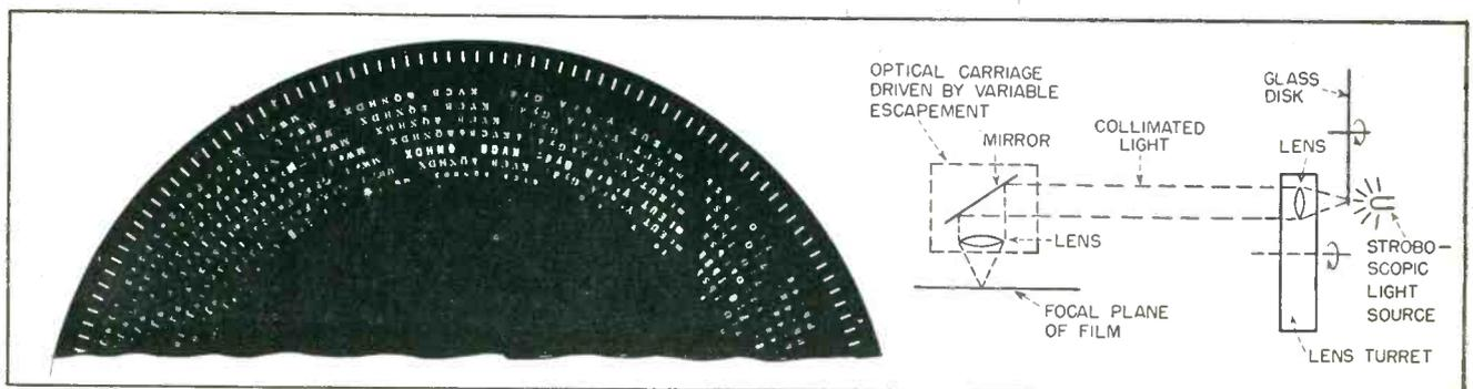
FIG. 2—Portion of typical matrix disk for typesetter, containing 16 completely different fonts of type. This 1½-lb disk is equivalent to 4,000 pounds of lino type matrixes costing over \$25,000. Precision character-positioning slits fill outermost circle. Optical system for disk is shown at right
