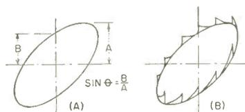
FIG. 1—Ratio of  $B$  to  $A$  is sine of the phase angle ( $A$ ); typical pattern with sawtooth superimposed ( $B$ )
