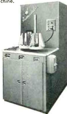
Exterior view of Westinghouse INDUCTALL gear hardening machine which shows the clean, compact design of this modern machine tool for mass-production gear hardening.
