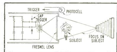
FIG. 1—A plastic Fresnel lens collects sufficient light from the spark source to make shock waves visible. The photocell triggers the spark
