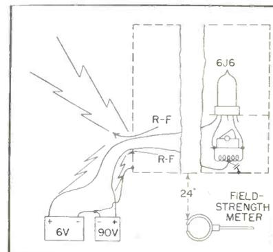
FIG. 3—Power leads conduct r-f out of shielded compartment
