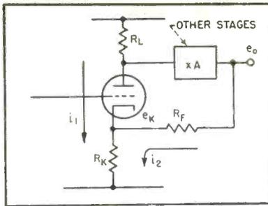
FIG. 2—Circuit with feedback current adding to normal tube cathode current
