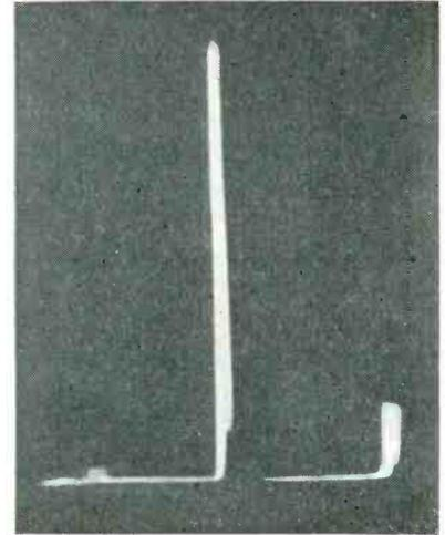
Spectrum-analyzer waveforms illustrate technique for locking magnetron's r-f output to a crystal-controlled signal. Sidebands appear as locking oscillator is turned on two megacycles above the magnetron's unlocked frequency. Waveforms (3) and (4) show
