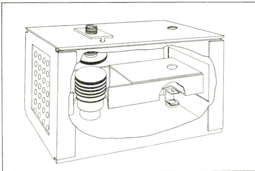
Internal construction of the transmitter tuned cavity
