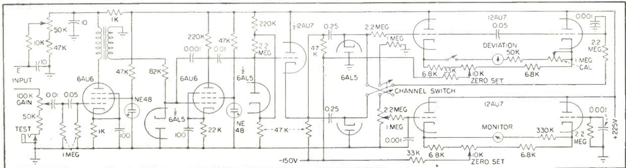
FIG. 6—Circuit diagram of crystal-signal amplifier and metering circuit
