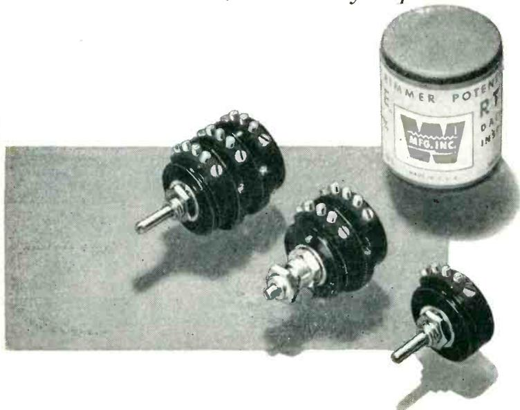
THE WATERS TYPE RT SERIES of miniature, wire-wound potentiometers will satisfy your most stringent requirements. Anodized-aluminum bodies with sealed, line-reamed shaft bushings and sealed terminal plates enable these units to meet severe environmental tests — immersion, salt spray, fungus, shock, vibration, and wide temperature range.
