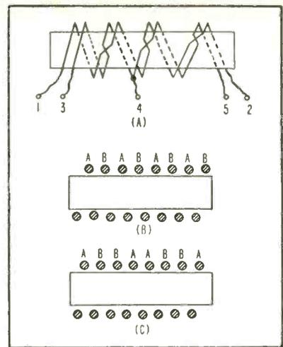
FIG. 2—Bifilar winding technique (A) showing method of crossing conductors. Cross section of conventional (B) and new winding (C) shows how conductors are placed
