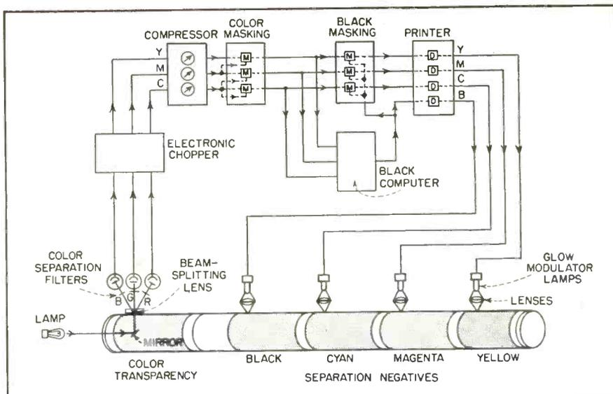
FIG. 3—Functional diagram of Time-Life scanner for producing four corrected separation negatives from one color transparency simultaneously
