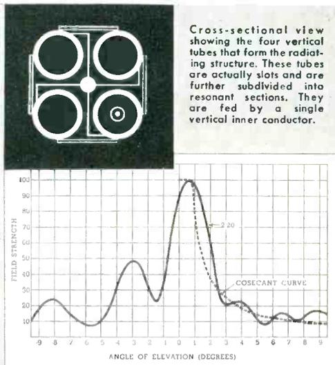
Radiation pattern of Model WA-25-XX with null fill-in and beam tilt of  $0.65^\circ$ .
