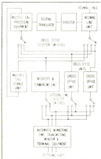
FIG. 1—Block diagram of message handling system in Army switching center
