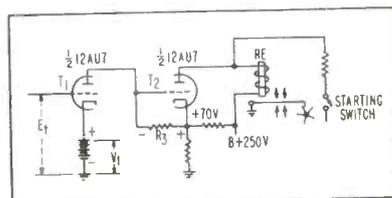
FIG. 4—Trigger circuit that actuates fly fan
