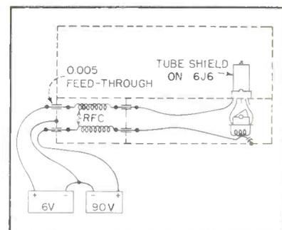
FIG. 4—No r-f leaks out on filtered power leads
