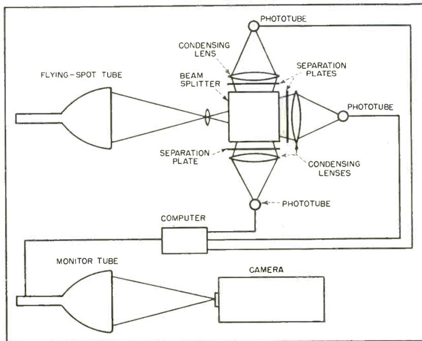
FIG. 4—Method of using cathode-ray tubes in RCA all-electronic machine equipment. This system converts separation plates into four corrected negatives
