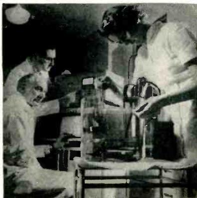
Flowability of a fluid is measured instantly and continuously with this new instrument for industry and the medical profession. A small ultrasonic sensing probe is applied to a blood sample while an electronic computer and recorder chart how fast a clot is formed
