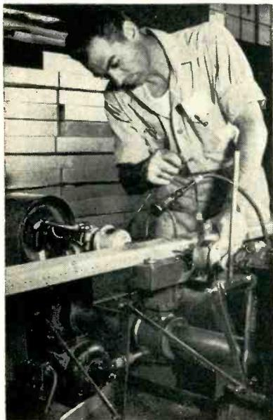
Dual-head tapping machine uses single-lever control to speed tapping of holes in U-channels. The W-shaped linkage is in foreground. Dual-outlet coolant pipe is directly over taps
