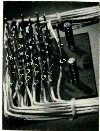
Closeup view of relay base, showing appearance of solderless wrapped connections. The wrapping tool starts its winding at the bottom of the terminal and works outward until it runs out of wire
