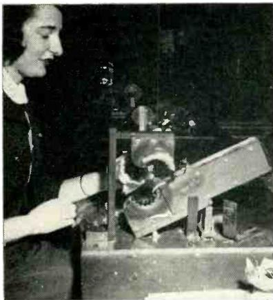
Placing yoke coil assembly in insulation-wrapping fixture, after placing tape on slide, adhesive side up, and placing end of varnished cambric strip on tape
