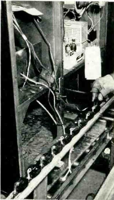
Plugging television set into connector that slides in power trough mounted alongside conveyor line
