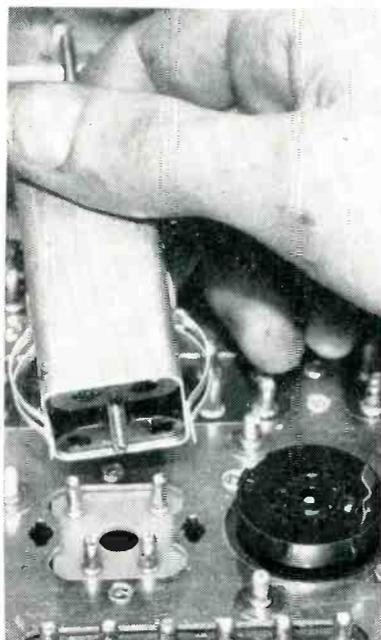
This i-f transformer has a built-in adapter and spring-type mounting clips that make mounting and connecting a single quick operation
