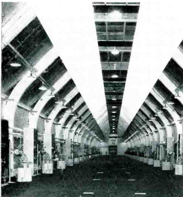
Interior of rocket test laboratory, as viewed downrange from station 3. White reflective strips on ceiling are required for silhouette photography. Sandbag missile stop is at far end. Camera takes six images in sequence, as at top of page
