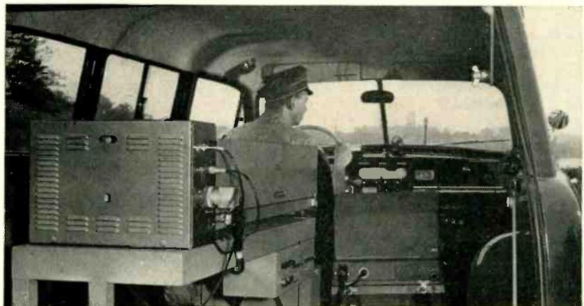
Facsimile equipment connected to two-way radio circuit produces a telegram while the driver proceeds to point of delivery. Six cars being tested in Baltimore, Md. use special radio and conversion equipment shown at left. Facsimile machine to right of driver reproduces telegram transmitted from office
