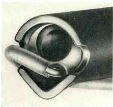
End of wrapping tool, with wire in position ready for wrapping. Wire is inserted in outer slot of spindle as shown, and terminal goes in round hole of spindle
