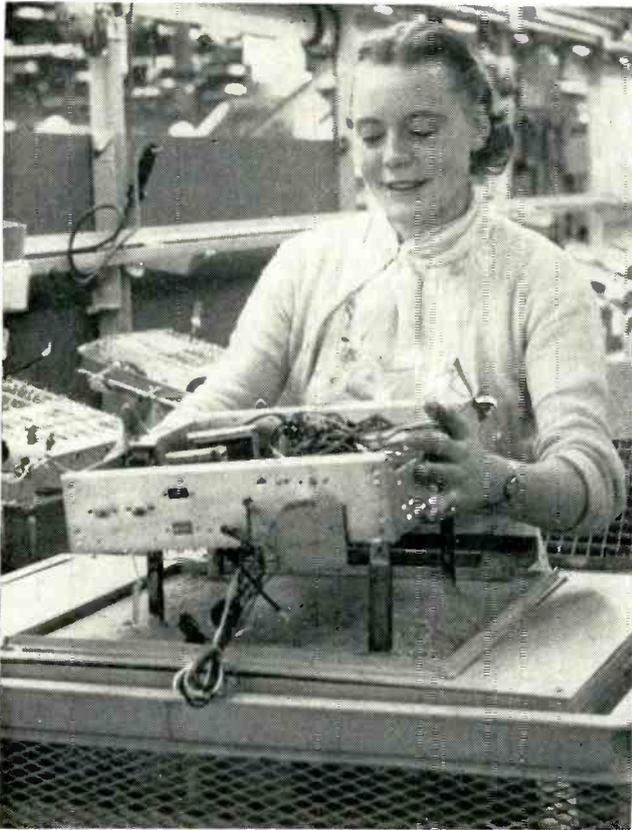
Shake table clears chassis of loose solder and scraps, and also shows up imperfect joints
