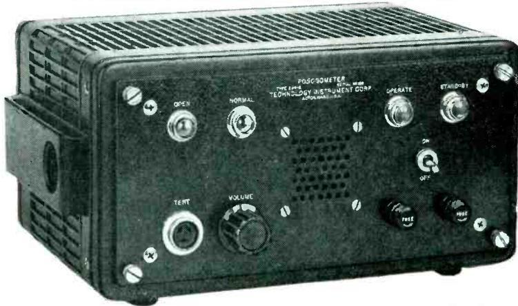
Designed as a production and laboratory test instrument by the Technology Instrument Corporation for quality control in the manufacture of their precision potentiometers, the Type 394-A Ponometer is now available for such uses as:
