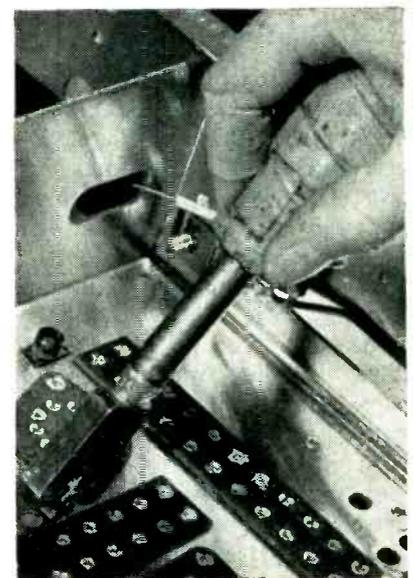
Method of installing coil-mounting clips in chassis of GE dip-soldered television receiver. Mounted clip can be seen just above head of tool
