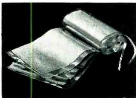
*Unrolled view (one-third size) of capacitor unit wound with "Mylar." The transparent film is only 0.0005" thick yet stands handling without breaking.*
