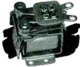
**R 83 SERIES**—Available with A.C. or D.C. coils. Contact ratings up to 30 amperes continuous, 150 amperes inrush with single pole double-break arrangement. Multiple contact springs with proportionately lower ratings also available. Size: 1-7/8x1-5/16x1-5/8 high.
