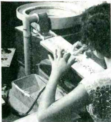
Arrangement used for cleaning and inspecting tiny punched mica parts. Vacuum cleaner under bench is connected to flared metal outlet over screen with thin metal tubing
