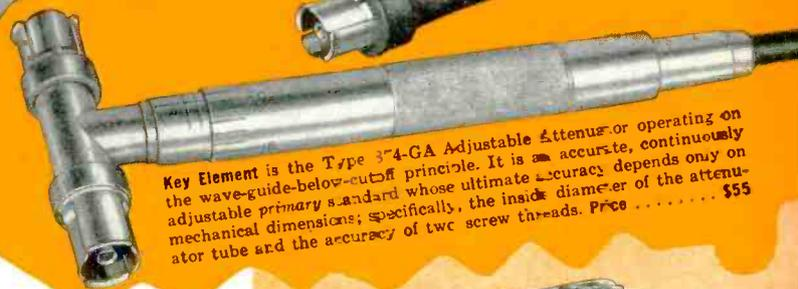
Key Element is the Type 374-GA Adjustable Attenuator operating on the wave-guide-below-cut-off principle. It is an accurate, continuously adjustable primary standard whose ultimate accuracy depends only on mechanical dimensions; specifically, the inside diameter of the attenuator tube and the accuracy of two screw threads. Price . . . . . \$55
