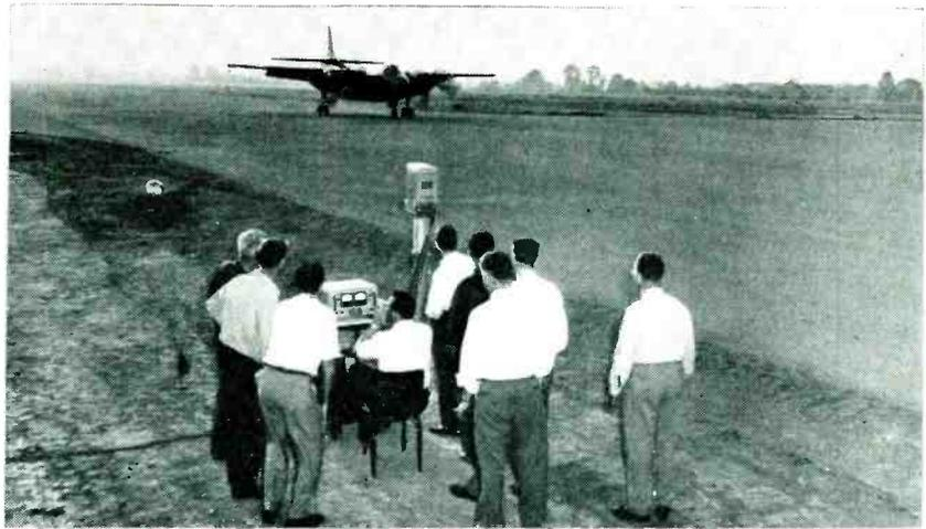
Two-unit descent indicator measures time required for plane to descend one foot
