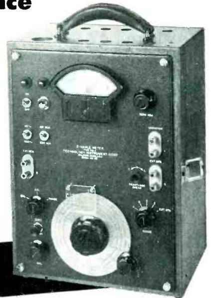
The type 310A Z-Angle Meter measures impedance directly in polar coordinates as an impedance magnitude in ohms and phase angle in degrees:  $Z/\theta$
