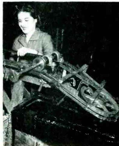
Wax-dipping machine using coil spring attached to rubber V-belt. Operators are loading belt by pressing one lead of each capacitor between turns of the spring. Length of belt is sufficient for wax to harden before units are knocked off automatically
