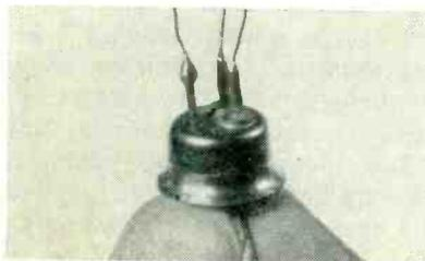
Conduction-cooled 20-watt transistor
