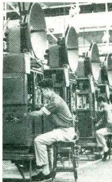
Skyscraper radar production line. Entire unit is later packaged in single steel container for shipment
