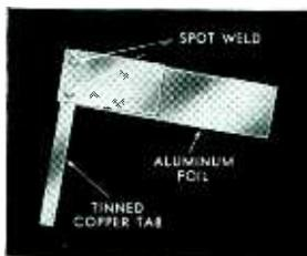
*Inserted welded-flag tab construction insures positive contact from flag to tab — protects paper from edge of tab stock — provides larger area of contact to the foil.*
