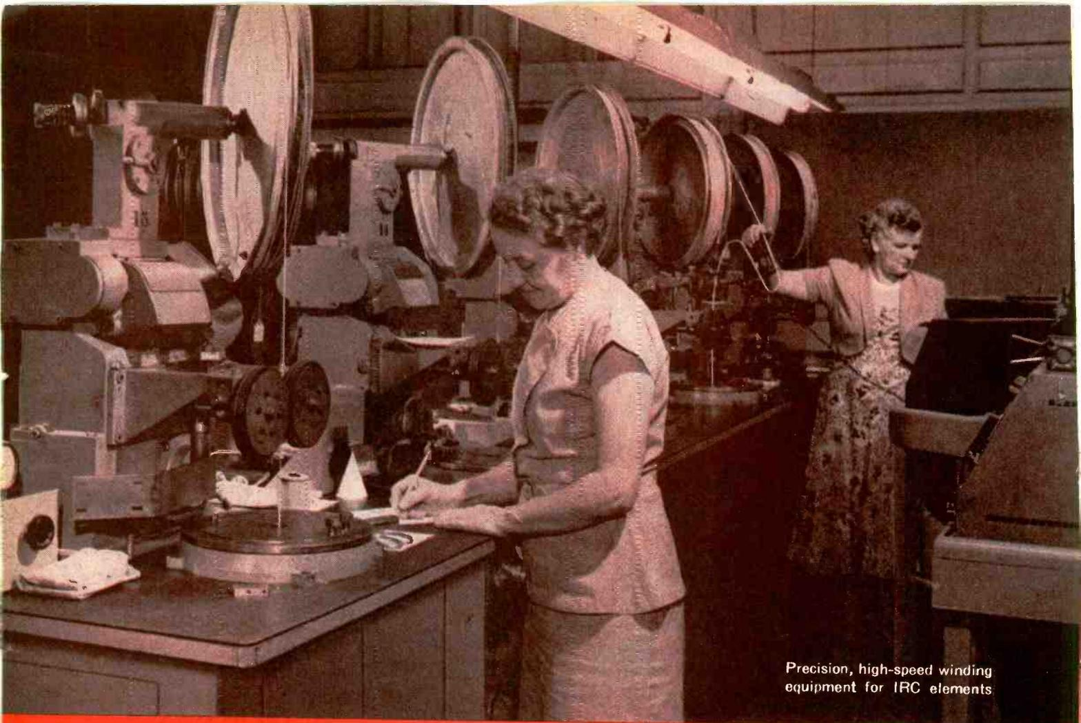
Precision, high-speed winding equipment for IRC elements
