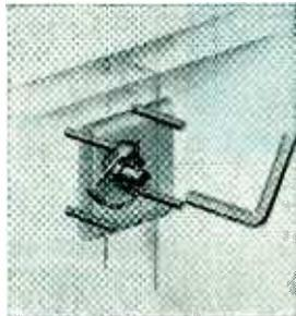
**ROTO-LOCK** Serrated, tapered cam is engaged by formed lug as fastener is locked. Cam action draws panels together tightly, insures locking even under conditions of misalignment. Opens easily for demounting. ROTO-LOCK carries heavy tension and shear loads; can be used for air and water-tight seals; recesses completely into panels. Solidly built without springs or delicate mechanical parts, unaffected by arctic temperatures or field service.
