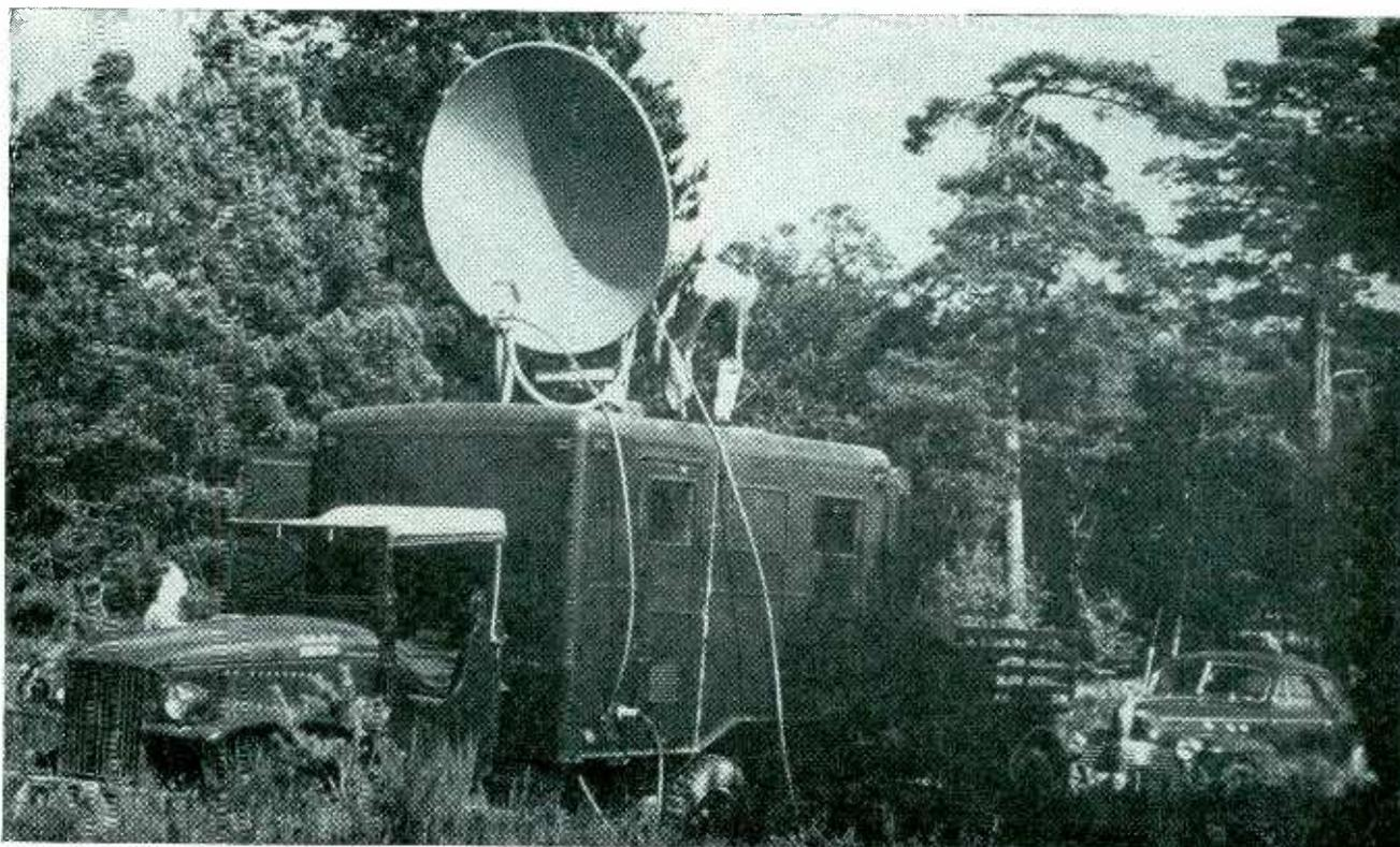
Microwave equipment in use during NATO maneuvers somewhere in France. Military van contains electronic equipment; 5-kv gasoline-driven generator follows in trailer
