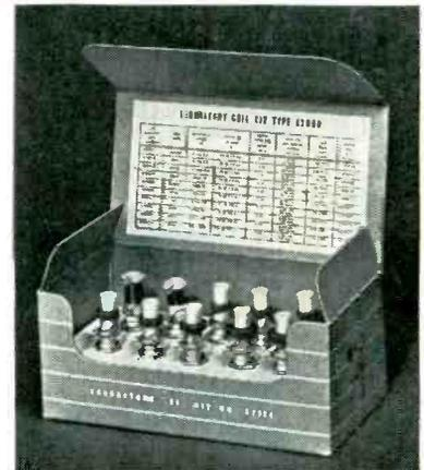
**NEW COIL KIT X2060** for developing prototypes and pilot models contains 10 slug-tuned coils of LS6 size, type C, with silicone fibreglas collars. Range: from 2 Microhenries to 800 Microhenries, each coil slightly overlapping next coil in scale. Kit includes mounting hardware plus chart listing data of interest to designer. Coils are color-coded to chart, enabling designer to order in quantity once specifications are determined.
