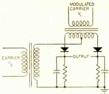
**PHASE-SENSITIVE DEMODULATOR<sup>4</sup>**—Has push-pull output. Input may be from balanced or single-ended carrier. Carrier signal is reference
