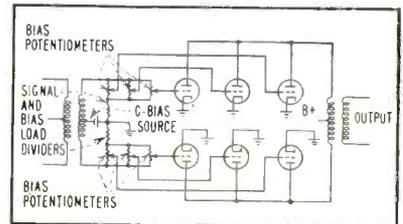
FIG. 4—Power tubes in push-pull parallel with bias adjustment
