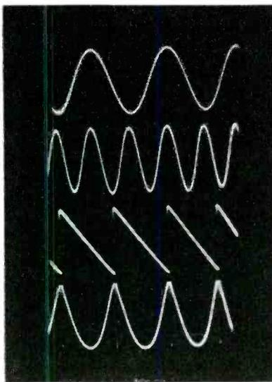
Sine wave (first line) applied to both inputs gives squared waveform (second line). Fourth line is squared version of sawtooth shown in third line
