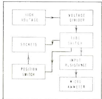
FIG. 1—A node current checker for phototubes used in Navy equipment
