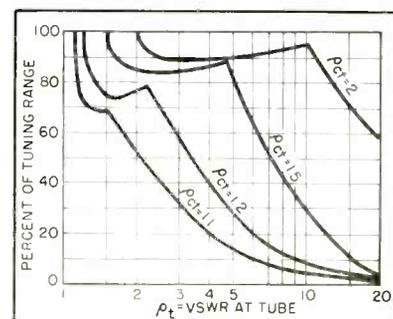
FIG. 6—Percent of tuning range accessible to continuous-wave oscillators when tube is tuned both ways
