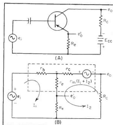
FIG. 1—Grounded-emitter transistor amplifier (A) and low-frequency equivalent circuit (B)
