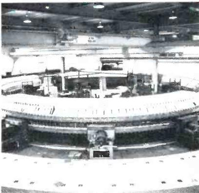
Brookhaven Cosmotron's 2432 magnet grid bars, operating in high vacuum, are "gapped" and insulated with "Kel F" plastic.
