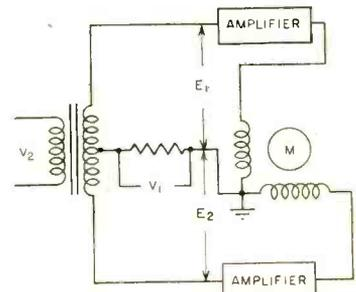
**SERVO MOTOR PHASE DETECTOR**— Phase detection is accomplished in two-phase motor. Output is a mechanical torque of reversible polarity.  $E_1 = V_1 + V_2$ ,  $E_2 = V_1 - V_2$
