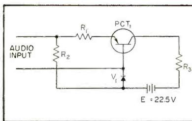
FIG. 5—Equivalent of oscillator circuit at d-c and audio frequencies
