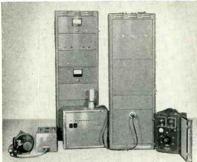
Microsecond flash equipment with high-speed camera at left. Pulse generator supplies triggering pulses for series of ten flashes
