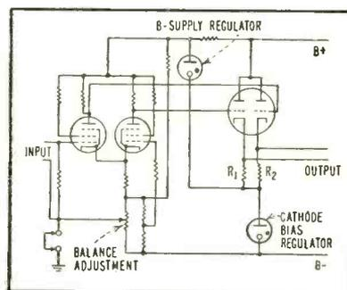
FIG. 5—Regulator tube is used in cathode-follower for bridge amplifier
