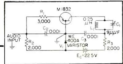
FIG. 1—Complete circuit diagram of vhf f-m transmitter capable of being picked up at several hundred feet when modulated with crystal phonograph pickup
