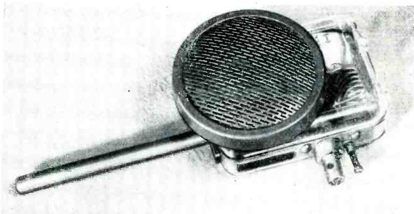
Transmitter containing extra transistor audio stage for use with crystal microphone. At left is lapel microphone model, and at right is hand microphone design in which microphone is mounted directly on transmitter housing
