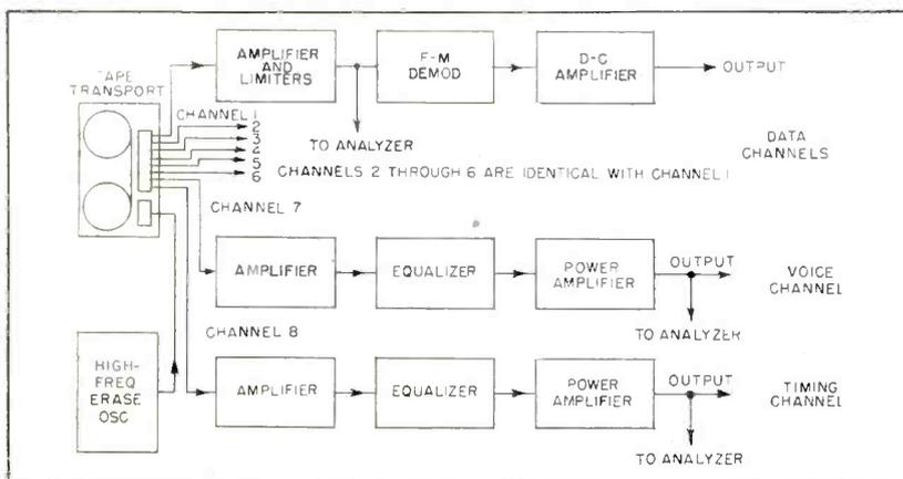
FIG. 2—Arrangement of reproducing equipment used at laboratory
