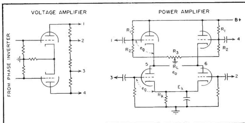
FIG. 2—Basic circuit diagram of transformerless amplifier
