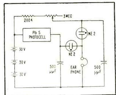
FIG. 1—Two neon-tube relaxation oscillators are initially tuned to same frequency so that discontinuity in reflected light shows up as beat frequency. Effect is caused when light variations produce small variations in cell resistance
