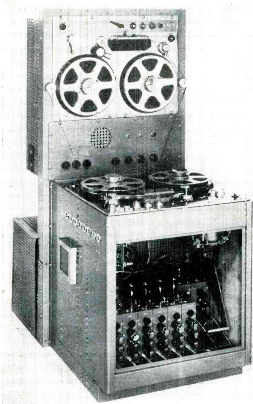
Reproducing equipment, with analyzer mounted on vertical rack at rear
