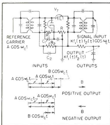
FIG. 3—Basic circuit of phase sensitive detector and output signal vectors
