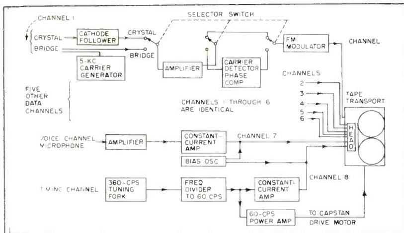
FIG. 1—Block diagram of eight-channel magnetic tape recorder
