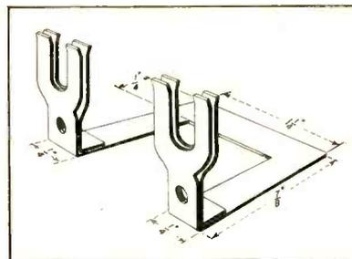
FIG. 1—Mounting bracket for two pencil triodes is grid-feed back loop
