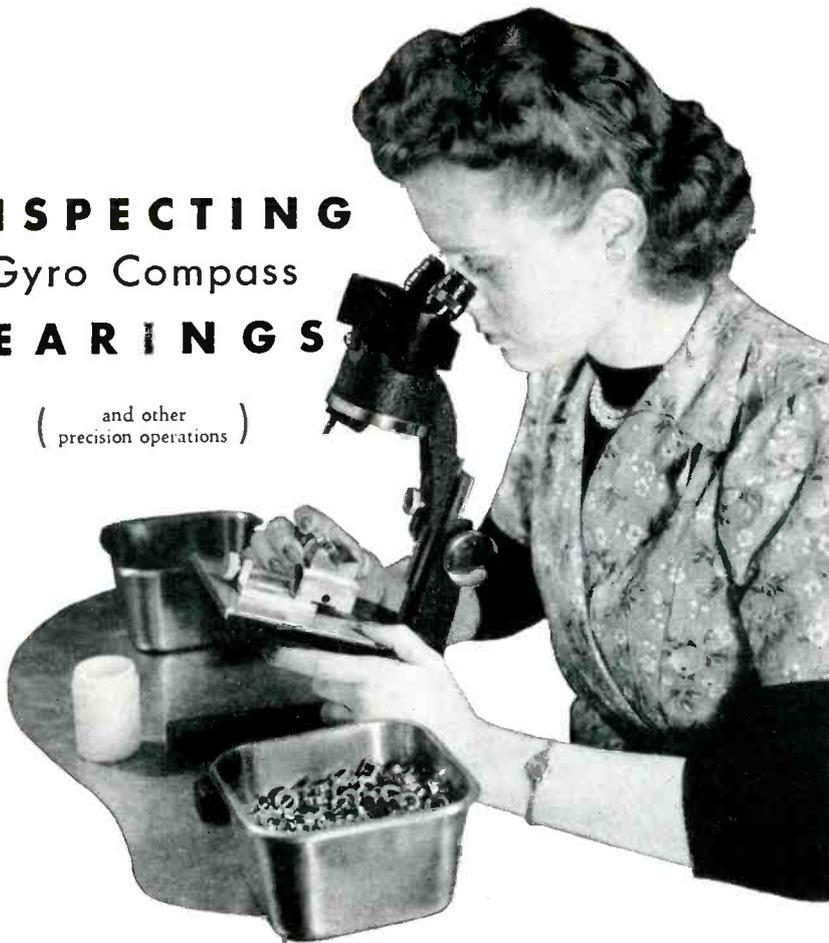
MARK IV GYRO COMPASS Bearings demand the most precise methods of fabrication and inspection — including the use of AO Stereoscopic Microscopes with special jigs.
