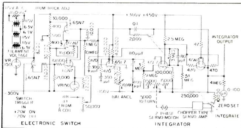
FIG. 3—Integrator and electronic switch provide voltage analog of magnetic field strength variation. Integrator uses Miller feedback circuit with d-c amplifier
