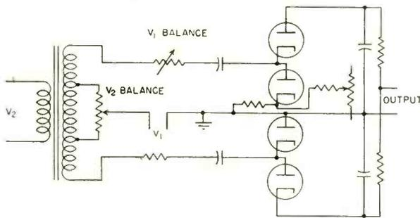
**R. L. FRANK PHASE COMPARATOR<sup>20</sup>**— Insensitive to the third and all even harmonics of both input voltages. Combines two 120-degree-conduction cascade doubler circuits
