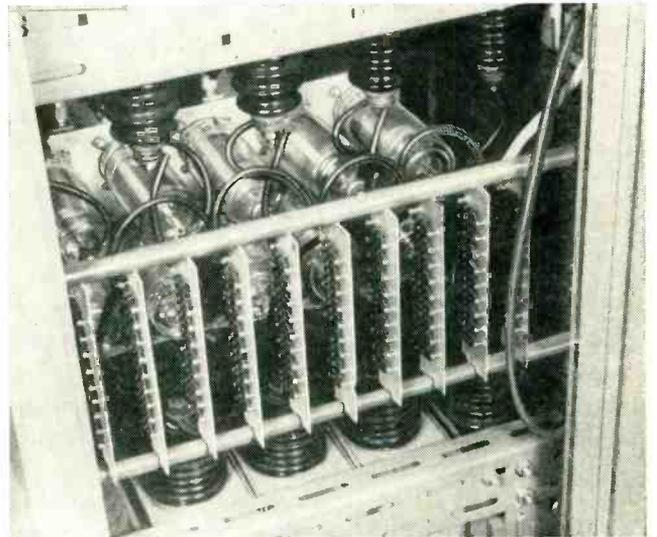
Thyratrons of pulser unit connect energy storage capacitors at bottom if picture across light source when triggered by counter circuit
