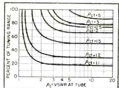
FIG. 3—Percent of tuning range accessible to pulsed magnetrons
