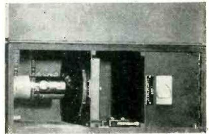
FIG. 2—Black box with end-on tube under test. Proper luminous flux is obtained by interposing different area apertures between light and photocathodes
