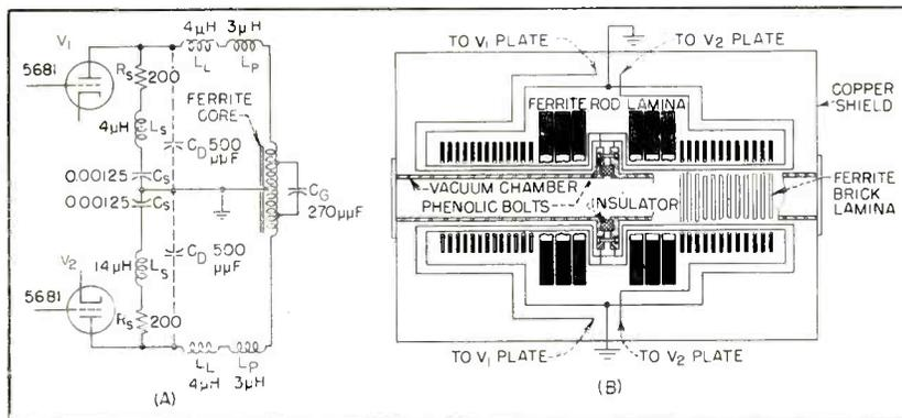
FIG. 8—Power-output system of r-f generator; push-pull 5681 triodes operating in class  $A_2$  deliver 100 kilowatts to ferrite-loaded output loop
