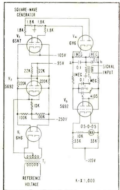
FIG. 1—Synchronous amplifier combines reference square wave with signal to obtain error voltage across filter circuit
