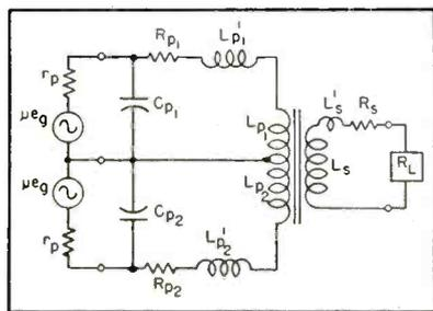
FIG. 1—Equivalent circuit of a typical output transformer illustrates its frequency dependence
