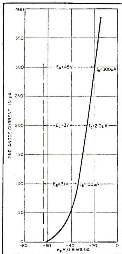
FIG. 11—Unequal signal drive takes advantage of tube curve
