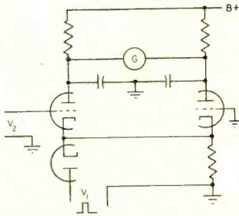
**GATED-CATHODE DETECTOR<sup>8</sup>**— Similar in operation to gated-grid circuit except that pulses are applied to cathodes. Common cathode resistor for all tubes provides nearly push-pull grid-cathode voltages
