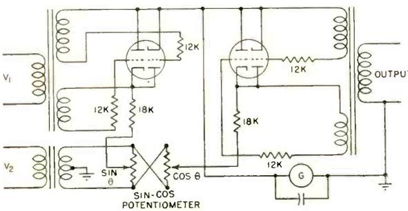
**DOUBLE-CLAMP PHASE DETECTOR<sup>20</sup>**— Used in British omnidirectional beacon. A 200-pps signal is applied to sine-cosine potentiometer as a reference signal. Output is indicated on a zero-center course meter
