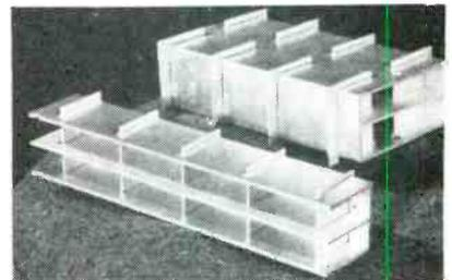
Complicated microwave component produced with high accuracy by dip brazing of stainless steel pieces
