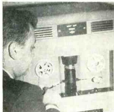
Microfilmed documents previously marked are read off by flying-spot scanner in new technique developed for computer input
