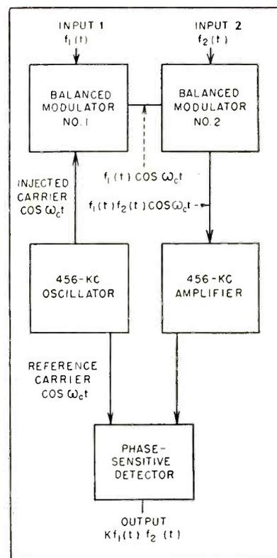
FIG. 1—Block diagram of multiplier
