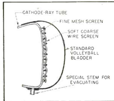
Technique used for cementing fine mesh screen to face of cathode-ray tube
