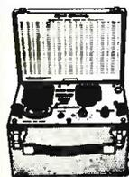
Model TS-127/U is a compact, self-contained, battery powered, precision (±1 Mc) frequency meter which provides accurate readings. Requires a standard 1.5V "A" and 45V "B" battery. Has 0-5 Min. time switch. Contains sturdily constructed Hi-Q resonator with average "Q" of 3000 working directly to detector tube. Uses 957, 1S6 and 6S4 Tubes. Complete new with inst. book, probe and spare set of tubes. Less batteries \$47.50
