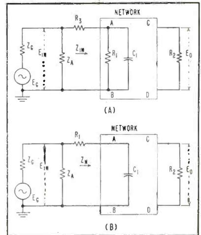
FIG. 3—Circuit for measuring frequency response (A). Circuit (B) is used when resistance of  $R_1$  may vary over test range
