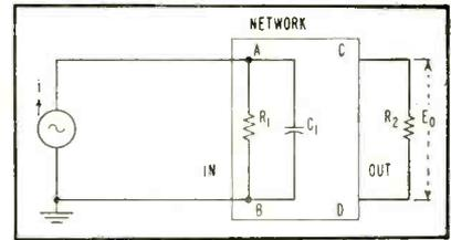
FIG. 1—Network driven by constant-current source
