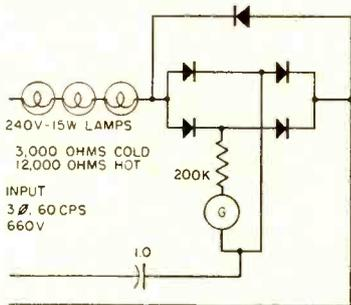
**LIVINGSTONE PHASE-SEQUENCE INDICATOR<sup>6</sup>**—A fifty-to-one voltage change will cause a four-to-one change in the meter indication
