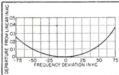
FIG. 7—Departure of frequency deviation from linear with alpha-cut-off
