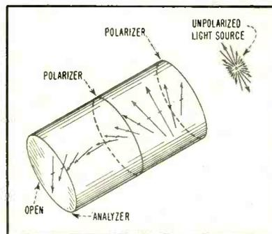
FIG. 1—Rotational effect of two polarizers and an analyzer
