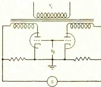
**COSENS PHASE-SELECTIVE BRIDGE<sup>7</sup>**—Triode amplification provides high sensitivity. Output proportional to phase angle divided by  $V_1 V_2$
