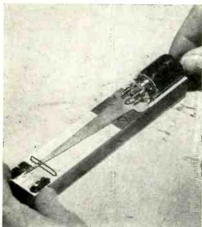
A V-BLOCK and a small pivoted indicator constitute a simple and efficient means of measuring the amount in degrees by which the bottom of a subminiature tube is off square from the plane of the tube. The tube is placed in the machined V of the metal block and
