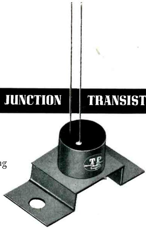
Transistor Products, Inc. is now offering the first commercially available Power Junction Transistor. Specifically designed for use in Class B audio circuits requiring two watts of power output, it can also be used as a Class A amplifier at reduced ratings.
