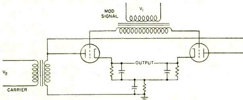
**BALANCED-TRIODE DEMODULATOR<sup>15</sup>**— Push-pull modulated signal is applied to grids. Unmodulated carrier is used as reference and to supply plate voltage. Output is push-pull error signal
