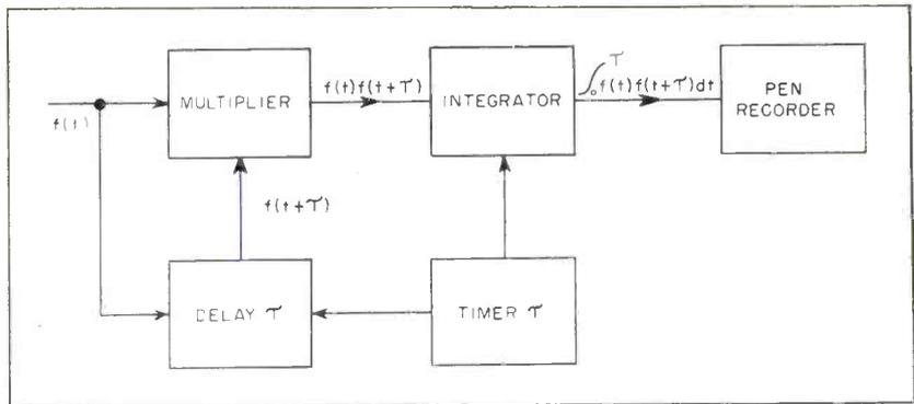
FIG. 4—Block diagram of circuit for obtaining autocorrelation of a function
