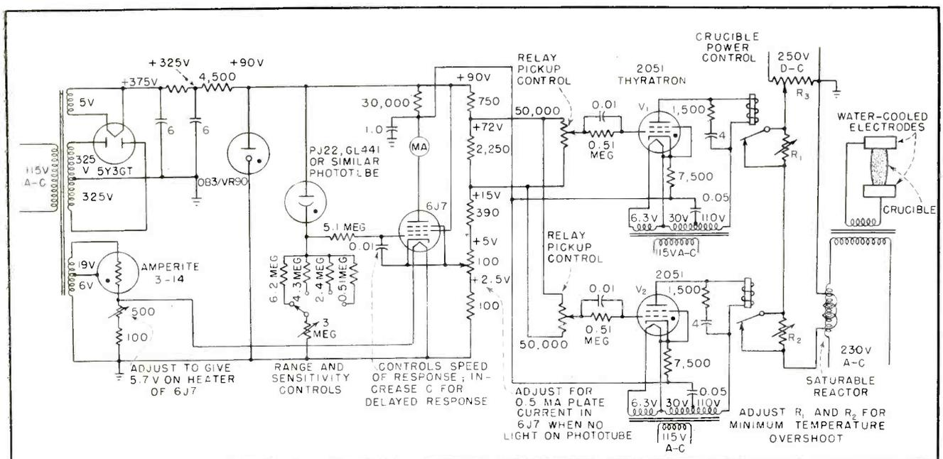
FIG. 1—Complete circuit of stabilized photoelectric amplifier as used for two-point control of temperature in graphite crucible
