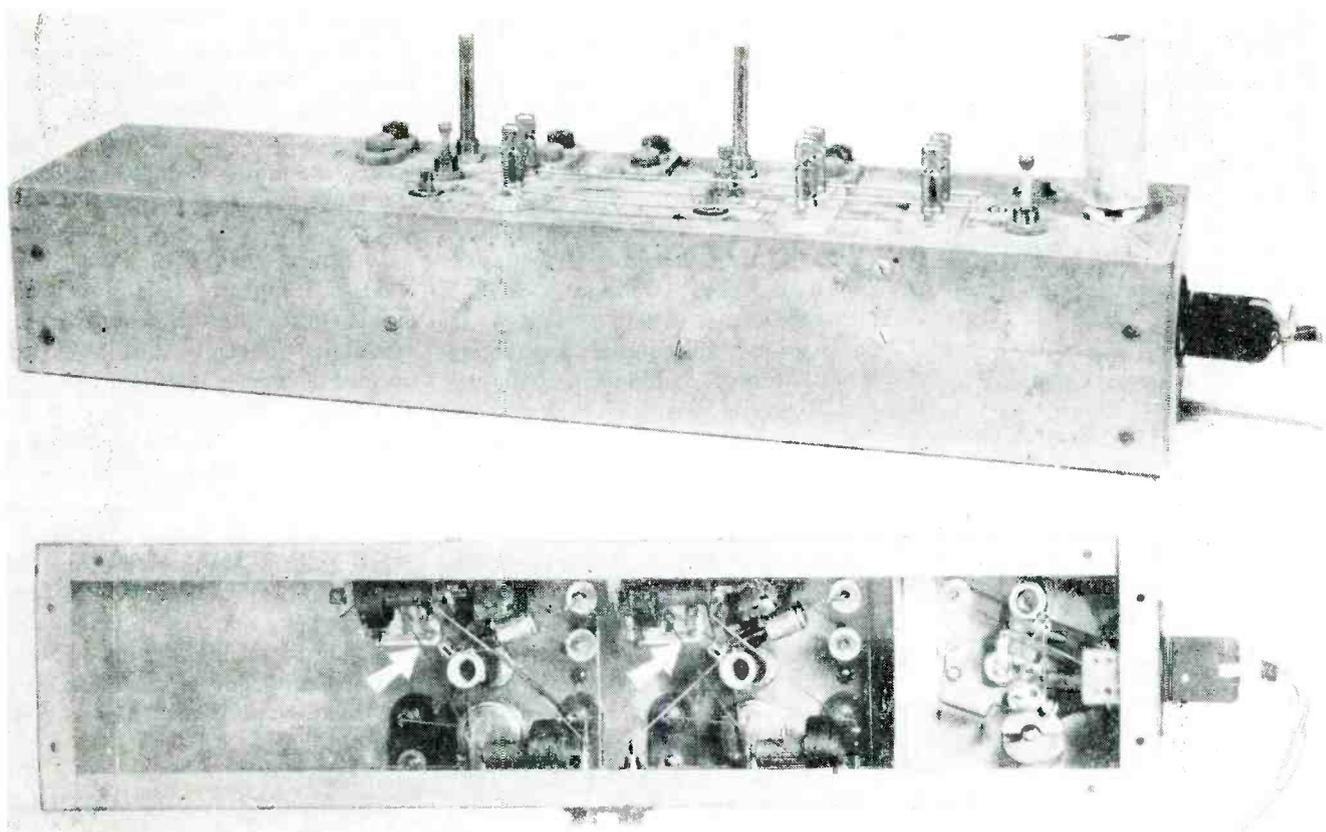
Top and bottom views of cascaded two-stage dielectric amplifier, with 6AQ5 carrier-source oscillator at right end of chassis. Arrows point to the variocaps under the chassis. Extra input and output terminals and controls are provided here for experimental purposes
