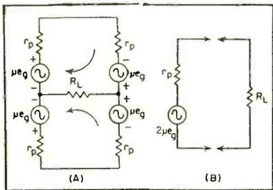
FIG. 3—Equivalent circuit of amplifier
