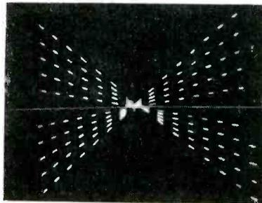
Product of sawtooth and different amplitudes of 500-cps square wave
