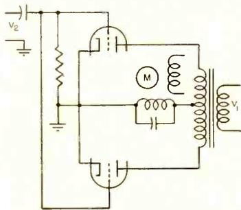
**BROWN DISCRIMINATOR<sup>9</sup>**—Basic circuit for electronic potentiometer. Modification of Cosens circuit for use with two-phase a-c servo motor
