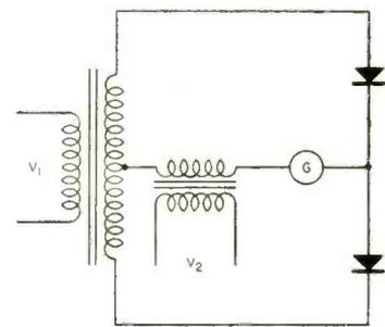
**WALTER PHASE-SELECTIVE RECTIFIER<sup>1,2</sup>**—Gives square-law response, with sensitivity decreasing near balance point. Meter reads zero if  $V_1$  and  $V_2$  are 90 degrees out of phase
