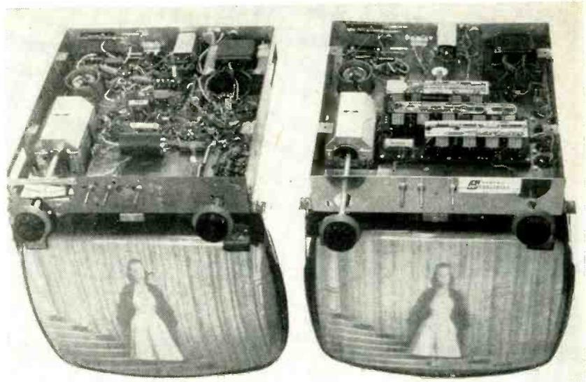
NEARLY 600 hand-soldering operations are eliminated and production and material costs are reduced as . . .
