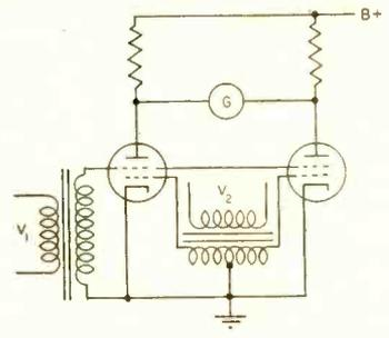
**MORTON SCREEN-GRID PHASE DETECTOR<sup>13</sup>**— Reference voltage  $V_2$  is applied to control grids and variable voltage  $V_1$  is applied to screens. System puts light load on power supply of variable phase
