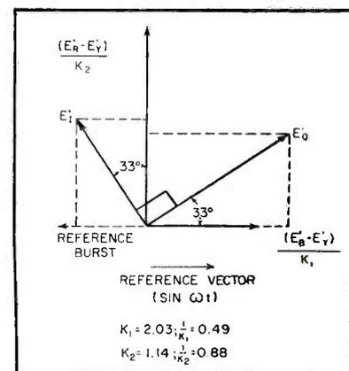
FIG. 13—Relationship between  $E'_r$ ,  $E'_0$  and color difference signals
