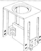
A parallelogram suspension confines the mass of the GLH to a virtual straight line motion and provides excellent lateral rigidity.
