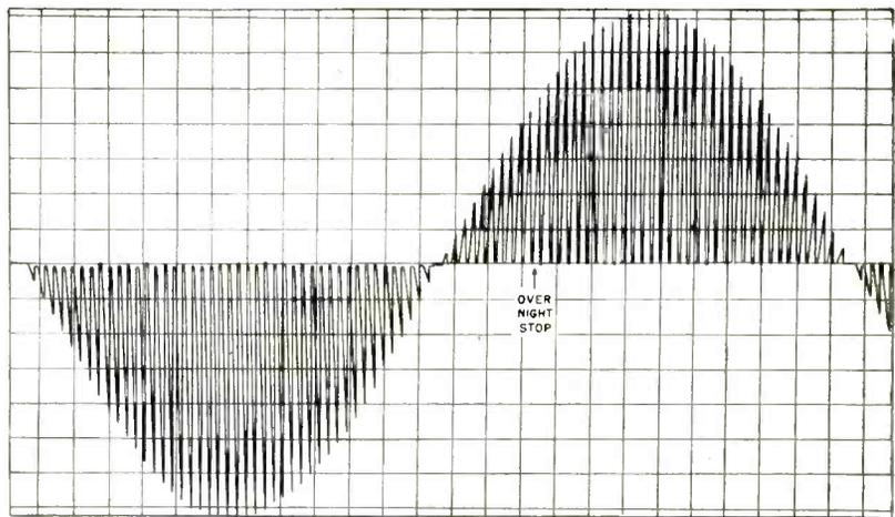
Autocorrelation of sine wave. Stability of equipment is indicated by absence of discontinuity at point where machine was turned off for sixteen hours
