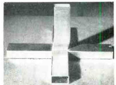
Completed waveguide junction, showing small fillets achieved through proper design for dip brazing
