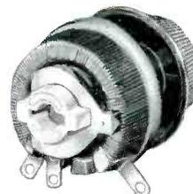
Opens the rheostat circuit at the high or low resistance position. The circuit is opened as the brush snaps into an insulated notch next to the lug, providing indexing.
