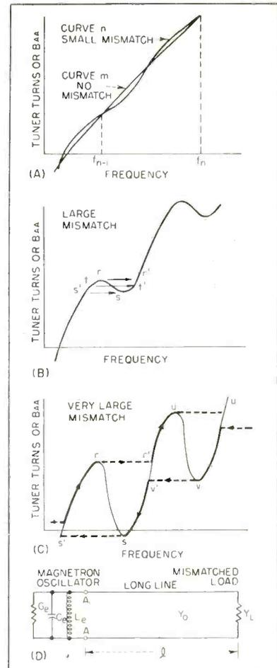
FIG. 1—Tuning curves of radar magnetron oscillator connected to long mismatched transmission line, and equivalent circuit for load mismatch
