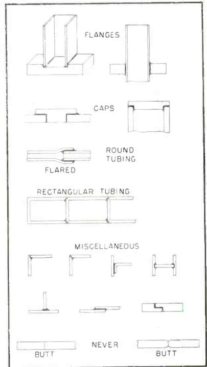
Typical joint designs used with dip brazing of microwave plumbing
