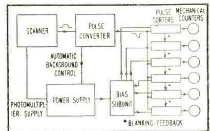
FIG. 1—Block diagram of the stain counter uses spiral scanner
