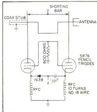
FIG. 2—Crystal in cathode circuit of f-m transmitter applies modulation
