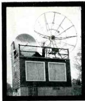
Highly Directive, high power (20-watt) transmitter with 18-ft. parabolic antenna, furnishes signal source.
