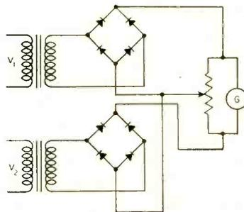
**DOUBLE-BRIDGE PHASE DETECTOR**— Used in CAA landing system as part of crossed-pointer indicator
