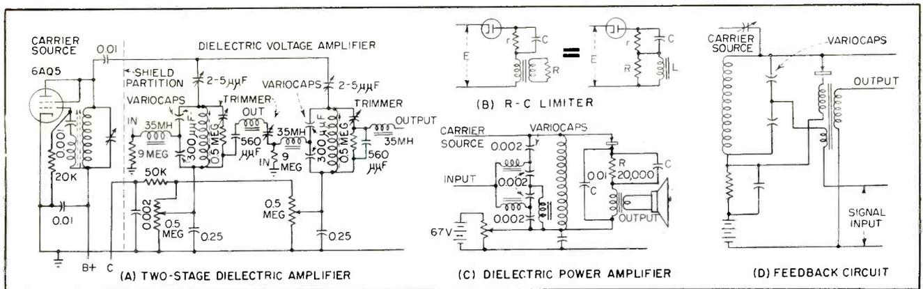
FIG. 3—Examples of dielectric voltage and power amplifier circuits using carrier sources. These circuit techniques are also adaptable to the small capacitance value used in vhf f-m oscillators. Mathematical derivations and further details are given in the original NBS reports by the author, 13.4-74R and 13.4-102R, available from the NBS Technical Reports Section
