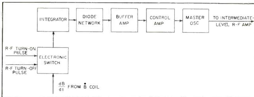
FIG. 2—Block diagram of frequency-control system illustrates how feedback from cosmotron magnet controls r-f generator frequency
