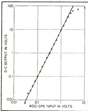
Amplitude range of input functions over which true product is obtained
