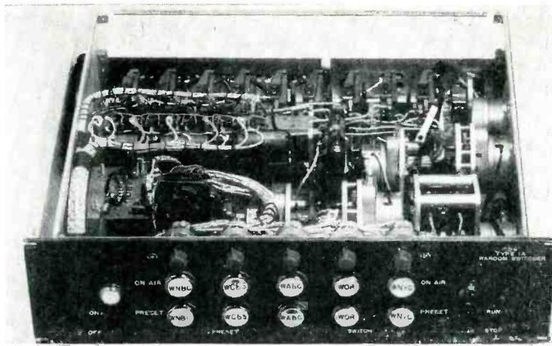
Equipment in use at New York makes provision for control of five broadcast stations, but circuits can be modified for additional transmitters
