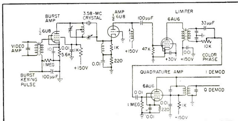
FIG. 15—Crystal filter and associated circuits for color sync
