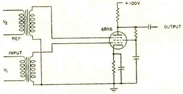
**GATED-BEAM PHASE DETECTOR<sup>14</sup>**— Plate current is at maximum for in-phase operation, and at a minimum for 180-degree phase difference
