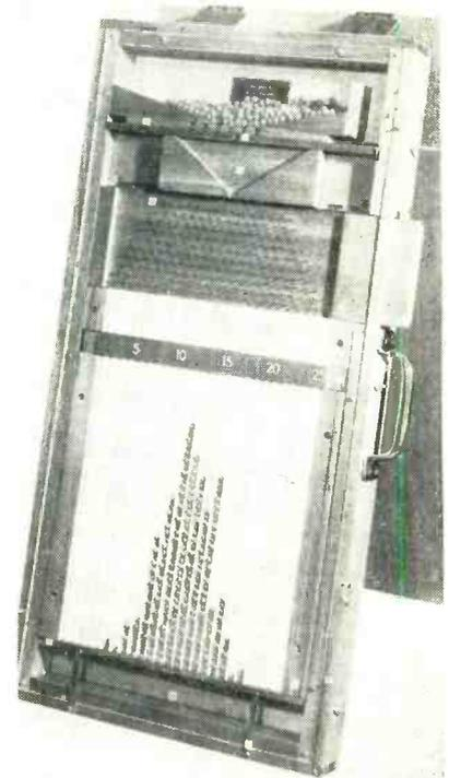
Quality control distribution pattern demonstrator. Nails must be somewhat irregular and balls should vary slightly to get most effective demonstration. Poor results would be obtained by using steel ball-bearings and precisely driven phonograph needles as pegs
