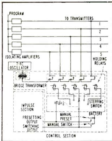
FIG. 1—Switching tone is superimposed upon one of five transmitter lines
