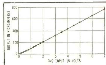
FIG. 2—Linearity of cathode-follower voltmeter circuit is shown in graph
