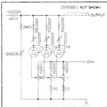
FIG. 4—Diode network converts voltage waveform from integrator to corresponding oscillator control signal
