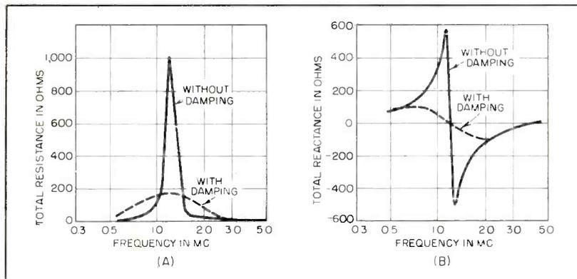
FIG. 9—Impedance of ferrite core with and without series resonant damping
