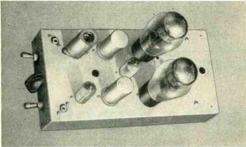
View of transformerless amplifier including preamplifier
