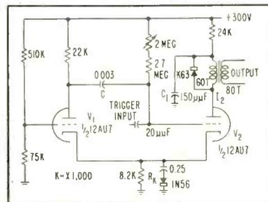
FIG. 2—Circuit of multivibrator cathode-shunt diode and plate-shunt capacitor to extend delay time
