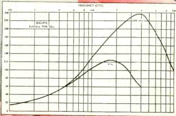
PLUG-IN DECADE COILS CAN ALSO BE DESIGNED WITH SPECIAL CHARACTERISTICS FOR SLIGHT EXTRA CHARGE. LIMITS GENERALLY AVAILABLE FROM STOCK ARE AS FOLLOWS:
