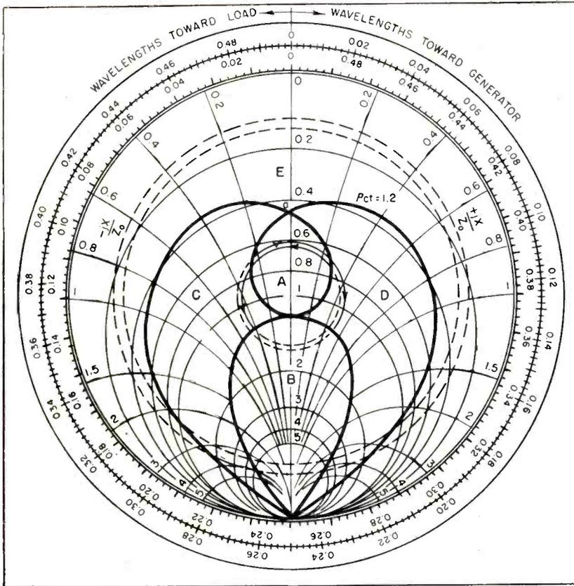
FIG. 4—Example of frequency-jumping behavior of a continuous-wave tube
