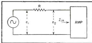
FIG. 3—Circuit used in measuring input impedance of transistor amplifier
