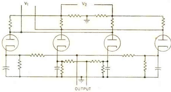
**FULL-WAVE DEMODULATOR<sup>15</sup>**— Push-pull inputs and output. Inputs are carrier-balanced. Signal  $V_1$  is compared to unmodulated carrier signal  $V_2$
