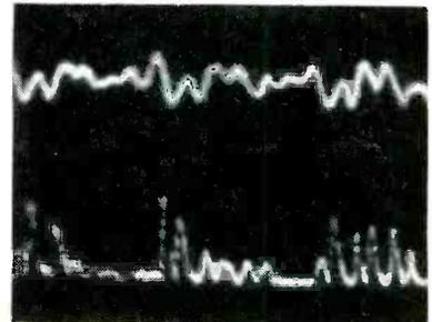
Lower waveform is square of complex waveform shown above
