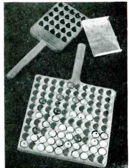
Closeup of paddles used in sampling simulator, with metal slide for covering rows of holes not wanted
