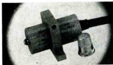
satisfies the needs of piezoelectric accelerometers, force gages and pressure pickups. Model 2608 cathode follower is internally shock-mounted and uses the latest of design techniques, including etched wiring, subminiature shock resistant tubes and tantalitic capacitors. The small size permits installation in cramped quarters. Input impedance is over 100 megohms.
