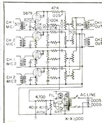
FIG. 2—Preamplifier-mixer unit
