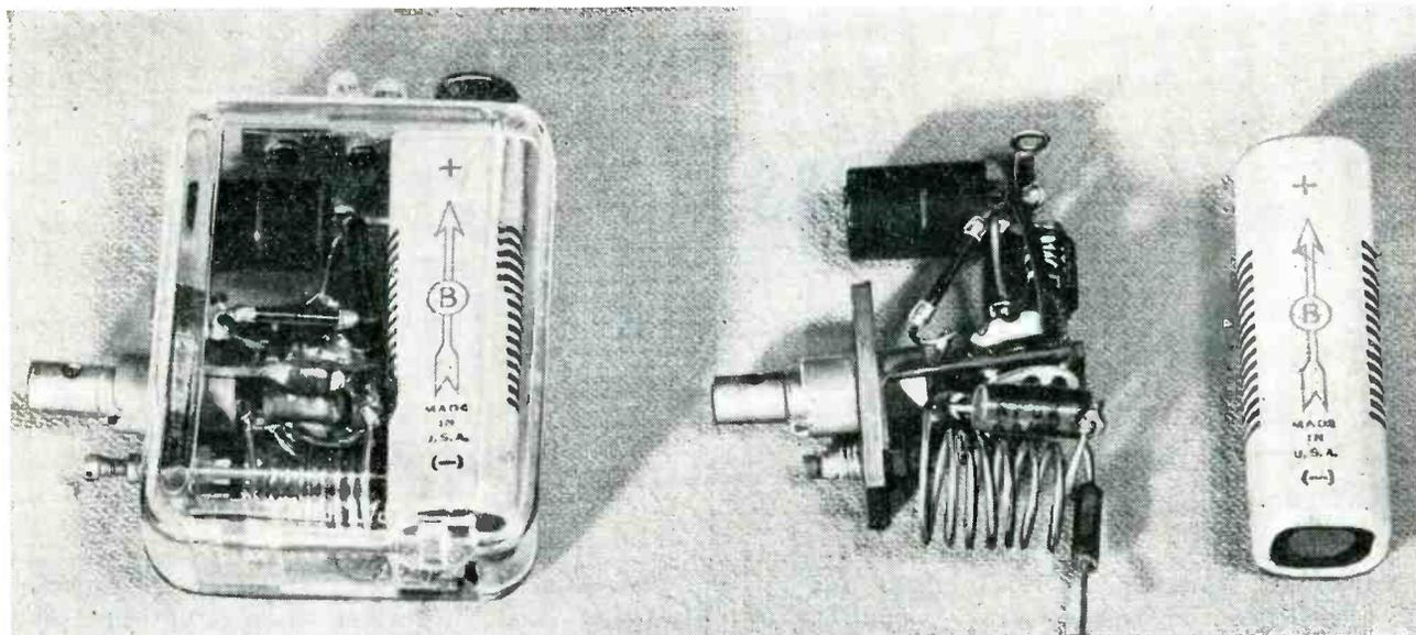
Actual-size photograph of assembled transmitter is shown at left and transmitter and battery with case removed (right)
