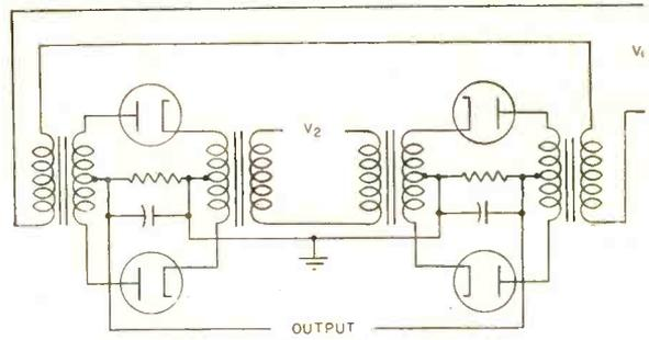
**WARD-LEONARD SYSTEM DETECTOR<sup>18</sup>**— Commercial variation of full-wave demodulator system. Output is used to control d-c motor through d-c amplifier
