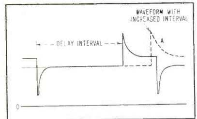
FIG. 1—Voltage between cathode and ground in monostable multivibrator showing effect of increasing delay time
