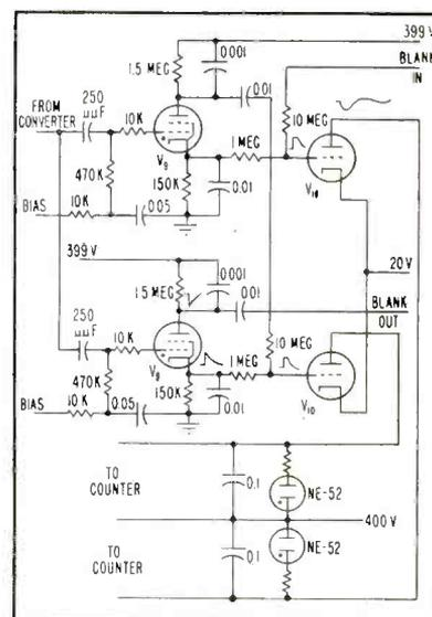
FIG. 3—Pulse sorter and counter outputs are handled in this stage by the thyatron circuits shown
