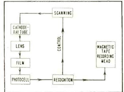
FIG. 1—Flying spot scanner and computer-input tape recorder
