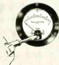
All Weston Ruggedized instruments have externally operated sealed zero correctors.
