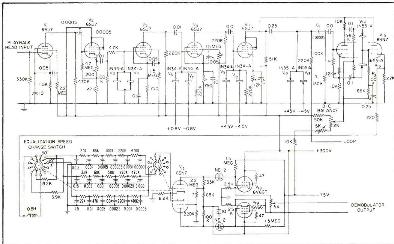
FIG. 6—Playback amplifier and demodulator for f-m channels. A separate channel amplifies voice and timing signals
