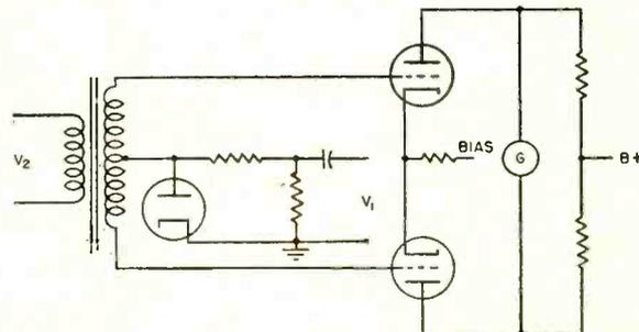
**GATED-GRID DETECTOR<sup>8</sup>**—Rectangular reference waveform produced from sinewave  $V_1$  by diode and R-C circuit
