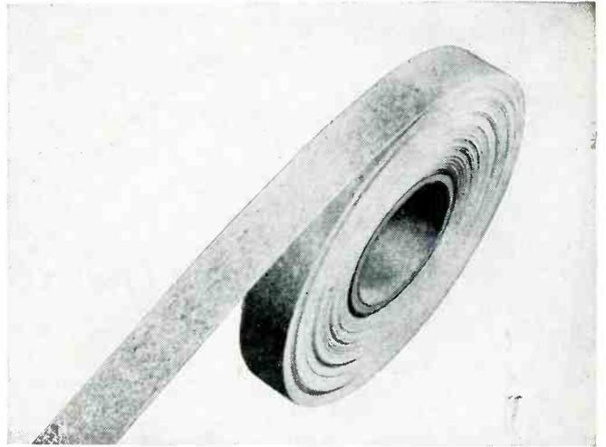
**2. Need a mica tape that can be run on taping machines at high speed?** ISOMICA® tapes are made from long rolls of thin continuous mica sheet... are more uniform in mechanical and dielectric strength... have no high spots or voids. For electrical insulation of class B or class H motors, generators and transformers.
