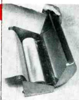
*Loading of the magazine is easy. Processing of paper in varying widths to 12" is handled by simple, adjustable guides.*
