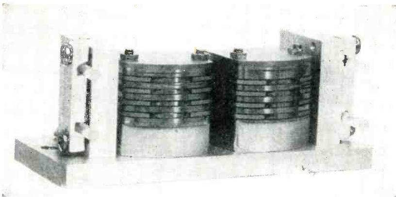
Recorder head assembly, showing staggered arrangement of the eight recording heads
