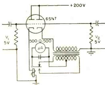
**WALD PHASE INDICATOR<sup>22</sup>**— Has high input impedance. Accuracy is  $\pm 1$  percent. Average output current  $I_{max} \cos \theta/\pi$ . Upper frequency limit is determined by chopper used
