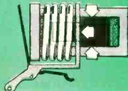
The hydraulic-magnetic principle allows maximum flexibility for special applications, ratings and protective characteristics. Since it does not employ thermal elements, set tripping points are completely unaffected by ambient temperature.
