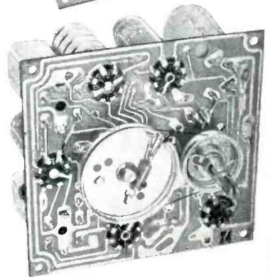
A five tube superheterodyne in volume production utilizing multiple soldering and semi-automatic assembly techniques... an excellent application of printed wiring methods by Raytheon Manufacturing Company.
