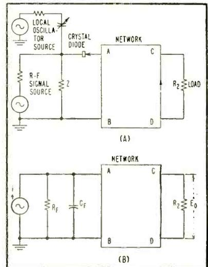
FIG. 2—Hetrodyne mixer circuit (A) and its equivalent (B) at intermediate frequencies
