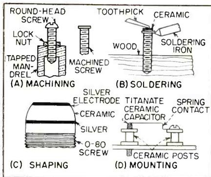
FIG. 1—Construction of variocap components
