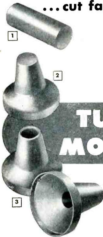
A short molybdenum rod (1) was hot forged to form basic cone (2), and the part (3) was finished by machining and drilling.
