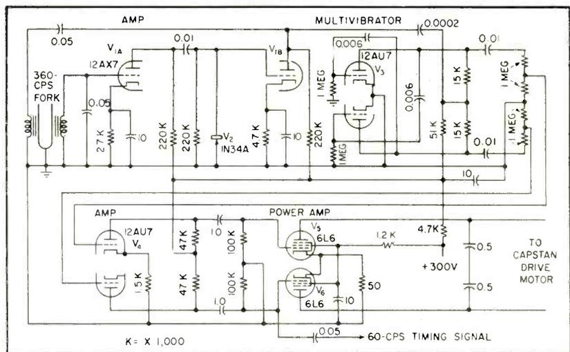
FIG. 5—Method of using tuning fork to generate precise 60-cps power for capstan drive motor and for timing purposes during analysis of the tape recordings
