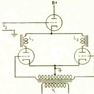
**CATHODE-GATED DETECTOR WITH CURRENT OUTPUT<sup>9</sup>**— Used with d-c servo motor. Coils  $L_1$  and  $L_2$  are split field of servo motor or differential relay. Provides differential current with low output impedance
