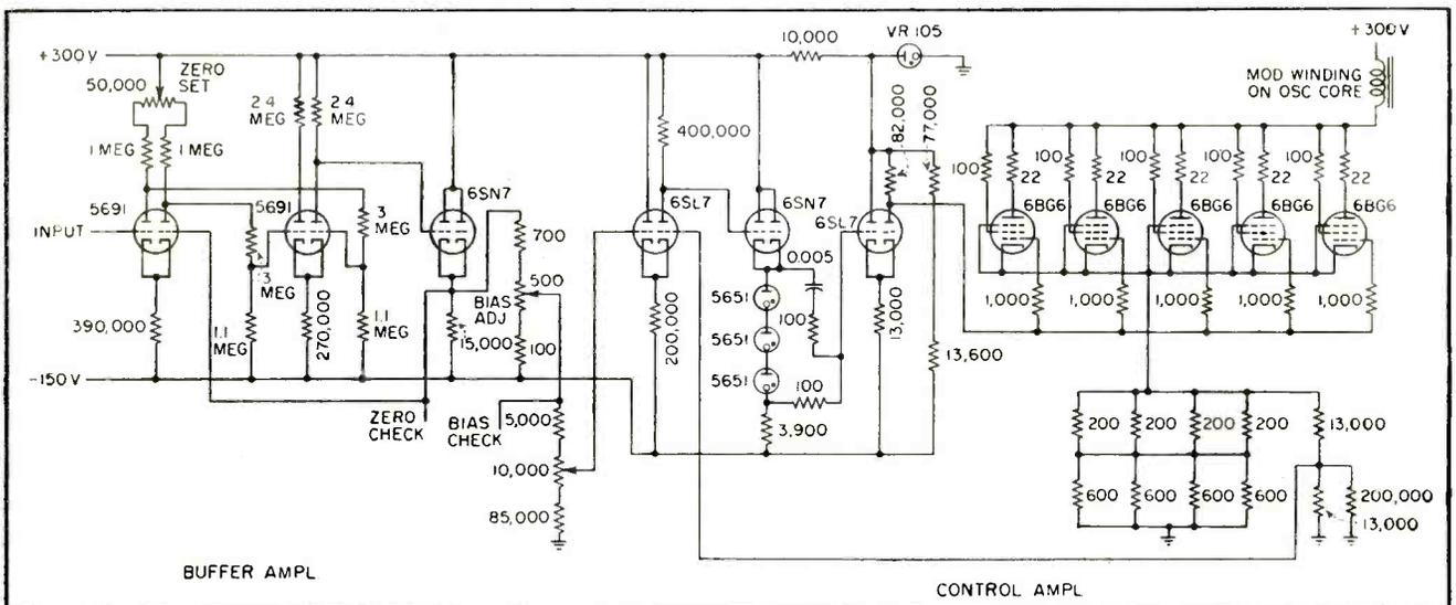
FIG. 5—Control amplifier delivers desired current waveform to control winding on oscillator tuning coil
