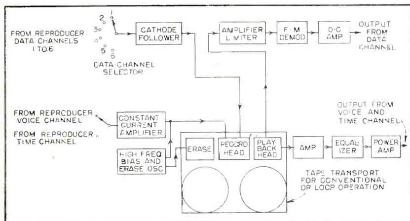
FIG. 3—Two-channel analyzer employed for detailed analysis of recording
