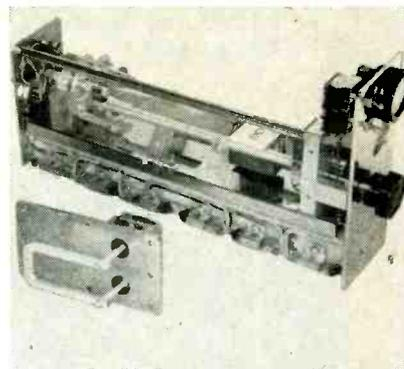
UHF frequency-modulated transmitter uses two pencil triodes in output
