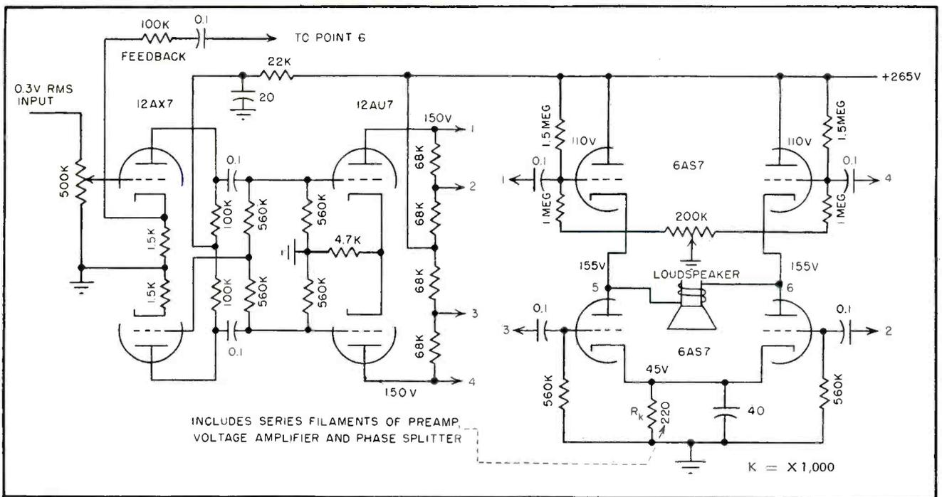
FIG. 5—Complete transformerless amplifier capable of outputs of 8 watts. Bridge-type output circuit matches voice-coil impedance
