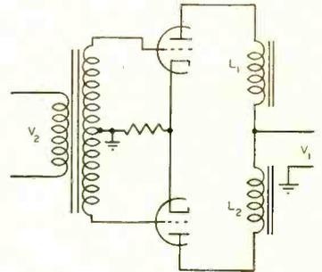
**MODIFIED COSENS BRIDGE DETECTOR<sup>8</sup>**—Applicable to servo control. Coils  $L_1$  and  $L_2$  are differential relay coils or fields of d-c servo motor
