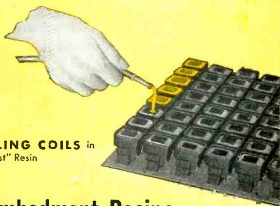
**2 SEALING COILS** in "Scotchcast" Resin
