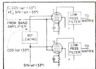
FIG. 4—Arrangement of the I-Q color demodulators in the receiver
