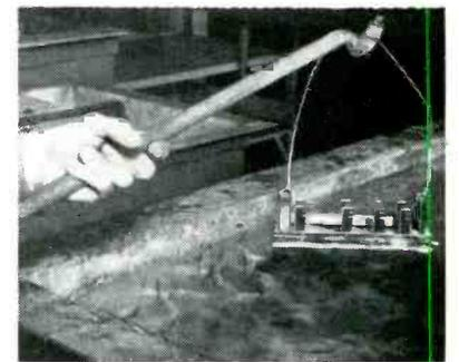
Lowering dip-brazed part into cold water quench, for heat-treatment
