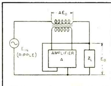
FIG. 1—Basic a-c equivalent circuit of electronic power supply filter
