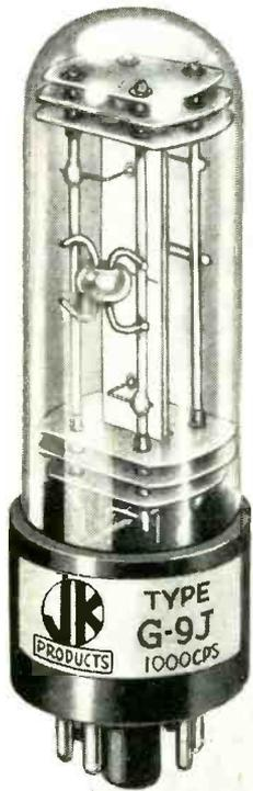
Now, the range of the JK G-9J has been extended to cover 1000 cycles to 10 kc. This provides a convenient source of stable time base for a wide variety of measurement problems, with a minimum of circuitry. Ideal for applications such as compact digital counters in the audio range. Balanced nodal-point mounting minimizes microphonics found in other resonators in this frequency range. Write for application and engineering information.
