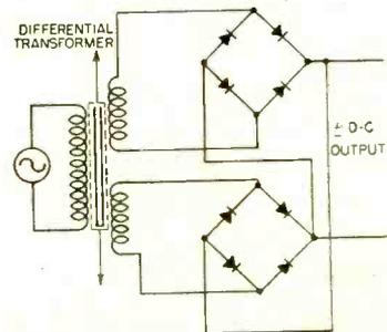
**DENSITROL RECTIFIER BRIDGE<sup>18</sup>**— Core of differential transformer is actuated by float
