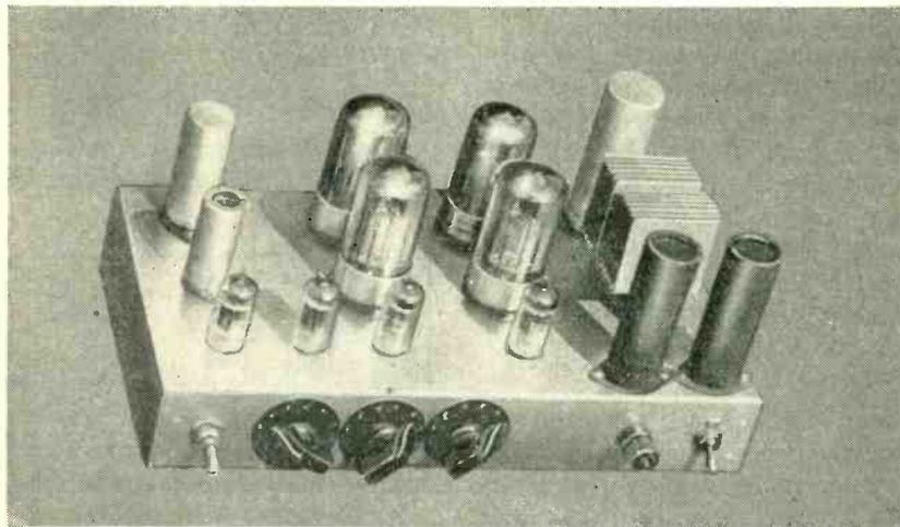
Chassis of 18-watt amplifier includes preamplifier and power supply
