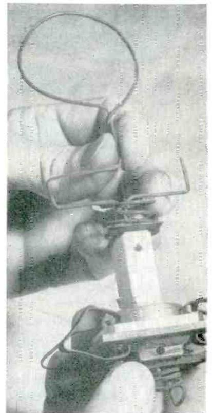
Waveguide flange assembly fixture consisting chiefly of wire springs and stainless steel spring clamps. Wire loop at top serves for placing assembly in pre-heating furnace and later suspending it in dip pot
