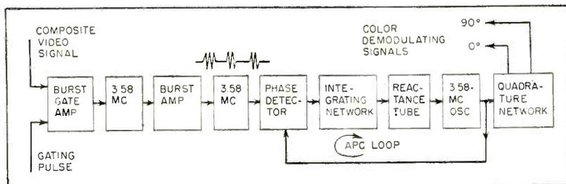
FIG. 16—Block diagram of automatic phase control circuit for color sync
