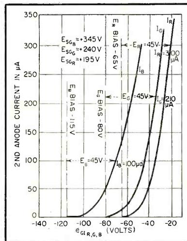
FIG. 10—Equal signal drive for color balance in one type of operation
