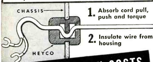
1. Absorb cord pull, push and torque
