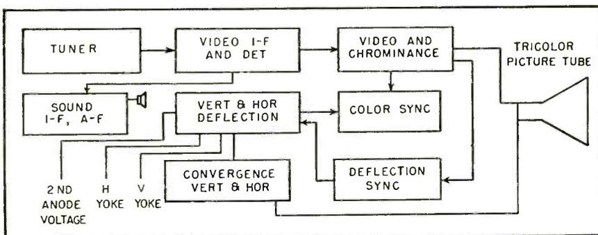
FIG. 1—Stages of basic receiver, emphasizing sections handling color signals
