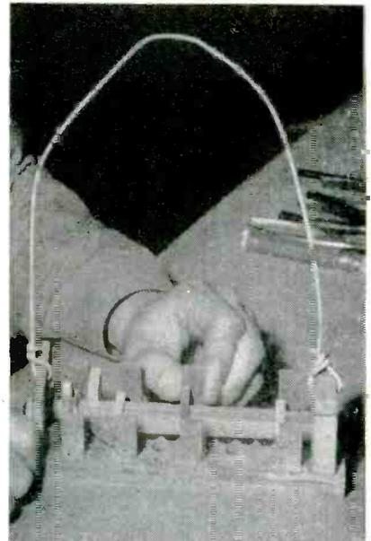
Fixture used to hold close tolerances on a small aluminum microwave antenna during dip brazing. Flat springs on fixture are made from stainless steel
