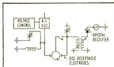
FIG. 1—Radio-frequency oscillator and detector system used for grading eggs
