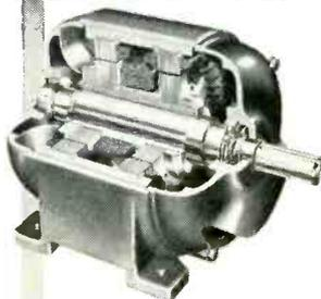
Here's how the American Electric Inductor Alternator is built. Note all windings are stationary. Output is taken directly off stationary windings. Even the excitation is fed to a stationary winding (center coil)!
