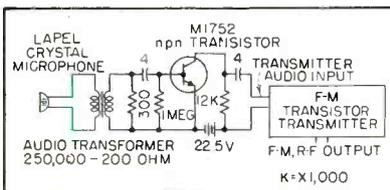
FIG. 8—Audio amplifier added to circuit of Fig. 1 for crystal microphone
