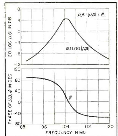
FIG. 4—Magnitude and phase of  $\mu\beta$  in oscillating frequency region
