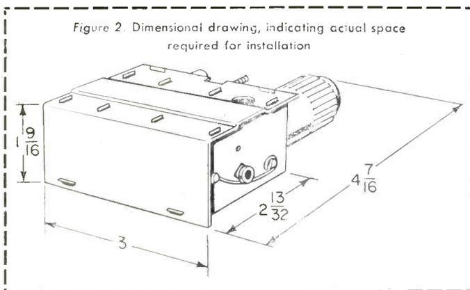
Solder tab terminals are provided for connection to a 300-ohm balanced antenna feed, and to heater and "B+" power supply. Trimmer capacitances are readily accessible on the same side of the chassis as the tube. Output impedance is nominally 50 ohms. The tuning shaft rotation can be either clockwise or counterclockwise, as desired.
