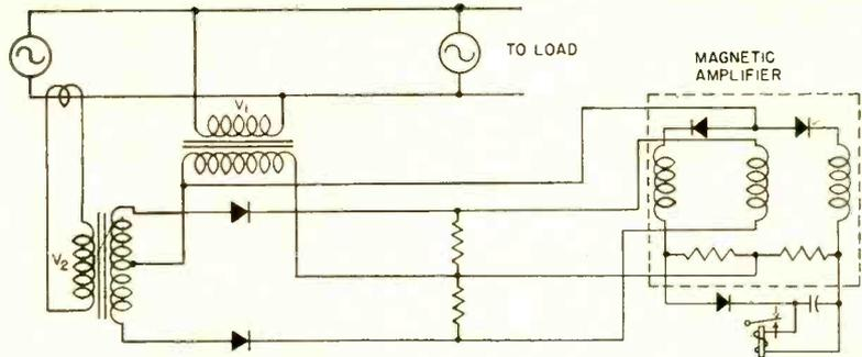
**MAMON PHASE DISCRIMINATOR<sup>5</sup>**—Uses balanced, polarized magnetic amplifier to boost output of phase-selective detector. Application shown is used to operate relay to disconnect alternator in case of field-excitation failure, loss of synchronization or drive failure
