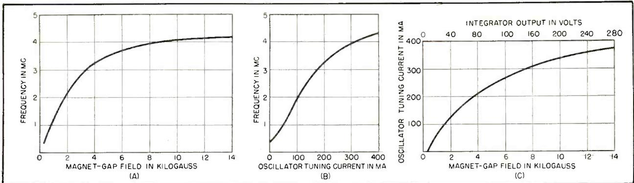
FIG. 1—How r-f generator frequency tracks cosmotron's magnetic field. Desired frequency vs field strength characteristic (A) is achieved by using voltage analog of magnetic field-strength variation to control oscillator tuning current
