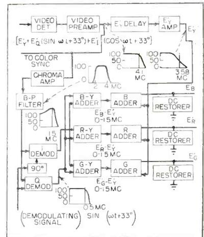
FIG. 3—Video system for ceiling-performance receiver
