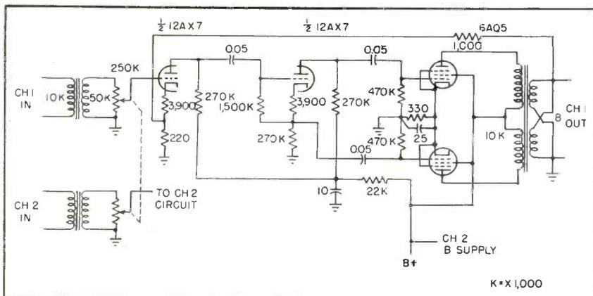
FIG. 3—Monitor amplifier furnishes 10 watts to each of two wall-mounted speakers
