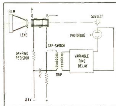
FIG. 2—Basis of a single-element magneto-optical shutter
