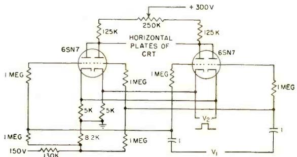
**SCR-615 PHASE-SENSITIVE AMPLIFIER<sup>16</sup>**— Radar application with cathode-ray tube display. Cathodes are gated by sine-wave generator. Reference voltage comes from two-phase generator synchronized with antenna
