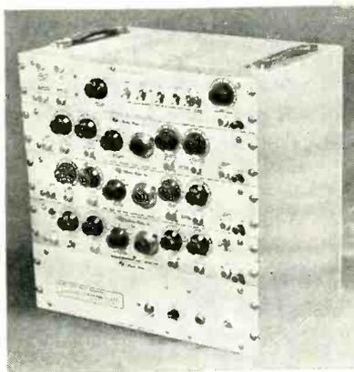
the main pulse is 80 v maximum across an internal 93 ohm resistor and may be continuously varied within 10-db steps. Pulse width is variable from 0.1  $\mu$ sec to 1,000  $\mu$ sec in four ranges and flatness of the pulse top may be adjusted to within 2.0 percent on all ranges. Block-unitized circuitry and construction allows use of the instrument as an independent frequency source and cascaded or parallel time-delay generator, among other applications.
