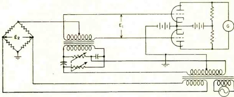
**BRIDGE-BALANCE DETECTOR<sup>10</sup>**—Current in meter is proportional to  $E_1 E_2 \cos \theta$ . By adjusting phase of  $E_1$ , output current can be made dependent on only the reactive or resistive component of either voltage. Phase is adjusted by dual potentiometer in phase shifting circuit
