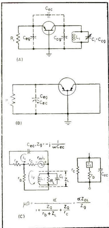
FIG. 2—High-frequency equivalent circuits of transistor oscillator
