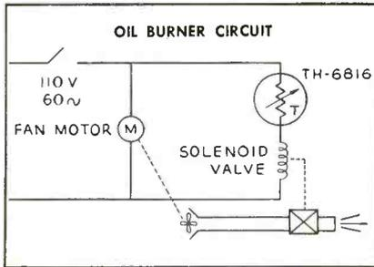
**Carboloy® Thermistors** in the electrical control of an oil burner, delay opening of solenoid valve until combustion chamber is ready to receive properly aerated oil. A mechanical timer was eliminated, and the cost of the unit reduced.
