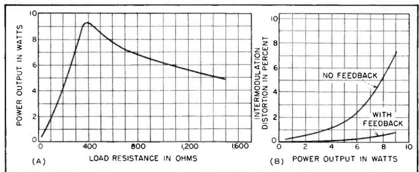
FIG. 6—Curves show output versus load (A) and distortion (B)
