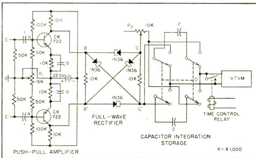
FIG. 1—Bioelectric integrator includes push-pull voltage amplifier using two pnp junction transistors with base input
