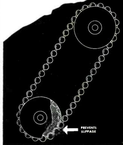
Because of its unique characteristics, Bead Chain is frequently employed by alert designers to make a simple, low-cost and highly efficient sprocket drive. Ideal for many products, it has been proved on business machines, television tuners, venetian blinds, etc. Slippage is absolutely prevented as each bead fits into an individual pocket.
