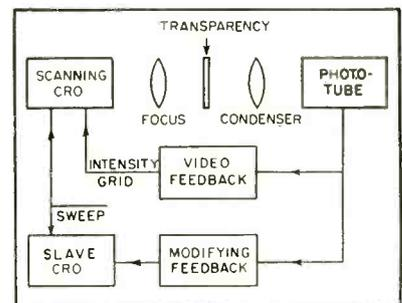
FIG. 1—Image feedback system produces desired type pattern on slave oscilloscope
