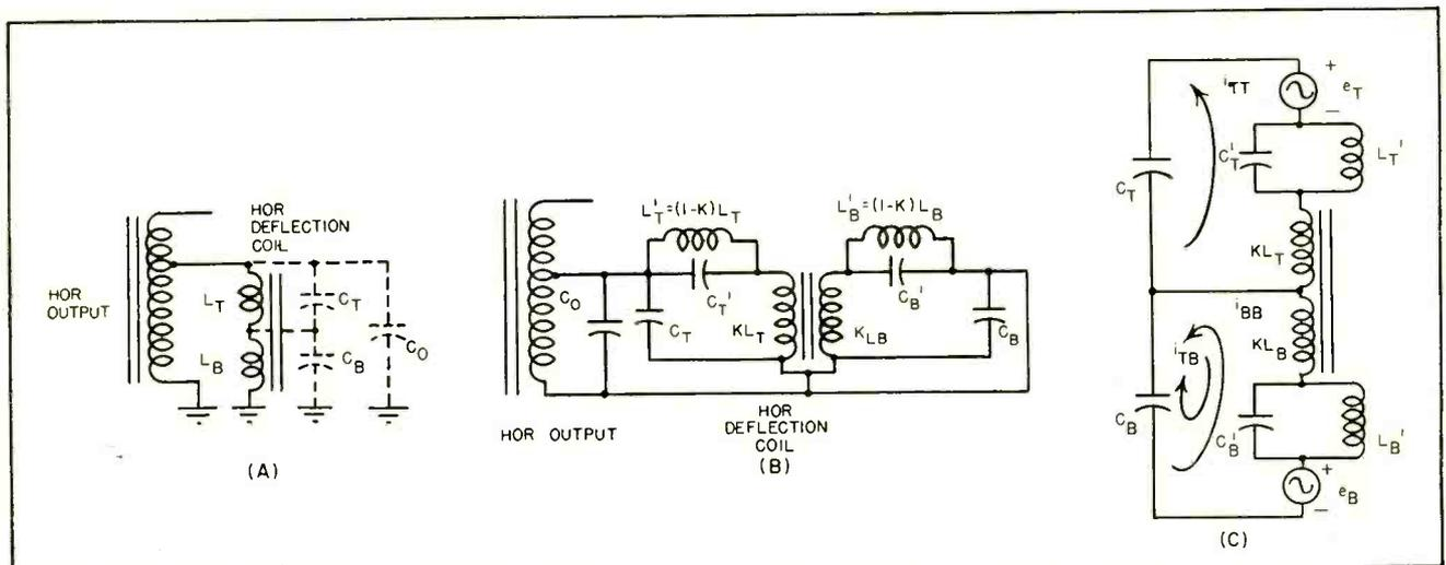
FIG. 1—Simple circuit of horizontal-deflection coil (A) is redrawn (B) to show leakage tuned circuits. Equivalent circuit (C) illustrates how coil balancing cancels ringing currents
