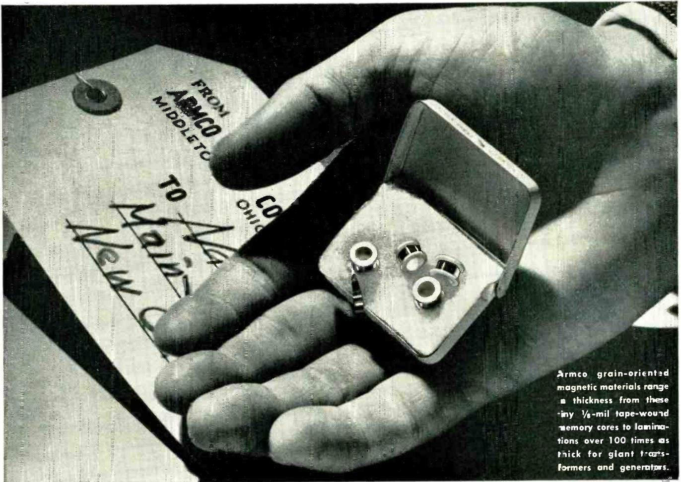
Armco grain-oriented magnetic materials range in thickness from these tiny 1/8-mil tape-wound memory cores to laminations over 100 times as thick for giant transformers and generators.
