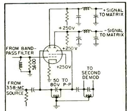
FIG. 5—Demodulator circuit using beam-deflection tube
