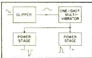
FIG. 1—Positive and negative output stages are separate in pulsing unit
