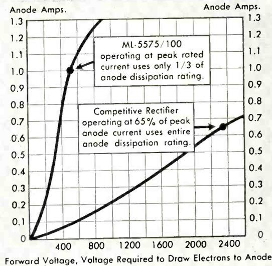
ML-5575/100 operates at 100% of current rating with 300% safety factor for anode dissipation. Competitive high vacuum rectifier tube operating at 65% of peak anode current is at limit of anode dissipation.
