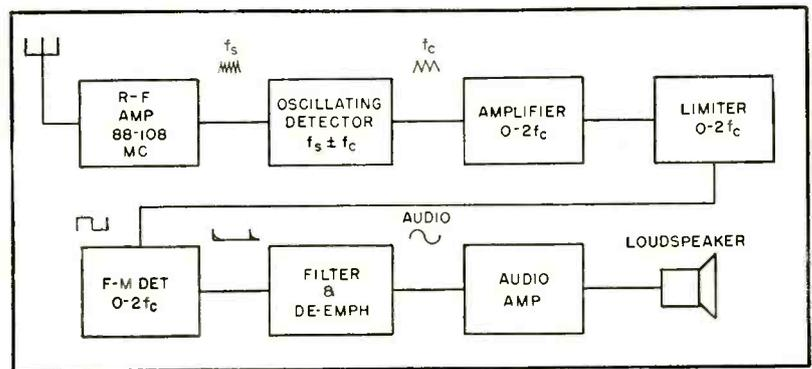
FIG. 2—Block diagram of simple receiver in which  $f_s$  is signal frequency and  $f_c$  the center frequency or half the widened bandwidth
