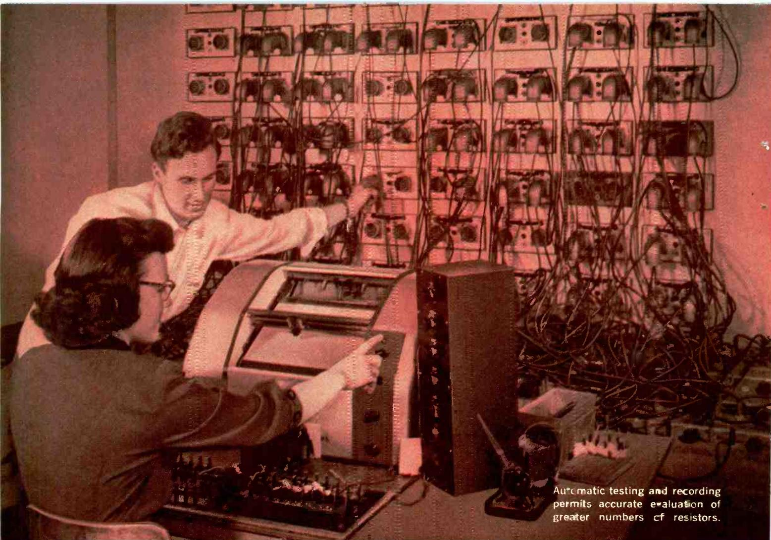
Automatic testing and recording permits accurate evaluation of greater numbers of resistors.
