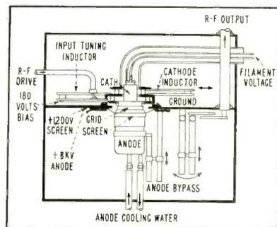
FIG. 2—Mounting of tube and tuning capacitors in 25-kw visual amplifier
