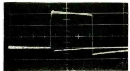
Output waveform of multipulse generator, left, with maximum delay time. Oscilloscope sweep speed was 20 microseconds per cm. Trace of pulse-generator output, center, was made with 0.1 microsecond-per-cm sweep. Output of delay generator, right, shows maximum and minimum pulse widths obtainable. Sweep speed in this oscillogram was 20 microseconds per cm
