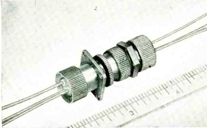
**TITEFLEX CONNECTOR**—lightweight, corrosion and moisture resistant with temperature ranges of  $-65^{\circ}\text{F.}$  to  $+400^{\circ}\text{F.}$  This connector's insulation properties will permit 3500 volts at sea level, 1200 volts at 50,000 feet altitude. Connector is available with 2 or 3 pins. 7 amperes. Weight  $\frac{3}{8}$  of ounce. Size 2" in length.
