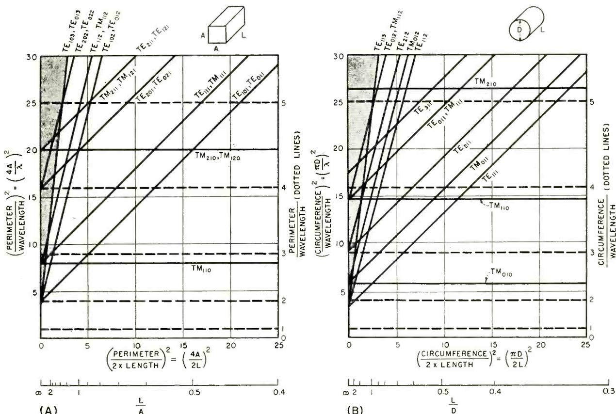
FIG. 1—Mode charts for square (A) and circular (B) cross sections. Shaded areas are incomplete. In B, every mode has a pair of crossed orientations unless the first index is zero
