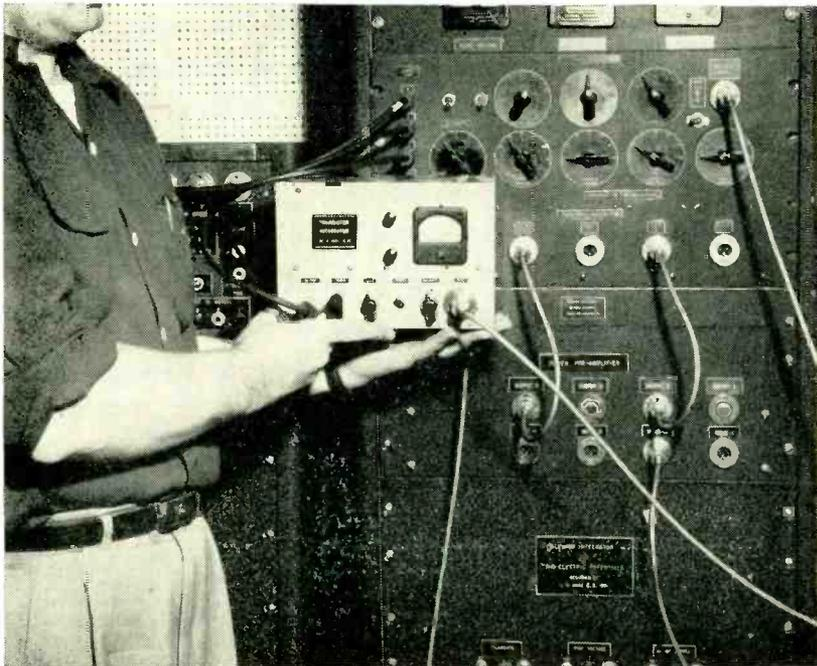
Compact transistor integrator (left) replaces bulky electron-tube unit mounted in rack at right
