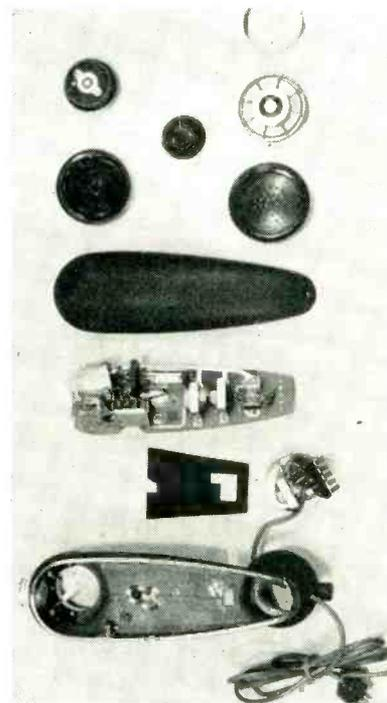
Exploded view of portable transceiver
