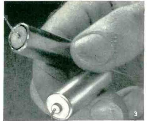
**3. Undamaged by dropping,** the two capacitors are shown here—note that there are no cracks in the G-E silicone-sealed unit.
