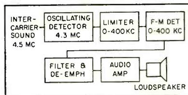
FIG. 6—Circuit can be used to improve tv sound
