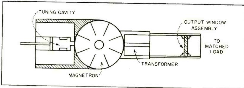
FIG. 1—Location of output window in magnetron output waveguide
