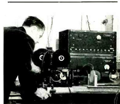
Television recording system designed for military operation comprises special film camera focused on kinescope. Ancillary electronic equipment enclosed in relay-rack cabinet is not shown
