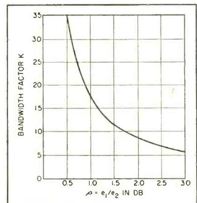
FIG. 1.—Bandwidth multiplication factor for various amplitude ratios
