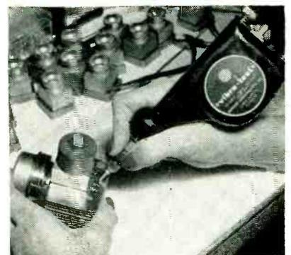
Writing serial numbers on magnetron cavity assembly with vibrating tool
