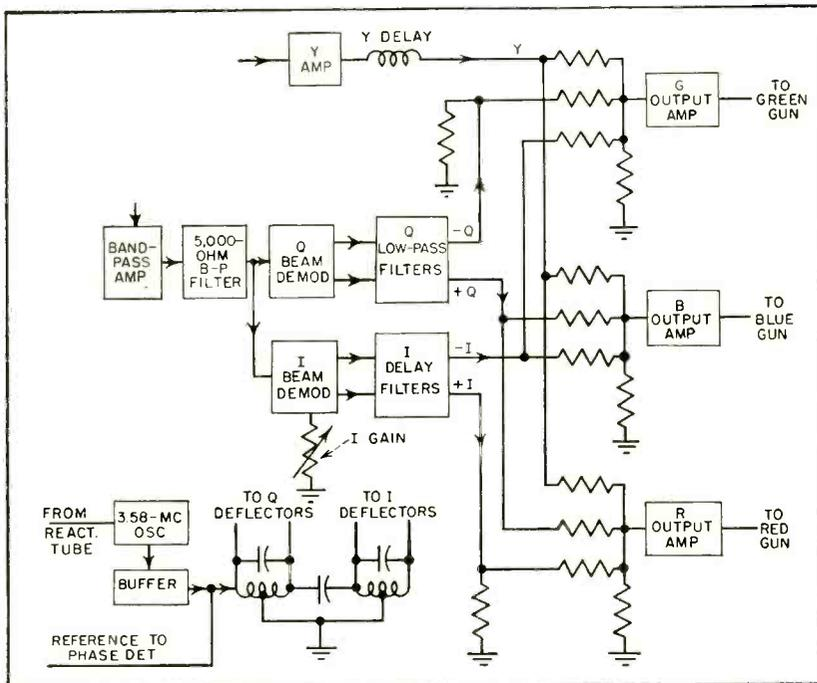
FIG. 4—Color decoder using 6AS6 demodulator tubes and low-level matrixing
