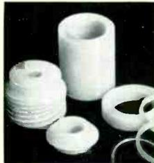
Nylon is drilled satisfactorily with ordinary twist drills. To obtain a smooth hole of uniform diameter, use a slow, uniform feed with the highest speed that will not cause "gumming" or burning. Keep holes chip-free by removing the drill from the hole frequently.
