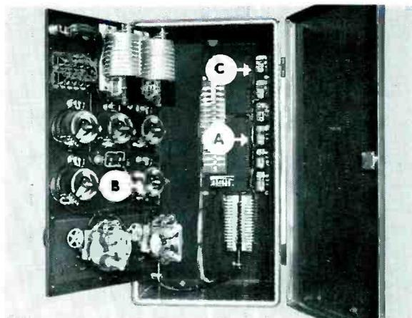
WARD LEONARD BULLETIN 110 RELAYS in Trafflex Master Controller are used for: A. Automatic selection of one of five timing cycles. B. Operation of pilot lights indicating which of three timing dials in Trafflex Secondaries is in use. C. Remote control of off-duty flashing amber and remote control of signal shut-down for entire system.
