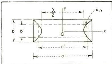
FIG. 3—Sectional view of rectangular waveguide
