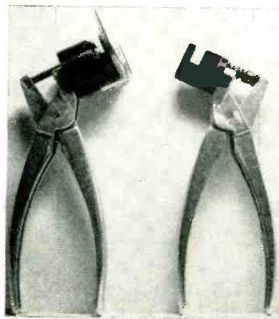
Half-circle punch (left) and small round punch for making gasket holes in moisture-proofing material
