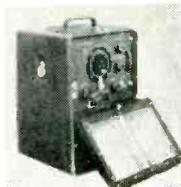
The justly famous UHF Heterodyne Frequency Meter TS-175/U is now available from WESTON LABORATORIES. Of new manufacture, this improved equipment operates over the range of over 80-1000 meg. cy. with an overall accuracy of better than .001 at fixed room temperature. Supplied complete with AT-66/U Antenna, 2 cords, spare tubes, original calibration book and instruction book at a net price of \$550. ORDER YOUR UNIT TODAY.
