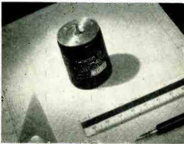
DALMOTOR Co., 1329 Clay St., Santa Clara, Calif. Rated for continuous duty with an output frequency of 20 cps and a maximum of 3-percent harmonic distortion, type 44A generator is recommended for instrument indicating and other similar applications. Voltage is linear with speed, and the unit develops 33 v of 2-phase a-c at 4,500 rpm. Internal
