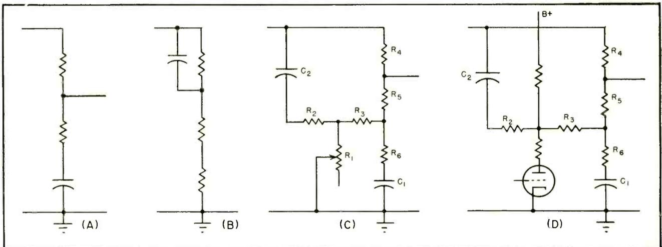
FIG. 1—Low-frequency (A) and high-frequency (B) boost circuits are combined to obtain combination boost circuit (C). Basic tone-compensation control (D) uses triode plate resistance as arm of T-pad
