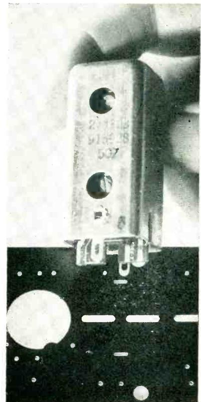
Method of inserting etched i-f transformer in etched video amplifier panel. Wiring is on other side of panel
