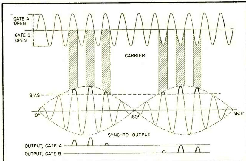
FIG. 1—Synchro output exceeds bias during part of each half revolution producing pulse to trigger flip-flop
