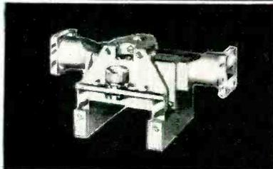
**SLOTTED SECTIONS**—The mechanical and electrical design of PRD slotted sections emphasizes these important features: Instrument accuracy assured indefinitely by virtue of three bearing carriage suspension to minimize wear; waveguide section machined from solid aluminum alloy stock, to avoid warpage no castings are used.
