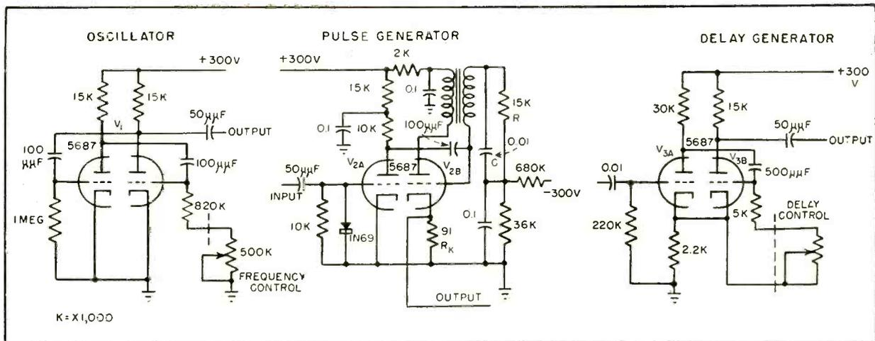
FIG. 1—Oscillator, pulse generator and delay generator circuits have power supply, input and output leads connected to pins of plug-in socket. Frequency and delay-time control potentiometers are mounted on main chassis
