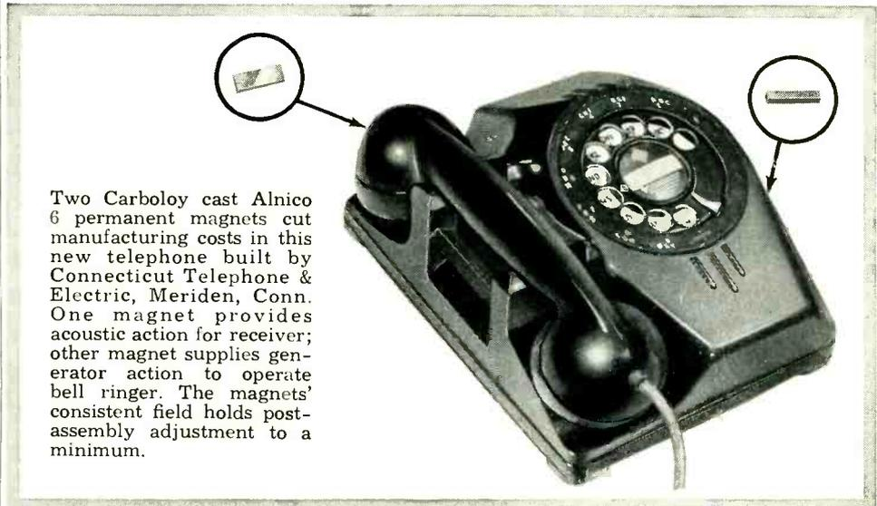
Two Carboloy cast Alnico 6 permanent magnets cut manufacturing costs in this new telephone built by Connecticut Telephone & Electric, Meriden, Conn. One magnet provides acoustic action for receiver; other magnet supplies generator action to operate bell ringer. The magnets' consistent field holds post-assembly adjustment to a minimum.
