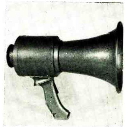
rounding noise conditions. Outstanding feature is the virtual elimination of acoustic feedback. The present unit is completely self-contained with batteries and 3-stage vacuum-tube amplifier in the main housing. It is small and light, only weighing slightly over 5 lb, and being just over a foot long. The form-fitting handle incorporates a press-to-talk trigger switch.
