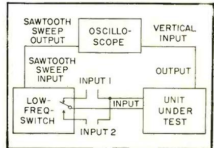
FIG. 1—Switch setup for operation as synchronous step-function producer. Sawtooth sweep input triggers relay
