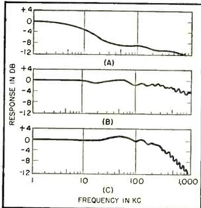
FIG. 3—Frequency response curves for three sections of delay line (A), with parallel resistors inserted (B), and with transistor amplifiers added (C)
