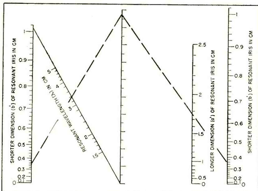
FIG. 4—Nomograph for determining iris dimensions for a waveguide  $0.900 \times 0.400$  inch ( $2.286 \times 1.016$  cm)
