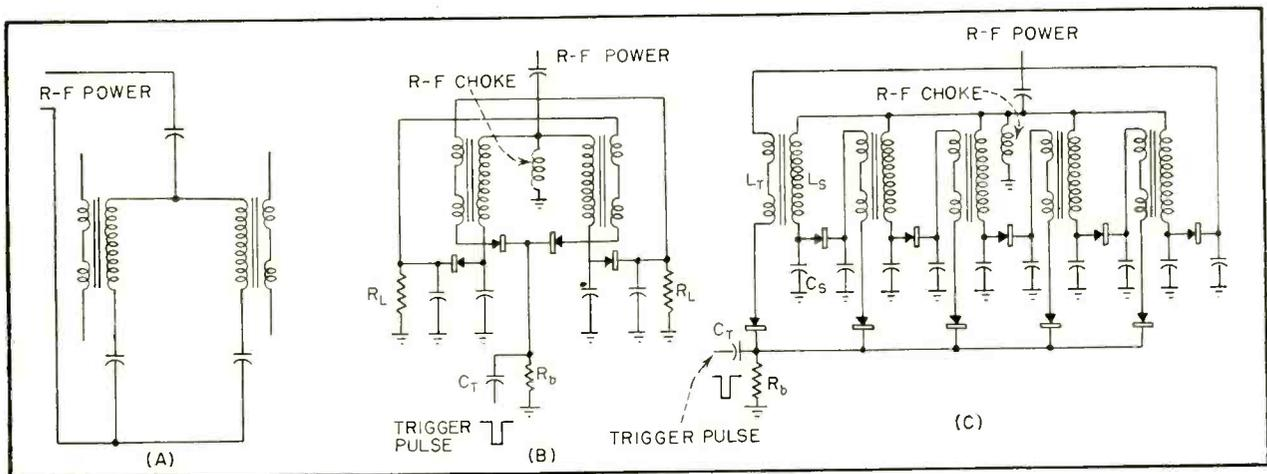
FIG. 1—Basic flip-flop unit (A) can be triggered as shown in (B). Five stage ring counter (C) shows simplicity of circuit
