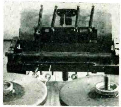
Input end of sleeving chopper, showing two reels in foreground. Other two are off to left and right. The four springs pull back the levers on the knurled wheels after each operation. Five-position pointer, fixed in position, can be seen between the springs
