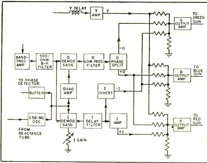
FIG. 7—Color decoder with 6AS6 demodulators replaced by beam-deflection tubes
