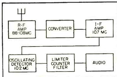
FIG. 5—Block representation of improved receiver using commercial tuner
