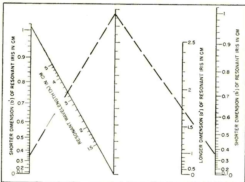
FIG. 4—Nomograph for determining iris dimensions for a waveguide 0.900 × 0.400 inch (2.286 × 1.016 cm)
