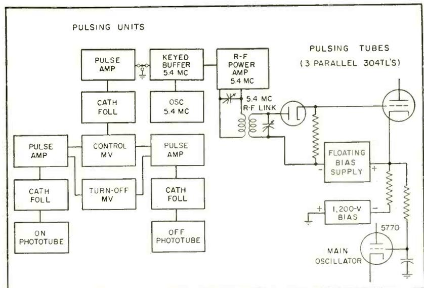
FIG. 2—Pulser circuit turns oscillator on and off to accelerate particles during descending part of the f-m cycle
