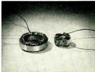
input to the synchro is 26 v, 400 cps. Stator output is 11.8 v. Input power when loaded with one control transformer is 0.973 w and sensitivity at control transformer output is 397 mv per deg. The synchro reflects to its shaft no measurable cogging effects or mechanical loading. Outline drawings, mounting information, complete characteristic basic data and typical error curves will be mailed on request to the company.
