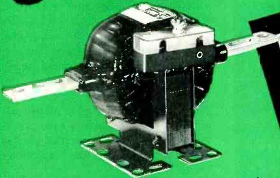
Sangamo Type MA-25 Current Transformers are designed for indoor service on metering applications. They are wound type with single primary and single secondary, and meet A.S.A. 2.5 KV insulation class test requirements—15 KV at 60 cycles and 45 KV full wave impulse. Natvar 400 Extruded Vinyl Tape is used because of high insulation value, resistance to heat and ability to form itself to the shape of parts being insulated.
