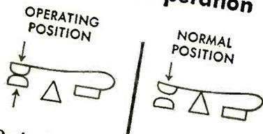
Preloading contact spring applies pressure of 50 grams when contacts close. Contact spring also absorbs overshoot thus preventing a permanent set or change in calibration.
