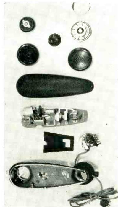
Exploded view of portable transceiver
