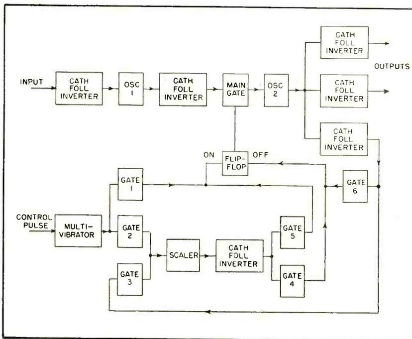
FIG. 3—Control system provides for several modes of operation including normal continuous operation, series of pulses per control pulse and 1 pulse for a group of control pulses
