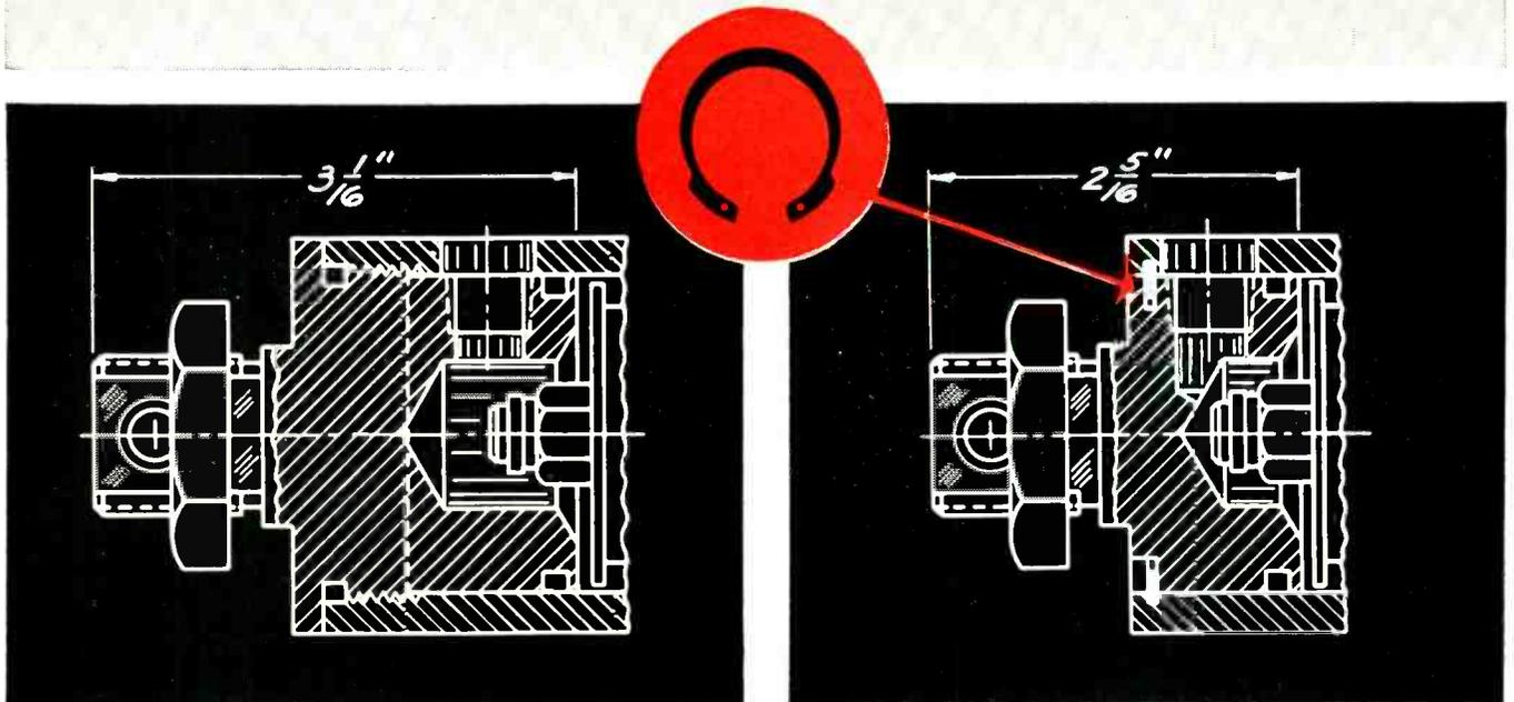
**OLD STYLE** air cylinder, with thread-secured head, required costly tapping, chasing and assembly operations. Also, satisfactory maintenance of packing unit necessitated use of pipe wrenches on painted surfaces.
