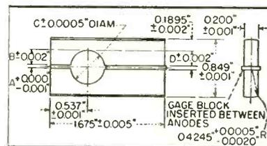
FIG. 2—Dimensions and tolerances required for copper anode blocks of a magnetron
