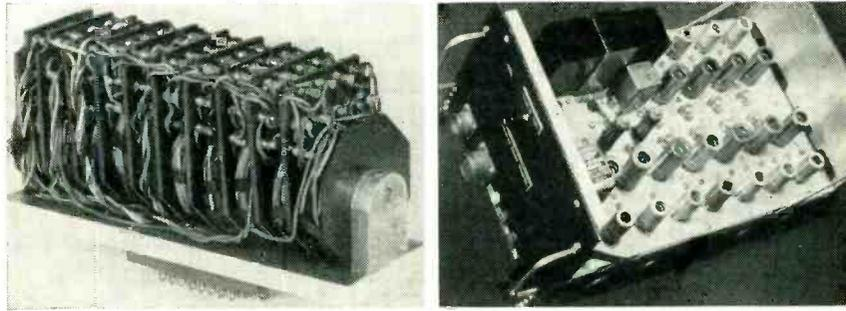
Magnetic-matrix switch before potting illustrates details. Top of chassis view of binary counter shows how switch clamps in place
