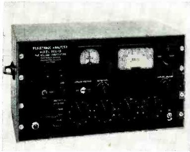
resistor up to a power rating of 1.5 w can be determined down as low as 0.0002 percent per volt. Voltage across the measured resistance is continuously variable in two ranges from 0 to 500 v by a self-contained regulated power supply. Sensitivity of balance is within 0.04 percent on all ranges. It is designed for 115-v, 60-cycle operation.
