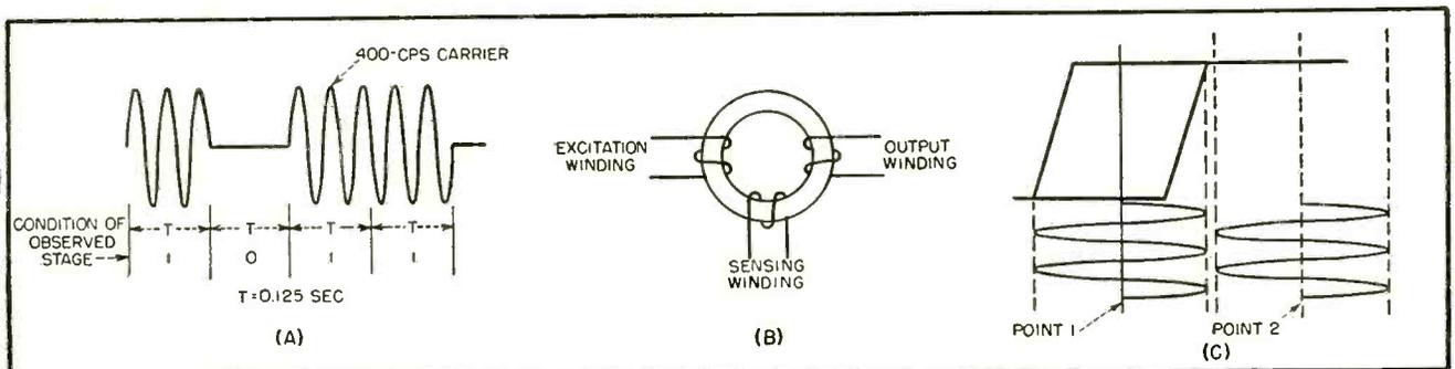
FIG. 1—Idealized switch output (A) with schematic of important core windings (B) and operating characteristics of magnetic circuit (C)
