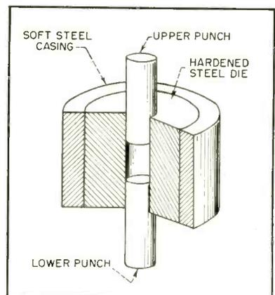
FIG. 1—Small coining die used in preliminary experiments with this technique
