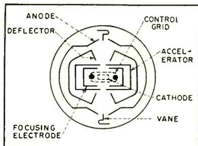
FIG. 2—Cross section showing location of beam-tube elements
