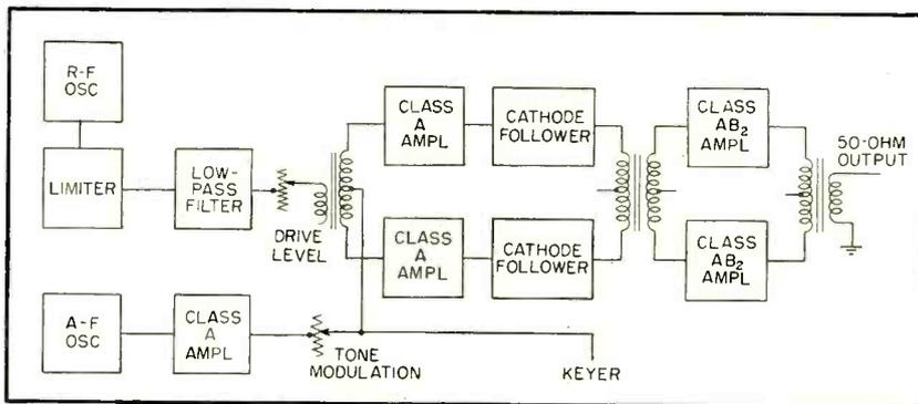
FIG. 1—Layout of low-frequency transmitter employing tone modulation
