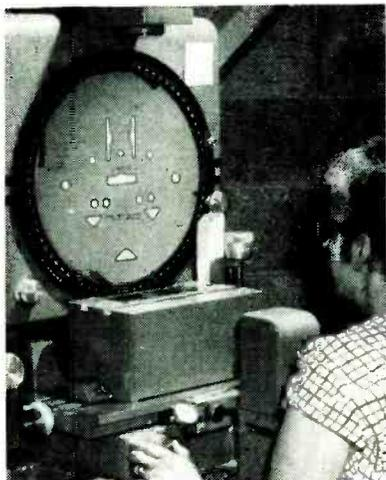
Checking locations and diameters of holes in mica spacers. Light from vertical illuminator at top projects shadow of mica resting on glass staging table
