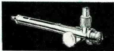
**TYPE 250-A BROADBAND PROBE** — Frequency range of 1 to 12.4 Kmc/s; two tuning knobs permit precise adjustment for maximum power transfer from the probe tip to the crystal or bolometer detector; third knob controls depth of probe tip insertion.
