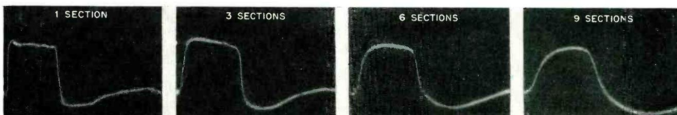
FIG. 5—Transistorized delay line output pulse shape after passing through 1, 3, 6 and 9 sections
