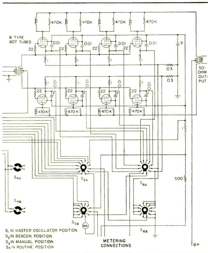
Final stage uses eight type 807 tubes in push-pull parallel
