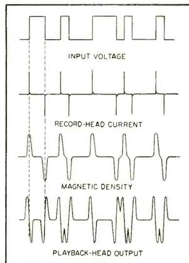
**FIG. 2—Waveforms in pwm recorder.** Trailing edge of output pulses coincide with leading edge of input pulses
