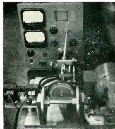
Setup for running in the tuning mechanism of a five-band oscillator by rotating the tuning dial 20 turns in each direction alternately. Clutch-reversing solenoids are at left
