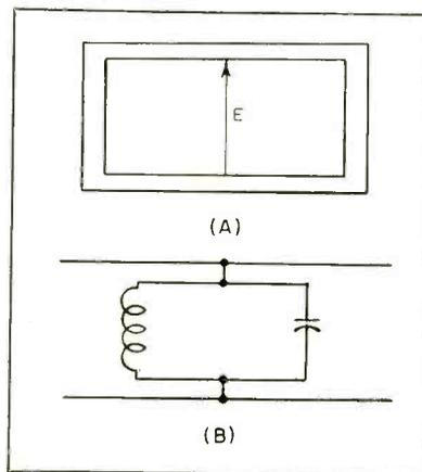
FIG. 2—Cross section (A) and equivalent circuit (B) of typical resonant iris
