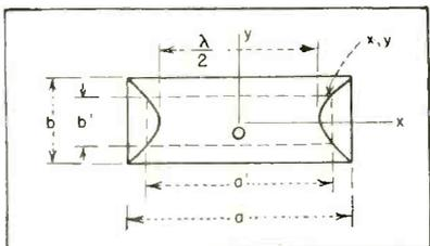
FIG. 3—Sectional view of rectangular waveguide
