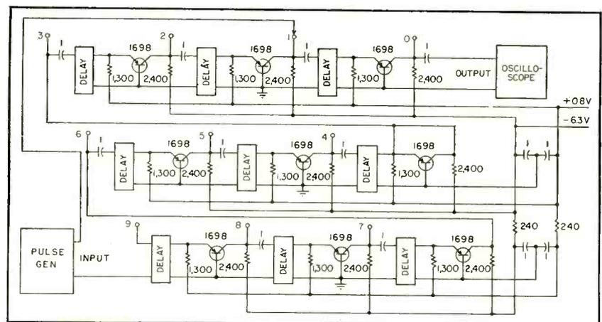
FIG. 4—Nine-section transistorized delay line using cascaded distributed-constant sections of 7.8- $\mu$ sec delay each
