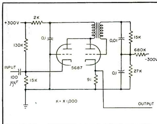
FIG. 3—Alternate plug-in pulse-generator circuit can be used when low power consumption is important
