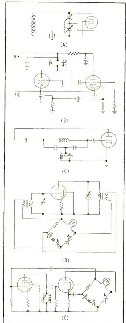
FIG. 2—Simple series oscillator (A), cathode-coupled (B), Bridged-T (C), Meacham bridge, transformer coupled (D) and Meacham oscillator with R-C feedback (E)
