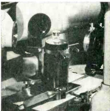
Details of multiple-lamp projector, showing rotatable staging table
