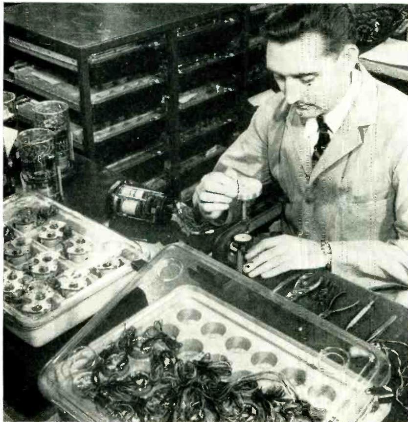
**Typical use of hinged-cover containers at work bench. Only one subassembly is removed at a time from the protective tray, to minimize chances of damage**
