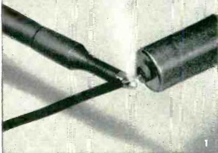
**1. Solder right up to the case** with new G-E silicone end seal—no need to waste ¼ inch of valuable space because of danger of cracking glass.
