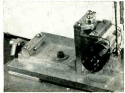
Close-up of tube holder, with pendulum resting at point of impact
