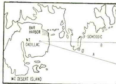
FIG. 1—Unobstructed path A compared with path B over knife-edge used for diffraction observations
