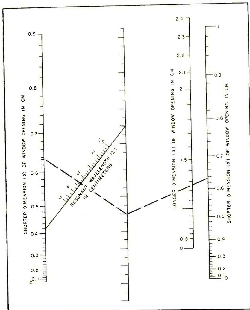
FIG. 6—Nomograph for determining resonant wavelength of sandwich-type ceramic output windows for a waveguide  $0.900 \times 0.400$  inch with  $\epsilon_r = 6$
