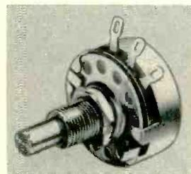
The Type J Bradleyometer has a solid molded resistor ring which can be made to satisfy any resistance-rotation requirement. All ferrous parts are made of corrosion-resistant metal. There are no riveted, welded, or soldered connections in the Bradleyometer.
