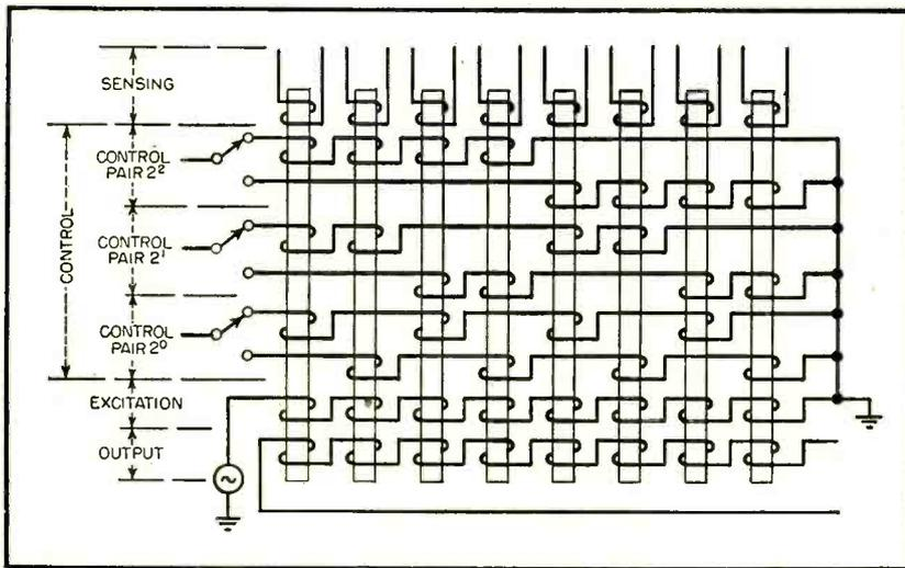
FIG. 2—Basic circuit of magnetic-matrix stepping switch illustrates how the principle of core saturation can be utilized in a switching operation
