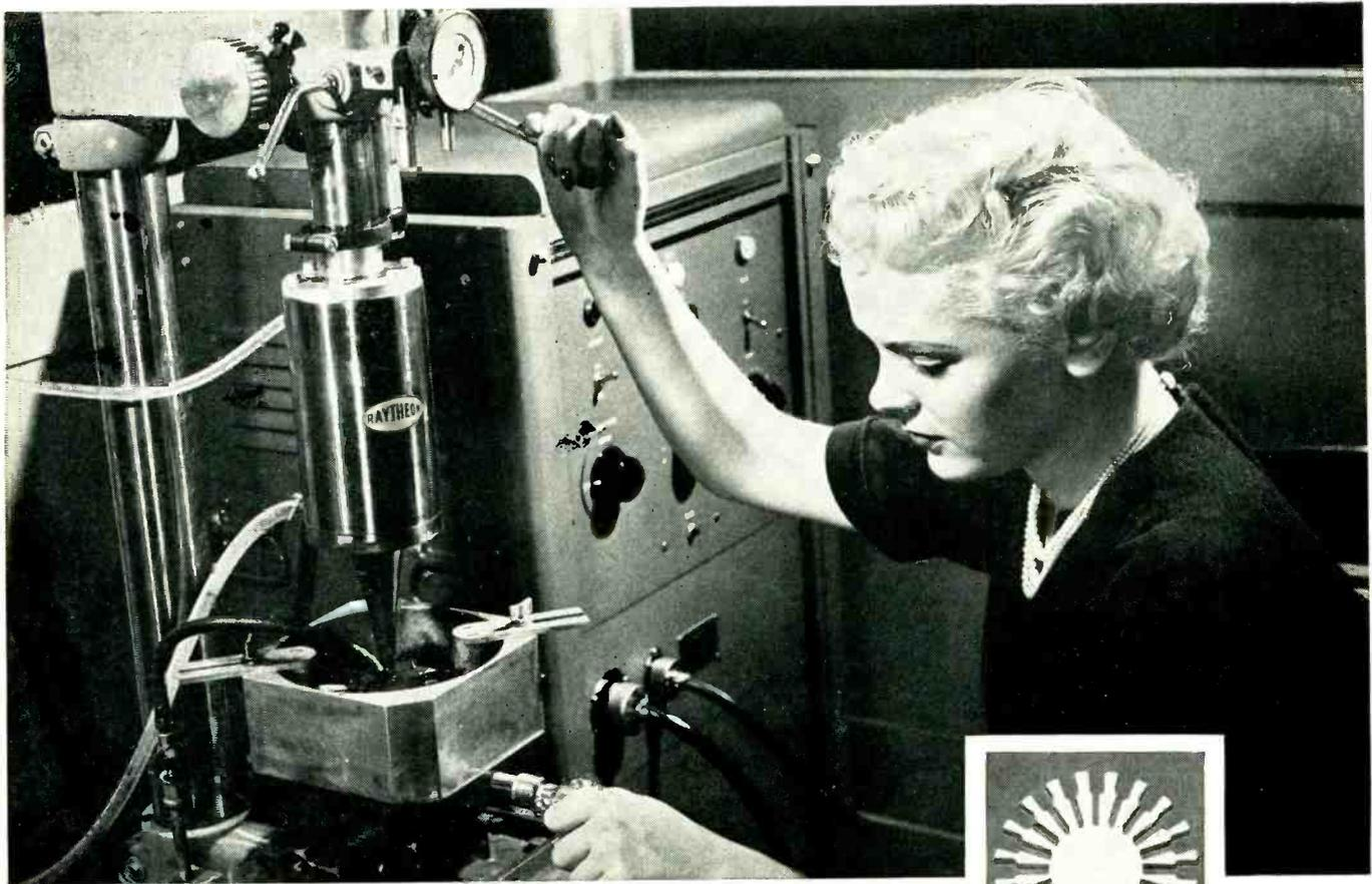
**Ultrasonic Machine Tool**—Raytheon Manufacturing Company, Waltham, Mass., uses Inco Nickel to keep its magnetostrictive transducer working; tough, fatigue-resisting Monel for the toolholder; chromium-nickel stainless steel for the transducer housing. A pattern Raytheon's UMT can cut in tungsten carbide is shown at right.
