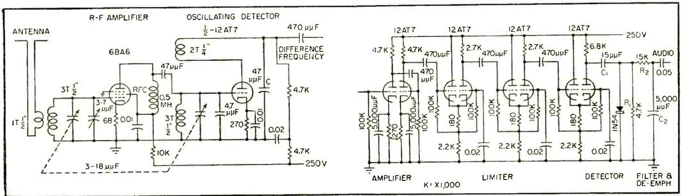
FIG. 3—Simple receiver using single r-f amplifier, oscillating detector, triple limiter and counter detector
