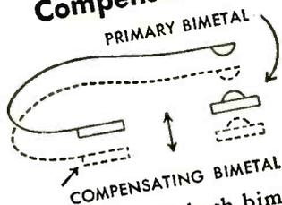
Ambient affects both bimetals exactly alike. Contact gap maintains relative position independent of ambient temperatures from  $-60^{\circ}\text{C}$  to  $+85^{\circ}\text{C}$ .
