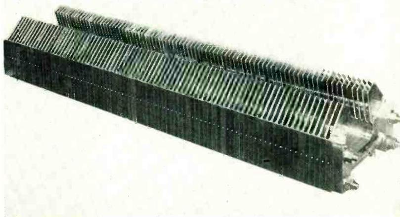
Water-cooled stator of 3,600- $\mu$ f capacitor is mounted in a vacuum with other parts of cyclotron r-f system
