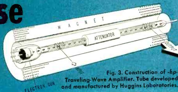
Fig. 3. Construction of **-hp-** Traveling-Wave Amplifier. Tube developed and manufactured by Huggins Laboratories.
