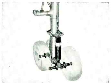
**In shock struts** The landing gear pistons on some of our largest planes are made of Synthane. Properties of light weight, toughness, durability and shock resistance were needed; Synthane supplied them.
