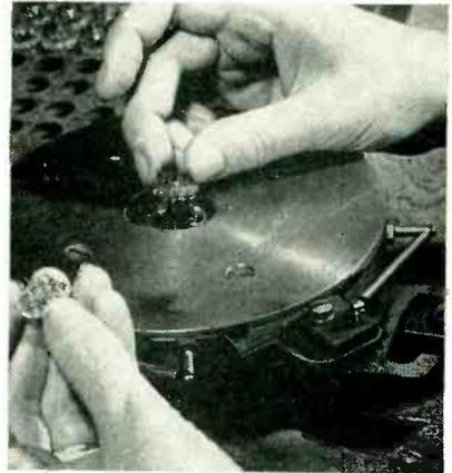
Miniature stem die bends some or all of the nine wires to correct specifications in one operation
