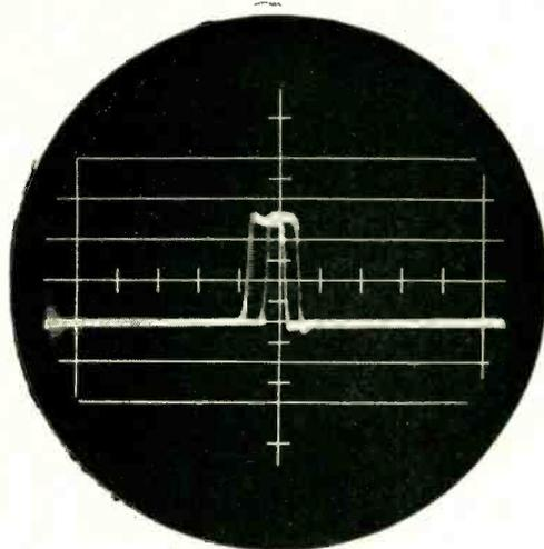
Figure 1. Unique modulating fidelity of -hp-490A is shown in double-exposed oscillogram of 0.1  $\mu$ sec pulses. First pulse (applied by -hp-212A Pulse Generator) is modulating pulse having rise time of 0.02  $\mu$ sec; delay through tube approximately 50 millimicroseconds. Second pulse is rf output; note absence of deterioration.
