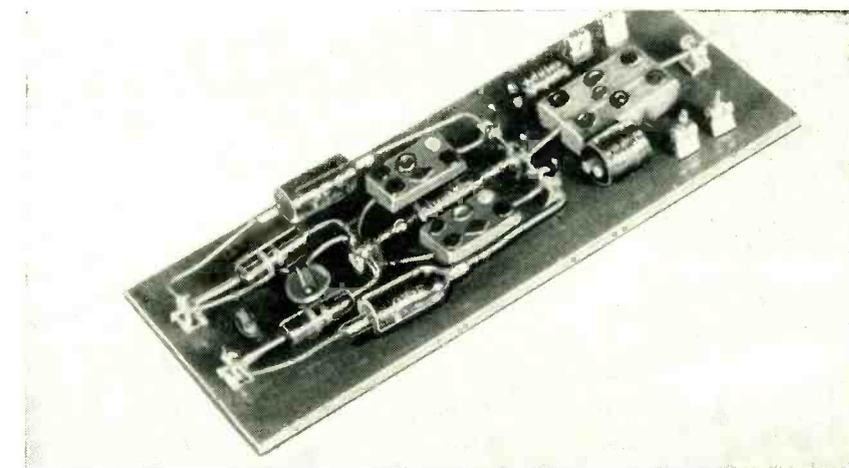
Complete ferroresonant flip-flop unit with coupling capacitor and diodes
