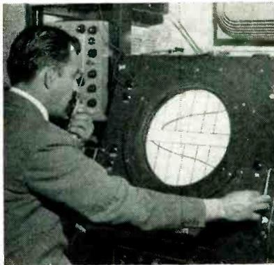
Scope presentation of airfield approaches gives ground operator plane position information from which he can direct pilot by radio
