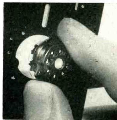
Inserting special snap-in socket into keyed hole in panel
