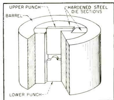
FIG. 3—Coining die used for anode blocks
