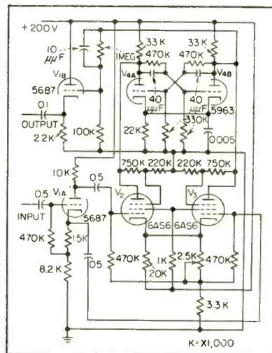
FIG. 3—Integrator circuit sensitive to amplitude and rate polarities near zero
