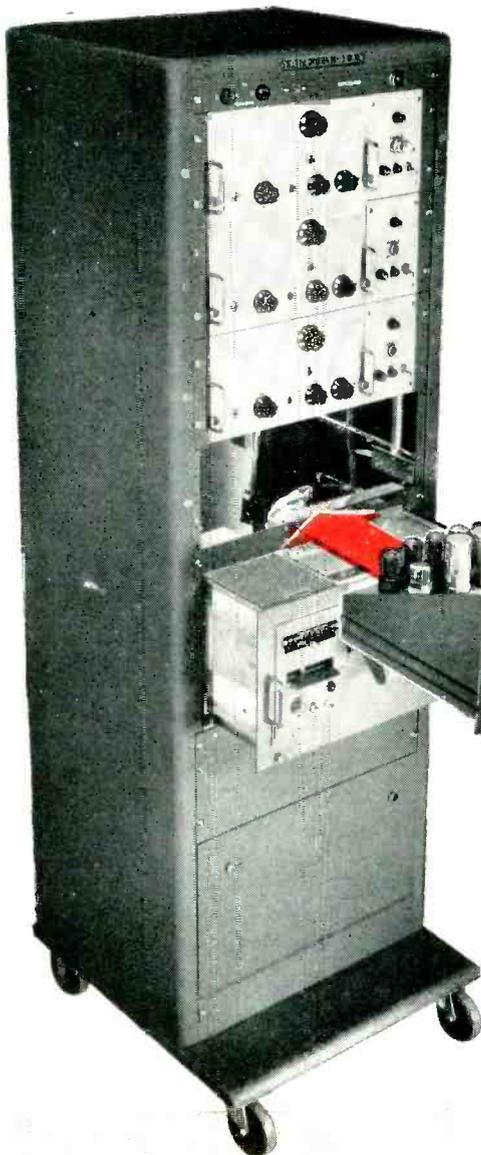
The **BASIC** four-channel assembly includes: Cabinet, Recorder, and, for each channel, a **BUILT-IN** unit (A), which comprises a Driver Amplifier with frame, and a Power Supply with control panel.
