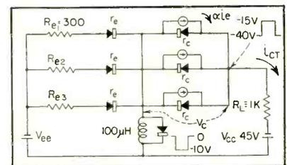
FIG. 3—Equivalent circuit used in calculating power requirements
