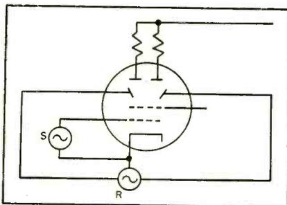
FIG. 1—Schematic representation of beam-deflection tube
