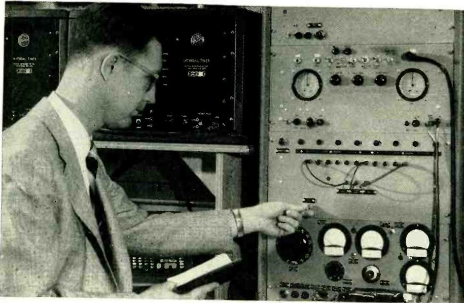
Equipment for generating pulses indicating shaft position uses flip-flop circuit which is immune to false triggering
