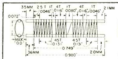
Example of wound grid, showing dimensions and profiles requiring inspection
