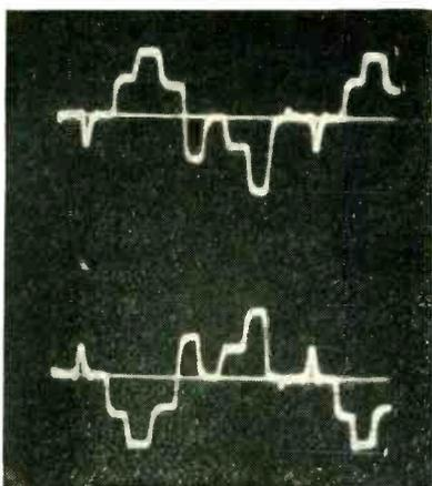
Fig. 9—Waveforms of  $+Q$  and  $-Q$  outputs on bar pattern signal with chrominance signal applied to deflectors. Peak-to-peak voltages are 180 volts across 15,000-ohm plate loads
