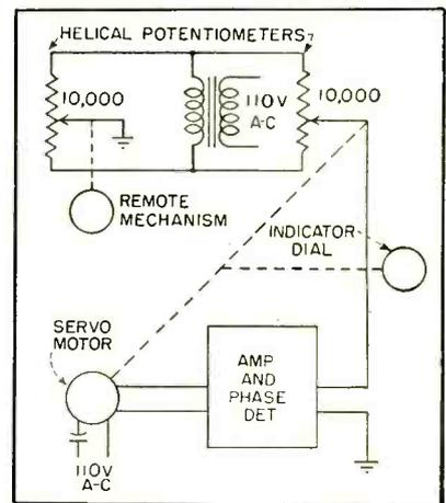
FIG. 4—Null-type servo system indicates position of pulser phototubes
