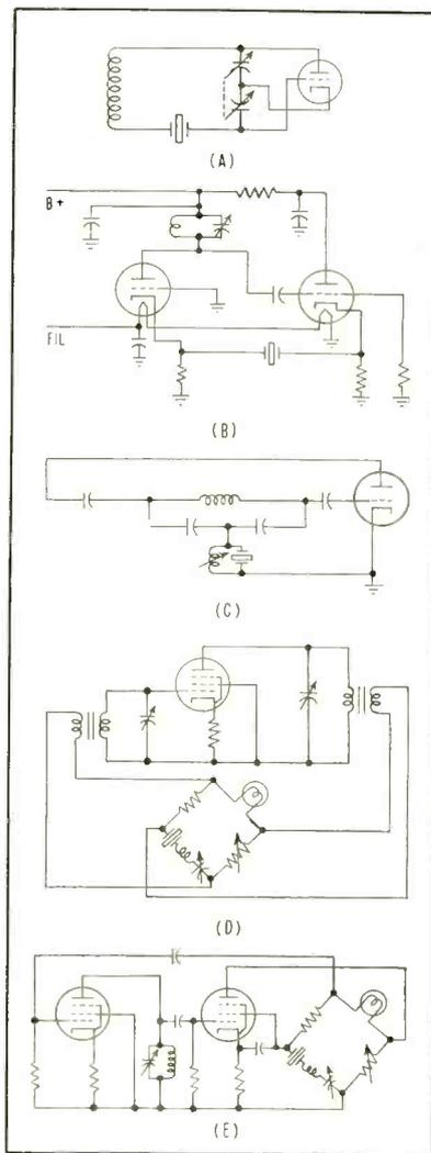
FIG. 2—Simple series oscillator (A), cathode-coupled (B), Bridged-T (C), Meacham bridge, transformer coupled (D) and Meacham oscillator with R-C feedback (E)
