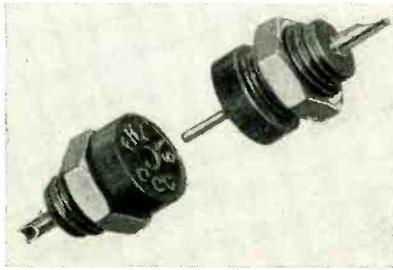
port strength and arc resistance; and Diallyl Phthalate (blue) with high dimensional stability plus excellent dielectric properties. Precision-machined socket and pin contacts are of spring temper phosphor bronze and brass respectively, gold plate over silver giving low contact resistance and ease of soldering.
