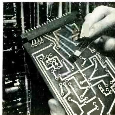
Phenolic plates with circuits etched in advance eliminate elaborate wiring and permit cheaper soldering methods for new rural-line carrier equipment that also includes transistors of the type shown
