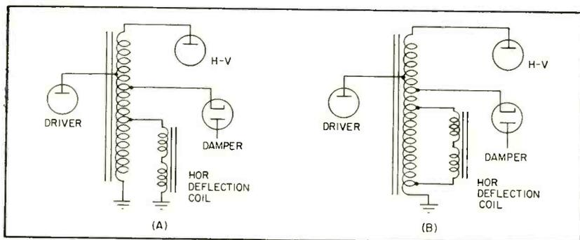
FIG. 3—Cancellation of ringing results when deflection coil is raised electrically from its normal position (A) to new balanced position (B)
