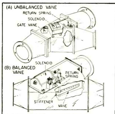
FIG. 3—Two types of reject gates used to divert contaminated hay
