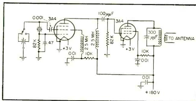
FIG. 2—Schematic and picture of altitude transmitter. Pressure sensitive capacitors at input are alternately switched to create frequency difference indicating altitude
