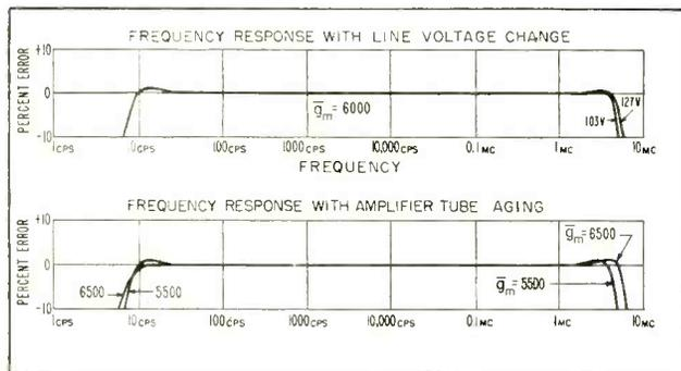
Fig. 1. Typical variation in accuracy with line voltage changes and mutual conductance changes (geometric mean value of the four amplifier tubes).
