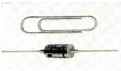
INTERNATIONAL RECTIFIER CORP., 1521 E. Grand Ave., El Segundo, Calif., is producing a Red-Dot series of germanium diodes for high temperature applications. Each unit is so well sealed that exposure to 95 plus percent relative humidity for 500-hours at temperatures from
