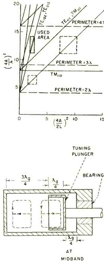
FIG. 2—Region of mode chart (above) chosen for crossed-mode tuner of square cross section (below)
