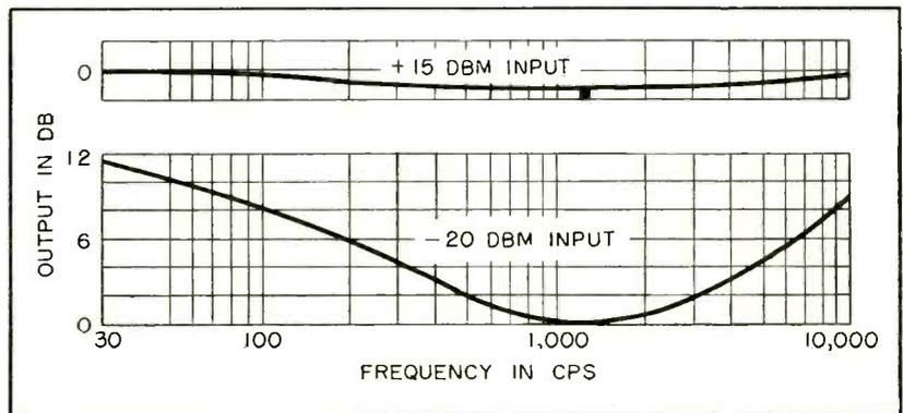
FIG. 3—Response of amplifier to different input signal levels
