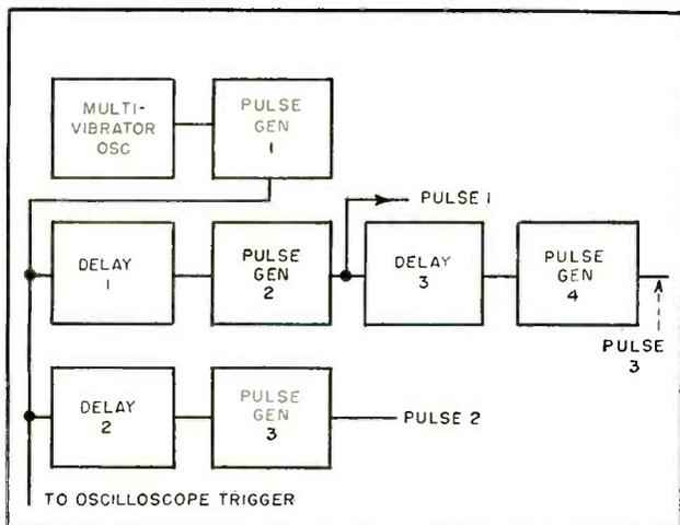
FIG. 2—Block diagram of typical delay-generator system made up of plug-in units described in text
