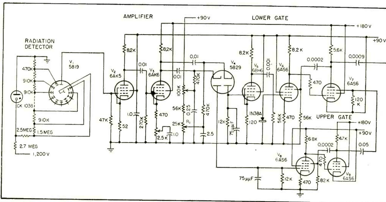
FIG. 1—Balloon-borne unit employs sodium-iodide crystal as radiation detector. High-voltage regulator circuit is maintained at
