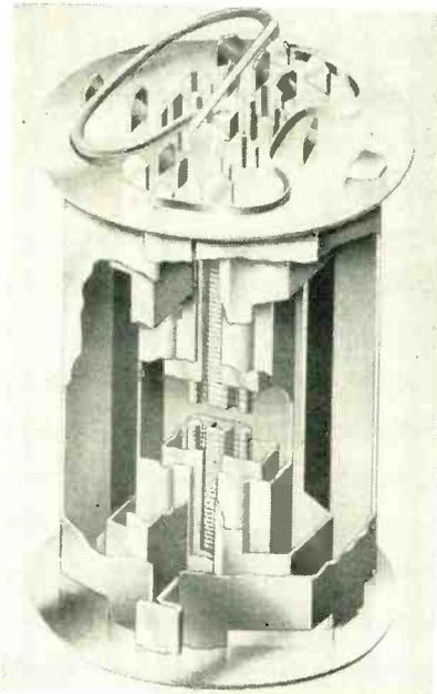
Cut-away view of General Electric 6AR8 beam-deflection tube
