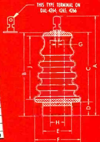
These terminals are made of glazed Alumina Ceramic. Lugs and eyelets are hot tinned brass and metallized areas are silver fired on ceramic, copper electroplated and tin fused for soft soldering. Im-
