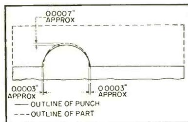
FIG. 4—Effect of springback of copper Steps in coining an anode block
