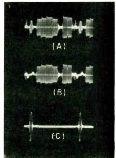
FIG. 11—Burst-gate input chrominance signal (A), gated output to chrominance channel (B) and gated output to burst channel (C)
