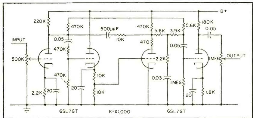
FIG. 2—Audio-frequency voltage amplifier incorporating tone-compensation control
