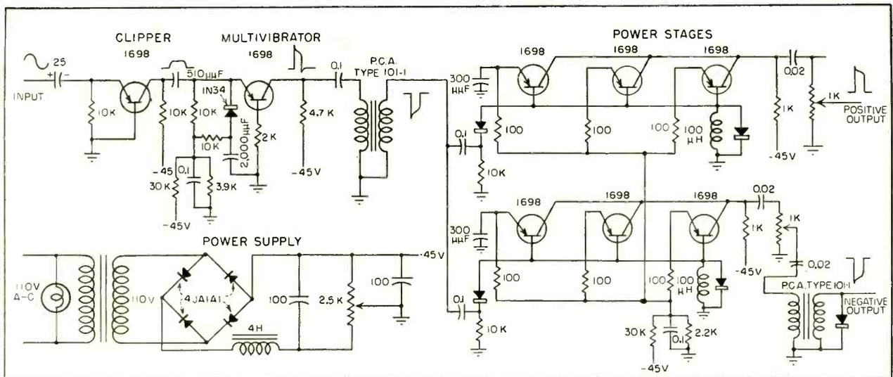
FIG. 2—Sine-wave-to-pulse converter uses diode bridge power supply. Pulse transformer in negative output inverts pulse
