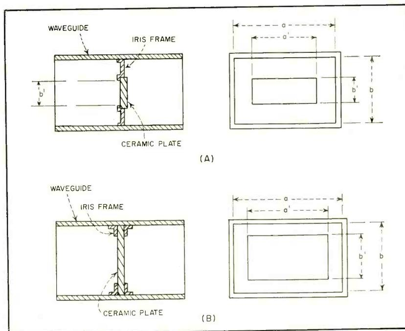
FIG. 5—Ceramic output windows with ceramic plate fitted into single metallic frame—single-frame type (A) and between two metallic frames—sandwich type (B)
