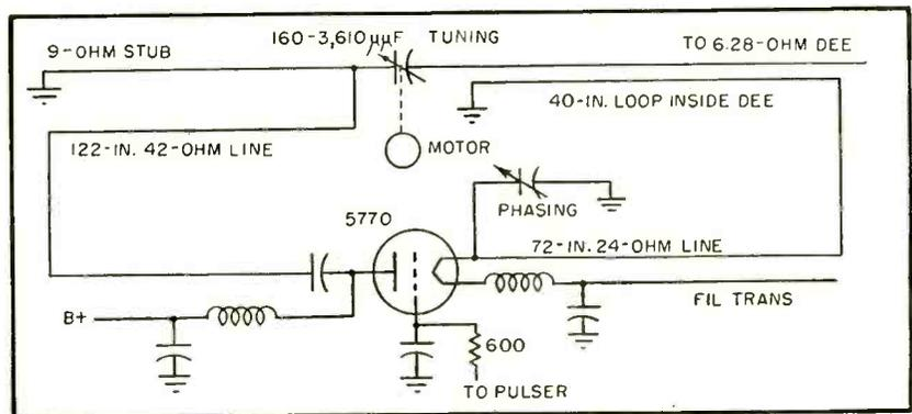
FIG. 1—Sweep-frequency oscillator generates 40-kw r-f signal
