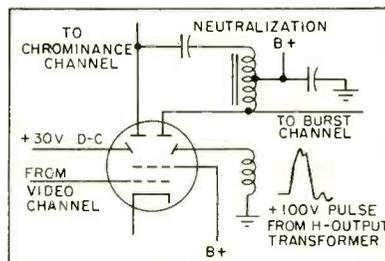
FIG. 10—Beam-deflection burst gate circuit. Only shaded portion of input pulse is effective in deflecting beam from plate to plate
