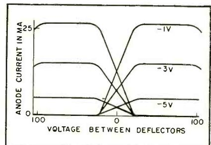
FIG. 3—Deflector characteristics for -1, -3 and -5 volts control-grid bias
