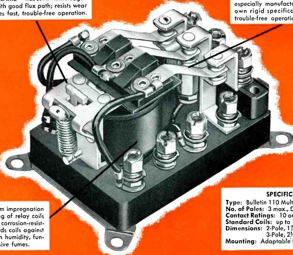
**COIL** — vacuum impregnation and end sealing of relay coils plus a special corrosion-resistant finish guards coils against salt spray, high humidity, fungus and corrosive fumes.
