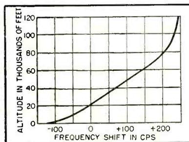
FIG. 3—Altitude-transmitter frequency shift as a function of altitude
