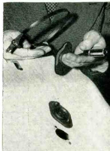
Sensing element, feed-through gasket and terminal plug (in hands) and example of hole required in moistureproof wrapping material for installation of feed-through gasket
