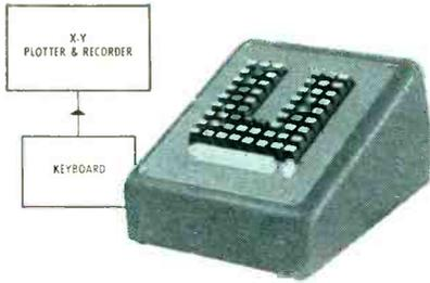
**DECIMAL KEYBOARD:** Consists of a three-decimal bank for each axis with associated plus-minus keys. Depressing plot bar initiates plot and clears keyboard automatically. Also manual clear button. Size: 8½ x 11 in., Weight: 12 Lbs.
