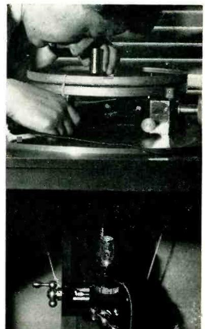
Color mask alignment setup, showing crater lamp mounted on cross-feed screws under bench. Operator is holding portable ultraviolet light source in right hand to activate phosphors
