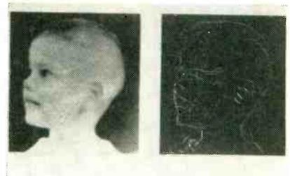
FIG. 2—Video picture (left) produced from original photo negative. At right, outline resulting from singly differentiated and rectified video signals that were then amplified and clipped at constant level
