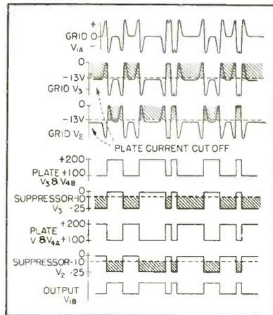
FIG. 4—Pulse sequence in integrator circuit. Shaded area indicates plate current is cut off by suppressor grid
