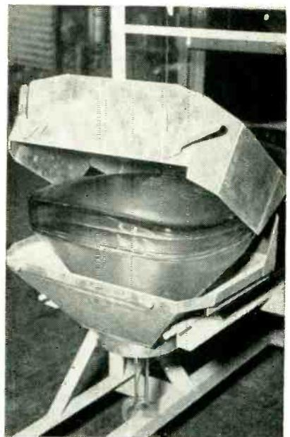
Clam shell metal housing for picture tube. The two latches lock over studs on the lower part when the cover is down
