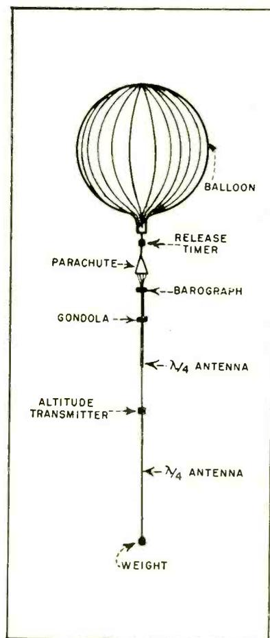
Plastic balloon used to carry telemetering equipment being inflated. Diagram at right shows balloon rigging
