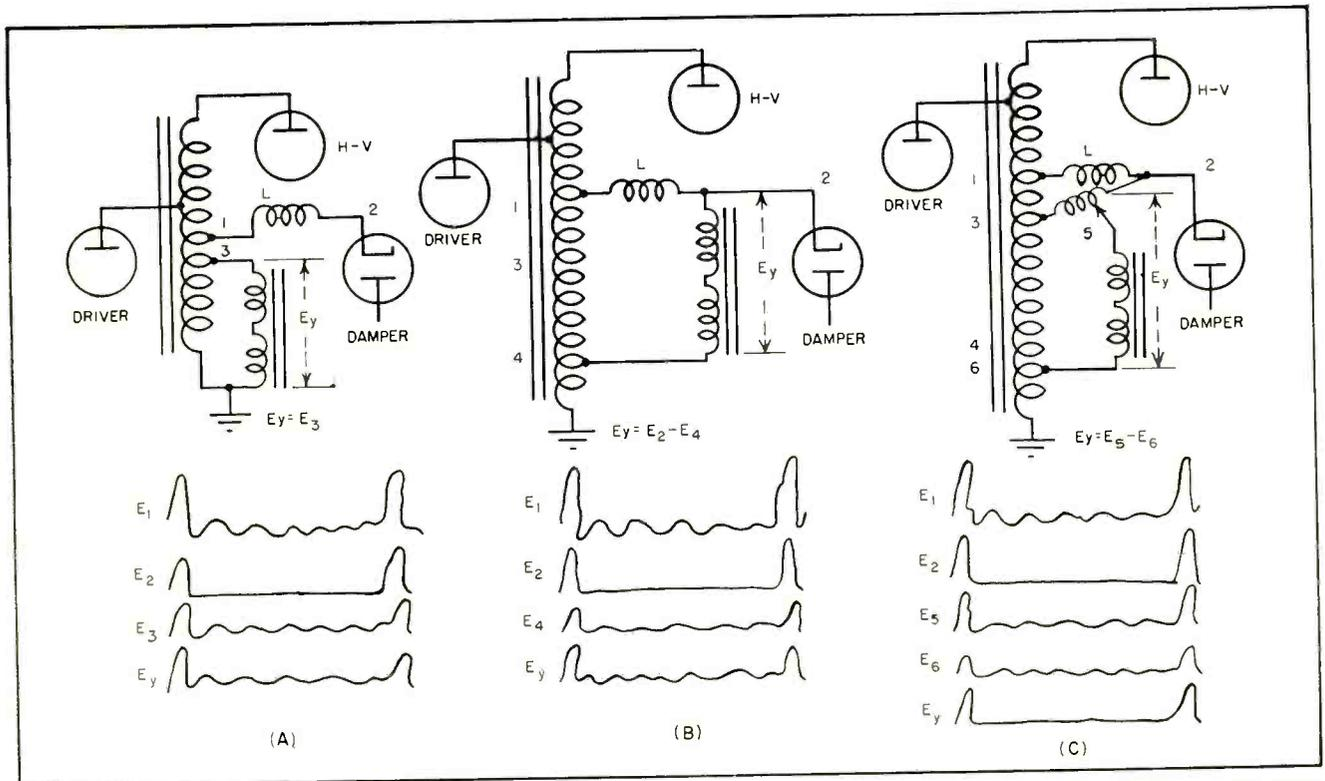
FIG. 4—How deflection coil connections cancel ringing: normal position (A) fails to make use of damper; raising bottom of coil above ground is intermediate step (B); clean waveform results when balance is achieved (C)
