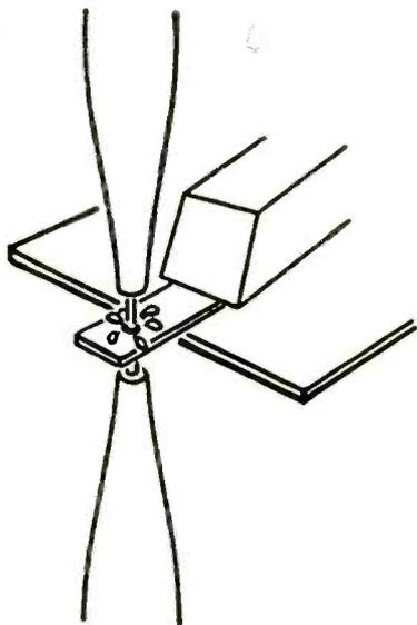
Glass nozzles direct jets of salt solution onto silicon wafer. Jets are negative for etching cycle, positive for plating phase
