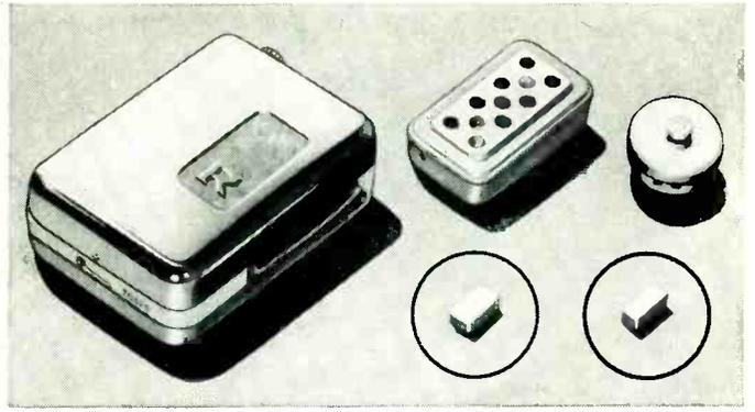
New all-magnetic, all-transistor hearing aid uses permanent magnets in both microphone and receiver. These tiny magnets eliminate hearing-aid failure caused by operational heat, and by humidity.
