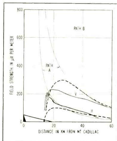
FIG. 3—Diffraction over knife edge with path A curves shown for comparison). Horizontal (H) and vertical (V) polarization. Frequency is 55 mc
