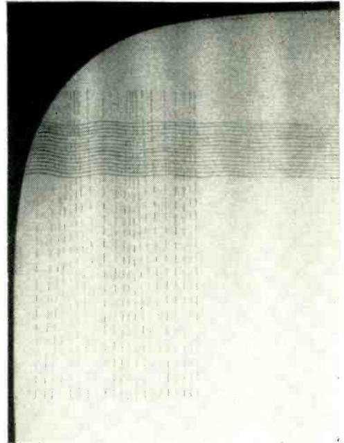
Television raster (left) displays unique appearance of horizontal deflection coil unbalance. Enlarged section of same raster (right) has scan lines emphasized and shows magnetic field lines
