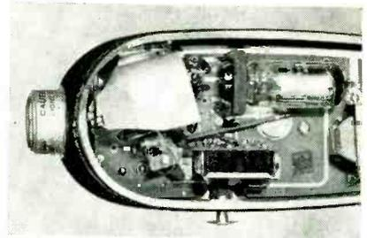
Switching assembly detail, tuning control and tuning loop
