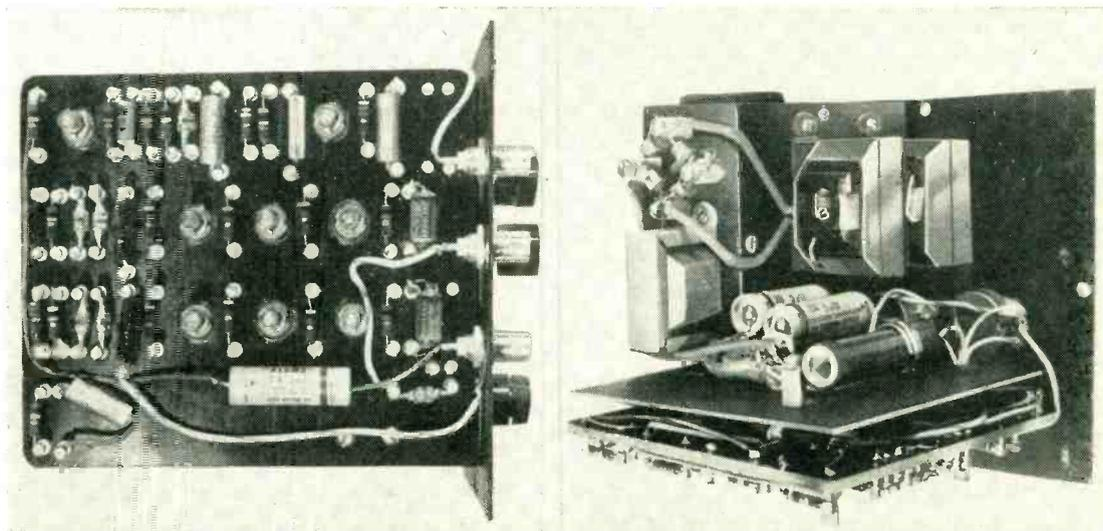
Bottom and rear views of complete pulser. Power supply with diode bridge is mounted on back of panel
