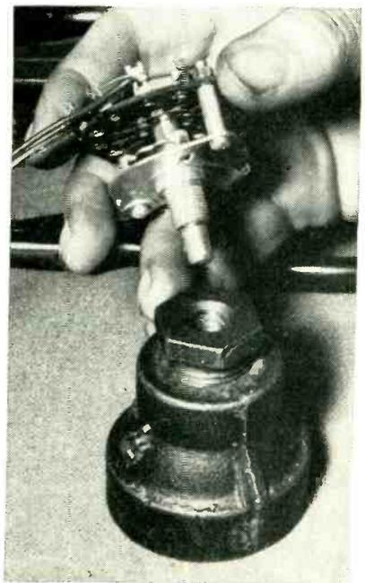
To load switch in pipe-nipple holding jig, operator inserts the assembly and gives it a clockwise spin
