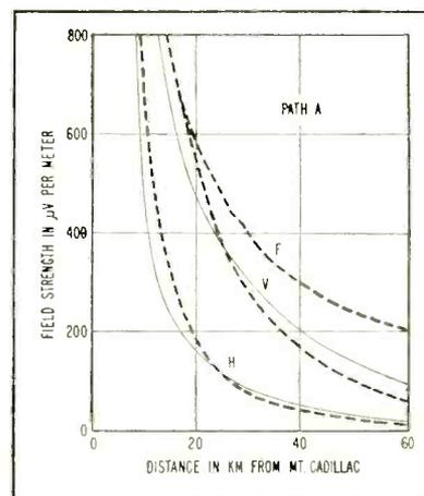
FIG. 2—Path A propagation at 55 mc over sea water. Dashed lines show computed values; free-space (F), horizontal (H) and vertical (V) polarization
