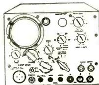
Provides four types of presentation (a) Panoramic (b) Aural (c) Oscillographic (d) Oscilloscopic. Designed for use with AN/ARR-7, AN/ARR-5, AN/APR-4, SCR-587 or other equipment with I.F. or 455 kc., 5.2 mc or 30 mc. Includes 21 tubes with 3" scope tube. PRICE \$99.50
