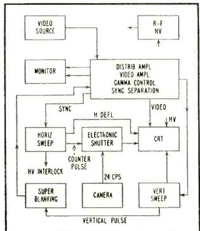
Block diagram shows interconnection of special tv recording system developed at Naval Research Laboratory
