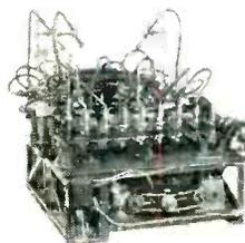
CR TUBE FACE PLATE SEALING
