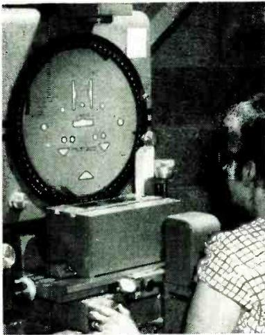
Checking locations and diameters of holes in mica spacers. Light from vertical illuminator at top projects shadow of mica resting on glass staging table
