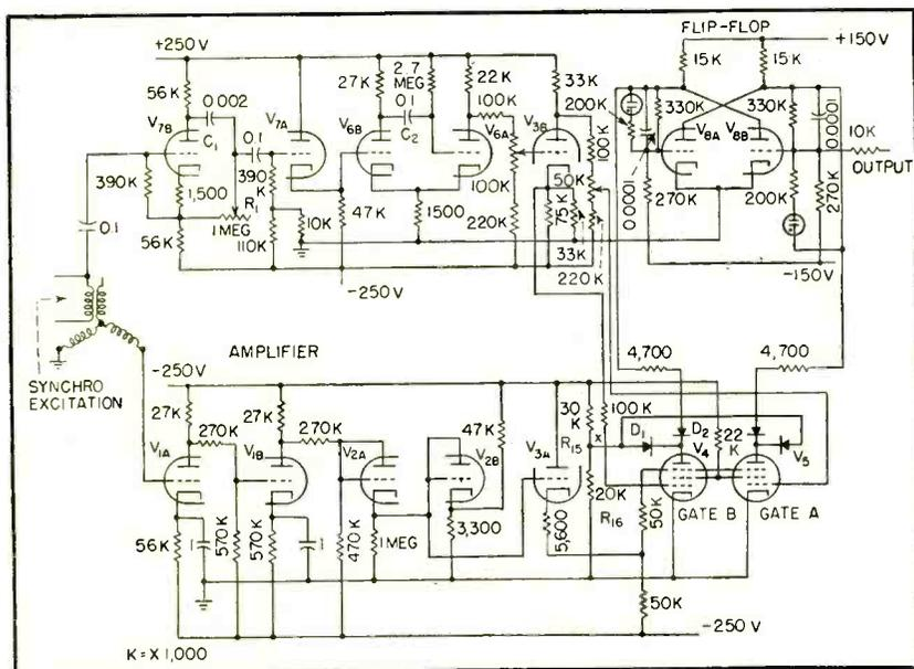
FIG. 2—Flip-flop triggered through two polarized gates generate marker pulses indicating shaft position
