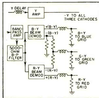
FIG. 8—Beam-deflection tubes supplying chrominance information from color decoder directly to picture tube
