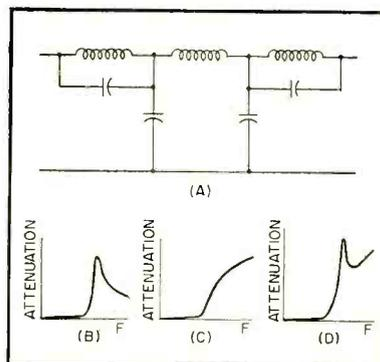
FIG. 2—Low pass filter (A) gives L-section response as in (B),  $\pi$ -section response as in (C) and combined characteristic (D)
