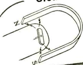
Patented Magnetic Calibrating Slug provides method of factory-adjustment of the timing through the glass envelope. All relays are calibrated after sealing.
