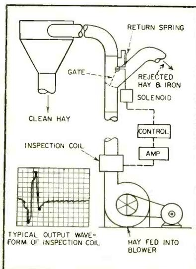
FIG. 1—Iron detector system
