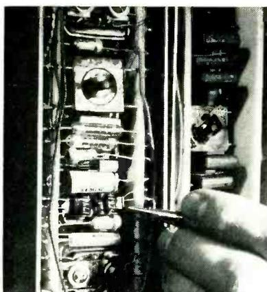
Two transistors are used in each oscillator subassembly for rural carrier telephone system
