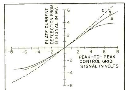
FIG. 6—Demodulator characteristics of 6AS6 (A) and beam-deflection tube with 0-signal cathode current of 10 ma (B) and 16 ma (C)
