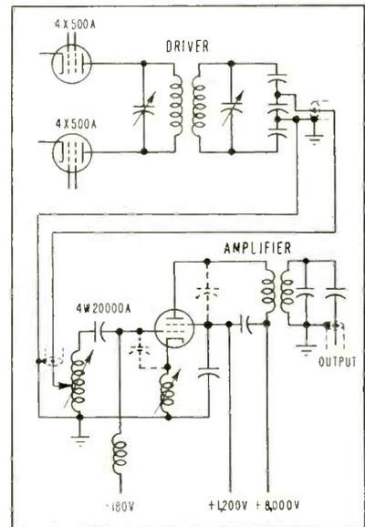
FIG. 1—Circuit of 25-kw amplifier showing coupling methods used
