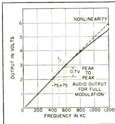
FIG. 4—Response of limiter and f-m detector showing deviation from linearity
