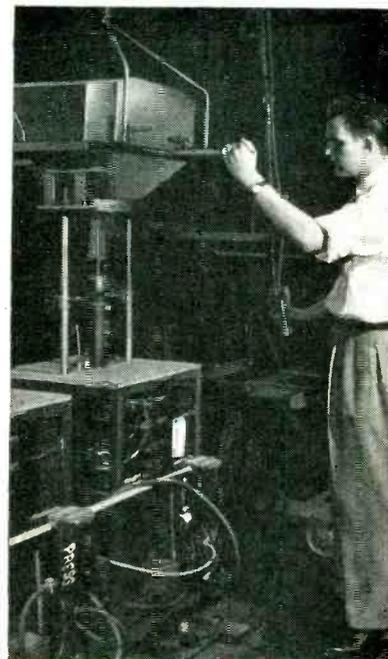
Lowering protected picture tube onto exhaust cart with overhead hoist having a fork-type lift
