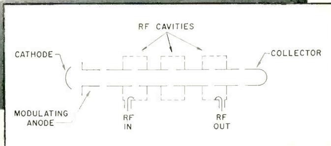
**A** new concept in klystron design is introduced by Eimac with the X557 modulating anode klystron. An insulated modulating anode placed between the cathode and drift tube section permits:
