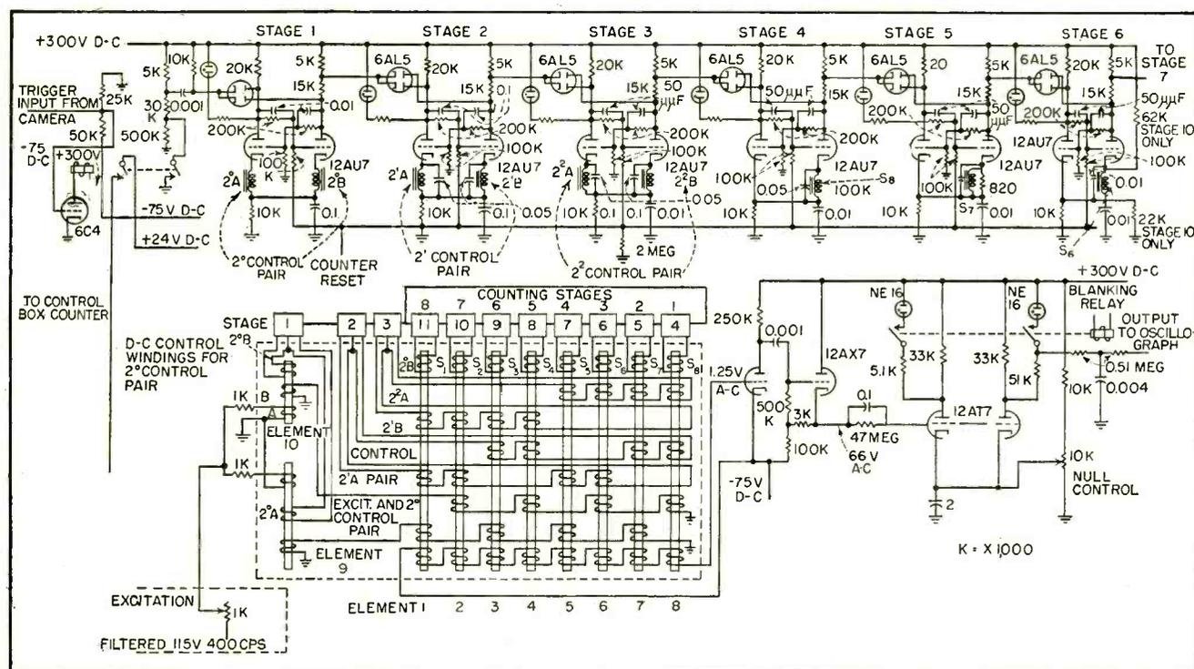
FIG. 3—Schematic diagram of electronic binary counter with magnetic-matrix switch readout. Unit is used in flight-testing airborne fire-control equipment
