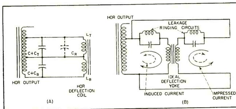
FIG. 2—Other means to combat deflection yoke ringing: connecting deflection coil center tap to center of output transformer (A) and connecting deflection coil windings in parallel (B)
