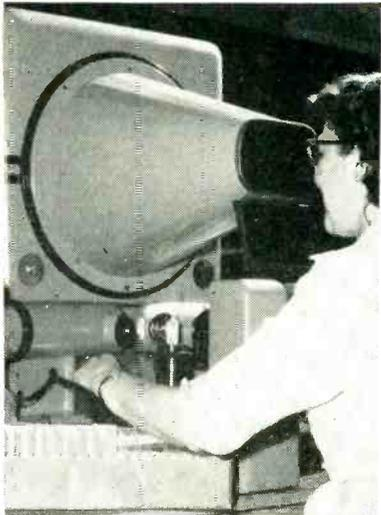
Special multiple-lamp contour projector used for inspecting tube assemblies prior to evacuation
