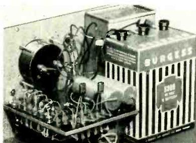
Integrator permits quick change of resistors to match transistor characteristics
