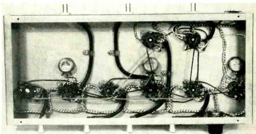
Wiring of main chassis is simplified by plug-in construction. Potentiometers control delay time
