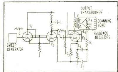
FIG. 2—Circuit of the broadband video amplifier employing feedback
