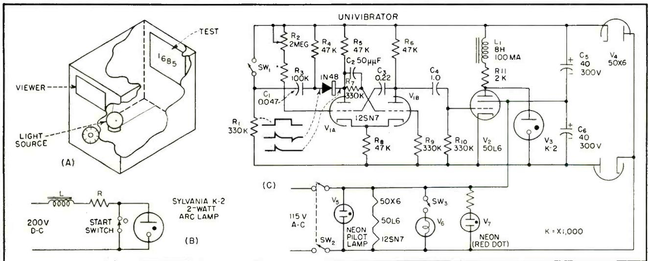
FIG. 1—Example of tachistoscope construction, simplified diagram of arc-lamp control system and complete control circuit
