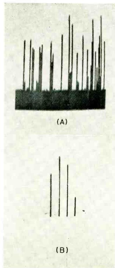
FIG. 1—Scope presentation of 88 pwm channels (A). Commutation system permits viewing selected groups of channels (B)
