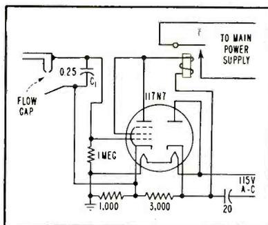
Safety interlock disconnects main power supply when water flow falls below 3 cc per sec
