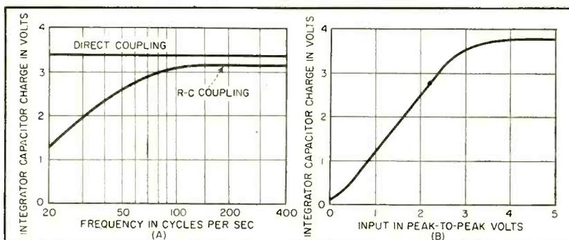
FIG. 2—Characteristics of direct and R-C coupling to transistor amplifier (A) and integrator capacitor charging characteristic (B)
