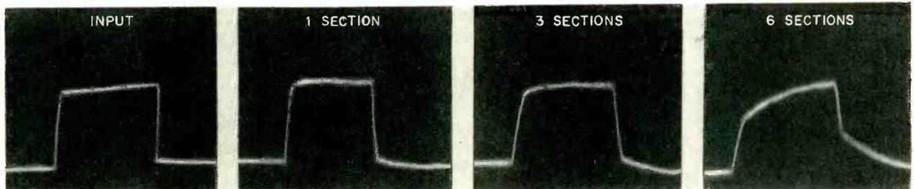
FIG. 2—Pulse distortion is reduced by inserting parallel resistance between delay line sections
