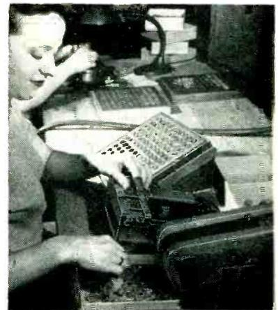
Wire-cutting setup, located at output of conveyor coming from stem machine. Bending machine is on same bench, in background
