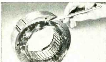
"Mylar" film used to insulate this motor stator is about half as thick as the material it replaces.
