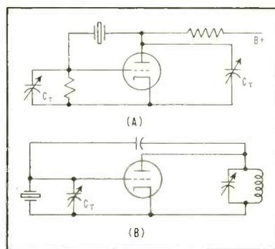
FIG. 1—Pierce oscillator circuit (A) and Miller circuit (B)
