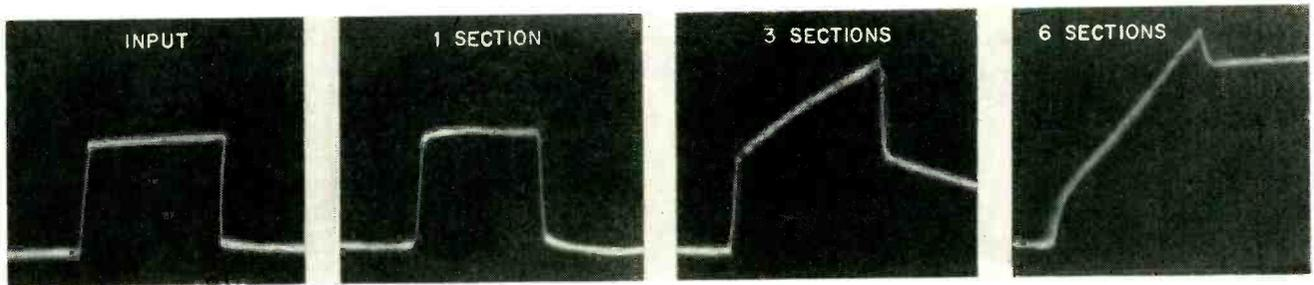
FIG. 1—Distortion of pulse shape after passing through various sections of cascaded delay line
