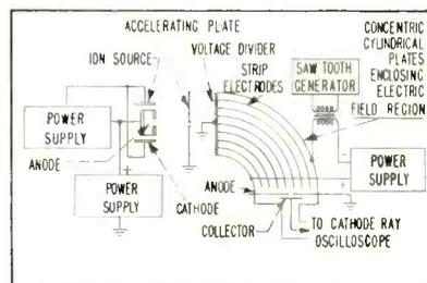
FIG. 14—Electronic portion of focused mass spectrometer
