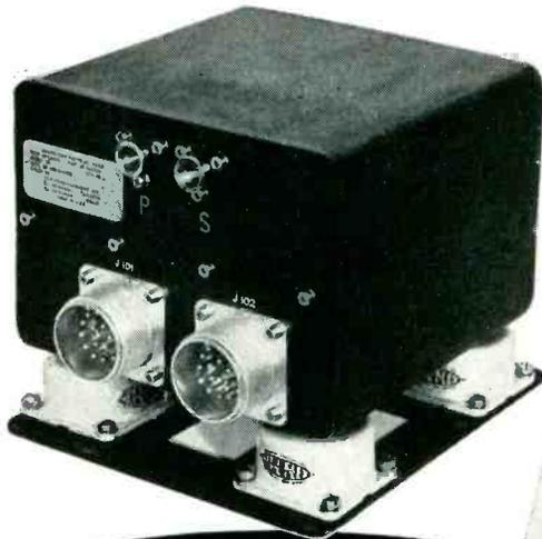
Pin-point accuracy, ruggedness and exceptional lightweight (4½ lbs.) are features of Servomechanisms' "Mach Master". This precision-built 400 cycle computer utilizes a force balance linkage to determine Mach number, thus eliminating vacuum tubes and other complexities. Pressure ratio is measured directly.
