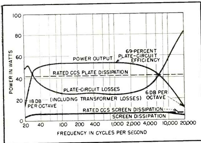
FIG. 10—Power characteristics at 2-percent distortion
