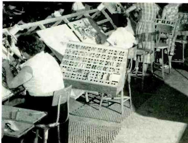
Bench setup in lacing board department, showing frames for supporting boards on bench and method of using pull-out breadboards to support tools and wire rack
