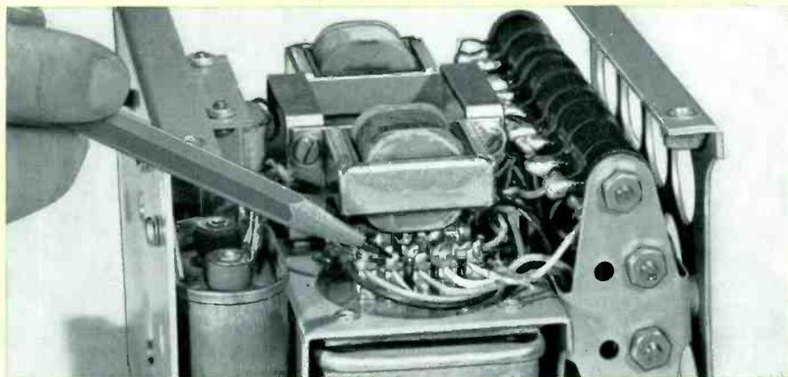
This Inverter Control Assembly, which regulates output of DC to 400-cycle AC converters, used in aircraft, contains miniature Tensolite wire coated with Du Pont "Teflon". The equipment, which utilizes two Regohm Circuit Controllers, was developed by Electric Regulator Corp., Norwalk, Connecticut. It easily withstands ambient temperatures encountered—from -70°C. to 85°C.—and operates efficiently at high altitudes, the manufacturer states.
