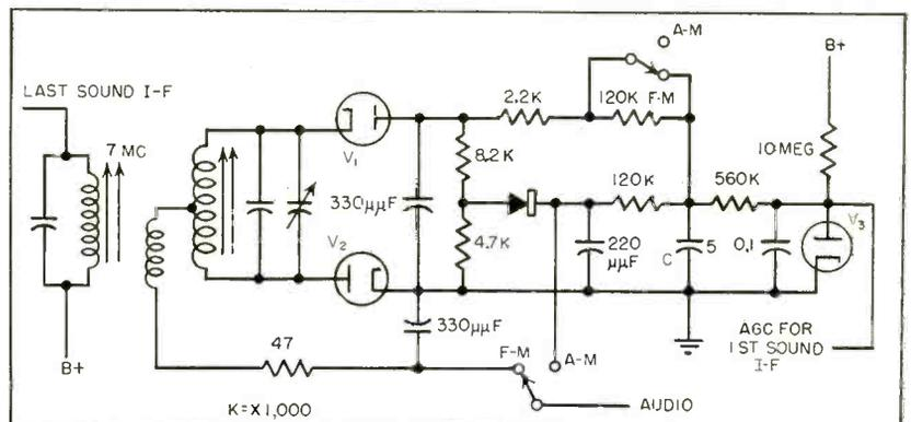
FIG. 3—Sound-detector stage uses diodes  $V_1$  and  $V_2$  in a radio-detector circuit tuned to the 7-mc sound i-f
