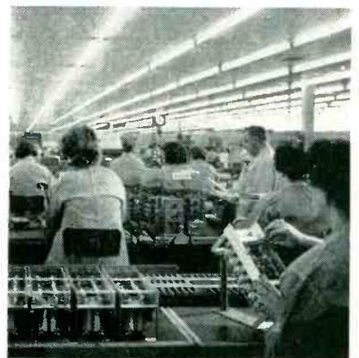
Production floor of new relay plant, showing method of installing fluorescent lighting on low ceiling to get shadowproof illumination
