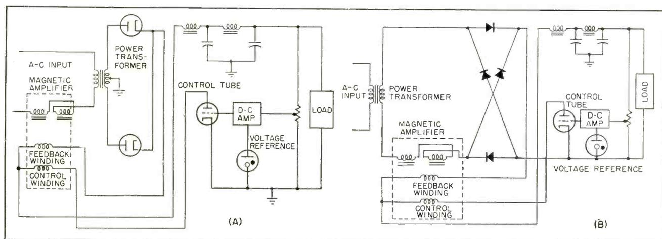
FIG. 1—Direct-current power supplies with L-input filters using magnetic amplifiers for regulation; full-wave (A) and bridge (B)
