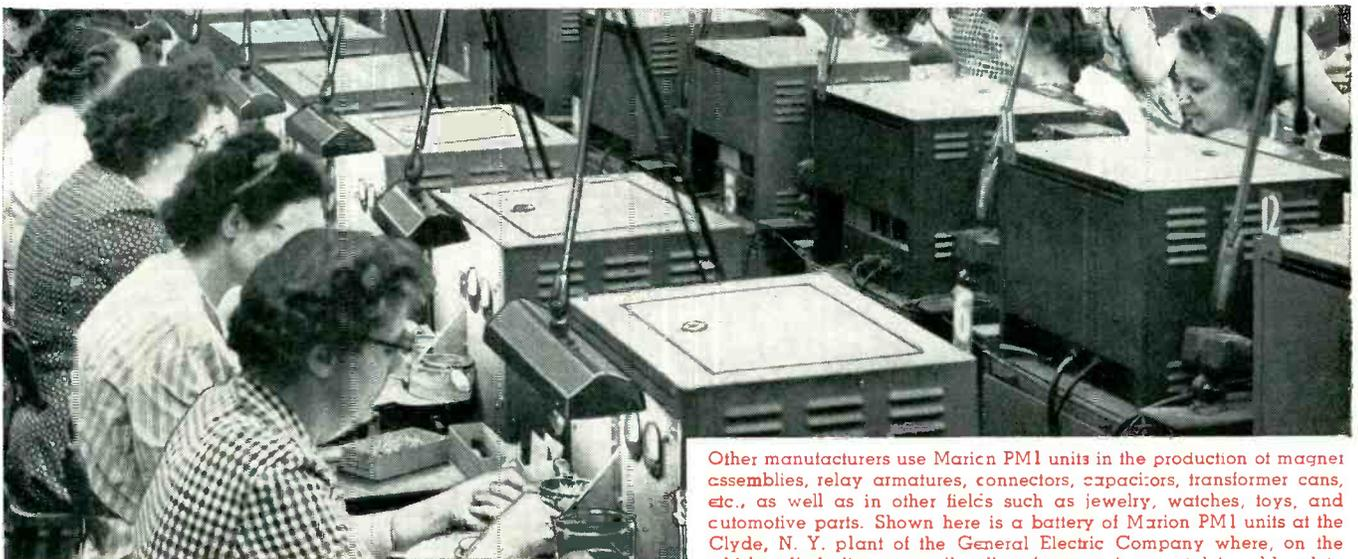
Other manufacturers use Marion PMI units in the production of magnet assemblies, relay armatures, connectors, capacitors, transformer cans, etc., as well as in other fields such as jewelry, watches, toys, and automotive parts. Shown here is a battery of Marion PMI units at the Clyde, N. Y. plant of the General Electric Company where, on the whisker diode line, a small pellet of germanium metal is soldered to the end of a nickel pin.
