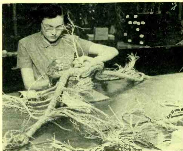
FIG. 5—Cabled wiring may often be required in military and commercial equipment. Operator at left is fabricating cable for a communications receiver. She lays wires on harness board, then binds them with linen cord. Operator at right is stripping ends of wires comprising cable for large radar set
