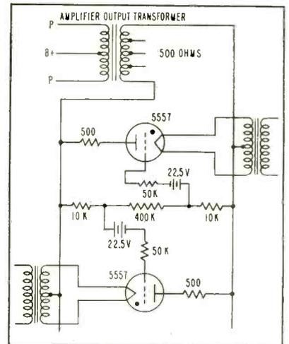
Thyratron circuit across 500-ohm tap of amplifier output transformer affords protection under no-load conditions
