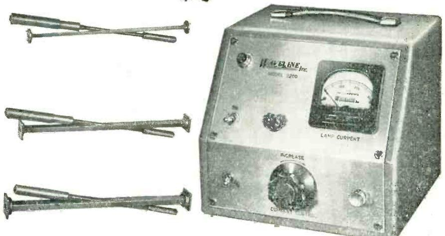
The WAVELINE Model 2200 microwave noise source—gas noise tube in combination with its Waveguide mount and power unit—provides a random noise source of known output level in the frequency range from 2,600 to 26,000 MCS. Throughout this range it also functions as an untuned termination.
