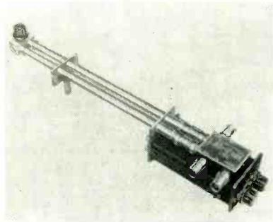
GENERAL RADIO CO., 275 Massachusetts Ave., Cambridge 39, Mass. Type 1000-P7 balanced modulator has a modulation-frequency response flat from d-c to 20 mc, thus making it suitable not only for short pulses but for any wide-band modulation. The usable carrier-frequency range extends from 60 to 2,300 mc and 100-percent a-m can be obtained throughout this range.
