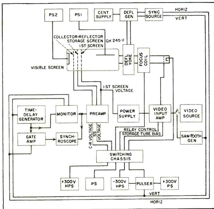
FIG. 3—Complete equipment arrangement for experimental operation and evaluation of magnetic-deflection storage tubes. System is sufficiently flexible to be adapted to most available storage and dark-trace tubes
