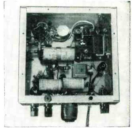
Underside of chassis shows simplicity of wiring and relay at upper right
