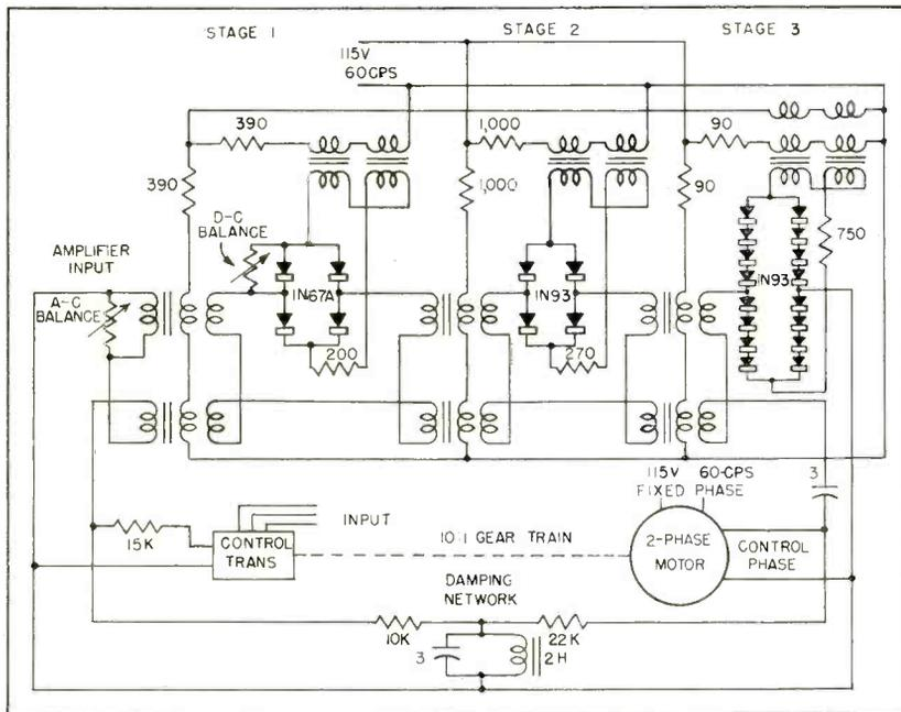
FIG. 4—Cascaded three-stage magnetic-amplifier circuit for servo-motor control
