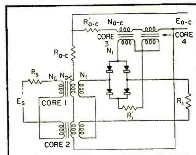
**FIG. 3—Magnetic amplifier circuit designed for full-wave operation**
