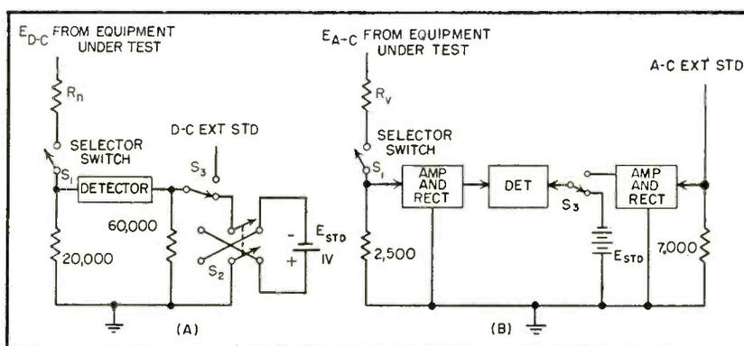
FIG. 3—Circuit of d-c voltage-test circuit (A) and a-c voltage-test circuit (B)
