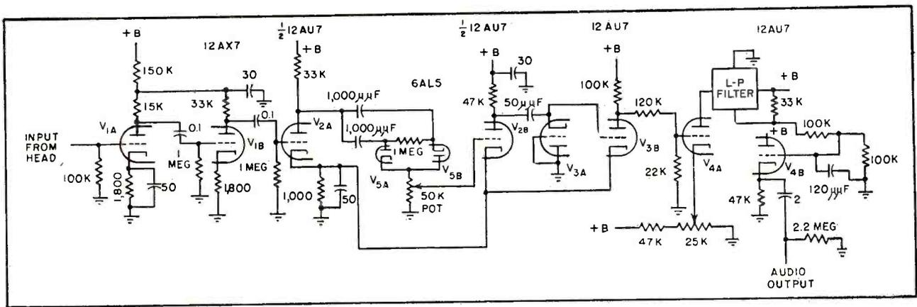
FIG. 5—Demodulator unit converts signal into pulse-width modulated train before demodulation in low-pass filter
