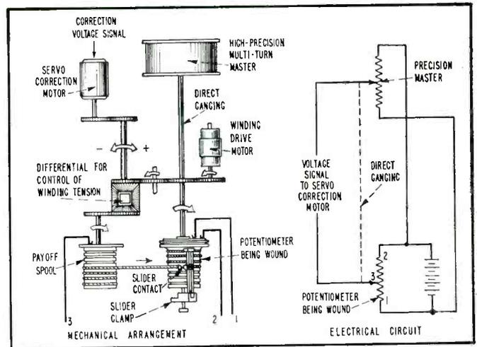
FIG. 5—Servo control system used by TIC to correct winding tension in accordance with error compared to master potentiometer
