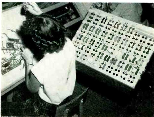
Storage rack for different lengths and colors of stripped wires used on lacing board. As many parts as possible are wired directly into the harness
