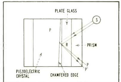
FIG. 13—Top view of piezoelectric structure
