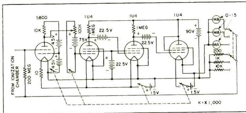
FIG. 2—Direct-current amplifier uses battery power to achieve portability for maximum usefulness in measuring Grenz rays
