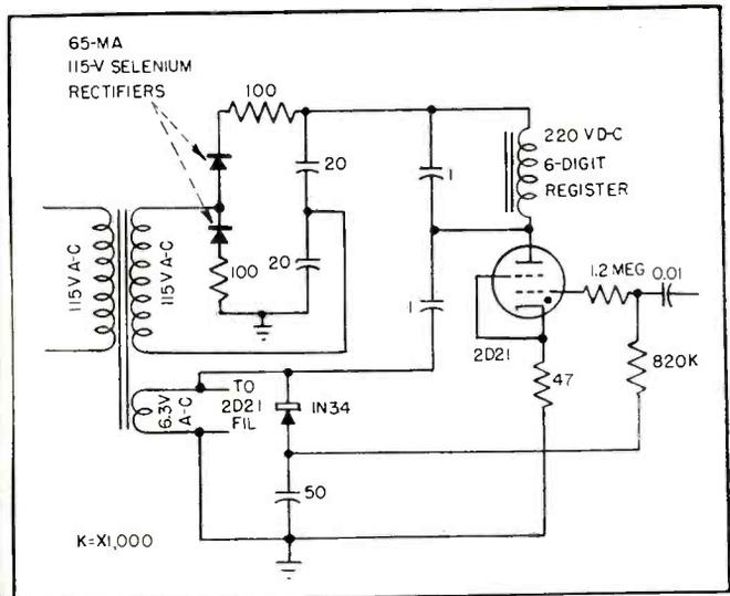
FIG. 8—Modification of circuit in Fig. 7 with power supply. Photograph shows complete unit mounted on 4 by 6 by 1½ in. chassis
