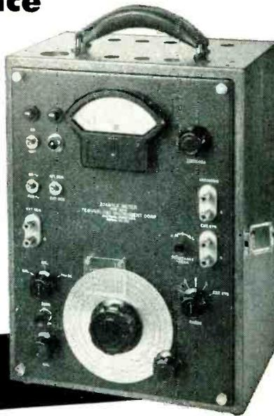
The type 310A Z-Angle Meter measures impedance directly in polar coordinates as an impedance magnitude in ohms and phase angle in degrees:  $Z/\theta$
