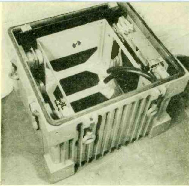
FIG. 6—Cabinet for radio transmitter designed to function under-water; gasket provides waterproof seal
