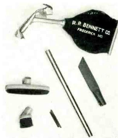
New model of industrial cleaner which operates from air line and takes all standard vacuum cleaner attachments
