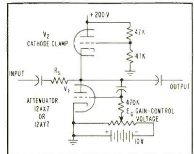
FIG. 3—Circuit providing 40 db attenuation with about 3 percent distortion
