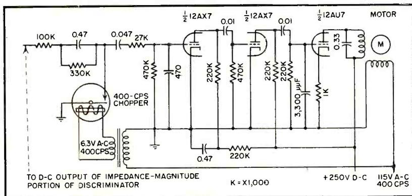
FIG. 5—Typical 400-cps servoamplifier used in matching unit adds phase shift
