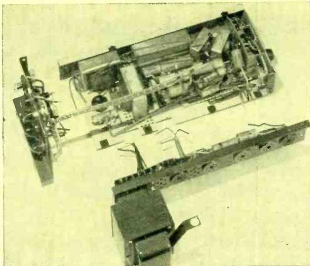
FIG. 4—Self-retaining U-shaped fasteners fit over edge of chassis to permit attaching dust cover
