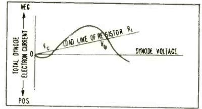
FIG. 2—Stable operating point  $V_b$  and 0 of secondary emitter
