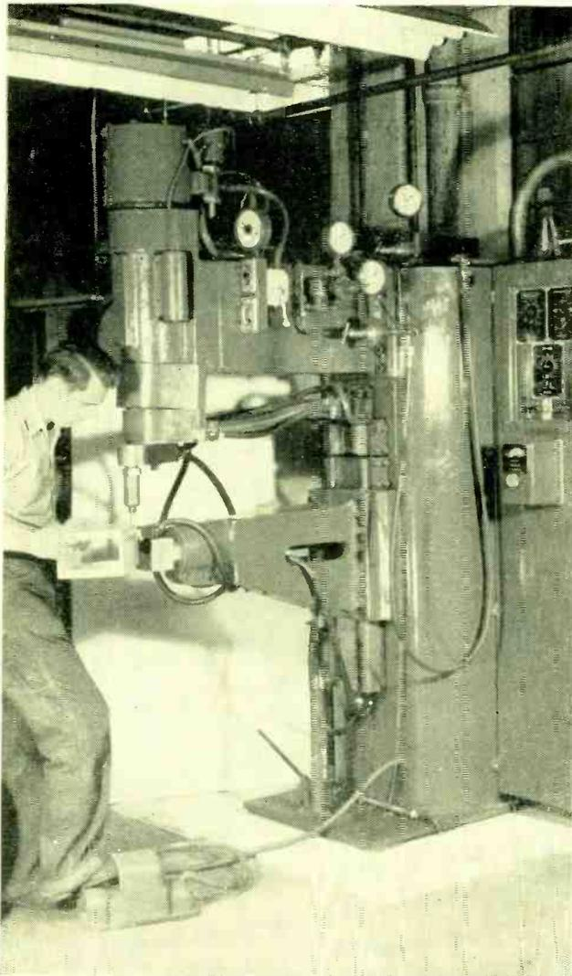
FIG. 12—Chassis work with resistance welding equipment
