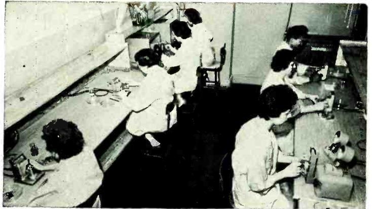
Inspection of all parts, sub-assemblies, as well as completed instruments, is a fetish at Ketay. For instance, all bearings are inspected with specially developed equipment in air conditioned work space. This is just one of the many techniques that assure maximum performance when Ketay units are specified.
