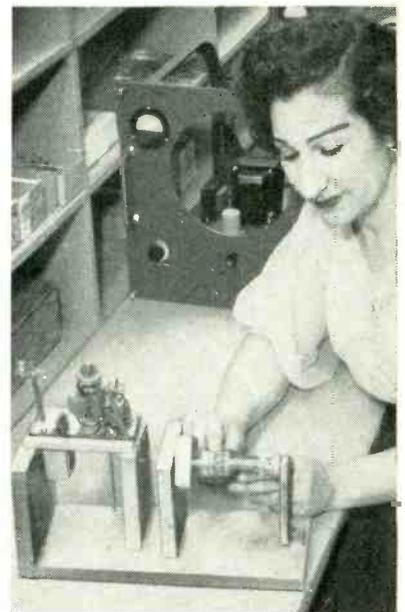
Method of using fixture for supporting turret socket during assembly. Finished chassis is shown in nest on other part of fixture
