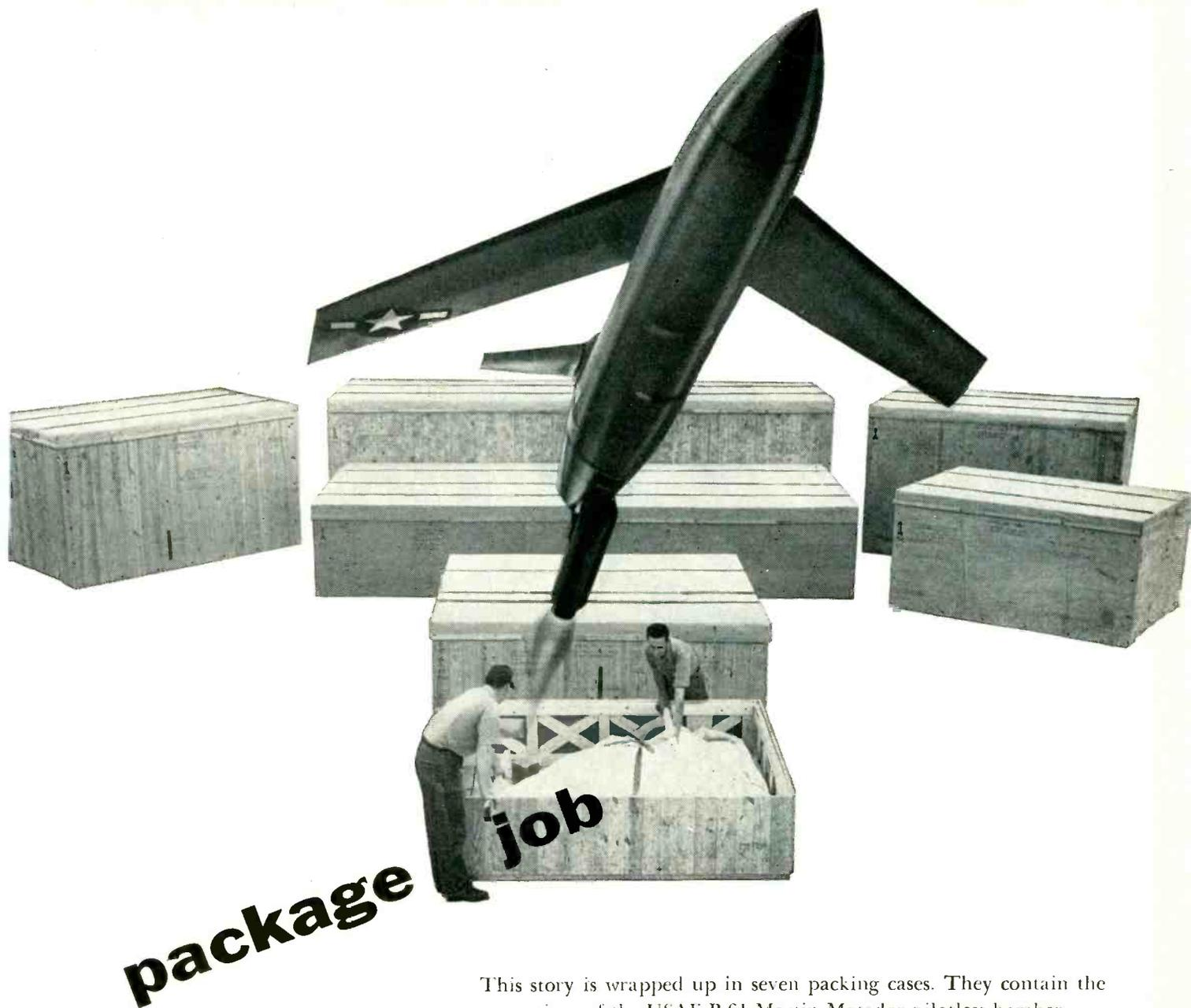
This story is wrapped up in seven packing cases. They contain the seven sections of the USAF B-61 Martin Matador pilotless bomber.
