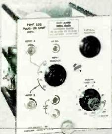
**TYPE 53B**— Same as Type 53A with additional calibrated ac-sensitivity to 5 mv/cm. . . . \$125
