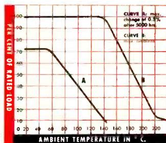
Typical derating curve for  $\frac{1}{2}$  watt Allies' Products carbon deposit resistors.
