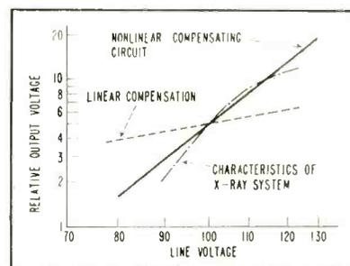
FIG. 4—Characteristic of three-stage compensator plotted against x-ray characteristic curve and curve of single-stage compensator
