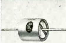
New IRC VARISTORS are voltage sensitive and provide sharp variation of resistance with applied voltage. Designed to meet most needs for non-linear resistors, they are available in 5 convenient cell sizes, and a complete choice of enclosures including hermetic seals.
