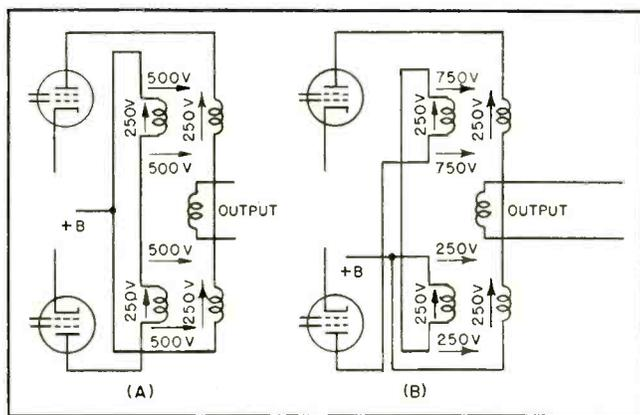
FIG. 2—Voltage relations in bifilar output transformer with different primary connections
