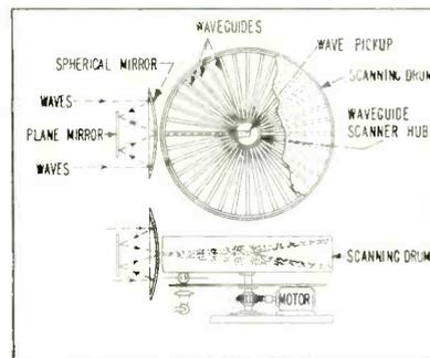
FIG. 3—Basis of microwave scanning system
