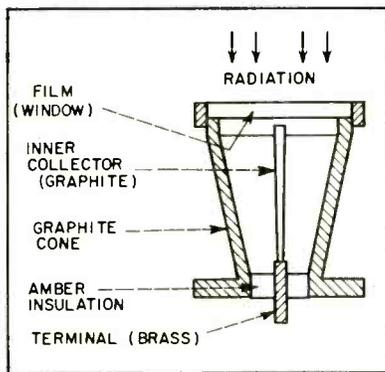
FIG. 1—Sectional view of ionization chamber used as sensing element
