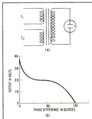
FIG. 1—Phase detector (A) uses double-winding filament transformer with neon bulb to indicate when two a-c signals are in phase. Graph (B) shows variation in output voltage with phase relationship
