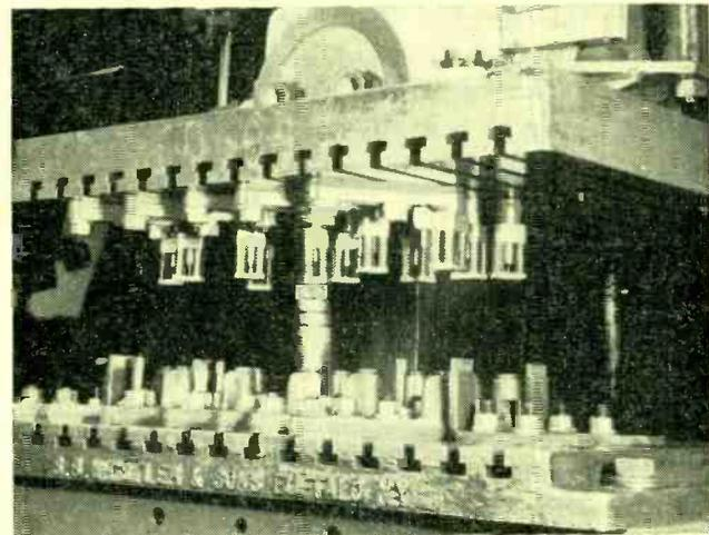
FIG. 4—Special punch and die sets (top, center) permit knocking out chassis with a single blow. Setup at right (bottom) is made with movable punches and dies bolted to die bed
