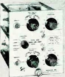
**TYPE 53C**—Dual-trace unit. Two identical amplifier channels, dc to 8.5 mc, 0.05 v/cm to 50 v/cm. Electronic switching triggered by oscilloscope sweep . . . or free running at about 100 kc. . . . \$275
