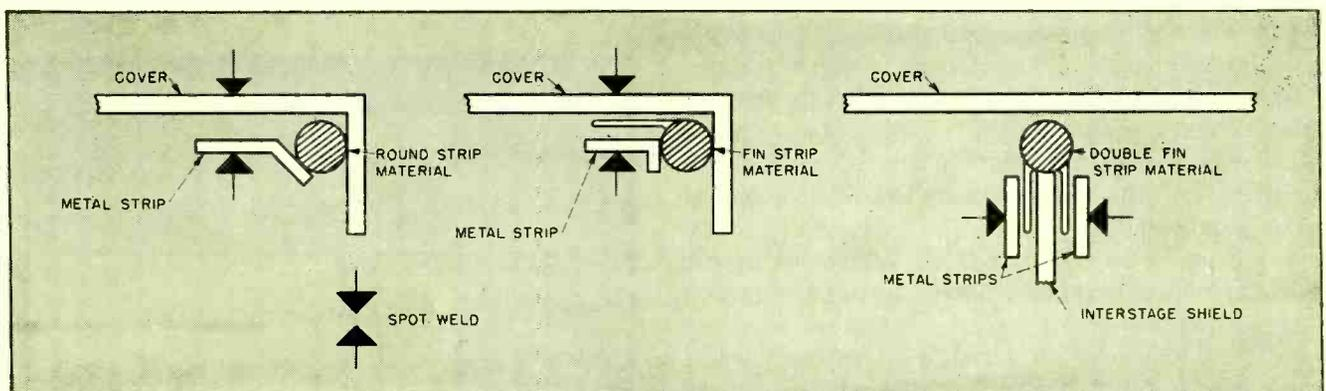
FIG. 2—Three ways to design electrostatic shielding. When shields are spot welded metal gaskets are compressed forming a tight radiation seal
