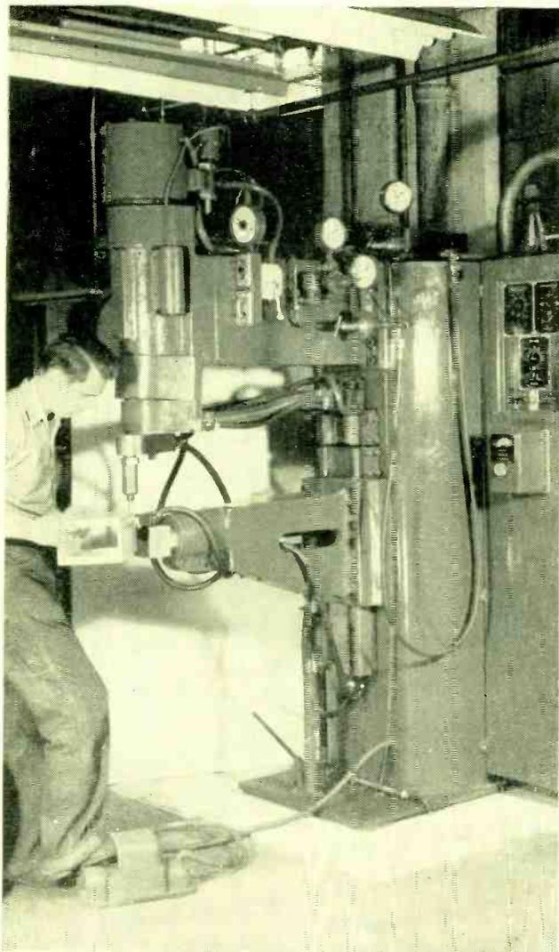
FIG. 12—Chassis work with resistance welding equipment
