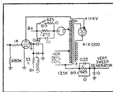
FIG. 8—Horizontal output stage
