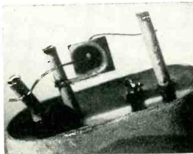
Heart of intrinsic barrier transistor as seen through microscope. Input and output electrodes are connected to the indium dots on opposite sides
