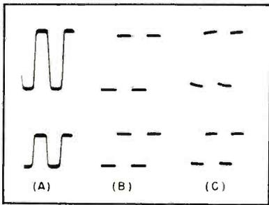
FIG. 7—Square-wave response of amplifier at 50 (A), 500 (B) and 5,000 cps (C). Amplifier input level is 40 watts for upper waveforms and 10 watts for lower waveforms
