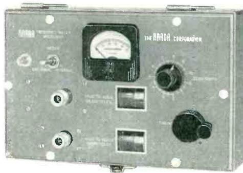
A self-contained instrument with two coaxial resonators tuned by a single control, type N input connectors, crystal detectors, and crystal current meter for resonance indication. Features 0.2% accuracy, high loaded Q, frequency reading from a universal calibration chart in the removable cover (not illustrated). No correction charts are required. The entire frequency range is free from spurious responses or other ambiguities.
