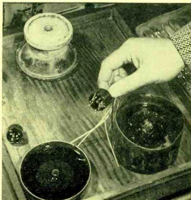
FIG. 10—Soldering of leads to octal plug is performed by first fluxing connections then dipping part in soldering pot, rear
