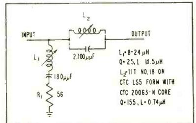
FIG. 1—Color remover filter for transmitter input
