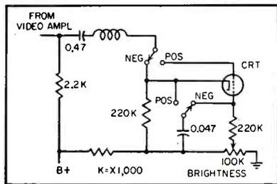
FIG. 4—Positive and negative modulation of the picture information in the four-system receiver requires switching arrangement shown
