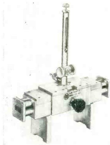
tion. The slotted sections are available in 4 waveguide sizes ranging in frequency from 2.60 to 12.40 kmc. They are designed to accommodate a broadband probe which can readily be replaced with a special micrometer probe quickly to change the unit to a variable susceptance transformer.
