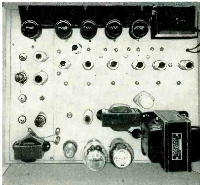
Front and top views respectively of experimental circuit consisting of one-mc strip, 100-kc circuit and three 30-kc circuits
