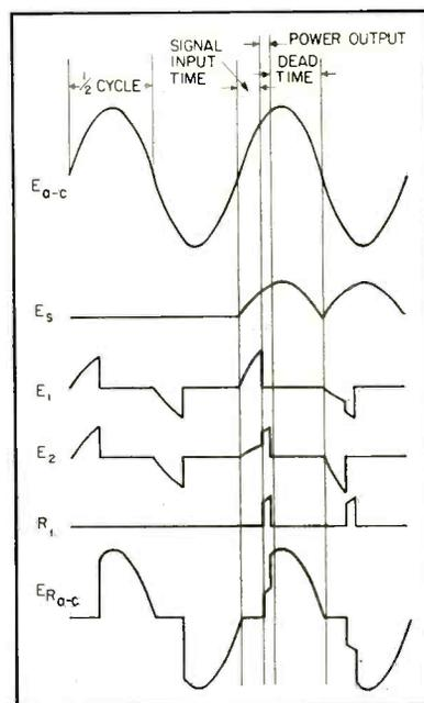
**FIG. 2—Waveforms in high-speed amplifier circuit of Fig. 1A**
