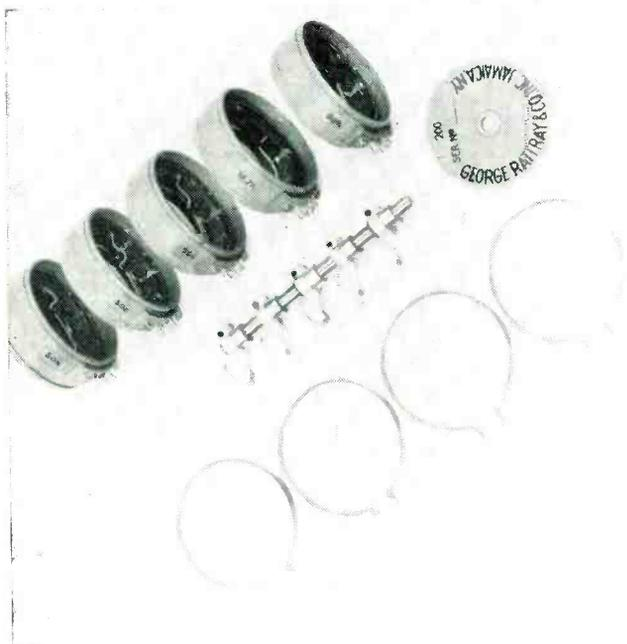
Typical assembly of ganged potentiometers, as made by George Rattray & Co. Inc. All wipers mount on single shaft to avoid backlash. Clamp rings enable units to be phased individually
