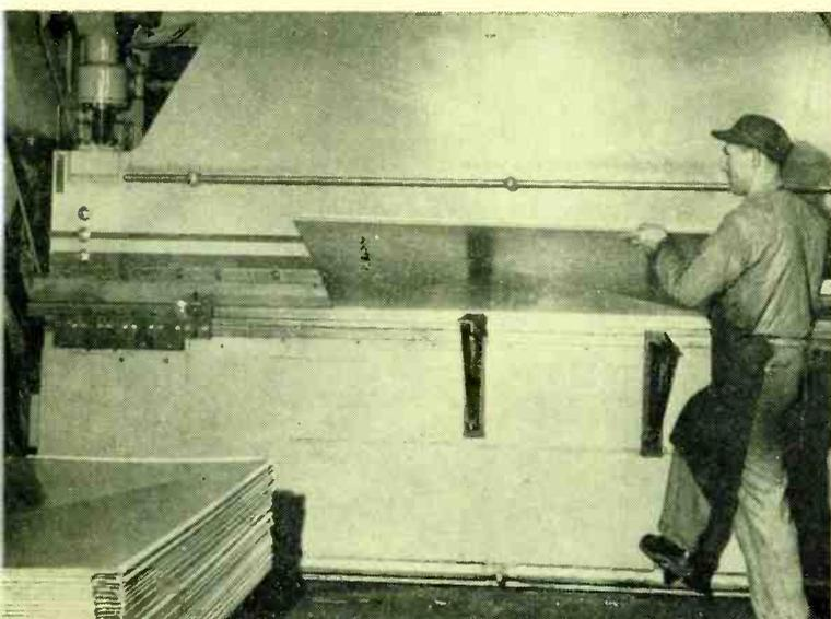
FIG. 7—Power brakes accomplish heavy bending operations on sheet metal
