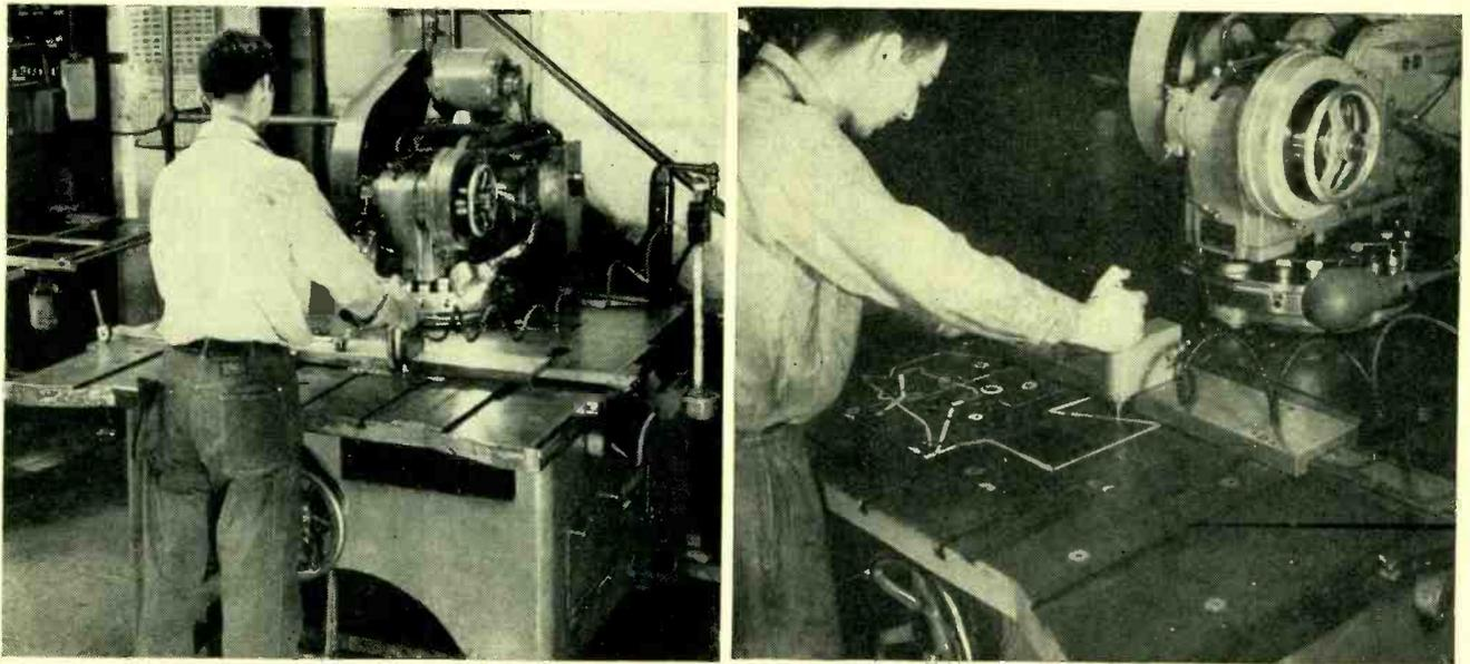
FIG. 5—Punching chassis with turret press, left. Model at right uses pantograph and template
