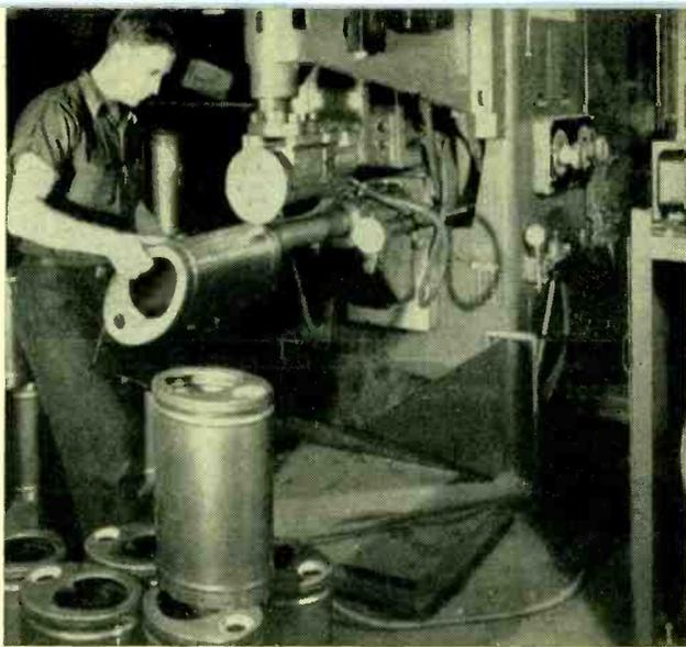
FIG. 7—Seam welding. This resistance-welding process can provide a liquid-tight joint
