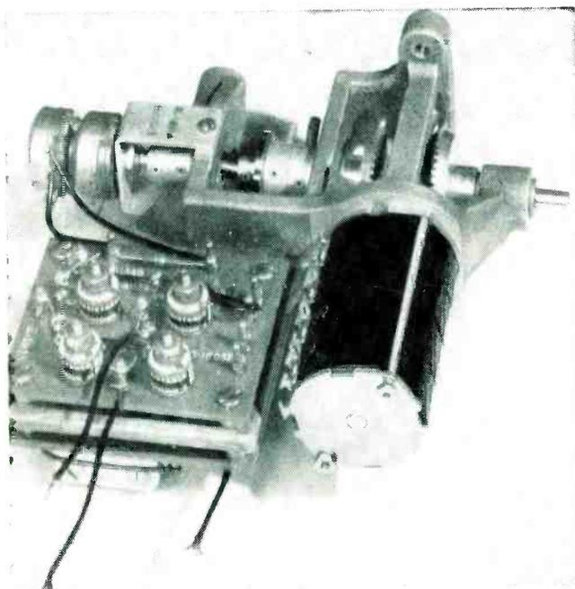
Typical Fairchild servo application uses ganged precision potentiometers at right for accuracy and general-purpose potentiometers at left for gross control
