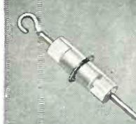
New IRC Feed-Thru Terminals are designed for assured hermetic sealing for electrical and electronic components. IRC's exclusive molding technique bonds KEL-F\* to metal in a superior, consistent hermetic seal. Molded bodies are chemically inert to solvents, acids, alkalis, etc., and have high resistance to thermal shock (-70°C. to +190°C.) HS-1 Terminals meet the sealing requirements of MIL-T-27.
