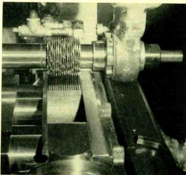
FIG. 2—Ganged carbide-tipped cutters mill 32 cooling-fin slots in magnetron shell. Sixteen slots are cut at a time. Tolerance is on width  $+0.002$ ,  $-0.002$  and  $\pm 0.005$  for depth and location
