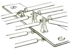
Make speedy, flexible wiring terminals.
