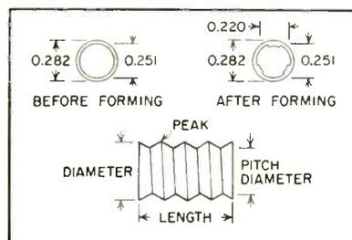
FIG. 3—Typical embossed form and V-type core
