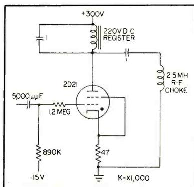
FIG. 7—Register driving circuit employs 2D21 miniature thyatron
