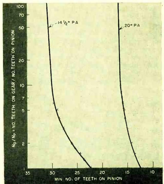
FIG. 5—Interference effects in gears
