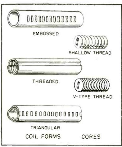
FIG. 1—Types of internally threaded coil forms and mating threaded iron cores
