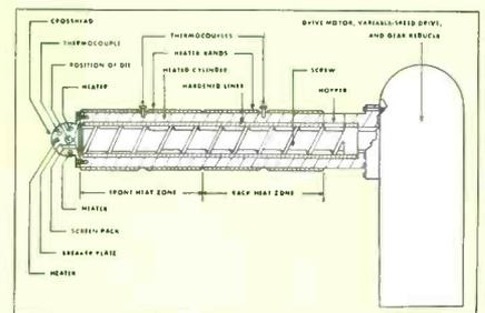
Components of typical screw extruder which might be used to extrude "Zytel" nylon resin.
