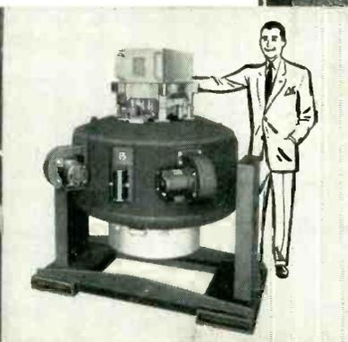
**MB MODEL T-25 MC CONTROL CABINET** with automatic cycling system developed to control the action of vibration exciters to a specified cycle of events, and with little or no supervision.
