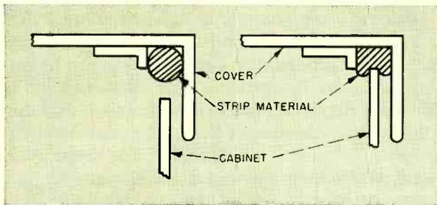
FIG. 1—Wire-mesh gasket around top of cabinet is compressed when lid is closed and forms radiation-proof electrostatic shield
