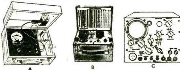
Fig. A **FLUXMETER.** Measures field strength of magnets from 500 to 4000 gauss. Indicates polarity. Probe gap 1/4". British handcraft in fine hardwood case with hinged cover. Operating instructions on underside of cover. Size 12-3/4 x 9 x 6 in. A lab instrument. Also ideal for classroom magnetics instruction. \$24.50
