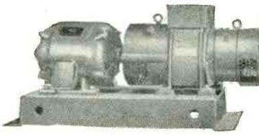
**Bogue Laboratory 400 Cycle Supply.** Motor 7.5 HP, 220/440-3-60 direct-coupled to self-excited alternator output. 5 KVA, 120/208 V, 3φ, 400 Cy. Voltage regulated. Harmonic content less than 1%. NEW. \$1475.00
