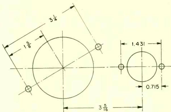
FIG. 2—Close-tolerance dimensions are given decimally, while wider tolerance dimensions are given fractionally
