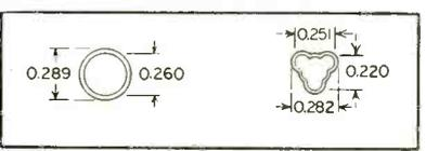
FIG. 2—Typical triangular or cloverleaf type coil form
