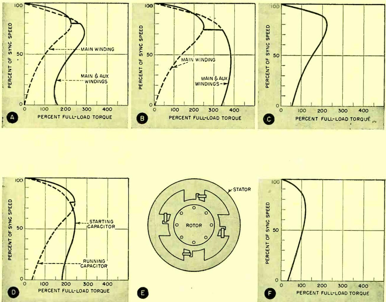
FIG. 3—Single-phase motor characteristics. Curves illustrate split phase (A), capacitor start (B), permanent split (C) and capacitor start-capacitor run (D) motors. Configuration and characteristics of shaded-pole machine are given in (E) and (F)
