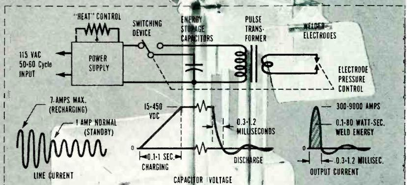
Ultra-short current pulse permits welding Copper, Silver, Magnetic Alloys and most other metals. Welds wires, tabs, lugs, posts and other parts instantly. Eliminates solder, flux, brazing, rivets, etc.
