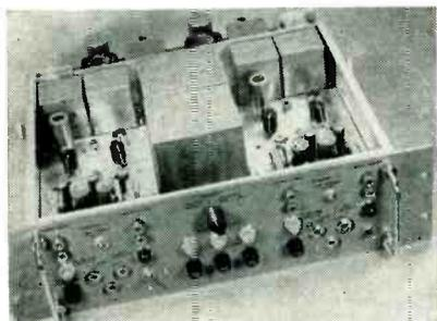
FIG. 2—Channel transmitter drawer is typical of chassis construction
