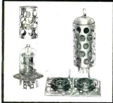
"Ventikator" shields not only improve "hot" tube performance by dissipating heat but are the most economical shields in Methode's extensive line. Easily handled and compression fitted to ground terminals on Methode laminated or printed circuit sockets, shields are available in lengths of 1-11/16" or 2-1/16" with one standard diameter which fits either seven or nine pin tubes. Available with tin or black oxide finish.
