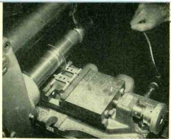
**MAKING SMALL PARTS** requires processes such as machining, casting, brazing and welding. Operator pictured uses a hand milling machine to trim rods on variable capacitor
