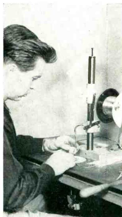
Soldering setup in which iron mounted vertically under bench moves up to work when foot pedal is pressed. For some operations, the iron can be rigid in this mounting with foot pedal serving only to feed solder
