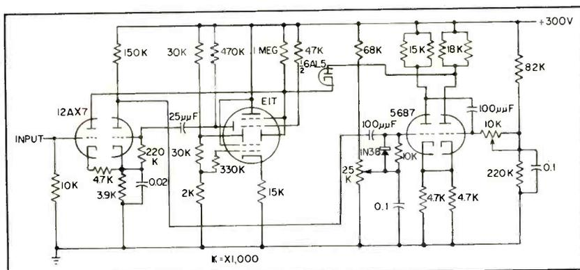
FIG. 9—Experimental one-mc scaling unit. Further development is needed to make circuit reliable enough for routine use
