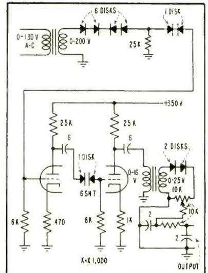
FIG. 3—Circuit of three-stage nonlinear compensation circuit
