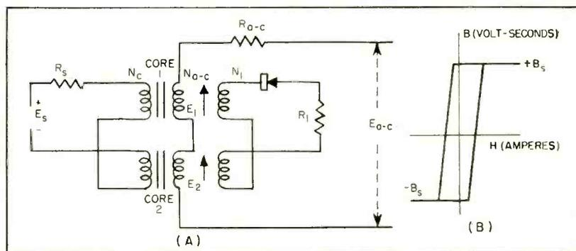
FIG. 1—Basic circuit (A) of high-speed amplifier and idealized hysteresis loop for core material (B)
