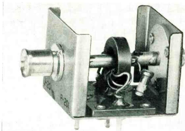
Discriminator is formed from transmission line surrounded by powdered-iron toroid to which is coupled five-turn, center-tapped loop
