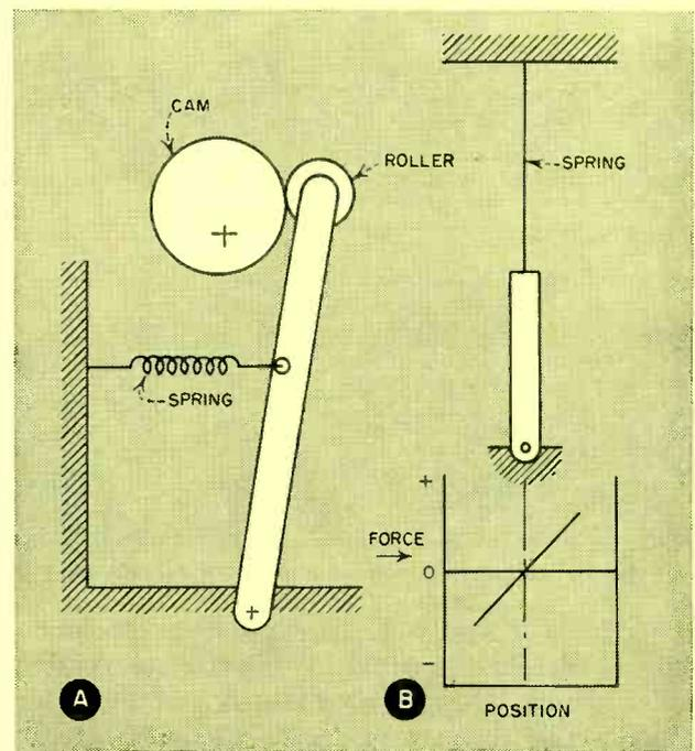
FIG. 6—Use of springs in electronic equipment: to keep roller in contact with cam (A) and as a self-centering device (B)
