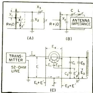
FIG. 3—Autotransformer combines properties of two T-sections (A), complete impedance-matching network (B) and discriminator for sensing phase and impedance (C)
