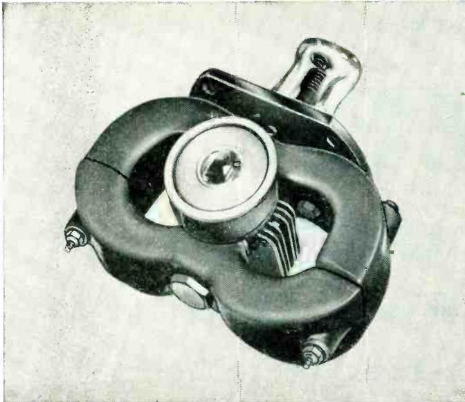
**Search Radar Magnetron Tube.** Two large Carboloy Alnico permanent magnets supply the electron beam control in this Raytheon magnetron. They help reduce size and weight, with no decrease in performance.
