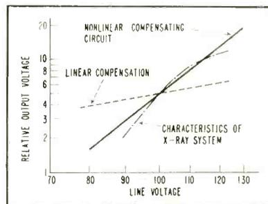
FIG. 4—Characteristic of three-stage compensator plotted against x-ray characteristic curve and curve of single-stage compensator
