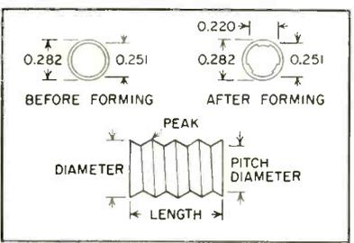
FIG. 3—Typical embossed form and V-type core
