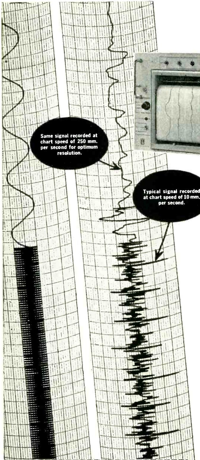
Same signal recorded at chart speed of 250 mm. per second for optimum resolution.
