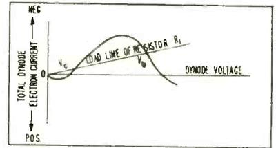
FIG. 2—Stable operating point  $V_b$  and 0 of secondary emitter
