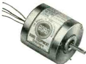
Two phase, 115 volt, 400 cps induction type Borg-Motors for servo control applications. Approximate size 1½" diameter x 2" long with a locked rotor torque of 0.82 ounce-inch.
