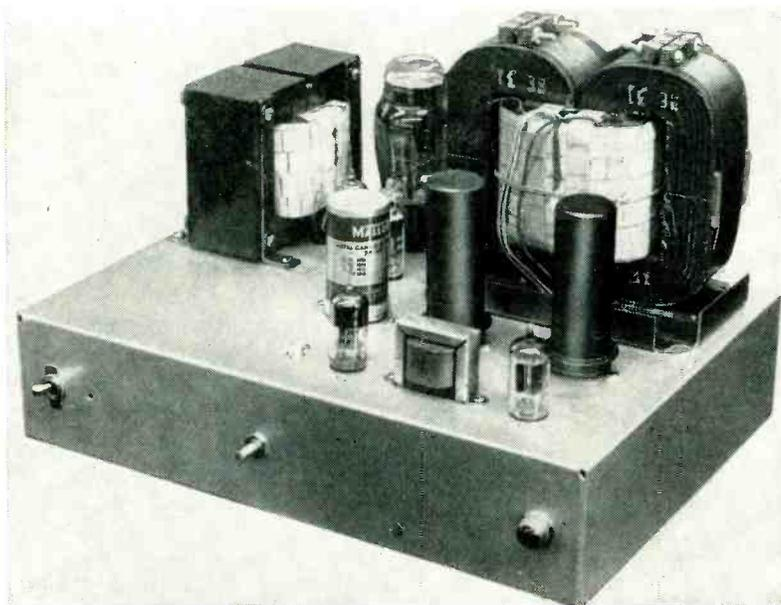
Fifty-watt amplifier uses 1614 output tubes. Output transformer is shown mounted on chassis in its normal position, but not potted
