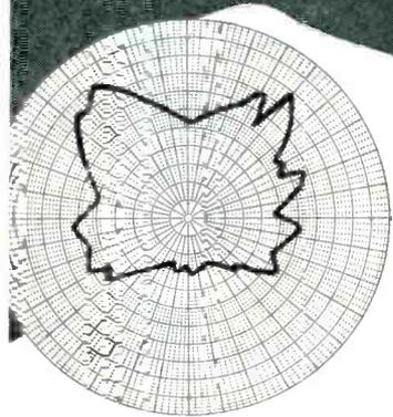
Spherical radiation patterns for antennas automatically drawn in standard polar coordinate form.
