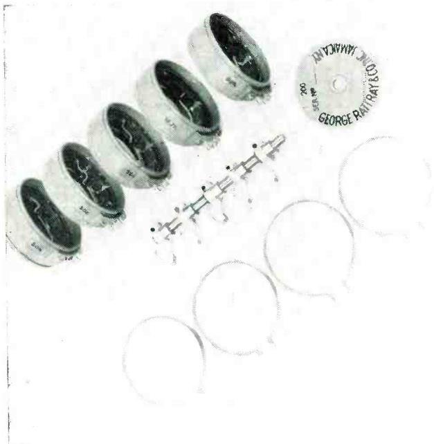
Typical assembly of ganged potentiometers, as made by George Rattray & Co. Inc. All wipers mount on single shaft to avoid backlash. Clamp rings enable units to be phased individually
