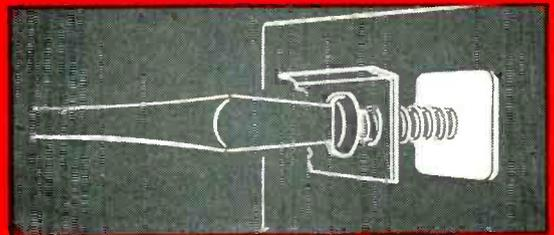
Ordinary sheet metal screw cuts its own threads as it is driven into the nut, expands fingers, locks nut and screw securely.
