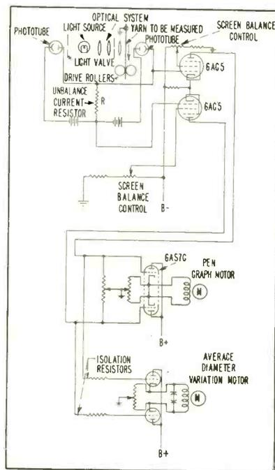
FIG. 5—Circuit of the photometric yarn measuring device
