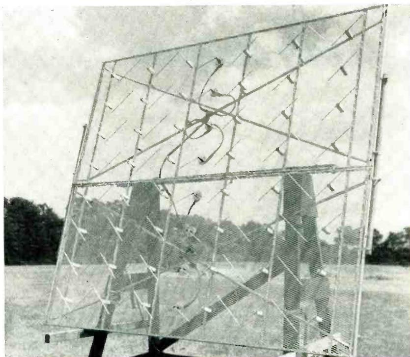
Receiving antenna made up of eight zigzag rods receives weak television signal 37 miles from the WJTV transmitter in Jackson, Miss. Signal is amplified and rebroadcast from low-power RCA transmitter attached to similar high-gain antenna to fill holes in coverage area of this uhf television station
