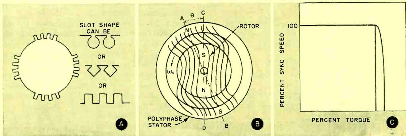
FIG. 4—Rotor lamination of four-pole reluctance motor (A), magnetic field (B) and speed-torque curve (C) of hysteresis motor
