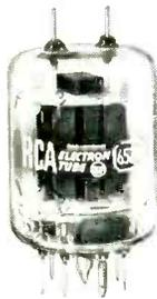
RCA-6524 is a new twin-beam power tube well-suited for fixed and mobile UHF design—as a balanced push-pull rf power amplifier or frequency tripler. The tube can deliver 20 watts (approx.) in class C cw and fm services—at 462 Mc! Max. plate dissipation is 25 watts (ICAS). A common cathode for the two units reduces cathode inductance to a negligible value.
