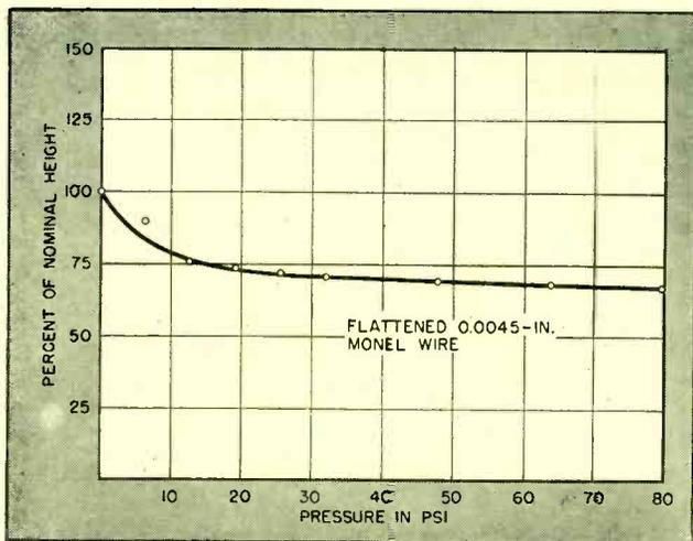
FIG. 4—Deflection characteristics of wire-mesh gaskets (Metal Textile Corp.)
