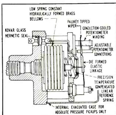
FIG. 6—Hermetically sealed potentiometer made by Trans-Sonics, Inc. is actuated by gas or liquid pressure through bellows and bearing-free linkage; resolution is 0.33 percent of full scale
