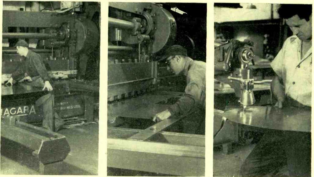
FIG. 3—Sheet-metal shearing. Operations shown are conventional shearing (left), front shearing (center) and use of circle shears (right)
