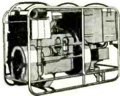
400 cycle, single phase, 115 volt, 60 cycle, single phase, 115 volt. Delivers 2500 watts each, both freqs. can be used simultaneously for total 5000 watts. 400 cycle generator is permanent mag. type. Power plant is Hercules 4-cyl., water-cooled, short block engine. Complete control panel incl. Running time, cycle, voltmeter, temperature and oil pressure gauges. 1700-1725 RPM. Wt. approx. 500 lbs. .... \$350.00 ea.
