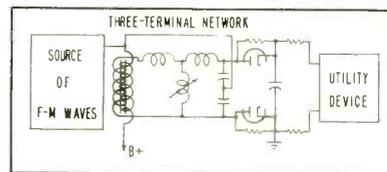
FIG. 6—Frequency discriminator uses network and unity coupling
