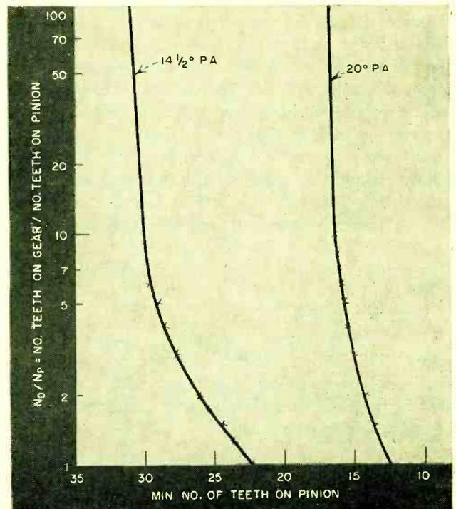
FIG. 5—Interference effects in gears
