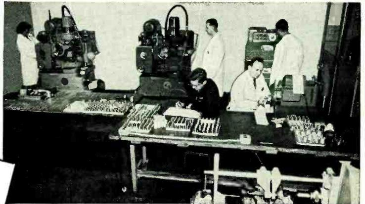
Precision of manufacture is vital in every Ketay unit. To assure continuing reliability for its products, Ketay employs the very latest facilities and techniques. Typical is this "gear room" where modern gear cutting machinery produces gears to the finest of tolerances.
