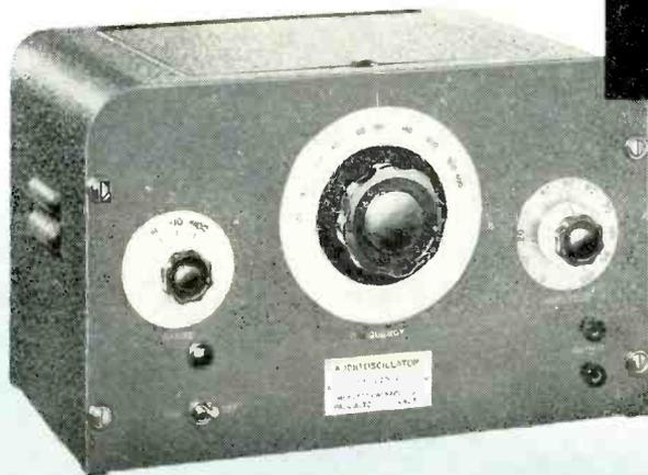
In 1939, *-hp-* designed and manufactured the first commercial RC (resistance-capacity) oscillator. Today, this type is recognized as the most versatile, practical, dependable and convenient of all oscillators. Through the years, *-hp-* RC oscillators have become world-famous for their high stability, accuracy, wide frequency range and compact size.
