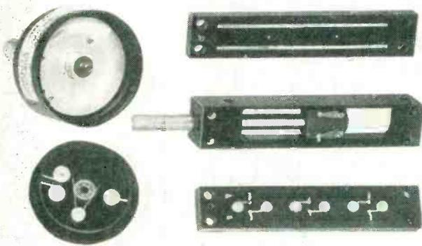
Markite conductive plastic rotational and strip-type translational potentiometers provide long life and infinite resolution. For strip-type unit, taps molded into back of resistive element (bottom) leave conductive track (top) clear for slider in center
