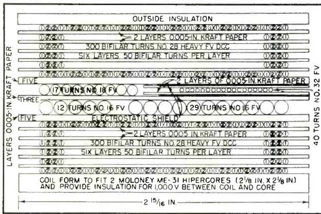
FIG. 3—Output-transformer coil buildup for fifty-watt amplifier using 1614 tubes
