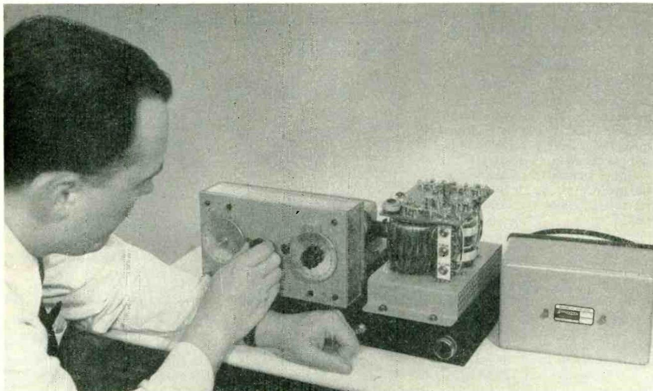
Response time of magnetic amplifier can be cut to less than a half cycle of the line frequency
