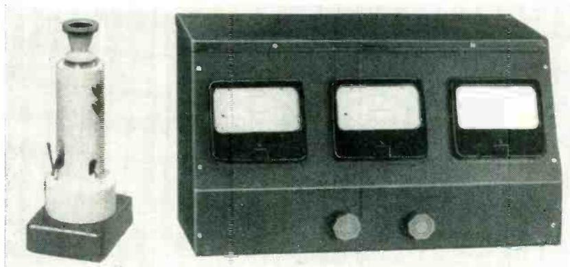
Saturation current of graphite ionization chamber (left) produces a meter indication proportional to roentgens per minute. Three meters prevent reading wrong scale
