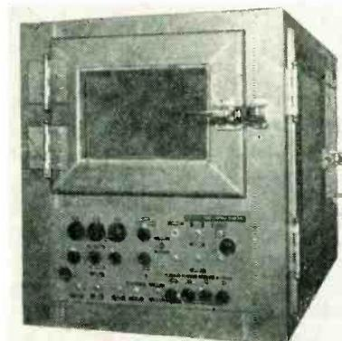
FIG. 4—Shielded enclosure contains storage tube and readout preamplifier
