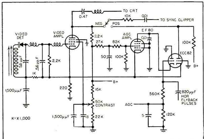
FIG. 5—The agc voltage, with negative modulation, is determined by the sync-level of the video signal across the cathode resistor of the video-output tube
