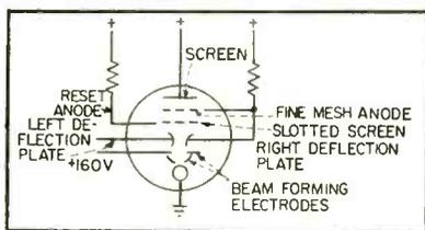
FIG. 1—The E1T decade scaling tube
