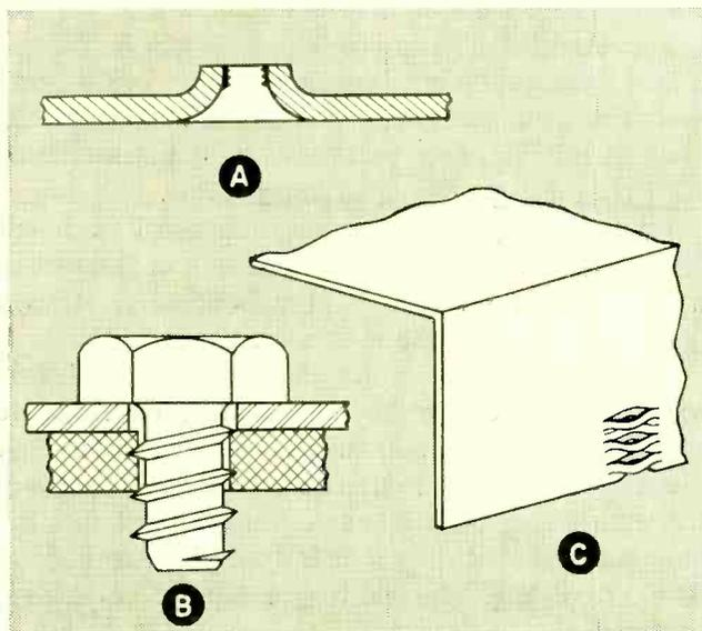
FIG. 9—Holes extruded in sheet metal can be threaded (A), self-tapping screws utilized (B) or the chassis lanced at its edge (C)
