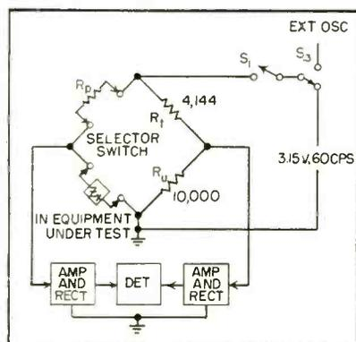
FIG. 2—Impedance-test circuit
