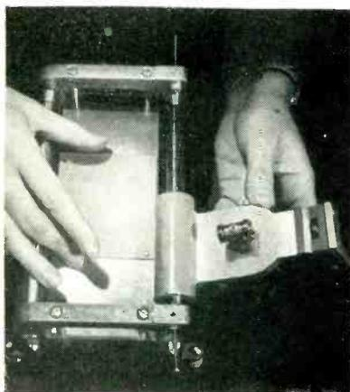
Lucite dial window panels are positioned in the tool by studs that mate with panel holes. Windows of five different shapes and thicknesses are accommodated by moving the studs to different positions in the tool
