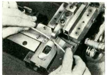
Method of using banding machine for splicing two wires together. Resulting joint is mechanically satisfactory for electronic circuitry
