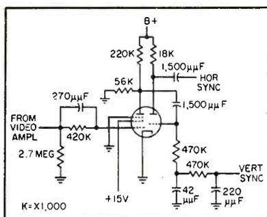
FIG. 6—Sync clipper circuit details
