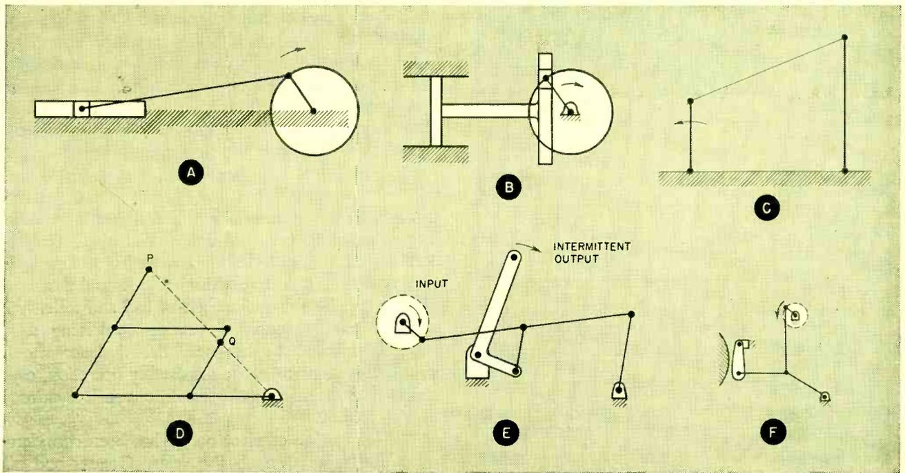
FIG. 7—Various bar linkages: slider-crank mechanism (A), Scotch yoke (B), four-bar linkage (C), pantograph (D), wrapping-paper mechanism (E) and stone-crusher mechanism (F)
