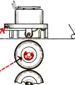
■ Miniature Truarc E-Rings on .040 diameter shaft and on continuously running capstans eliminate projecting bolts and screws. Rings permit rapid assembly and disassembly, fast replacement of worn rubber capstans.
