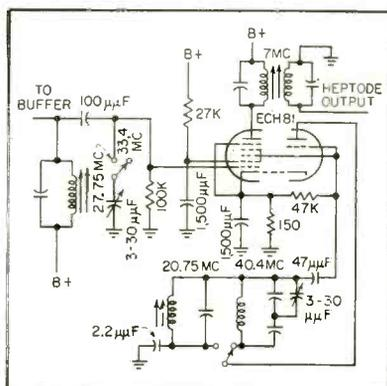
FIG. 2—Converter stage uses triode-heptode ECH 81
