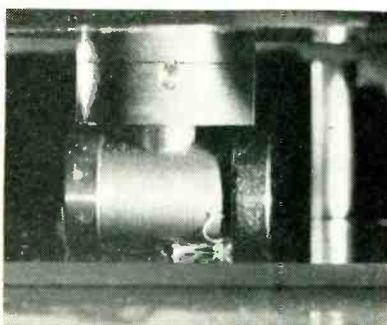
Operator drops needle on Lucite and moves needle-supporting slide the length of the panel to cut line. Needle here projects downward from center of spool-shaped holder. Ends or flanges of holder roll freely on plastic
