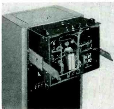
racks. They feature automatic out position locks (especially useful for sloping cabinets) and instant push-button return or chassis removal from cabinet for bench servicing or unit replacement. The slides support 175 lb in the full extended position and allow the chassis to be tilted back for servicing bottom components. They are permanently dry lubricated and meet JAN slide specifications. All attaching hardware, installation templates and instructions are included with each pair of slides.
