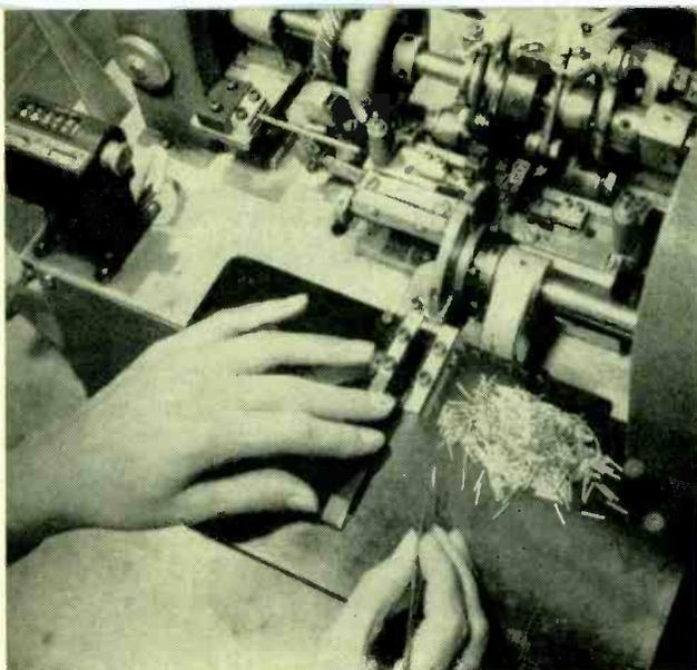
FIG. 8—Miniature welding machine used in making miniature tubes. Wire tabs 0.006 × 0.002 in. are welded to 0.25-in. diameter cathodes
