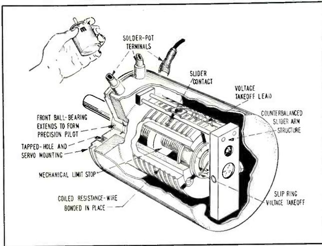
FIG. 4—Multiturn potentiometer construction as used by TIC provides high resolution along with low noise and long life
