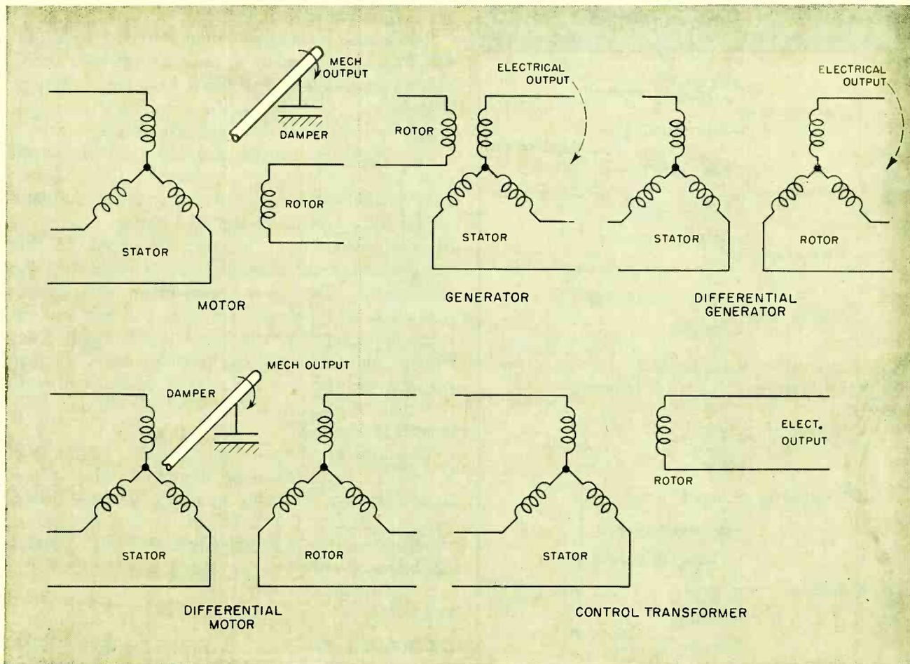
FIG. 7—Five common synchro types used in instrument applications
