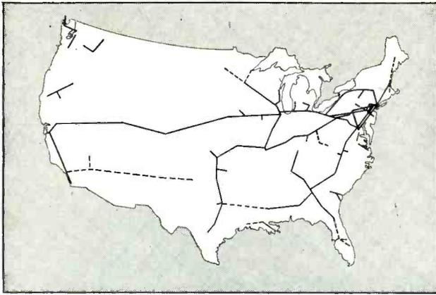
FIG. 2—Map shows extent of common carrier (public telephone & telegraph) microwave service in U. S.
