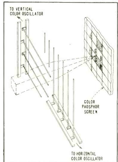
FIG. 8—Lens-grid screen for color tubes directs beam to desired area
