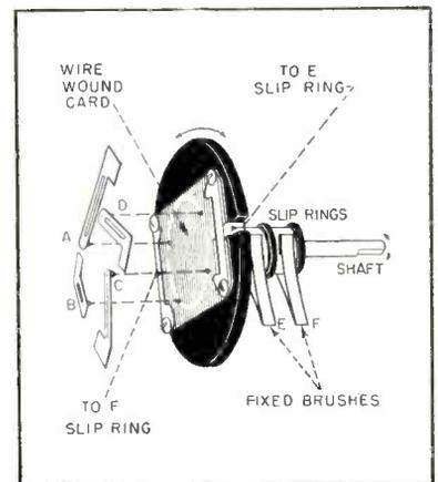
FIG. 3—Sine-cosine potentiometer made by Rawson Electrical Instrument Co. uses linear resistance card
