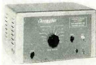
in to permit checks on convergence and linearity of color receivers. Output at video frequency is variable to 1.4 v peak-to-peak positive and negative, into a 75-ohm load. It includes a crystal controlled color subcarrier and built-in horizontal sync generator. Price is \$395.
