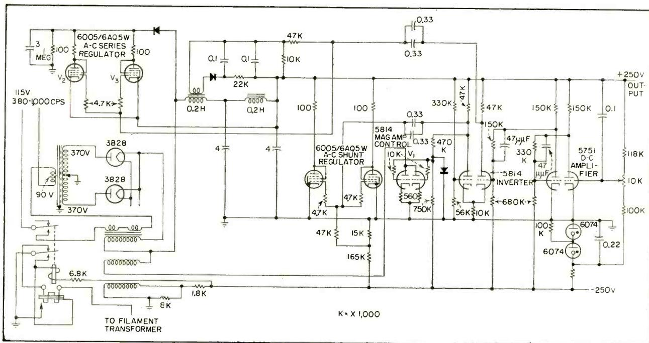
FIG. 3—Power supply with magnetic amplifier and clamper regulation has 250-v, 800-ma output at 55-percent efficiency
