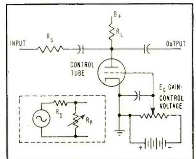
FIG. 1—Control tube in electronic attenuator acts as variable shunt to ground
