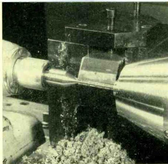
FIG. 1—Ten special grooves are machined in tuning-pin support, using Stellite skiving tool and 10-in. power-feed lathe
