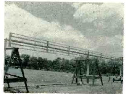
FIG. 2—Experimental transmitting antenna undergoing tests found later use in uhf booster installation for channel 25
