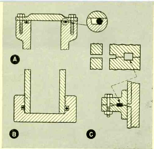
FIG. 7—Three methods utilizing O-rings to seal cabinets of water-proof or pressurized equipment
