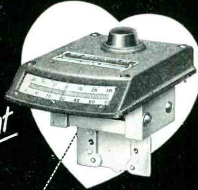
FOR MEASURING LIGHT reflectance and color, the Photovolt Corporation of New York uses a Model 600 G-M Galvanometer for its popular Reflection Meter (left). Whatever your own particular instrument field, you can achieve this same self-contained portability, ruggedness and high sensitivity with G-M Galvanometers. Complete catalog on request.
