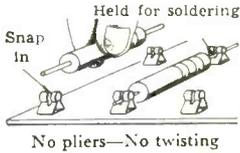
Used in printed circuitry Terminals 652T and 654T form solder eyelet.
