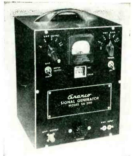
gain generator features coaxial tuning elements, continuous and precision tuning over the entire uhf band, calibration in both frequency and channel designations, and balanced detector meter circuit and gain control. Frequency range is 440 to 910 mc and to an accuracy of  $\pm 2$  percent, indicated by a single direct-reading scale. The instrument measures gain, tracking, calibration, accuracy and range of uhf tuners, converters, antennas, strips, boosters and receivers.
