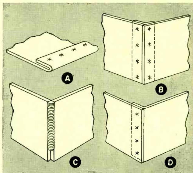
FIG. 8—Dutch bend (A) strengthens edge of light-gage metal. Other drawings illustrate various corner configurations
