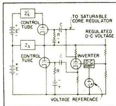
FIG. 2—Clamper circuit with d-c supply
