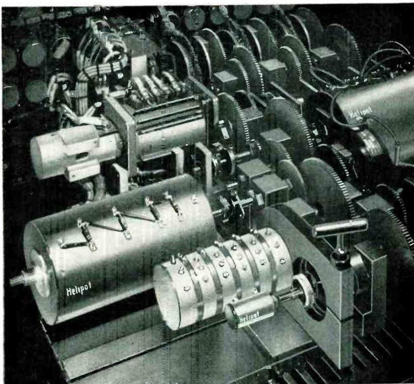
Setup used at Helipot for recording linearity of single unit, ganged unit and large tapped unit under test at left, by automatic comparison with master precision potentiometer at right center. At top can be seen some of the trim potentiometers that have been pre-set to insert voltage in series with master pot at 360 points to give tester accuracy within 0.003 percent. Gear train gives correct drive for models having from 1 to 40 turns, in phase with 40-turn master
