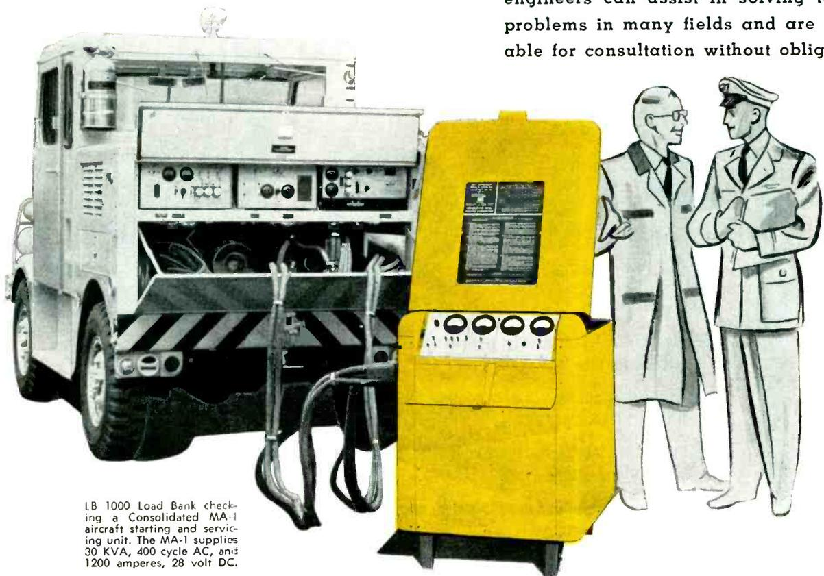
LB 1000 Load Bank checking a Consolidated MA-1 aircraft starting and servicing unit. The MA-1 supplies 30 KVA, 400 cycle AC, and 1200 amperes, 28 volt DC.
