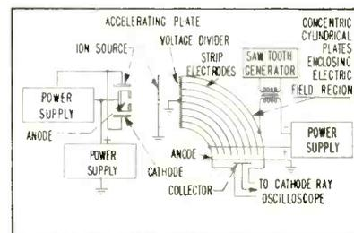
FIG. 14—Electronic portion of focused mass spectrometer
