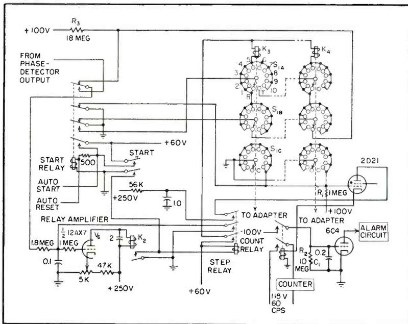
FIG. 5—Basic circuit used to achieve automatic control. Details such as range-changing circuitry, safety provisions and manual provisions are not included
