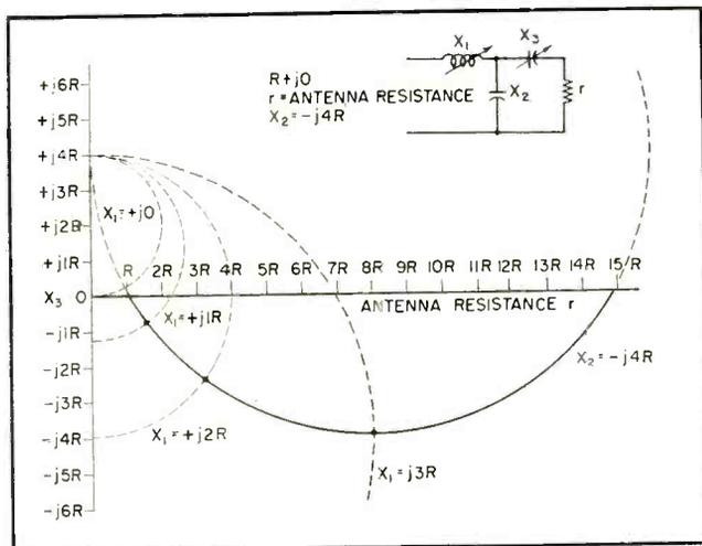
FIG. 1—T-section matching properties when  $X_1$  and  $X_3$  are variables in antenna-matching section
