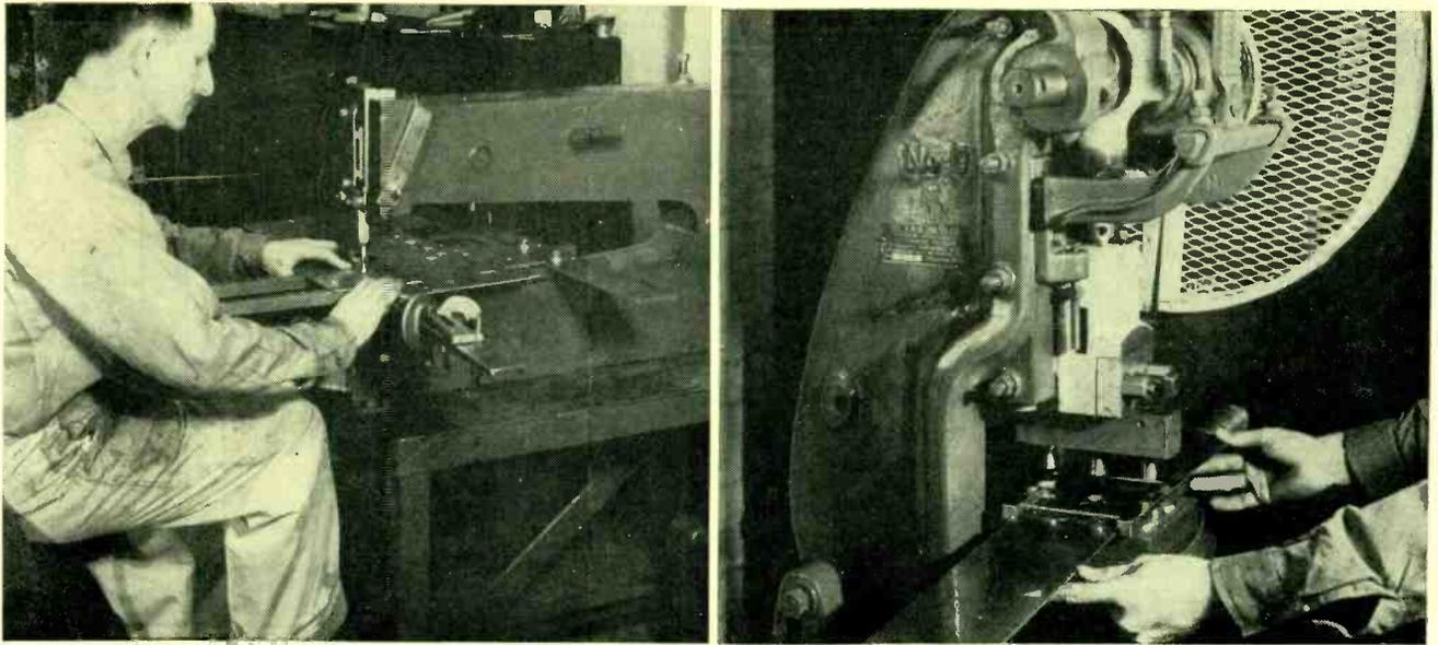
FIG. 6—Kick presses and small power presses are useful for small production runs
