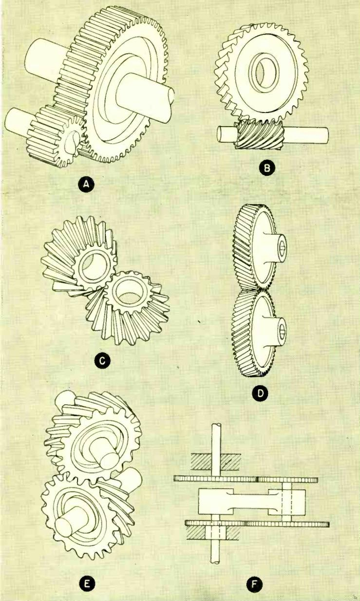
FIG. 3—Types of gears used in electronic equipment: spur (A), worm (B), bevel (C), helical (D) and spiral gears (E). Also shown is planetary or epicyclic gear train
