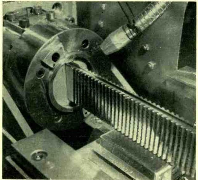
FIG. 4—Rectangular opening in magnetron shell is broached in two operations. Grooves running the length of the broach fit into keys and guides on fixtures to insure concentricity
