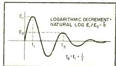
FIG. 1—Waveform shows transient method of determining *Q*
