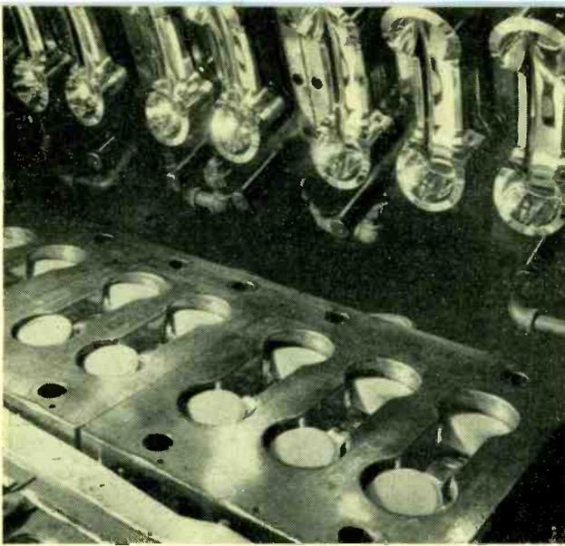
FIG. 5—Compression molding eight telephone handsets at a time. Preformed shapes of thermosetting plastic are fed directly to heated metal mold
