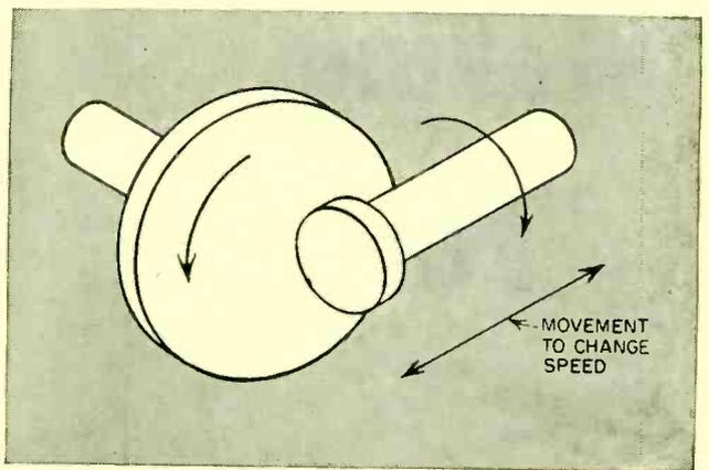
FIG. 2—Disk and wheel friction drive mechanism
