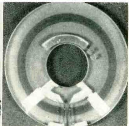
Miniature Fairchild potentiometer with metallic-film element provides essentially infinite resolution, is stable to 225 C and can be produced in a wide range of resistances for applications requiring high accuracy
