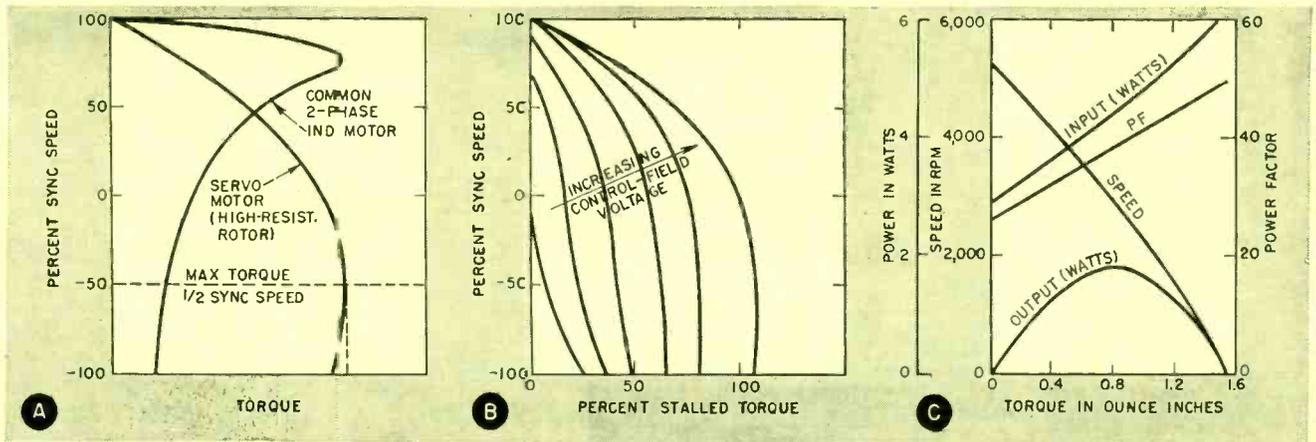
FIG. 1—Servo motor characteristics. Speed-torque curves illustrate effects of rotor resistance (A) and control field voltage (B); (C) shows typical motor performance
