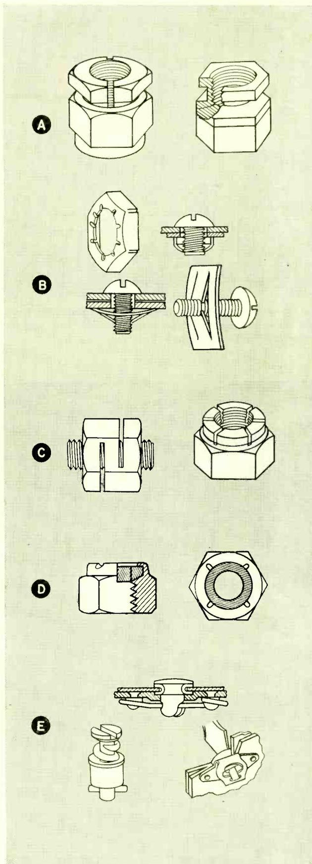
FIG. 10—Special fasteners are widely used in commercial equipment such as television sets and home radios. The several varieties illustrated include: wedge type (A), spring seating fasteners (B), spring stopnuts (C), interference stopnut (D) and quick release fasteners (E)
