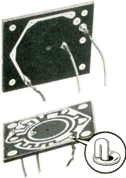
Made for each other! Hubbell Interlock's sub-miniature connectors make wiring of printed circuits fast and safe. Note how Interlock Type "C" Connectors pass through set-in eyelets from back and lock automatically on opposite side. Eyelets manufactured by United Shoe Machinery Corp. Eyelet setting machines are available.
