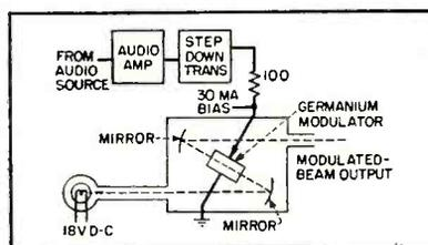
FIG. 3—Demonstration infrared transmitter uses parabolic mirrors to focus light beam of modulator crystal
