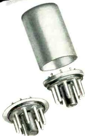
These new plug-in hermetic seals mate with a standard octal socket. They have the desirable feature of all Triad terminals: heavy moulded construction of mineral-filled MIL-P-14 approved phenolic, high dielectric strength, high conductivity gold alloy plated pins, hot-tinned solder rings, and resistance to "tracking" and fungus growth. They meet MIL-T-27 requirements.
