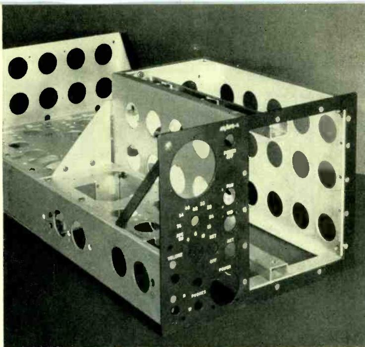
Fig. 1—Military equipment chassis, illustrating use of removable top and side skirts and plug-in subchassis
