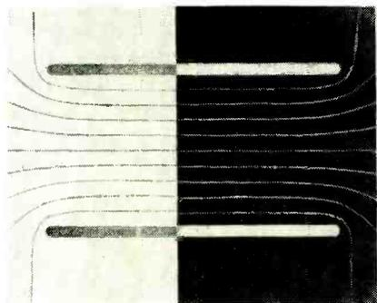
FIG. 2—Typical field plot made with manual method (left) and with automatic field plotter (right)
