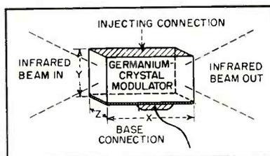
FIG. 1—Modulator uses transistor-type connections. Signal across modulator varies charge density in crystal
