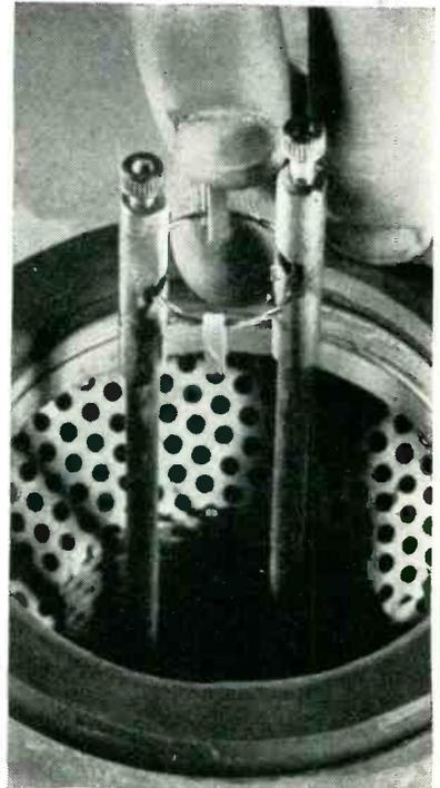
Loading bent aluminum strips on tungsten filament
