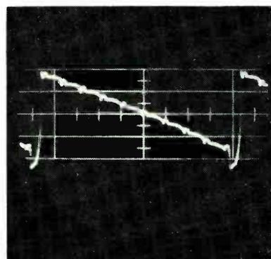
Voltage waveform of right deflection plate of EIT tube. Pulses are ten microseconds apart
