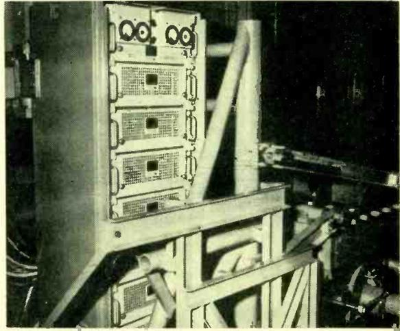
**DESIGNING THE CABINET** entails planning housings for both stationary and mobile equipment. Cabinet shown is undergoing test on a vibration table
