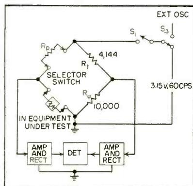
FIG. 2—Impedance-test circuit
