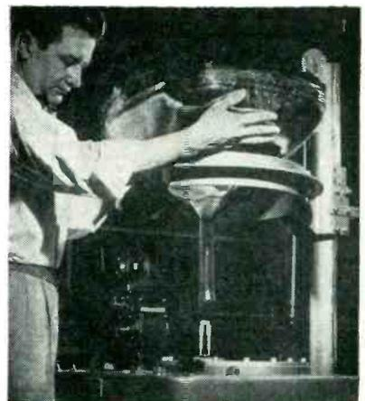
Placing picture tube in counterweighted yoke of automatic lowering device that lowers tube accurately into position, neck first
