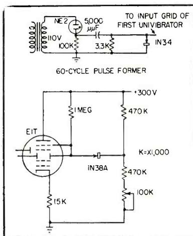
FIG. 5—Basic circuit for interval timer. System shown is for scale of six
