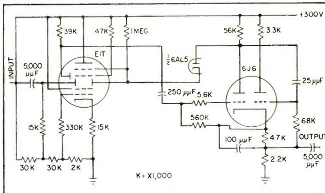
FIG. 4—Circuit for driving the tube to 100,000 counts per second incorporates certain modifications
