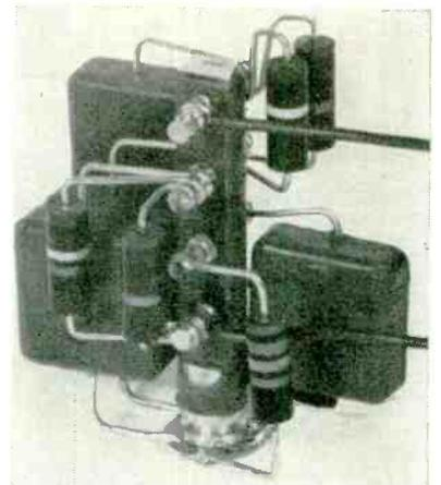
Single four-terminal totem pole here provides mounting for complete parallel-T network. This subassembly is electrically tested before final assembly. Identifying numeral is on adhesive-tape tab on top of post
