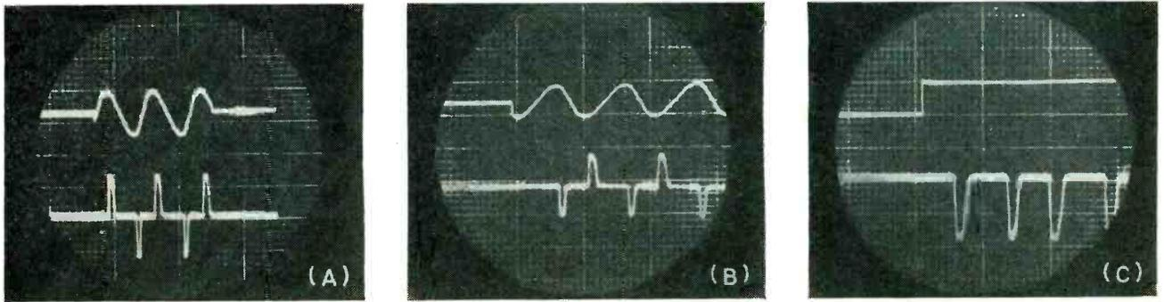
FIG. 5—Input and output waveforms for 2-v 60-cps control signal with minimum delay (A) and maximum delay (B). Output (C) is for d-c step-voltage control
