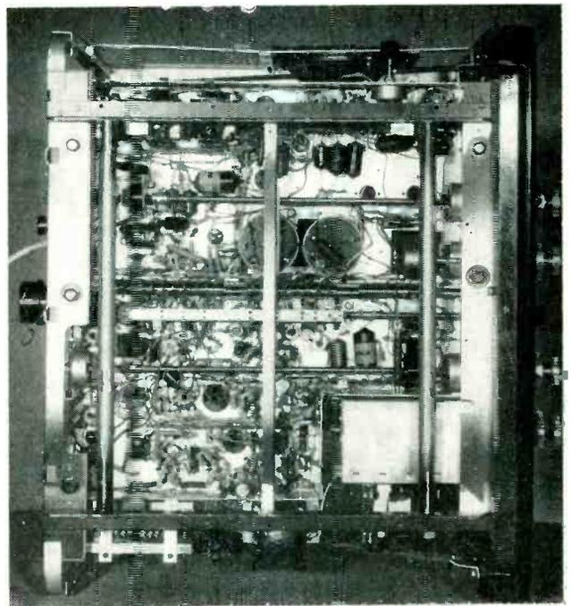
Detail of chassis construction in four-system receiver
