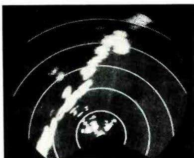
Limited range of light intensities in cathode-ray tube screen makes storm display appear uniform throughout with ordinary circuits
