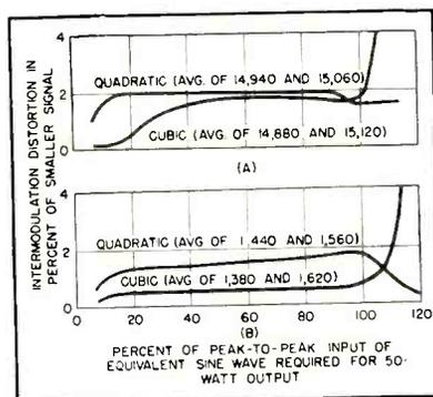
FIG. 12 — Intermodulation-distortion characteristics with 4:1 ratio of 60 and 15,000 cps signals (A); 60 and 1,500 cps signals (B)
