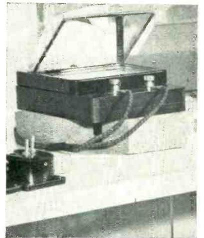
Method of mounting standard meter with mirror on shelf above production bench
