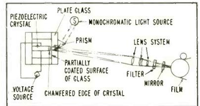
FIG. 12—End view of piezoelectric voltmeter
