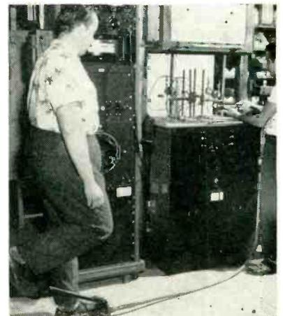
Method of using air-operated vise to seal off the metal tubulation of a magnetron after pumping. Assistant is operating control valve on floor at left
