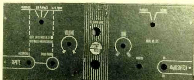
FIG. 14—Screen printing on hammer-finish background.
