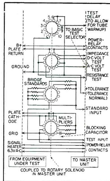
FIG. 6—Typical wiring form to test a resistance-coupled amplifier
