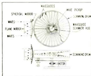
FIG. 3—Basis of microwave scanning system
