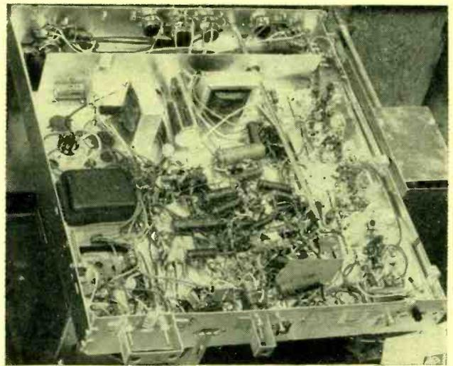
FIG. 4—Use of point-to-point wiring in a tv receiver. Photo, left, shows set with parts assembled to chassis and basic wiring installed. Photo, right, shows a set completely assembled and wired
