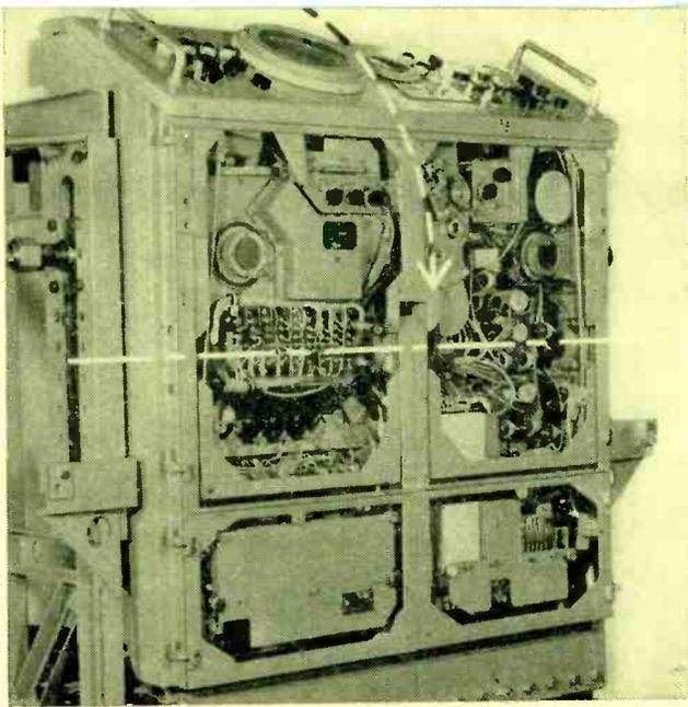
FIG. 4—Hinged chassis pivots about axis indicated. Arrow illustrates how chassis is swung forward and down
