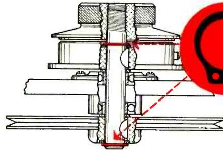
■ Truarc Standard Rings (Series 5100) hold the reel shaft assembly firmly in place and permit the use of quick-lock hubs so that the reel tapes can be changed in seconds as they are finished.
