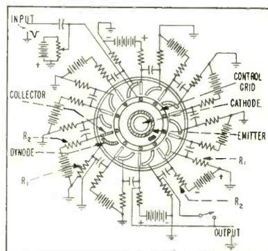
FIG. 1—Internal structure of the impulse counter tube
