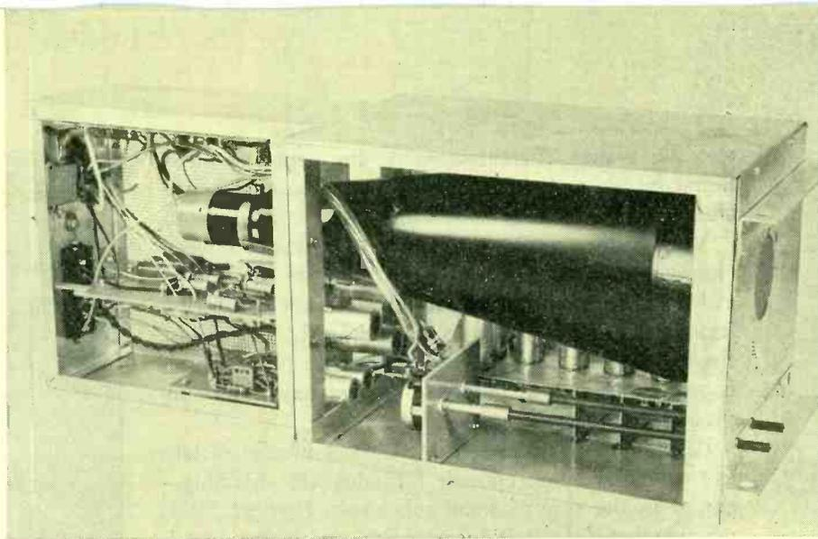
Cathode-ray storage tube for large digital computer requires magnetic shielding to exclude stray fields. Shield is fabricated from magnetic alloy by sheet-metal development
