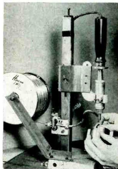
Overhead mounting of soldering iron. Action of foot pedal lowers iron and pulls down lever arm that rotates gears between which solder runs, so that wheels push solder through bent copper tubing to the work
