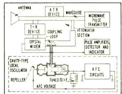
FIG. 7—Microwave superheterodyne eliminates separate afc crystal
