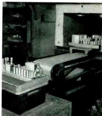
Vibrator at input of heat-cycling oven
