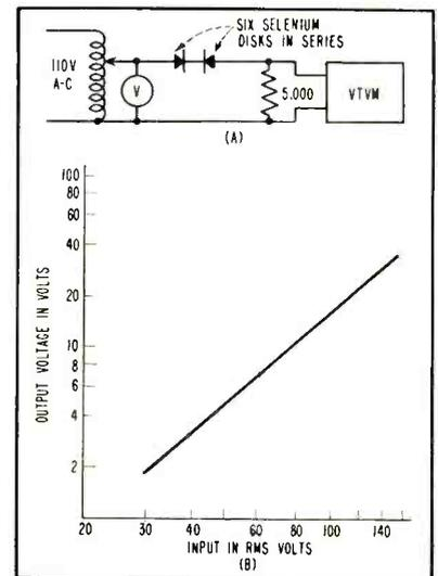
FIG. 2—Test circuit for single-stage nonlinear impedance (A). Curve (B) shows impedance variation with change of line voltage
