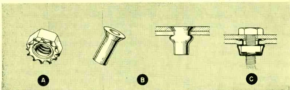
FIG. 1—Keeps (A) combining nut and lockwasher, blind rivets, shown before and after upsetting (B), and nut retainer (C) are useful in inaccessible locations
