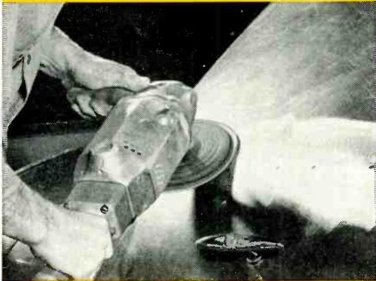
Flexibility gives long life to abrasive discs backed with Taylor Vulcanized Fibre, which retains strength under repeated bendings.
