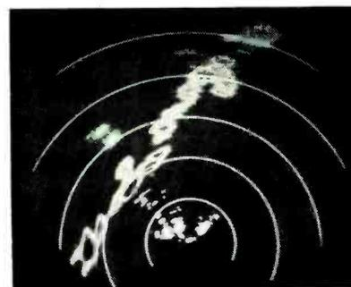
Intense portions of storm where rainfall is heaviest are seen as black holes using new isoecho circuits in Bendix RDR-1 radar
