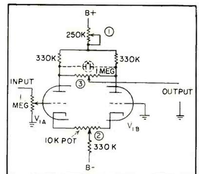
FIG. 4—Detail of amplifier  $V_1$  of Fig. 3
