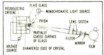
FIG. 12—End view of piezoelectric voltmeter
