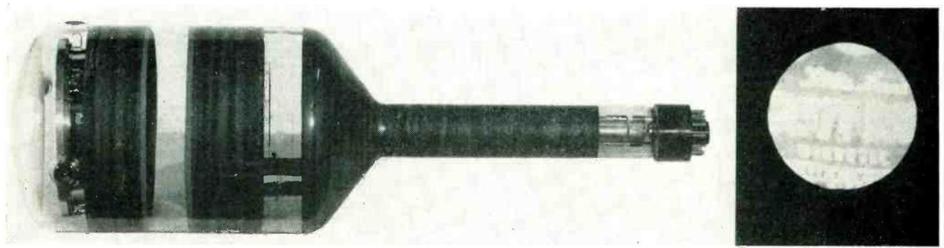
Hergenrother recording storage tube QK 245F (left) has both direct view and electrical output. Television signal readout (right) after an hour's storage in the QK 245F which has relatively low light output
