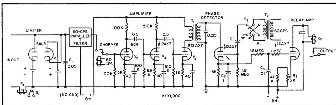
FIG. 4—Detector used in bridge circuits of Fig. 1, 2 and 3. Note that both input terminals are floating with respect to ground
