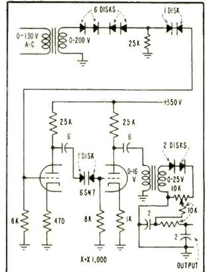
FIG. 3—Circuit of three-stage nonlinear compensation circuit
