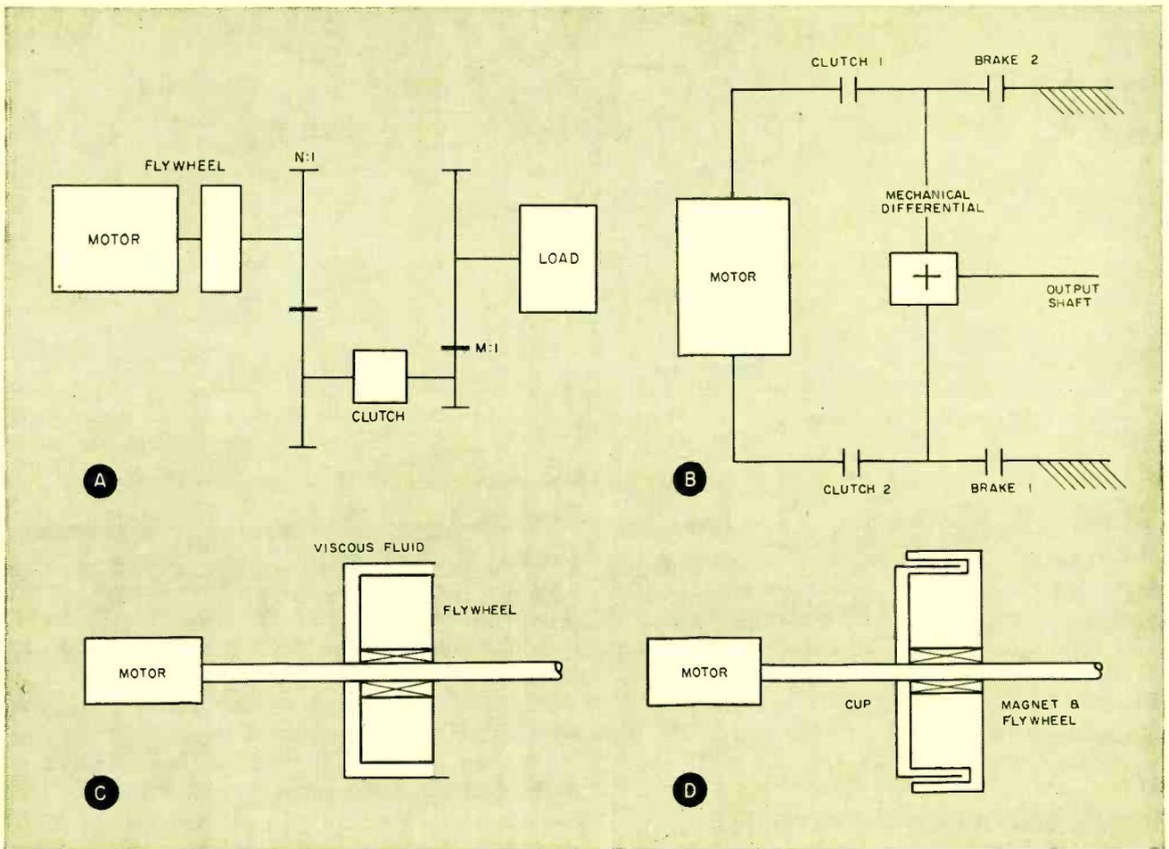
FIG. 6—Associated motor devices. Clutch and brake applications, top, and servo damping devices, below
