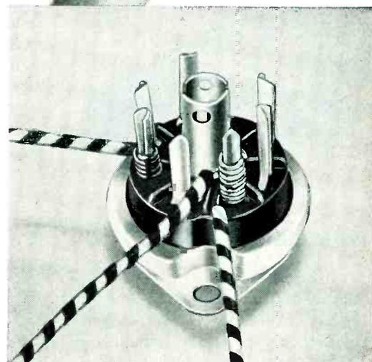
**1.** New Sylvania 7-pin Miniature Printed-circuit Sockets. Contacts and center shield are shaped so that sockets can be stacked one upon another for automatic feeding and assembly. Small slots are used on the circuit board to receive the contacts, resulting in stronger chassis construction. Only one socket assembly need be stocked since terminals can be interconnected by printing the circuit on the chassis board rather than using a metallic connector on the socket itself.
