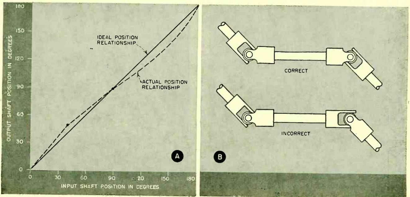
FIG. 1—Universal joint joining two shafts. Typical curve for input-output shaft position (A) and method of positioning shafts (B)
