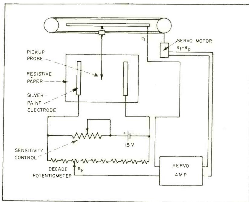
FIG. 1—Simplified diagram of automatic electrostatic field plotter setup
