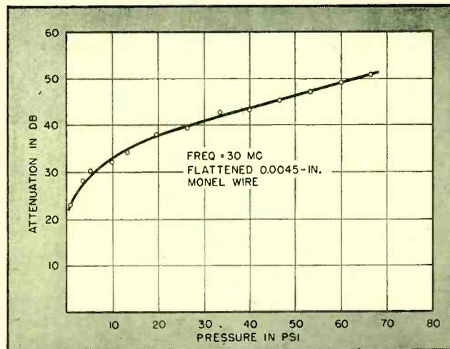
FIG. 5—Shielding properties of metal gaskets are improved by compression
