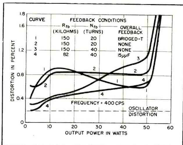
FIG. 8—Feedback-distortion characteristics
