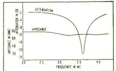
FIG. 2—Characteristics of the input filter
