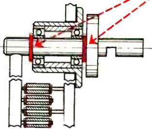
■ Truarc E-Rings snap quickly into place, act as shoulders for the ball bearings with a minimum of friction. Additional Truarc Rings are used as spacers on shafts, can be located accurately to extremely close tolerances.
