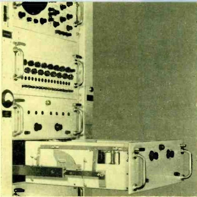
FIG. 2—Drawer type of construction in which broad side of chassis is horizontal
