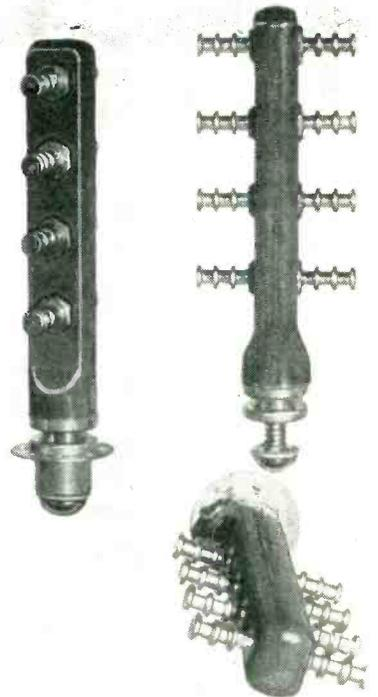
Totem poles may be assembled with or without ground terminal and spacer pillar. Terminals are of solid bronze, hot-solder-coated and staked into the melamine post
