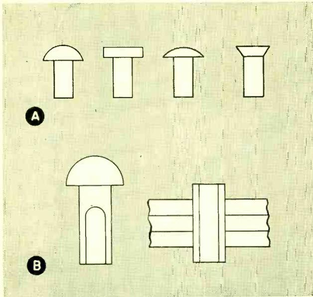
FIG. 11—Rivet types; from left to right (A) shows round, flat, brazier and countersunk heads. Tubular rivets (B) include solid head with hollow shank and tubular type
