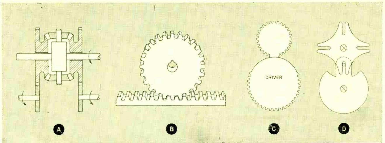
FIG. 4—Special gearing systems: differential gears (A), rack and pinion (B), intermittent gears (C) and Geneva mechanism (D)
