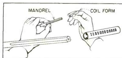
FIG. 4—Recommended winding arbor
