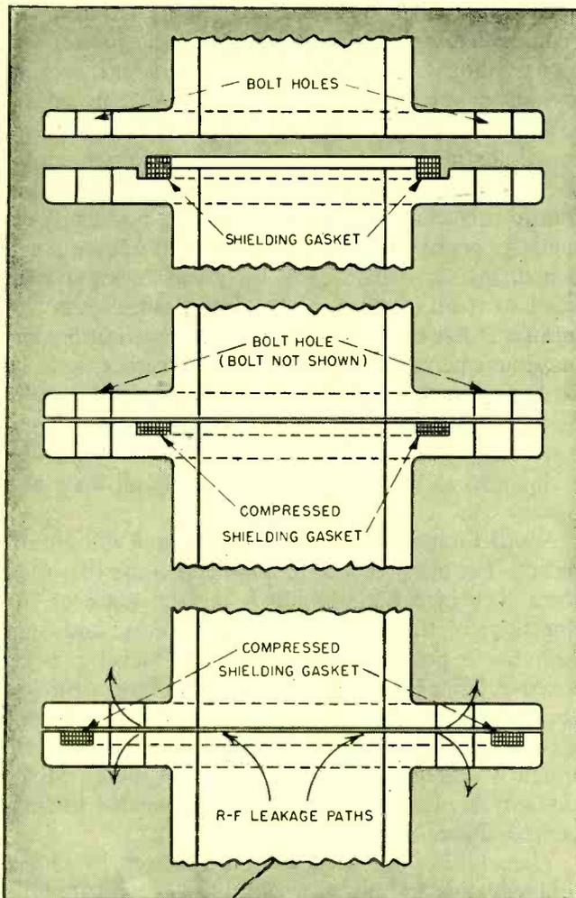
FIG. 3—Sealing a flange joint against radiation. For best results metal gaskets should be located inboard of bolt holes
