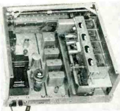
New amateur receiver made by Hammarlund uses printed circuits in r-f section and sectionalized mechanical construction
