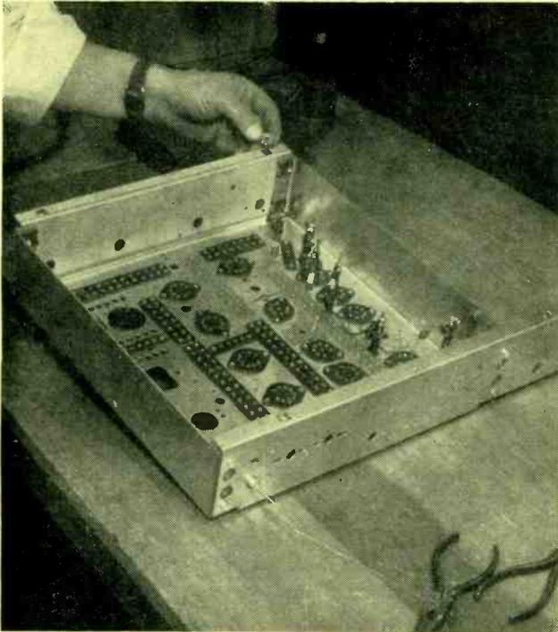
FIG. 6—Eyeleted component boards and wafer-type tube sockets installed on chassis
