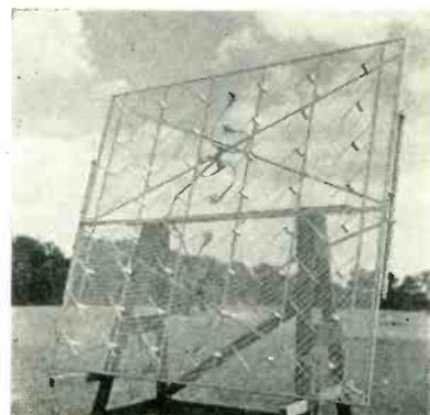
FIG. 1—High-gain receiving antenna picks up main-station signal for rebroadcast by booster on same frequency
