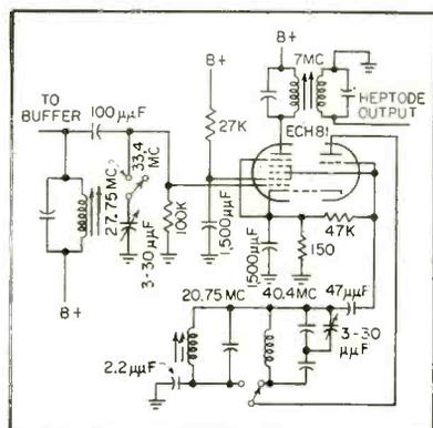
FIG. 2—Converter stage uses triode-heptode ECH 81
