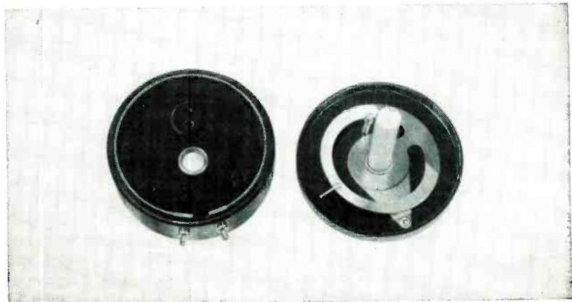
Typical of new wire-wound potentiometers designed to hold capacitances to minimum is this General Radio unit using phenolic winding form, cup and cover along with glass polyester shaft, for a-c linear-resistance applications. Tolerance is 2 percent for 1.25-inch diameter units and 0.2 percent for 4.25-inch units
