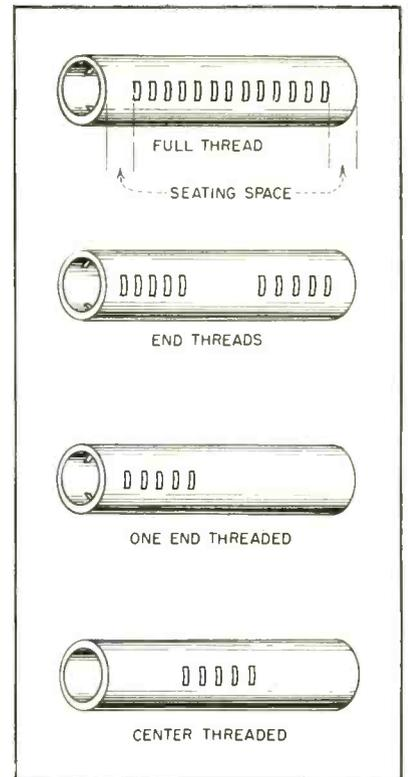
FIG. 5—Methods of positioning embossed threads on coil forms
