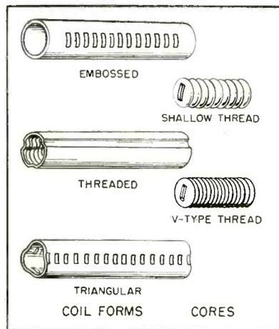
FIG. 1—Types of internally threaded coil forms and mating threaded iron cores
