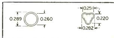
FIG. 2—Typical triangular or cloverleaf type coil form
