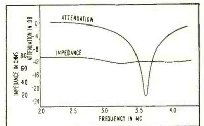
FIG. 2—Characteristics of the input filter
