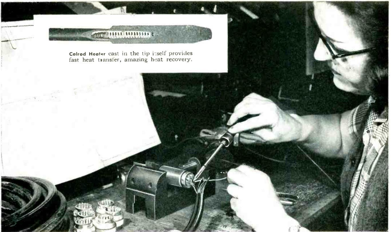
Calrod Heater cast in the tip itself provides fast heat transfer, amazing heat recovery.
