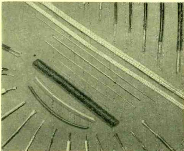
FIG. 1—Wire used in electronic equipment manufacturing. At the top are five examples of solid insulated wire and two of shielded cable. In the center are shown two types of flexible copper braid, five of bare hookup wire and three of sleeving or spaghetti. At the bottom are shown two samples of twin lead and 11 of stranded insulated wire
