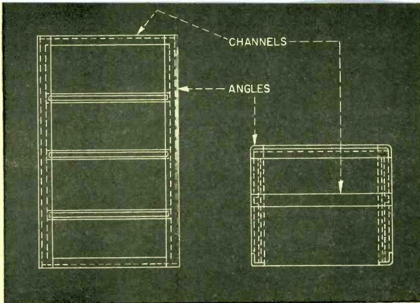
FIG. 1—Plan and front elevation of a Christmas-tree frame. This provides a rigid structure of channels to which panels can be fastened. Chassis are mounted in horizontal drawers
