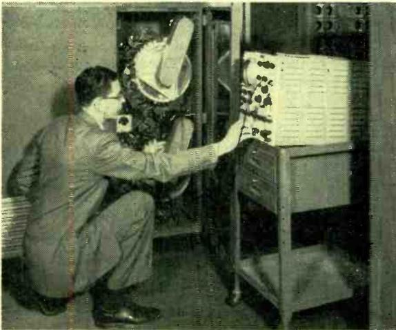
**POWER DEVICES** employed are subfractional a-c and d-c motors, clutches, brakes, damps and complete synchro systems. Engineer is checking a 2,929-rpm magnetic drum
