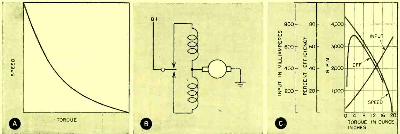
FIG. 5—Direct-current machines. Speed-torque curve of series motor (A), method for reversing rotation (B), and typical d-c motor performance (C)
