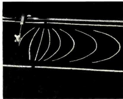
FIG. 4—Field plotter in operation; silver-paint electrodes can be seen at the top and bottom of the field lines
