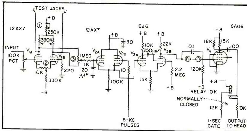
FIG. 3—Modulator accepts 1-volt peak signals and is triggered by 5-kc pulses
