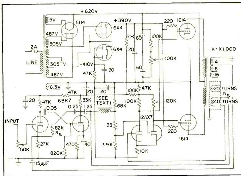
FIG. 5—Complete fifty-watt amplifier with preamplifier delivers full output with 0.8-volt rms input signal. Voltages indicated are measured with zero-signal input
