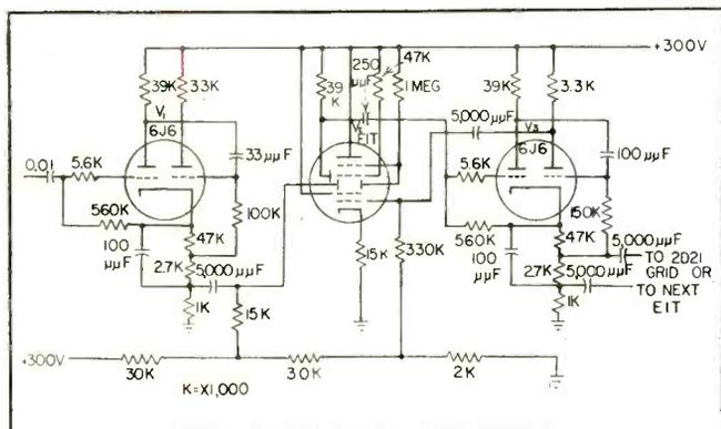
FIG. 3—Philips 30,000 counts per second circuit. The 6J6 resets the tube on the tenth pulse
