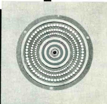
Increased production of Mycalex 410 Telemetry Commutators now brings new savings to the user. Universally accepted as the finest commutator plate in the field, this precision-built unit injection-molded of Mycalex 410 glass-bonded mica insulation assures permanent dimensional stability — provides a tenacious bond to the metal inserts.
