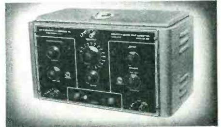
A very wide range square wave generator producing ideal wave forms without slope or overshoot. Rise time of 0.02 microseconds permits ready examination of amplitude, phase, and transient response limitations of wide band video amplifiers. Variable symmetry permits generation of waveforms with high second harmonic content.
