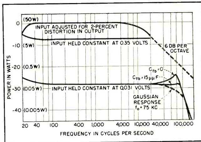
FIG. 11—Overall frequency response of amplifier
