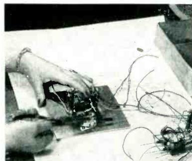
Jig facilitates production of two-post subassembly, using sample and diagram as guides. Note accessibility of terminals for inspection and wiring
