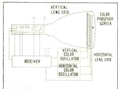
FIG. 9—Method of energizing color-tube grid with vertical and horizontal oscillators controlled by receiver
