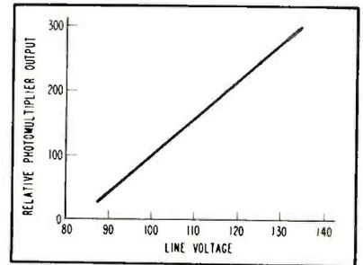
FIG. 1—Variation of phototube output with line voltage
