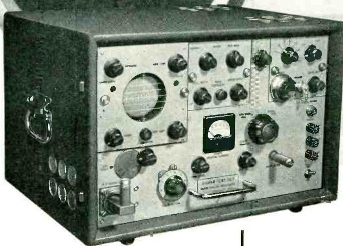
**Combined in this equipment** are means to measure power...observe transmitter spectra distribution...measure frequency and supply artificial signals. You can analyze bandwidth characteristics. A self-contained square wave generator aids in making standing wave measurements. *One* portable unit *does all*—on the bench or in the field—efficiently and at much lower first cost than with separate instruments.
