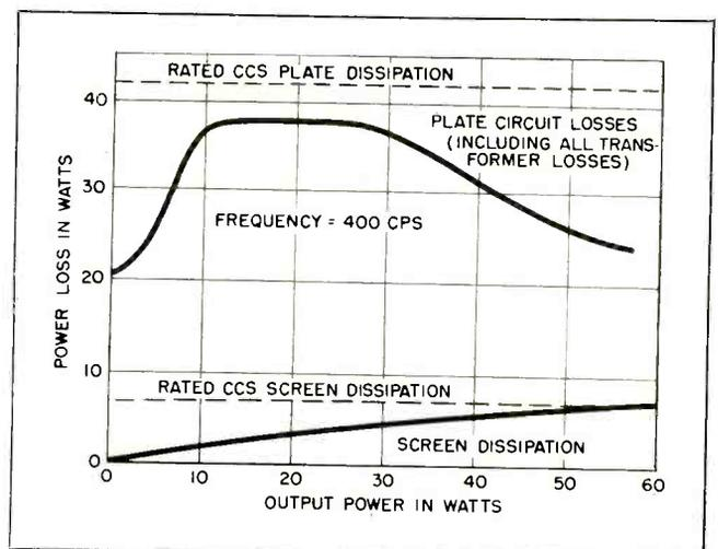
FIG. 9—Plate-circuit power loss characteristics
