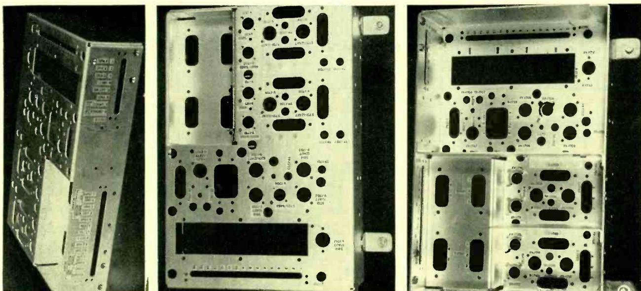
FIG. 13—Three chassis with nomenclature imprinted by silk-screen process
