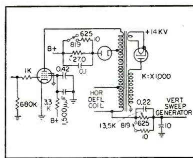
FIG. 8—Horizontal output stage
