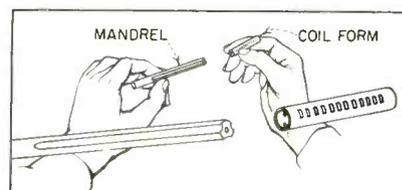
FIG. 4—Recommended winding arbor
