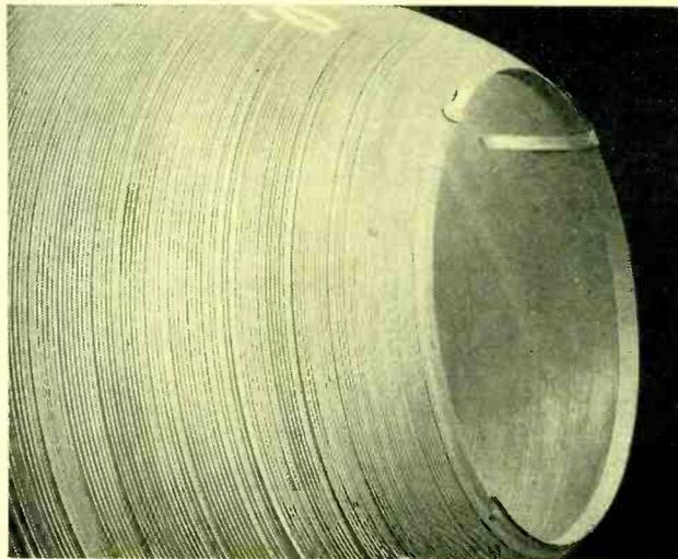
FIG. 1—Wire-mesh gasket around top of cabinet is compressed when lid is closed and forms radiation-proof electrostatic shield
