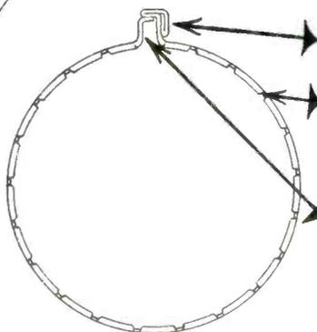
**THREADED TRIPLE-FOLD RING HEAD**, .075" thick eliminates nuts . . . avoids loosening.
