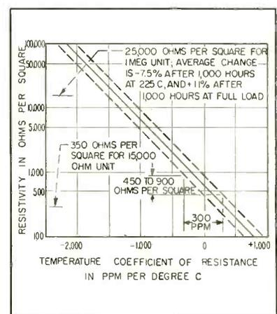
FIG. 1—Typical relation between temperature coefficient of resistance and resistivity of Fairchild film unit
