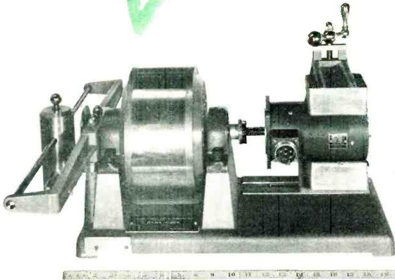
*Dyna-Chek* provides tested and proven accuracy in measuring the output of fractional and integral horsepower motors —
