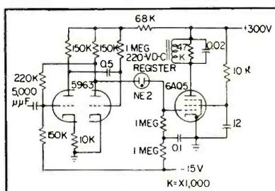
FIG. 6—Register driving circuit uses type 5963 as a long time constant univibrator triggered by the final counter
