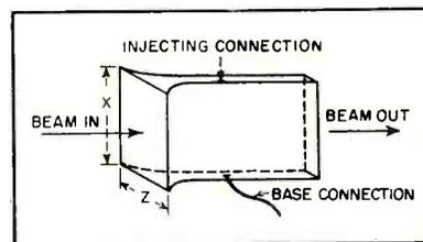
FIG. 2—Modified design of modulator providing larger acceptance area *yz* for improved performance
