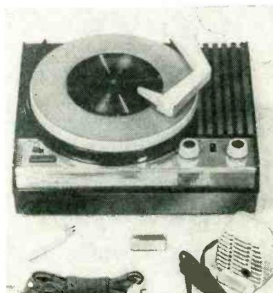
Magnetic disc recorder can be converted to standard 45-rpm phonograph with plug-in cartridge and spindle adapter button
