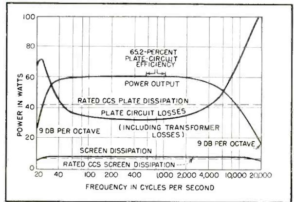
FIG. 4—Power relations for fifty-watt basic amplifier with transformer-coupled input
