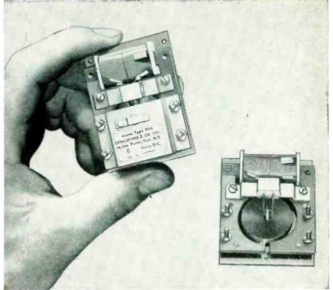
**Miniature Electric Motor.** Tiny, powerful Carboloy permanent magnet replaces wound electromagnet as rotor. The magnet's self-contained power supply reduces battery drain, requires less power.
