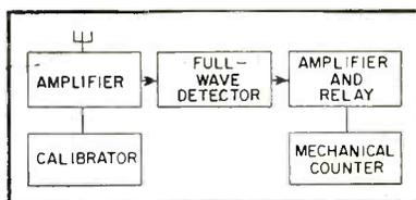
FIG. 1—Block representation of low-frequency lightning receiver
