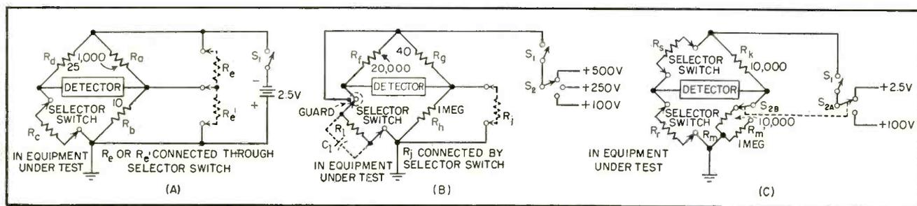
FIG. 1—Simplified schematic diagrams of continuity-test circuit (A), leakage-test circuit (B) and resistance-test circuit (C)
