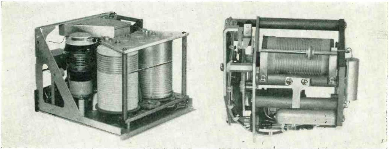
Rear view of matching unit shows variable vacuum capacitor (left) and variable inductor (right) on which ribbon is wound. Autotransformer assembly used to match antenna coupling unit to 52-ohm output comprises rotating inductor and contact wheel.
