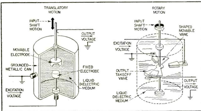
FIG. 2—Liquid dielectric potentiometer provides infinite resolution. Capacitance to output electrode varies in same ratio as does resistance, hence time constant is substantially unchanged by rotation
