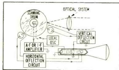
FIG. 4—Method of reproducing radio-wave images
