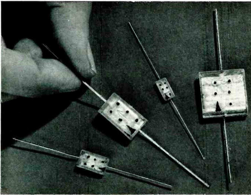
Miniaturation means fewer physical sizes to cover a large capacitance range. Non wire lead capacitors can be made ever smaller.
