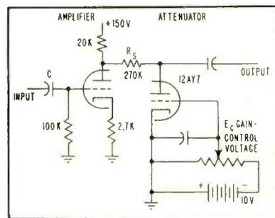
FIG. 2—Attenuator circuit for low-level signals
