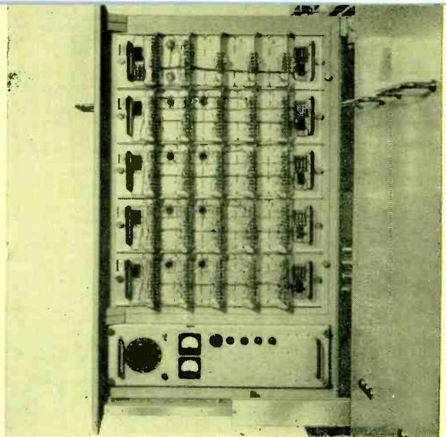
FIG. 3—Drawer type of construction in which broad side of chassis is vertical
