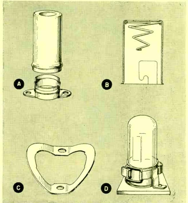
FIG. 7—Bayonet (A) and bead (B) type tube shields; also ring (C) and collar (D) type tube clamps
