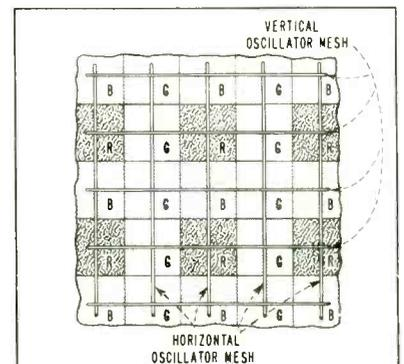
FIG. 11—Position of the color areas that are activated by the beam
