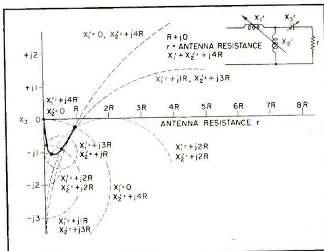
FIG. 2—T-section matching properties when  $X_1'$ ,  $X_2'$  and  $X_3'$  are variables in antenna-matching section
