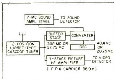
FIG. 1—Diagram shows buffer sound stage between tuner and converter. Small trimmer capacitor switches resonant frequency of tuned circuits in buffer intermediate frequency sound stage from 33.4 to 27.75 mc
