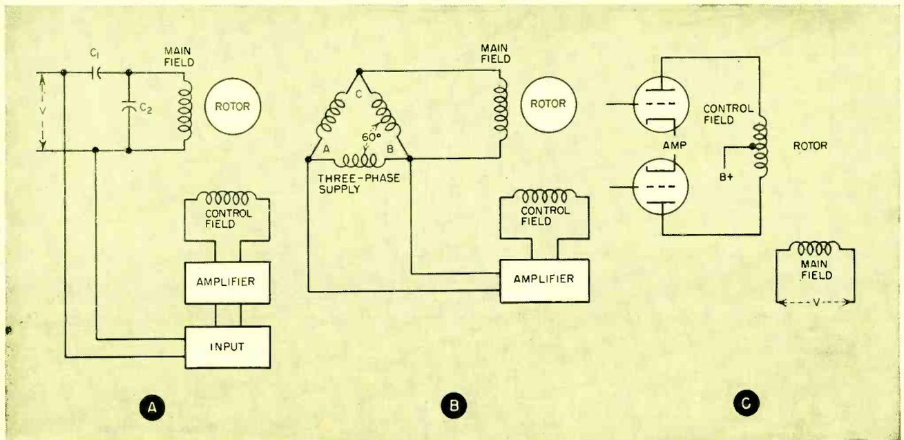
FIG. 2—Servo motor connections. Phase shift may be obtained with capacitors (A) or by using two phases of three-phase supply (B). Split-field motors are available for plate-to-plate operation (C)
