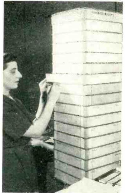
Master lamp-controlling chart on which are drawn the master curves for last 1,000 tubes produced. Each tube type has three cards in a horizontal row, for separate entry of noise, electrical and mechanical defects
