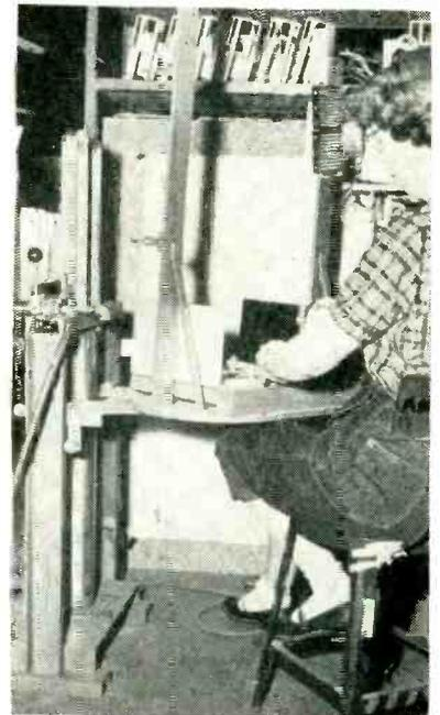
Using lift at knee level for initial stages of assembling parts on a panel.
