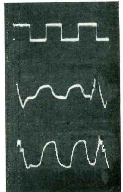
FIG. 2—Storage-tube input at top, output signal after 15 minutes storage, read out by a 1.20 microampere beam current, middle and 6 microampere beam current at bottom
