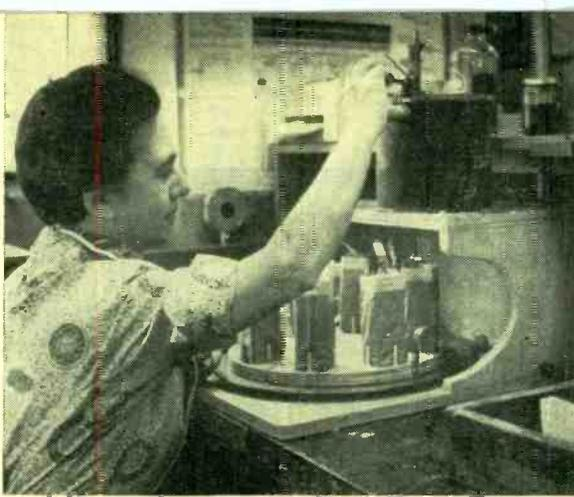
**SHIELDING AND POTTING** include both electric and magnetic shielding as well as use of casting and potting resins. These transformer cans are filled with molten beeswax
