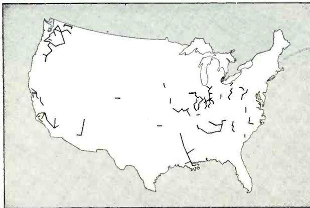
FIG. 4—Major power utilities are developing extensive microwave networks within their areas of operation
