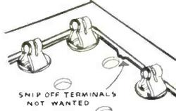
Jumper strip eliminates wiring—can be used to lay out prototype printed circuits.
