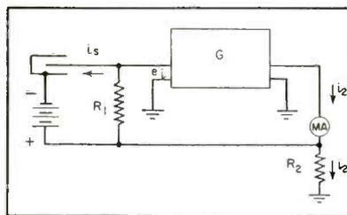
FIG. 3—Four-terminal network representation of amplifier in Fig. 2
