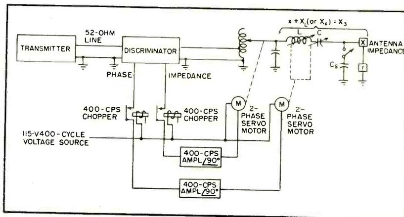
FIG. 4—Elements of complete motor-controlled automatic antenna-matching unit
