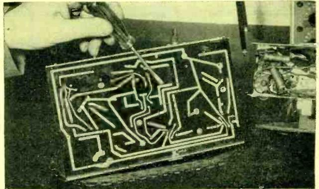
FIG. 9—Printed circuit techniques include use of conductors sprayed on dielectric plate, left, and stamped from metal foil and embedded in plastic, right
