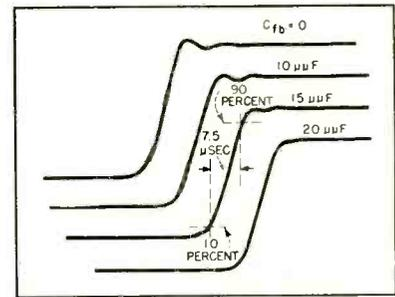
FIG. 6—Response of complete amplifier to a 10-watt 5-kc square-wave input. Increasing the value of the feedback capacitor tends to reduce the slight amount of ringing present
