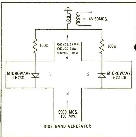
Showing klystron local oscillator and conventional AFC system replaced by silicon diode side-band generator.
