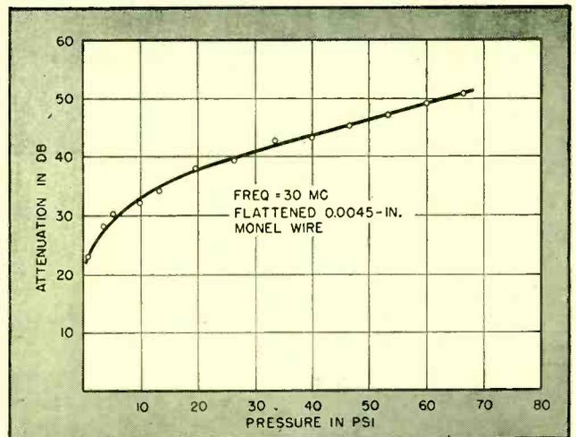
FIG. 5—Shielding properties of metal gaskets are improved by compression
