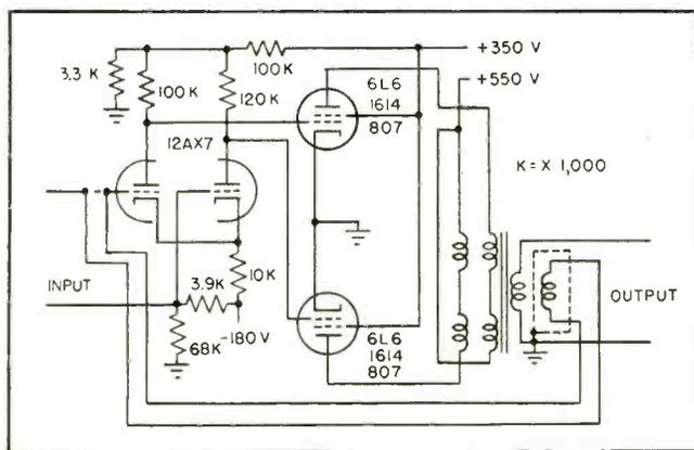
FIG. 1—Basic power amplifier has large amount of inverse feedback without trace of instability
