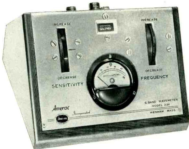
Precision manufactured—just like its sister model for the "S" Band—Amerac's new, Model #230, "C" Band Wavemeter is a co-axial line instrument covering the frequency range from 3500 MC to 6500 MC, by either the transmission or absorption method.
