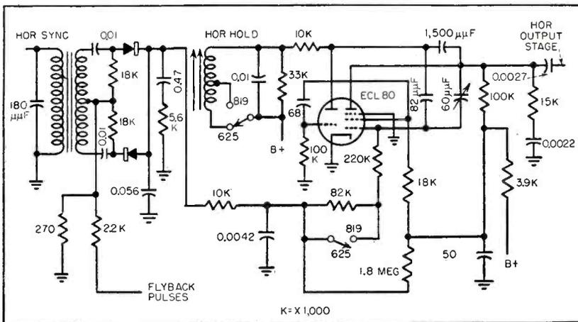
FIG. 7—Horizontal-sweep generator employs triode-pentode in multivibrator circuit
