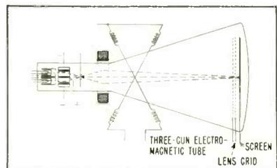
FIG. 10—Three-gun tube used to demonstrate how beam can be directed to a common point on screen area
