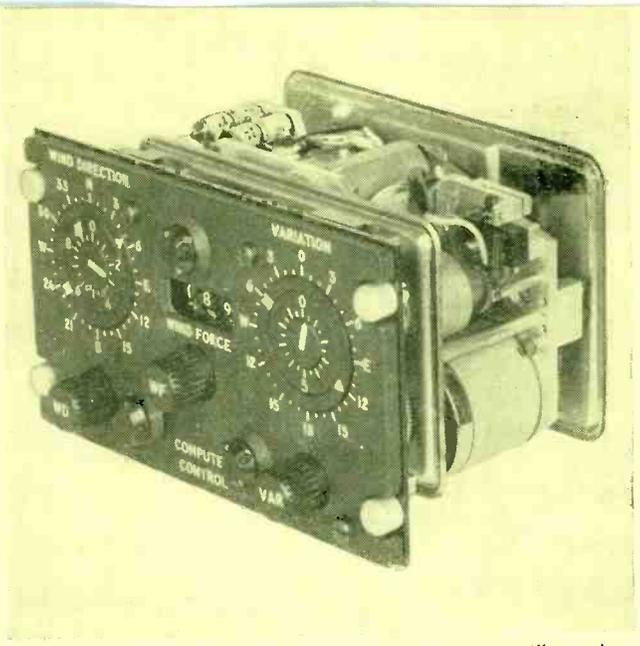
FIG. 5—Front panel of airborne navigational computer, illustrating arrangement of controls
