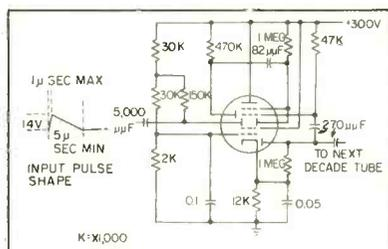
FIG. 2—One-tube decade counter circuit with passive elements
