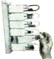
Complete circuits can be divided function by function mounted in planes.
