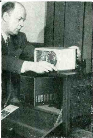
Pick-up unit behind receiver feeds tuning information to unit recorder in cabinet
