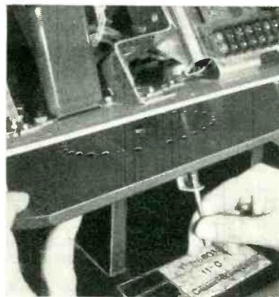
Chassis can be rotated when detent pin is pulled down as shown here
