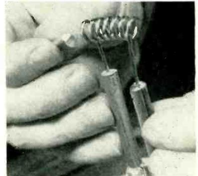
Aluminum slug placed in coiled filament is vaporized by heating filament, so that molecules of aluminum are deposited on screen
