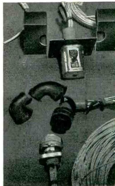
Examples of molds and potted connectors for aircraft wiring
