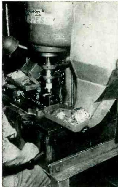
Sheet-metal hoppers alongside press feed brass shafts and supports, for riveting together when loaded into press manually. Note semicircle cut into bolster, with chute below leading to tote box for finished pieces. Spring clips welded to hopper at right can be used to hold work cards
