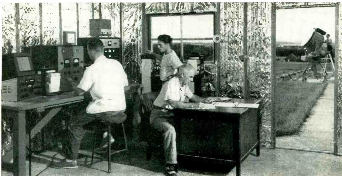
Experimental 0.87-cm sextant (visible through doorway) at Collins Radio's Feather Ridge Observatory. Receiving equipment is in shielded room where recorders indicate results
