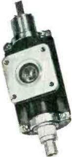
**RK6410/QK338** — fixed frequency, pulse magnetron (2750-2860 Mc), 5 megawatt average peak power
