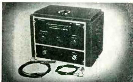
Permits examination of any signal under observation without the amplitude loss or waveform distortion generally experienced with conventional R-C probes. The low input capacitance (less than 2 MMF) results in a minimum of loading, particularly on high impedance circuits. Invaluable for operational checks on computers, TV sync amplifiers, and pulse circuitry.
