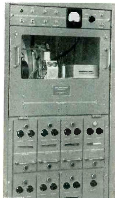
Truck-mounted seismic recorder contains seven dual-channel modulators
