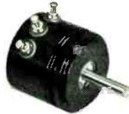
Designed for minimum-torque uses. Minimum torque is 0.01 inch-ounce. Dissipates one watt at 80° C. Resistances — 100 to 100,000 ohms. Weight is only 1/2 ounce. Ganging to 6 decks, internal clamps hold 7/8 in. diameter.
