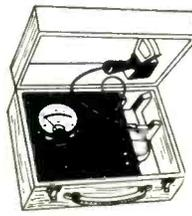
Used to calibrate field strength of magnets from 500 to 4000 gauss and indicate polarity. Probe has gap of 1 1/4". Beautifully built in hardwood case with hinged cover. Instructions for operation on under side of cover. Size 12 1/2 x 9 x 6 in. Ideal for lab and school use. New.
