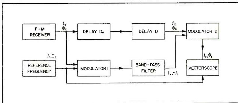
FIG. 6—Application of the vectorscope as an f-m monitor. The signal from the receiver is fed to the vectorscope through a double-beat converter
