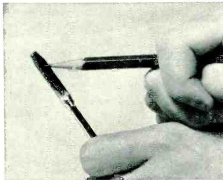
**RAPID HEAT TRANSFER** is achieved through a Calrod heater cast in copper. The Midget iron can melt solder in less than a minute, recovers heat in seconds.
