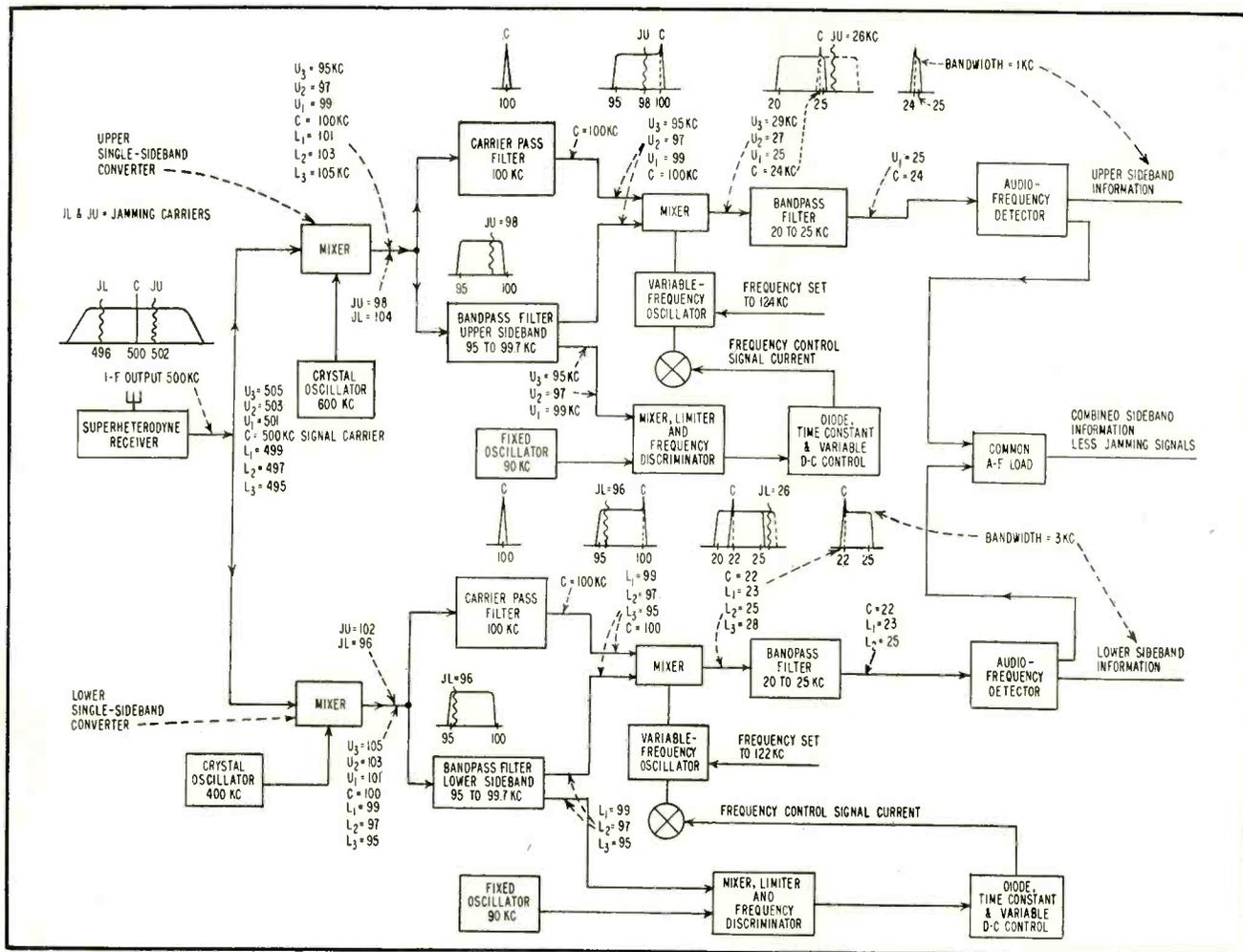
FIG. 6—Automatic bandwidth control rejects jamming carriers in a dual single-sideband receiving system
