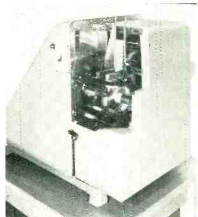
New high-speed printer as set up for applying four color bands to molded paper capacitors at rate of 50 parts per minute. Painted parts drop down slide at left into tote box (not shown)
