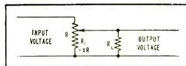
FIG. 1—Simple potentiometer circuit showing symbols used in design equations
