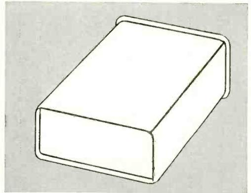
BOTTOM OF CASE IS INDENTED to permit mounting in inverted position.
