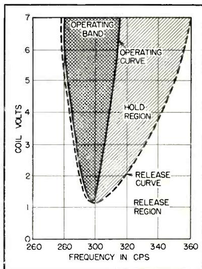
FIG. 7—Typical characteristic of resonant relay shows that operate and release are substantially at same coil voltage below resonance
