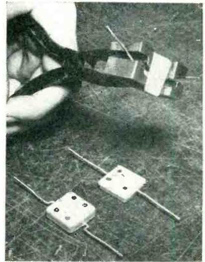
Tool for making double bends in leads of mica capacitors for mounting on turret terminals
