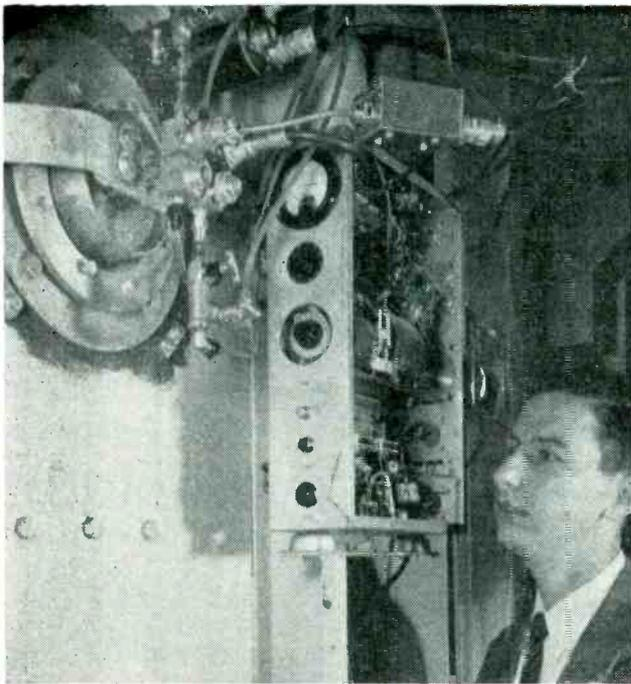
Primary frequency generator uses what is basically a grounded-anode Colpitts circuit
