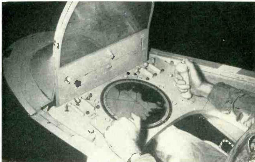
Mockup of aircraft cockpit made by Douglas Aircraft for Navy's instrument simplification program. The two large instruments are flat-plate Willys tubes on which information needed to fly aircraft will be displayed
