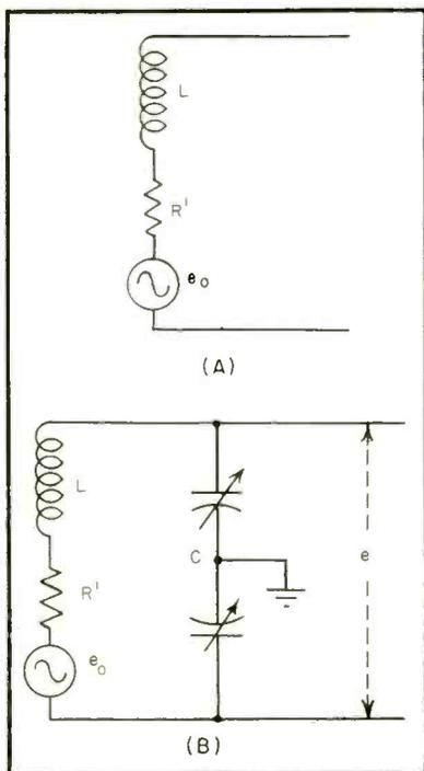
FIG. 1—Equivalent circuit (A) of loop antenna and loop with capacitance added (B) to form resonant circuit
