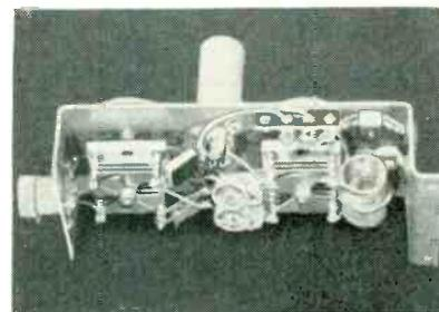
Amplifier subchassis has shafts of two-gang capacitors coupled together for tuning in range of 30 to 40 mc
