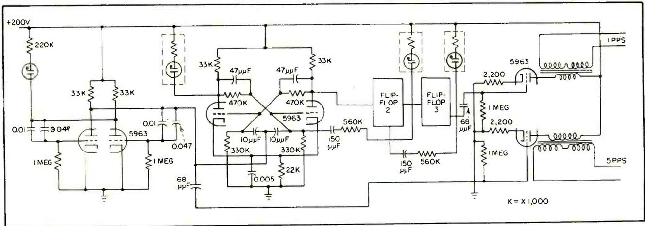
FIG. 6—Schematic of time base generator for laboratory checkout of main control rack circuits
