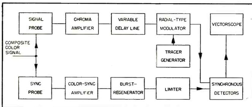
FIG. 4—Setup for using vectorscope as color monitor. Bandwidths of chroma and color-sync amplifier should be 2 to 4 and 0 to 4 mc respectively
