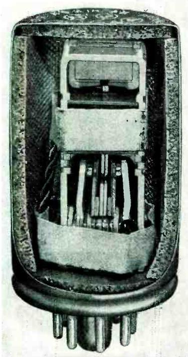
FIG. 14—Cutaway of chopper in which oversize contacts operated with high impact give long life (Airpax Products)
