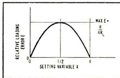
FIG. 2—Error in voltage transmission in potentiometer caused by load is maximized at halfway point in potentiometer range
