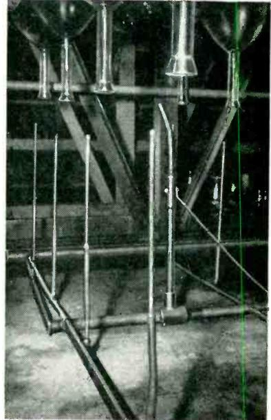
Drying rods on carriage which moves at same speed as overhead conveyor for picture tubes
