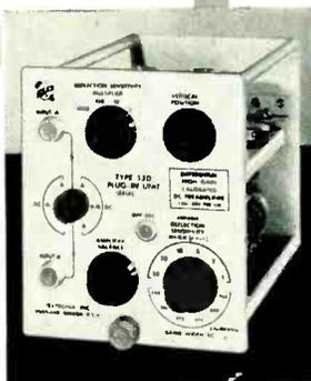
**TYPE 53A**—DC to 5 mc, 0.07- $\mu\text{sec}$  risetime. Sensitivity 0.05  $\text{v/cm}$  to 50  $\text{v/cm}$ , ac or dc, continuously variable, with 9 calibrated steps from 0.05  $\text{v/cm}$  to 20  $\text{v/cm}$ , **\$85.00**
