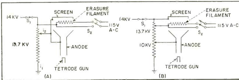
FIG. 2—Divider circuits for elimination of erasure-filament shadow during writing in conventional operation (A) and with post-deflection acceleration (B). Switches are shown in write position. For erasure  $S_1$  would be open and  $S_2$  closed
