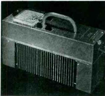
The toxic limit is a full scale reading on the high sensitivity scale of Model 23, illustrated above. The weight is 7 pounds and the size is 13 x 8½ x 4½ inches.
