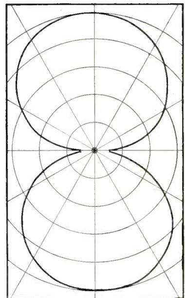
FIG. 3—Directivity pattern of resonant loop in region of 30 to 40 mc
