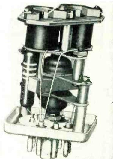
FIG. 8—Frahm oscillator control consists of two reeds mounted on a bar to form a vibrating element isolated by rubber mounts from base (James G. Biddle)
