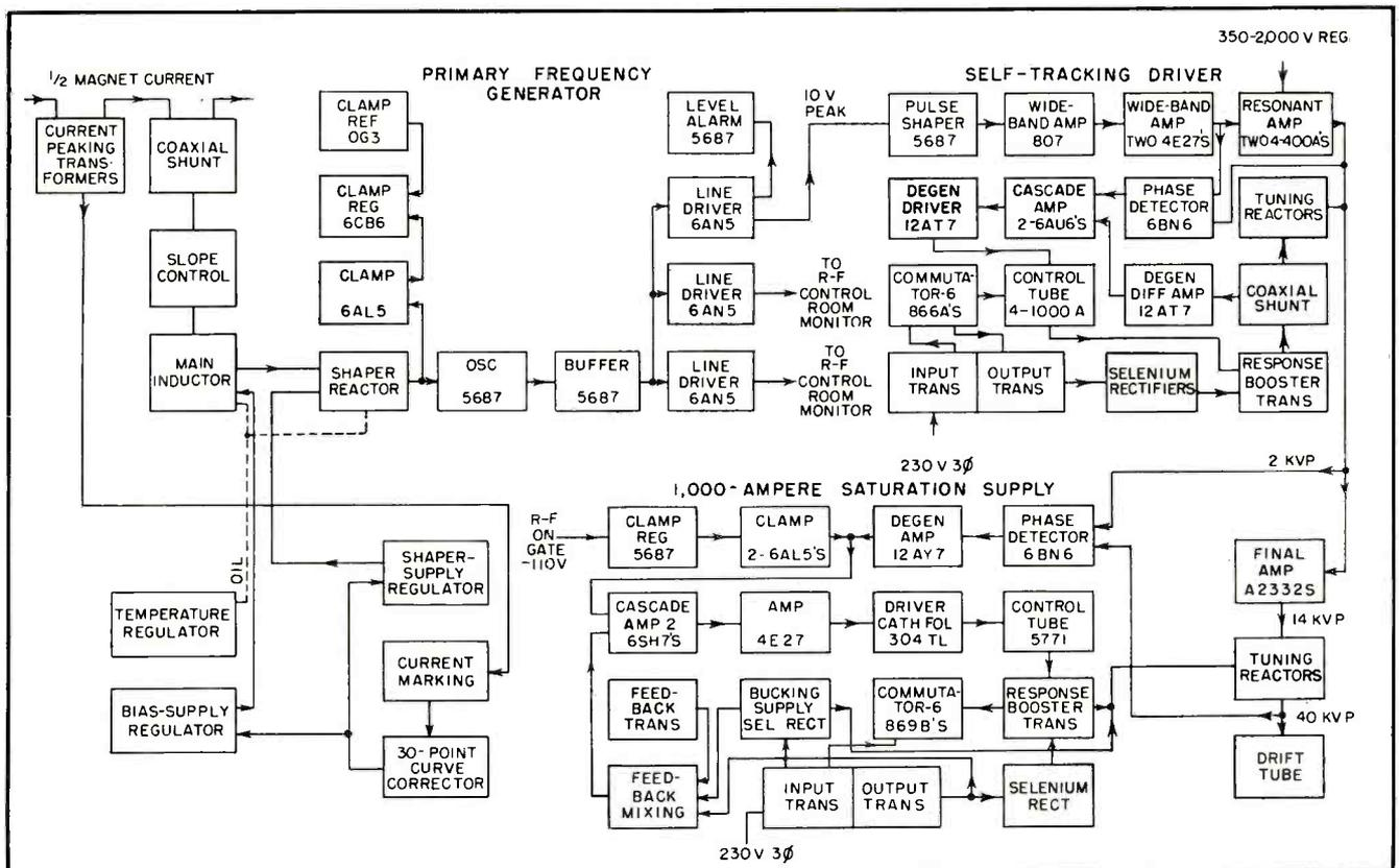
FIG. 4—Block diagram of the bevatron radio-frequency system. Output frequency is virtually independent of vacuum-tube parameters
