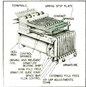
FIG. 6—Ten armatures are attracted sequentially by series of pulses applied to single winding (Kellogg)
