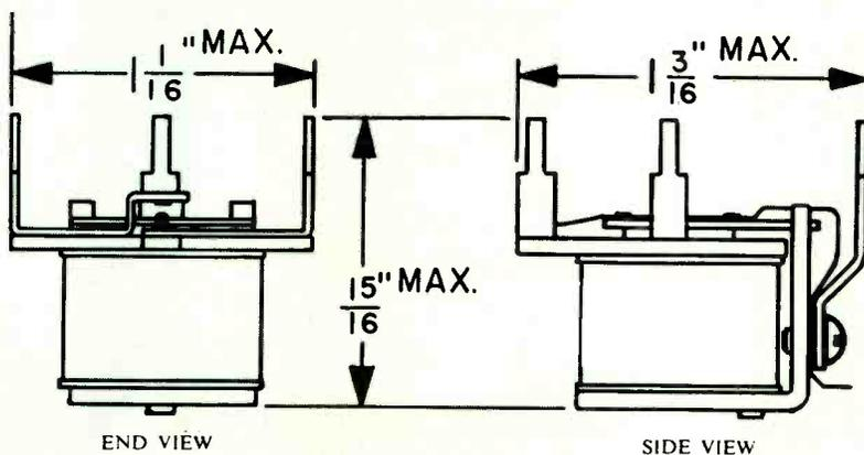
Here are the completely new **Phil-trol Type 15QA Relays** (above and below). Sub-miniature in size, light in weight, they are ideal where dependable performance is a "must"—as in delicate instrumentation, Radiosonde equipment, or the Autronic Eye. Available for DC operation up to 60 V., with contact 1 Form C (S.P.D.T.).
