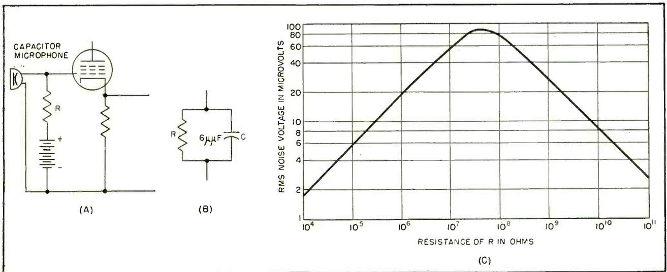
FIG. 1—Hypothetical microphone cathode-follower circuit (A) and equivalent circuit (B). Plot (C) shows open-circuit rms noise voltage produced by thermal agitation in real component of impedance of equivalent circuit
