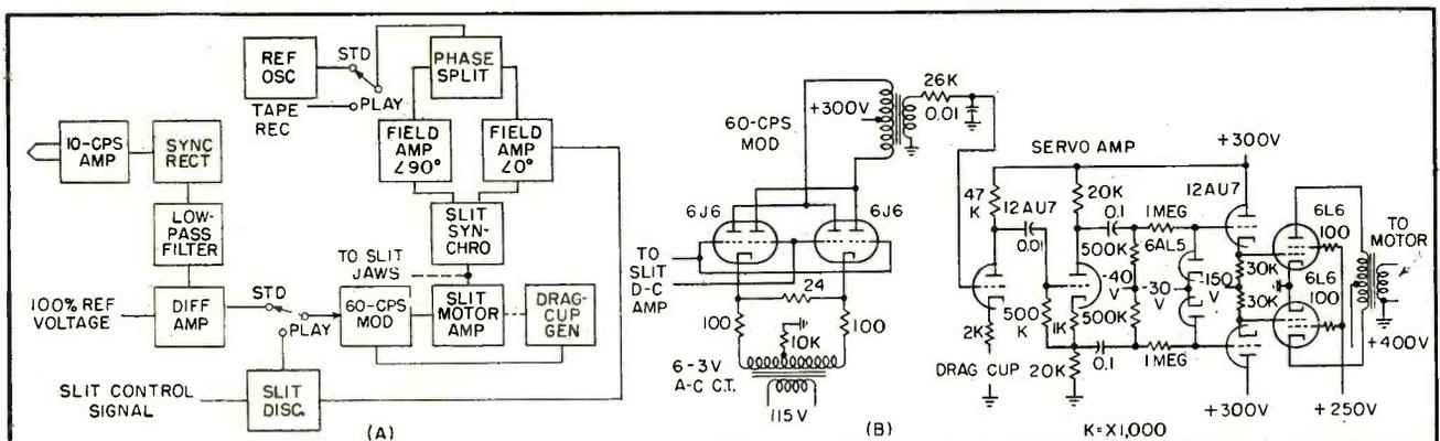
FIG. 5—Block diagram of slit control system (A) and schematic of slit modulator and motor amplifier (B)
