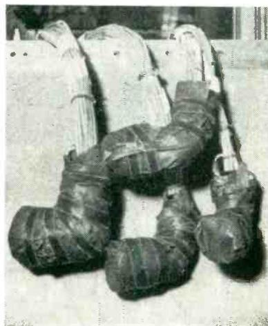
Old method of waterproofing plugs by wrapping and taping
