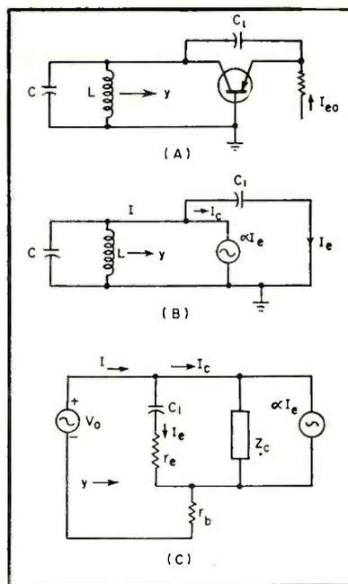
FIG. 3—Basic transistor reactance circuit used in Fig. 2(A) simplified (B) and complete (C) equivalent circuits
