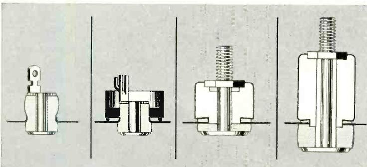
FOUR BUSHINGS STYLES are available for applications below 2000 volts d-c, special skirted bushings for higher voltages.
