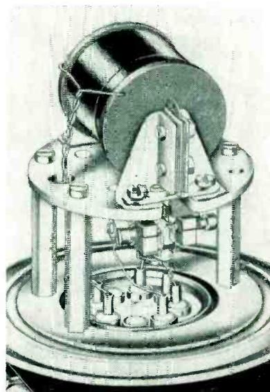
FIG. 13—Chopper provides highly symmetrical low-level switching with stable phase of switching action (Bristol Co.)
