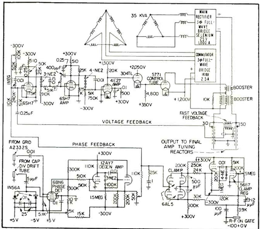
FIG. 7—Saturation supply regulates current from 0 to 1,000 amperes
