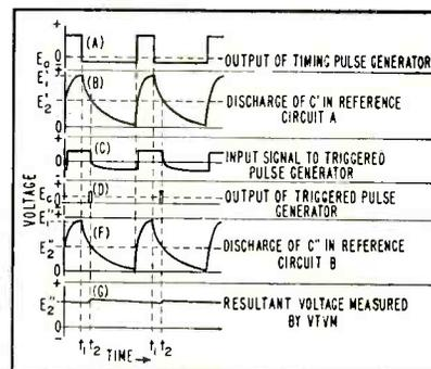
FIG. 2—Timing generator operation in terms of waveforms
