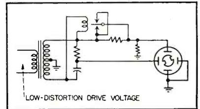
FIG. 15—Test setup for measuring dwell times of Airpax chopper. Accuracy is improved by reversing polarity to drive coil to interchange dwell time periods
