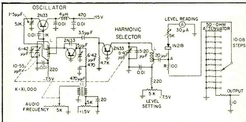
FIG. 2—Oscillator is modulated by 2N33 reactance transistor over vhf range
