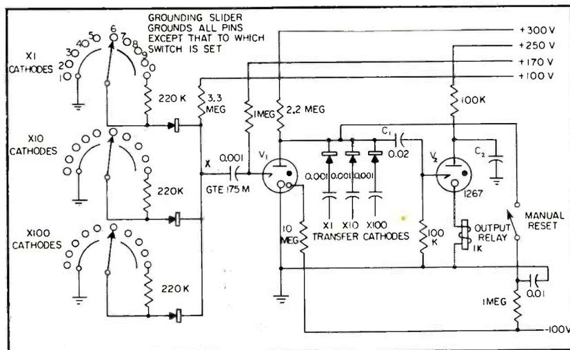
FIG. 2—Selector and reset circuit uses three rotary switches for unit selection. A negative pulse fed to all the cathodes resets the counter to zero
