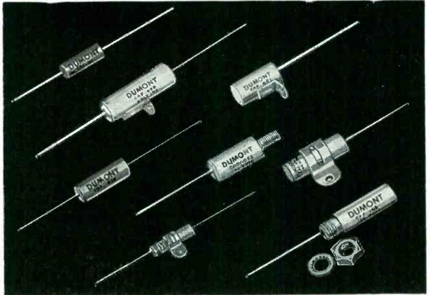
MILCAPS are subminiature paper capacitors hermetically sealed in tinned brass tubular cases. Perfect enclosure of the impregnated paper sections is achieved by the use of glass-to-metal solder seal terminals. MILCAPS are recommended for all applications where size is a primary consideration . . . and are available in any one of the following impregnants: Stabilized Halowax (85° c); Mineral Oil (85° c; or Duroil (125° C).
