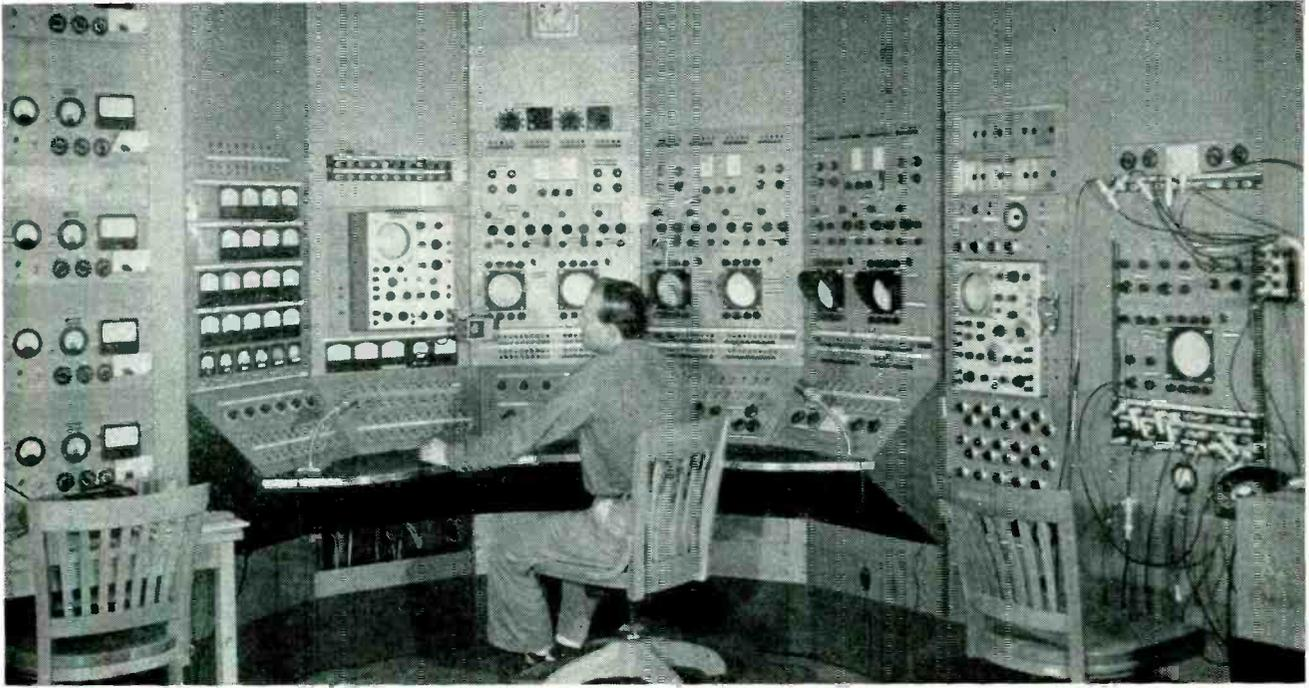
Main control room showing use of special dual-beam oscilloscopes. Accelerator operator is looking at the frequency monitoring scope (above left hand). Bevatron employs practical self-tuning system
