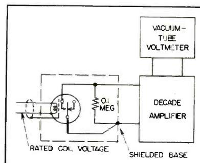
FIG. 12—Measuring noise from chopper
