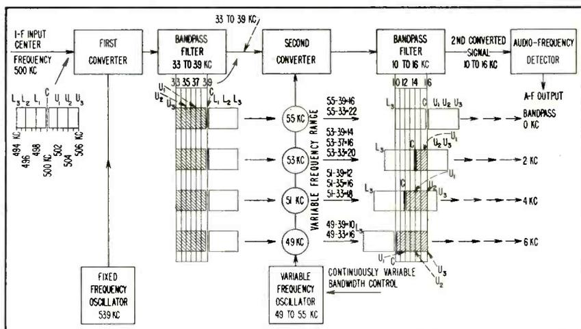
FIG. 2—Elements of electronic variable-bandwidth control system using two converters, crystal and variable frequency oscillators and filter
