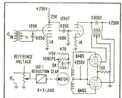
FIG. 3—Integrator for electromechanical system can provide a-c or d-c output depending on the signal used to excite the motor-driven potentiometer
