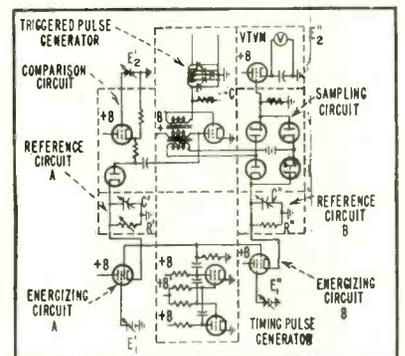
FIG. 1—Number can be raised to power greater or less than unity in this circuit, which forms portion of new computer design
