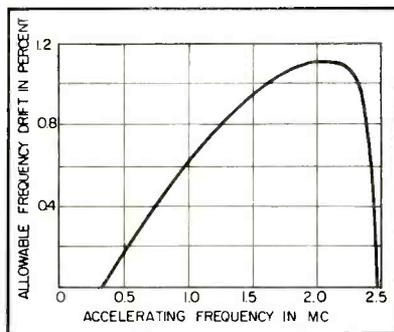
FIG. 3—Frequency tolerance of the radio-frequency system
