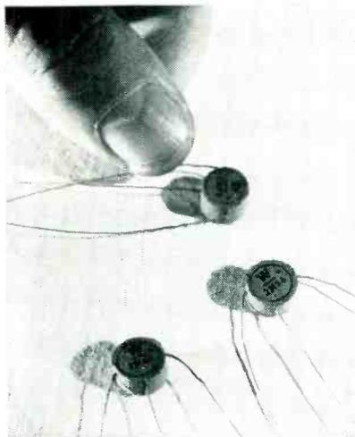
junction transistors. The transistors (types 2N54, 2N55, and 2N56) are designed for low-power, low-frequency amplifier applications. Each is capable of dissipating 200 mw at 25 C. All are provided with leads for wired-in installation. The average cutoff at the 6-mw power level is 500 kc. The average current gain of the transistors are: 2N54—0.97; 2N55—0.95; and 2N56—0.92.
