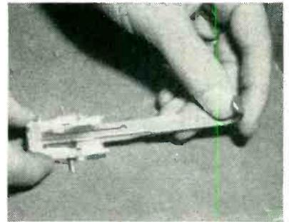
Gage in position in stub that has been sawed in half to show inner construction of coaxial unit
