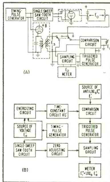
FIG. 3—Blocks showing system for solving an equation (A) or finding logarithms to any base (B)
