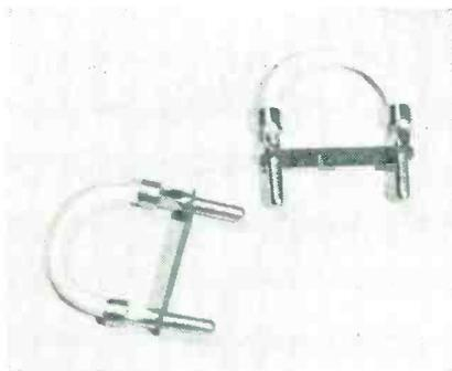
but will fuse when surge becomes dangerous to expensive components. An example of this type resistor is the series 4FYG-001, Part No. CM14282, a 7.5-ohm resistor normally carrying 1 ampere and withstanding surge currents of 1.75 amperes. It is designed to fuse at 2.3 amperes in less than 30 sec.
