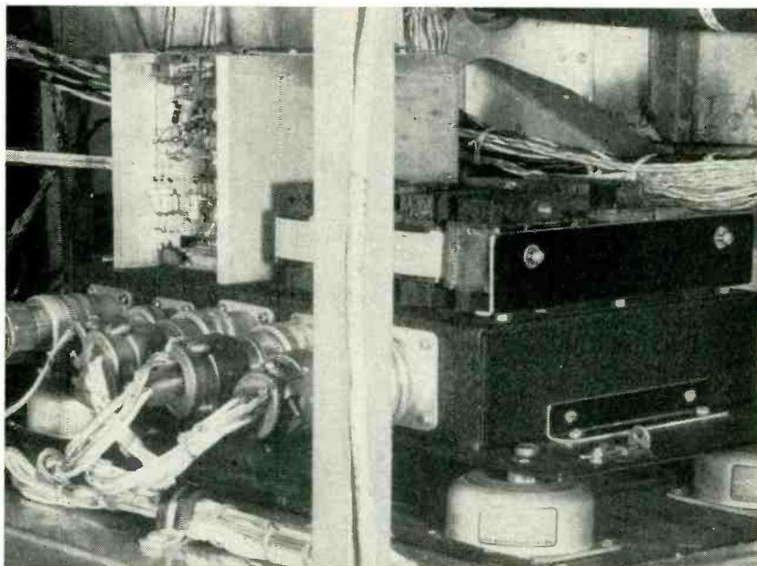
**ENGINEERING** prototype of the Bendix autopilot that uses card-type transistorized amplifiers, top left, is flight tested as . . .
