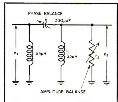
FIG. 3—Tuned-pi quadrature network employed in circuit of Fig. 2
