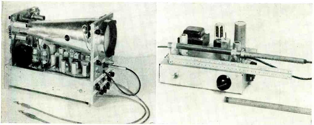
Vectorscope for color-signal monitoring. Separate sync and signal-probe inputs permit constant maintenance of phase reference while the signal probe explores various parts of receiver or transmitter circuitry. Each probe consists of a small head with an input capacitance of less than  $3 \mu\text{mf}$  attached to a 3-foot cable. Variable time-delay control unit consists of single-layer helix on top of slotted metal tube, with moving-coil pickup inside
