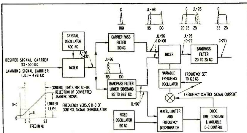
FIG. 5—Elements of automatic bandwidth control that rejects jamming
