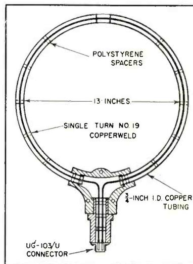
FIG. 4—Cross-section of antenna. Shield is discontinuous at top and bottom
