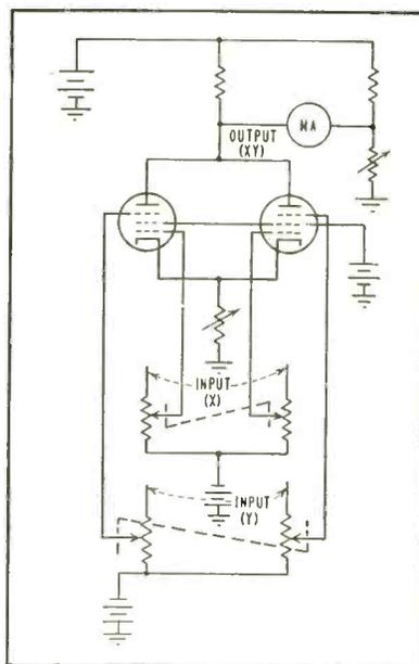
FIG. 4—Product of two independent variables is continuously indicated
