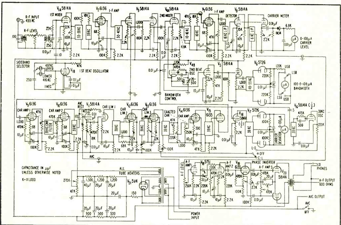
FIG. 4—Upper or lower sideband can be selected at will. Electronic bandwidth control operates by tuning oscillator V4B
