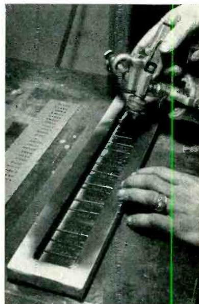
Spraying resistor board with DeVilbiss spray gun, using stencil frame having wires that automatically press stencil against board
