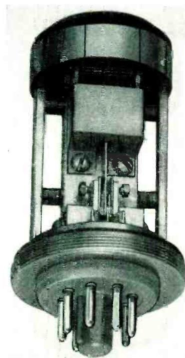
FIG. 11—Chopper housed in M<sub>2</sub>-metal case, giving noise level below one microvolt into 100,000-ohm load, rated for operation from 0 to 43 C (Stevens-Arnold)
