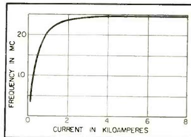
FIG. 2—Accelerating potential frequency plotted as a function of total magnet current
