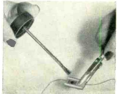
Holding photocell element together with padded spring clamp while applying cement
