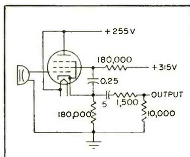
FIG. 2—Stick-type capacitor microphone has free-grid cathode follower incorporated into microphone base
