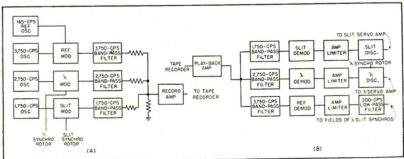
FIG. 4—Recording (A) and playback systems (B) permit use of magnetic tape for instrument calibration
