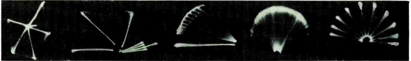
Left to right: NTSC color-bar signal as displayed on vectorscope; vector rotation of color carrier with and without phase multiplier; spurious phase rotation in a color-video stage; standard quality f-m signal; phase and amplitude response of delay band-pass filter
