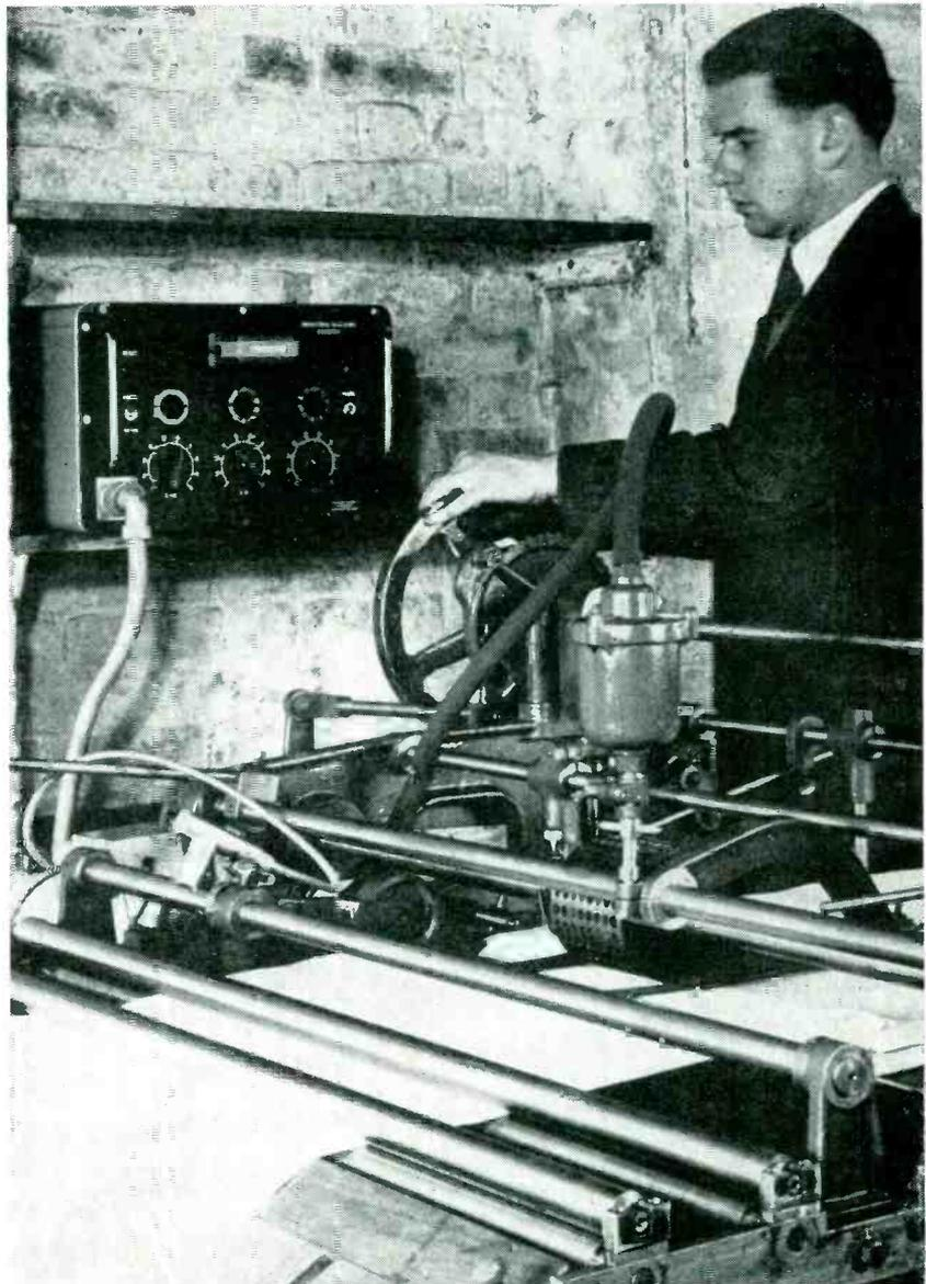
Typical installation of counter on paper cutter counts and batches sheets of paper into quires or other quantities
