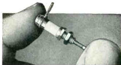
*New CST-50 variable ceramic capacitor* surpasses range of capacitors many times its size. Stands only  $1\frac{1}{2}$ " high when mounted, is less than  $\frac{1}{4}$ " in diameter and has an 8-32 thread mounting stud. A tunable element of unusual design practically eliminates losses due to air dielectric giving large minimum to maximum capacity range (1.5 to 12MMFD).
