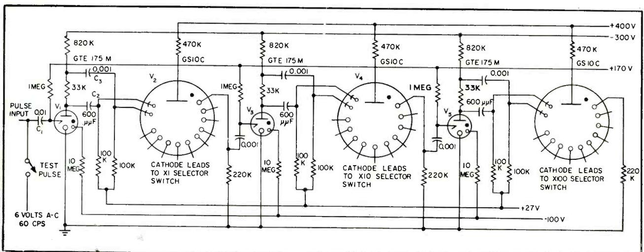
FIG. 1—Counter circuit uses three GS10B dekatron selector tubes. These tubes have a counting rate of 500 per second. Test-pulse switch permits injecting of 60-cycle signal into counter to check its operation
