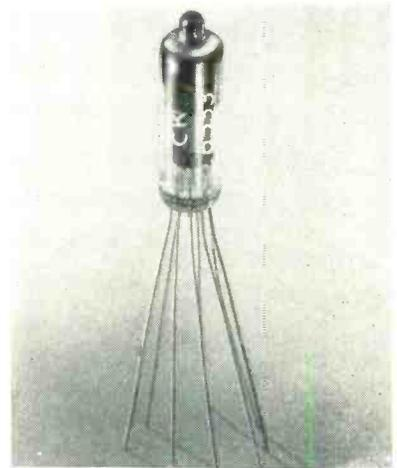
the plate circuit is a maximum of 1 mv with typical tubes usually reading between 100 and 200  $\mu$ v. At vibration frequencies as high as 10,000 cycles, 15 g, the noise output seldom exceeds 1 mv thus making this type of extreme interest for guided missile and other critical electronic equipment applications.
