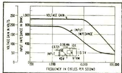
FIG. 3—Grounded-emitter transistor amplifier response curves
