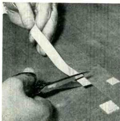
Applying NBS adhesive-tape capacitors manually to steatite blank wafers
