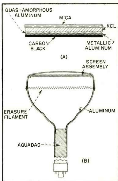
FIG. 1—Scotophor deposited on mica sheet (A) has aluminum and carbon-black backing to absorb infrared radiation. Complete tube assembly (B) shows position of erasure filament
