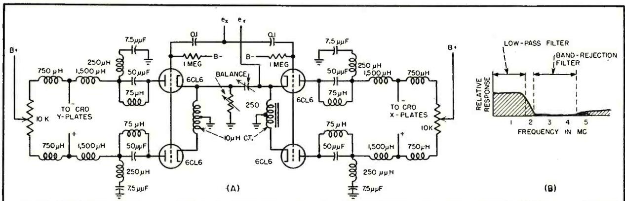
FIG. 2—High-level pulsed envelope detector used in vectorscope (A); relative frequency response of detector (B)
