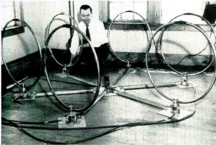
Sextuple goniometer driven synchronously records noise or signals at various frequencies. Loop antennas complete a revolution every 15 minutes
