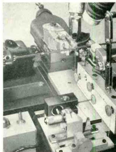
Winding lathe as seen from rear, with tension-sensing system in foreground
