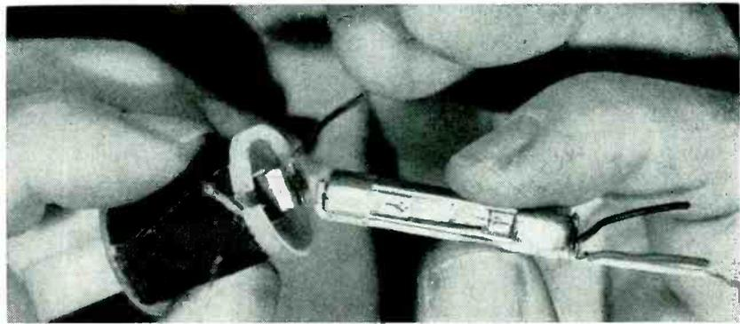
FIG. 10—High-speed relay operates in 0.2 millisecond when driven from a high-resistance power source, and releases somewhat faster (Stevens-Arnold)
