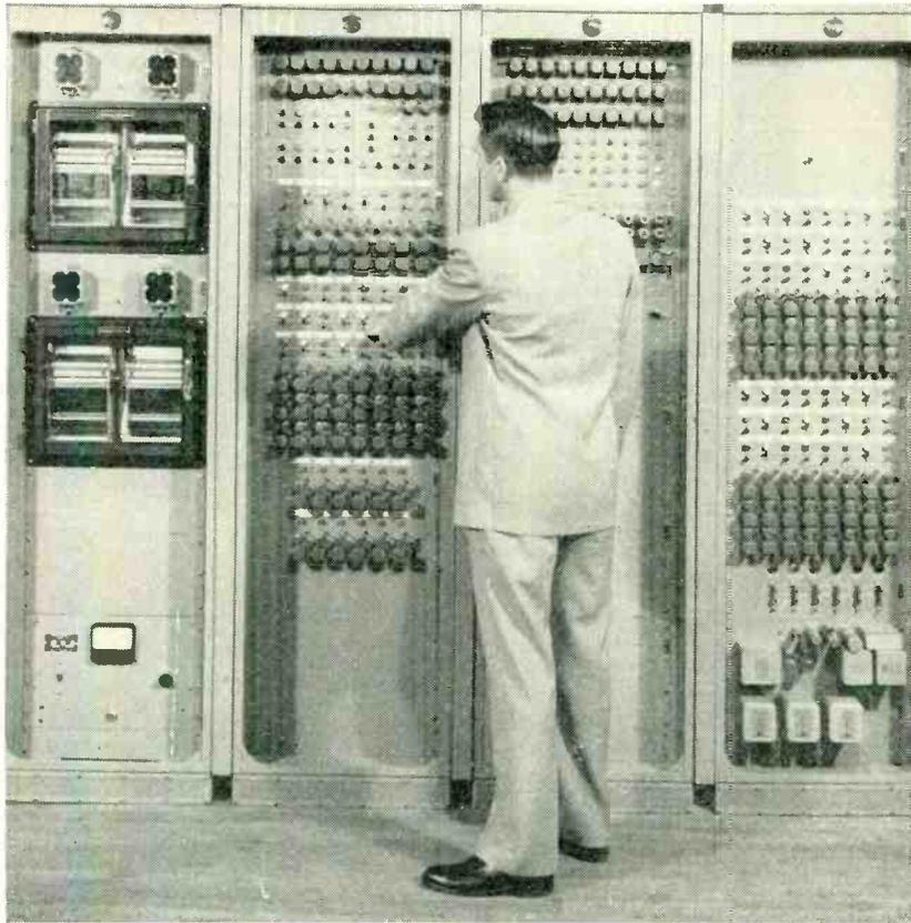
View of main control racks illustrates complexity of equipment. Engineer is checking function relays
