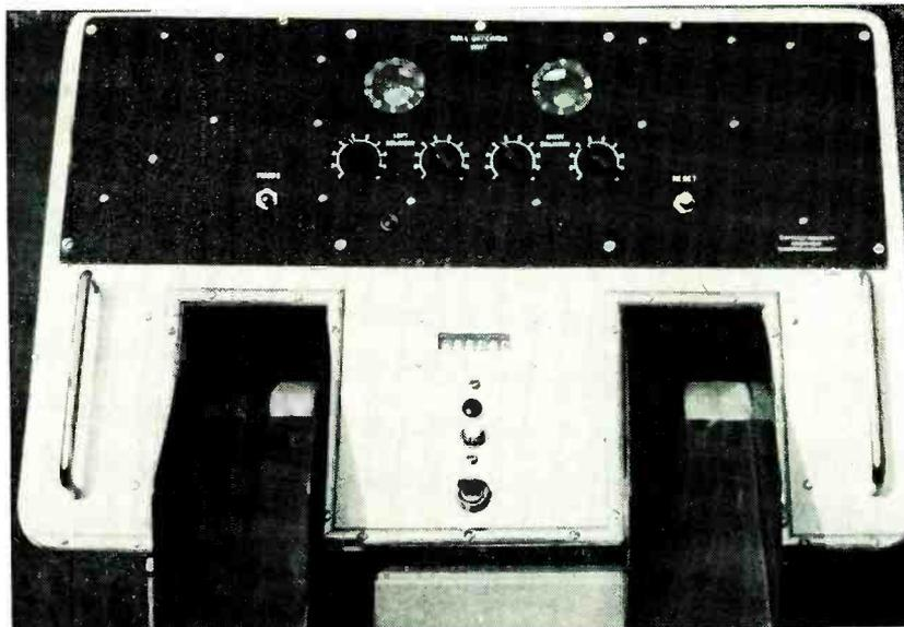
Counter for batching bread rolls into two loading chutes
