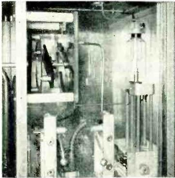
FIG. 4—Vacuum relay for 10-kv power supply has adjustable trip setting from 1 to 8 amp (Jennings Radio)
