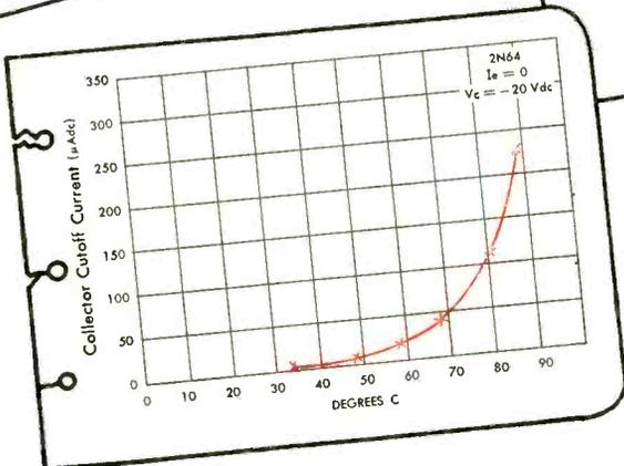
Look at these typical curves taken on a Raytheon 2N64. You can see for yourself how reliably they perform at high temperature. These transistors are rated up to 85°C operating temperature — maximum storage temperature up to 100°C.
