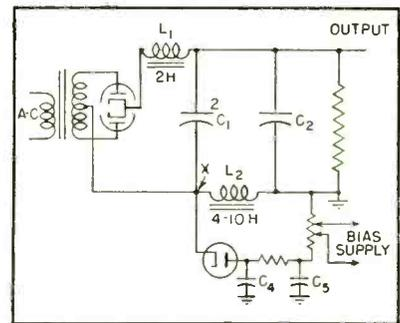
Half-wave power supply provides 100-volt bias source without excessive loading of power output
