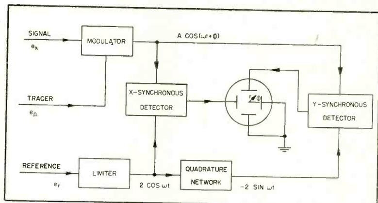
FIG. 1—Basic arrangement of vectorscope elements
