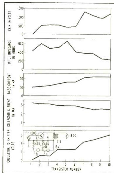
FIG. 4—Uniformity of characteristics for ten CK 721 transistors
