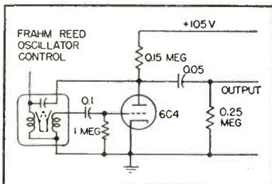
FIG. 9—Oscillator circuit with resonant-reed control of frequency provides 1.5 v output at 20 C with 20,000-ohm load
