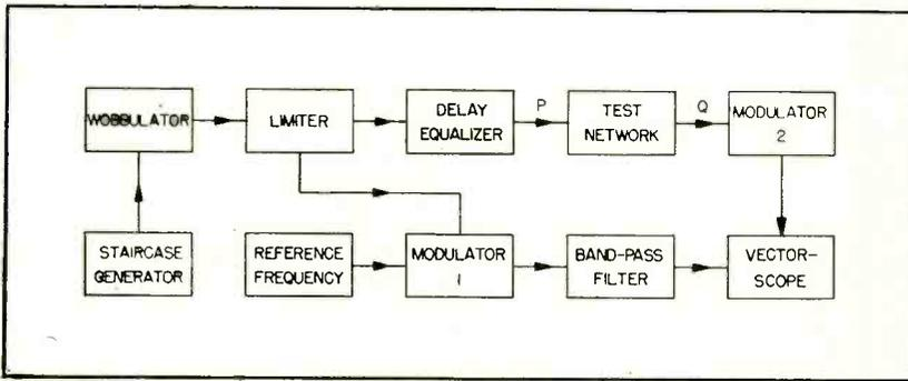
FIG. 7—Setup for phase-delay presentation with the vectorscope. Circuit resembles that of Fig. 6 except that f-m signal is replaced by signal generator
