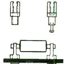
An efficient, new way of holding crystal diodes. Three types available. Model #9000 for front panel mounting. Model #X9000 for front panel mounting with a blind hole for dip solder application. Model #9020 for rear-of-panel connections. All models available for standard terminal board thicknesses, or to your specifications. Silver plate on half hard brass assures good contact resistance. Retains excellent grip after multiple insertions.
