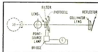
**FIG. 1—**Optical system of photometer has two positions. Reflective surfaces are measured with point-source lamp in position shown. Retroreflective surfaces (like reflector buttons) are measured with the lamp and lens retracted (dashed lines)
