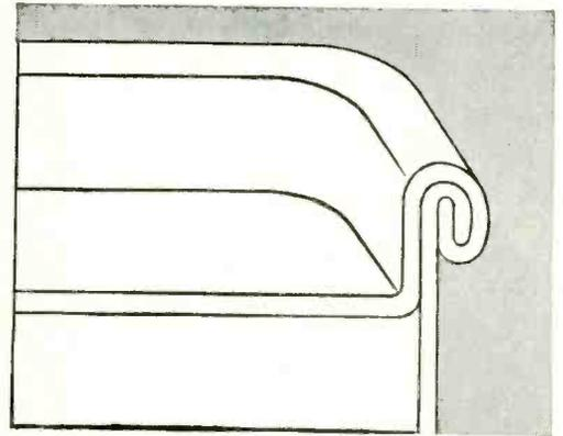
SOLDERLESS DOUBLE-ROLLED COVER SEAM makes a mechanically strong, hermetic seal.
