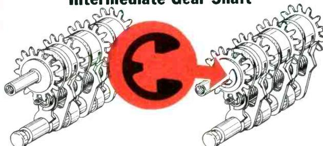
**Old Way.** Washer riveted on end of assembly for zoning control. Costly, troublesome, hard to obtain critical zoning required.
