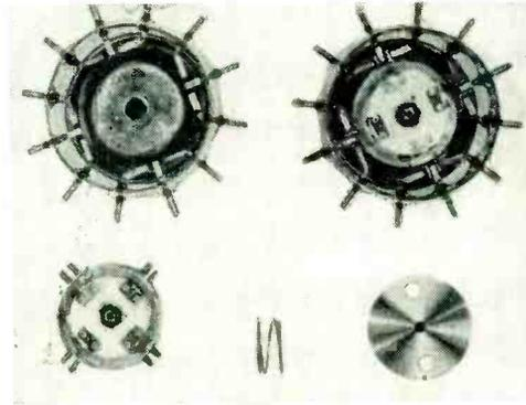
FIG. 5—Jennings multiple-pole double-throw vacuum relay can switch several high-voltage high-current circuits in synchronism
