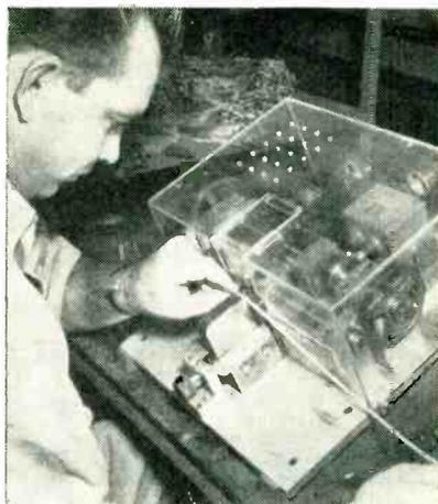
Method of holding shielded wire on anvil of automatic cutter
