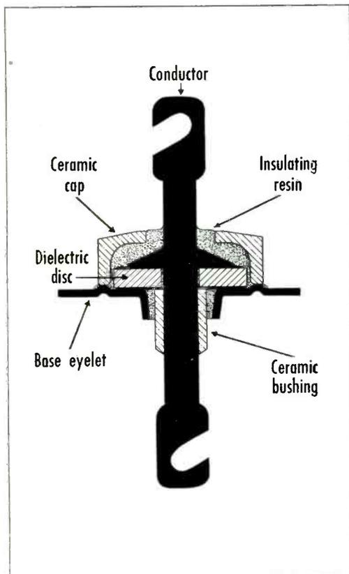
The isolating or filtering performance of a feed-thru capacitor is a function of its common or "coupling impedance." This is the shunt impedance between its free electrode and the metal shield or chassis on which it is mounted. Capacitors which exhibit the smallest "coupling impedance" are superior for those applications where filtering is desired.
