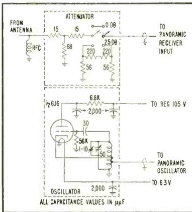
FIG. 1—Attenuator and supplementary oscillator extends frequency range of commercial panoramic spectrum analyzer that is used by monitoring officers to check mobile transmitters
