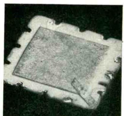
Finished unit. Conductive tape connects top element to tinned notch
