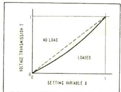
FIG. 3—Effect of resistive load on dial calibration of potentiometer
