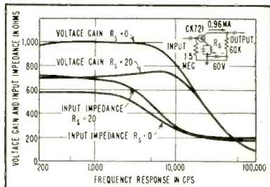
**FIG. 2—Frequency response of grounded-emitter amplifier with series emitter resistance**
