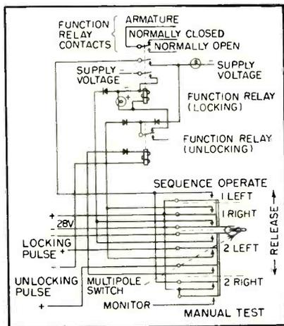
FIG. 4—Typical circuit of a function relay
