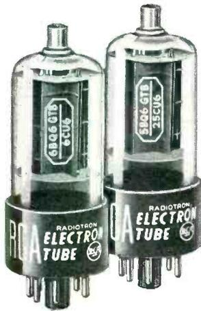
**NEW—RCA-6BQ6-GTB/6CU6, 12BQ6-GTB/12CU6, and 25BQ6-GTB/25CU6** are directly interchangeable with similar types in the 6BQ6 family. In comparison with previous versions, these types retain the same desirable characteristics, but feature a modified mount design to provide higher perveance and to permit higher ratings.
