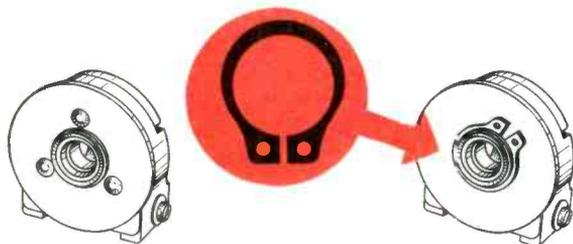
**Old Way.** Collector Disc assembly was formerly riveted, requiring skilled labor. Riveted Collector Disc could not be removed in the field.
