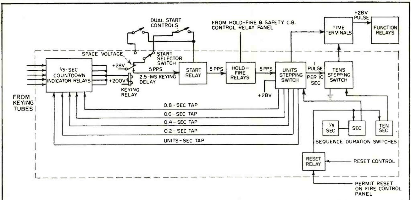
FIG. 2—Functional block diagram of automatic sequence panel
