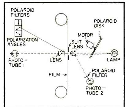
FIG. 8—Film scanner for chart drive
