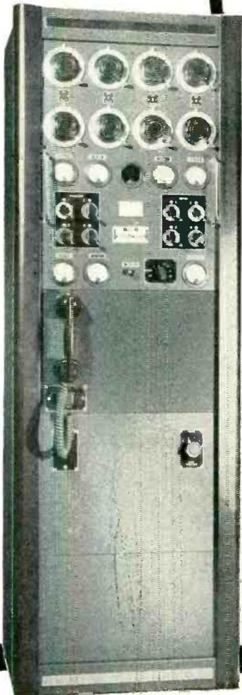
*Model 446 transmitter operates on 4 crystal-controlled frequencies (plus 2 closely spaced frequencies) in the band 2.5-24.0 Mcs (1.6-2.5 Mcs available). Operates on one frequency at a time; channeling time 2 seconds. Carrier power 350 watts, A1 or A3. Stability .003%. Operates in ambient -35° to 45°C. Nominal 220 volt, 50/60 cycle supply. Conservatively rated, sturdily constructed. Complete technical data on request.*
