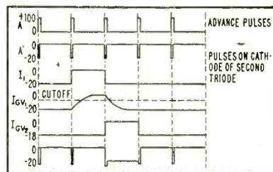
FIG. 7—Time relationship of pulses in shift register
