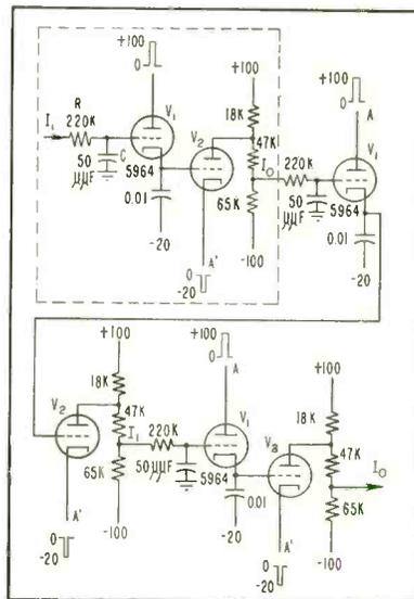
FIG. 6—Three-stage shift register (one stage within dashed lines)
