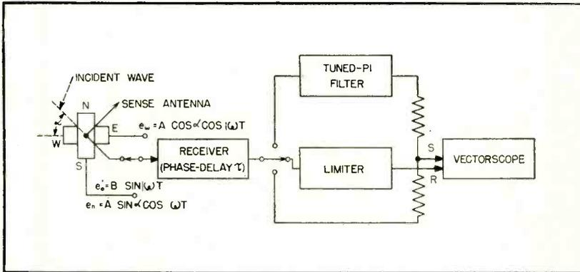
FIG. 8—As an element of an all-electronic direction finder, the vectorscope displays small differences in the time of arrival of a signal carrier at the site of various component antennas forming a directive antenna array
