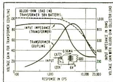
**FIG. 1—Frequency response of transistor amplifier with load matched for maximum power output**
