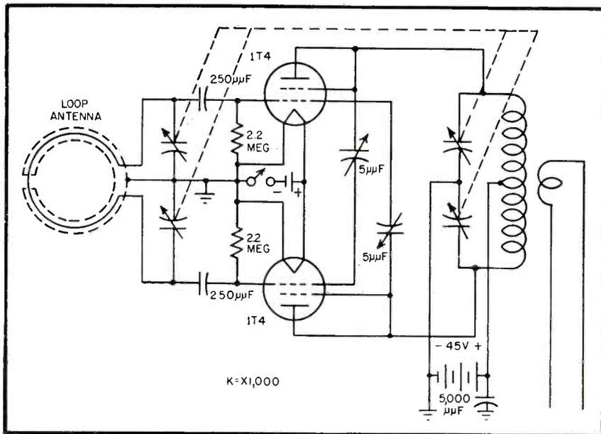
FIG. 2—Push-pull amplifier provides balanced input for direction-finding antenna along with unbalanced 50-ohm output to coaxial line
