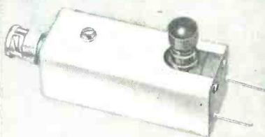
**RCA WG-298A UHF DEMODULATOR**—connects the output of the WR-86A sweep generator and a 300-ohm termination for use in measuring the approximate standing-wave ratio of a 300-ohm-transmission line throughout the UHF range of 300-950 Mc. The WG-298A may also be used with other instruments such as the WR-40A, WR-41B or any UHF sweep generators using a 50-ohm BNC type output connector.
