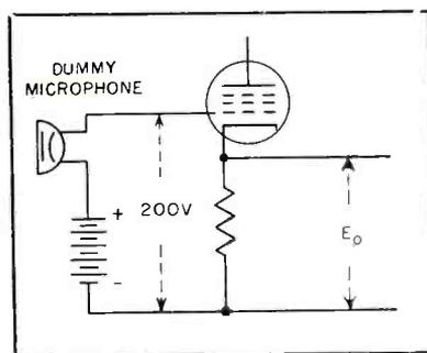
FIG. 3—Circuit used to determine noise
