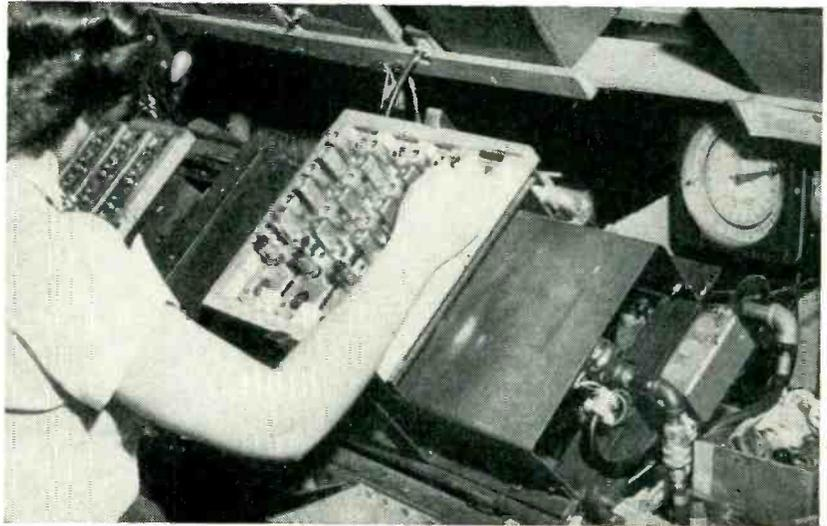
Air cylinder under metal cover here operates every four minutes to drive plunger that pushes racks on line at left one position further down slowly
