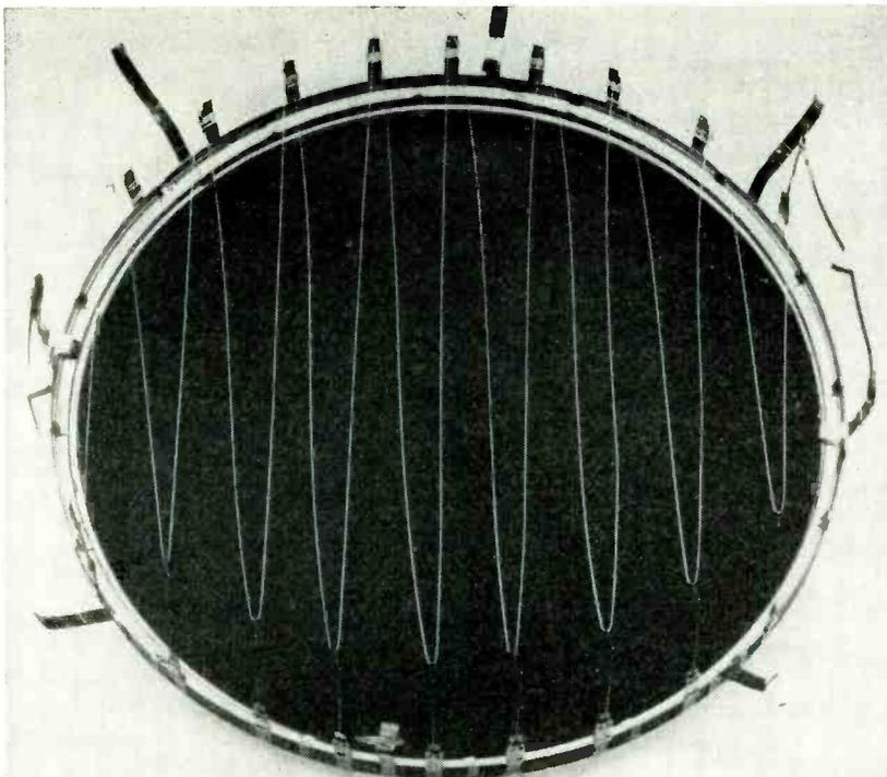
Zig-zag erasure filament is mounted on hangers about 2 inches from screen
