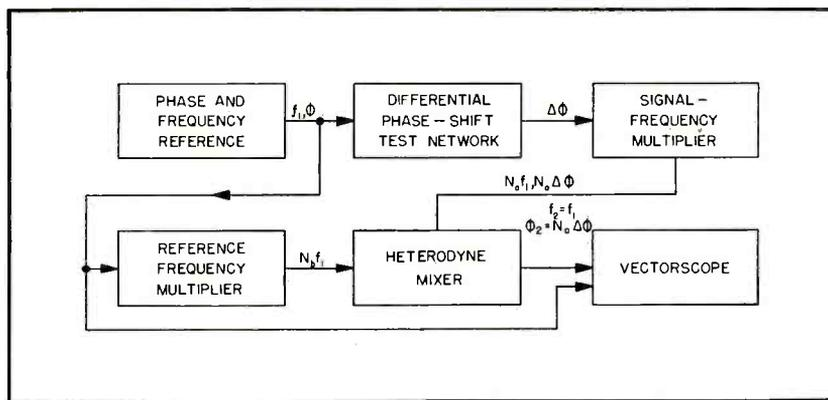
FIG. 5—Use of a phase magnifier in conjunction with the vectorscope permits observation of phase angles that would normally be too small to be seen
