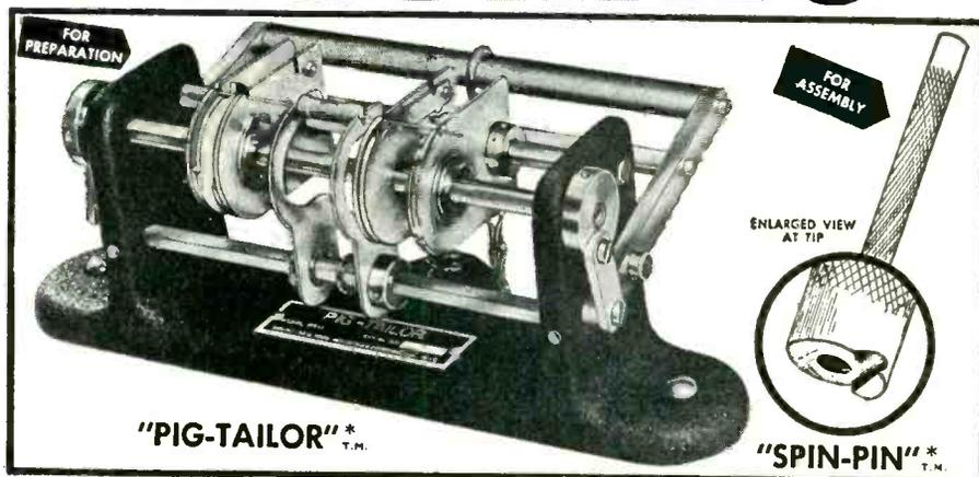
The "PIG-TAILOR" plus "SPIN-PIN" — Accurately Measures, Cuts, Bends, Ejects and Assembles both leads simultaneously to individual lengths and shapes — 3 minute set-up — No accessories — Foot operated — 1 hour training time.
