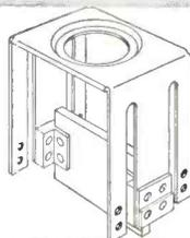
A parallelgram suspension confines the mass of the GLH to a virtual straight line motion and provides excellent lateral rigidity.
