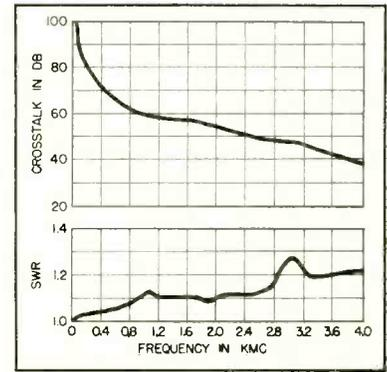
FIG. 3—Measured crosstalk and swr for coaxial spdt relay in which blade shorts to cavity wall in one position
