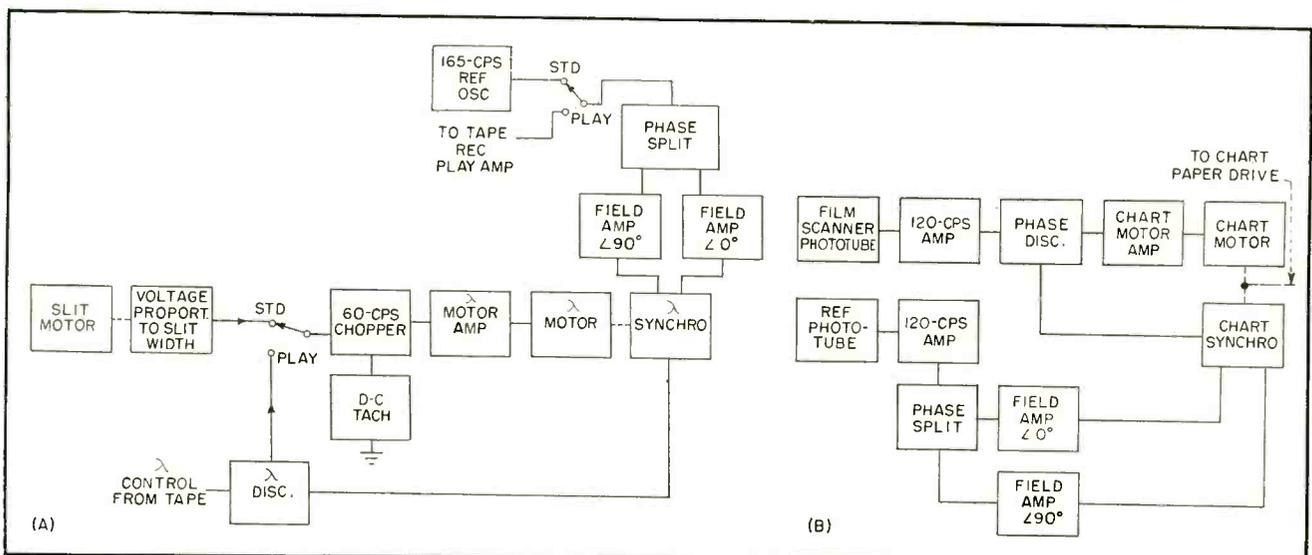
FIG. 6—Wavelength control system (A) and chart drive system (B) demonstrate similarities in their electrical design
