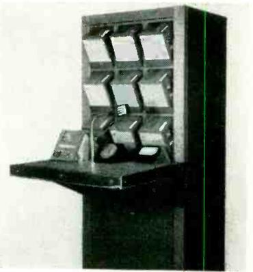
Battery of ten tape recorders that can be switched in sequence
