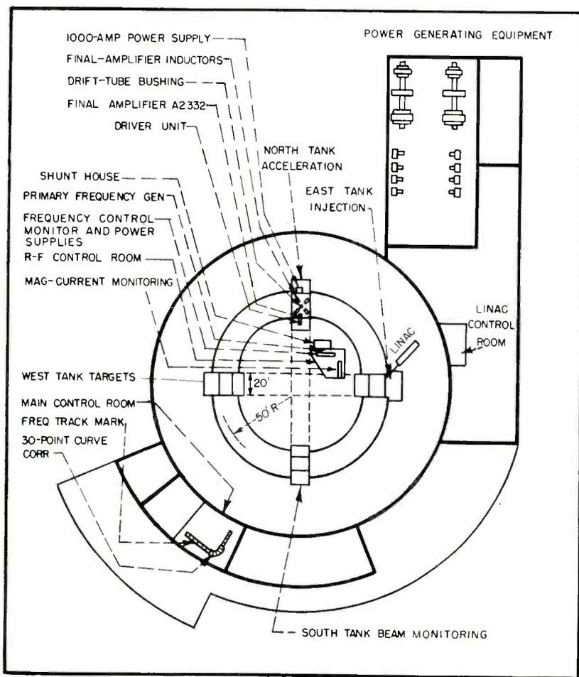
FIG. 1—Simplified plan view of 6-billion electron volt accelerator
