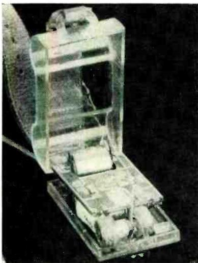
TECHNICAL information on the experimental wrist watch radio developed by the Army Signal Corps in 1953 (ELECTRONICS, p 5, October, 1953) has been released by the Commerce Department's Office of Technical Services.
