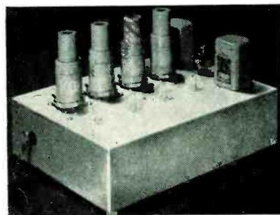
Time base generator for laboratory checkout uses plug-in circuits
