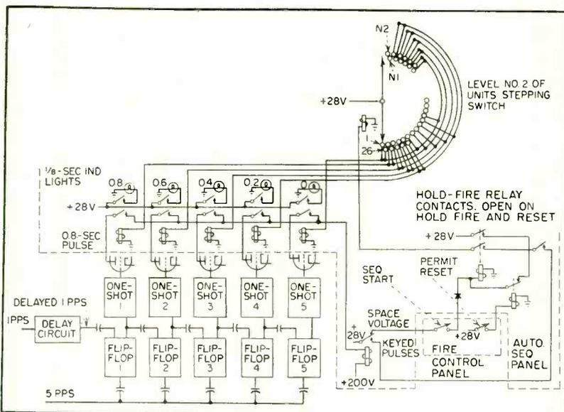
FIG. 5—Basic schematic of stepping-switch synchronizing circuits
