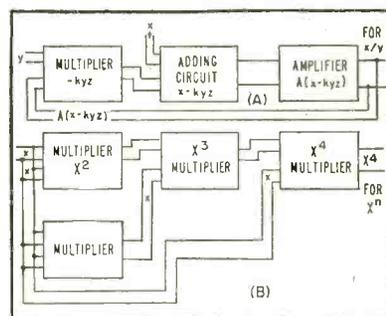
FIG. 5—Method of dividing (A) or raising to a power (B)
