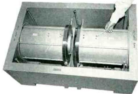
**1/2-TON PERMANENT MAGNET** . . . Here is one of the world's largest permanent magnet assemblies. Used in nuclear resonance research, it contains over 1,000 pounds of Indiana Hyflux Alnico V, and produces a magnetic field of 6,750 gauss in the air gap.
