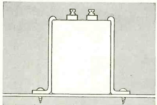
UPRIGHT OR INVERTED MOUNTING is possible using either spade lug, or footed brackets (above)
