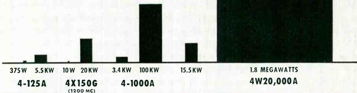
EXAMPLE OF HIGH POWER OUTPUT CAPABILITIES OF EIMAC TUBES
