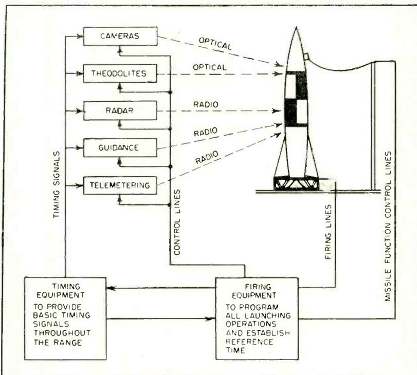
FIG. 1—Relationship of guided-missile firing system to other range instrumentation
