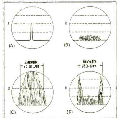
FIG. 2—Unmodulated carrier (A) is frequency modulated (B) with attenuator in. Bandwidth is read (C) with attenuator out. Deviation-limited transmitter has similar bandwidth (D)
