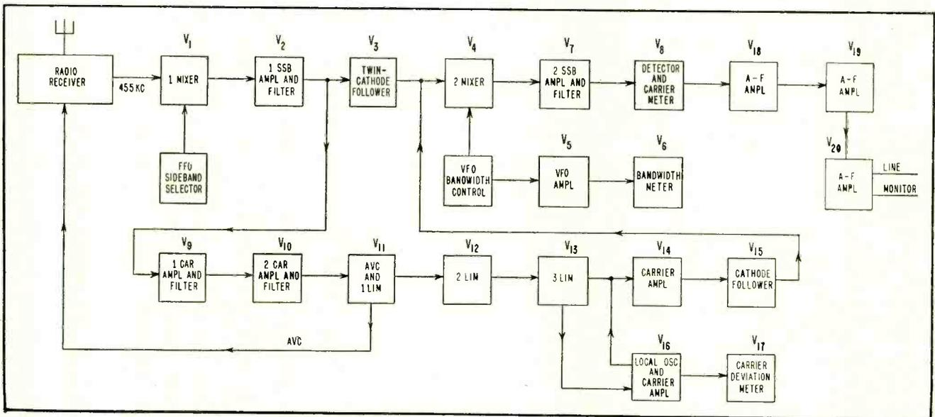
FIG. 3—Block diagram shows signal splitter for which schematic is given in Fig. 4
