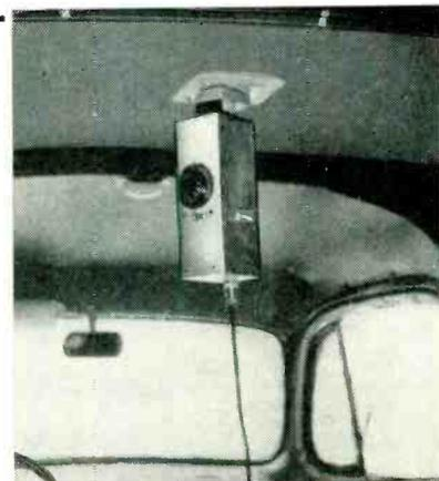
Method of mounting amplifier under roof of car
