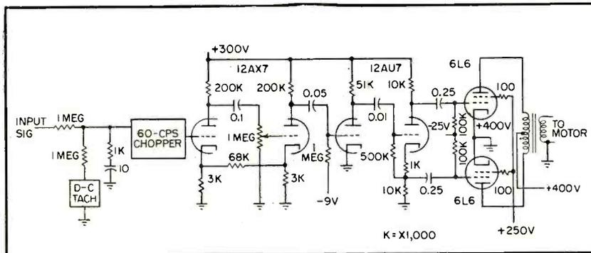
FIG. 7—Schematic of wavelength servo amplifier
