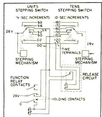
FIG. 3—Simplified schematic of stepping circuit
