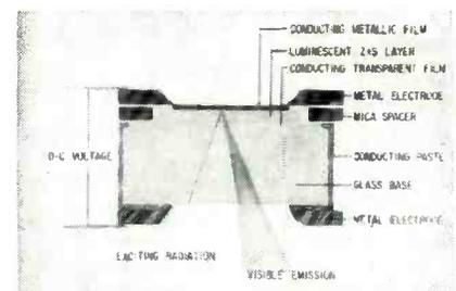
Special phosphor cell used to effect amplification of light. Ultraviolet photons from a slide projector hit the cell, which reflects visible light. Application of d-c increases intensity
