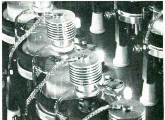
it delivers 300kw of power output in pulse modulator service with only one kilowatt of pulse driving power. From the 100T power triode, used in the first Navy sea radar tests, to the 4W20,000A, Eimac pulse-rated tubes have filled key sockets in sea, land and air pulse operation.
