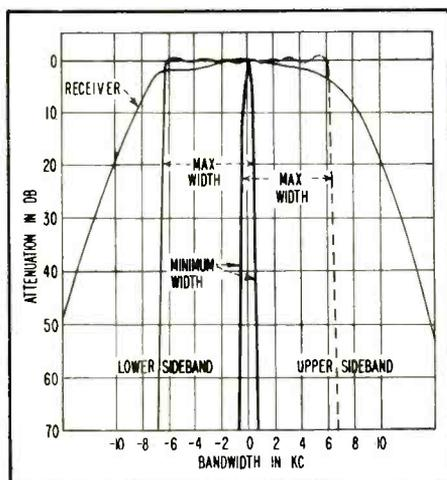
FIG. 1—Single-sideband selectivity versus selectivity of associated receiver
