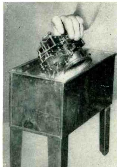
Cleaning clock movement in ultrasonic bath having two Mullard transducers fed by r-f generator
