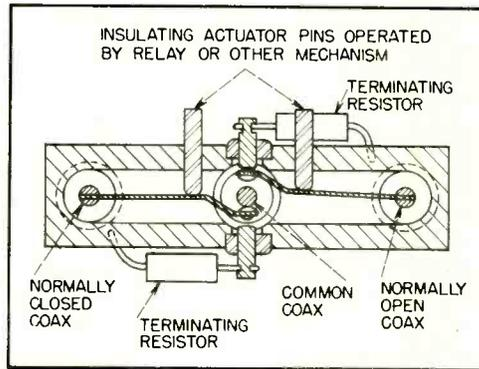
FIG. 2—Actuator pins transfer spring arms between center conductor of common coax and pin grounded through terminating resistor
