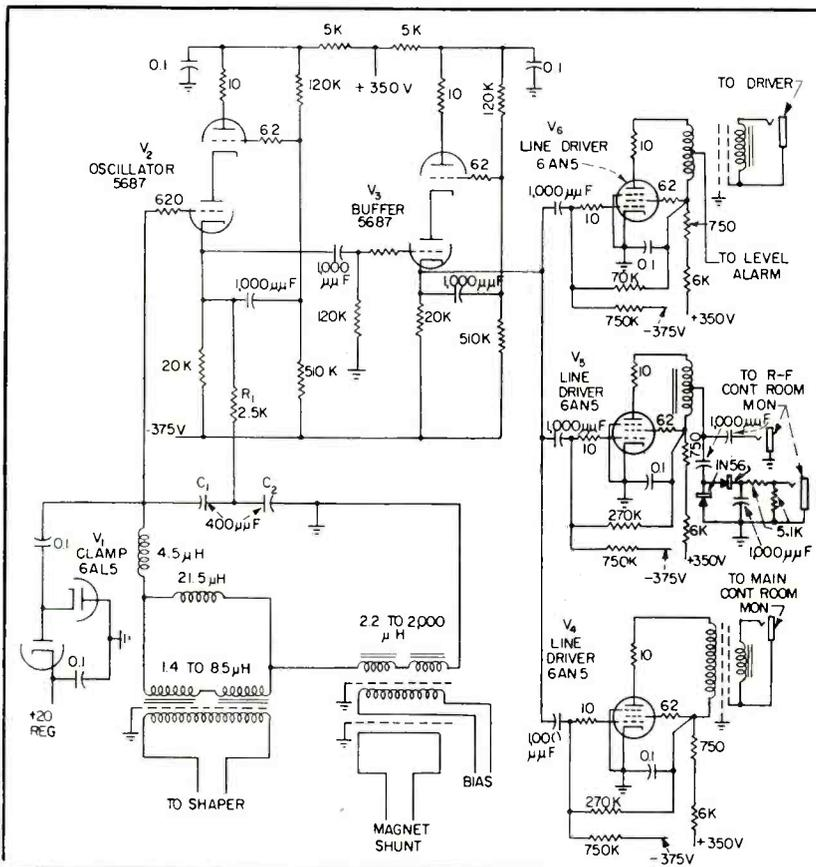
FIG. 5—Simplified schematic of primary frequency generator
