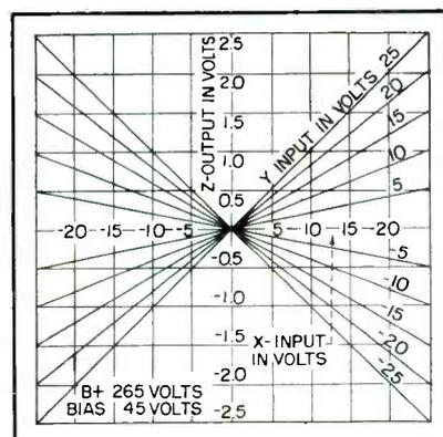
FIG. 4—Plot of multiplier characteristics, Z-KXY, using square-law tubes
