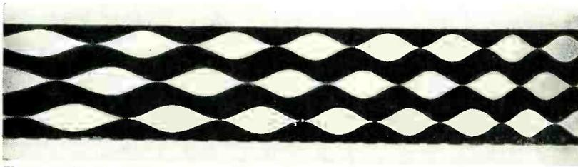
Three tracks of varying area on 35-mm film provide memory for chart drive
