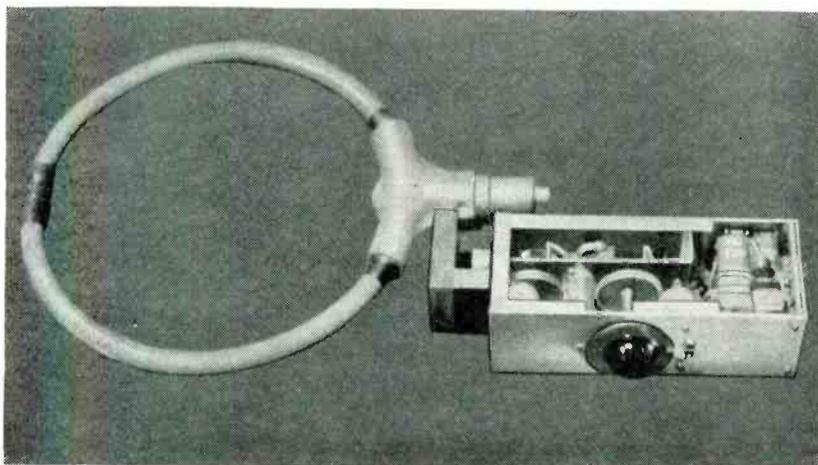
Antenna and amplifier assembly; amplifier unit is mounted against roof of truck and antenna is screwed into place through a 160-mc mobile antenna mounting hole
