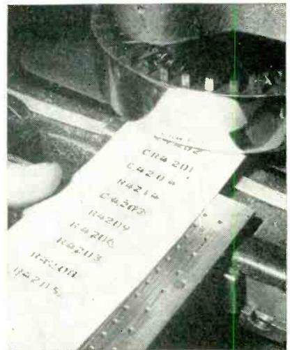
Closeup of punching head, showing finished stencil for resistor board. Paper backing tape feeds automatically from right to left. Tape supply reel is off at right. Stencil can be fed either in or out
