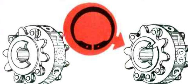
**Old Way.** One-piece assembly was spun together. Spinning operation was costly, resulted in high scrap loss.
