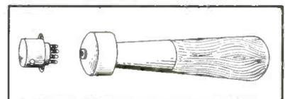
Terminal-spreading tool for miniature sockets. Two sizes are needed, for 7-pin and for 9-pin sockets respectively
