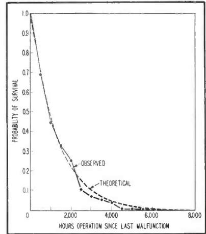
FIG. 2—Theoretical curve fitted to observed reliability of ground equipments
