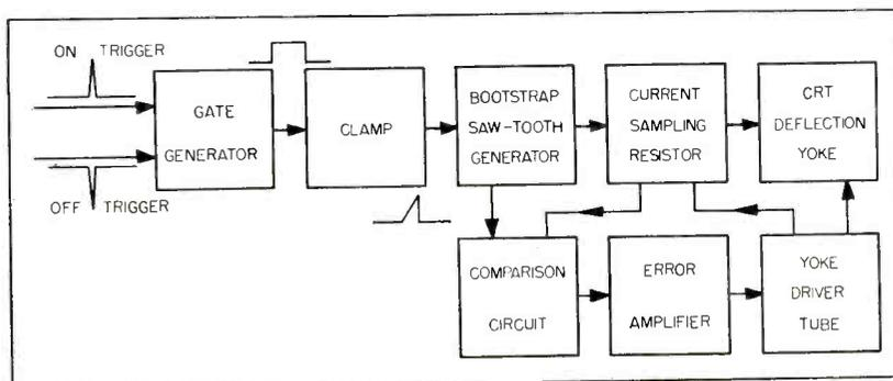
FIG. 1—Commonly used electron-tube system for CRT beam deflection
