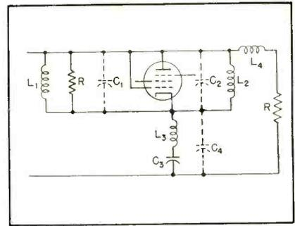
FIG. 3—All-pass amplifier stage, showing stray capacitance to ground with inductance  $L_1$  inserted in output
