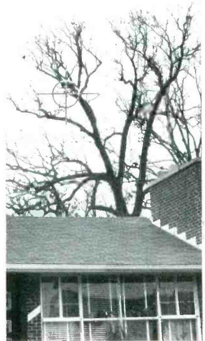
Sighting through surveyor's transit toward transmitting antenna showed tree branch acting as reflector of tv signal
