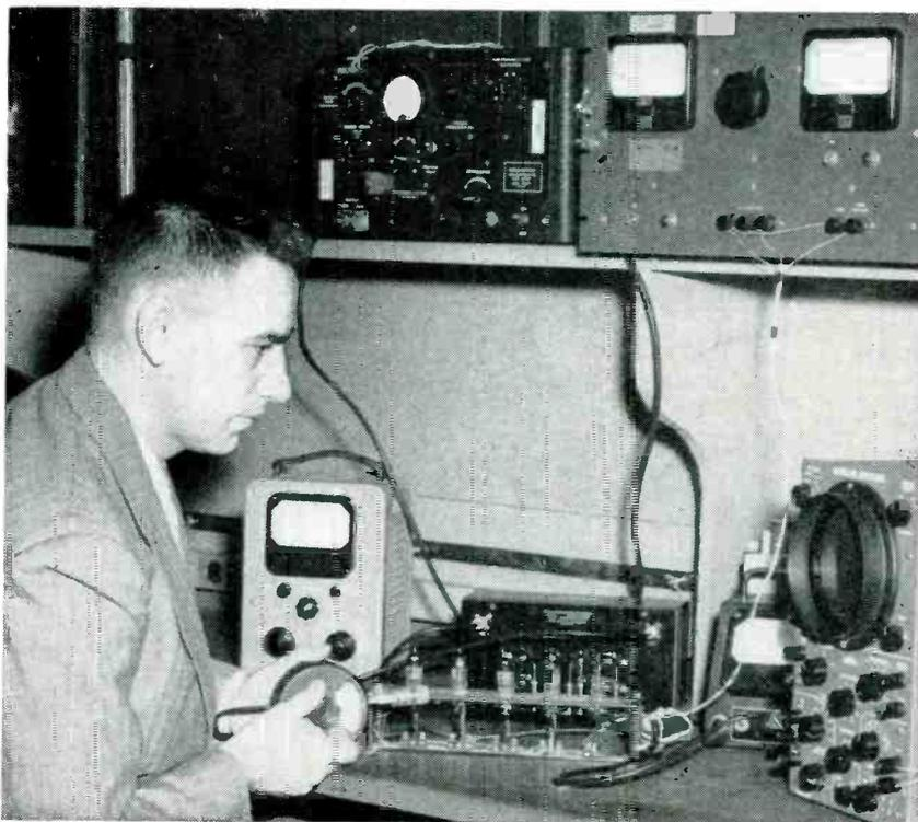
Experimental five-stage 10 to 70-mc all-pass amplifier test setup. Amplifier is shown immediately to right of author's hands
