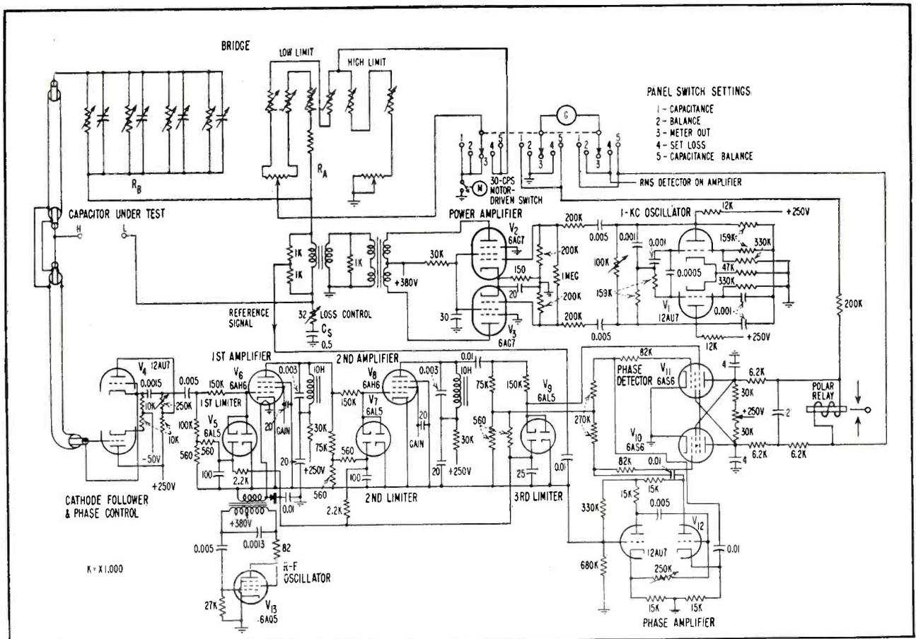
FIG. 2—Circuit of 1-kc limit bridge. Capacitor under test goes into bridge network at upper left. Polar relay controls sorting
