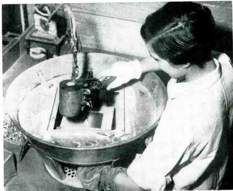
Spraying counterelectrode on 6-inch-square selenium rectifier cell. Mushroom plug covers center hole to mask its edges. Operator wears glove on left hand to keep plates clean and protect hand. Flexible air line and line cord for heater in pot are taped to steel supporting cable
