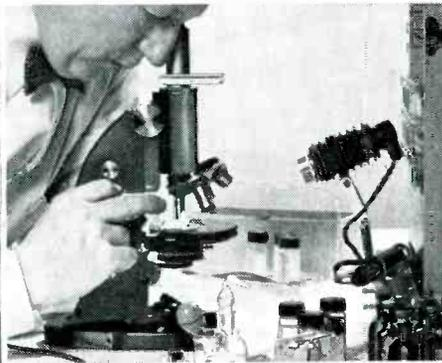
A microscopic look at disc often provides lead to nature of trouble. Unlike actual contact, print can be examined with transmitted light and high magnification.
