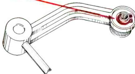
Use of one Waldes Truarc Ring (Series 5100) eliminates time-consuming riveting over the flange, retains and holds the connecting knob captive. A compact, neat design is made possible, rejects caused by poor riveting eliminated.
