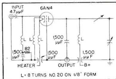
**FIG. 1**—Circuit of the 6AN4 amplifier stage used to drive power amplifier. Several stages are cascaded to improve bandwidth
