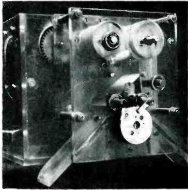
Disks are measured as they drop down between roller-type contacts driven by motor at speed just slow enough to give time for setting sorting gates below
