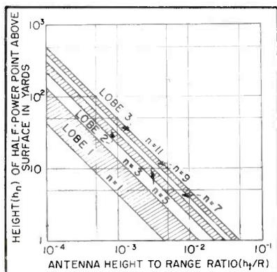
FIG. 2—Half-power width and lobe height for antenna mounted above perfectly reflecting plane surface
