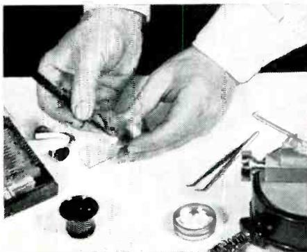
Preparing disc for microscopic examination. On-the-spot examination may reveal acid, alkali, sulfur, soot or other polluting agents peculiar to an area.
