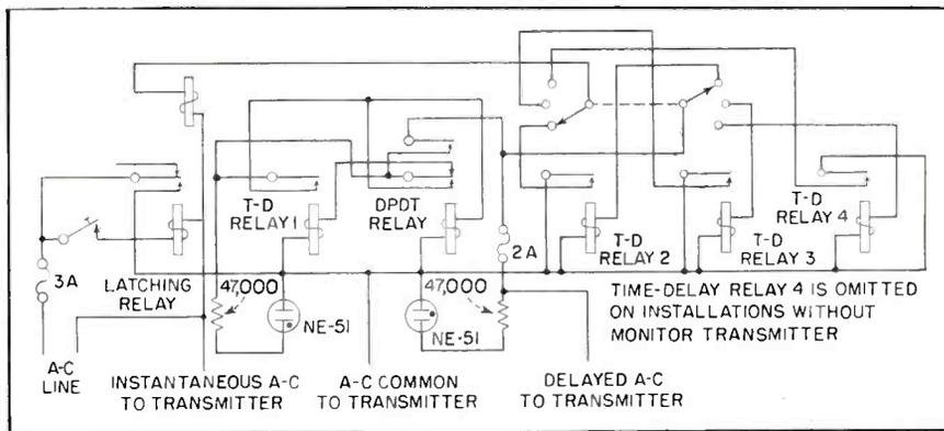
FIG. 3—Wiring diagram of transmitter control unit. Time-delay relays provide warmup period for transmitter and determine transmission periods. Unit has two controls, one to select desired operation and other to turn equipment on
