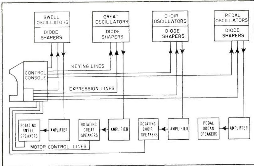
FIG. 1—Three keyboard organs and one pedal organ are controlled from console. Keying lines select one oscillator and expression lines determine waveshaping
