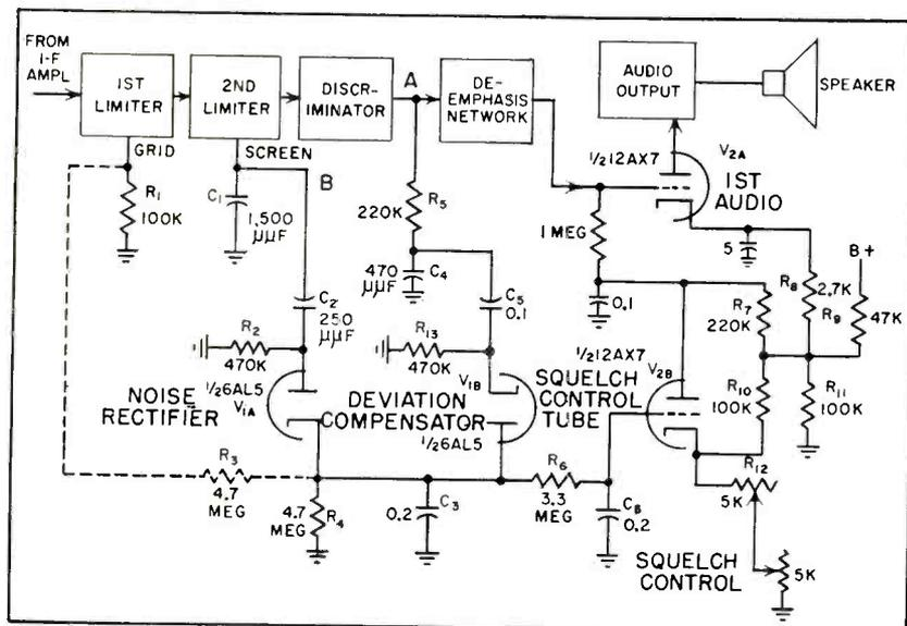
FIG. 2—Deviation-compensated squelch circuit uses audio output from discriminator to prevent muting during wide excursions of signal
