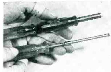
Nut starters for work at close quarters. Upper starter is hex wrench with threaded core to hold nut during starting. Lower starter, having threaded stud inserted in coil spring, is shown with nut in position
