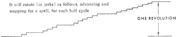
Note that each full cycle produces 2 jerks, and that 10 full cycles produce 1 revolution.
