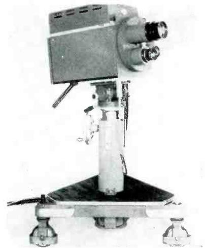
Mobile light source generates a scanning beam that is directed towards the scene to be televised
