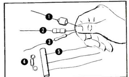
**VARIETY OF HOUSINGS** available for Vac-u-Sel rectifiers. 1) Metal-clad casing, 2) Textolite tube, 3) Ceramic tube, 4) Nylon tube, 5) Slotted Textolite tube.
