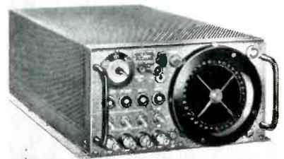
Compact indicator suitable for small airports tunes vhf aircraft radio bands and furnishes bearings even when voice signals are unintelligible. Built by Olympic Radio and Television, Inc., it was described in technical article on p 184 of June 1955 issue of this magazine but without company designation
