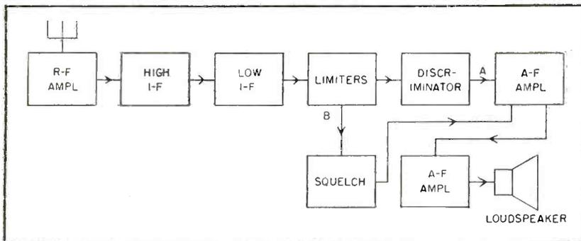
FIG. 1—Conventional squelch operation uses output from limiter circuit to bias off audio in the absence of signal
