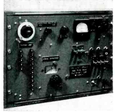
Front panel of 1-mc bridge used for checking low-value disk capacitors. Here only one set of tolerance buttons is used, for 0 to 49 percent
