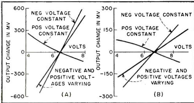
FIG. 4—Change in output of amplifier of Fig. 3 with variation of supply voltages for 68-db (A) and 78-db (B) feedback
