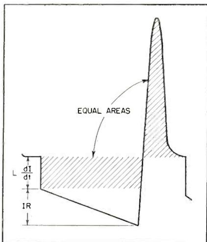
FIG. 3—Voltage waveform required by yoke and feedback resistances
