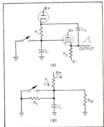
FIG. 2—Bootstrap circuit: schematic (A), equivalent circuit (B)
