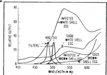
FIG. 1—Spectral response curves of good and infected eggs, with response curves of filters used on phototubes
