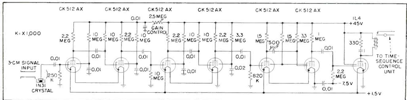
FIG. 5—Receiving unit uses CK512AX subminiature hearing-aid-type tubes to reduce battery current drain
