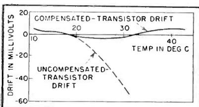
FIG. 6—Amplifier drift characteristics with and without temperature compensation
