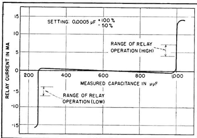
FIG. 4—Current in polar relay of 1-kc bridge when set for tolerance range of 150 percent at 0.0005  $\mu\text{f}$
