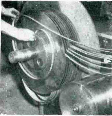
Core plate recoiler being set up for winding twelve 3/8-inch silicon-steel slit strands coming from slitter
