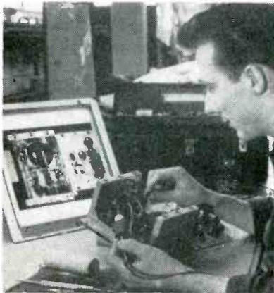
Color transparency mounted in illuminator guides assembler by showing in true color the correct position of each lead and component
