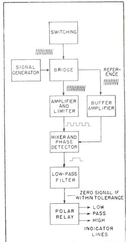
FIG. 1—Capacitor disk under test forms one leg of a-c bridge in which a different leg is automatically switched between desired tolerance limits of preset capacitance to give waveforms shown
