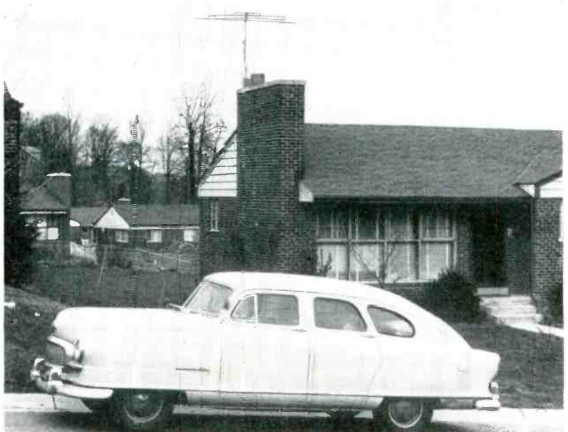
Car shown in location where reflection from car roof interfered with reception of channel 9 signals
