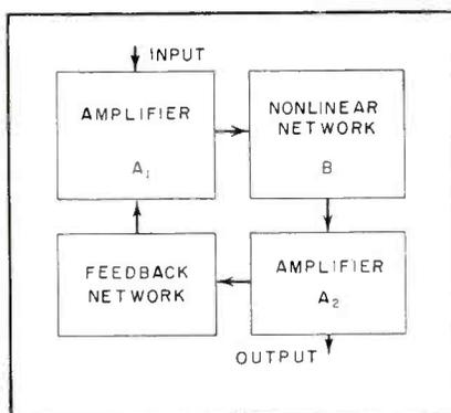
FIG. 2—Waveform generator consists of nonlinear stage and two amplifiers
