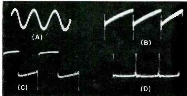
FIG. 3—Laboratory model of oscillator uses experimental *pnp* junction transistors similar to 2N45. Circuit values may have to be adjusted for transistors used. Waveforms A, B and C were obtained with  $R_3 = 100, 50$  and  $10$  ohms. For D,  $R_3 = 10$  ohms and  $R_2 = 600$  ohms
