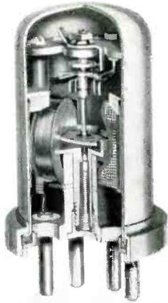
So sensitive — so sure in action is the new EDISON 219 Sensitive Control Relay that it actually eliminates the need for a vacuum tube amplifier. Because of low operating power level, the Model 219 can operate *directly* from a thermocouple or photocell output. And this extreme sensitivity is matched with compact design and relative lightness in weight.
