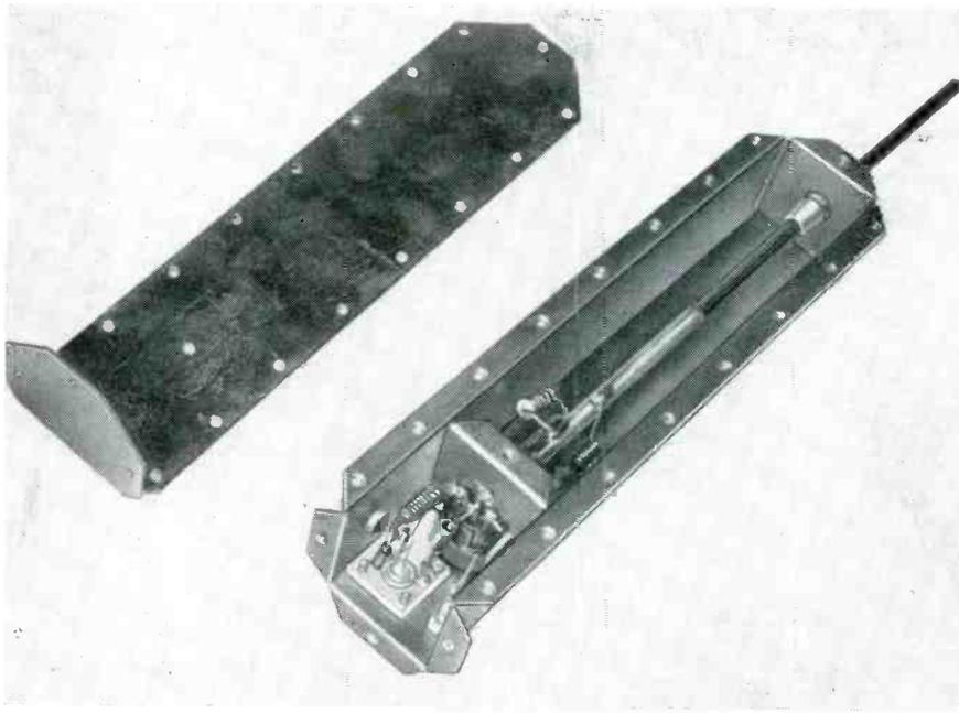
Voltage amplifier stage uses simple design that provides good shielding
