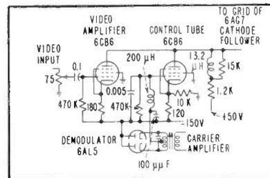
FIG. 5—Demodulator and control tube circuit
