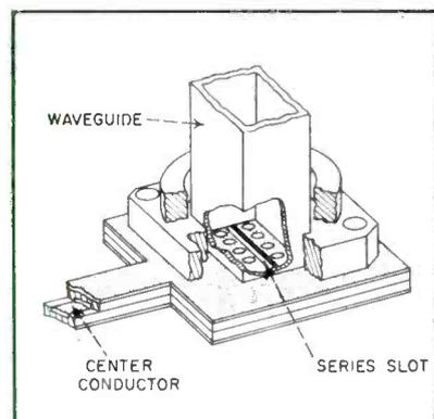
FIG. 3—Etched plate-to-waveguide transition using series slot as a transformer
