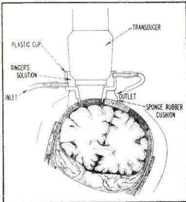
Method of transmitting ultrasound to the brain after removal of bone button over each prefrontal area
