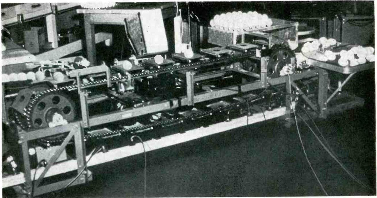
Egg candler detects infected eggs by measuring internal fluorescence with two phototubes in housing at center. Housing is lowered over egg to produce light-tight seal during measurement
