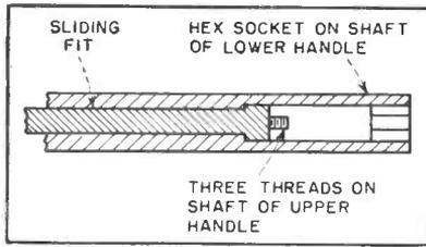
FIG. 1—Cross-section of two-handle starter for nuts
