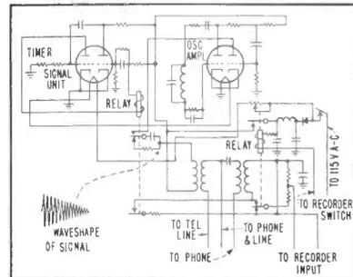
FIG. 1—Beep tone unit for attachment to tapped telephones
