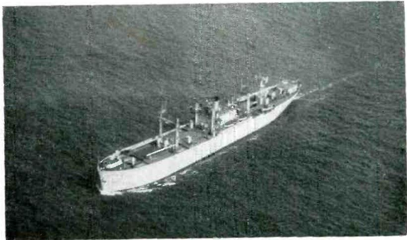
Latest addition to northern hemisphere defense is the radar picket ship that can pick up signals reflected from aircraft far off the shores of the continent. First ship to be commissioned for this service is the USS Guardian, YAGR-1, shown at left. First official photographs of the vessel indicate no details of the extensive radar and electronics installations in this floating laboratory
