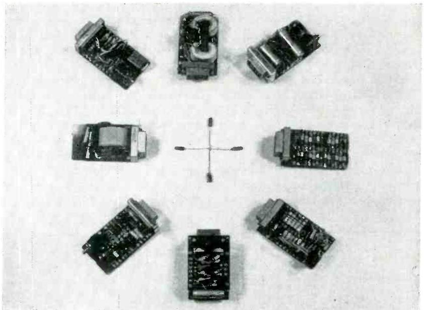
Complete transistor units compared with transistor types used. Reading clockwise from bottom: high-gain tape-recorder amplifier; low-gain d-c amplifier; power-supply unit; voltage discriminator; magnetic modulator; high-gain d-c amplifier; voltage-controlled attenuator; audio amplifier
