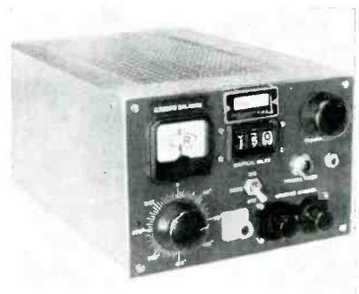
Production of a civilian version of military tactical air navigation transmitter-receiver is scheduled to start in October if the system is finally adopted for civil airways. The mechanical mockup shown above was built by Federal Telecommunication Labs., in Nutley, N. J. Tacan provides both distance and bearing information from appropriate beacons located on the ground (or on an aircraft carrier)
