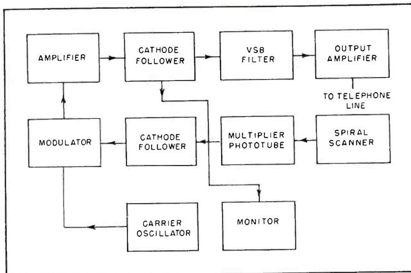
FIG. 1—Elements of the continuous-feed facsimile scanner-transmitter
