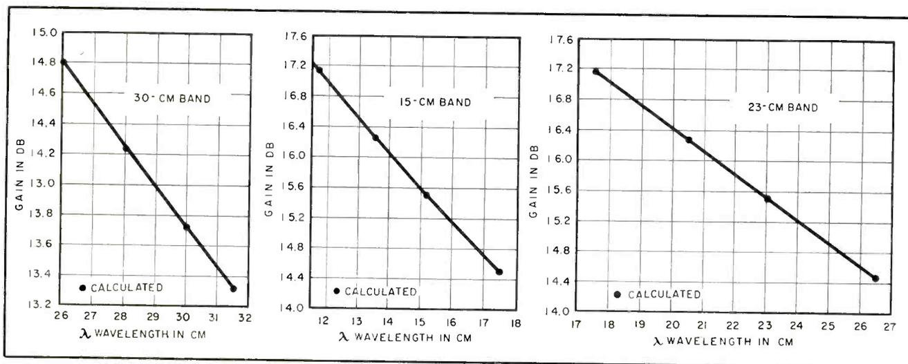
FIG. 6—Gain curves for gain-standard horns in the 15-cm, 23-cm and 30-cm bands
