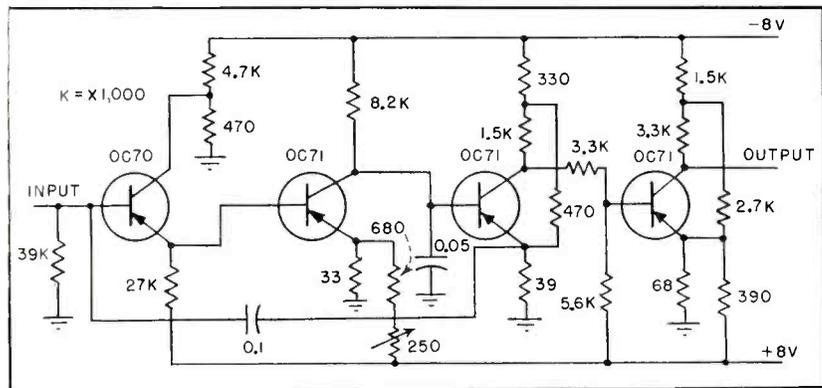
FIG. 3—Direct-coupled amplifier has gain of 25,000 with maximum output voltage of 5 volts into 1,500 ohms
