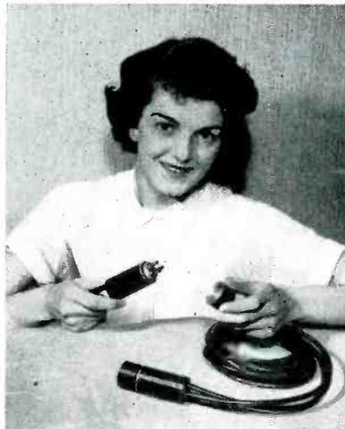
Transistorized RCA adapter makes possible substitution of different microphones and headset types
