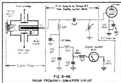
Schematic of a ship radar frequency-conversion circuit illustrated in "License Manual for Radio Operators"
