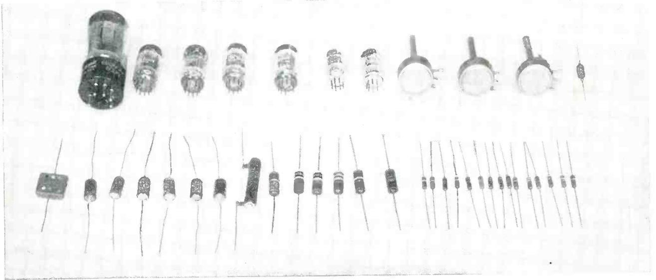
the 40 components of an electron-tube crt deflection system . . . . .
