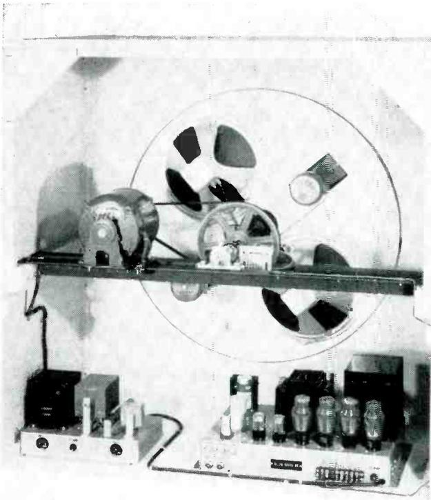
Loudspeakers are mounted on motor-driven baffle plate to produce pitch-fringing effect for realistic imitation of pipe organ
