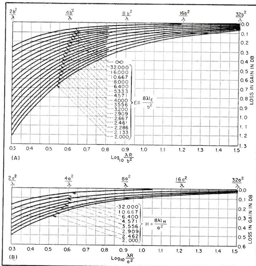
FIG. 7—Braun's E- and H-plane correction curves
