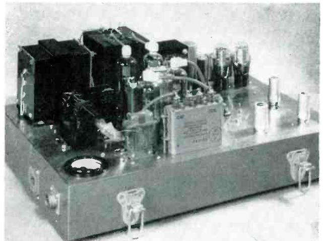
FIG. 4—Microwave transmitter and modulator. Magnetron output tube is mounted on left side of chassis
