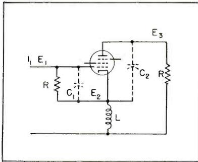
FIG. 1—All-pass amplifier stage is equivalent to conventional amplifier stage and high-pass filter
