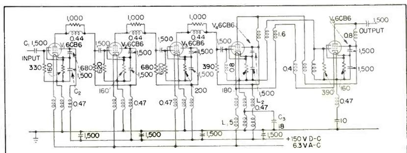
FIG. 4—Five-stage 10 to 70-mc amplifier. Heater and plate voltages are supplied to the tubes through trifilar coils. Capacitances are in  $\mu\mu\text{F}$  and inductances in  $\mu\text{H}$
