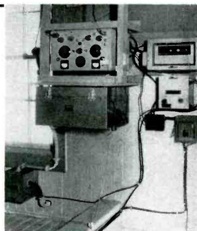
Interior installation at Barrett Rock control point. Antenna changeover switch is at upper right; radiotelephone receiver, with microwave transmitter mounted above, is at center. Antenna selector and transmitter controls are at left side of photograph
