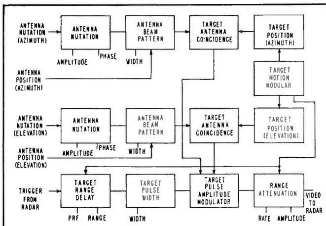
FIG. 2—Test arrangement for a tracking radar. Antenna information is derived from simulator modulars
