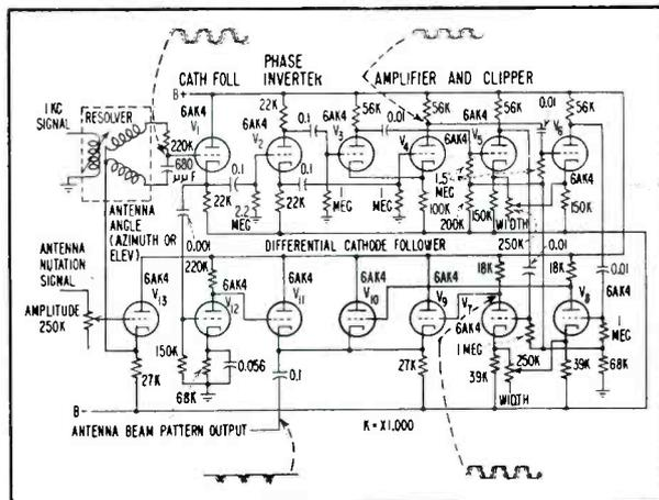
FIG. 3—Echo-pulse simulator uses differential cathode follower output to select most positive of three signals
