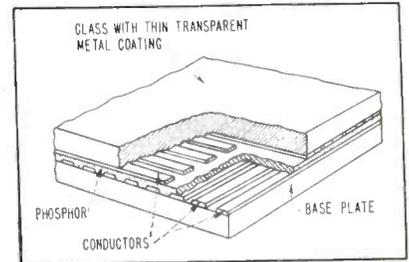
FIG. 2—Construction of phosphor screen
