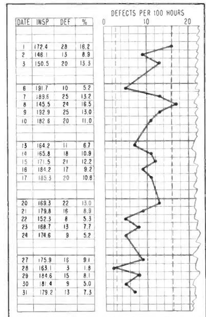
FIG. 1—Example of one-month quality control chart for printed wiring boards
