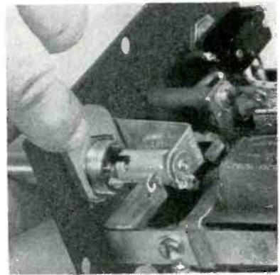
Using filed-down open-end wrench to hold mounting nut behind panel
