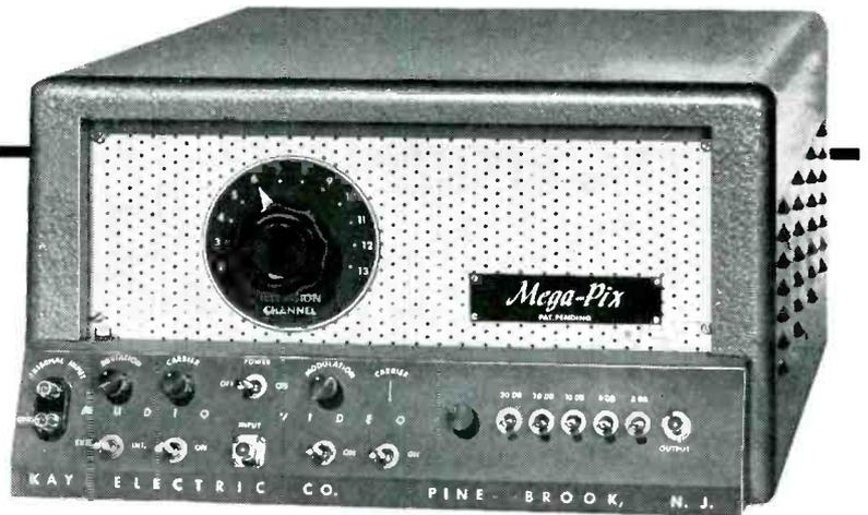
The Kay Mega-Pix provides two separate twelve-channel crystal controlled oscillators, frequency multipliers and output amplifiers to develop a crystal controlled RF picture and sound carrier on each TV channel.
