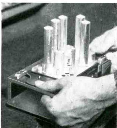
Method of pressing side levers to pry chassis out of jig
