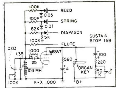
FIG. 2—Sinusoidal output of Hartley oscillator is modified by copper-oxide rectifier circuits to provide four basic tones
