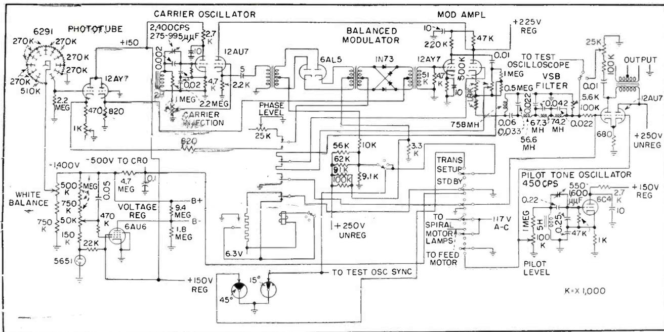
FIG. 3—Scanner amplifier used in system with common power synchronization. Additional subcarrier modulation can be added for remote locations using pilot tone oscillator like that shown to right
