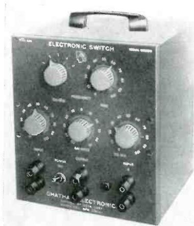
other or separated by a desired amount. Direct comparison of amplitudes, waveforms, frequencies, and phase relationships may be observed. A square-wave voltage of variable frequency and amplitude is available at the output terminals for use as a test signal in studying the transmission characteristics of v-t amplifiers and other circuits.
