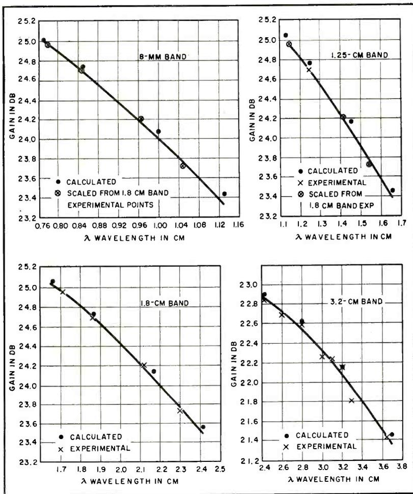
FIG. 4—Gain curves for gain-standard horns in the 8-mm, 1.25-cm, 1.8-cm and 3.2-cm bands. Comparisons of measured gain for horns scaled from one band to another show good agreement
