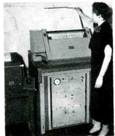
Alden weather map recorder at Logan Airport, East Boston, Mass., produces weather record from continuous roll of paper, making it possible to read copy as it is received.
