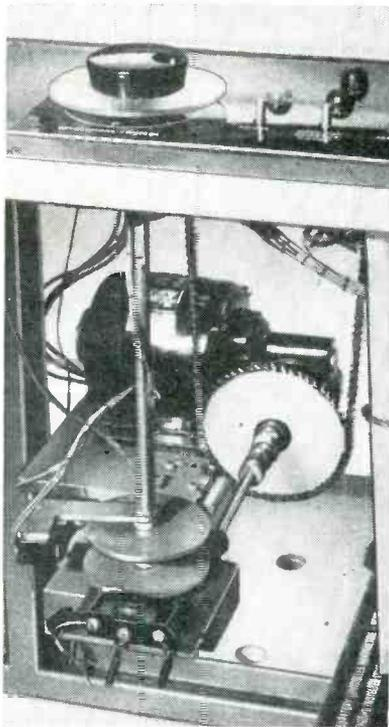
Two cams at bottom control revolutions per cycle. Switch for lower cam is fixed, but switch for upper cam can be rotated around cam by knob on control panel at top
