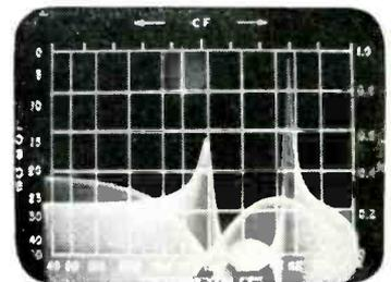
Response of an audio band stop filter with null marker showing frequency of one peak.
