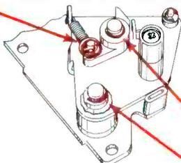
Three types of Waldes Truarc Retaining Rings are used in this assembly. One circular self-locking ring (Series 5105) retains pawl return spring. One external E-ring (Series 5133) retains roller used to prevent gear motion during transport cycle. One crescent ring (Series 5103) retains pawl which indexes gear. Second crescent ring retains sub-assembly. Truarc Rings speed assembly, cut rejects, eliminate parts.
