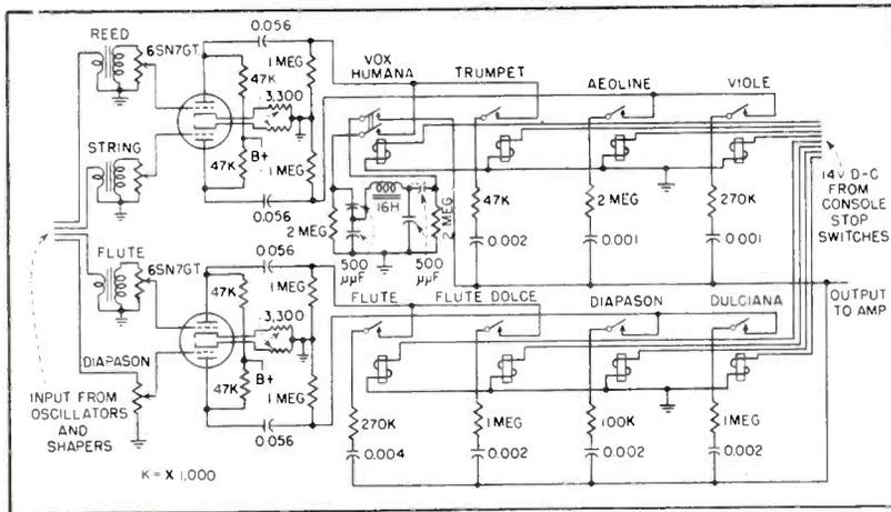
FIG. 3—Four basic tones from oscillator section are further subdivided in tone-modifier section to provide equivalent of eight sections of pipes
