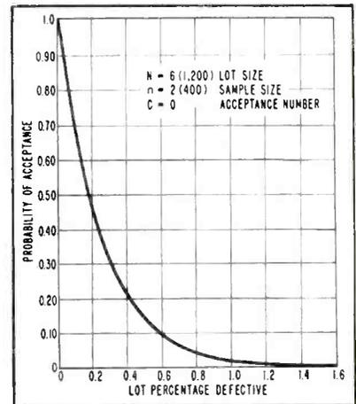
FIG. 2—Operating characteristic curve for typical small-lot production of printed wiring boards
