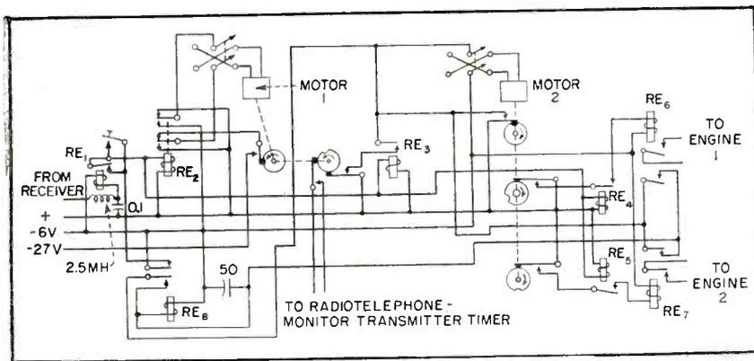
FIG. 6—Time-sequence unit has timing cams driven by reversible motors
