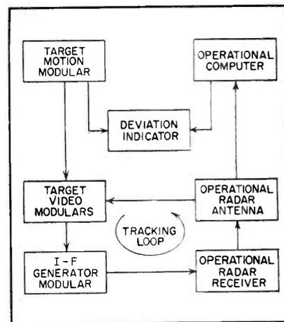
FIG. 1—Typical arrangement for testing radar system
