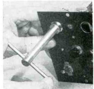
Using ferrule wrench to tighten ferrule of socket
