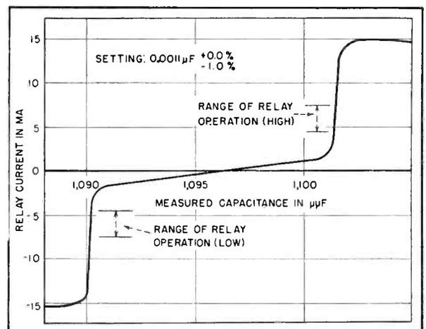
FIG. 5—Current in polar relay of 1-kc bridge when set for tolerance range of 1 percent at 0.0011  $\mu\text{f}$
