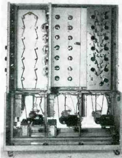
Three stages of undress in life tester. At right are units mounted on door. Center door is swung open to show clutches. At left, both door and inner panel are swung open to show chain drive for bay
