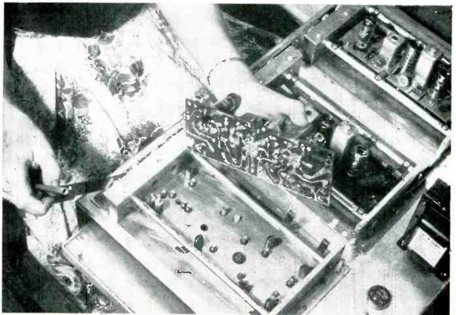
Placing board on empty position while tubes are warming up preparatory to alignment at other two positions
