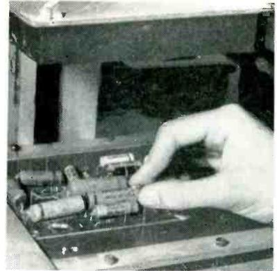
Setup using overhead pressure pad having its own air cylinder
