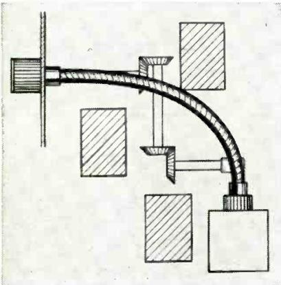
One flexible shaft is all it takes to do a job that might otherwise require an entire system of bevel gears, straight shafts, universals, etc. Added to this is the fact that installation is greatly simplified and alignment problems are eliminated.
