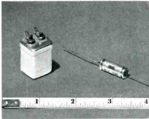
**125 C TANTALUM\* CAPACITORS**—for high speed aircraft and missile systems where quality, long life, and small size are main requirements. In plain or etched foil, and rectangular or tubular designs. Ratings: .25 to 180 uf, 10 to 100 volts. Tolerance:  $+20\%$  (plain foil),  $-15$  to  $+75\%$  (etched). Temp. range:  $-55^{\circ}\text{C}$  to  $+125^{\circ}\text{C}$ . Write for GEA-6258. \*Reg. trade-mark of General Electric Co.
