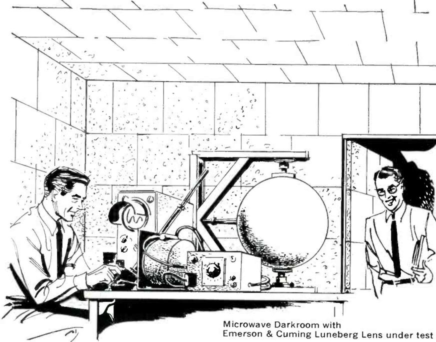
Microwave Darkroom with Emerson & Cuming Luneberg Lens under test
