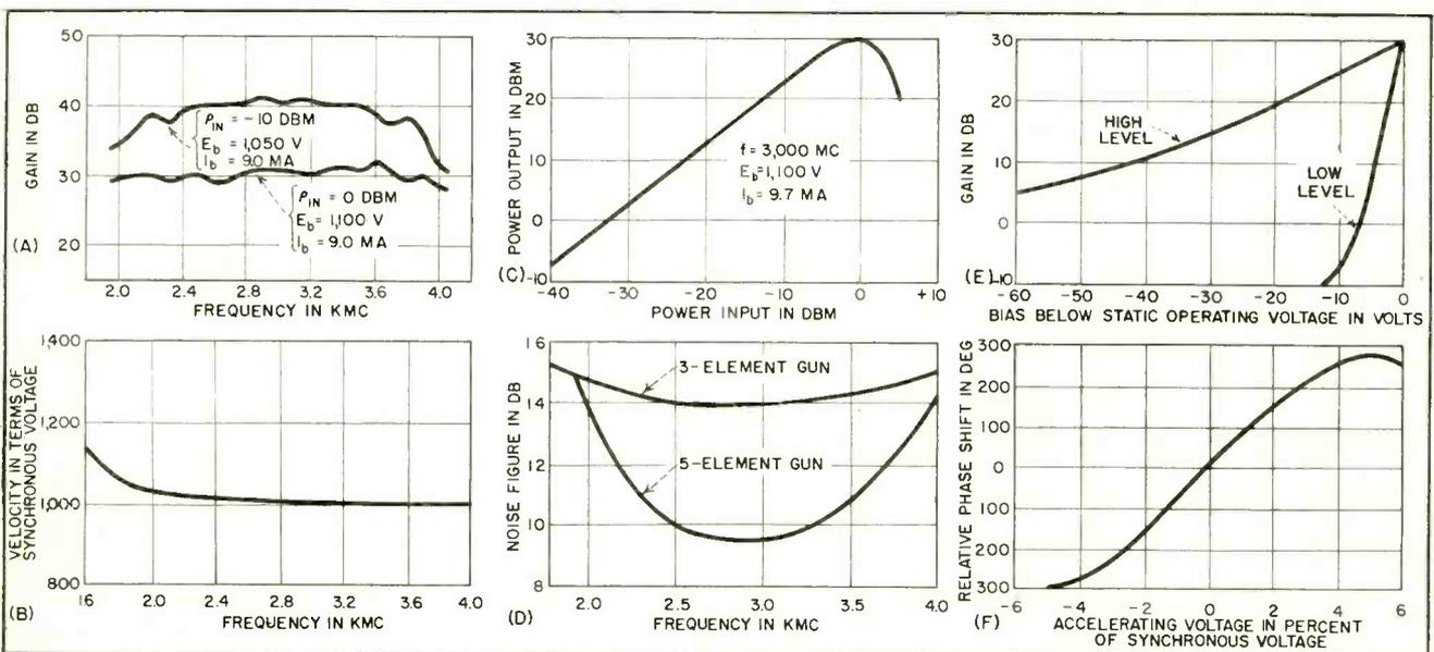
FIG. 1—Typical traveling-wave tube characteristics show value of tube in wide variety of applications described in text
