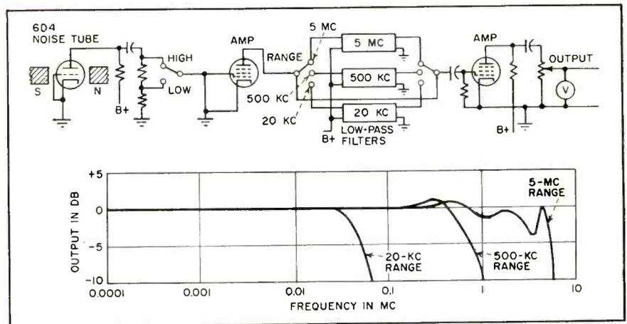
FIG. 1—Circuit (A) and spectral density (B) of noise generator using hot-cathode arc
