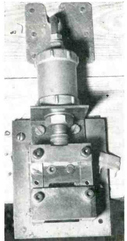
**Air-actuated lead chopper for ceramic components**
