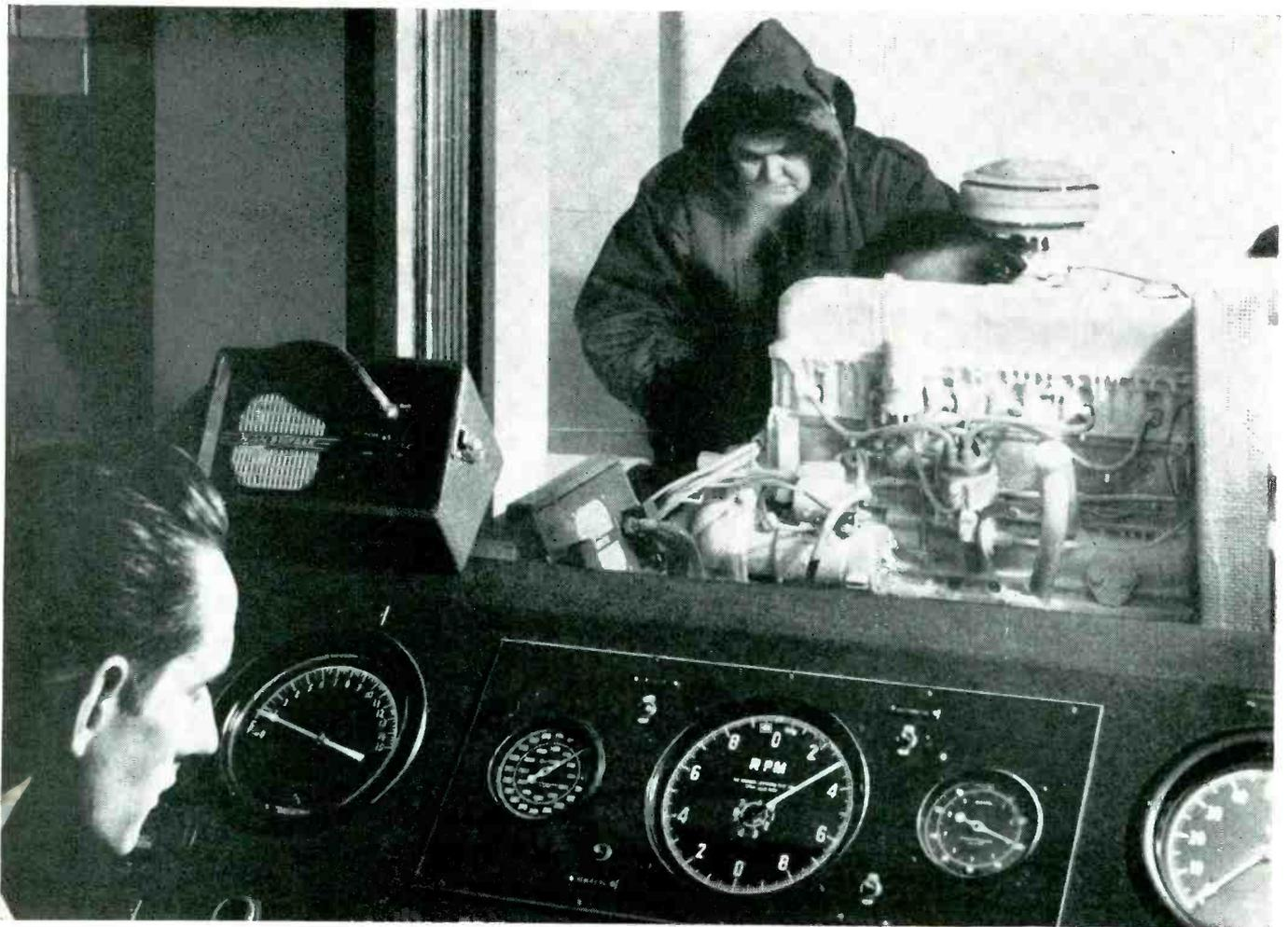
Standard Chrono-Tach shown front and center in "deep freeze" engine testing laboratory. (Courtesy of Thompson Products, Inc.)
