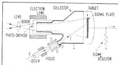
Cross-section of image iconoscope showing deflection coils *D* and scanning beam *E*. In the new tube, the insulated mica target plate is replaced by a conducting glass plate
