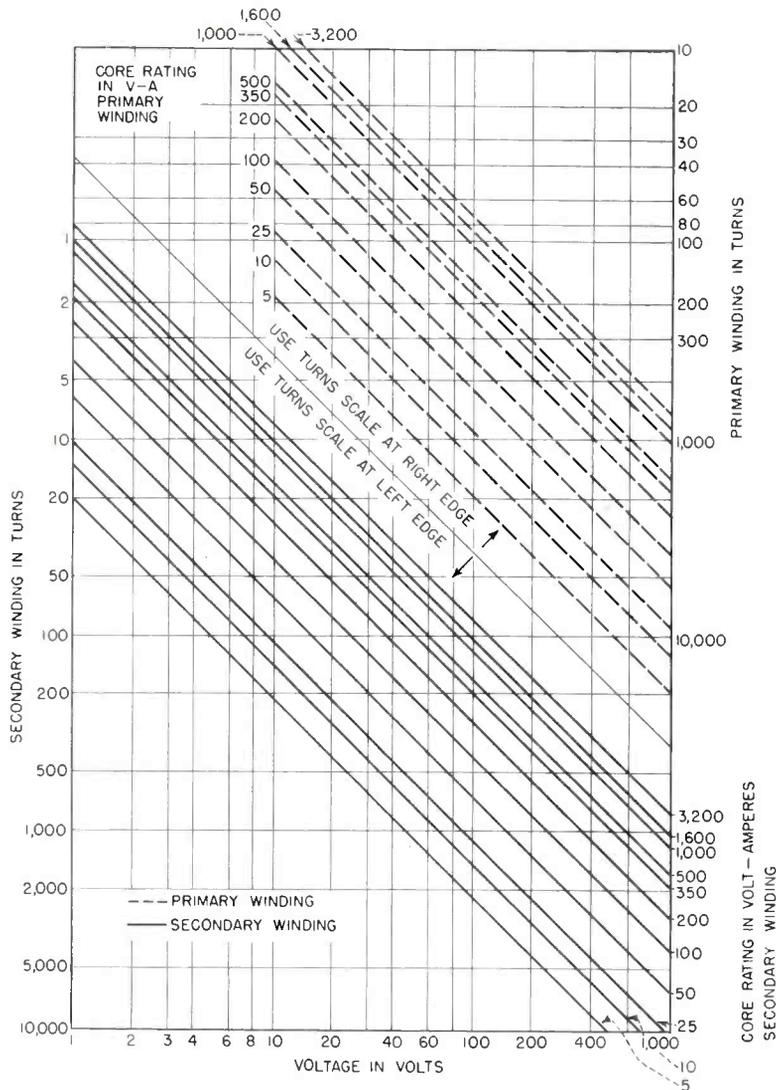
FIG. 1—Primary and secondary winding turns as determined from core volt-ampere rating
