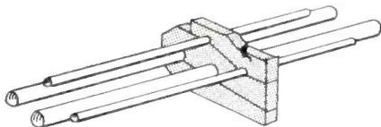
**Fuel line clamp** for a fighter airplane's "pipe-line" system is machined from Taylor fabric base laminate which has high mechanical strength and resists extreme temperature and humidity.
