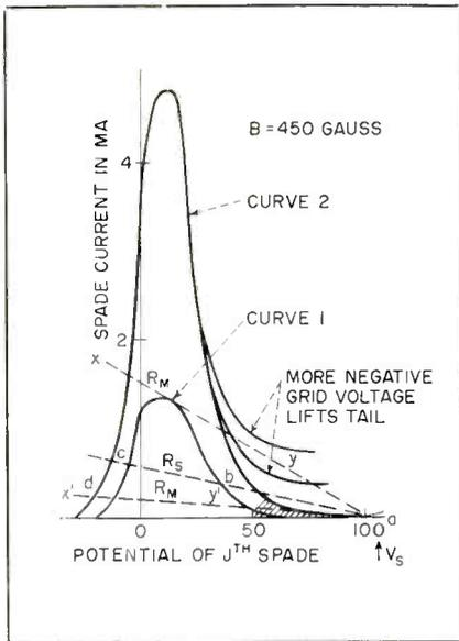
FIG. 2—Spade characteristic curves
