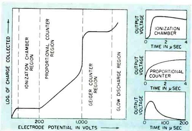
**FIG. 10—Operating regions of various nuclear radiation detection instruments and shapes of output-voltage pulses. Waveshapes shown are for infinite input time constants**
