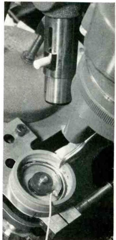
Closeup of welding operation, showing light source mounted at rear of stereo microscope
