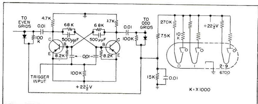
FIG. 13—Transistor driver used with low-voltage version of beam switching tube. One switching tube can do all the functions of approximately twenty transistors
