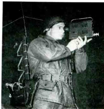
The hand-held television camera shown weighs only 8 pounds. Transmitter, complete with power supply that will transmit pictures continuously for two hours, weighs 47 pounds. Developed by Signal Corps Engineering Laboratories, the new equipment has a range of about a mile. It could be set up to report, unmanned, from a radioactive or other hazardous location
