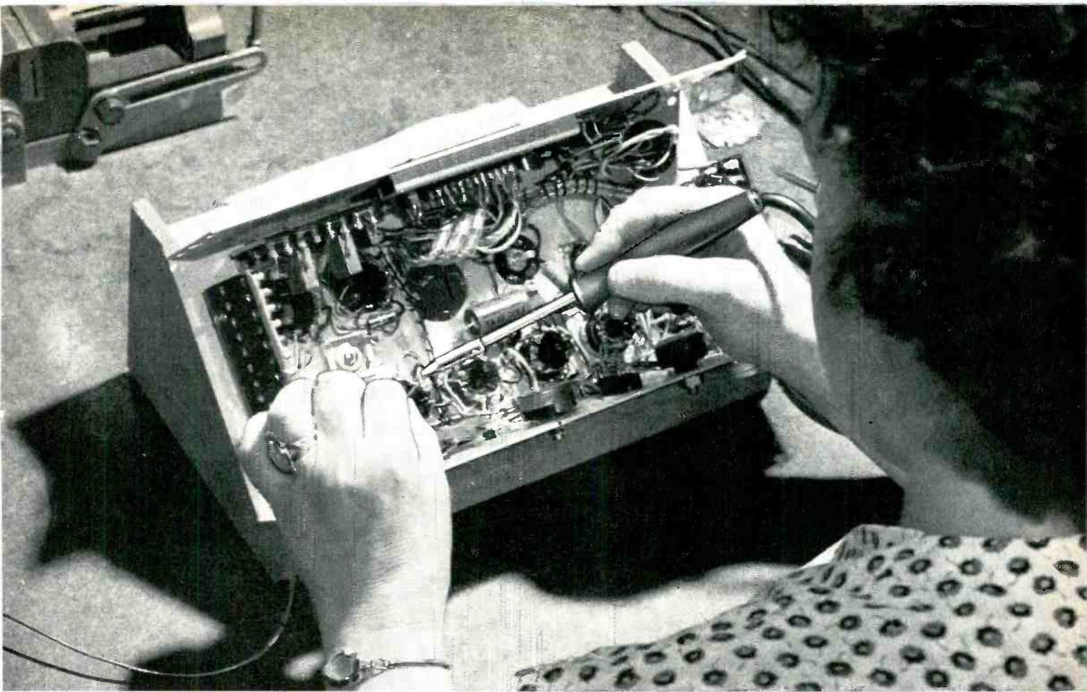
**HARD-TO-REACH JOINTS** in Sanborn Co.'s electro-cardiographs are soldered quickly with the fine-point G-E Midget iron—with no damage to adjacent parts. Weight of iron—less
