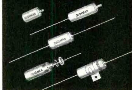
The development of the Gudeman "XC" capacitors results in a new line of high temperature capacitors that has exceptionally high insulation resistance, low power factor and low dielectric absorption. The case sizes were selected whereby no voltage derating is required when the capacitors are used within a temperature range from -65° C. to +165° C.
