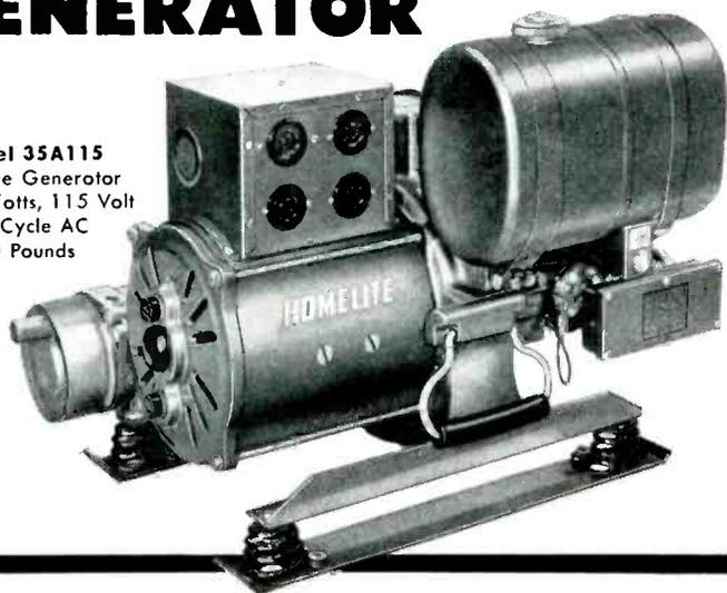
**1. New Money-Saving features**... No DC brushes; just two easy-to-get-at collector ring brushes... No commutator or DC windings... No intermediate couplings; armature keys directly to shaft. Fewer parts to wear out — longer trouble-free generator service.
