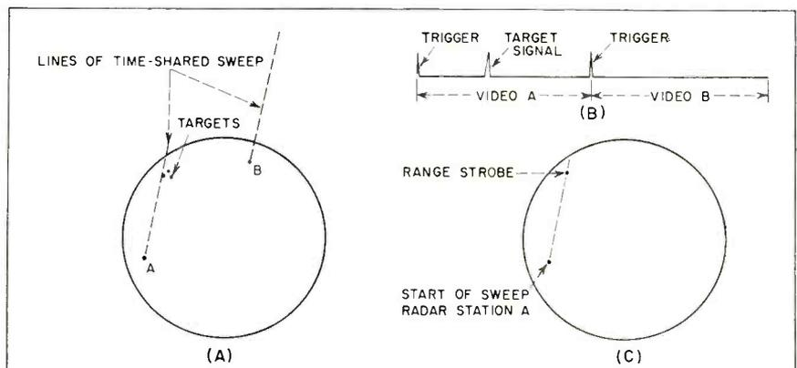
FIG. 2—Target pattern (A), video output (B) and method of writing targets on storage tube (C)
