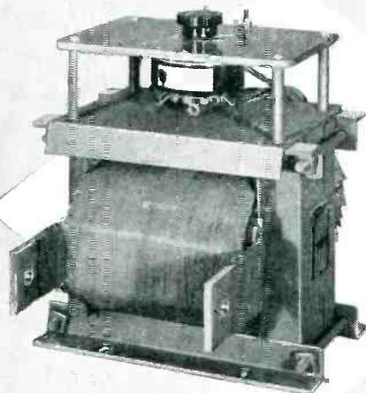
**Resistance Welding Transformer** with eight point tap-changing switch on primary winding. Used for a varying secondary current output. Unit shown is 3 KVA. Units are available from .5 to 50 KVA.
