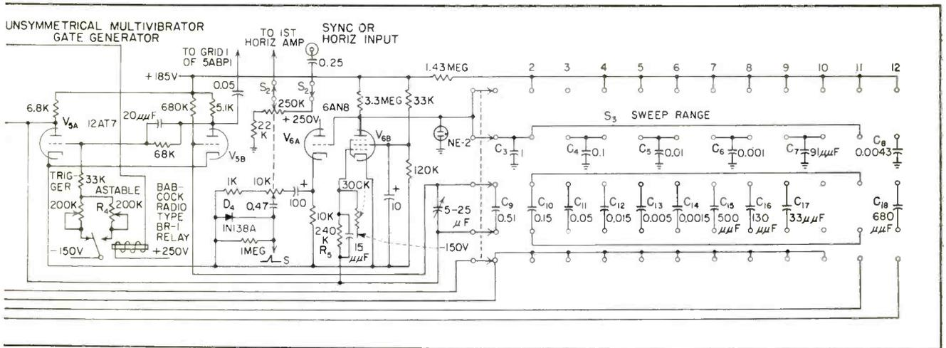
scope circuit omitted for simplicity. Recurrent sweep is provided in absence of vertical signal to avoid burning screen
