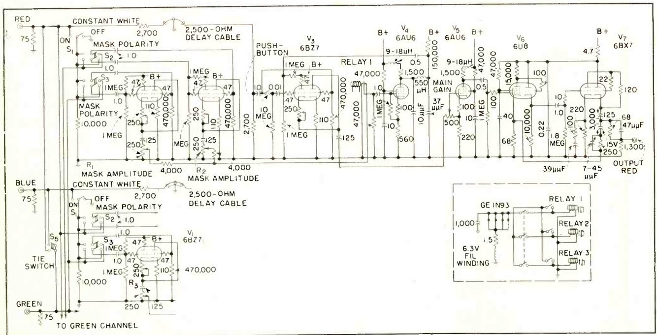
FIG. 5—Complete red-channel circuit for universal or matrix masking amplifier, with first stage of identical blue channel and input of identical green channel
