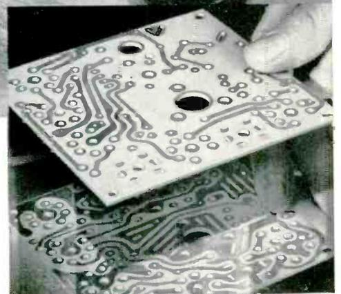
G-E "Thru-Con" Printed Circuit Boards offer positive connection through the holes, without staking pins, patterns on both sides if needed. Printed circuitry cuts assembly time, eliminates product bulk and weight, reduces inspection time and parts inventory.
