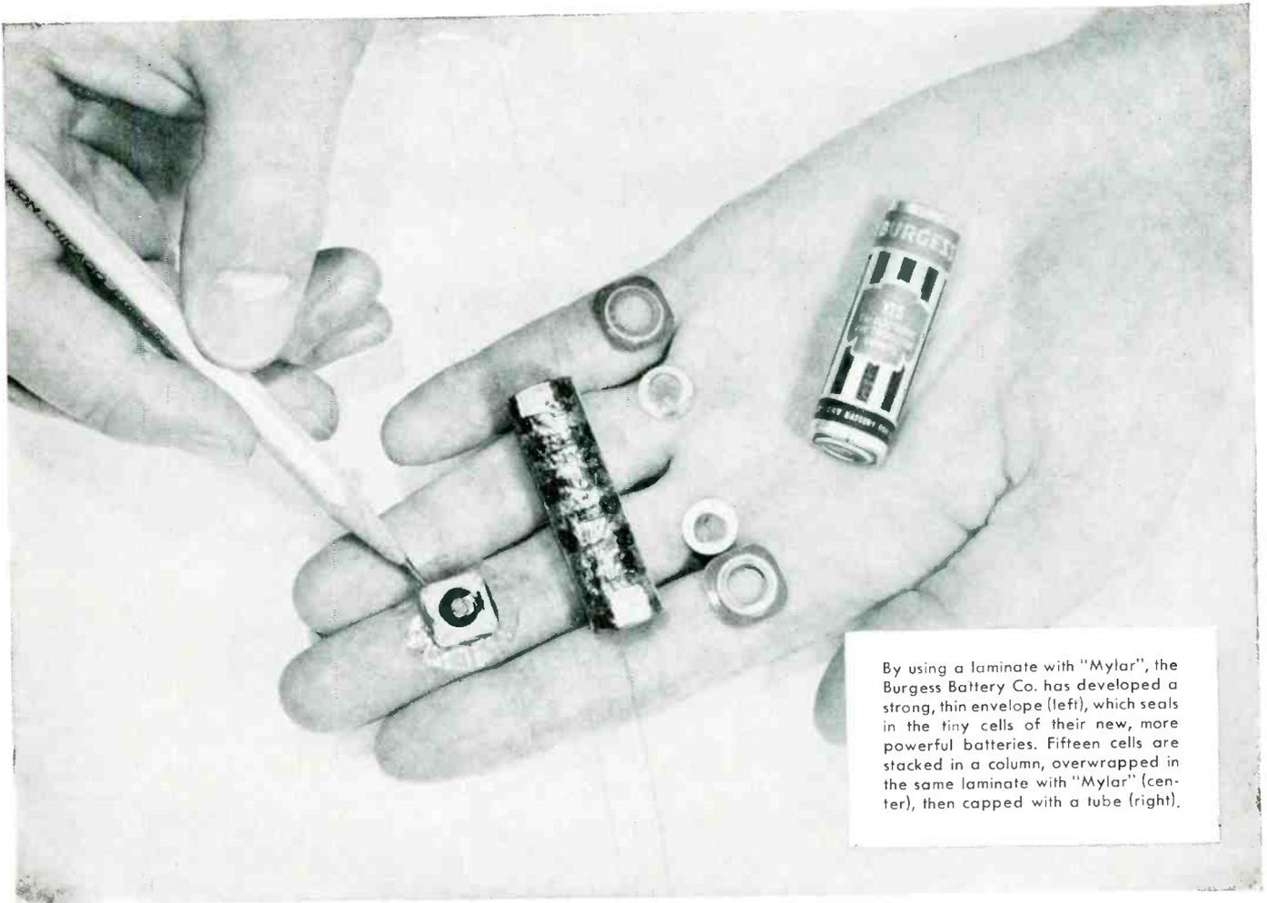
By using a laminate with "Mylar", the Burgess Battery Co. has developed a strong, thin envelope (left), which seals in the tiny cells of their new, more powerful batteries. Fifteen cells are stacked in a column, overwrapped in the same laminate with "Mylar" (center), then capped with a tube (right).
