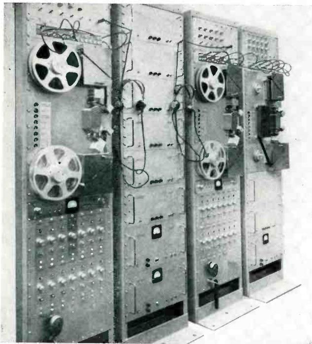
Double 14-track magnetic-tape data recorder system built by A-V Mfg. Corp. runs one machine while other is reloaded with tape. End machine reproduces loops for repetitive analysis. Tape speed is 60 ips
