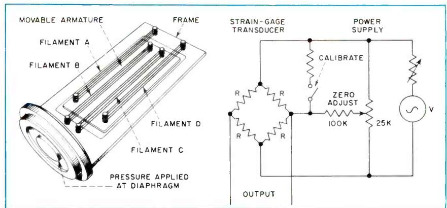
FIG. 7—Unbonded strain-gage pressure transducer has diaphragm mechanically coupled to movable armature. Pressure variations cause armature to move and change tension of wire filaments. Typical circuit is shown at right; source voltage can be a-c or d-c
