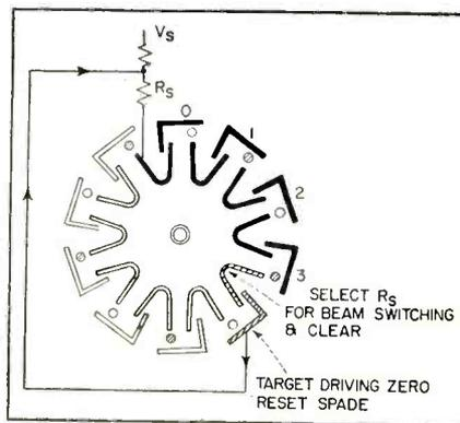
FIG. 8—Tube interconnection for four-position indication
