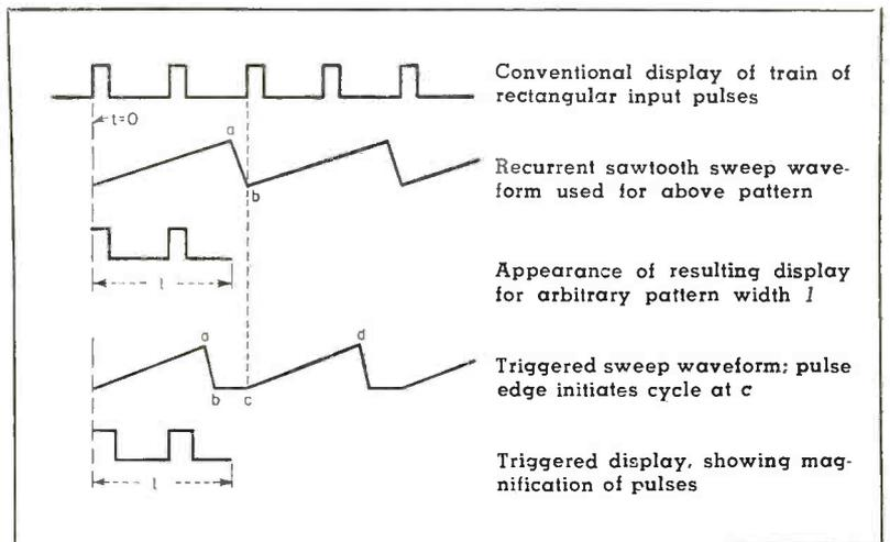
Comparison of triggered or driven sweep with synchronized free-running sweep
