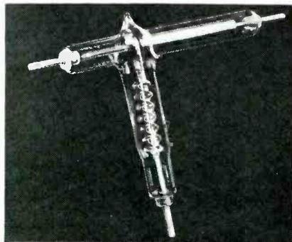
armature. High-vacuum exhaust allows it to withstand a voltage of 22,000 v across the open contacts, even though contact spacing is only 0.020 in.
