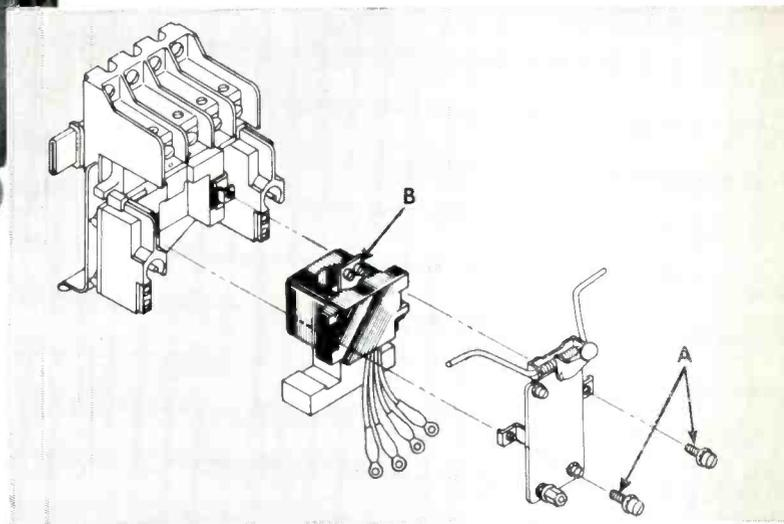
New coil design has stretched mechanical life of starter more than 50%. Extracting two bracket screws "A" and loosening of cross arm screws "B", as shown in exploded drawing, make coil removal easy.
