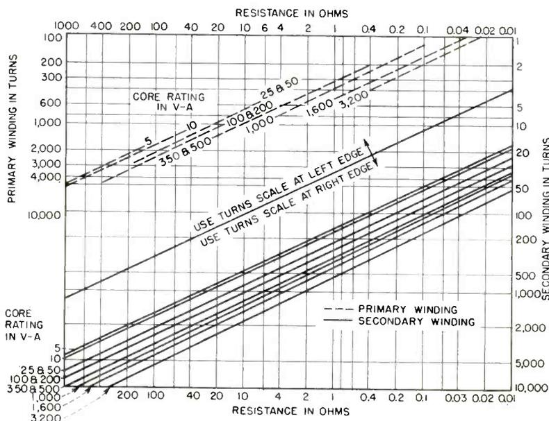
FIG. 3—Resistance of primary and secondary windings for type-C cores
