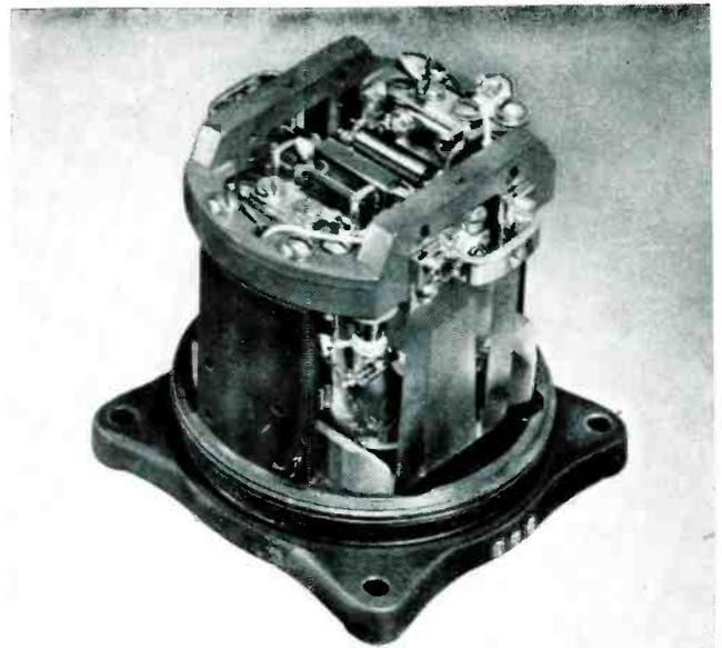
Giannini potentiometer accelerometer consists of magnetically damped, spring-supported mass system which actuates wiper arm of linear potentiometer through linkage system
