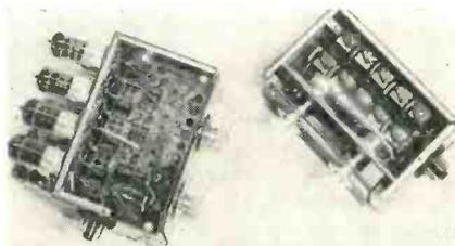
Two decimal counting units shown in the photograph use tubes (left) and ferristors (right). Reduced size results from using a 50-year old principle in development of a modified magnetic amplifier (*Electronics*, p 128, Oct. 1955). The particular application is that of Beckman Instruments, Inc.
