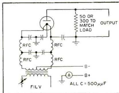
FIG. 2—Noise diode and its circuit
