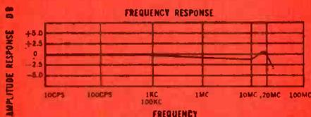
The Polarad Wide Band Video Amplifier offers an extremely wide band coverage: flat within  $\pm 1\frac{1}{2}$  db from 10 cycles to 20 megacycles per second. It has a time delay of 0.02 microseconds and assures extreme stability because of its associated electronically regulated unit. A low capacity input probe is provided.
