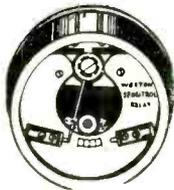
Stationary contact is a small powerful permanent magnet and movable contact is iron "rider" mounted on pointer which travels over relay scale. Operating torque moves pointer into magnetic field of stationary contact
