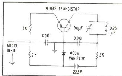
Circuit of simple 1-m transistor transmitter originally described in *ELECTRONICS*, p 130, Feb. 1954
