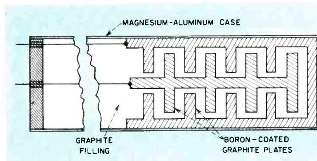
FIG. 11—Parallel circular-plate ionization chamber has boron-coated electrodes for detection of slow neutrons. Wire leads are of lead and are coated with quartz
