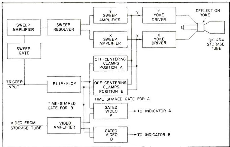
FIG. 3—Time-shared sweep permits alternate display on two radar indicators
