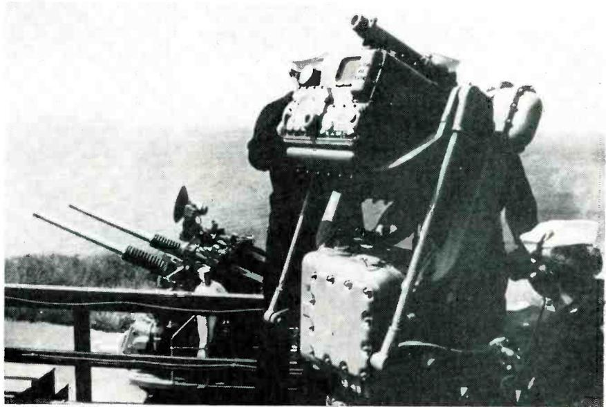
Tracking jet aircraft with 3 and 5-inch naval guns in any weather is possible using U. S. Navy's mark 63 gunfire control system manufactured by Sperry Gyroscope Co. Newer gunfire controls and radars have been combined with gyro-optical tracking principles used previously
