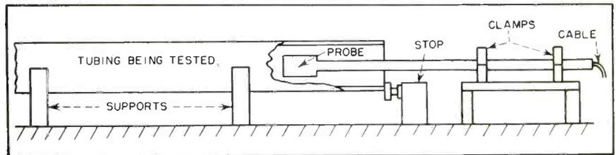
FIG. 3—Method of using probe for testing hardness of steel tubing
