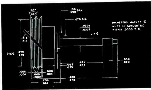
Inspection of incoming precision shafts took 10 to 15 minutes each by mechanical gaging—involving concentricity, diameters, shoulder locations, and other tough-to-measure dimensions to tolerances of .0002". Doing the work on a Kodak Contour Projector cut time to 2 to 3 minutes per shaft.
