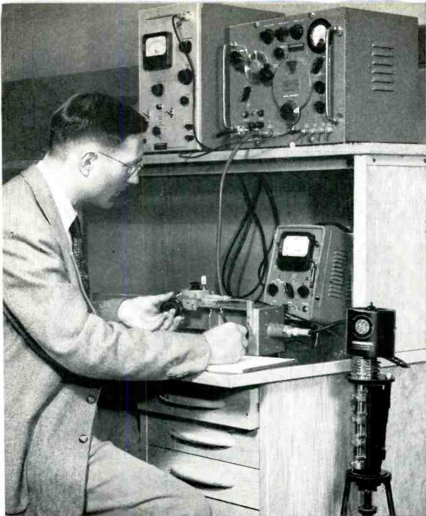
A research engineer at the General Electric Microwave Laboratory, Palo Alto, California, measures the output-cavity tuning characteristics of G.E.'s new 15-kw high-gain klystron that features single-knob tuning.
