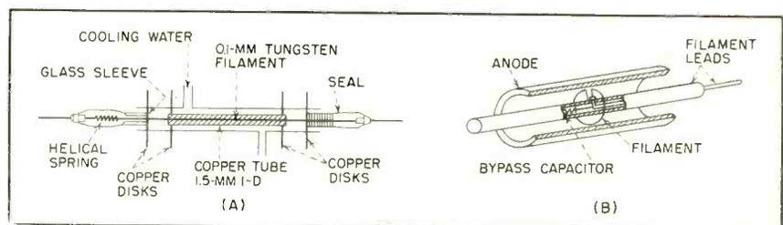
FIG. 3—Disk-seal coaxial noise diode (A) and coaxial-line noise diode (B)
