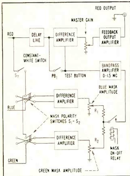
FIG. 4—Matrix amplifier for red channel
