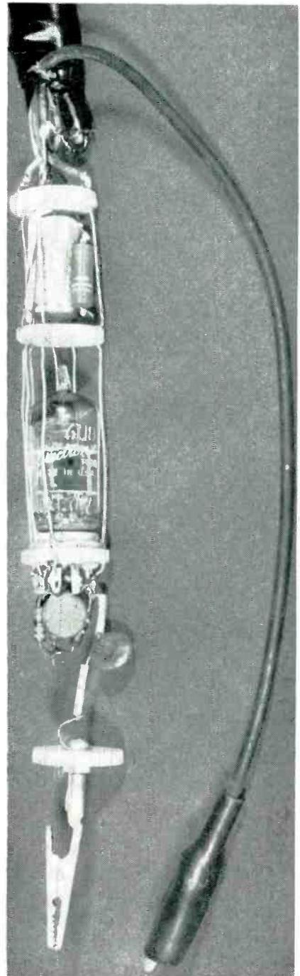
Components mounted on tube socket are connected to power supply and output wiring by bus wires running up sides of tube as shown in the photograph
