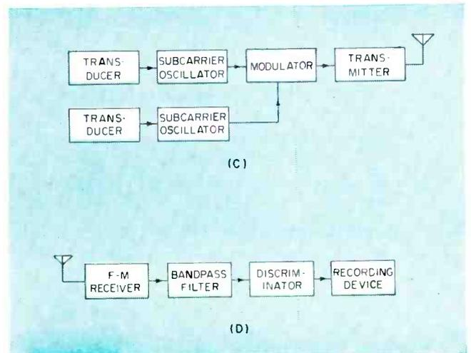
FIG. 19—Basis of pulse-width modulation of a frequency modulated carrier (pwm/f-m) transmitter (A) and receiver (B). Two-channel f-m/f-m transmitter (C) and receiver (D)
