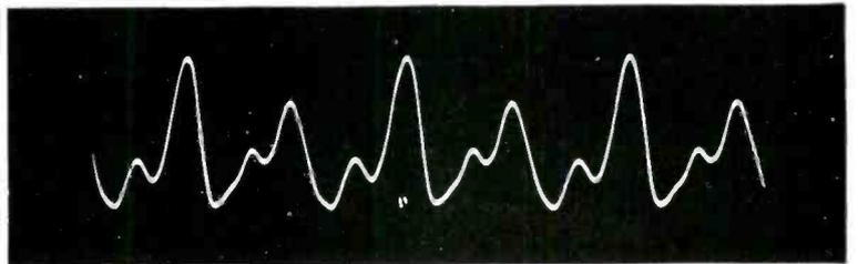
The selected samples are "stretched" for transmission. They travel in a narrower frequency band than complete sound.
