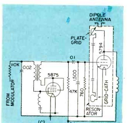
FIG. 27—Elements of a modern weather radiosonde (A) that show dependence upon the commutating system (B). Modulator and r-f transmitter shown at (C) transmit tones representing weather measurements
