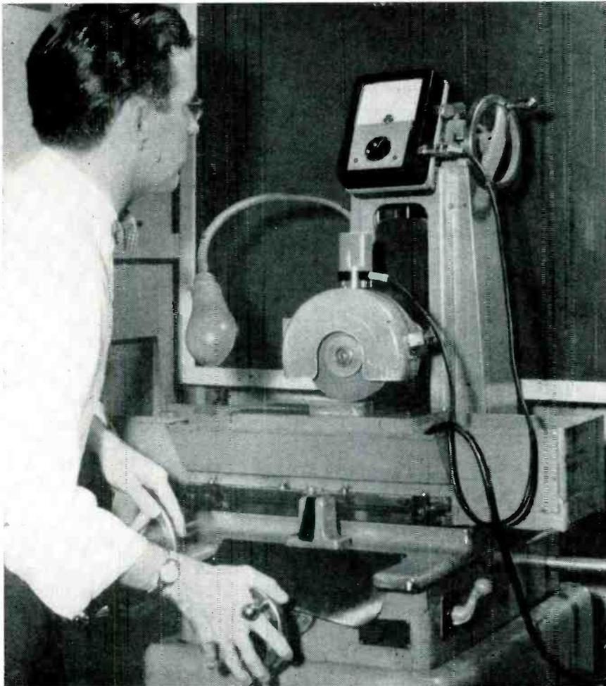
Engineer uses transistor vibration meter to check performance of grinding machine
