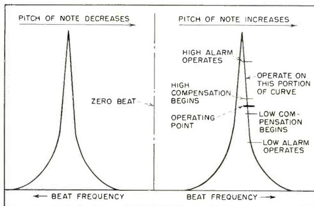
FIG. 2—Curves used for slow differential corrective system
