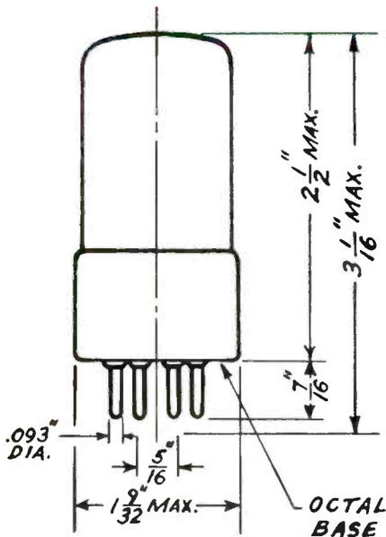
This precision sealed-in-glass crystal unit provides exceptional stability with minimum ageing when used as a reference source in secondary frequency standards.
