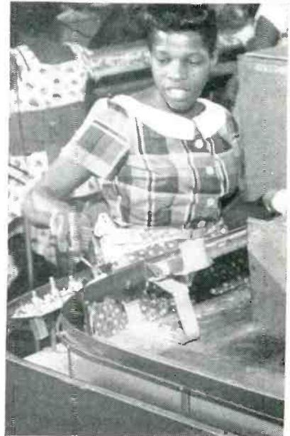
Method of using pliers to push a panel around the bend
