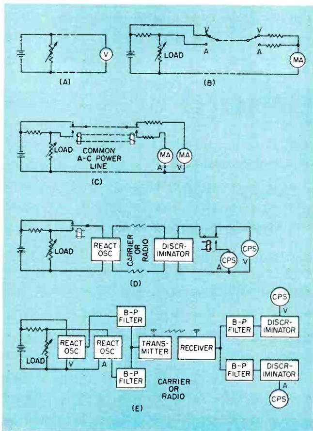
FIG. 1—Development of time-division and frequency-division telemetering systems. Means of computing power at a distance using wire line, radio or carrier is shown
