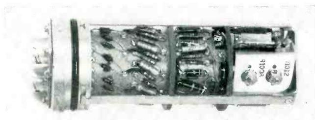
Signal Corps telemetering unit designed by Stavid Engineering
