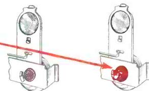
**Truarc way:** Molded plastic knob with pin is easily and quickly held by a Truarc self-locking ring (series 5105). No groove is necessary. Washer is eliminated and it is possible to remove ring if necessary without damage to knob.
