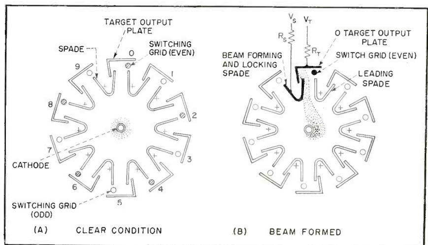
**FIG. 1**—Electron beam in 450-gauss axial magnetic field serves as equivalent of contact arm in switching from one to another of the ten target output plates under control of spade and grid potentials. Tube designation is now type 6700 (formerly type MO-10)
