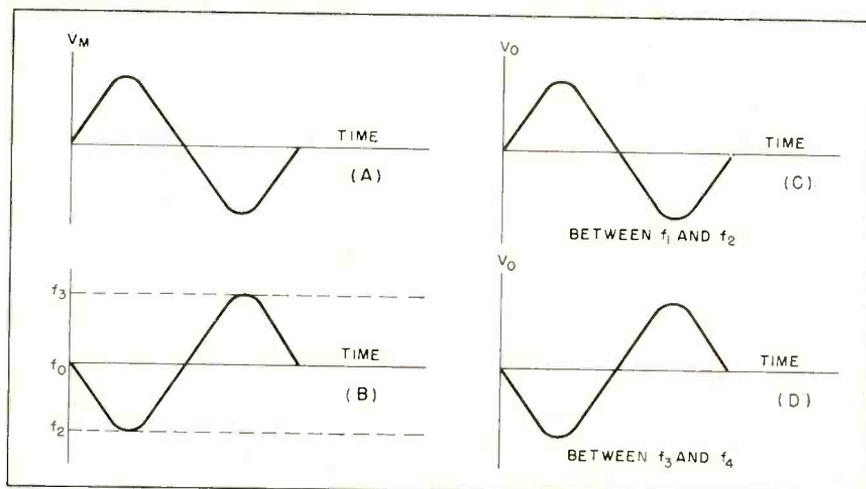
FIG. 4—Phase comparison between modulating voltage (A), reactance-tube resonant frequency (B) and servo output (C) and (D)
