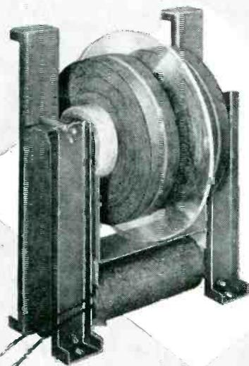
**High Voltage Plate Transformer** for use under oil with other equipment in same tank. Unit shown is 50 KV center tap grounded, 4 KVA and high impedance. Note plastic insulation shield between coils. This unit available from 100 VA to 100 KVA.
