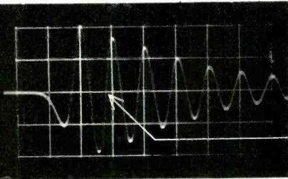
Arrow indicates 1100-cm/ $\mu$ sec writing-rate point on 100-mc damped oscillation, displayed on single 0.01  $\mu$ sec/cm sweep of Type 517A Oscilloscope with T54P11H crt. Recorded on 35-mm TRI-X film at  $f$  1.9 with 4.2 to 1 reduction, developed 26 minutes in D-19 at 68° F.
