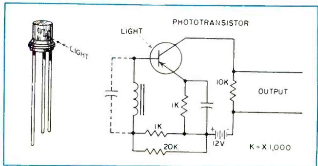
**FIG. 9—Typical Radio Receptor pnp germanium-junction phototransistor and circuit for modulated-light use. Base inductance is tuned to light-modulation frequency for best signal-to-noise ratio**
