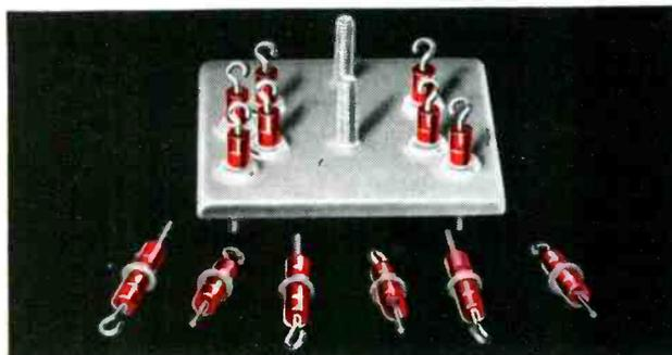
**HERMETICALLY-SEALED TERMINALS** with KEL-F plastic insulation handle high voltage without flash-over or tracking. Won't shrink, swell, age or lose hermetic seal at high and low operating temperatures. Can be used in contact with highly corrosive chemicals.
