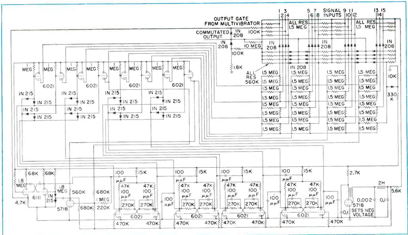
FIG. 25—Circuit diagram of an electronic commutator using tubes and diodes. Time sharing of radio-frequency channels is possible without use of rotating devices when fifteen channels are employed. Equipment is built by Electro-Mechanical Research
