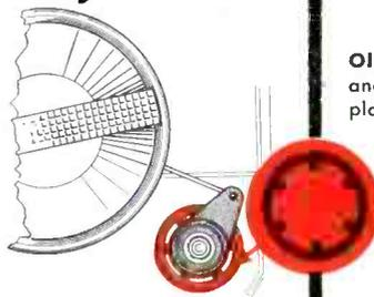
Parts originally designed for self-locking Truarc ring (series 5105). Some cameras in the past had brass cup staked to the body. At times staking operation cracked the plastic, resulting in loss of expensive part.
