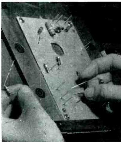
Method of loading components into wiring board on cut-and-clinch machine. Operator bends leads herself
