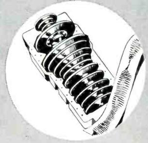
**GENERAL ELECTRIC** ... uses Frequency Response Recorder to check mechanical resonance points of both steam and jet turbines when blades are magnetically vibrated.
