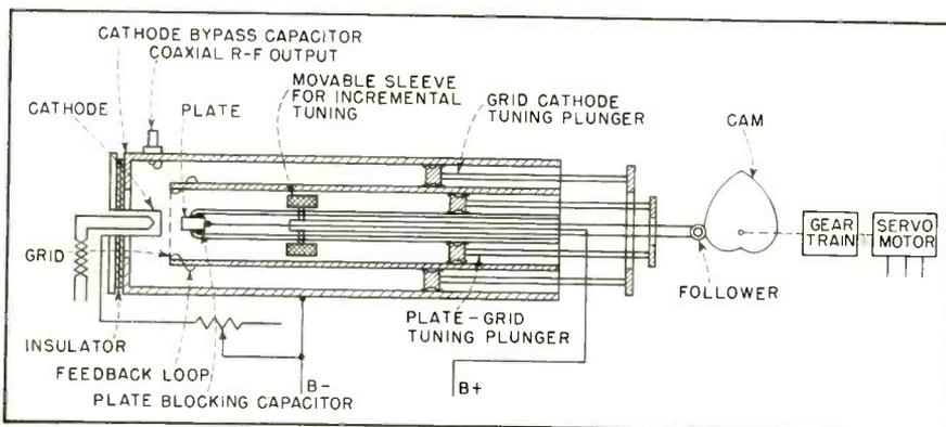
FIG. 1—Cross-section of stable L-band local oscillator
