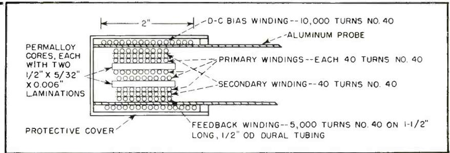
FIG. 2—Probe construction details. Spacings and insulating techniques are critical
