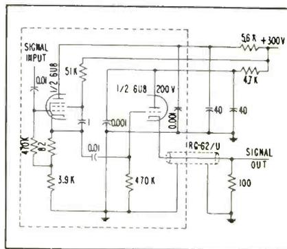
Tandem cathode-follower probe has attenuation of only 2 to 1 with input capacitance of less than 3  $\mu\text{m}$
