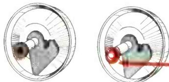
**Truarc way:** Truarc "E" ring (series 5133) allows removal of winding knob without major disassembly of camera, reducing repair time. Use of stacked rings and Truarc applicator saved \$10.40 per M on labor. Material saving: \$2.29 per M.
