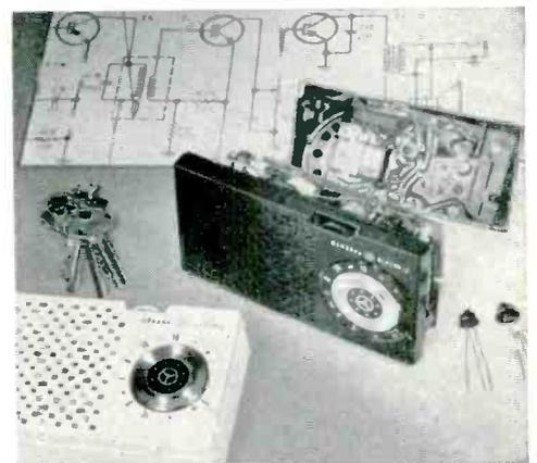
**Positive Proof.** This new transistorized portable radio features a full printed circuit using a General Electric "Thru-Con" Board. Combining other advances in electronics with a "Thru-Con" circuit makes possible sweeping changes in size, weight, and styling.
