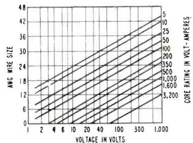
FIG. 2—Winding wire size in relation to voltage and core rating
