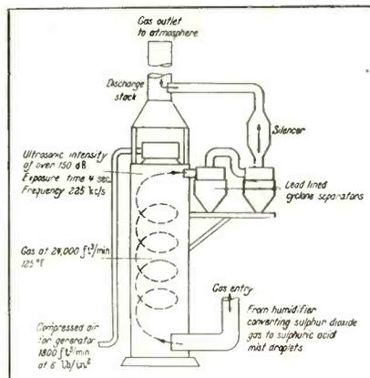
Schematic arrangement of acid fog precipitation using sonic agglomeration
