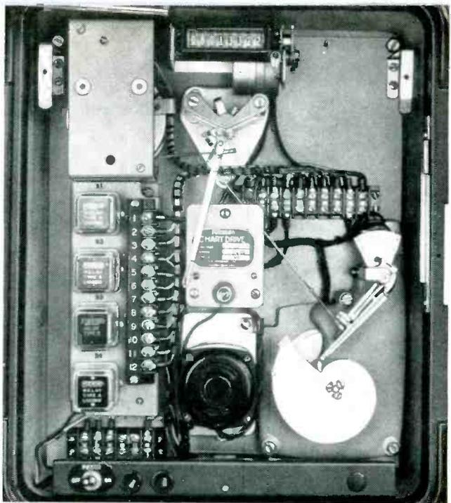
This telemeter transmitter (left) uses a cam to transmit the temperature pickup reading. The receiver (right) has a reversible motor that moves in either direction or remains motionless. A pen is attached to the drive
