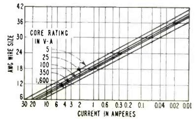
FIG. 4—Relation of winding wire size to current
