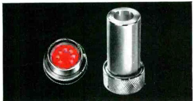
**TUBE SOCKETS** of tough KEL-F plastic. Hermetic seal defies thermal cycling, aging and humidity. Withstands high shock loads without chipping or cracking insulation. Plastic's high dielectric strength prevents shorting or arc-over at high altitudes.
