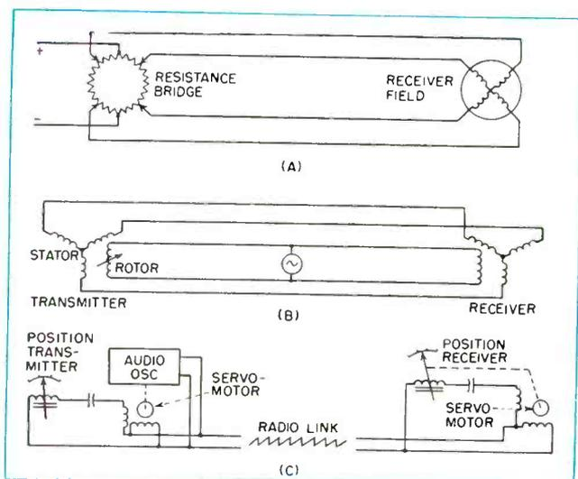
FIG. 15—Remote dial reading systems. So-called d-c synchro (A), conventional a-c synchro (B), and tuned audio system (C)
