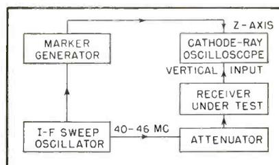
FIG. 1—Sweep generator and marker generator connections to equipment
