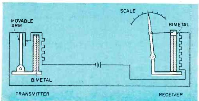
FIG. 2—Simple telemeter that depends upon the heating of bimetallic strips. Position of the movable arm determines height on scale to which pointer will rise
