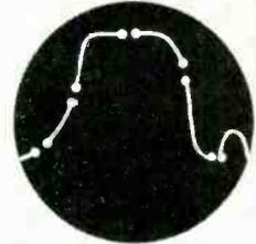
Response curves accurately displayed. Ideal for use with Weston intensity marker display. A fast, retrace sweep circuit with cathode follower output prevents pattern distortion.
