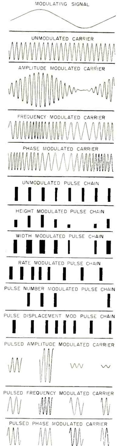
FIG. 20—Comparison of various types of modulation useful in telemetering data
