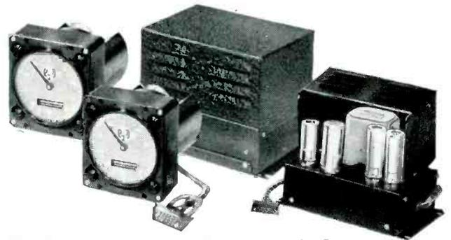
The Transcoil servo assembly used in the Lorac receiver. Components include a 400 cycle oscillator supply for two indicators and two servo amplifiers. System is built on separate chassis to permit the indicators and amplifiers to be located in separate parts of the ship.
