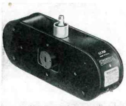
The MA-200 is a pulsed-type fixed-tuned magnetron generating approximately 40 kw peak power at 35 kmc. Its r-f spectrum is unchanged when subjected to vibration conditions of 15 g at 1,000 cycles.
