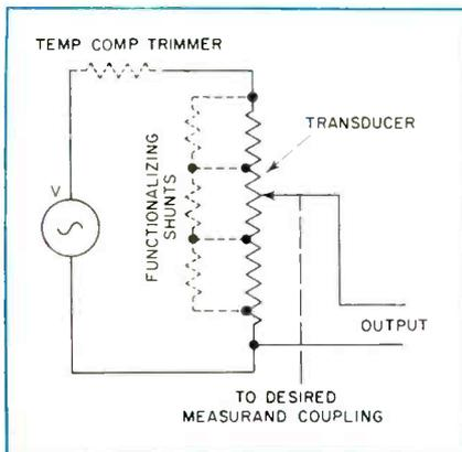
FIG. 6—Typical potentiometer-transducer circuitry. Dashed-line components may be added as needed
