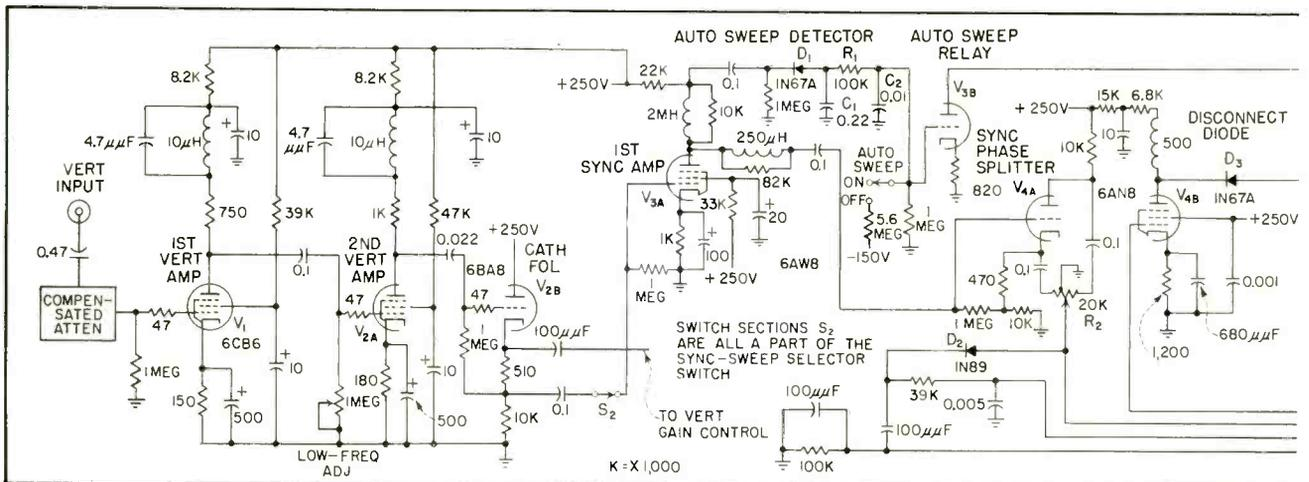
FIG. 1—Automatic triggered sweep circuit as used in Hycon model 622 oscilloscope, with conventional unmodified stages of
