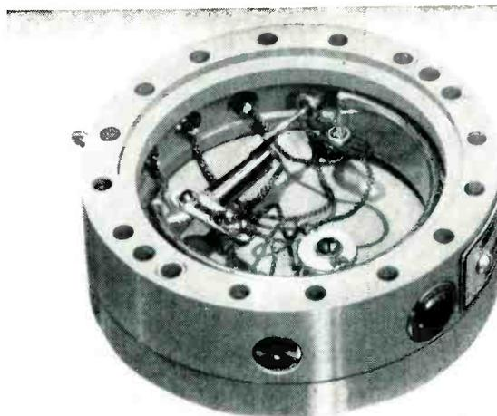
Giannini Bourdon-tube potentiometer pressure transducer has liquid-filled case to isolate mechanism from corrosive media and to provide damping against shock and vibration
