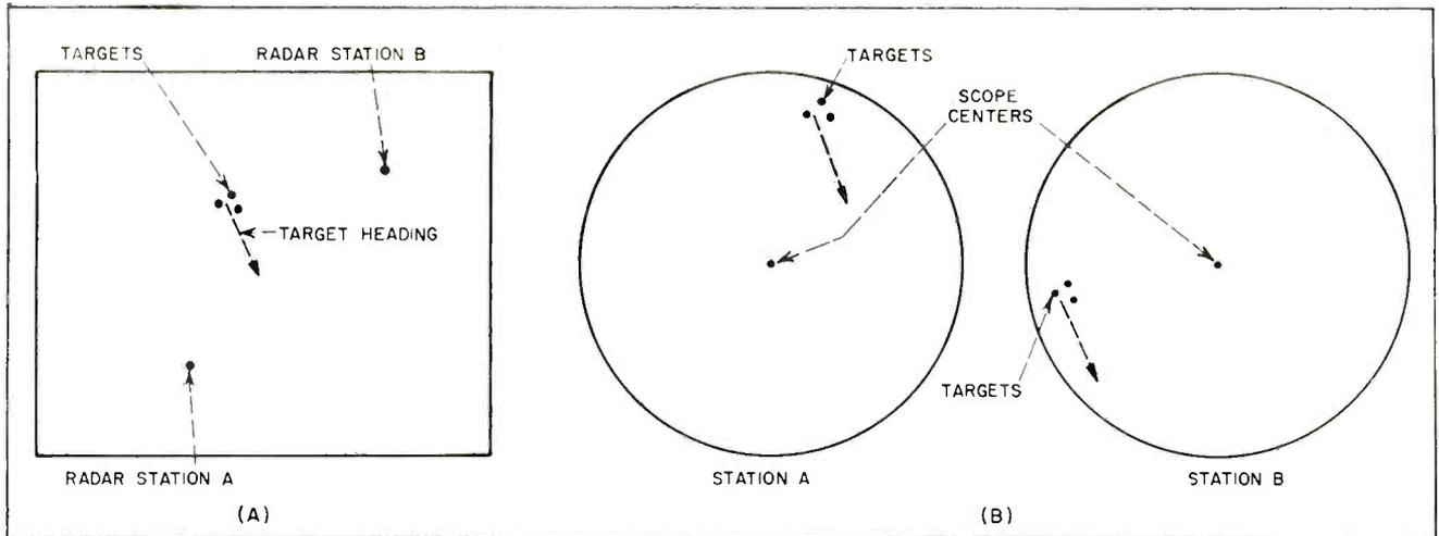
FIG. 1—Configuration of targets and radar stations (A) and simulated ppi presentations (B)
