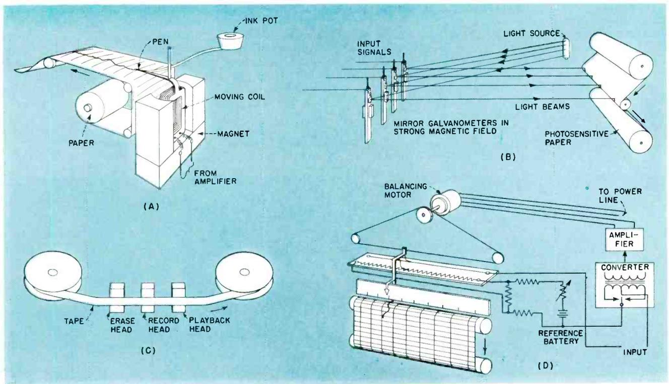
FIG. 28—Typical data recording devices include direct-writing oscillograph (A), galvanometer oscillograph (B), magnetic-tape recorder (C) and self-balancing recorder (D). Telemeter signals are usually stored on tape then played back, processed and recorded on one of other types of recorders. Information is processed as many times as necessary to get into desired final form
