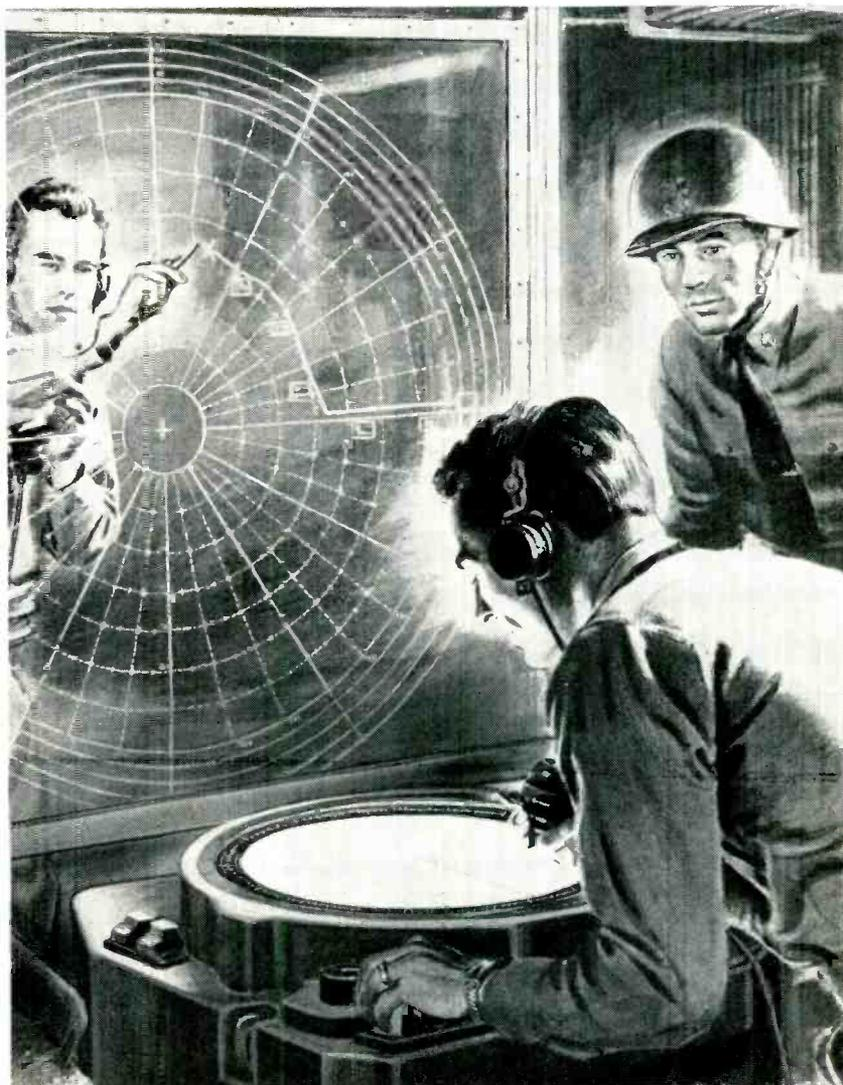
Direct plotting on the face of a 22-inch indicator is now possible through the use of our AN/SPA-23 (XN-1) indicator.
