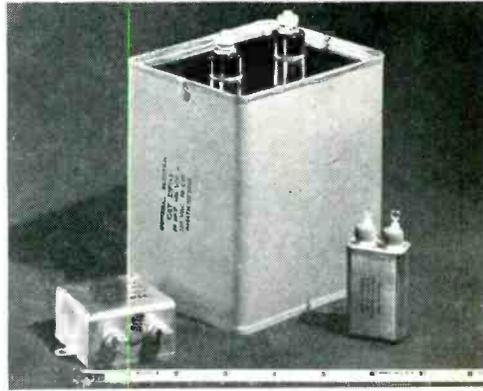
**MIL-C-25A CAPACITORS**—for filter, by-pass, and blocking in military equipment. Built to MIL-C-25A specifications. Ratings: .05 to 15 uf at 100 to 12,500 v. d-c in case styles CP50, CP60, CP70 series. Temp. range:  $-55^{\circ}\text{C}$  to  $+85^{\circ}\text{C}$ , and  $-55^{\circ}\text{C}$  to  $+125^{\circ}\text{C}$ . Write for GEC-810.
