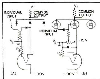
FIG. 11—Beam-gated sampling circuits
