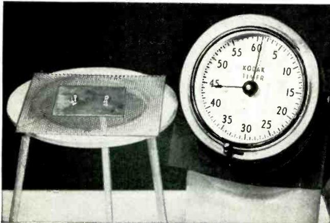
**Set test up like this!** Place one-inch, doubled-up samples of ordinary rosin core and "Dutch Boy" *activated* rosin core solders on sheet of clean copper. (In these pictures, "Dutch Boy" sample is on your right.)
