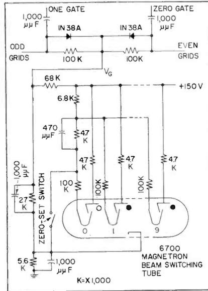
FIG. 3—Basic switching circuit
