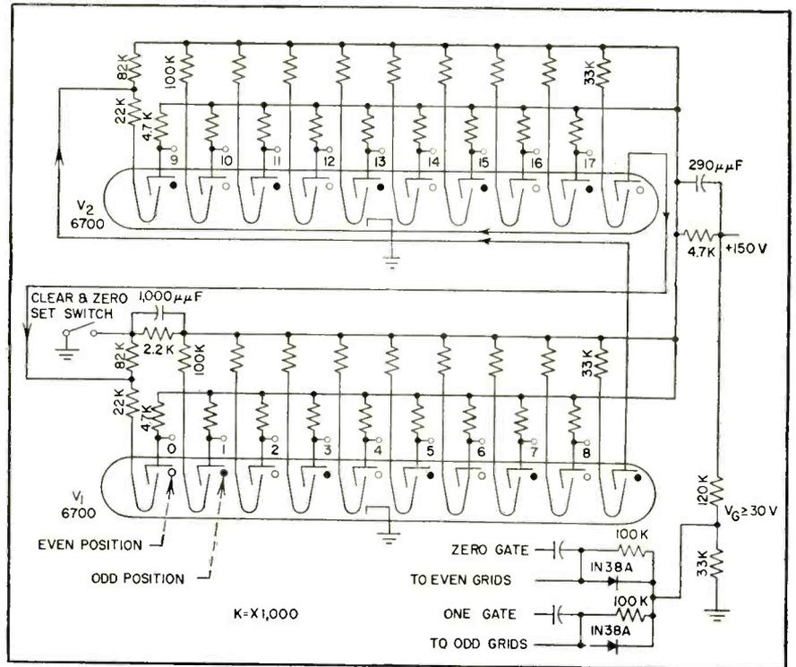
FIG. 7—Multiposition distributor using two type 6700 magnetron beam switching tubes
