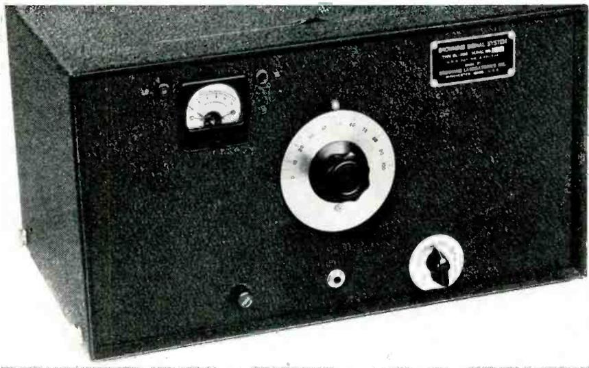
Front view of control unit, showing tuning dials, tuning meter and phone jack
