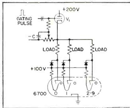
FIG. 9—Single-triode gating circuit
