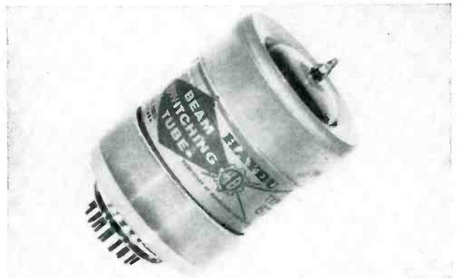
Beam switching tube of a type being used in telemetering equipment
