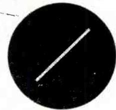
Phase shift between horizontal-vertical amplifiers, 0-500 kc-0°, to 1 mc within 2°; by internal adjustment with gain controls at max 0° phase shift possible on any specific frequency to 6 mc.
