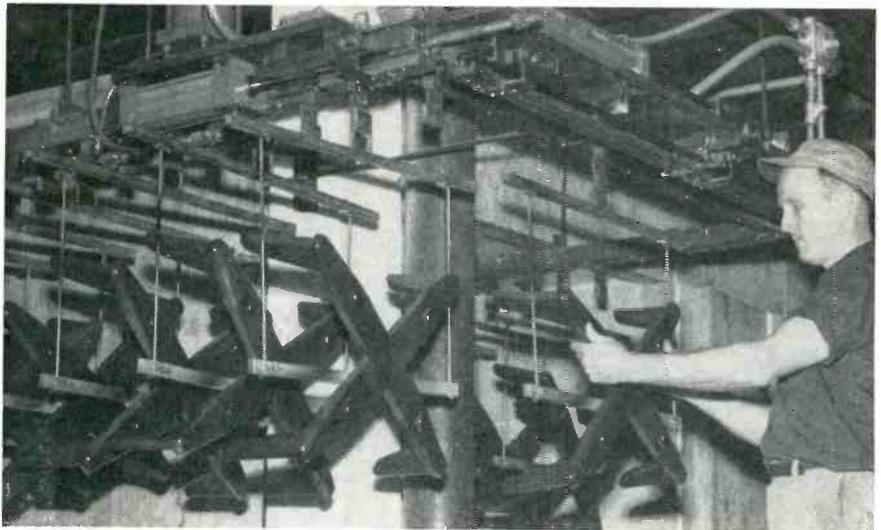
Square-corner conveyor transfer setup at output of drying tunnel for spray-finished bases
