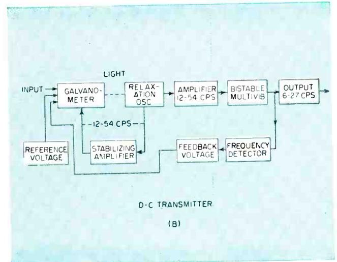
FIG. 18—Power-line telemetering system sends low-frequency pulses derived from rotation of disk between light and phototube caused by variation in a-c parameters (A). Information derived from d-c is transmitted by equipment (B)
