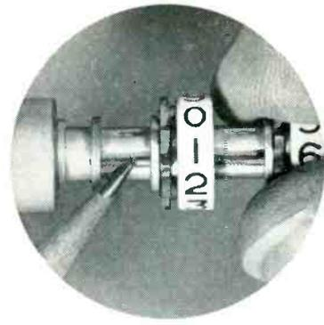
The problem was to check many small calculating machine parts averaging about 13 critical dimensions for each with shapes mostly complex. With carefully engineered mechanical gages, inspection time averaged 50 seconds each. Optical gaging on a Kodak Contour Projector brought the average down to 12 seconds.
