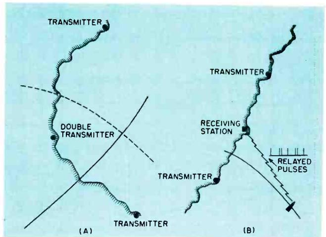
FIG. 5—Data transmission in position-finding system often depends upon time of propagation. A standard hyperbolic fix from two pairs of transmitters is shown at (A). A relayed line of position comes from the lifeboat at (B)
