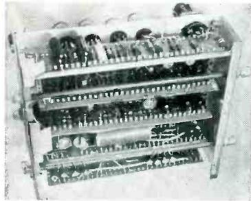
**BUT THIS**—Neat, compact vertical "planes of circuitry" result from construction based on Alden Terminal Card Mounting System.
