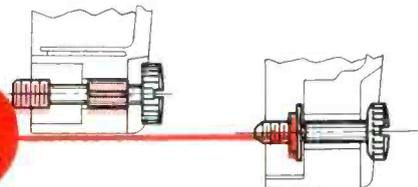
**Truarc way:** Series 5133 E-Ring snaps onto unthreaded shank of screw quickly, needs no special groove. Labor saving \$7.06/M.
