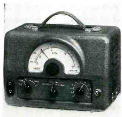
from 30 cps to 30 kc which largely covers the acoustic frequency range. It is intended for adjustments of a-f amplifiers and measurements at audio and acoustic frequencies. Output level is adjustable from 10 μv to 10 v by an accurate attenuator system. An automatic regulation circuit keeps the output level constant with changes in frequencies.
