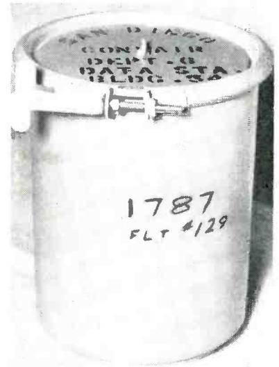
Shipping container ready for shipment to data reduction station, with identifying data marked on side with grease pencil
