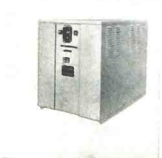
**INDUCTROL POWER PACK**— This is a load center unit substitution for a-c power and lighting service. Unit includes a transformer, Inductrol, circuit breakers, and distribution panel board. Generally applied in three-phase circuits—600 volts and below—indoor service.
