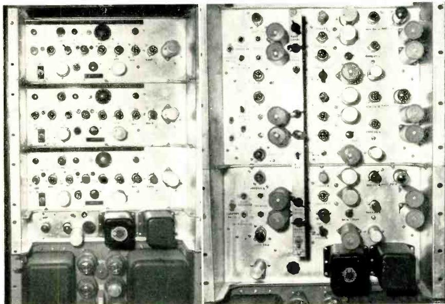
Complete three-channel gamma correction amplifier
