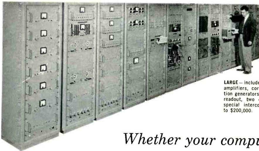
**LARGE**—includes two control units with 200 pots, 80 amplifiers, corresponding number of multipliers, function generators, etc., plus digital voltmeter with printed readout, two 4-channel recorders, timing matrix and special interconnecting panel. Price range, \$100,000 to \$200,000.
