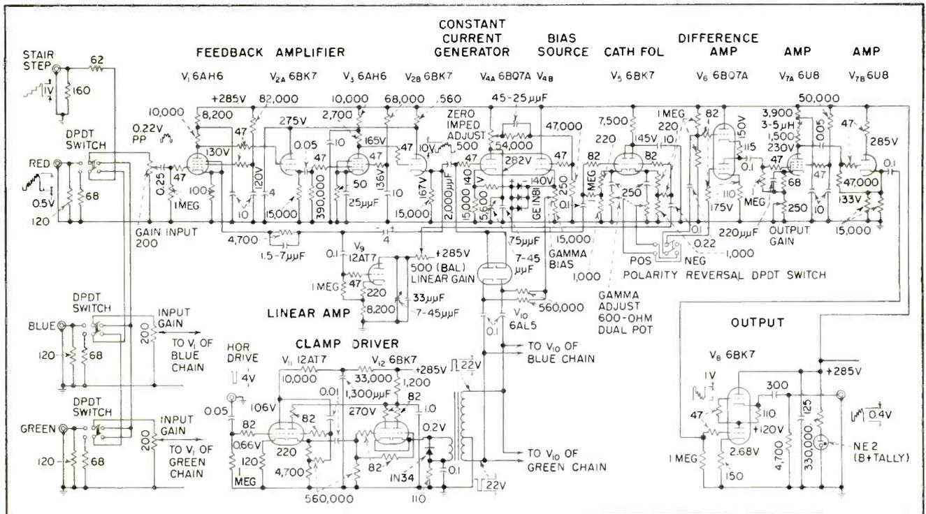
FIG. 2—Red-channel gamma or gradient correction amplifier. Blue and green channels are identical
