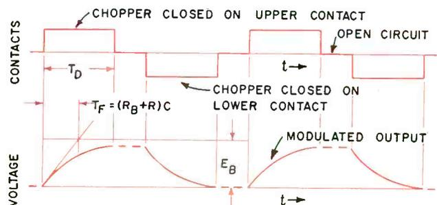
Upper diagram shows timing of chopper action, lower one shows effect of low-pass filter on output
