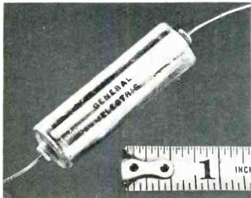
**METAL-CLAD TUBULAR CAPACITORS** for all d-c uses where utmost reliability is required. Ratings: .001 to 1.0 uf, 100-600 v. d-c. Tol:  $\pm 5\%$ ,  $\pm 10\%$ , or  $\pm 20\%$ . Temp. range:  $-55^{\circ}\text{C}$  to  $+125^{\circ}\text{C}$  with solid impregnant;  $-55^{\circ}\text{C}$  to  $+85^{\circ}\text{C}$  with mineral oil. Write for GEC-987.
