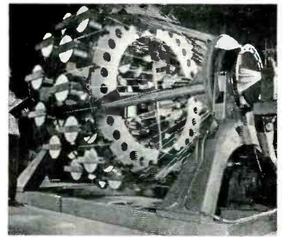
Cable-maker for short-run orders can be easily changed over for producing wide variety of cables
