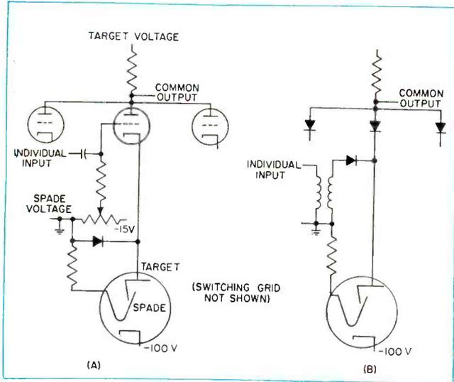
FIG. 26—Typical beam-gated sampling circuits using the Burroughs magnetron beam switching tube built by Haydu.
