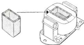
**Coil forms** for this solenoid have to operate at high temperatures . . . an ideal application for Taylor glass melamine laminate.
