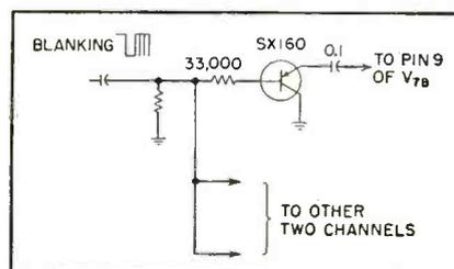
FIG. 3—Noise reduction circuit for blanking in gamma correction amplifier
