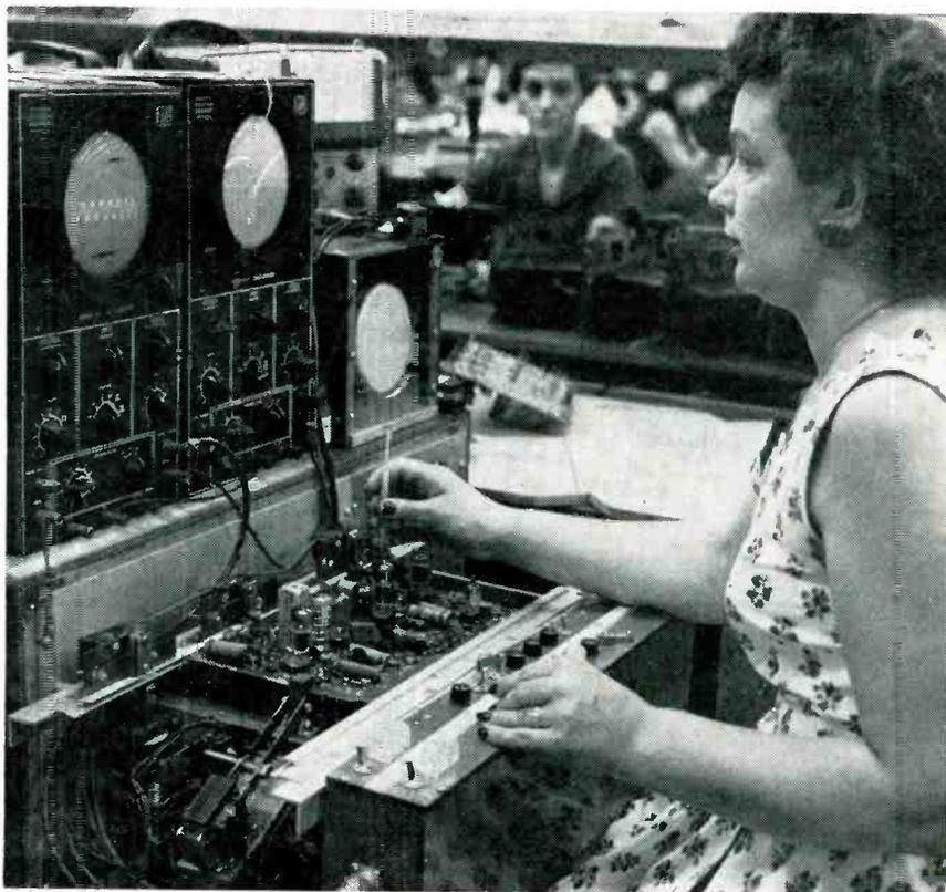
Adjusting transformer on sync board. All connections are made automatically by solenoids after operator slides board into position on test stand
