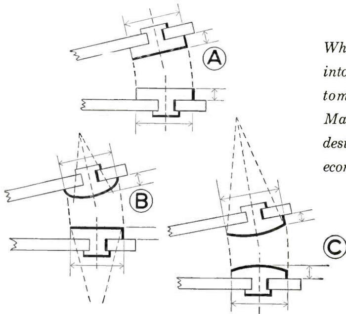
When Original Design A ran into alignment trouble, the customer proposed design B. Mallory engineers recommended design C as the most efficient and economical solution.
