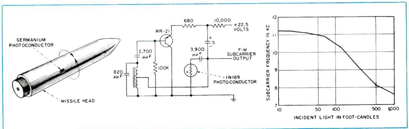
FIG. 8—Test-missile head contains germanium photoconductor which is employed as frequency-determining element of transistor f-m subcarrier oscillator. Spinning of missile causes light falling on photoconductor to vary and in turn vary subcarrier frequency
