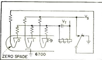
FIG. 6—Automatic zero reset circuit
