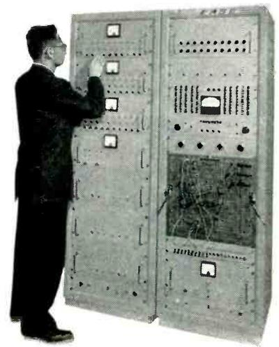
**SMALL**—includes control unit with 50 pots, 30 amplifiers, 2 electronic multipliers, 10 initial condition voltage sources, power supplies. Price range, \$12,000 to \$25,000.
