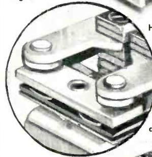
Heavy, double break contacts of 11-D and 22-D Relays—SPDTNO only. Rated 20 amps. at 115 VAC or 32 VDC, non inductive load.
