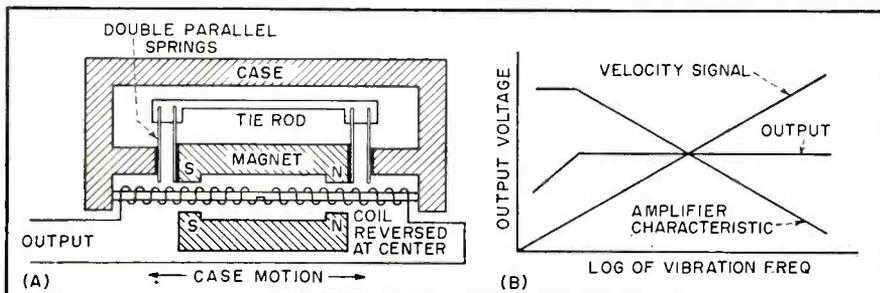
FIG. 1—Electromagnetic vibration transducer used as pickup (A) and voltage-frequency transfer characteristics of system (B)
