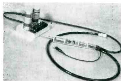
Video probe with power-supply filter chassis. Cable terminating resistor is located in cable connector
