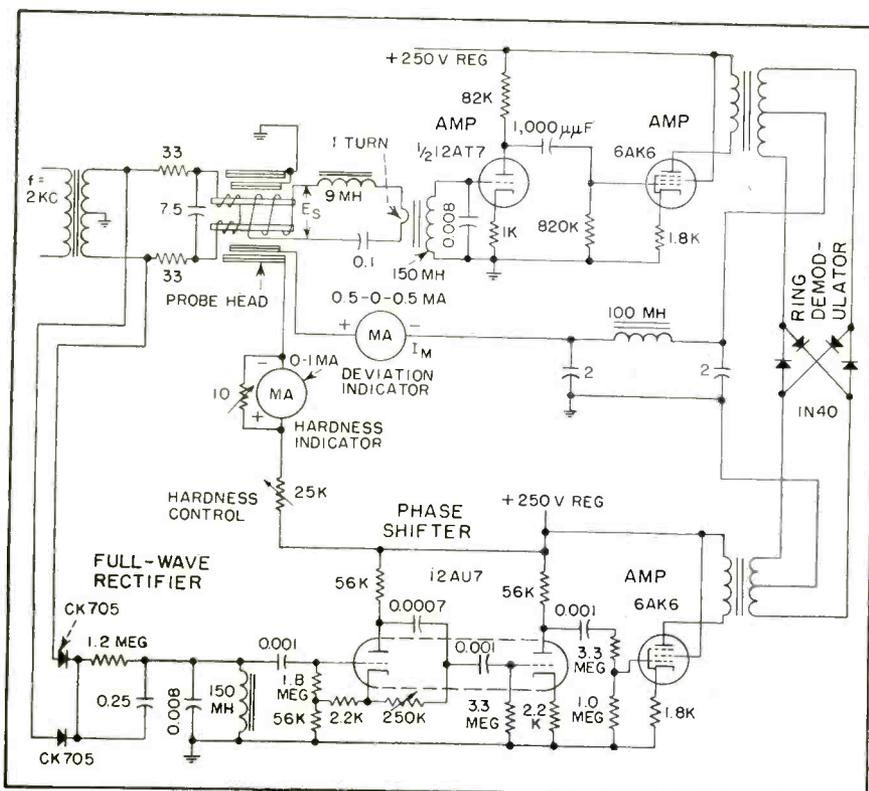
FIG. 1—Circuit of hardness tester. Readings proportional to hardness are obtained from either meter, depending on technique of use
