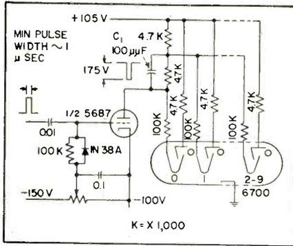
FIG. 5—High-speed clear and reset circuit using direct coupling
