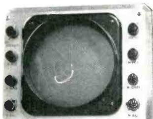
**DIRECT DISPLAY OF IMPEDANCE** can be obtained by using the Type 1025 Hybrid in conjunction with the AMCI type 1028 Polar Display Unit (frequency range 120 mc to 240 mc) together with a standard d-c oscilloscope and suitable swept oscillator. A typical display is shown in the unretouched photograph at the left.
