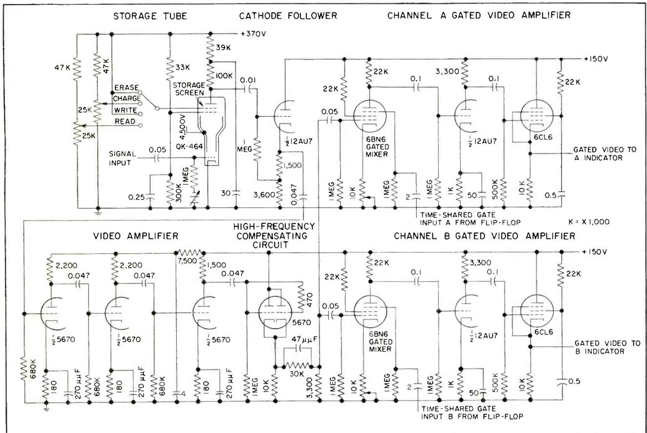
FIG. 4—Storage tube circuits, video amplifier and gated video circuits constitute heart of radar simulator
