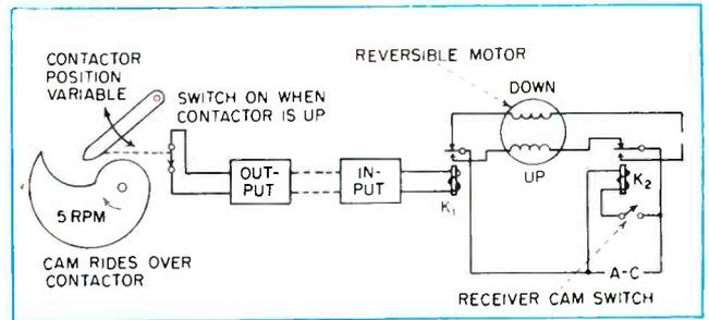
FIG. 17—Position of mechanical contactor arm relative to rotating cam is compared with a similar cam that controls direction of rotation of motor to move receiver dial in the Foxboro telemeter
