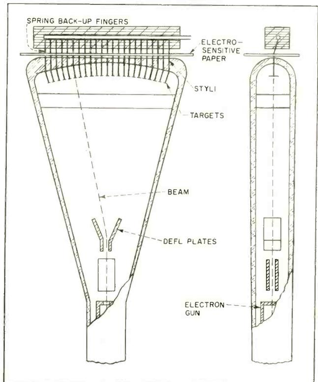
FIG. 1—Original concept of recorder tube, as shown by front and side views in patent application. Recording paper is pulled across face of tube by drive mechanism
