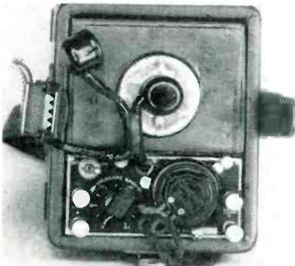
Vacuum tube repeater (EE-89) that weighs 16 pounds will be replaced
