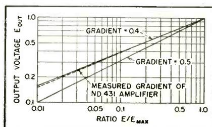
FIG. 1—Measured transfer characteristic of gamma correction amplifier
