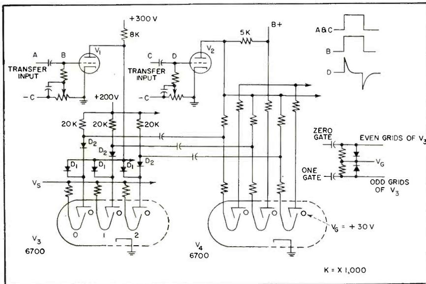
FIG. 10—Transfer-storage circuit using two switching tubes
