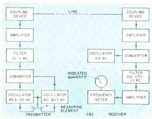
FIG. 16—Frequency telemetering system depends upon transmission of audio tone (A). Variation of the system uses two oscillators whose frequencies are varied in opposite directions (B)
