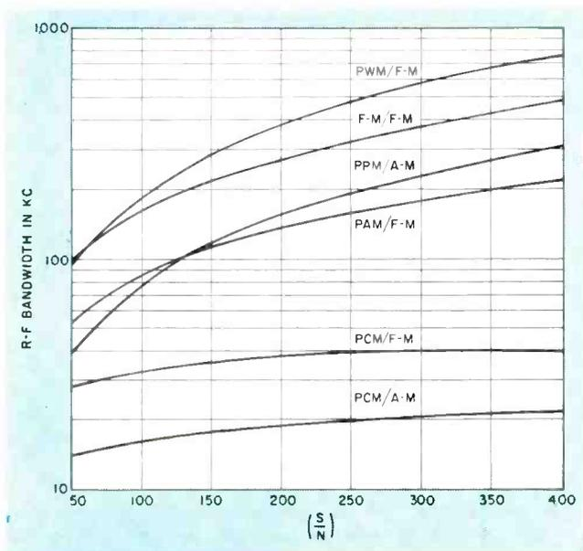
FIG. 21—Pulse-code signaling systems compared with other types on the basis of signal-noise ratio and bandwidth
