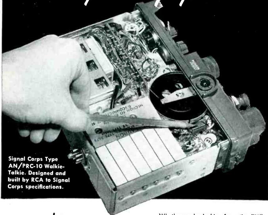
Signal Corps Type AN/PRC-10 Walkie-Talkie. Designed and built by RCA to Signal Corps specifications.
