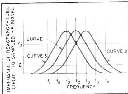
FIG. 2—Variation of impedance-frequency characteristic of resonant circuit
