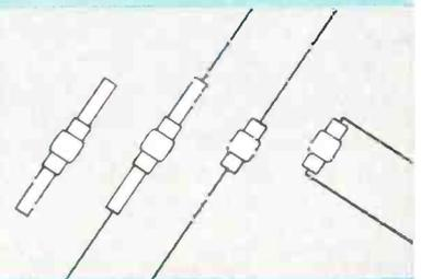
PSI germanium and silicon diodes (here, actual size) are offered with these four basic lead arrangements.
