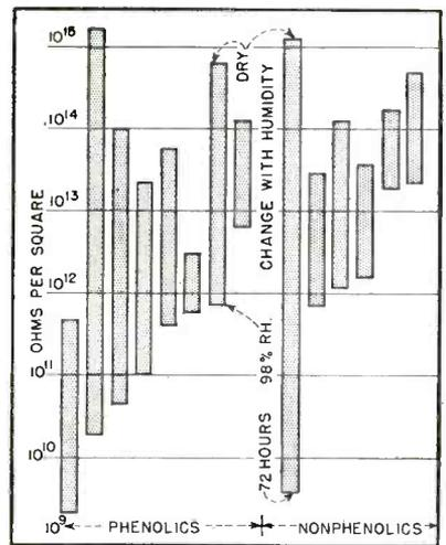
FIG. 1—Apparent surface resistivity of copper-clad plastic materials. Lengths of vertical bars represent change in resistivity; upper end of each bar is dry value and lower end is value after 72 hours at 98-percent humidity
