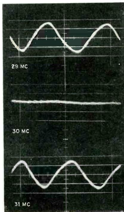
FIG. 6—Servo amplifier output waveforms at null and at either side of null
