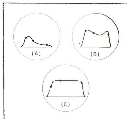
Fig. 2—Positive pulses as they appear before alignment (A), curve shape after positive pulse peaking (B) and i-f response after touchup (C) using negative pulses as reference markers
