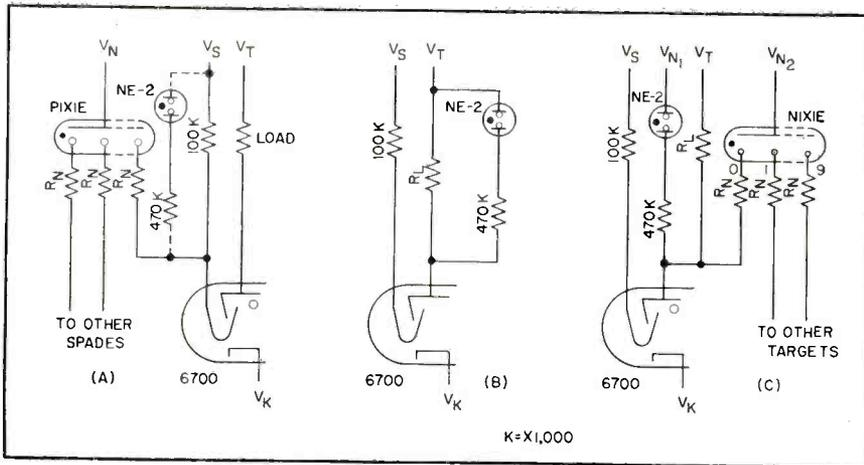
FIG. 12—Three methods of obtaining visual read-out
