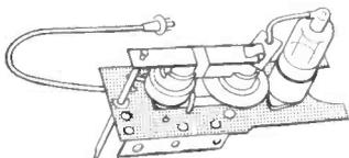
**Base plate** for high-voltage TV component, punched from Taylor canvas melamine laminate, has high dielectric strength and arc resistance.
