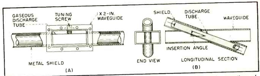
FIG. 4—Glow-discharge noise source for microwave frequency (A) and mounting of small-bore tube to generate shf noise (B)
