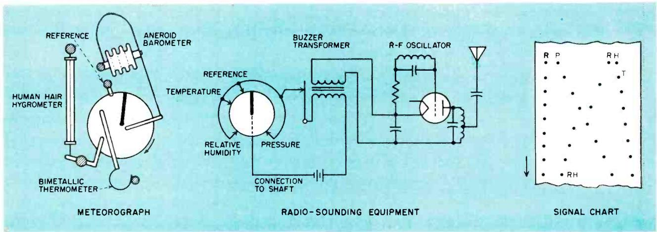
FIG. 3—Elements of a radiosonde based upon the Olland sampling principle. Relative displacement of elements is shown by a series of short dashes on moving chart paper at ground station
