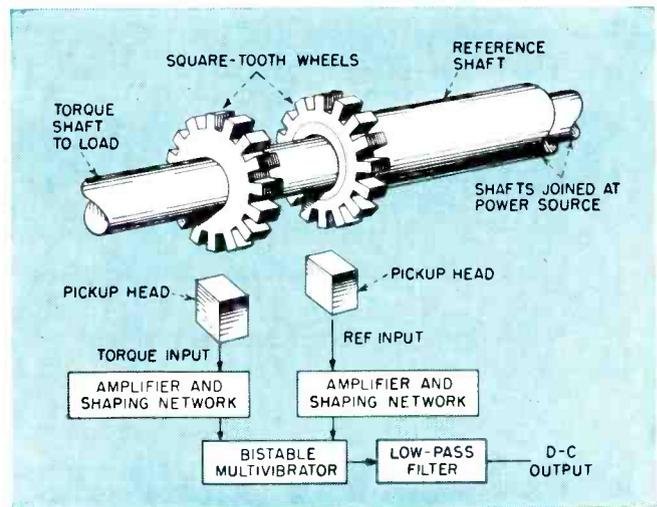
FIG. 12—Phase shift between signals from two pickup heads is proportional to amount of twist between torque-carrying shaft and reference shaft and gives indication of dynamic torque
