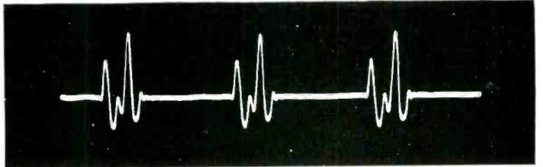
An electronic sampling of the "or" sound. One "pitch period" in three has been selected for transmission. This permits great naturalness when voice is rebuilt. Intelligible speech could be sent through a 1 in 6 sampling.
