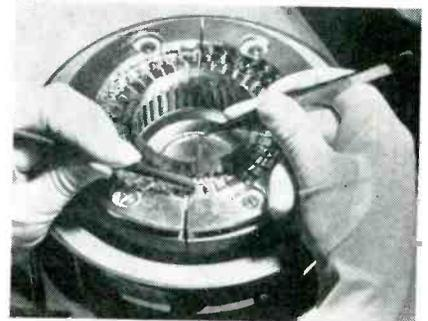
Typical of the step-by-step sequence of operations in assembling a beam-power, water-cooled RCA tetrode for use in uhf television is that of placing cathodes in position with tweezers. As shown in the photograph, the tool in the left hand is used to depress the pantograph cathode spring to which the cathode is clipped
