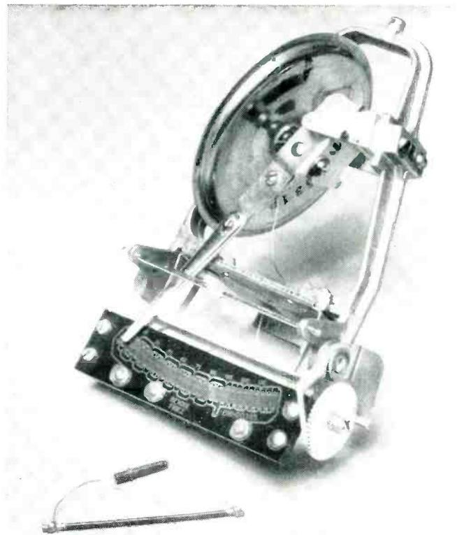
Transducer elements of radiosonde include, from top to bottom, barometer for altitude, thermistor for temperature and lithium-chloride coated plastic sheet for humidity measurements
