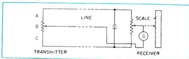
FIG. 14—Elementary bridge system requires manual operation at receiver but is easily adapted to servo balancing control
