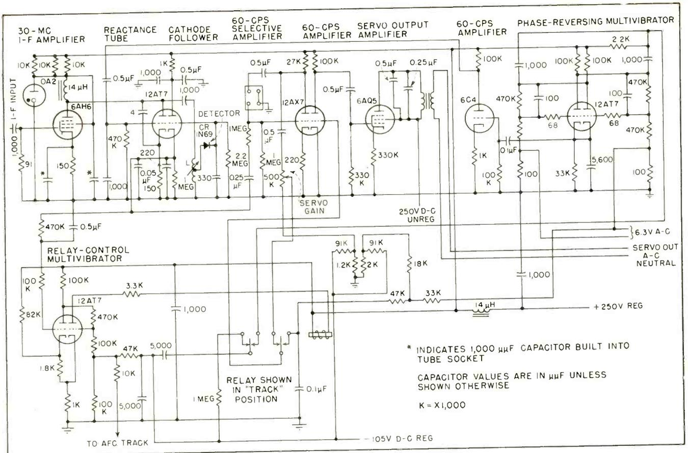
FIG. 5—Complete circuit provides frequency deviation detection and electronic control over search-afc transition
