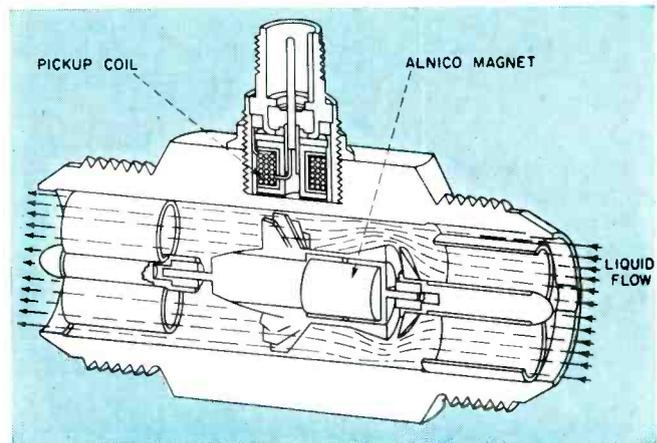
FIG. 13—Permanent magnet in hub of hydraulically suspended Potter flow meter induces signal in pickup coil. Signal frequency is proportional to flow rate; total pulses are proportional to total flow
