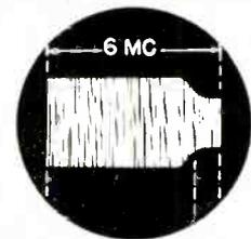
Note flatness throughout specified range; to 3.6 mc down 1.5 db, at 4.5 mc down 3 db, at 6 mc down 6 db.
