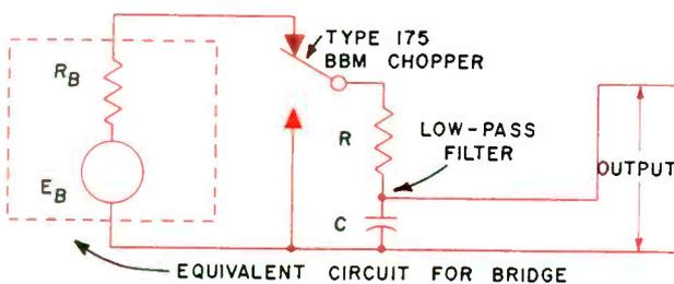
In basic modulator circuit, chopper alternately connects filter across bridge and then shorts filter
