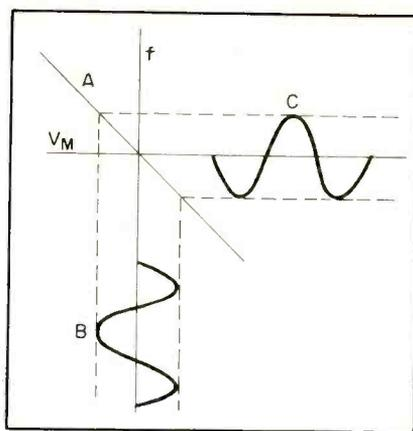
FIG. 3—Transfer characteristic of reactance-tube circuit
