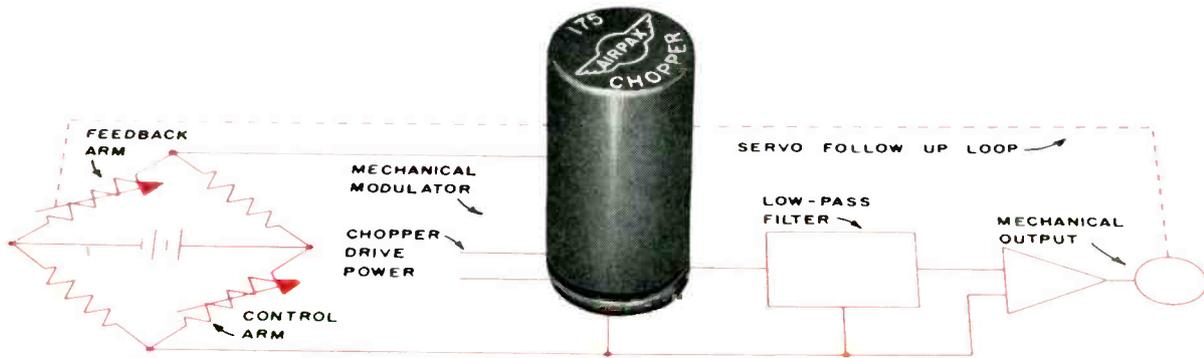
To minimize loading the bridge, a high-impedance modulator is used such as Airpax Type 175
