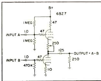
FIG. 6—Simplified diagram of difference amplifier used in each masking amplifier channel
