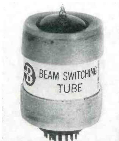
Tube is 3 inches long including polyethylene end caps, 1.7 inches in diameter and weighs 5 oz including its encapsulating cylindrical permanent magnet
