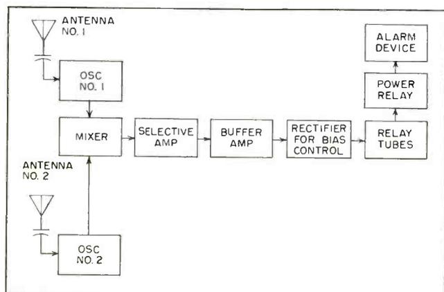
FIG. 1—Elements of complete electrostatic intrusion alarm
