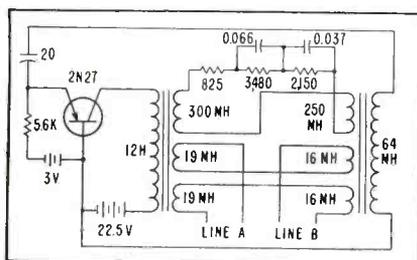
FIG. 1—Transistor negative-impedance telephone line repeater
