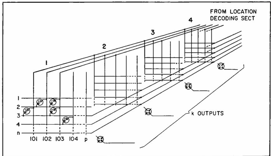
FIG. 5—Neon-tube matrix memory with four-bit output
