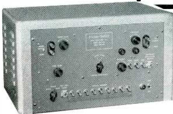
A combined sweeping oscillator and crystal marker generator, the Rada-Sweep is designed especially for rapid alignment of radar IF amplifiers. Used with an oscilloscope, it will display response curves of IF amplifiers and mark up to nine frequencies to allow precise adjustment of response.
