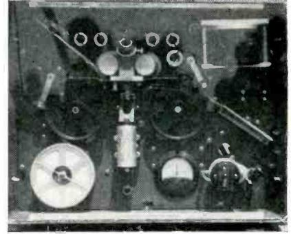
Back (left) and front (right) of a nerve gas detector built by RCA for Army Chemical Corps. In principle, a chemically treated paper tape is drawn past a photocell. Then it is wetted and exposed to ambient air pumped through the unit. Hazardous industrial or commercial gases react with the impregnated paper to change its color, which is sensed by a second photocell. If the before and after colors do not balance, an alarm is sounded
