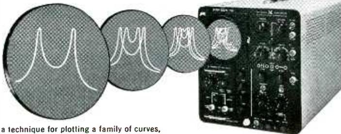
Illustrated: a technique for plotting a family of curves, representing a coupled circuit with varied parameters.
