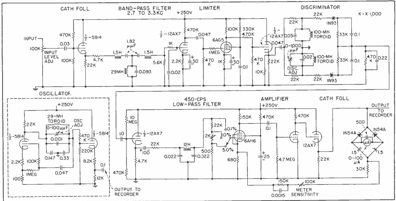
FIG. 1—Flutter and wow meter uses dual-tank discriminator with tanks tuned 300-cps on either side of 3,000-cps center frequency
