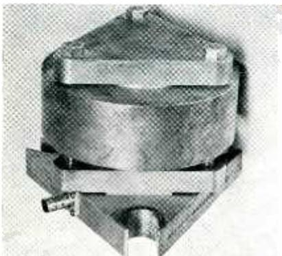
Large barium titanate velocity meter is bolted to structure being shock tested. It acts as a transducer to convert shock into an electrical signal
