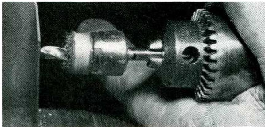
A COMBINATION drill and wire brush developed by Martin serves to drill holes and remove aluminum cladding from duralumin in one operation. This insures positive electrical connections when grounding airborne electronic equipment to aircraft structures, without need for an extra cleaning operation. The drill is mounted in the center of a standard wire brush.
