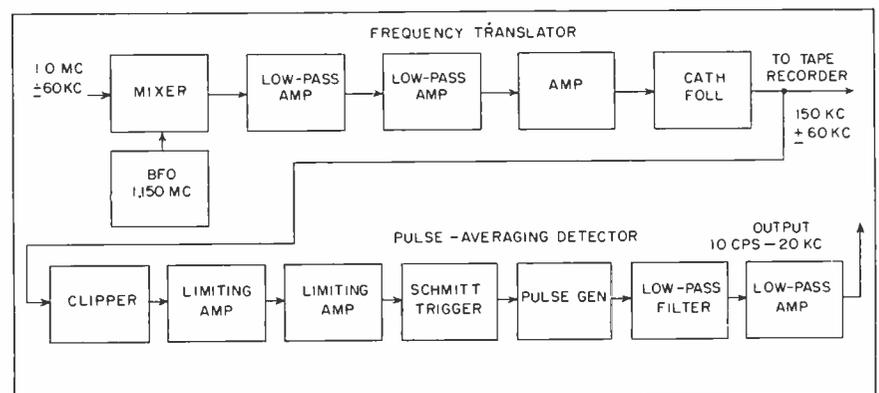
FIG. 1—Subcarrier translator and demodulator for tape recording of telemetered data
