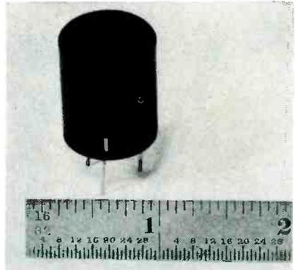
especially adaptable for printed circuit applications in that there are three leads which may be inserted with printed circuit boards and dip soldered.
