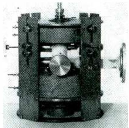
Aluminum-foil focus coils in use on Eitel-McCullough klystron here have less weight and lower power requirements than equivalent copper-wire coils
