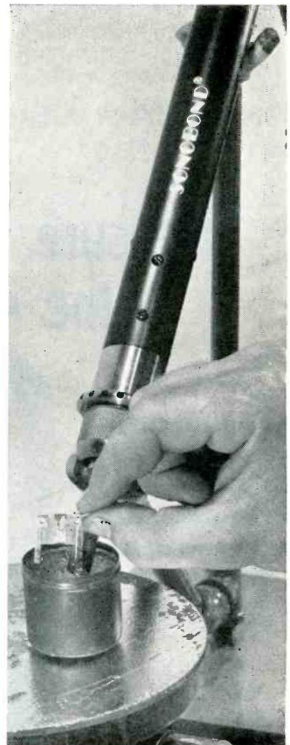
Each terminal of coil in turn is held against ultrasonic soldering head immersed in solder
