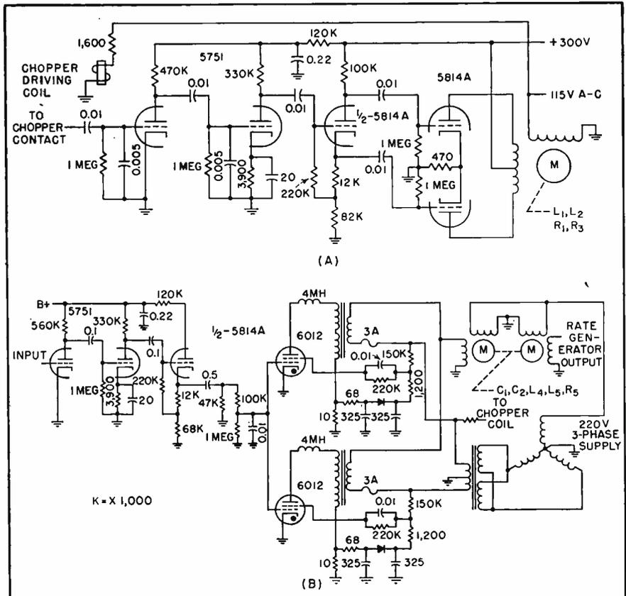
FIG. 6—Circuits of 1/2-watt (A) and 25-watt (B) servo amplifier systems
