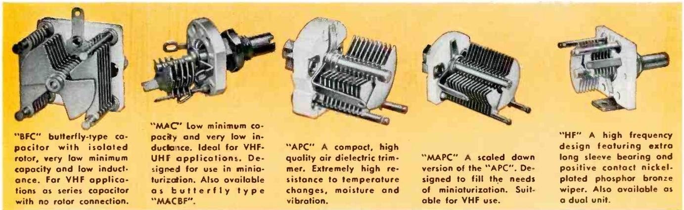
"BFC" butterfly-type capacitor with isolated rotor, very low minimum capacity and low inductance. For VHF applications as series capacitor with no rotor connection.
