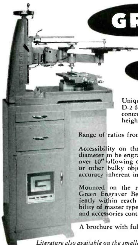
**GREEN****Model D-2****Pantograph Engraver**
