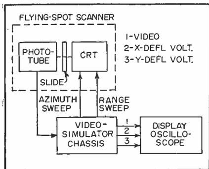
FIG. 1—Complete radar display system for three-dimensional presentation
