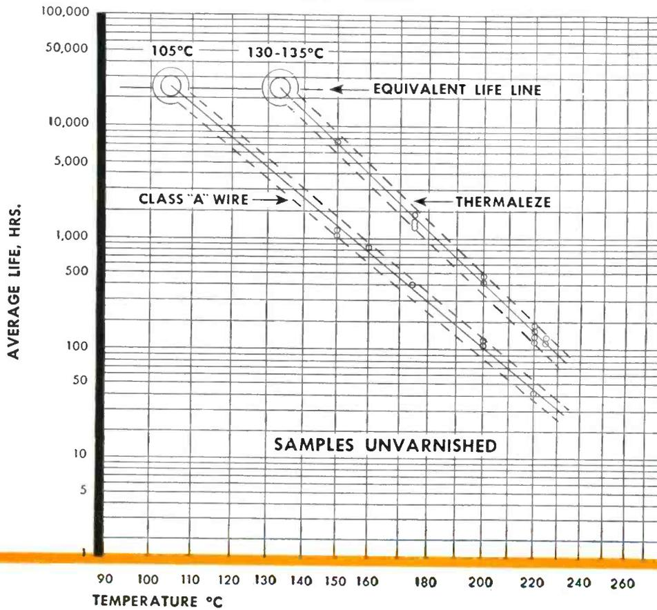
NEMA twist samples aged in oven at various temperatures following AIEE aging procedures
