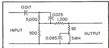
FIG. 2—Filter circuit for solid-circle curve
