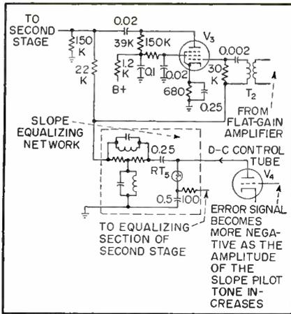
FIG. 4—Two slope-correcting amplifiers are used in cascade
