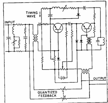
FIG. 4—Transistorized regenerative repeater produces results shown in Fig. 3
