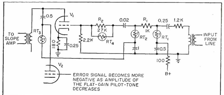
FIG. 3—Flat-gain regulator uses four thermistors
