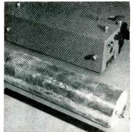
Aluminum-foil solenoid producing 850 gauss for focusing traveling-wave tube. At rear is solenoid housing complete with magnetic shield and cooling blower. Coil alone here is 12¾ inches long and weighs 12 lb
