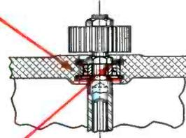
Bearing is held in position by two Waldes Truarc Rings—Standard (Series 5000) and Bowed (Series 5001). Two grooves are turned and housing rough bored in one operation. Alternate method would require at least two additional machining operations. Bowed Truarc ring takes up accumulated tolerances resiliently.
