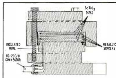
Cross-section drawing shows the four barium-titanate wafers that are the heart of the electromechanical transducer that was recently developed at NBS
