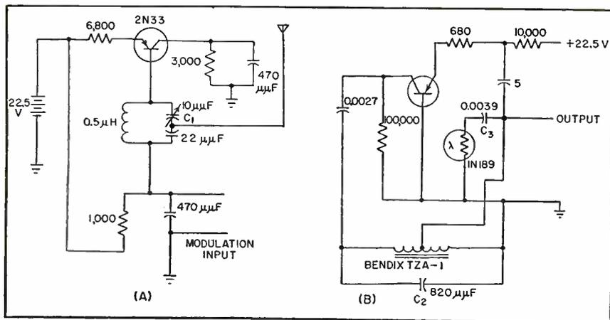
FIG. 1—Point-contact transistor r-f oscillator (A) and light-modulated subcarrier oscillator (B)
