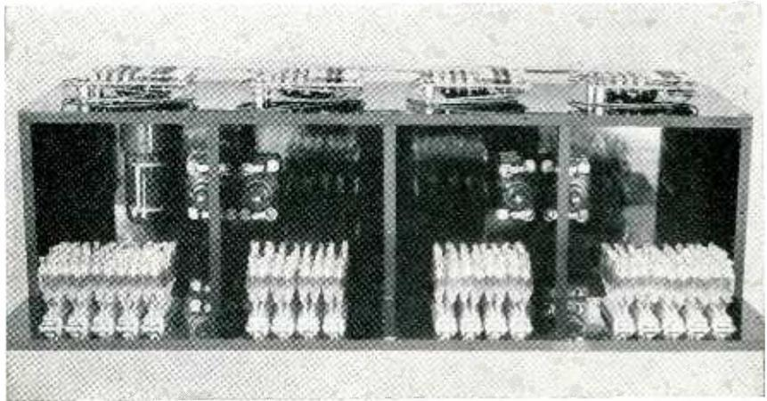
Memory matrix with light-tight cover open. Only one multiplier phototube is shown
