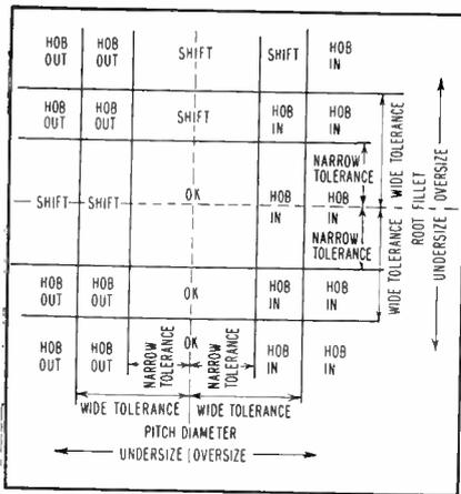
FIG. 4—Classification diagram showing method of classifying hobbing-machine errors according to observed defects
