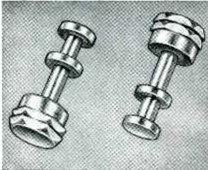
CAMBRIDGE THERMIONIC CORP., 445 Concord Ave., Cambridge 38, Mass., announces the first of a series of three new barbed and press mount terminals. These press mount solder terminals, designated series PM do not require riveting or swaging. They are designed to be press mounted into snug holes in all kinds of material, including laminated or cast material of 3/32 in. thickness or more.
