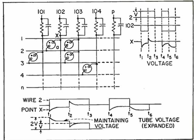
FIG. 2—Section of matrix and extinguishing waveforms
