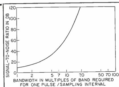
FIG. 2—Pulse-code modulation provides exponential signal-to-noise improvement with bandwidth
