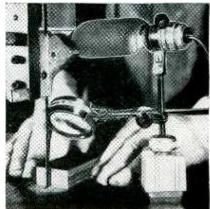
New production aid mounted on band saw helps operator follow fine scribed line precisely when cutting aluminum block
