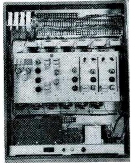
Electronic control cabinet. Hinged chassis at center drops forward to expose relays at rear. Main power supply is at bottom of cabinet
