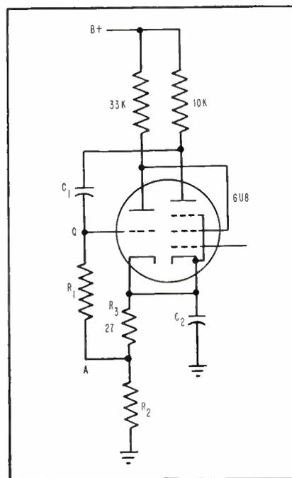
FIG. 1—Basic multivibrator-type circuit. Component values for free-running, one-shot and Schmitt trigger circuits are given in text
