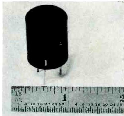
especially adaptable for printed circuit applications in that there are three leads which may be inserted with printed circuit boards and dip soldered.
