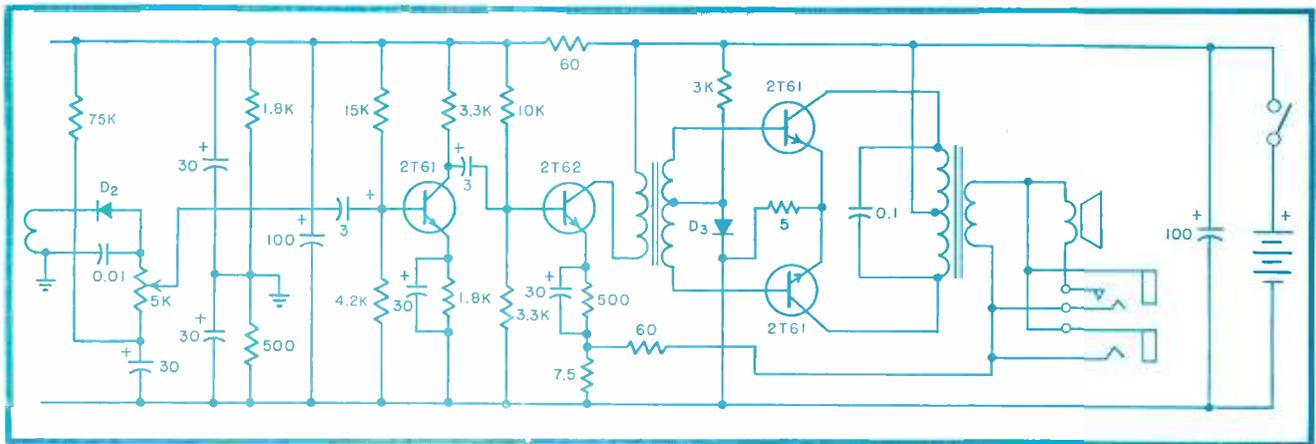
FIG. 4—Audio circuits of the seven-transistor receiver differ materially from those of the portable model
