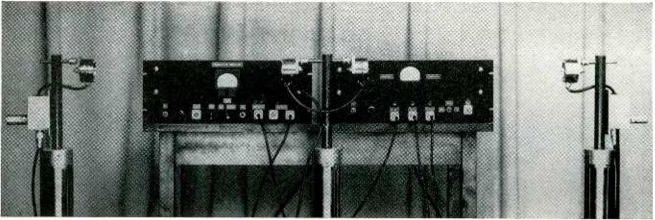
Multipath simulator with transducers spaced for delay of about two milliseconds. Transmitting transducers are on stand at center and the receiving transducers are on stands at left and right
