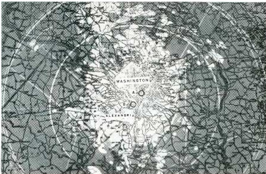
Ground clutter, the generally unwanted signal return from hills, trees and other low objects, has been put to use by the Signal Corps. Propagation maps, showing possible uhf signal paths, can be prepared by superimposing radar reflections upon terrain maps. The light areas shown above indicate good communications paths from a 147-foot tower at Washington National Airport
