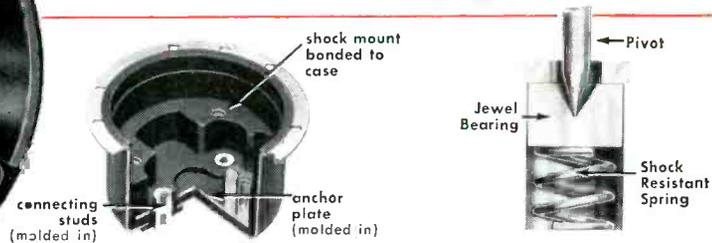
Cutaway view of instrument case, showing how the ruggedized WESTON movement is cradled on a shock mount of specially formulated rubber. Case is completely lined for high dielectric strength.
