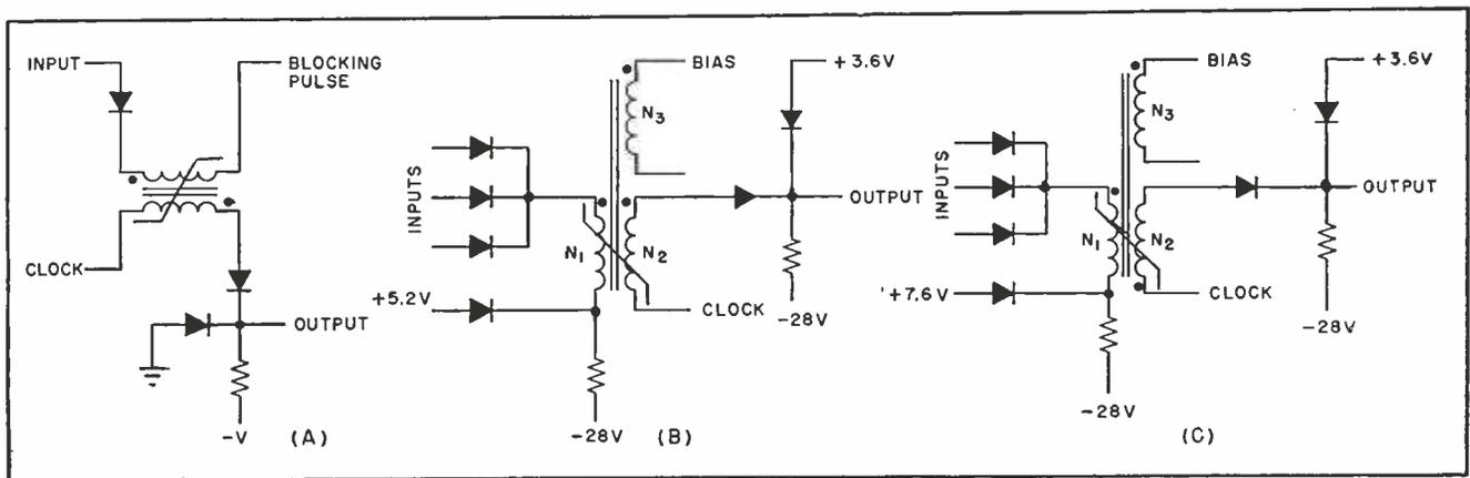
FIG. 1—Basic magnetic circuit is serial amplifier (A) which is used in complementing (B) and noncomplementing (C) amplifiers
