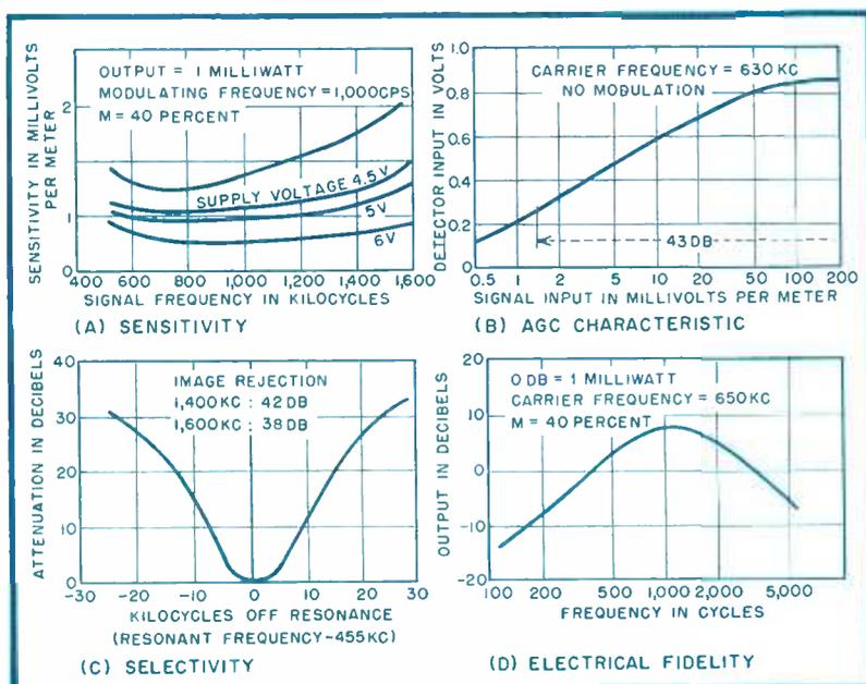
FIG. 3—Characteristics of the five-transistor receiver
