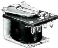
TYPE 15QA — Miniature relay, single pole. Nominal sensitivity .200 watts, available with solder terminals or printed circuit terminals, single hole mounting. Coil available to 60 volts DC.
