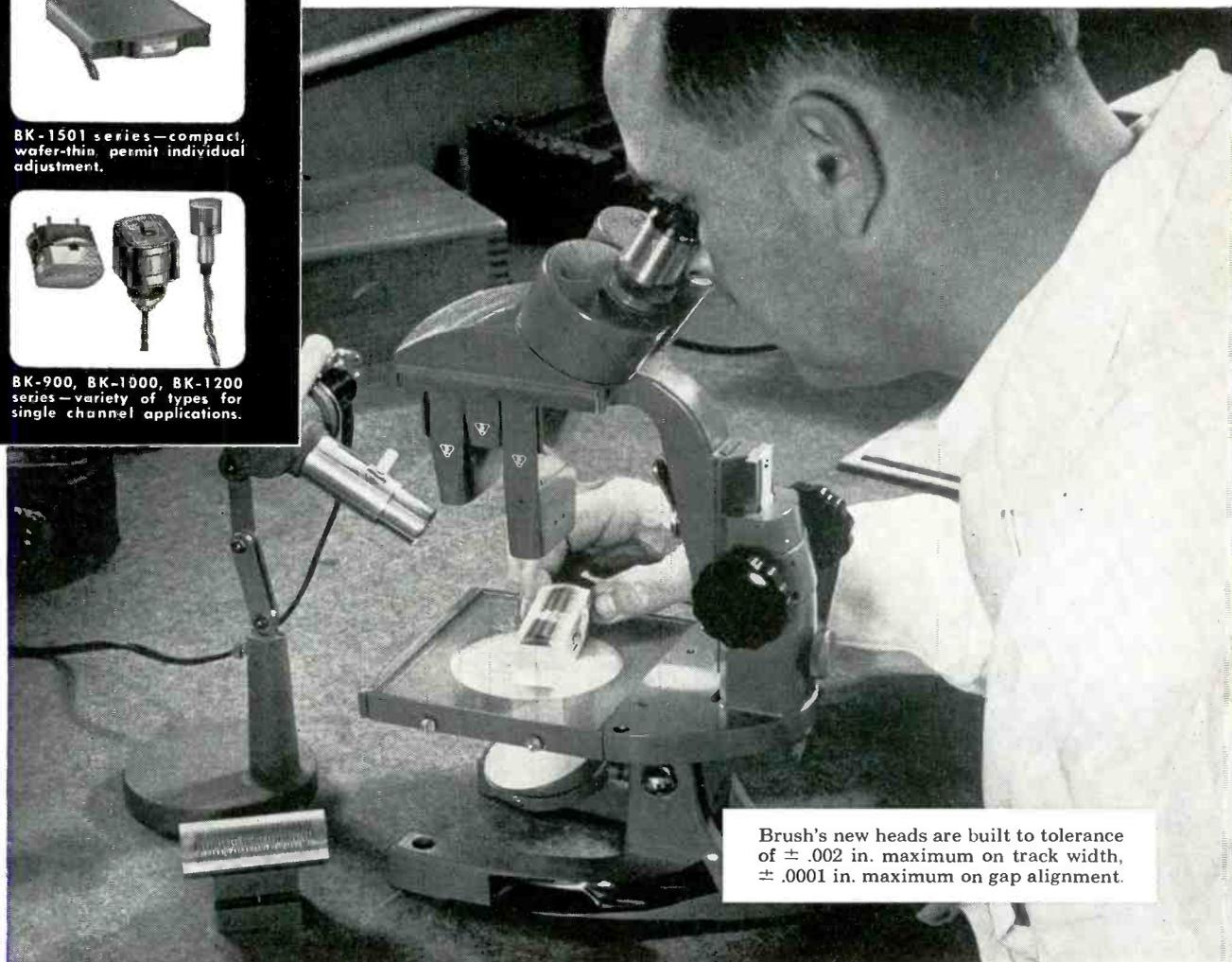
Brush's new heads are built to tolerance of  $\pm .002$  in. maximum on track width,  $\pm .0001$  in. maximum on gap alignment.
