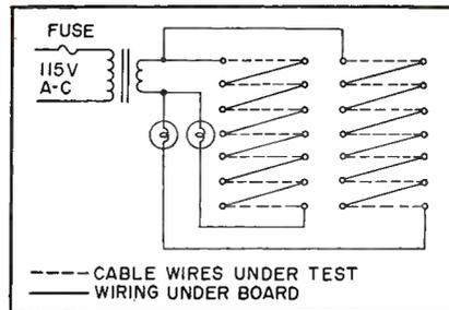
Twelve circuits identical to this are installed on board. Use of only two lamps per transformer permits use of small and inexpensive transformers under board
