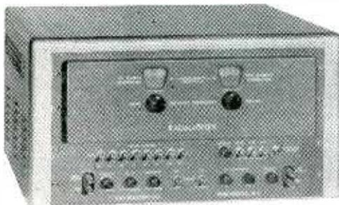
The Radaligner is a two-band sweeping oscillator designed to be used with a standard oscilloscope to determine frequency response of circuits from 10 to 170 mc. For frequency identification, the Radaligner includes eight narrow, customer-specified, crystal-controlled markers and a single variable marker covering both sweeping oscillator ranges. Center frequencies of sweep ranges also set to customer's requirements.
