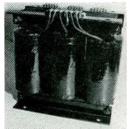
Experimental three-phase transformer wound with aluminum foil. On overload test, winding temperature reached 350°C without damage
