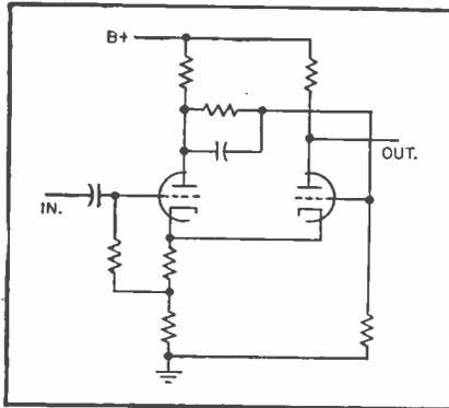
FIG. 4—Schmitt-type trigger used in timing generator
