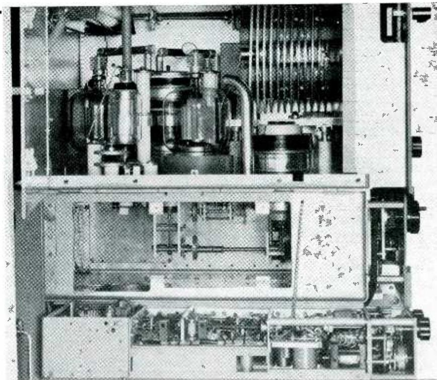
Twin-sideband transmitter is automatically tuned by setting exciter control to desired frequency
