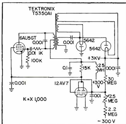
FIG. 2—Regulated high-voltage supply for storage-tube anode
