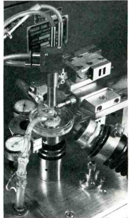
FIG. 3—Precision etching head, showing operator pushing work carrier into position. Outer housing has been removed for clarity
