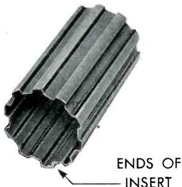
Six sizes of the corrugated inserts are necessary to fit the six sizes of miniature tubes. The seven-pin tubes require a certain corrugation height and three widths: for the small, medium, and large sizes. The nine-pin tubes require a different corrugation and three different widths: for small, medium and large tubes.
