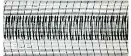
Output of Curtiss-Wright Distortion Eliminating Voltage Regulator from same input. Full recovery in 330 microsec.
