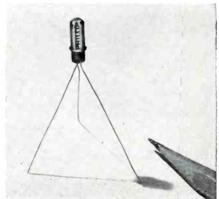
Example of transistor now in mass production, with pencil shown alongside for size comparison
