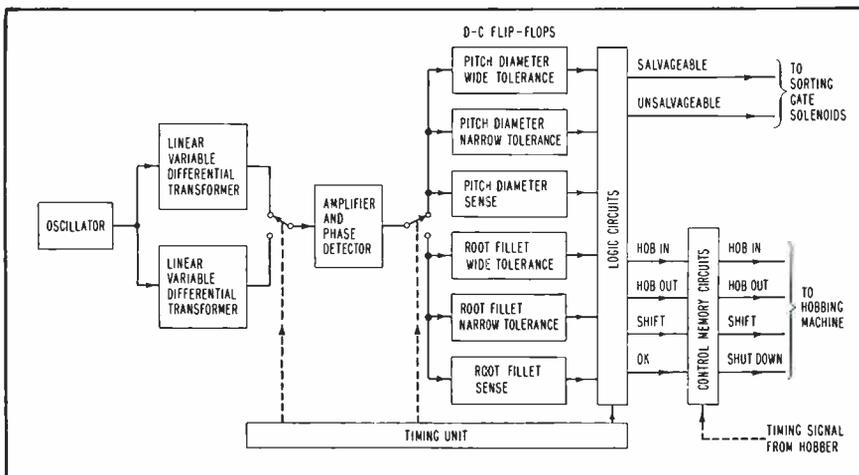
FIG. 2—Probes act on linear variable differential transformers of control system
