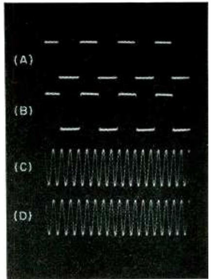
FIG. 6—Waveform of 500 cps signal before (A) and after (B) demodulation. Waveforms of 20-kc sine wave before (C) and after (D) demodulation
