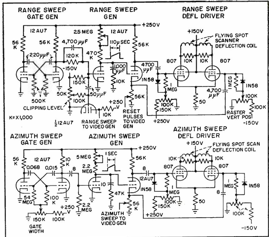
FIG. 6—Flying-spot-scanner sweep chassis generates range and azimuth sweeps
