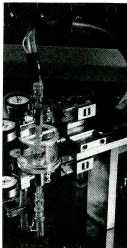
FIG. 4—Precision indium plating setup using jets for plating indium in etched holes on germanium. Dial gages serve for making precision head adjustments
