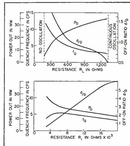
FIG. 5—Effect of changes of load resistance (A) and emitter resistance (B) on circuit performance
