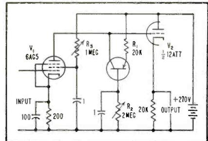
FIG. 2—Practical amplifier circuit uses transistor load stage followed by cathode follower
