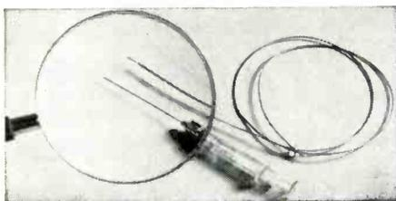
◀ **Nuclear reactors' temperatures measured**—Inconel® nickel-chromium alloy tube, almost as thin as a hypodermic needle, is both thermocouple unit and thermocouple protection tube. The Inconel tube resists oxidation, which might set up a heat barrier and interfere with accuracy of the reading. Photo courtesy of Argonne National Laboratory, Lemont, Ill.
