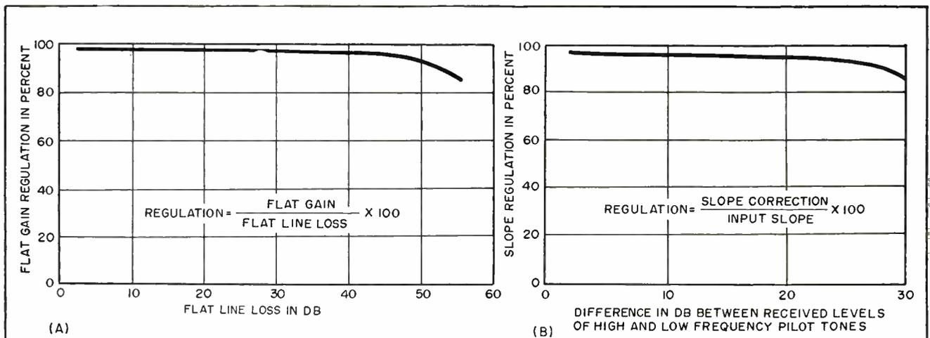
FIG. 5—Flat-gain regulation (A) and slope regulation (B) characteristics. Complete plug-in regulator comprises main chassis and four plug in units
