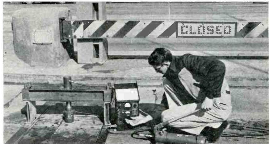
Accuracy of the electronic weighing mechanism used to determine load of trucks on turnpikes is tested with a hydraulic jack and load cell similar to that employed under scale platform. A series of weight readings obtained with the Baldwin-Lima-Hamilton SR-4 load cell is checked with those recorded in the toll booth
