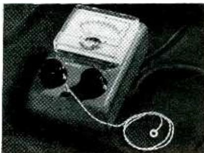
► Specifications—Scale ranges are 35 to 85 C and 95 to 185 F. Accuracy is  $\pm 1$  deg C with measuring unit within normal room temperatures. Battery life is approximately
