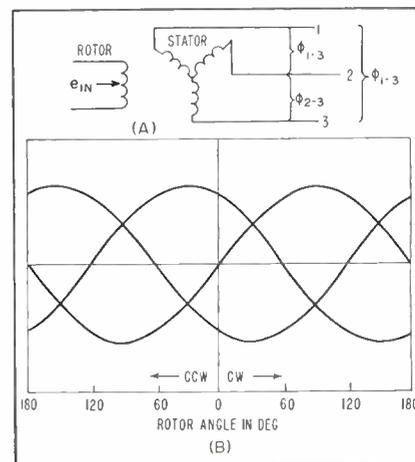
FIG. 1—Winding arrangement of synchro motor (A) provides 3-phase output (B) when sinusoidal signal is applied
