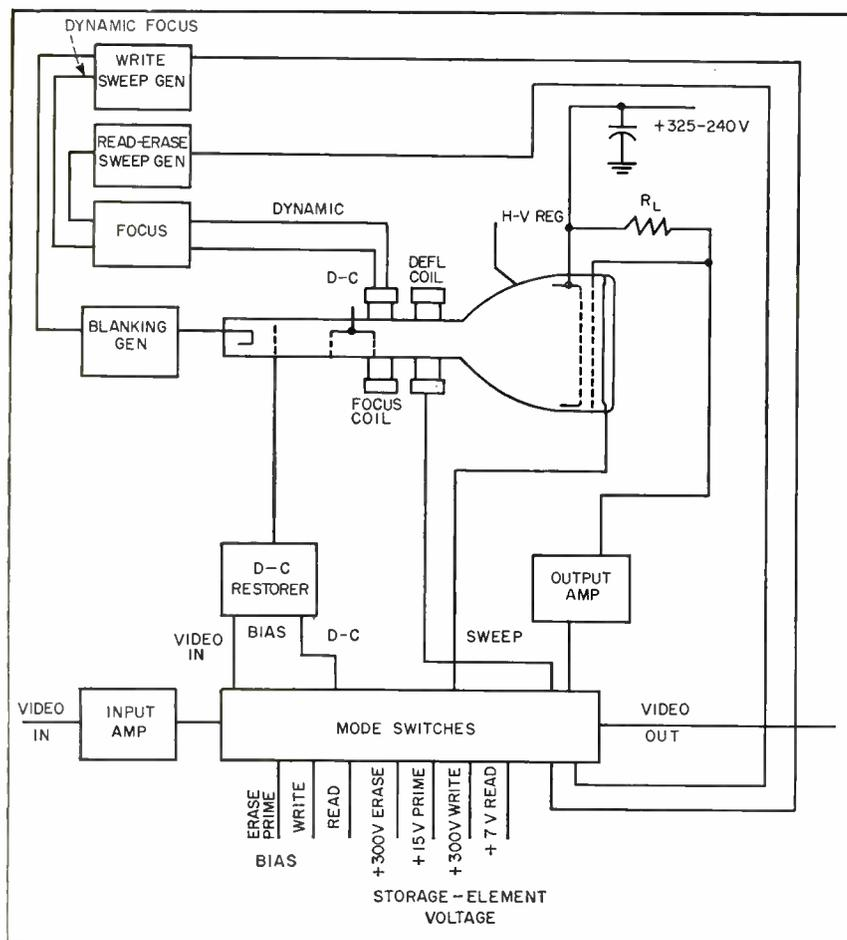
FIG. 1—Read, write and erase circuits used with recording storage tube
