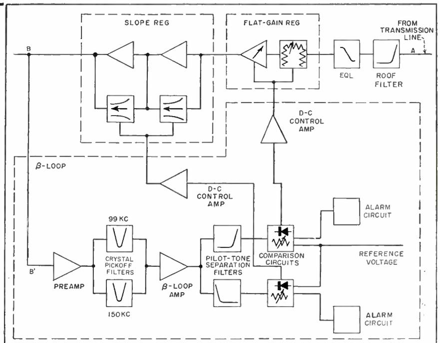
FIG. 2—Block diagram shows signal and pilot-tone paths
