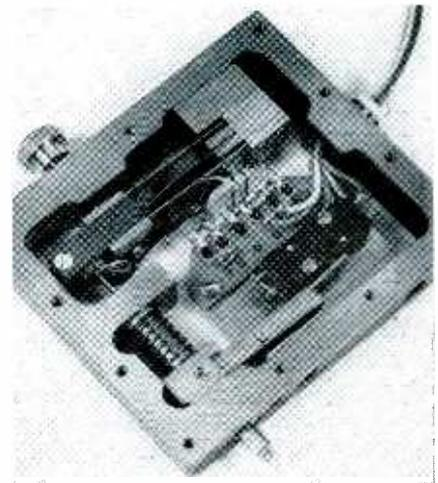
Interior of one of gaging heads. Probe is mounted on shaft projecting at bottom, which goes up to linear variable differential transformer mounted in plastic block supported by cantilever spring arrangement. Large knurled screw is zero adjustment for block
