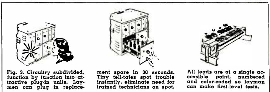
Fig. 3. Circuitry subdivided, function by function into attractive plug-in units. Laymen can plug in replacement spare in 30 seconds. Tiny tell-tales spot trouble instantly, eliminate need for trained technicians on spot.
