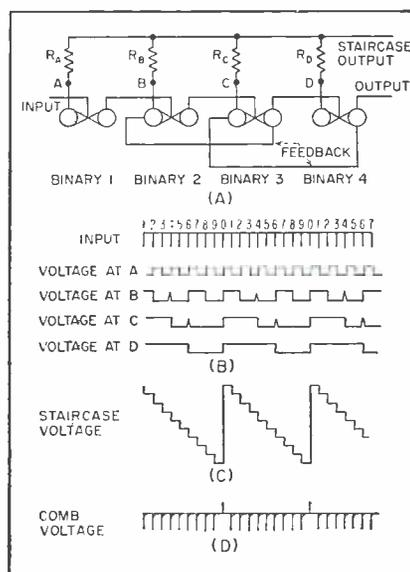
FIG. 5—Basic configuration of counter decade with staircase output (A) and waveforms (B, C and D)
