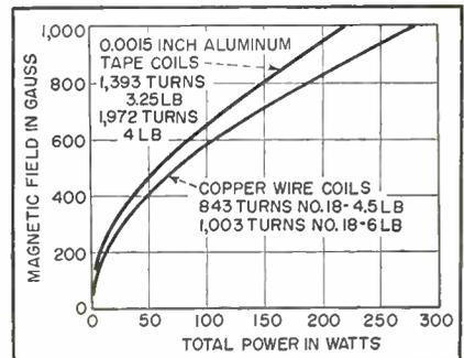
FIG. 1—Comparison of power requirements for copper-wire and aluminum-foil coils used for focusing a klystron. Data for curves was obtained in laboratory of Eitel-McCullough, Inc. Power saving with aluminum is due to better thermal conductivity within the aluminum coil
