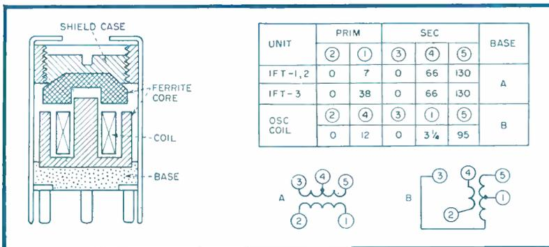
FIG. 2—Construction of i-f transformers and oscillator coil
