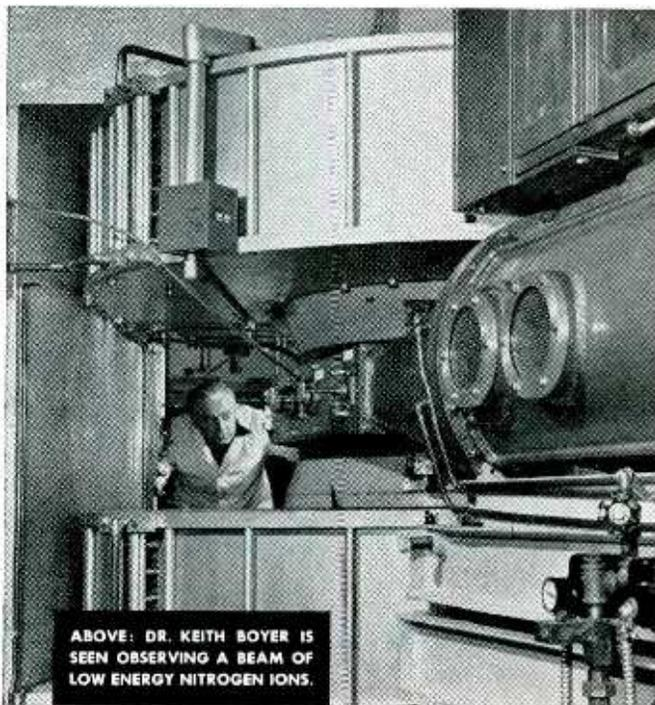
The cyclotron shown above is one of the many types of advanced research equipment in use at Los Alamos. This variable energy machine is designed to accelerate high intensity beams of all the hydrogen and helium isotopes.
