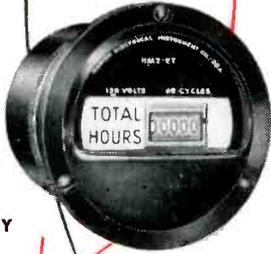
Glass-to-metal sealed ELAPSED TIME indicators. Compact, low cost, tamper-proof. Standard ASA-MIL dimensions, 2½" and 3½" sizes. Easy to read standard size counter registers 1/10 hour steps to 9999.9 or hour steps to 99999. Hermetically sealed. Shielded. Starts, operates continuously from -55° C. to +85° C. For 110-125 or 220-250 volt 50 or 60 cycle A.C.
