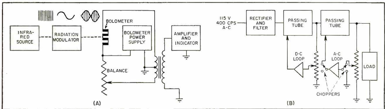
FIG. 1—Block diagram of test setup for infrared detector (A) and elements of the double-regulation power supply for bolometer (B)
