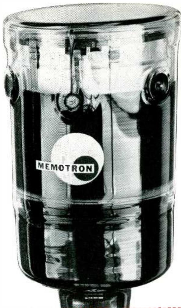
An application of the MEMOTRON is a commercial oscilloscope manufactured by Advanced Electronics Corporation, Los Angeles. MEMOTRON has an over-all length of 18 1/4 inches, and a neck diameter of 2 1/4 inches. It can replace most conventional 5-inch tubes without revision of space requirements in the equipment.
