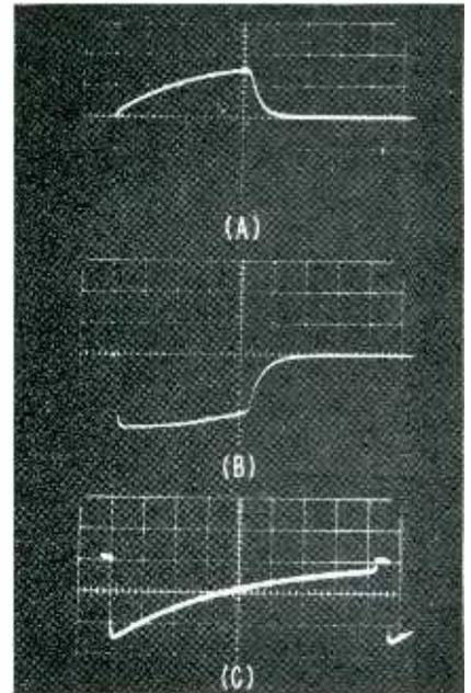
FIG. 2—Waveforms present at pentode plate (A), triode plate (B) and triode grid (C) in free-running circuit
