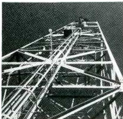
Instruments mounted on the 200-foot tower measure changing meteorological conditions during correlation tests on propagation ducts
