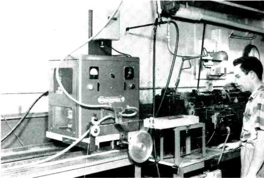
Reeve manufactures custom-made, high frequency heating equipment, including a device to eliminate hand retwisting and retraining of cut standard wire. It applies a high frequency pulse to the point at which the wire is to be cut, forming a solid bundle of the wire strands that resists the strain of cutting and stripping.
