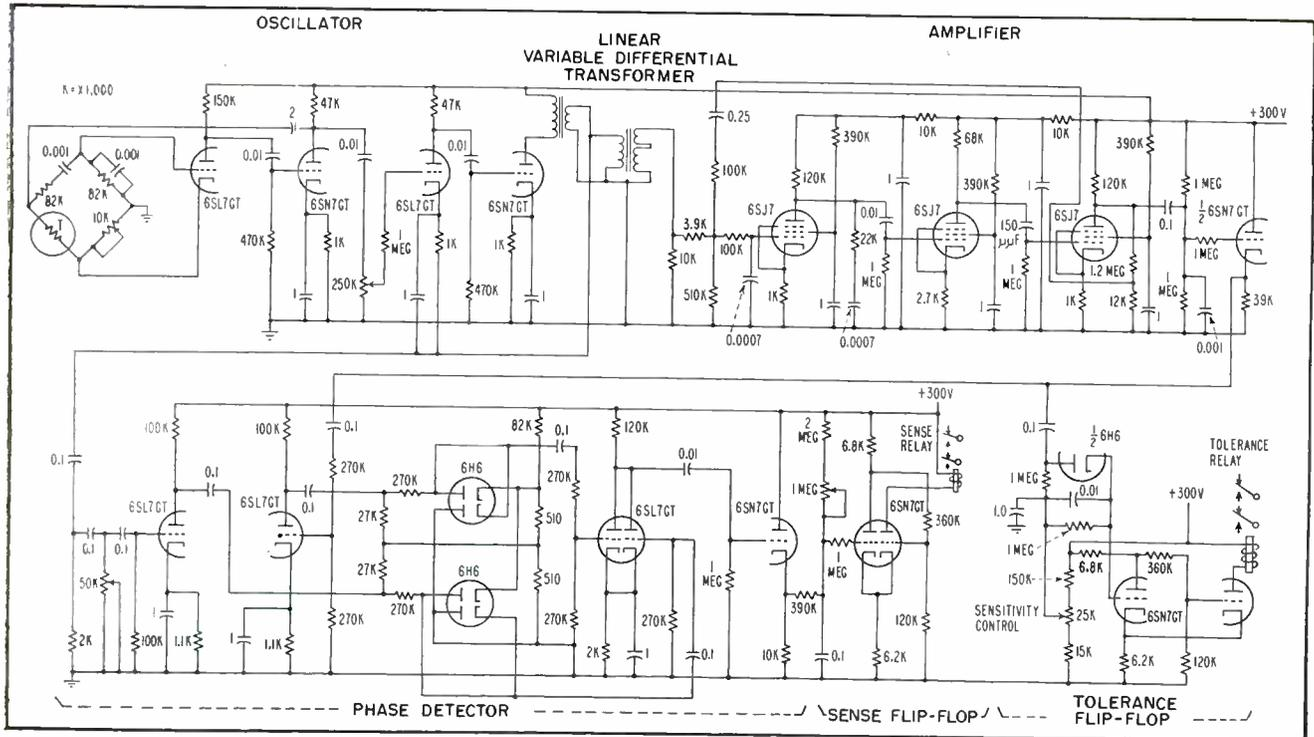
FIG. 3—Measuring circuit and two tolerance flip-flops. Other four tolerance flip-flops and other two sense flip-flops are identical
