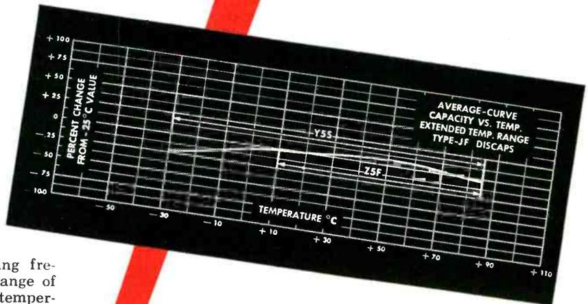
Type JF DISCAPS have outstanding frequency characteristics over a wide range of capacities and incorporate desirable temperature properties over an extremely useful range. Manufactured in capacities from 150 MMF to 10,000 MMF, Type JF DISCAPS extend the range of the RETMA Z5F capacitor between +10°-+85°C and meet Y5S specs from -30° to +85°C. (See graph)
