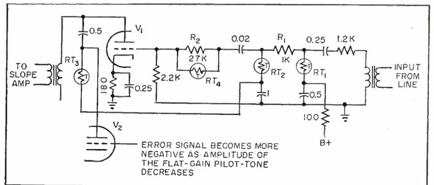
FIG. 3—Flat-gain regulator uses four thermistors
