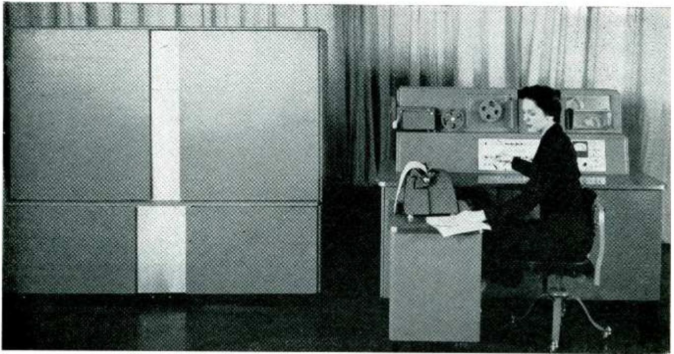
Installation comprises cabinet and desk-sized console. Input/output includes punched paper tape, typewriter and remote line
