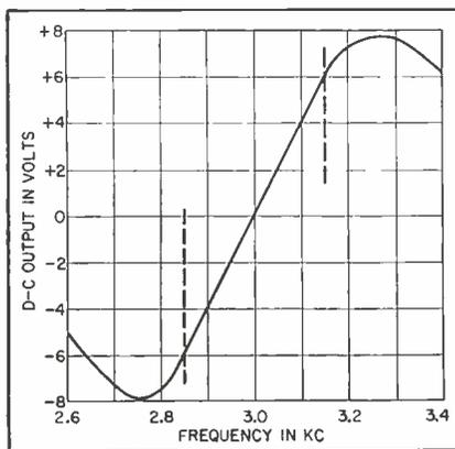
FIG. 2—Characteristic of dual-tank discriminator
