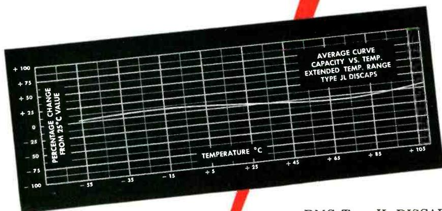
RMC Type JL DISCAPS feature exceptional temperature stability over an extended range. The maximum capacity change between  $-60^{\circ}$  and  $+110^{\circ}\text{C}$  is only  $\pm 7.5\%$  of capacity at  $25^{\circ}\text{C}$ . With a standard working voltage of 1000 V.D.C., Type JL DISCAPS are the ideal cost saving replacement for paper and general purpose mica capacitors.
