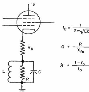
FIG. 1—Basic cathode trap circuit with design equations
