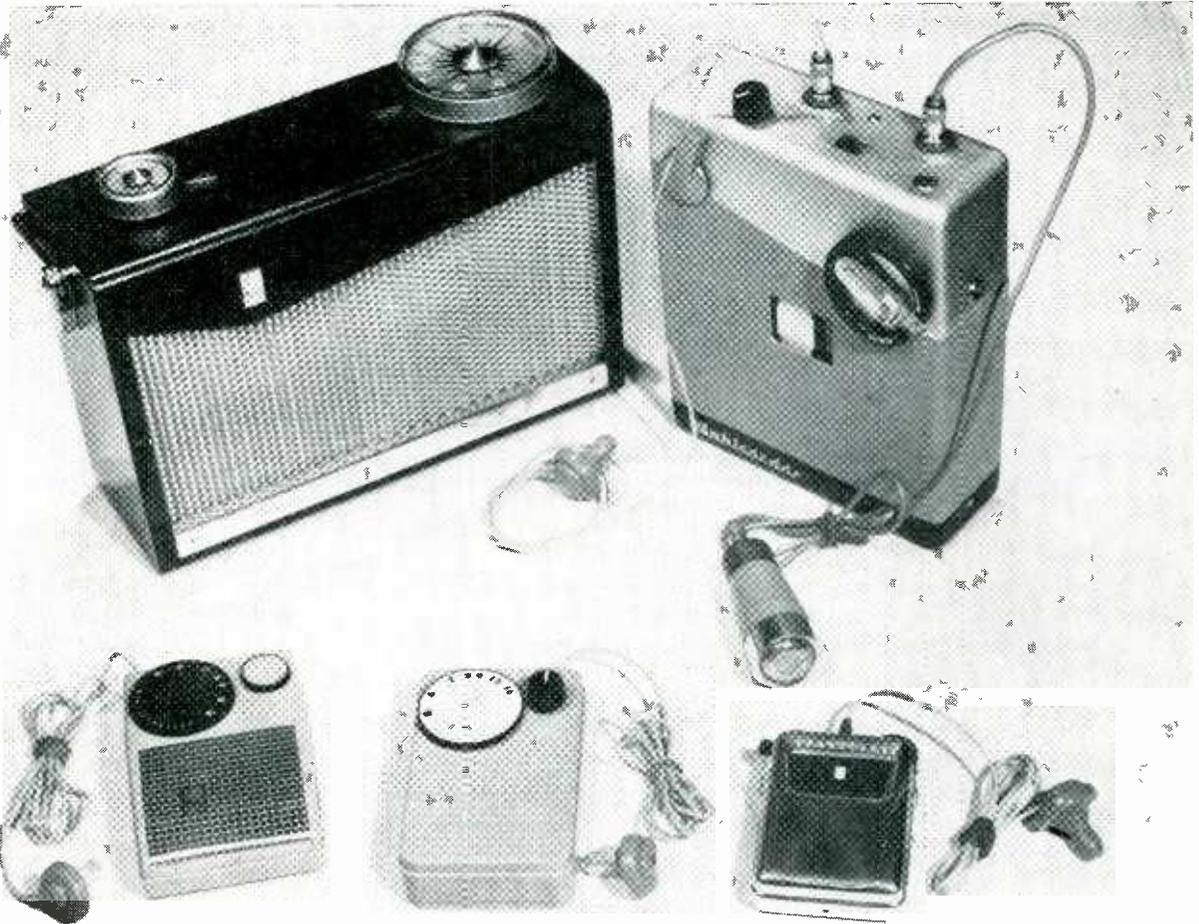
Transistorized products include a table-model receiver, battery-operated tape recorder, superheterodyne pocket receiver, regenerative pocket receiver and hearing aid. The portable receiver on facing page is not shown above
