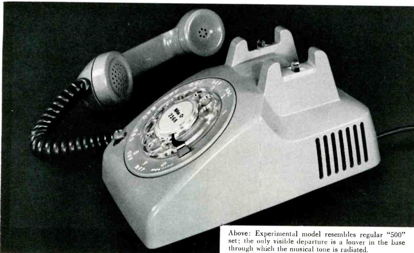
Above: Experimental model resembles regular "500" set; the only visible departure is a louver in the base through which the musical tone is radiated.
