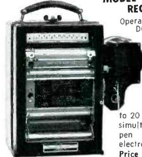
Operates on 24 volt DC. Chart speeds ranging from  $\frac{3}{4}$ " per hour to 6" per minute. Pens are electrically actuated. Instrument may have from 5 to 20 pens recording simultaneously. Each pen has separate electromagnet.
