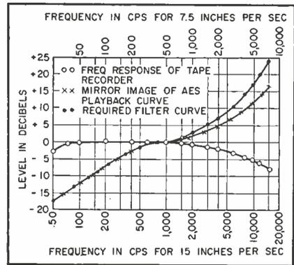
FIG. 1—Frequency response and filter compensation curves for combination tape-disk recording technique. Tape-recorder curve indicates frequency response obtained by recording at 15 inches per second (lower frequency scale) and playing back at 7½ inches per second (upper frequency scale). Use upper scale also for mirror-image of AES playback curve
