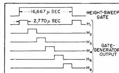
FIG. 8—Height gate generator output
