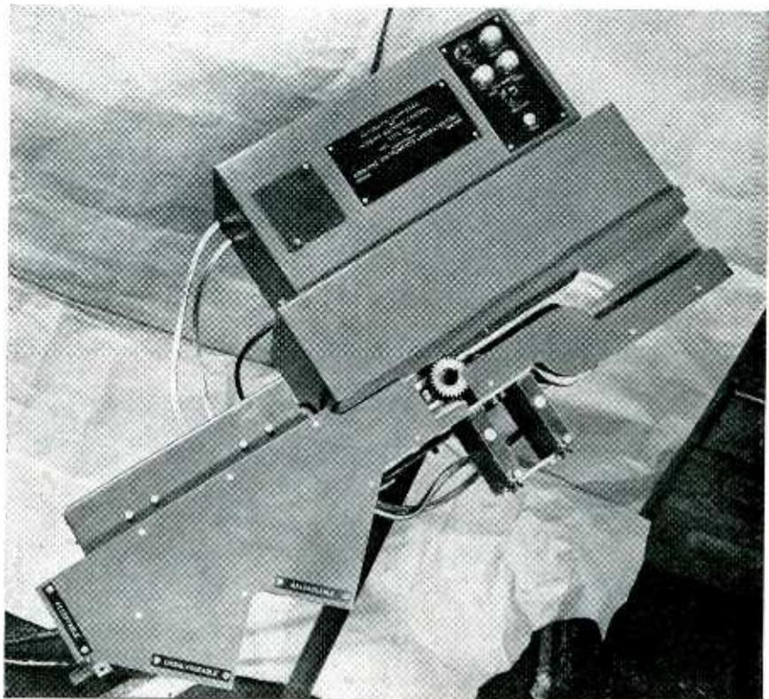
Sensing unit and sorting chutes of gear gage. Cables make interconnections with remotely located electronic control panel. Gear is in position for checking root fillet build-up. The three output chutes, for ACCEPTABLE, UNSALVAGEABLE and SALVAGEABLE gears, are at lower left
