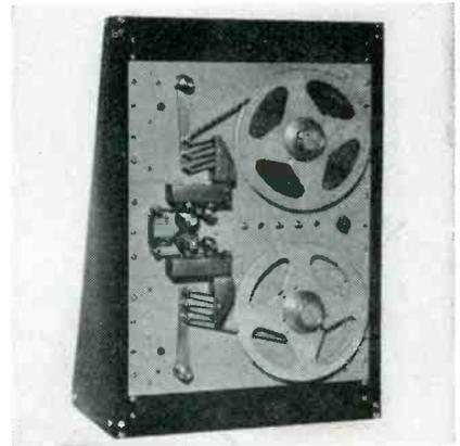
reliability for digital computing and data processing systems is provided by model 101 digital magnetic tape handler. Magnetic amplifier reel servos provide improved dependability, greater power output, and smaller size than the v-t amplifiers they replace.
