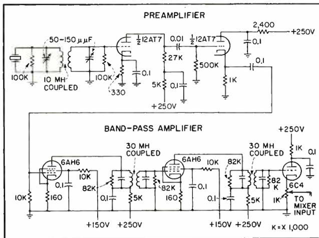
FIG. 3—Preamplifier-bandpass amplifier circuit for each delayed path boosts signal to 1-volt for mixing
