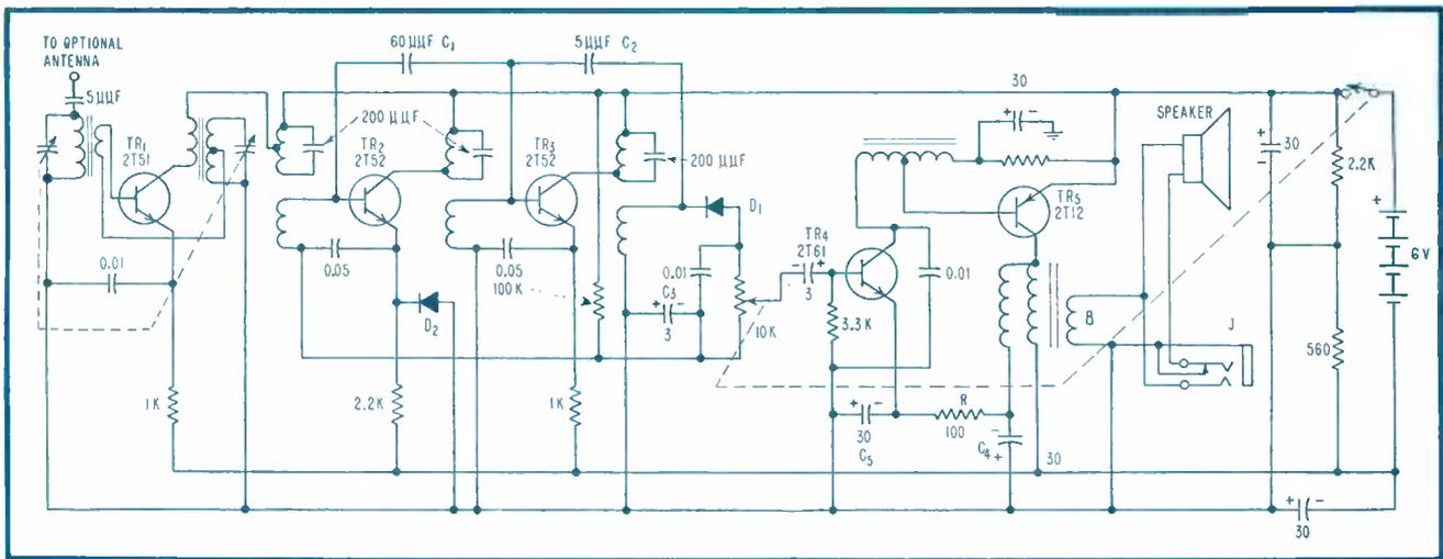
FIG. 1—Complete circuit of portable five-transistor Japanese receiver
