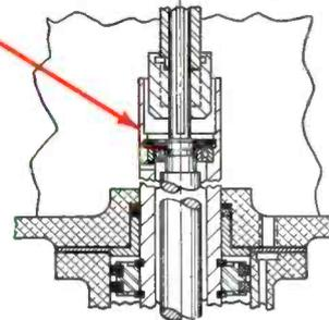
Easy assembly is assured by use of one Waldes Truarc Bowed Ring (Series 5001) to lock the bearing to the piston assembly. When unit is to be used in tapping applications, entire spindle assembly can be removed without disassembly.
