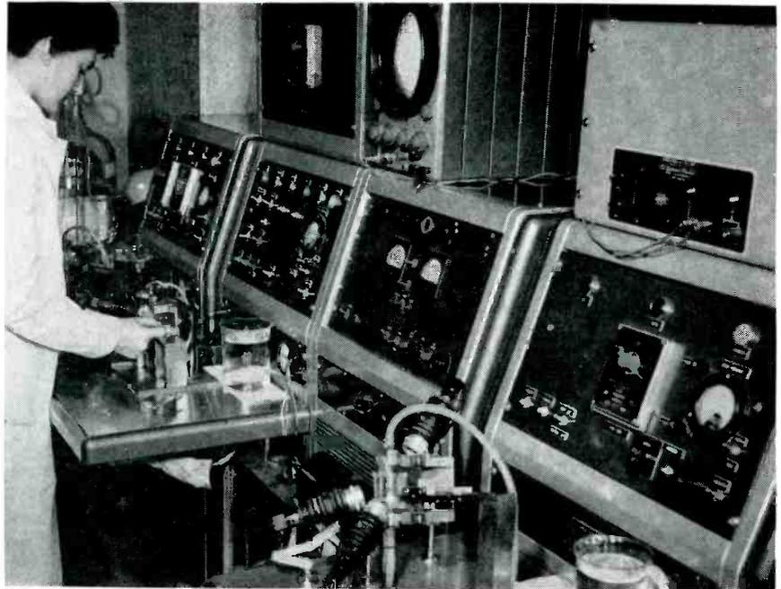
Battery of automatic etching machines producing surface-barrier transistors. Operator merely transfers work carriers from one setup to the next. These machines automatically etch concentric holes on opposite sides of the germanium pellet so the hole thickness remaining between them is less than 0.0002 inch, then plate the holes with indium
