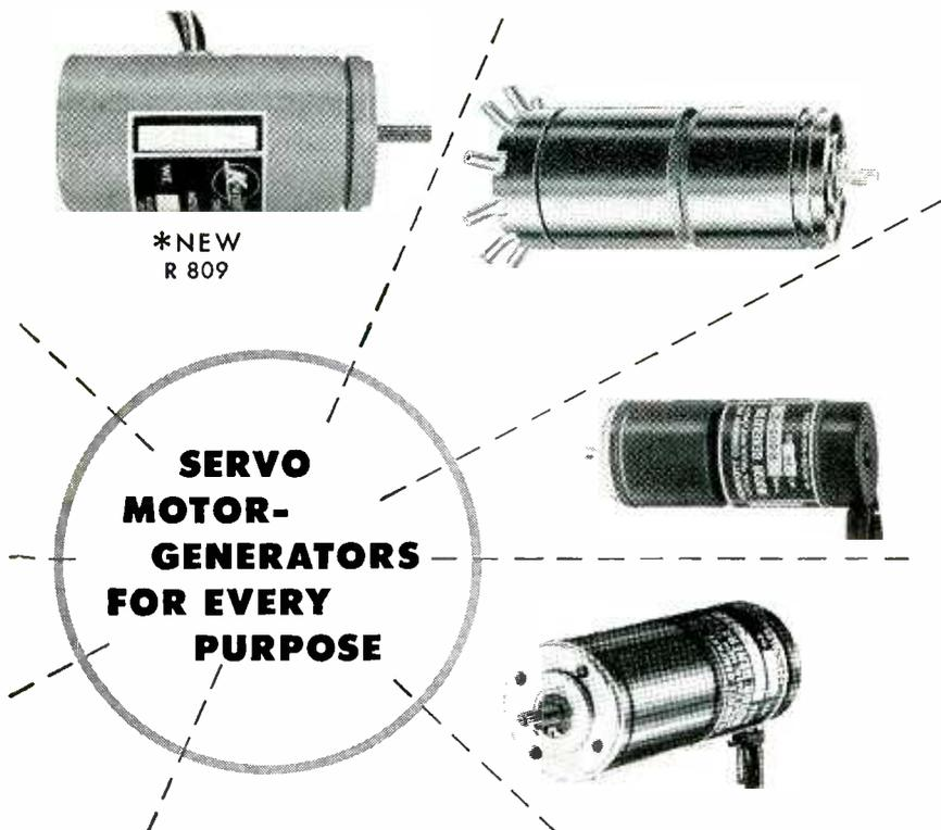
Kearfott Servo Motor-Generators are characterized by low rotor inertia, low time constants and high stall torque. Motor-Generator combinations provide 1/2 to 3.1 volts per 1000 R.P.M. with an extremely linear output over a speed range of 0—3600 R.P.M. and useful output up to 10,000 R.P.M.
