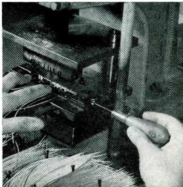
Spreading loops with pointed steel rod on handle. The seven different colors of insulated wire leads used are kept separated by long finishing nails driven into the bench
