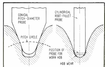
FIG. 1—How probes measure gear teeth
