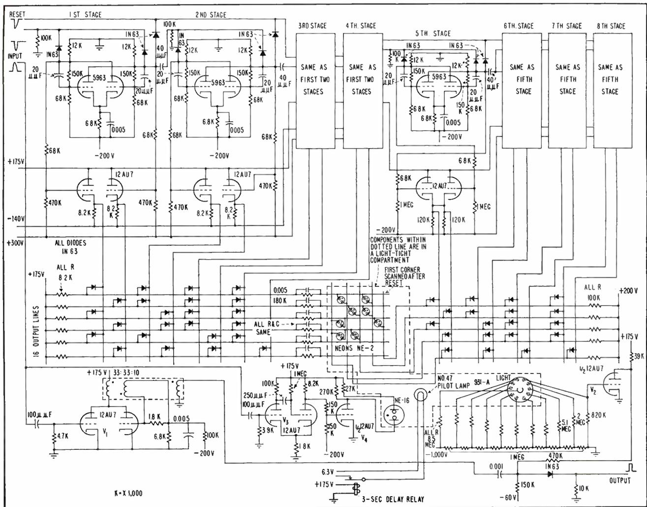
FIG. 4—Schematic diagram of neon-memory function generator
