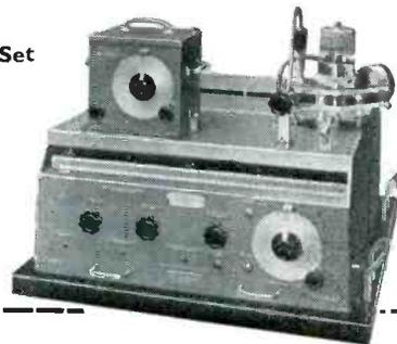
*In addition to the investigation of dielectrics, the high-frequency performance of resistors, capacitors, cables, etc., can be determined over a wide range.*
