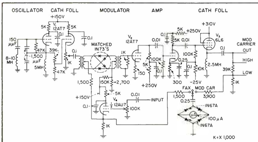
FIG. 2—Transmitter simulator provides modulated carrier output to drive sending transducer
