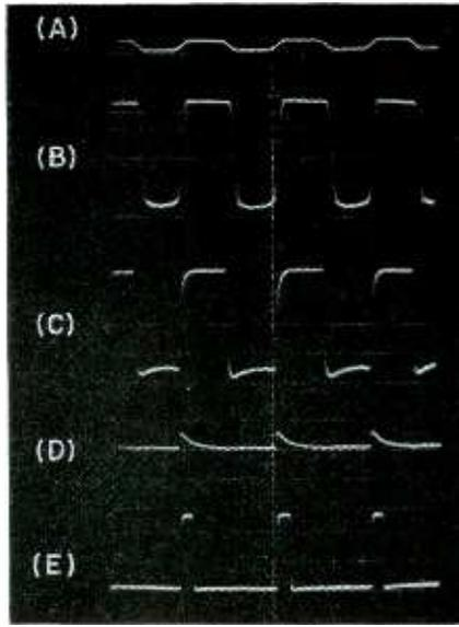
FIG. 5—Circuit waveforms at output of clipper (A), limiting amplifier (B) and trigger circuit (C). Pulse generator trigger (D) provides standard-pulse output (E)
