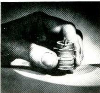
**ONE** of a new series, the Eimac ceramic receiving tube shown in the photograph is being made as a dual triode and pentode. Such a tube can withstand 15-g acceleration at frequencies up to 2,000 cycles. The tube is undamaged at envelope temperatures up to 300 C. Electrical terminals in the form of flat tabs facilitate incorporation of the tube as part of automatically produced circuit modules
