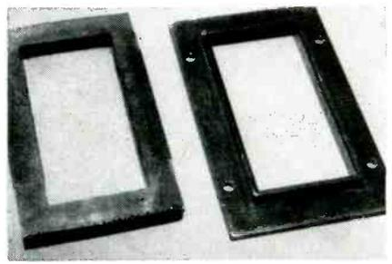
Finished steel waveguide flange for radar t-r tubes used for low-frequency scanning, at right, was coined in heavy presses from blank shown at left
