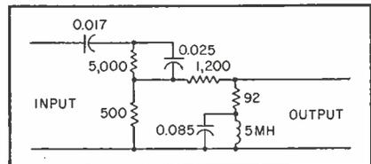
FIG. 2—Filter circuit for solid-circle curve
