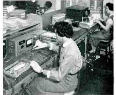
Each unit, from start to finish, is checked at least 5 times for voltage and capacitance before being shipped. In this step, capacitors are tested at DC voltages at least 200% of rated voltage at 25°C.
