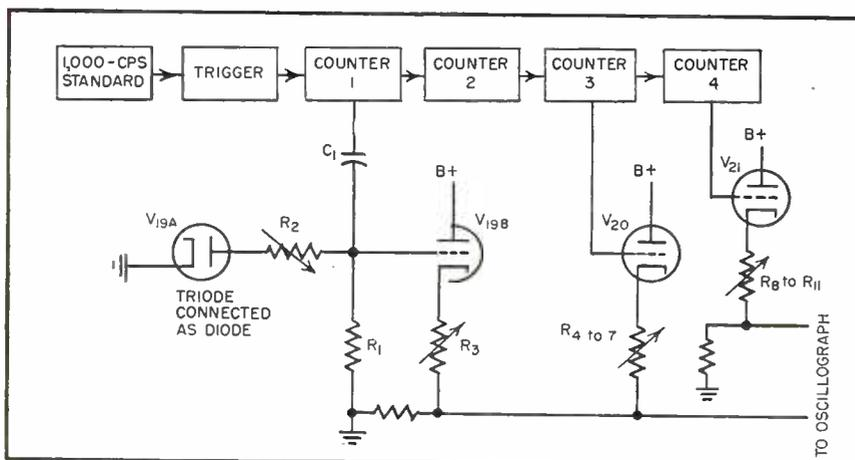
FIG. 2—Simplified diagram of timing generator; component designations correspond with complete circuit diagram, Fig. 3
