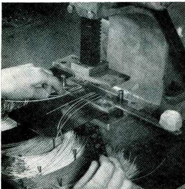
Loading wires into press. Stripped ends of wires go into holes at rear of slots in floating bed of press. Padded handle at right moves pointed steel rod used for spreading loops
