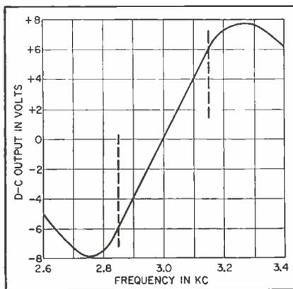
FIG. 2—Characteristic of dual-tank discriminator
