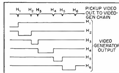
FIG. 7—Video generator chain output
