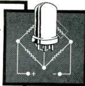
An Edison Sensitive D. C. Relay and an ordinary bridge circuit are versatile tools in solving temperature control problems.
