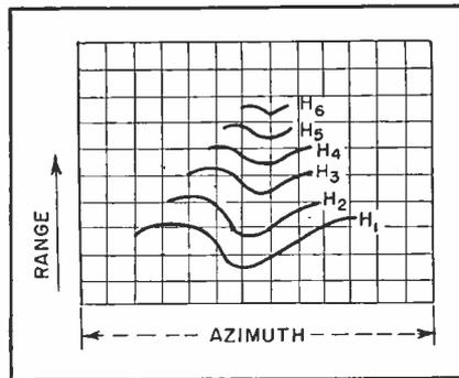
FIG. 2—Typical terrain-contour-line slide for flying-spot scanner
