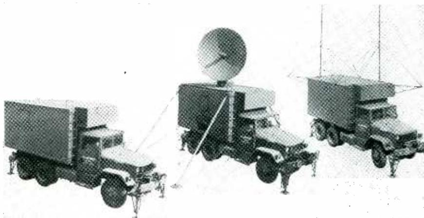
Computer, radar and radio vans, left to right, can go by plane as . . .
