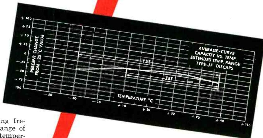
Type JF DISCAPS have outstanding frequency characteristics over a wide range of capacities and incorporate desirable temperature properties over an extremely useful range. Manufactured in capacities from 150 MMF to 10,000 MMF, Type JF DISCAPS extend the range of the RETMA Z5F capacitor between  $+10^{\circ}$ – $+85^{\circ}\text{C}$  and meet Y5S specs from  $-30^{\circ}$  to  $+85^{\circ}\text{C}$ . (See graph)
