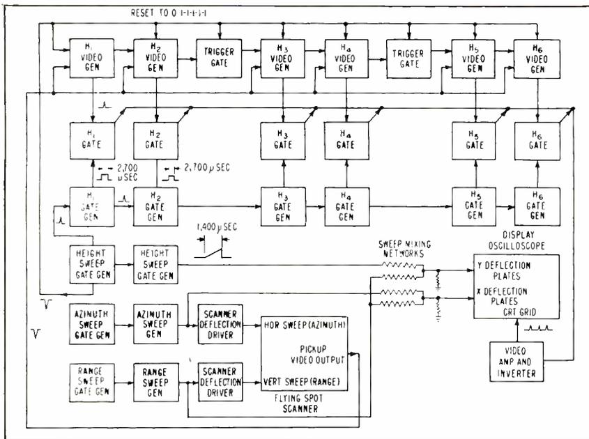
FIG. 4—Block diagram of radar-video simulator equipment
