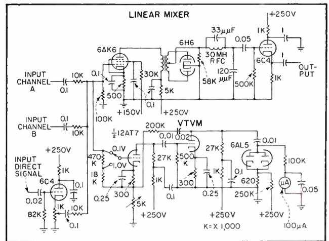
FIG. 4—Inputs from two delayed paths and direct path are combined and demodulated to drive recorder
