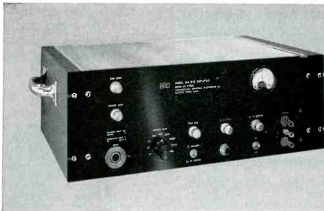
For voltage gain from transducers of all kinds, use the Model D-1. It will drive a 'scope, direct-writer, oscillograph, or magnetic recorder.
