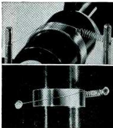
A new concept of slip ring brush design has shown life better than 100 million revolutions at low electrical noise level. A self-contained spring and wire contacts slip ring over a sector of approximately 180°. Size of wire used in tests, .004-.006 diam., with wear at end of 100 million revolution test less than one-half diameter. Write for information.
