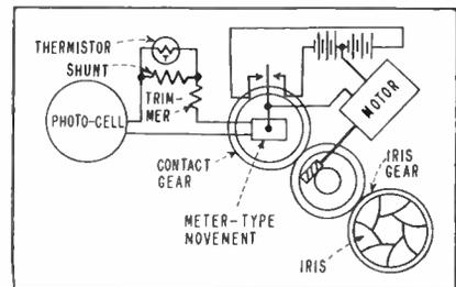
Circuit diagram of the photocell-actuated iris
