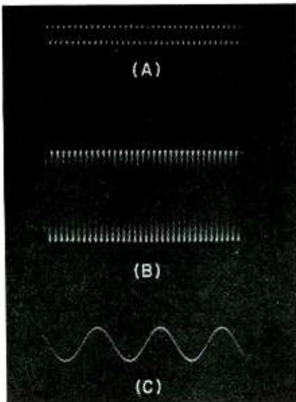
FIG. 4—Unmodulated subcarrier (A) is combined with bfo output (B) to give translator output (C) for frequency-modulation magnetic-tape recording
