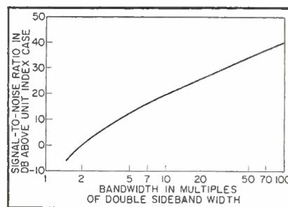
FIG. 1—Exchange of excess bandwidth for improved signal-to-noise ratio with frequency modulation
