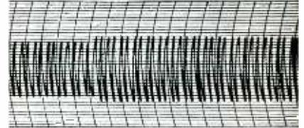
Output of typical electromechanical regulator in response to step change in input voltage. Average correction rate of 6v. per sec.
