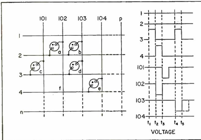
FIG. 1—Section of neon-tube matrix and firing waveforms
