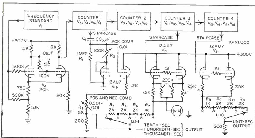
FIG. 3—Complete circuit of timing generator. Frequency standard and decade counters, represented by blocks, are commercially available plug-in units
