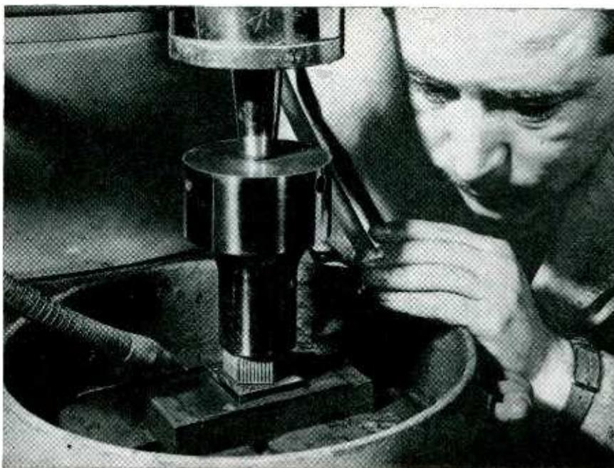
Dicing 271 disks of germanium from thin slab in one operation, using stainless steel cutters on ultrasonic machine tool. Abrasive particles in water suspension are directed across work by two hoses
