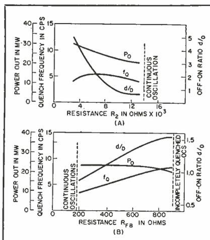
FIG. 4—Effect of changes in bias (A) and feedback (B) on circuit performance. Sum of  $R_2$  and  $R_3$  held constant in (A)
