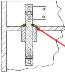
A Single Waldes Truarc External Retaining Ring (Series 5100) acts as shoulder, holds the lever in position. Labor savings are tremendous—a simple groove cutting operation replaces turning a shoulder, grinding and polishing.
