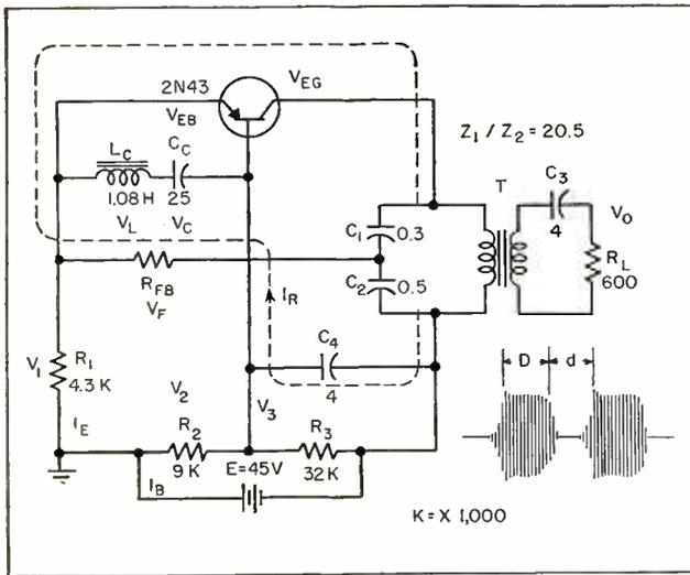
FIG. 1—Self-quenching superregenerative oscillator circuit uses junction transistor. Point contact may also be used
