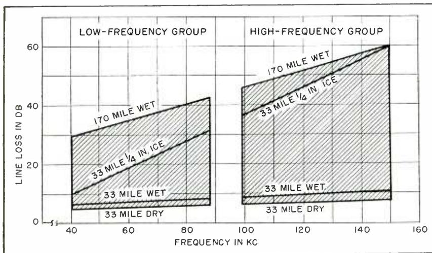
**FIG. 1**—Attenuation characteristics of open-wire line. Shaded portions show range of regulation of the equipment described in text
