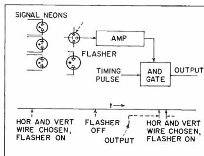
FIG. 3—Output circuit and timing cycle
