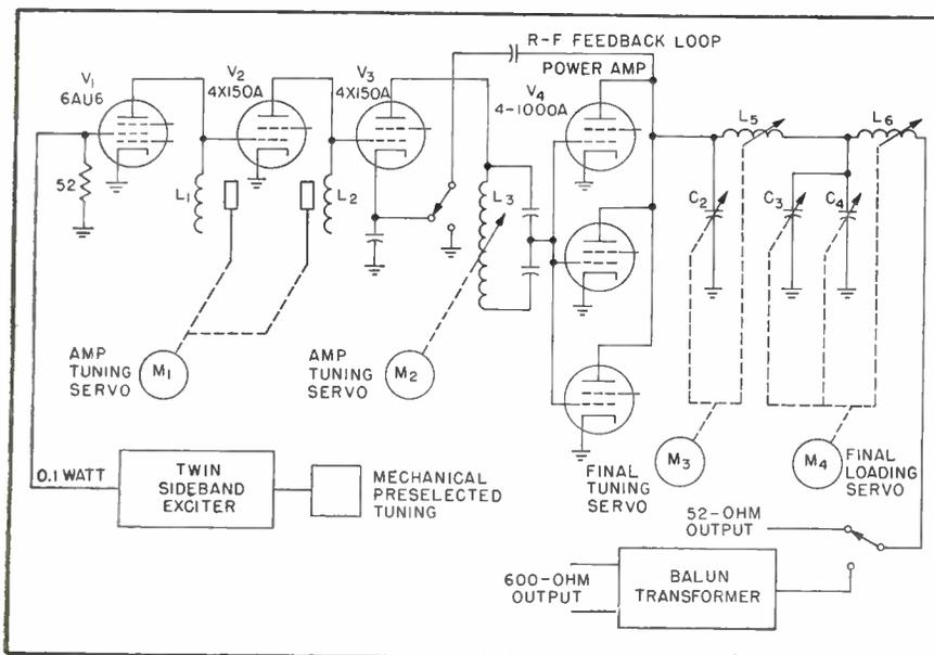
FIG. 1—Simplified diagram of r-f amplifier shows stages tuned by servo system
