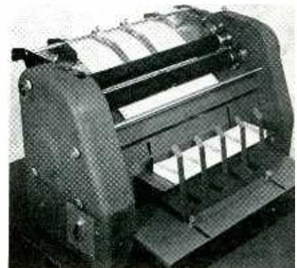
Office forms of varying length can be quickly processed using a forms burster that separates sections along a perforated line. Twenty-three different lengths from 3 to 22 inches can be selected by electronic timing in a machine recently developed by Standard Register
