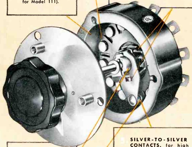
**"DEAD" SWITCH SHAFT.** Completely insulated from the load by a high-strength driving hub which will withstand a 2000-volt test.
