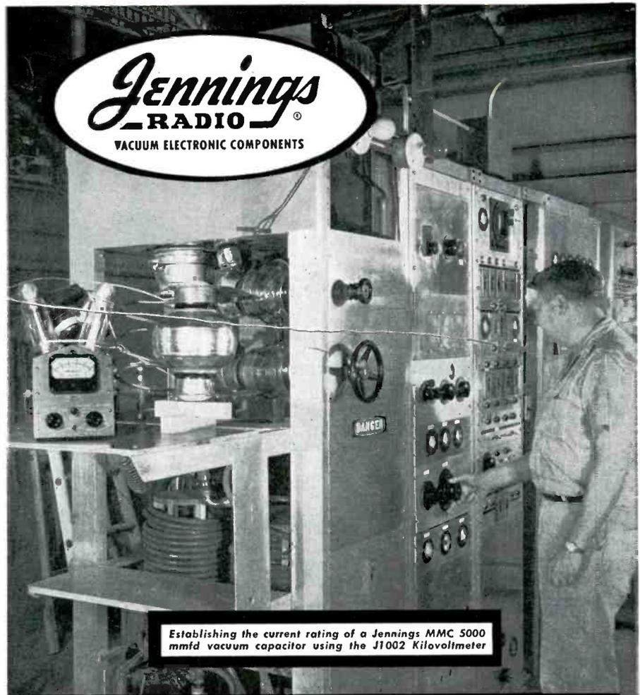
Establishing the current rating of a Jennings MMC 5000 mmfd vacuum capacitor using the J1002 Kilovoltmeter
