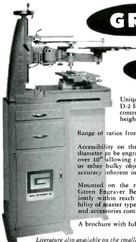
**GREEN****Model D-2****Pantograph Engraver**
