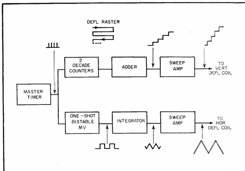
FIG. 6—Staircase raster generator for transmitting information in fast bursts
