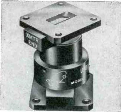
loads. It is essentially a modified polarization circulator employing permanent magnets and containing two sets of integral external dummy terminations. The external loads are capable of handling higher powers than internal types and also make possible the short length of 2.25 in.
