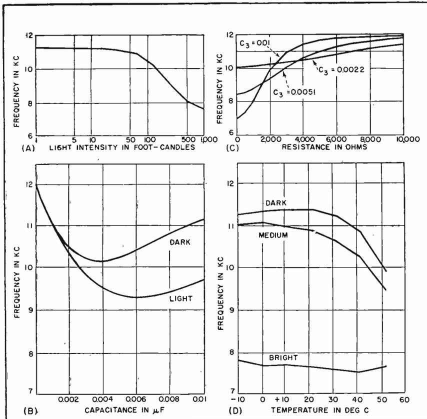
FIG. 2—Performance of subcarrier oscillator with frequency plotted against light intensity (A), capacitance in series with photocell (B), resistance of photocell (C) and temperature (D)
