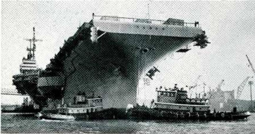
Newly commissioned *U. S. S. Saratoga* uses the latest electronic devices to improve detection and fire control besides furnishing navigational signals and communications to aircraft. Barrel-shaped structure at top of mast (left) is enclosed Tacan navigation-aid
