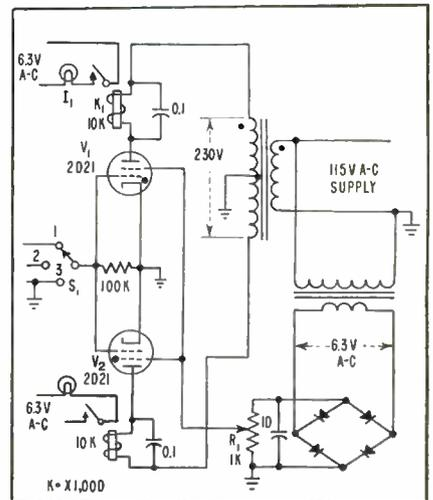
**FIG. 2—Phase detector for determining independent null points in synchro alignment**
