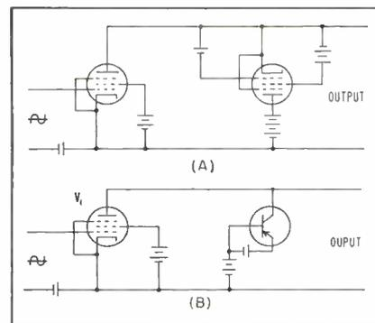
FIG. 1—Pentode gain increased (A) by using another as load impedance. Pentode load is replaced by transistor (B)
