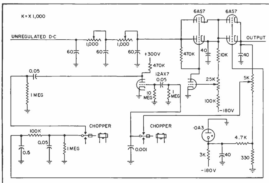
FIG. 2—Circuit diagram shows choppers used to generate and rectify a-c signal that compensates low-frequency variation
