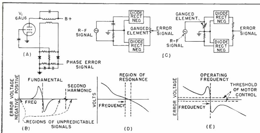
FIG. 2—Discriminator (A) with sharp response curve (B) is combined with R-C discriminator (C) with broad response (D) to obtain wide range with critical null (E)
