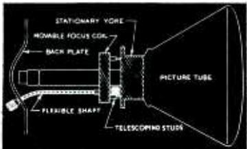
Mounting controls in convenient operating positions is easier when a flexible shaft is used as the coupling. The shaft allows the control to be mounted wherever desired.
