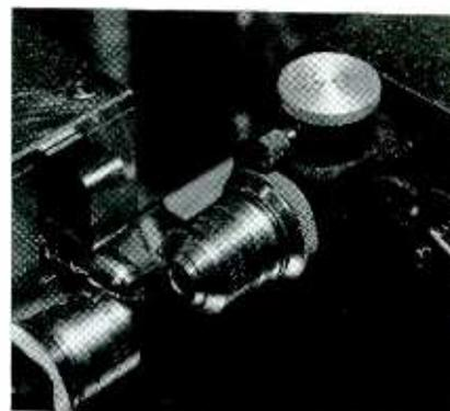
FIG. 7—Transistor in position between dual microscope lenses of concentricity checker
