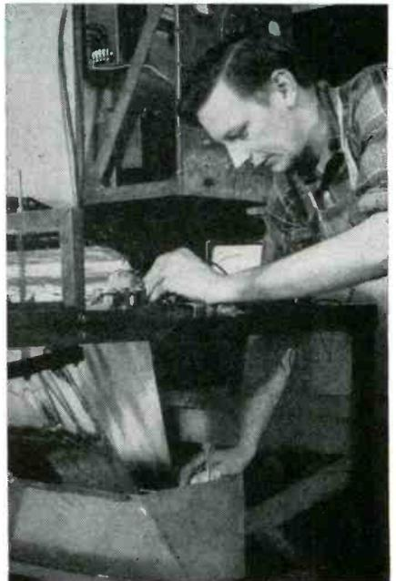
Test setup for foil coating and winding. Power supply for producing anodic coating is on overhead rack
