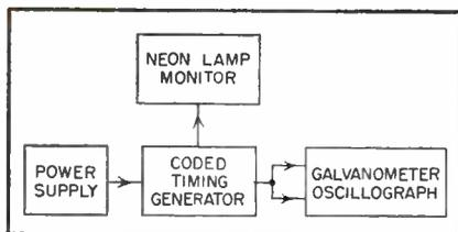
FIG. 1—Principle units of timing system
