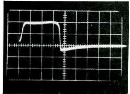
FIG. 3—Triode plate waveform for one-shot multivibrator-type circuit
