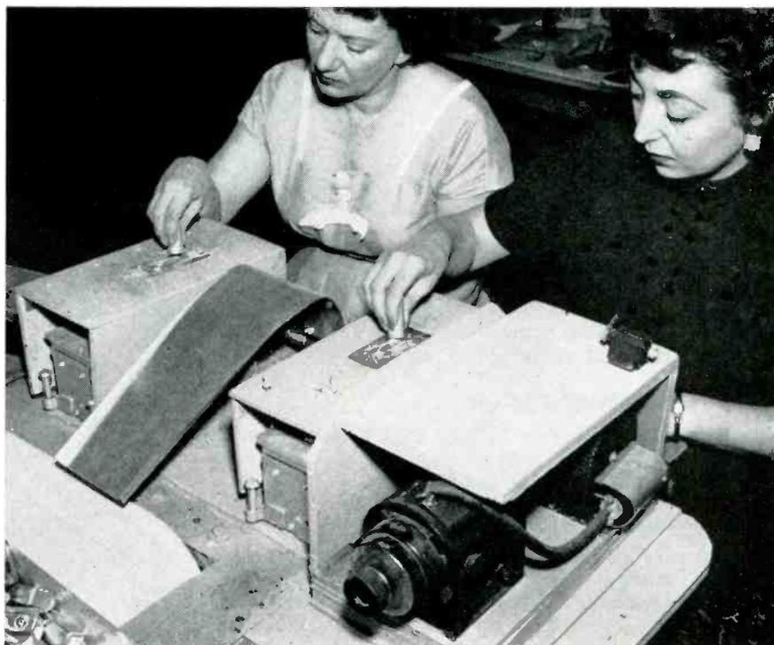
Swaging and soldering leads to paper-wound bathtub capacitors. Knurled, tin-plated steel wheels turning vertically in asbestos-enclosed electric solder pots bring hot aluminum solder to the slots in the tops of the asbestos boxes. Soldered units go down slide onto conveyor belt
