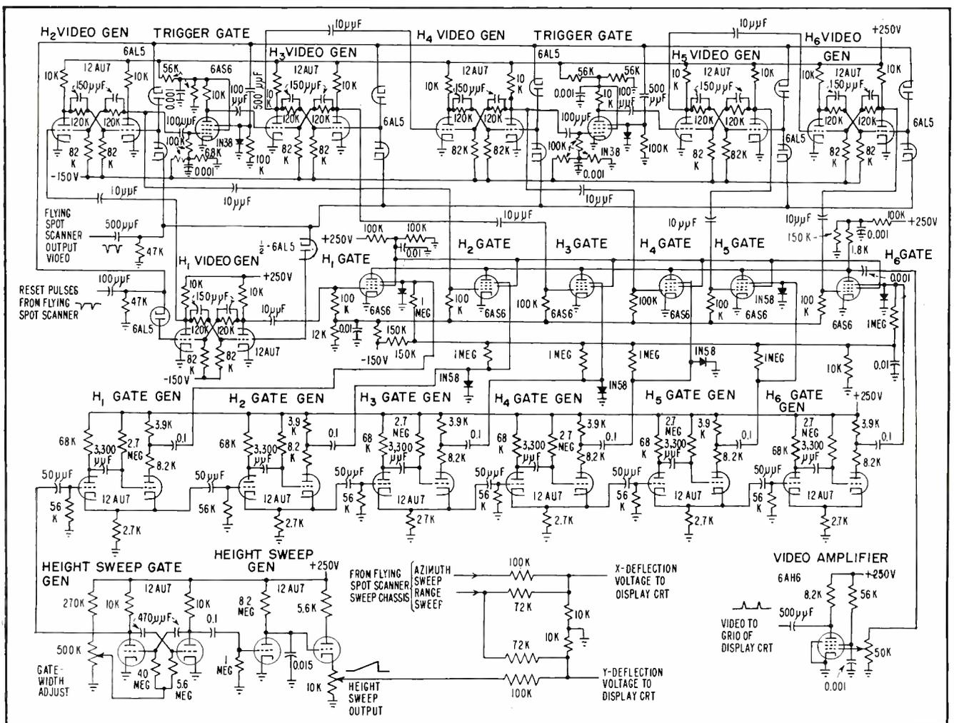
FIG. 5—Video simulator provides video signal for grid-modulation of crt and height-sweep-signal component of Y-deflection voltage
