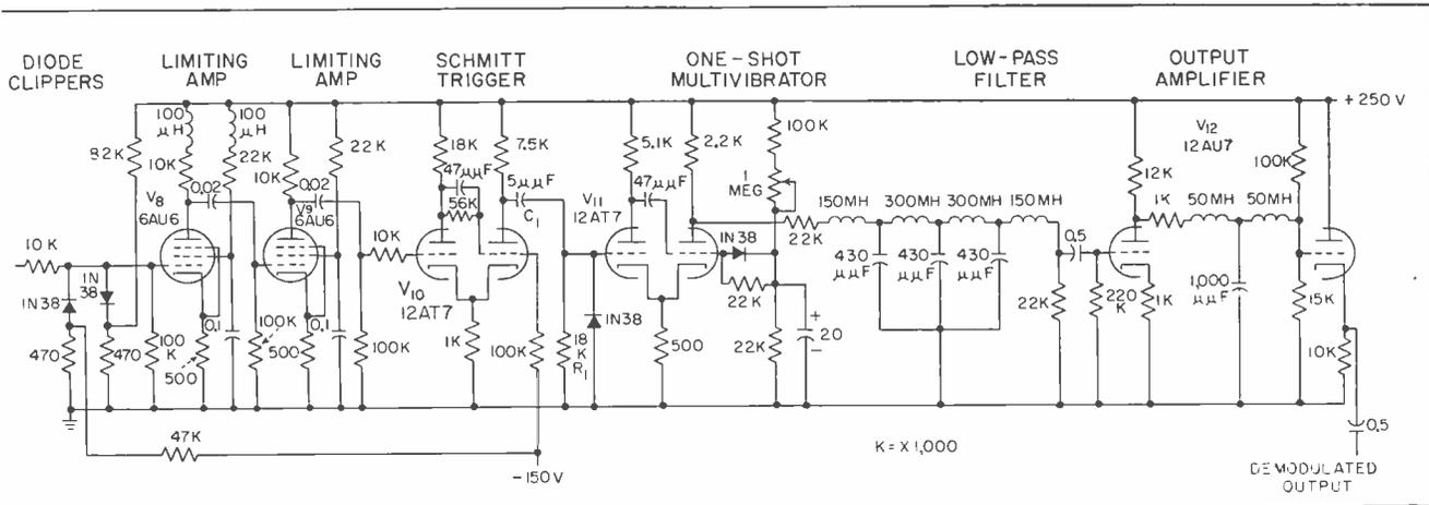
method is used in demodulator to give output signal from 10 cps to 20 kc for frequency-modulated tape recording
