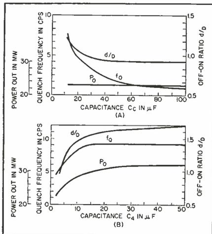
FIG. 3—Circuit performance with variation in quench capacitor  $C_c$  (A) and bypass capacitor  $C_b$  (B)
