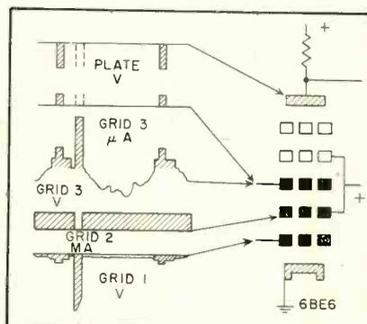
FIG. 4—Relationships at various tube electrodes for circuit of Fig. 3
