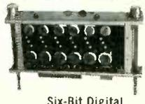
Six-Bit Digital Comparator Using Magnistors
