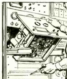
*Five seconds to put chassis in testing position. Slides smoothly out of rack, locks. Pivoting mechanism brings under-chassis parts to easiest working angle. Functioning of unit need not be interrupted!*
