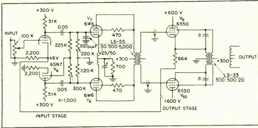
FIG. 1—Output transformer with two identical, interleaved 500-ohm windings permit true pentode cathode-follower operation, since the screens follow in exact phase with the cathodes. Bypass capacitors maintain this condition at high frequencies
