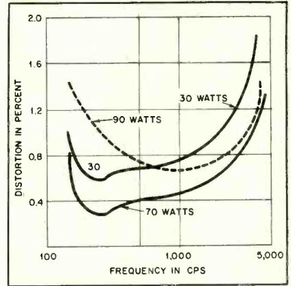
FIG. 2—Distortion curves were taken at 117-v output, using the 20-ohm output tap. Performance shows frequency response
