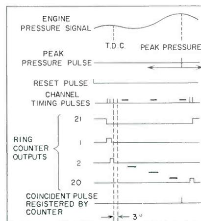
FIG. 3—Simplified timing chart. Pulse generated at peak pressure is gated through synchronized ring counter. Decade counters register coincidence between peak pressure and an open ring stage
