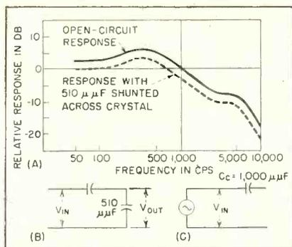
FIG. 1—Crystal response (A) shows effect of capacitive shunt that creates capacitive voltage divider
