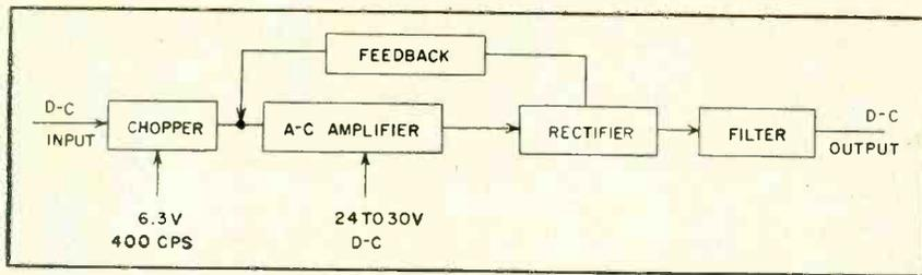
FIG. 1—Block diagram of transistorized chopper system utilizes synchronous modulation of d-c input and demodulation of output from a-c amplifier
