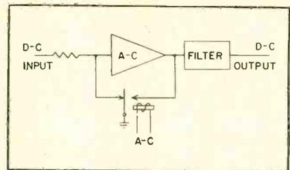
FIG. 2—Basic full-chopper d-c amplifier was adapted to missile instrumentation
