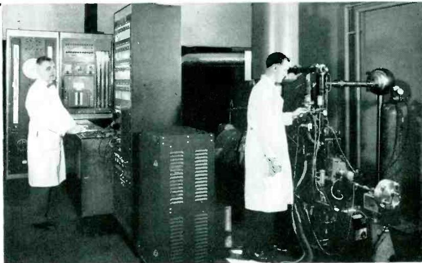
Information obtained from peak pressure distribution counter on racks at left, used with single-cylinder test engine at right, enables engineers to determine particle ignition characteristics of many fuels in a relatively short period of time
