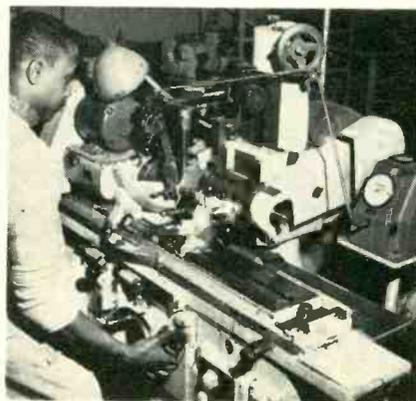
Operator brings grinder up to work with right hand while watching pointer of air gage which indicates outside diameter. Adjustable strips of black tape on dial window show tolerance range. Flexible air line runs from gage to air leak valve at overhead pivot of caliper arm which rides against stator
