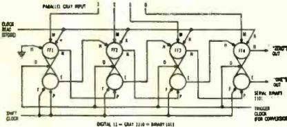
adaptable for use as a composite Gray-to-binary code converter and shift register. For this use, the Gray number is read into the shift register in parallel form (for example, from a code wheel or flip-flop register), converted internally to a binary number, and then shifted out in serial form.
