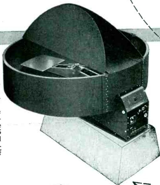
**MODEL B78** Used primarily for testing relays, switches, tubes, motors, valves, and other small components, and to calibrate and evaluate accelerometers. Accommodates objects weighing up to 25 lbs.; has G-range of 0.017 G to 120 G's. Maximum centrifugal capacity is 1200 G-pounds. Nominal radius of gyration 24".
