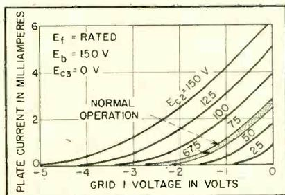
FIG. 11—Plate current plotted against grid-1 voltage shows transfer characteristics of the new tube
