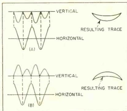
FIG. 3—Mouth generator waveforms, smiling (A) and frowning (B)
