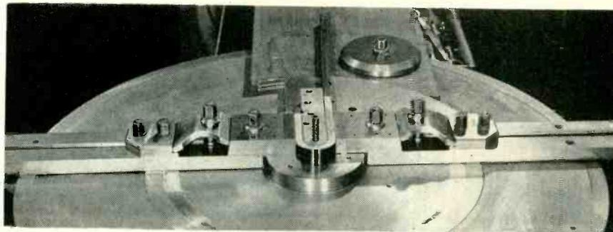
FIG. 5—Rectangular waveguide tubing formed into 180-deg bend, with top plate removed after bending to show bend
