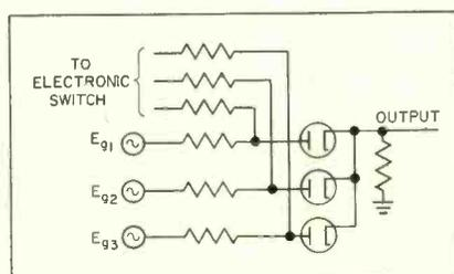
FIG. 6—Connection of tristable switching circuit
