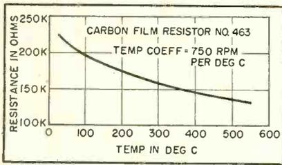
FIG. 1—Effect of temperature on 225,000-ohm GE carbon film resistor
