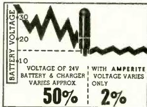
*Hermetically sealed*, they are not affected by changes in altitude, ambient temperature ( $-55^{\circ}$  to  $+90^{\circ}$  C.), or humidity ... Rugged, light, compact, most inexpensive.
