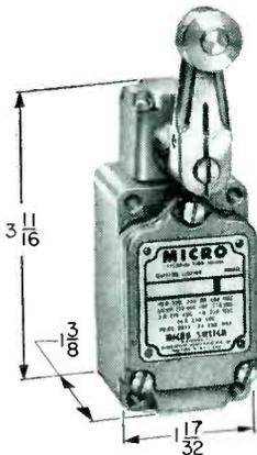
The MICRO SWITCH Type LS is a small two-circuit switch which meets a wide variety of industrial design requirements. It is extremely reliable, ruggedly housed and can be mounted in almost any location. Actuator head may be removed in the field and rotated to permit actuation from any of the four quadrants. The roller-arm actuator is field
