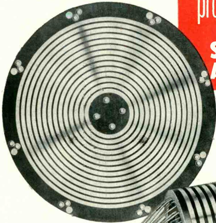
↑ An assembly with 14 concentric, hard silver rings electro deposited into machined plastic blank. Dovetail locks rings in place. Machined blank insures accuracy. Diameter approx. 11", thickness approx. 5/16".
