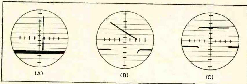
FIG. 3—Triggering pulse (A), time constant (B) and output waveforms of single-shot multivibrator used in expanded scale tachometer
