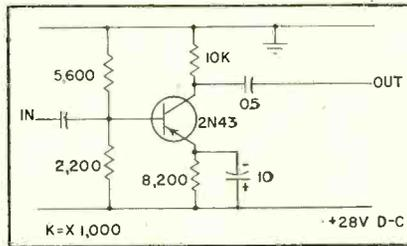
FIG. 7—Typical d-c amplifier circuit. The system employs three iterated common-emitter stages
