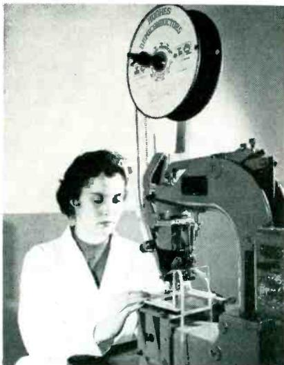
Ammunition belt feeds 3,000 semiconductors into machine that staples them into electronic circuits at Hughes Aircraft. A special machine was developed to fabricate the belts
