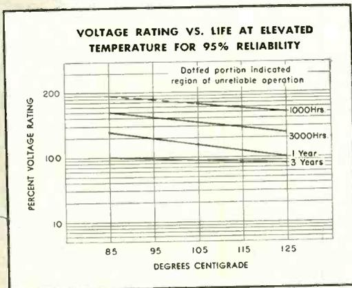
**OPERATES FOR 1 YEAR AT  $125\text{ C}$**  Molded PVZ capacitors are designed for a minimum of one year's life at rated voltage and  $125\text{ C}$  operation. Curves shown above are typical of performance.
