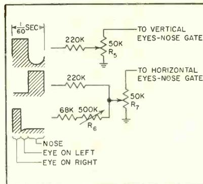
FIG. 5—Method of generating eyes and nose
