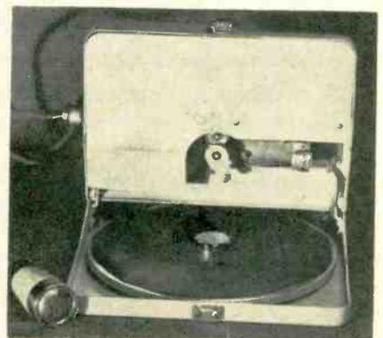
Working portion of a transistor portable dictating machine shows turntable driven by rotating dog (above). Magnetic head (upper right) moves across paper magnetic disk to record in spiral pattern. Built by Tokyo Tsushin Kogyo, Ltd., the unit employs four transistors and runs from four flashlight cells. The microphone is also used as a playback receiver.
