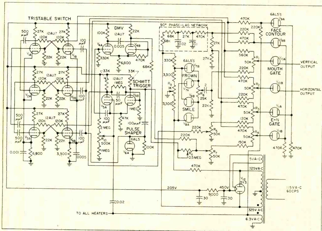
FIG. 7—Schematic diagram of the face generator used with standard oscilloscope
