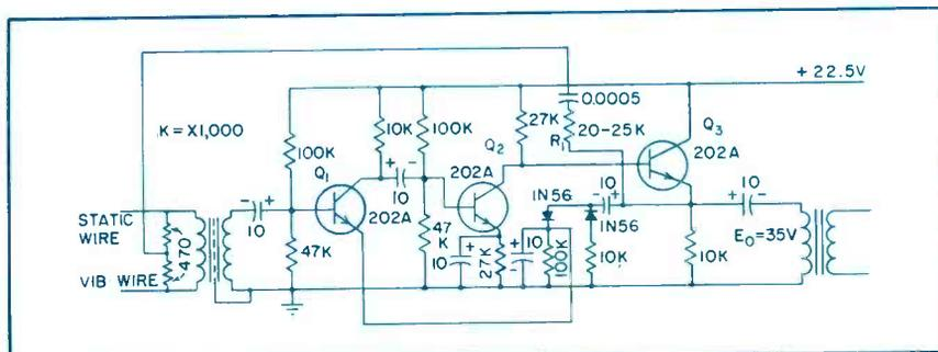
FIG. 2—Transistor amplifier for vibrating wire transducer uses agc to maintain output level at constant amplitude
