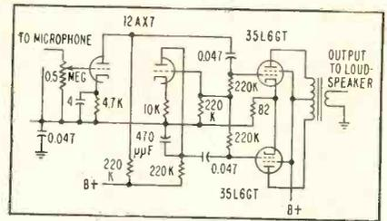
Amplifier for the delayed channel
