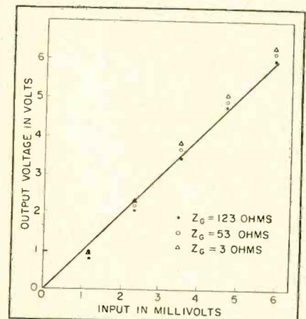
FIG. 5—Generator impedance variation at 3, 53 and 133 ohms
