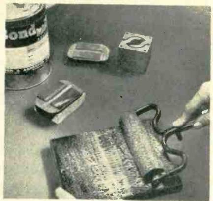
Rolling out Bondmaster M620 adhesive on palette just as it comes from can, to give uniform coating on application roller. Alnico magnets and lamination stack to be joined for Westinghouse recording wattmeter are shown in background
