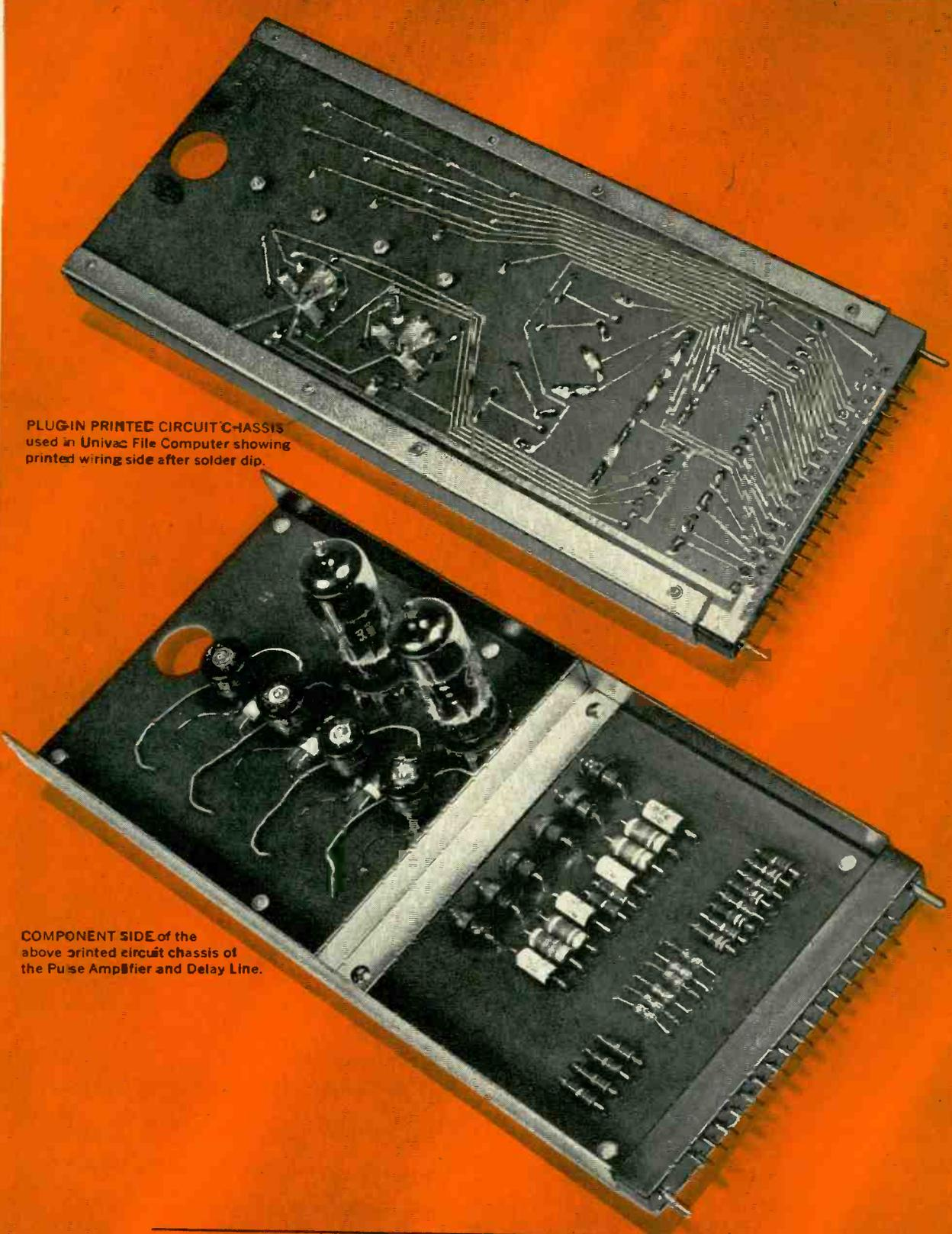
PLUG-IN PRINTED CIRCUIT CHASSIS
