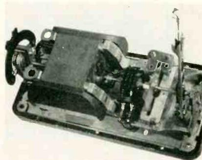
Completed wattmeter movement employing epoxy adhesive bonds in magnetic system
