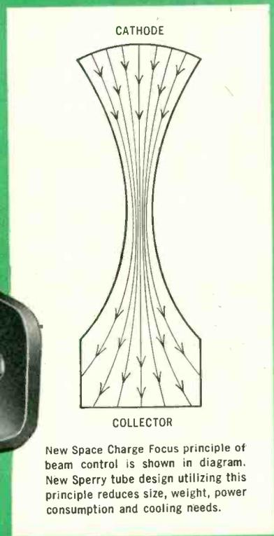
New Space Charge Focus principle of beam control is shown in diagram. New Sperry tube design utilizing this principle reduces size, weight, power consumption and cooling needs.
