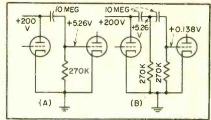
FIG. 3—Two coupling capacitors decrease effect of d-c leakage on grid bias
