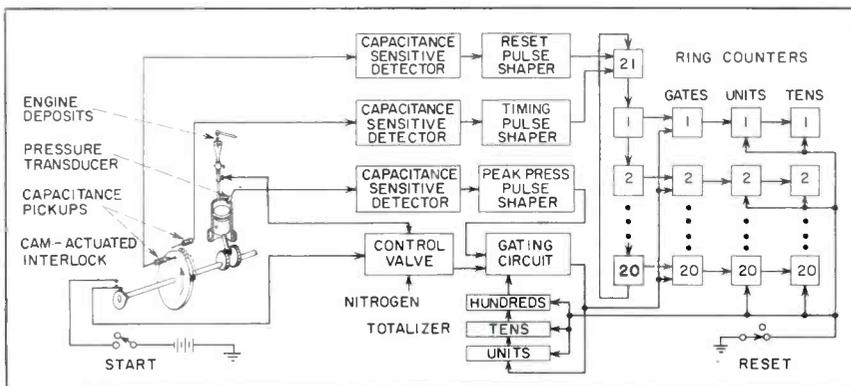
FIG. 2—Block diagram shows how crank angle is quantized into 20 channels that register distribution of peak pressure pulses occurring during ignition
