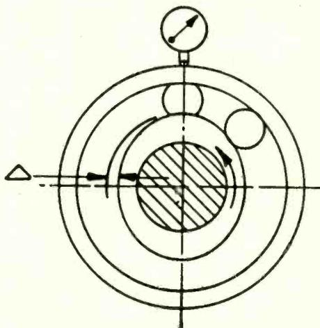
FIG. 2 — Inner raceway is out-of-round, although concentric with bore. Difference between the maximum and minimum readings indicates the degree of out-of-round.
