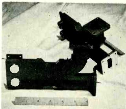
be modified to any standard or special fitting. An input vswr of 1.25 to 1 can be assured; recent measurements indicate a vswr of 1.15 to 1 is obtainable.
