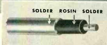
Cen-Tri-Core consists of a solder wire coated with either an energized or plastic rosin flux over which is formed an outer sleeve. It exceeds Federal Specs. QQ-S-571b and MIL S-6872.
