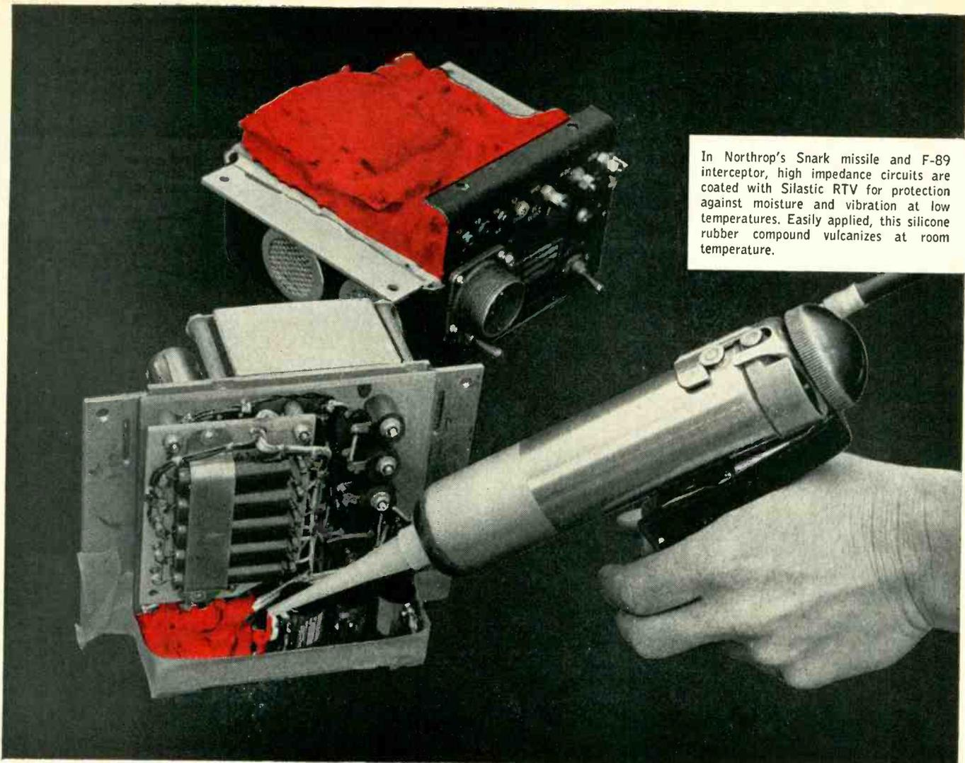
In Northrop's Snark missile and F-89 interceptor, high impedance circuits are coated with Silastic RTV for protection against moisture and vibration at low temperatures. Easily applied, this silicone rubber compound vulcanizes at room temperature.
