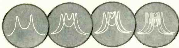
**SINGLE OR SUCCESSIVE** writings can be retained as permanent transients by the 104 MEMO-SCOPE Oscilloscope until intentionally erased. Stored traces may be almost instantaneously erased by front panel push button or external switch.
