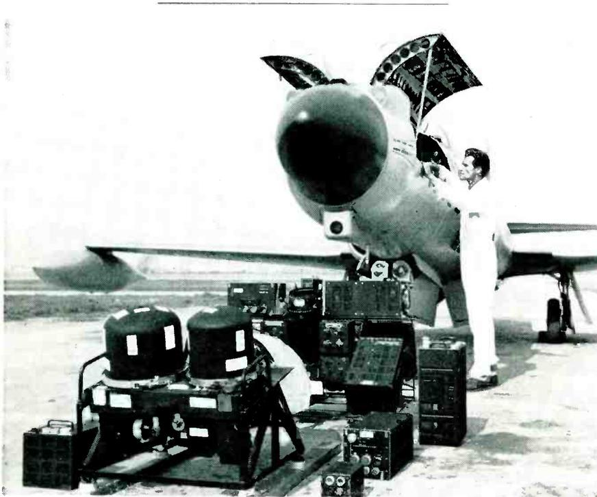
**COMPLEX** radar control, the brain of F-94 interceptor planes guarding the North American continent, is checked and installed by Hughes technician while . . .
