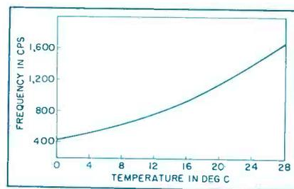
FIG. 5—Plot of oscillator frequency variation with temperature
