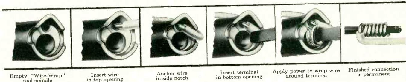
Empty "Wire-Wrap" tool spindle
