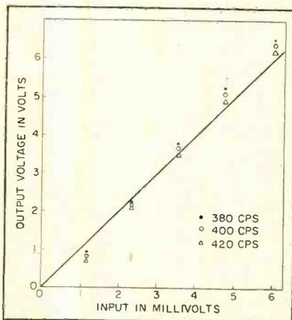
FIG. 3—Line frequency variation for 380, 400 and 420 cps at 6.3 volts rms
