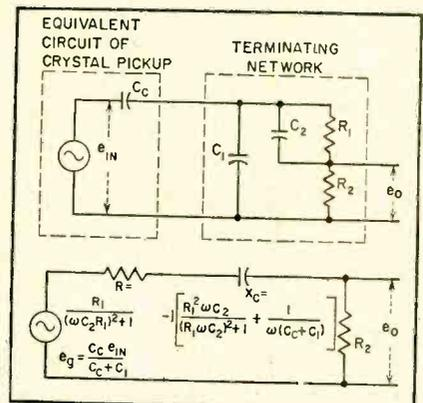
FIG. 5—Derivation of equivalent circuit for crossover region in Fig. 3A
