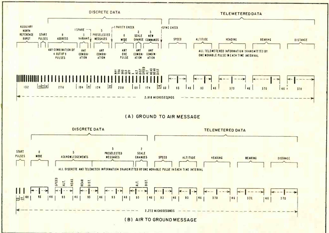
Tacan data-link code structure for ground-air and air-ground messages uses digital and analog codes
