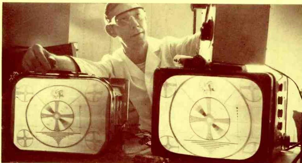
Superior sweep of G-E horizontal-amplifier tubes under low-line-voltage conditions, is demonstrated on screen at right. Large plate size and special finned or dimpled construction; advanced cathode processing; these and other features give improved performance. Tubes, moreover, are tested at factory for zero-bias plate current and plate-to-screen current ratio.
