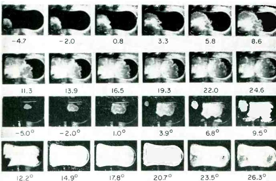
FIG. 1—Part of normal combustion sequence (upper two rows) as viewed through a quartz-headed engine and complex pattern resulting from particle-induced ignition (bottom rows). Numbers represent crank-angle position in degrees during power stroke
