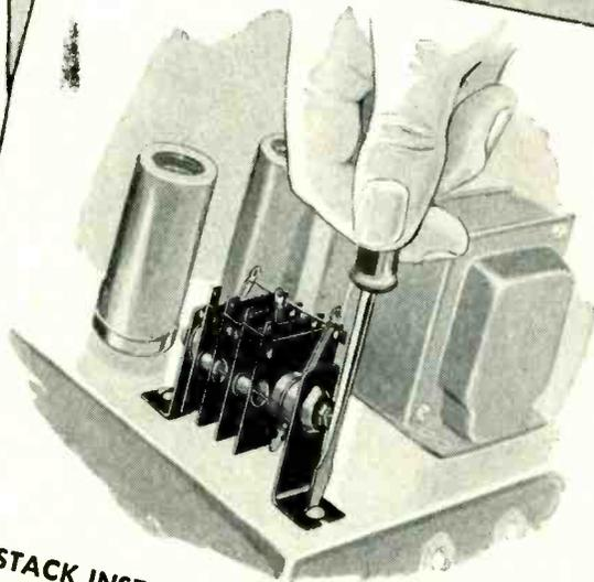
**STACK INSTALLATION.** A typical way of mounting General Electric Silicon Rectifier Stacks. Just two screws fasten the entire assembly in place.
