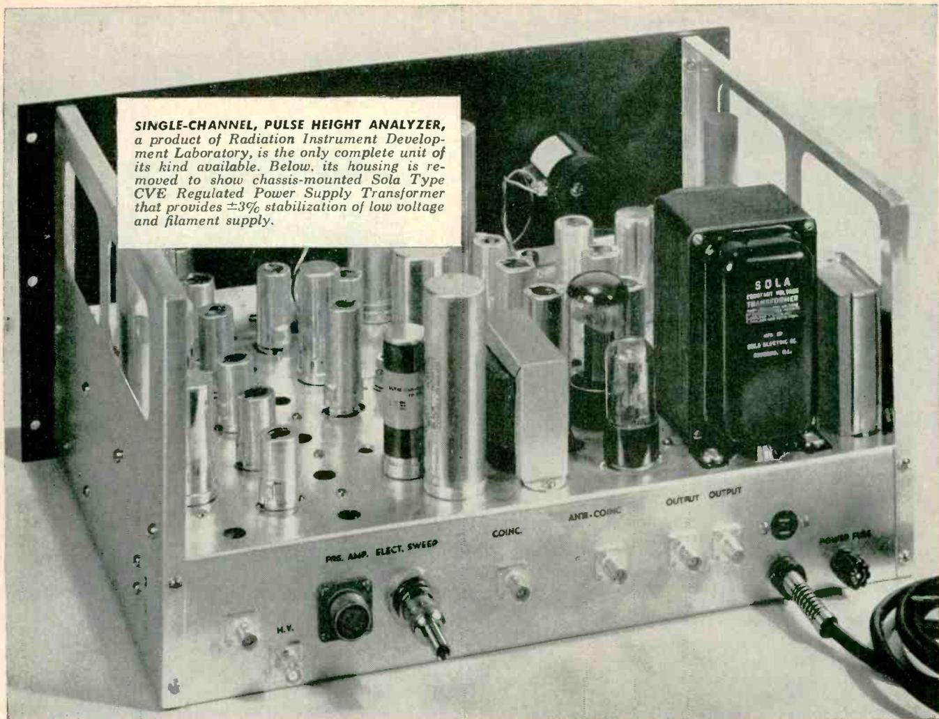
**SINGLE-CHANNEL, PULSE HEIGHT ANALYZER,** a product of Radiation Instrument Development Laboratory, is the only complete unit of its kind available. Below, its housing is removed to show chassis-mounted Sola Type CVE Regulated Power Supply Transformer that provides  $\pm 3\%$  stabilization of low voltage and filament supply.
