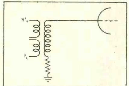
FIG. 4—Alternate circuit that eliminates rectifier
