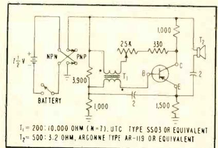
FIG. 2—Complete circuit of the transistor beta tester
