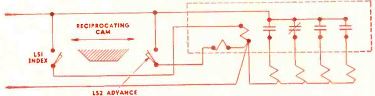
**Interlock sequence with several limit switches:** Each limit switch advances the Eagle step switch one position. Switches must operate in sequence or the step switch won't advance.
