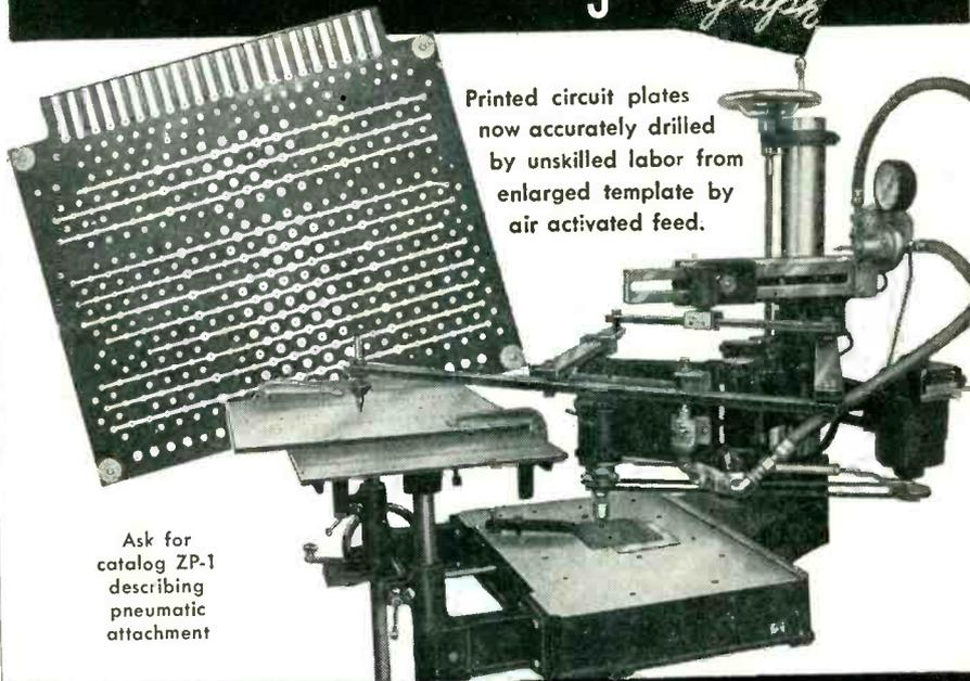
Printed circuit plates now accurately drilled by unskilled labor from enlarged template by air activated feed.
