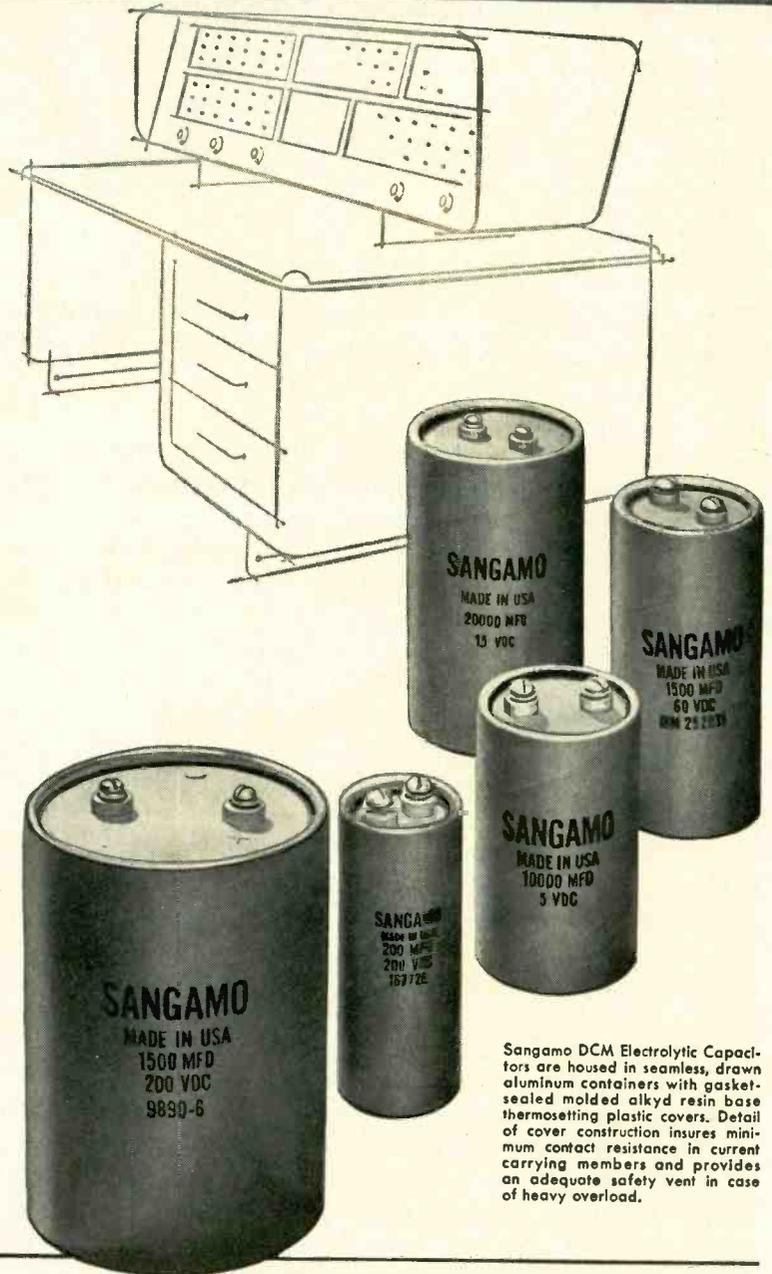
Sangamo DCM Electrolytic Capacitors are housed in seamless, drawn aluminum containers with gasket-sealed molded alkyd resin base thermosetting plastic covers. Detail of cover construction insures minimum contact resistance in current carrying members and provides an adequate safety vent in case of heavy overload.
