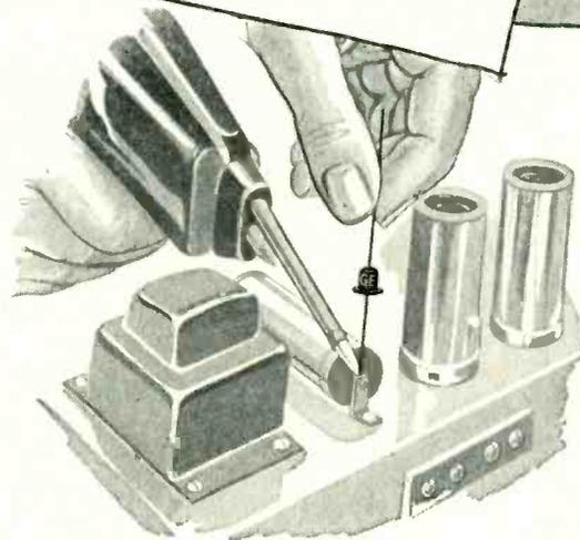
**AXIAL LEAD MOUNTED.** See the versatility of G-E Axial Lead models. They're easy to mount anywhere you need low current silicon rectifiers.
