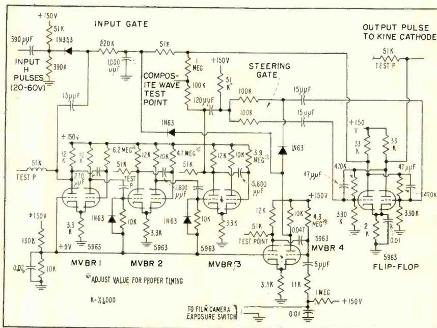
FIG. 2—Experimental version of control shutter. Most studio kinescopes will require additional triode input and output stages
