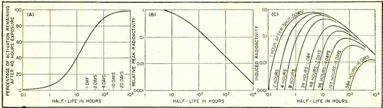
FIG. 2—Residual activation (A), radioactivity at shutdown (B) and relative radiation (C) of materials as a function of half-life
