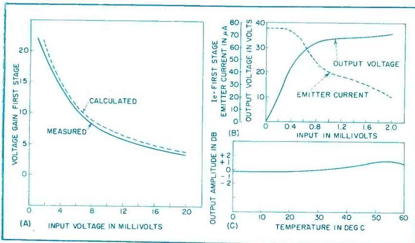
FIG. 3—First stage gain (A), output and  $ac$  response (B) and frequency response curve (C) for transistor amplifier used for depth measurement
