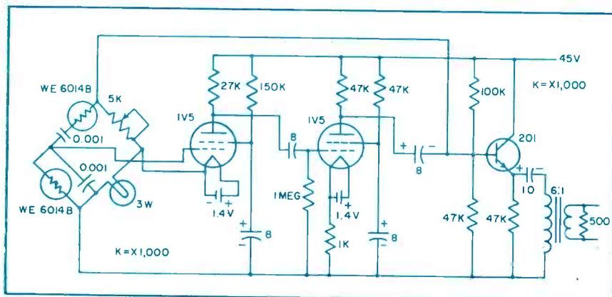
FIG. 4—Wien-bridge oscillator circuit used to measure water temperature. Units encapsulated in epoxy resin and sealed in pressure tight housing.
