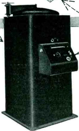
**MODEL E185** This newest and largest Genisco centrifuge was recently built for the U.S. Air Force. Two mechanical or electronic packages, each weighing up to 300 pounds, can be subjected to an acceleration environment of up to 65 G's simultaneously. Nominal radius of gyration of the machine is six feet. An automatic dynamic balancing system automatically compensates for any excessive unbalance in the machine during test runs.
