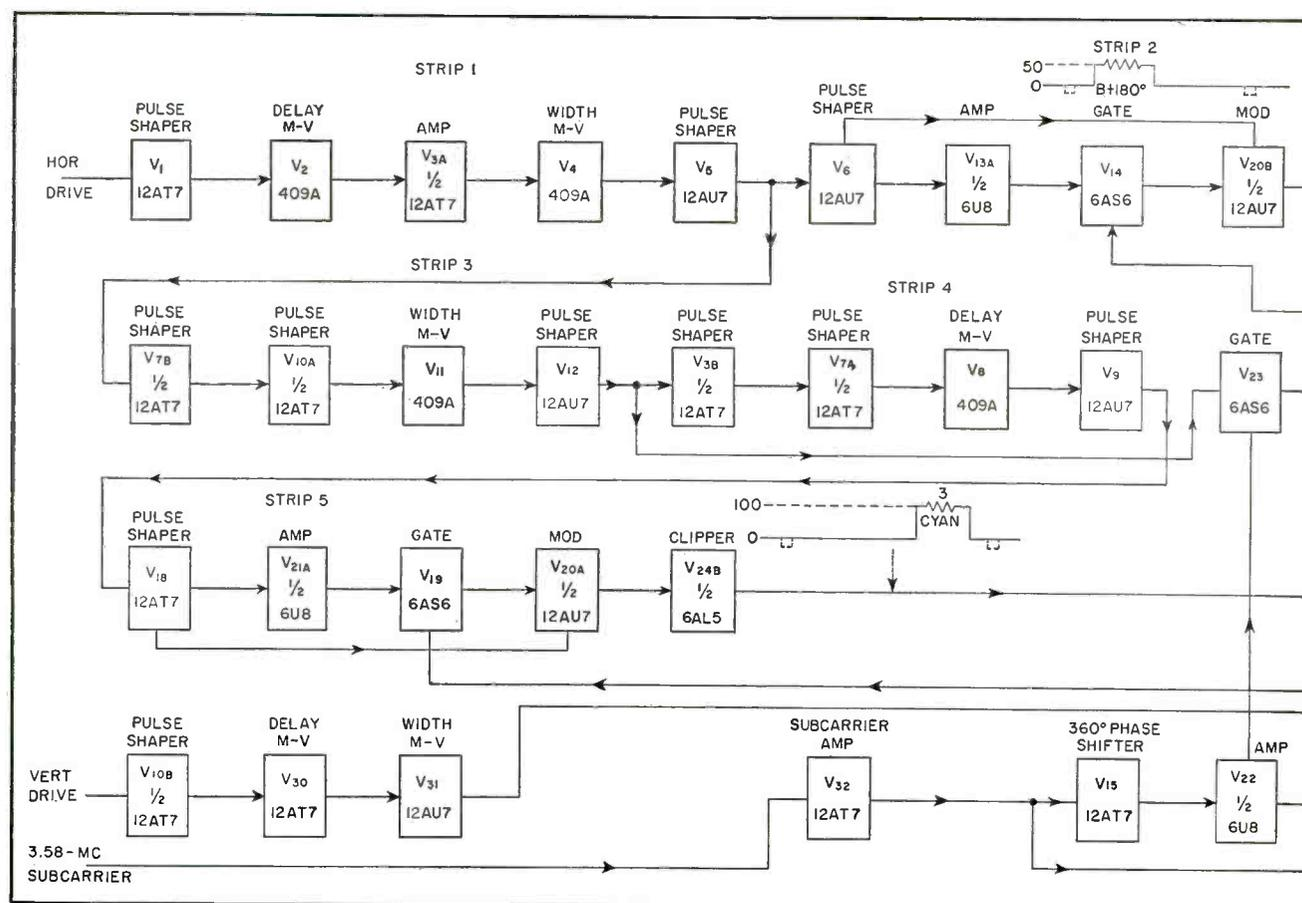
FIG. 3—Block diagram of the complete test signal equipment
