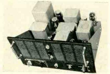
Chassis of 90-watt power amplifier indicates the simplicity and economy of construction, made possible because of the limited frequency applications
