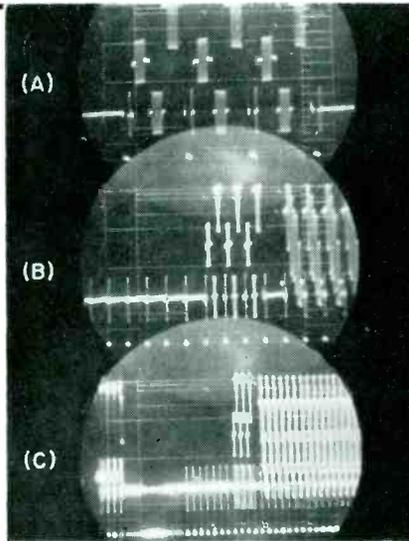
FIG. 1—Test signal for three sweep speeds. Signal appears after second set of equalizing pulses (A) in vertical blanks
