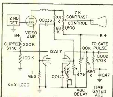
FIG. 2—Impulse noise is time gated but vertical sync output suffers
