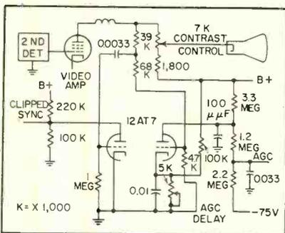
FIG. 1—Simple unprotected circuit for agc and sync separation
