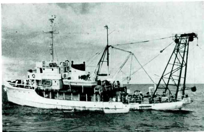
Research ship equipped with boom for raising and lowering bathythermometer to measure temperature gradient of ocean water
