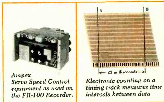
Ampex Servo Speed Control equipment as used on the FR-100 Recorder.
