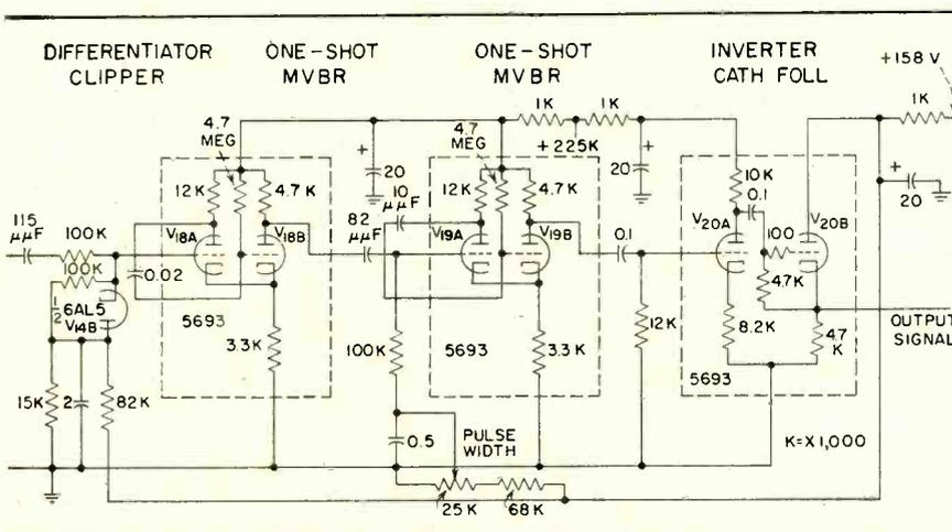
that is normally set to 20  $\mu\text{sec}$  by the pulse width control
