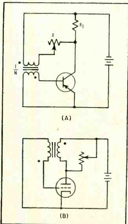
FIG. 1—Simplified form of beta tester (A) and tube analog (B)
