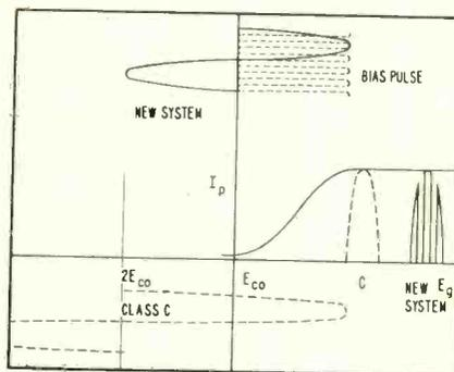
FIG. 1—Comparison of class C and new system
