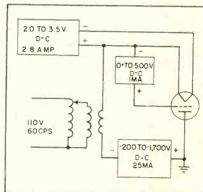
FIG. 2—Typical power supply requirements for the vtm
