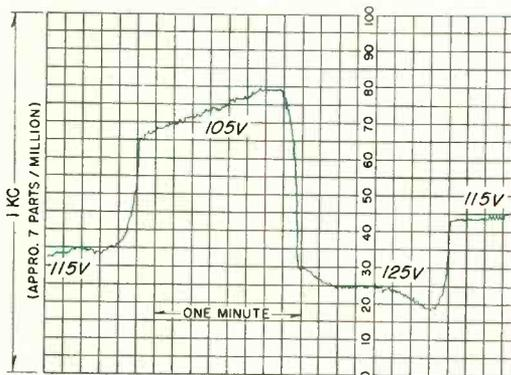
Figure 1. Frequency stability vs. line voltage;
