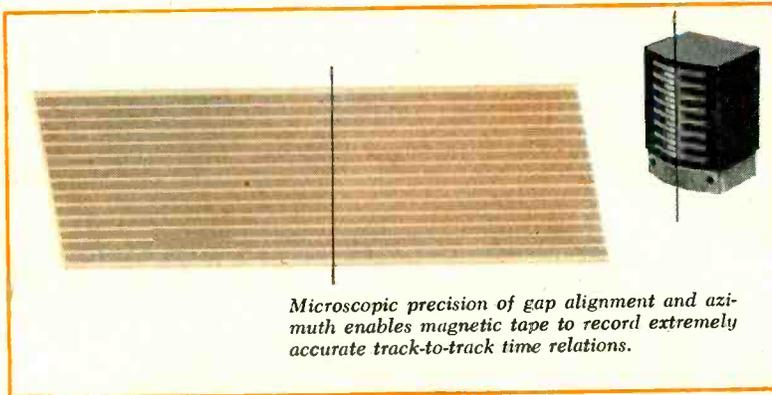
Microscopic precision of gap alignment and azimuth enables magnetic tape to record extremely accurate track-to-track time relations.
