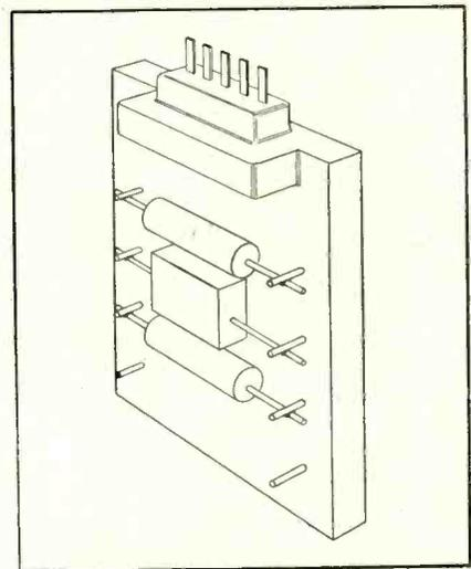
FIG. 5—Terminal arrangement in ceramic submodular chassis
