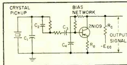
FIG. 7—Degenerative transistor preamplifier has higher input impedance and signal-to-noise ratio, with less distortion, than circuit shown in Fig. 6. Gain, however, is less
