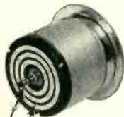
Three external stator rings in face of Autosyn.
