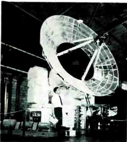
Direct calibration and immediate evaluation of the performance and behavior pattern of guided missiles is handled by this new instrumentation radar system developed by RCA. Antenna pedestal shown is designed for mounting on a separate tower to minimize vibration
