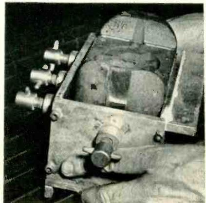
Placing jig in oven for curing bond
