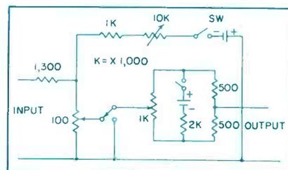
FIG. 6—Zero set circuit used with recorder. Variable resistor and potentiometer are helical type
