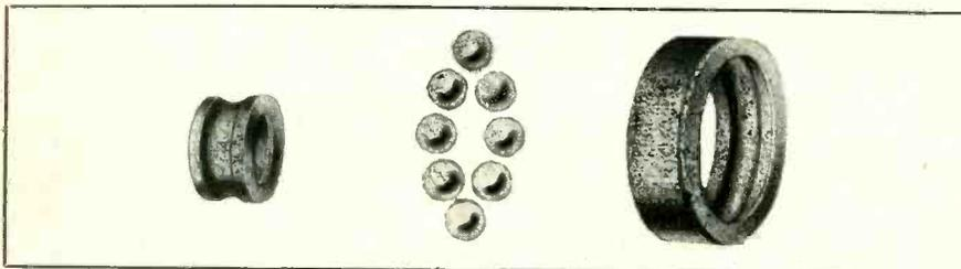
FIG. 3 Radial Runout is the result of eccentricity in the bearing parts. Principal factors producing it are eccentricity between bore and raceway of inner ring (left) and between raceway and outer diameter of outer ring (right). Out-of-round balls offer negligible effect, since effect tends to cancel out as balls roll.
