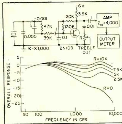
FIG. 6—Crystal pickup is matched through network to transistor preamplifier. Over-all response is shown for various amounts of treble cut
