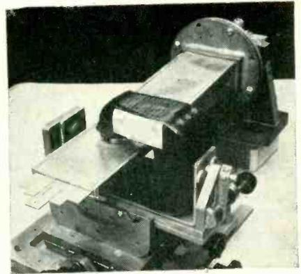
Magnet is shown in operating position over vtm inserted in tapered waveguide
