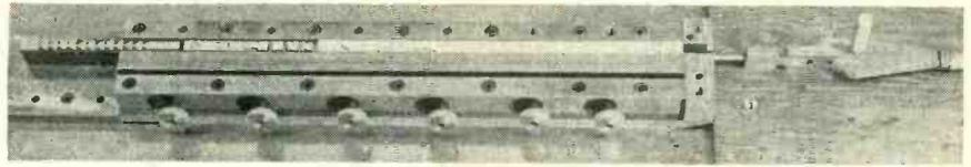
FIG. 1—Cable at right pulls sizing broach through waveguide tubing in preparation for bending. Vise clamp having six knurled screws holds tubing
