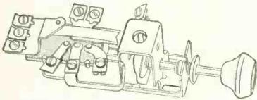
**Back plate** on an automobile headlight switch, punched and machined from Taylor Grade XP paper base laminate, has low moisture absorption and good dielectric strength.
