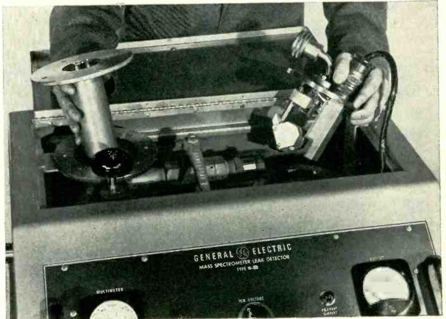
**DOWN-TIME IS REDUCED** through easy access and removal of the spectrometer tube (right) and by a simplified vacuum system design.
