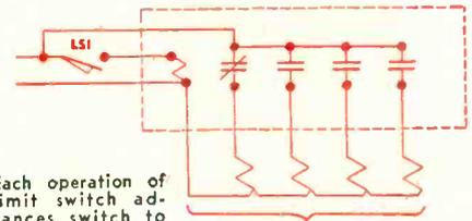
Each operation of limit switch advances switch to next position.
