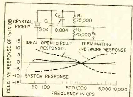
FIG. 4—Calculated parameters of terminating network for RCA 75476 pickup and resulting overall response
