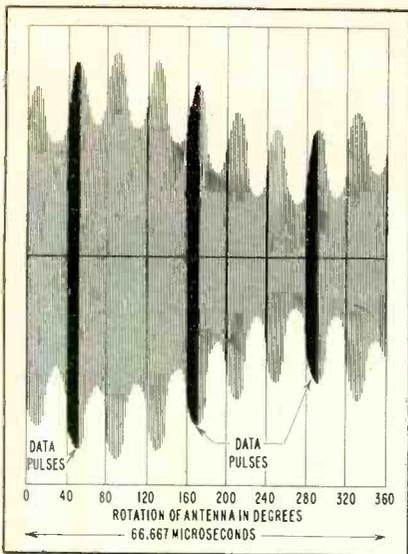
FIG. 1—Data-link beacon transmission
