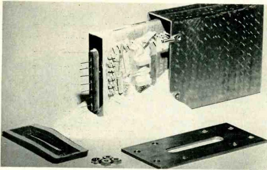
Subassembly encapsulated in alumina sand has high resistance to shock, vibration and nuclear radiation along with 500 C temperature rating. Component leads are welded to wire terminals cemented into holes in ceramic chassis
