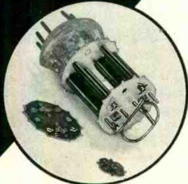
Insulating mica bridge for high-temperature electronic tube.
