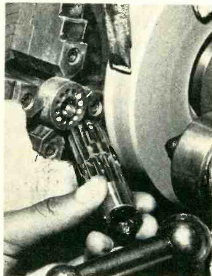
Assembled stator on 16-pin fixture is inserted in mating holes of fixture located in headstock chuck and held by spring-loaded tail stock
