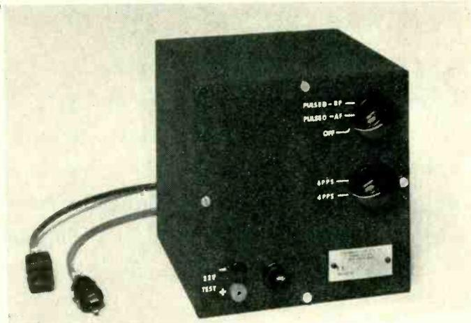
Compact keying unit contains all components except relays, which are mounted in signal generator cabinet
