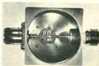
Invented by Myron C. Selby of NBS Boulder Laboratories, the radio-frequency micropotentiometer shown can be used to measure a microvolt at 1 kmc
