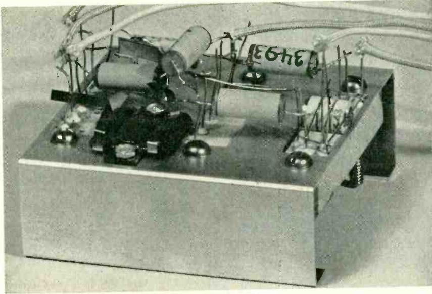
FRONT COVER: Operating tests in 500 C oven and on charcoal fire show that printed ceramic chassis using silver conductors performs equally as well as above metal-chassis subassembly with inset ceramic terminal strips, both using metallized resistor, mica capacitor and ceramic tube shown at right
