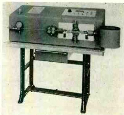
announced a new automatic wire cutting and stripping machine with features designed to meet specific needs of the electronics industry.
