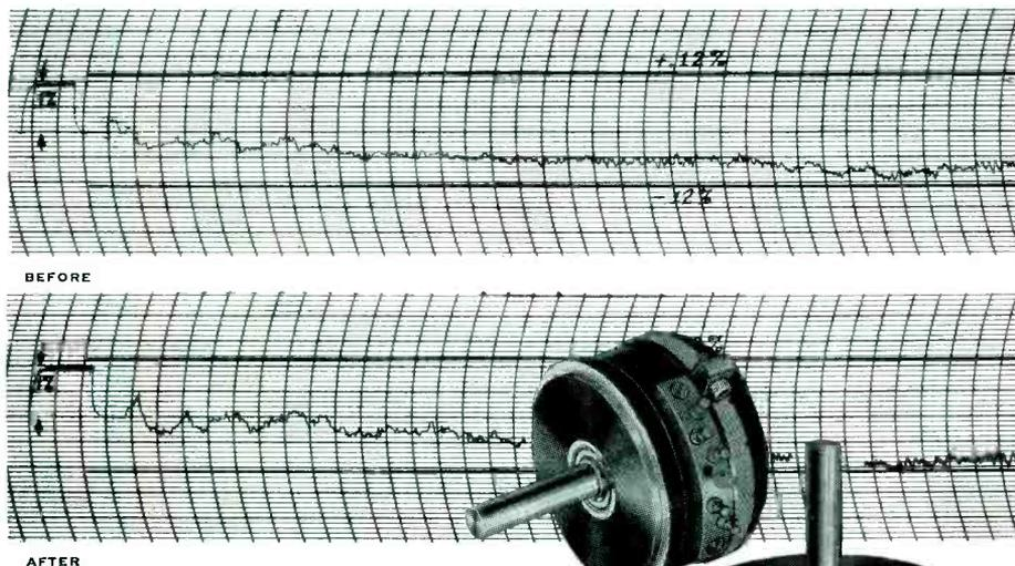
Take for instance a recent test report on the TIC Type ST20, a 2-inch, low-torque, ball-bearing precision potentiometer. The life test was conducted on a standard 6500 ohm unit. At 30RPM the ST20 was subjected to 700,000 cycles, reversing direction every 30 minutes. The linearity graphs shown above show the before and after of the ST20's independent linearity. As can be seen, the linearity change is imperceptible.
