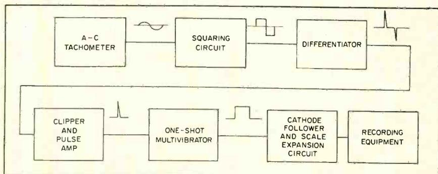
FIG. 1—Block layout of speed indicator, showing waveforms at various points in circuit
