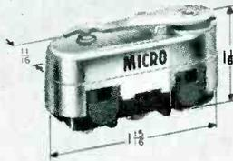
This small MICRO SWITCH Type HS precision switch is truly hermetically sealed (glass to metal and metal to metal) to insure constant operating characteristics under any environmental conditions—for example, no condensation problem.
