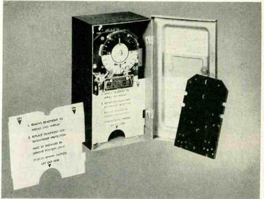
Time switch, made by the Tork Clock Co., uses two Taylor products . . . the deadfront is made of vulcanized fibre for its insulating properties, shock protection and printability . . . the mounting panel of the clock is made of Taylor laminate XP-1-231, chosen for high strength and good punchability.
