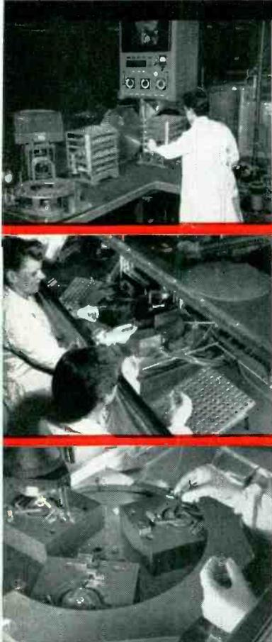
**Philco cold-welding process permits hermetic sealing in controlled atmosphere . . . assuring exceptional transistor life and performance!**
