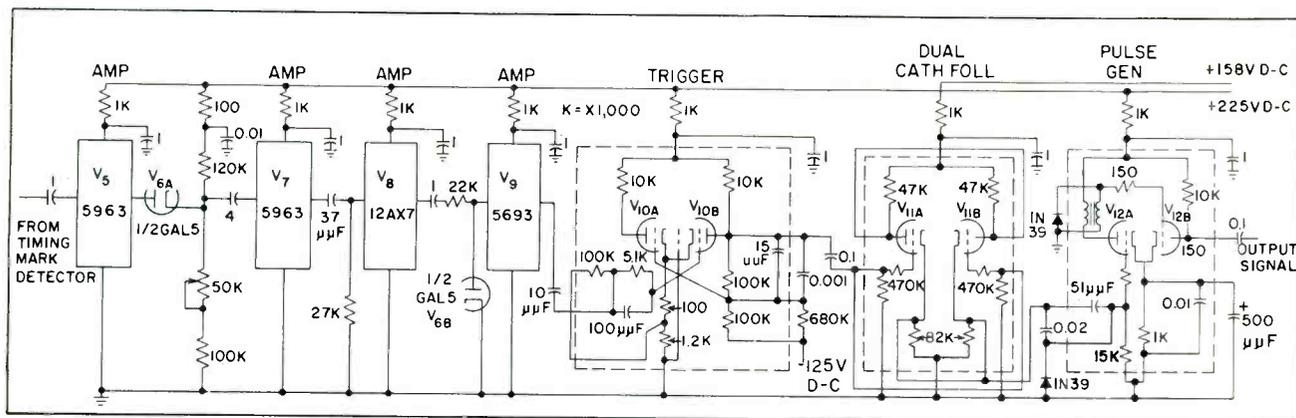
FIG. 4—Timing-pulse circuit. Negative pulses at 3-degree intervals are generated from capacitance variations between timing wheel and displacement pickup that are amplified and shaped to trigger the blocking oscillator output stage
