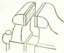
**Vise jaw caps**, made of Taylor Grade C phenolic laminate, are easily cut and machined to shape. Marring of precision or delicate parts is eliminated.
