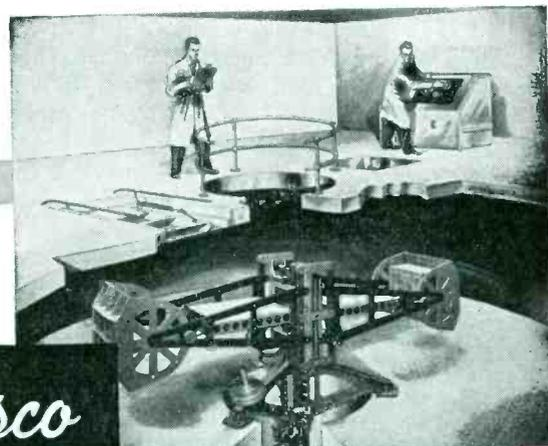
**ACCESSORIES ADD TO OPERATING EASE** A number of accessories including a strobe system, air system, optical system, tub cover, access doorway, and slip ring systems, designed to give greater operating convenience, are available for Genisco G-Accelerators, Models B78 and C159.
