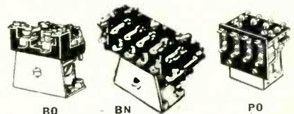
Allied's types BO, BN and PO are sturdy, compact, highly efficient, competitively priced relays made with bakelite insulation throughout. Contacts are silver with a non-inductive rating of 15 amperes or 30 ampere for double break contacts (U, V) at 24 VDC and 110VAC. Operate time at 2.5 watts DC: 18.5 millsec; release time: 8.0 millsec.
