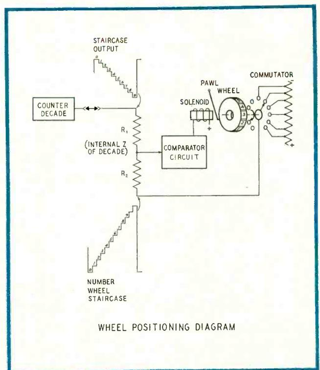
Figure 2. Principle of recorder operation. At the end of each counting period, the staircase voltage generated comes to rest on a step corresponding to the digit displayed by that decade. The number wheel rotates, generating its own staircase. At voltage coincidence, the number wheel is positioned by comparator and solenoid.
