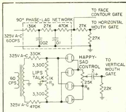
FIG. 4—Circuits for generating mouth contour
