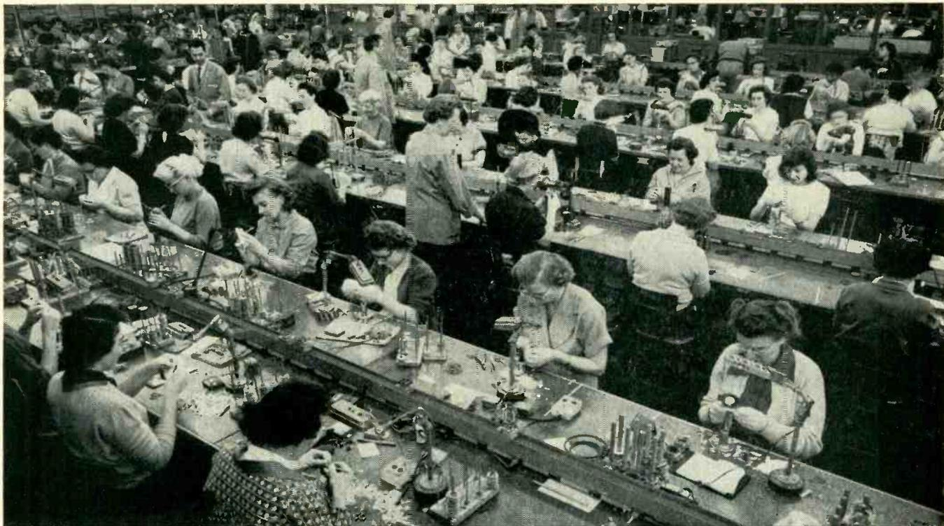
Section of department making stators for Bendix synchros and motors
