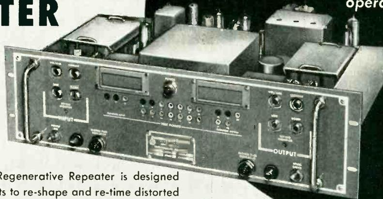
The new Northern Radio Regenerative Repeater is designed for use in telecommunication circuits to re-shape and re-time distorted signals for local use or retransmission. Special provision has also been made for use of this unit on half duplex circuits — where it will not only regenerate the ordinary teleprinter signals but also faithfully reproduce such special signals as "break" signals and "mark restoration" information.
