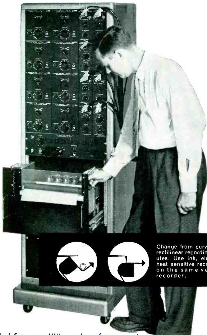
Change from curvilinear to rectilinear recording in minutes. Use ink, electric, or heat sensitive recordings—on the same versatile recorder.
