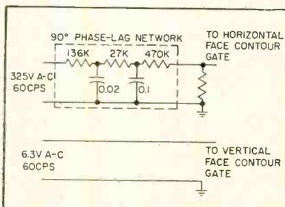
FIG. 2—Generation of face contour signals
