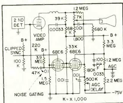
FIG. 5—Second type 6BE6 pentagrid tube is added for agc amplifier
