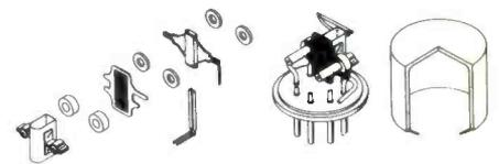
Exploded view of stacked tube demonstrates its rugged planar mount construction utilizing ceramic element spacers assembled on a ceramic stem. Note that element spacings are independent of the tube envelope.
