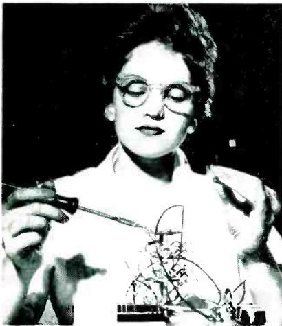
Nearly 500 small GE soldering irons of the type shown are used to solder about a half-million joints needed to make one IBM 705 function. Joints soldered in the magnetic core memory unit alone total nearly 9,000
