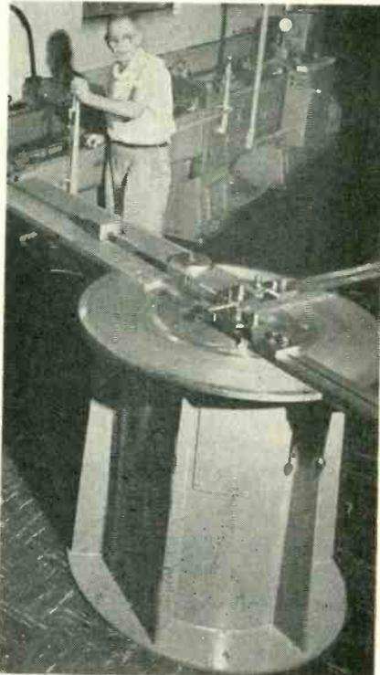
FIG. 6—Pulling mandrel out of tubing after 90-deg bend with  $\frac{1}{4}$  inch-radius
