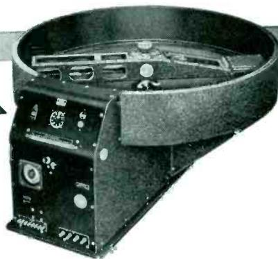
**MODEL D184** A high-speed machine, designed to test accelerometers and other instruments under acceleration forces from 1 to 850 G's. Full centrifugal capacity is 1000 G-pounds. Nominal radius of gyration 12".
