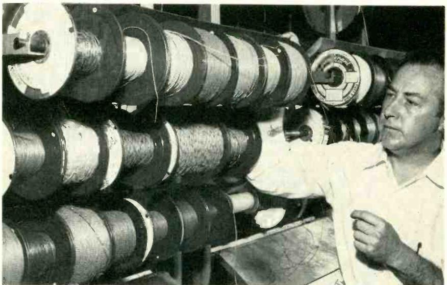
Strips of aluminum over rows of spools stop overrun and prevent wire from slipping over rim onto adjacent spool when operator reaches over harness board to pull down and cut off length
