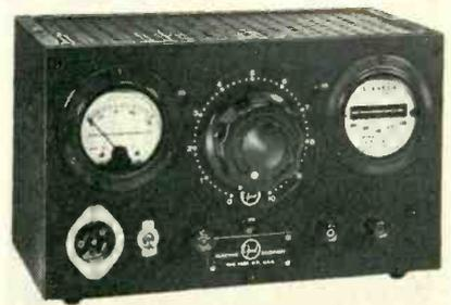
components. The unit operates on 115-v 400-cycle single-phase power and provides a continuously adjustable output from zero to 115 v under a maximum load current of 15 amperes. Standard instrumentation includes a  $3\frac{1}{2}$ -in. 21-reed  $\frac{1}{2}$ -percent accuracy frequency meter and a 2-percent accurate a-c voltmeter.
