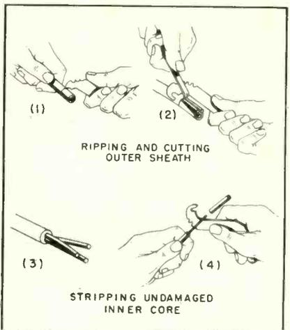
Special stripping knife used for removing cable insulation
