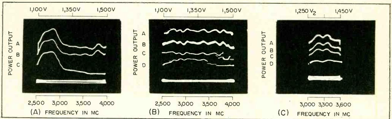
FIG. 1—Waveshapes show power output against anode voltage during wide-band operation in balun-ridge waveguide (A), tapered waveguide (B) (breaks in C and D are from too-low control voltage) and during narrow-band operation in tapered waveguide (C)
