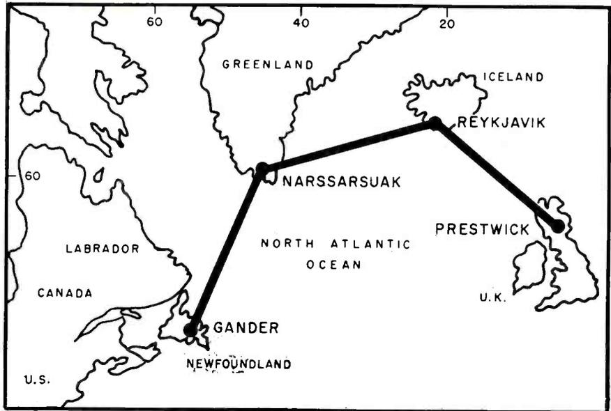
**PROPOSED** air-ground communications network connecting Newfoundland, Greenland, Iceland and the United Kingdom—Ireland will use forward propagation-by-ionospheric-scatter stations to help eliminate transmission blackouts as . . .
