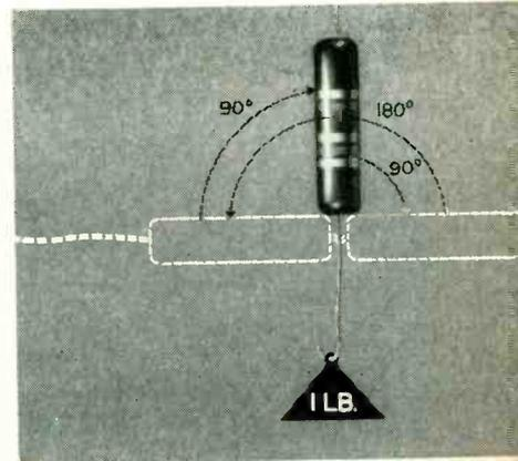
**HIGH LEAD BEND RESISTANCE** The new capacitors withstand one-pound-vertical-pull test moving the body of the unit  $90^\circ$ , then  $180^\circ$  in the opposite direction, then back  $90^\circ$ , to the original vertical position.
