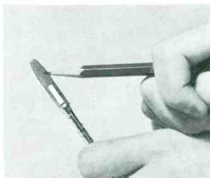
**RAPID HEAT TRANSFER** is achieved through a tubular heater located in the copper tip. Result: the General Electric Midget's heat efficiency is 90%.
