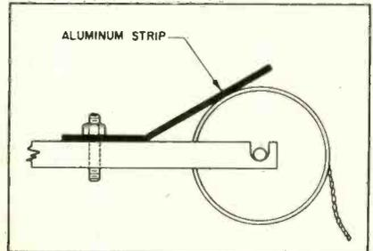
Method of mounting aluminum strip on frame of spool rack
