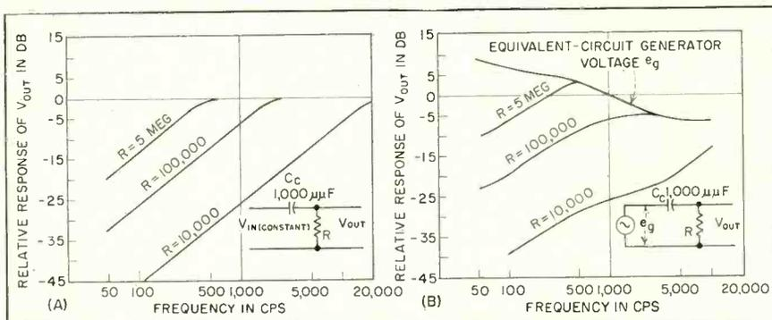
FIG. 2—Network formed when crystal is terminated with resistance and response for constant input voltage (A); equivalent generator circuit of crystal with terminating resistance and response (B)
