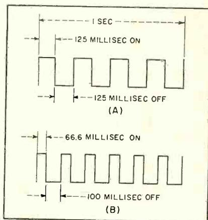
FIG. 1—Pulse times for four (A) and six pps repetition rates (B)
