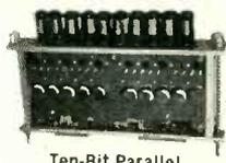
Ten-Bit Parallel Output (Serial Input) Using Magnistors
