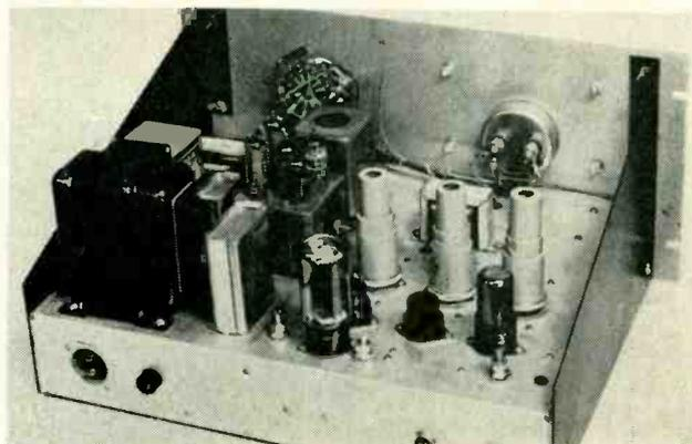
Speed indicating unit (left) is designed for rack mounting. Rear of chassis (right) shows plug-in units for squaring circuit, pulse amplifier and multivibrator at center of chassis. This design reduces instrument-repair downtime
