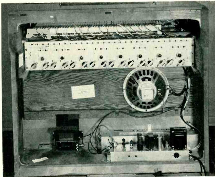
Rear view of organ shows tone generator chassis at top for keyboard. Chassis at bottom supplies pedal notes using single oscillator for the 13 tones
