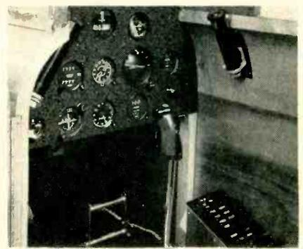
Flight trainer installation of data link. Canned messages are displayed on dial right center. They are sent from box lower right
