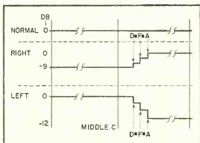
FIG. 3—Attenuation characteristic for solo control in its three positions
