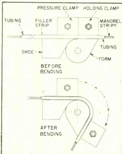
FIG. 3—Setup for bending tubing
