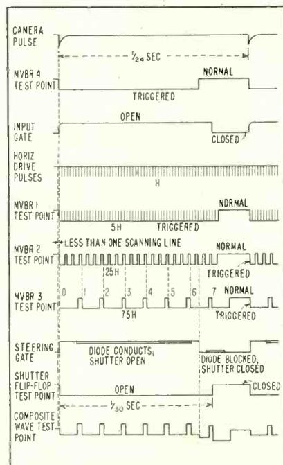
FIG. 3—Waveforms covering time of one horizontal line, one horizontal blanking period and start of next line. Circuit test points are shown in Fig. 2
