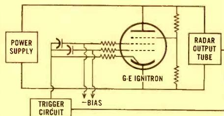
Trigger circuit goes into action whenever radar output tube receives an overload—actuates the ignitron, which instantly becomes a current bypass ("crowbar") in order to short out the threatened tube.
