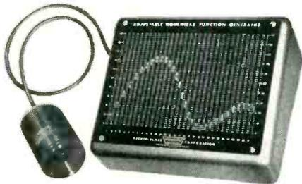
The VERNISTAT Adjustable Function Generator—a variation of the VERNISTAT a.c. potentiometer—permits quick and easy alteration of any nonlinear function. The adjusting mechanism provides a graphic display of the function which may be mathematical or empirical, including those with multiple slope reversals.
