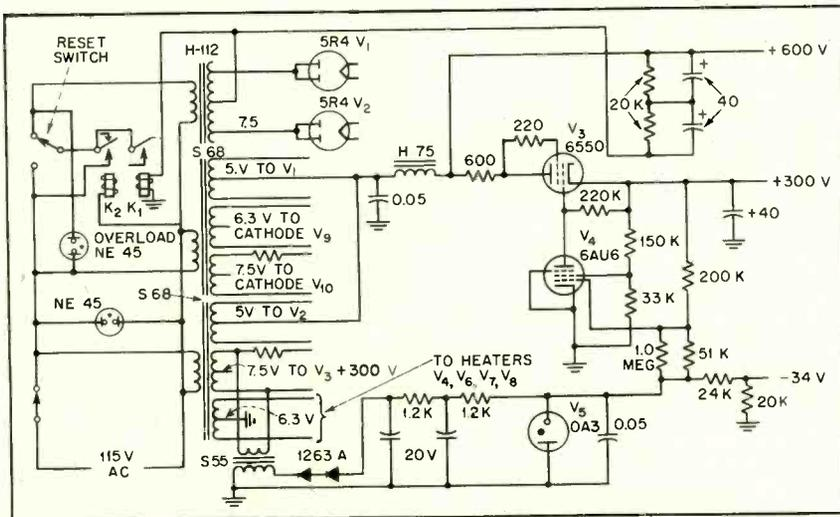
FIG. 3—Power supply for the 90-watt power source. Supply used for the final screens maintains constant screen voltage with a highly variable screen current
