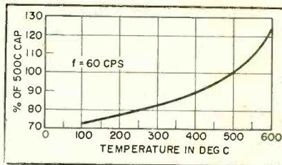
FIG. 2—Effect of temperature on typical mica capacitor unit
