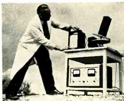
Mobile atmosphere radiation monitor finds radioactivity released from reactor stacks
