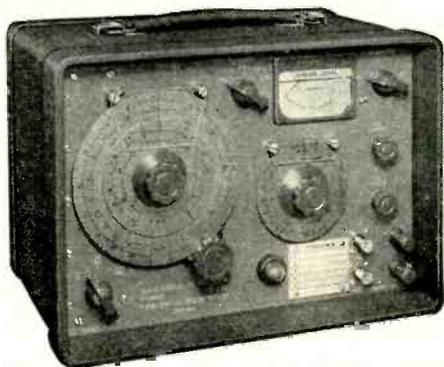
The 1064/2 provides high-grade fm outputs in the ranges 30 to 50, 118 to 185, and 450 to 470 mc; crystal-controlled i-f outputs at five spot frequencies; and a 1 kc af output.
