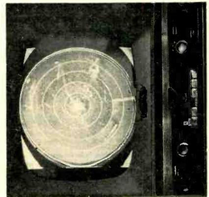
A special tube is making it possible to broadcast a television picture of a radar PPI presentation covering an area 100 km radius around Brussels National Airport. The radial trace is converted by the image-transforming tube into a 625-line tv picture to be broadcast to control centers and even to aircraft.
