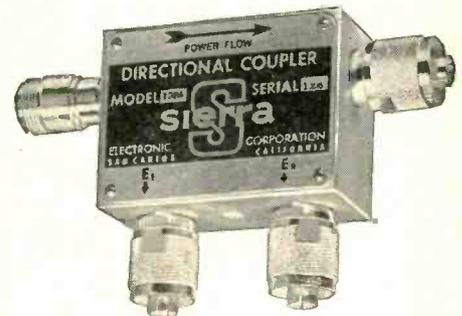
Versatile, accurate Sierra couplers are offered in 6 models for frequencies 10 kc to 2000 mc. Couplers provide transmission line measurements including reflection coefficient, VSWR, power. Also permit matching of loads to lines dynamically by indicating conditions providing minimization of reflected voltages. Request Bulletins 101, 104.
