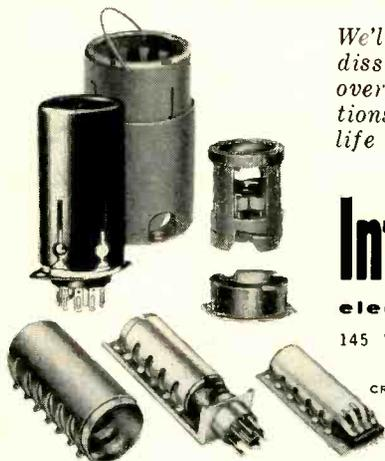
Heat-dissipating electron tube shields for miniature, subminiature octal and power tubes
