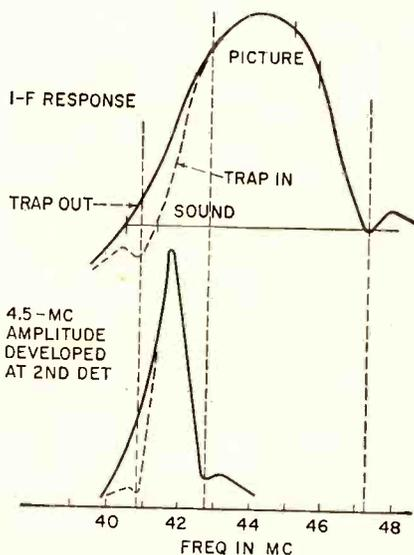
FIG. 4—Intercarrier sound amplitude against oscillator tuning is largely determined by receiver's agc system and characteristics of i-f system
