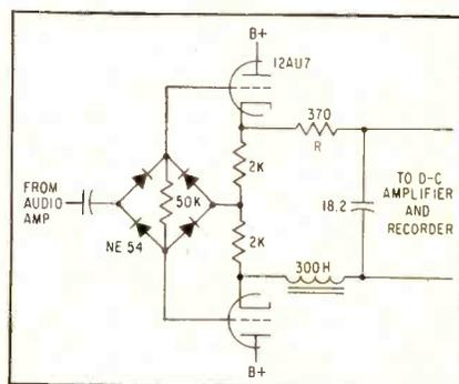
FIG. 3—Circuit used in standard VU recorder includes rectifier said to have characteristics similar to that used in standard VU meters
