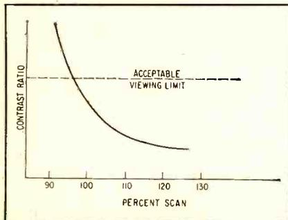
FIG. 1—Contrast ratio plotted against scan indicates loss of contrast with larger raster
