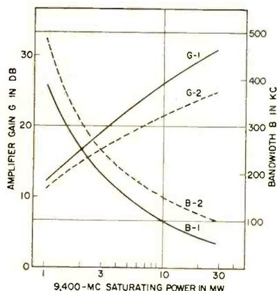
FIG. 8—Solid-state maser amplifier gain-bandwidth characteristics
