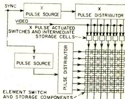
FIG. 5—Switching system for ELF screen
