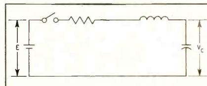
FIG. 2—Underdamped RLC circuit has transient response of standard VU meter
