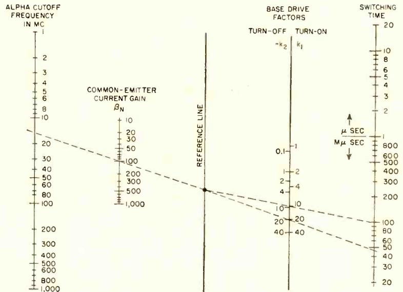
FIG. 2—Both rise and decay times are shown on nomograph scale at far right. Dashed lines show examples described
