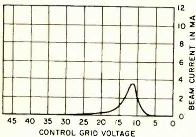
FIG. 7—Control grid voltage against beam current for annular-geometry crt
