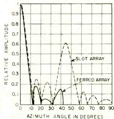
FIG. 8—Comparison of diffraction pattern of 40-element arrays. Rod pattern is superimposed on diffraction pattern of a slot. Only the envelope of maximum points is shown in the curve above
