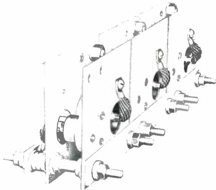
This is a 6-1-1 three-phase full-wave bridge using 322 cells on 5" x 5" copper plates. At an ambient temperature of 30° C it will deliver up to 132 amperes d.c. convection cooled, or 330 amperes d.c. with forced air cooling at 1000 l.f.m. The primary applications are welding, electro-plating, chemical reduction, arc furnaces, motor drive, battery chargers, etc.
