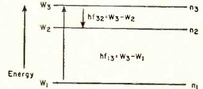
FIG. 2—Energy level diagram for a three-level maser of solid-state type
