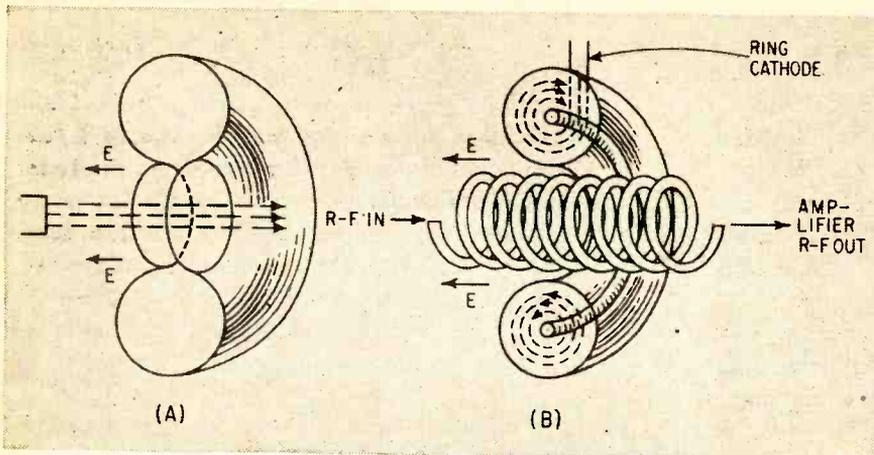
Conventional klystron (A) compared with antiklystron (B) shows duality of mechanical and electronic operation as . . .
