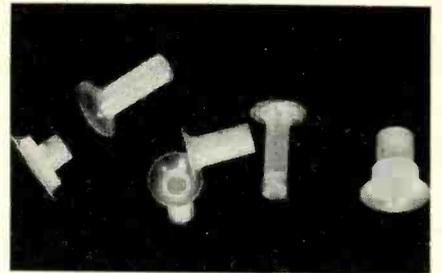
Nylon cones which hold magnetic cores
