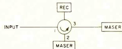
FIG. 12—Maser amplifiers can be cascaded by use of circulator
