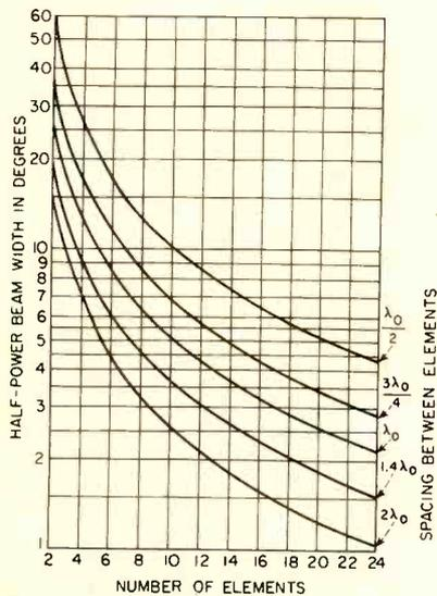
FIG. 2—Half-power beam width plotted as a function of the number of elements and spacing between elements. Elements were linear, phased uniformly and generated equal-amplitude patterns
