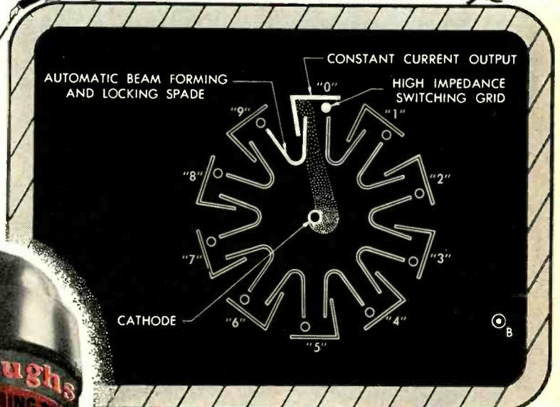
CROSS-SECTION OF BEAM SWITCHING TUBE SHOWING BEAM FORMED
