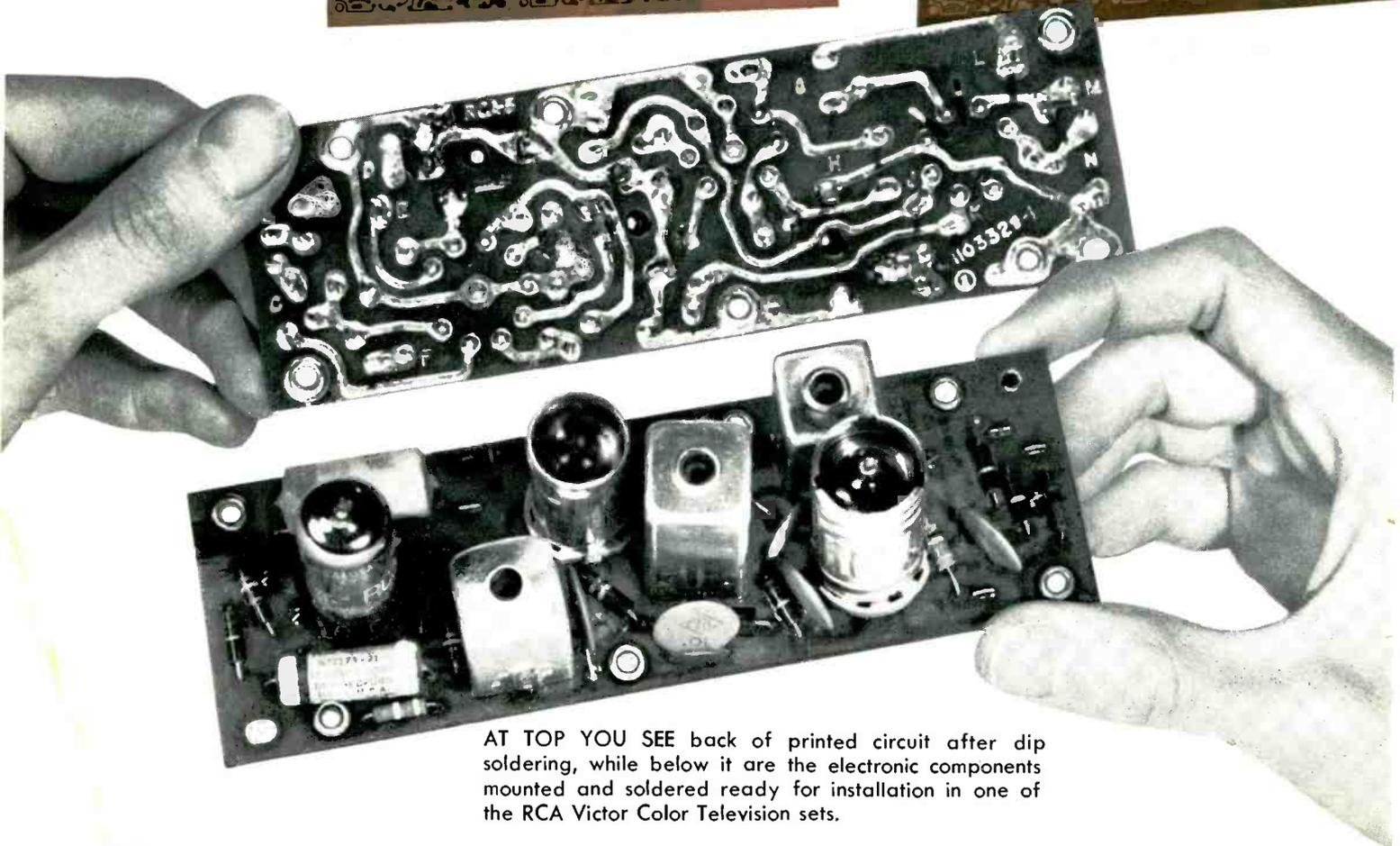
AT TOP YOU SEE back of printed circuit after dip soldering, while below it are the electronic components mounted and soldered ready for installation in one of the RCA Victor Color Television sets.
