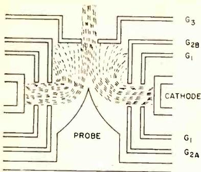
FIG. 6—Cross section of annular-geometry electron gun shows beam path
