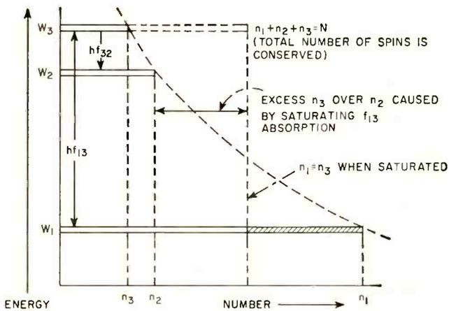
FIG. 3—Spin distribution over three energy levels
