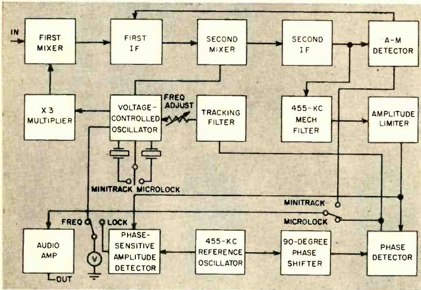
Either 108-mc microlock or 108.03-mc minitrack signals from U. S. satellites can be received and supplied to a tape recorder with this recently announced portable receiver
