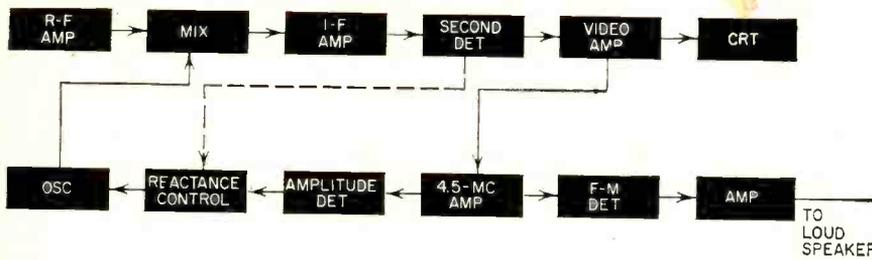
FIG. 1—Block diagram of the intercarrier sound aft control system used in Westinghouse tv receiver
