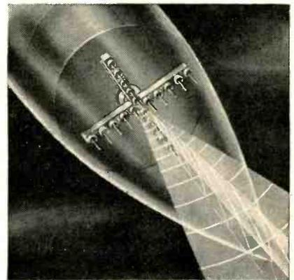
Two ten-element ferrite arrays mounted in ogive section of nose of a guided missile give idea of relative size
