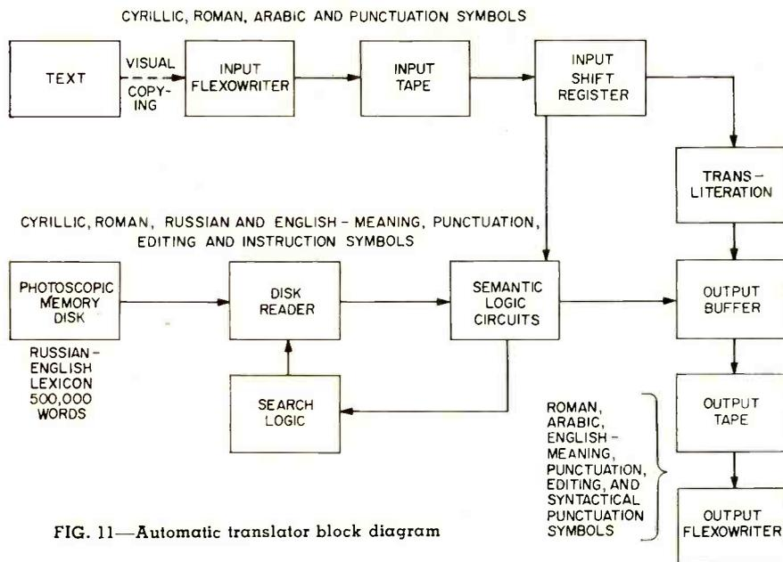
FIG. 11—Automatic translator block diagram
