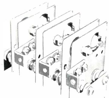
This is a 6-1-1 three-phase full-wave bridge using 302 cells on 3" x 3" copper plates. At an ambient temperature of 30° C, it will deliver up to 61 amperes d.c. with convection cooling, or 132 amperes d.c. with forced air cooling at 1000 l.f.m. The primary applications are d.c. power supplies, vibrator and magnet coil supplies, motor control, etc.
