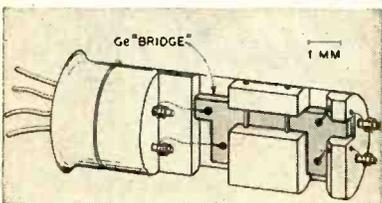
"Germanium Bridge" thermometer is accurate to a few ten-thousandths of a degree in the absolute temperature range
