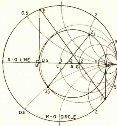
FIG. 1—Characteristic impedance is determined from diagram shown
