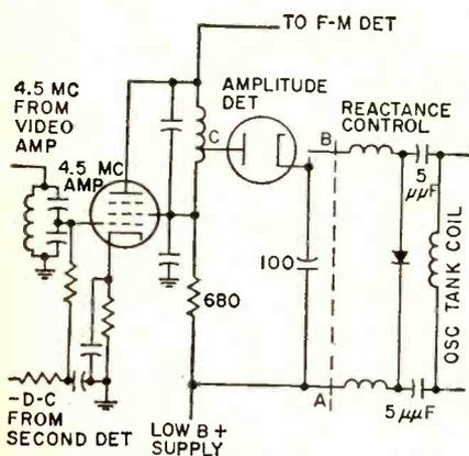
FIG. 2—Basic aft circuit. By opening the loop connection between the amplitude detector and the reactance control, terminals A and B, discriminator and reactance curves can be measured. Both curves give necessary automatic fine tuning information
