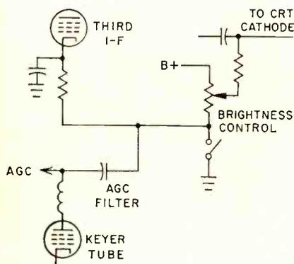
FIG. 10—Circuit shows how aft loop is held open during interchannel switching until the tuner turret falls into the proper detent corresponding to desired channel
