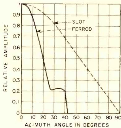
FIG. 4—Diffraction pattern for single ferrite and single slot element. Slot curve is shown for 76-deg half-power beam width; ferrite rod is shown for 28-deg half-power beam width
