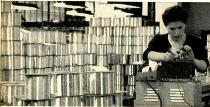
Hudson tests each spool for thickness of Silver Plate—to meet exact specifications.
