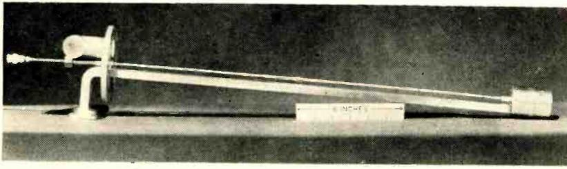
FIG. 6—S-band low-temperature head used for maser amplifier
