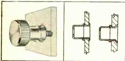
Simplicity of design contributes to clean, distinctive appearance and fast, low-cost installation. Stand-off is slipped into panel hole and secured by flaring. Screw is passed through stand-off and made captive by vinyl o-ring.
