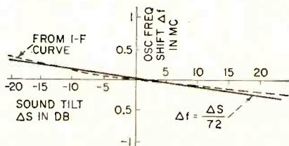
FIG. 11—Oscillator frequency change resulting from change in sound level
