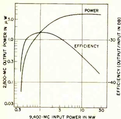
FIG. 10—Maser oscillator characteristics
