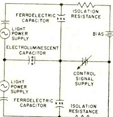
FIG. 4—Equivalent circuit of electro-luminescent-ferroelectric screen
