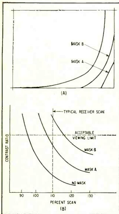
FIG. 3—Two simple masks such as those shown at A improve contrast as shown in plot at B
