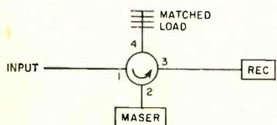
FIG. 11—Circulator provides necessary input and output terminals for reflection-cavity maser described in text.
