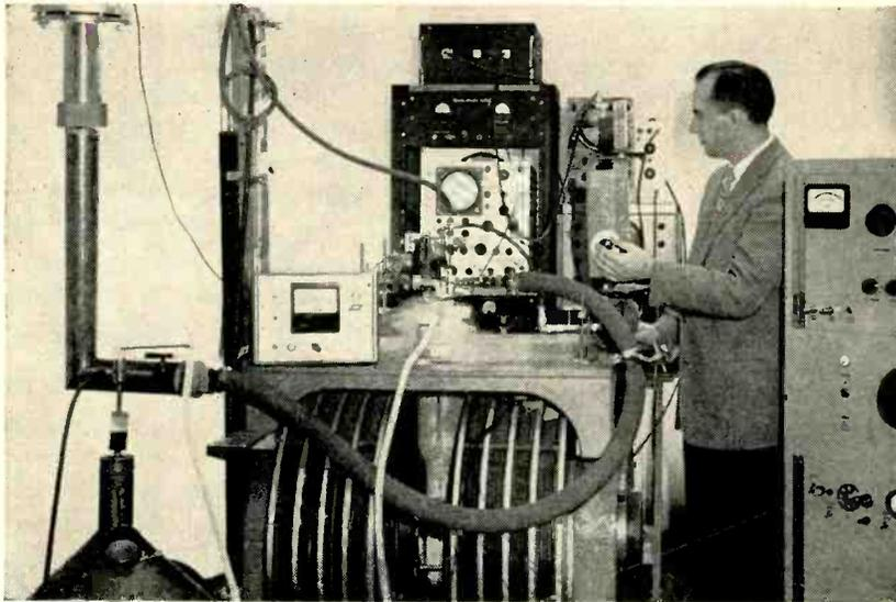
Experimental setup shows maser cavity (center) surrounded by high-voltage field coils
