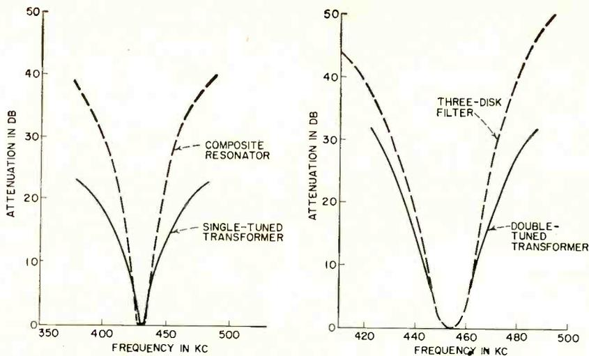
FIG. 2—Selectivity curves for composite resonator compared to single-tuned transformer (A) and three-disk filter compared with double-tuned transformer (B)
