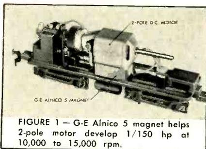
FIGURE 1 — G-E Alnico 5 magnet helps 2-pole motor develop 1/150 hp at 10,000 to 15,000 rpm.
