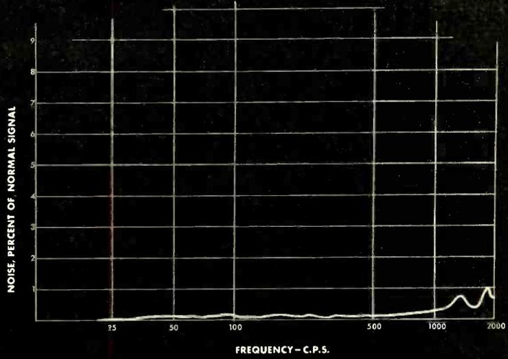
Eimac ceramic 4CX300A undergoing 20G vibration at 20 to 2000 cycles per second.
