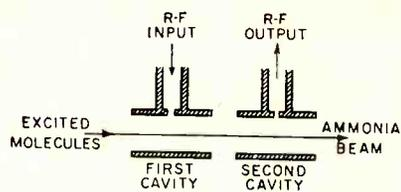
FIG. 8—Cross section of dual-cavity maser shows operating method
