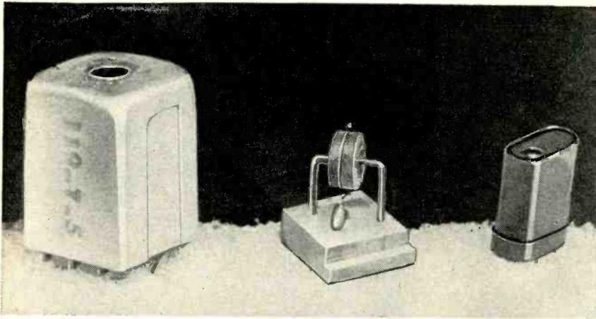
Composite resonator, center, compared with single-tuned transformer, left, and transistor enclosed in case at right gives idea of relative size of components
