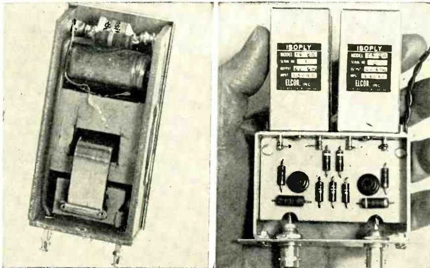
Interior (left) of miniature isolated power supply. Transformer construction gives high degree of isolation. Modular d-c discriminator (right) with two subminiature power supplies operates entirely on a-c power. Discriminator converts input waveform into a rectangular wave or pulse
