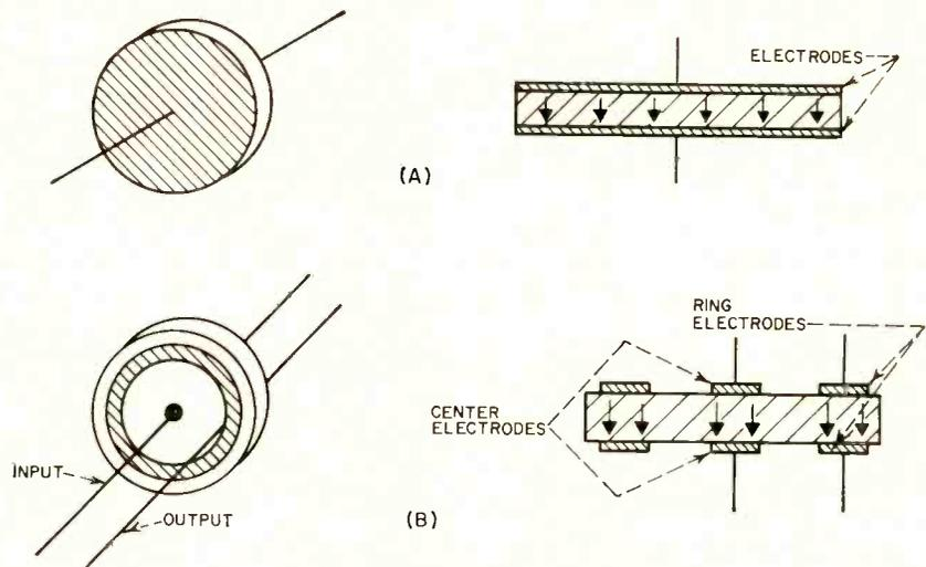
FIG. 1—Two constructions of a barium titanate filter used in tests. In the two-terminal (A) and four-terminal (B) cross sections the arrows indicate direction of polarization
