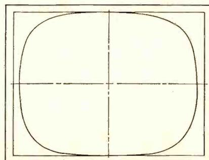
FIG. 2—Screen area of typical tv picture tube shows overlap of 4:3 aspect ratio rectangle
