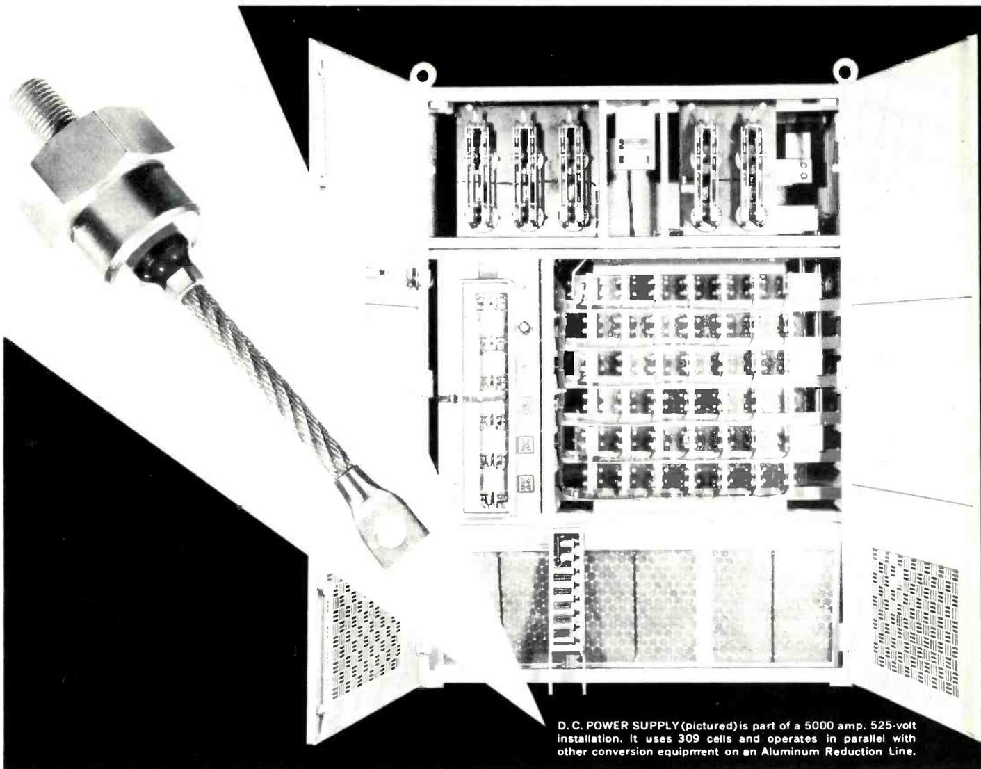
D. C. POWER SUPPLY (pictured) is part of a 5000 amp, 525-volt installation. It uses 309 cells and operates in parallel with other conversion equipment on an Aluminum Reduction Line.
