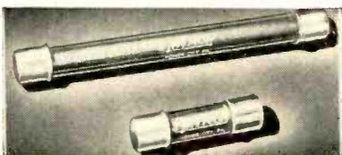
These new voltages are available in three current ratings: 5, 10, and 17 ma (capacitor loads). The containers (either glass tube and ferrule, or phenolic tube) are hermetically sealed, adapting them to continuous operation in salt fog and other adverse atmospheric conditions. **Circle 309 on Reader Service Card.**
