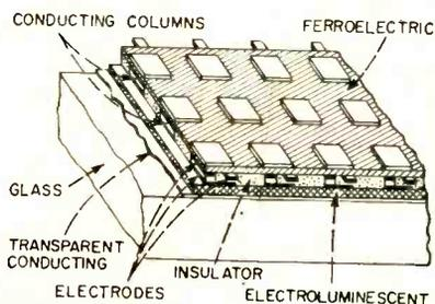
FIG. 3—Cross section of ELF screen
