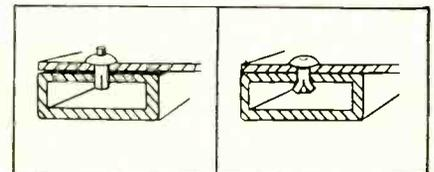
You "hit-the-pin" and the rivet's in. No special tools to limit production or require maintenance, no bucking, no finishing. For blind or open applications, Southco Drive Rivets save time, reduce costs.
