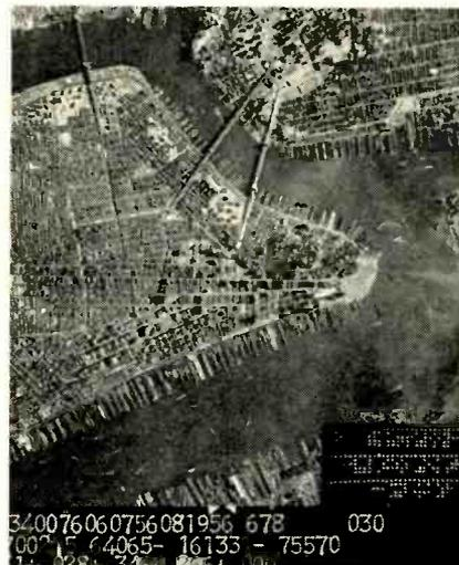
Position, altitude and other pertinent data necessary to U.S. Air Force reconnaissance now can be recorded automatically on photos with a device developed by Federal Telecommunication Laboratories. Digital data recording device records all information in coded-dot form from small crt on photograph. During development, a ground-based reader decodes and prints the data beneath the picture
