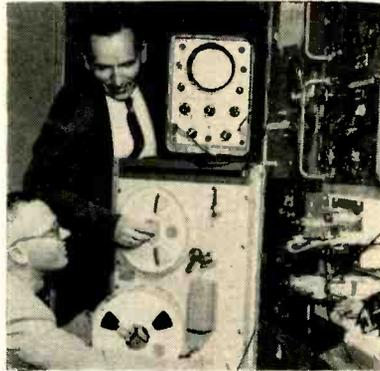
Ampex recorder at Stanford Research Institute picks up radar traces for analysis and later reproduction. Built for atmospheric clutter studies, it has been observing the satellites as well
