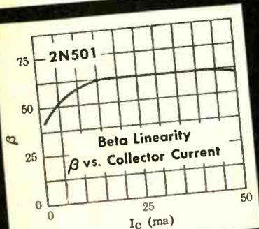
Here is a major breakthrough in the frequency barrier . . . a new family of *field-flow* Micro Alloy Diffused-base Transistors. Philco MADT's extend the range of high gain, high frequency amplifiers; high speed computers; high gain, wideband amplifiers and other critical high frequency circuitry.
