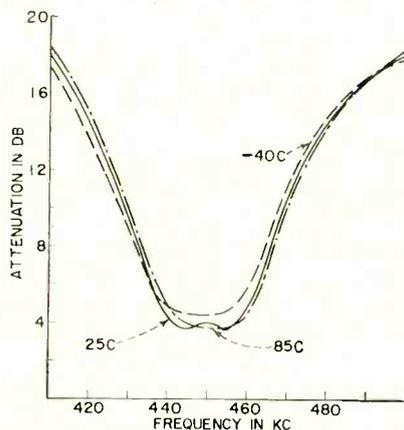
FIG. 3—Frequency selectivity of a two-disk ceramic filter at various temperatures
