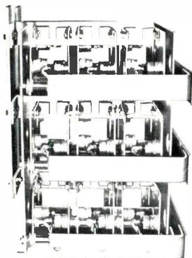
This is a 6-1-6 three-phase full-wave bridge using 322 cells on 5" x 5" copper plates. At an ambient temperature of 30° C, it will deliver up to 780 amperes d.c. with convection cooling, or 1980 amperes d.c. with forced air cooling at 1000 l.f.m. The primary applications are electro-plating, battery forming, arc furnaces, chemical reduction, motor drive, etc.
