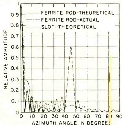
FIG. 7—Comparison of diffraction patterns of 10-element arrays. Actual diffraction pattern of ferrite rod is superimposed on theoretical diffraction patterns for a ferrite rod and slot
