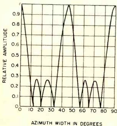
FIG. 3—Diffraction pattern of an isotropic four-element array. Half-power beam width was 11 deg. Elements were phased uniformly and spaced  $1.4\lambda_0$  apart, and generated equal-amplitude patterns
