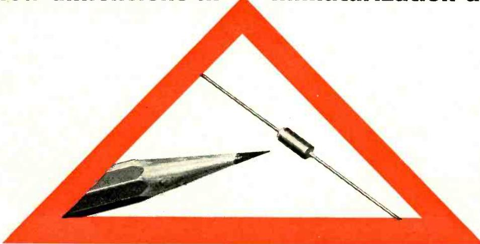
This solid-electrolyte Tantalex Capacitor (shown  $1\frac{1}{2}$  times actual size) is rated at  $4.7\ \mu\text{F}$ , 10 volts d-c, and is only  $\frac{1}{8}$ " in diameter by  $\frac{1}{4}$ " long.
