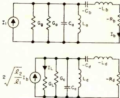
FIG. 9—Equivalent circuit of first cavity (upper) and equivalent circuit for transfer from first cavity to second
