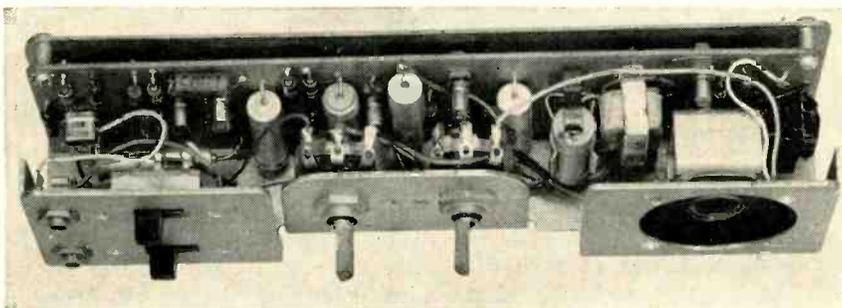
Interior view of chassis shows construction details. Printed circuit and automatic insertion techniques are evident in compact unit
