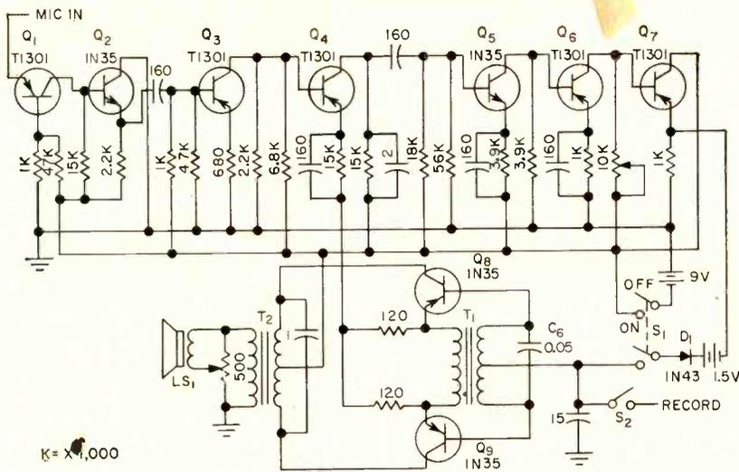
FIG. 1—Circuit schematic of foetal heartbeat detector. Amplifier low-frequency response is enhanced by large time constants in a-c coupled stages to insure that the low-frequency foetal heart signals are amplified
