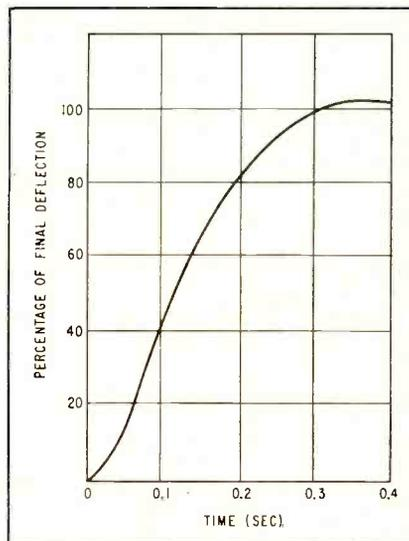
FIG. 1—High-speed motion picture studies indicate response of standard VU meter
