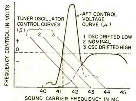
FIG. 3—Circuit of Fig. 2 accomplishes control function illustrated above
