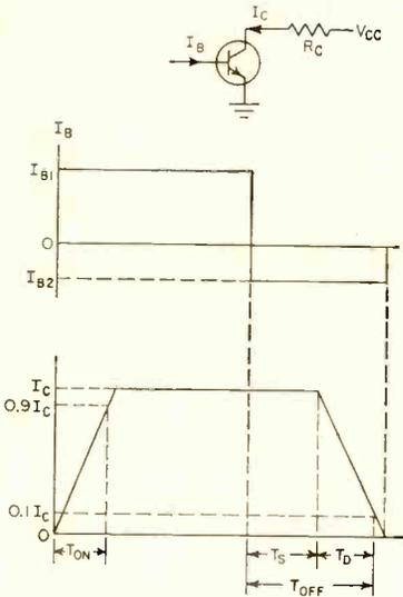
FIG. 1—Common-emitter switching circuit and waveform parameters
