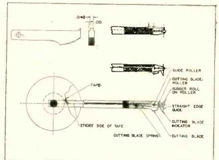
Photographic tape applicator is as long as a wooden pencil
