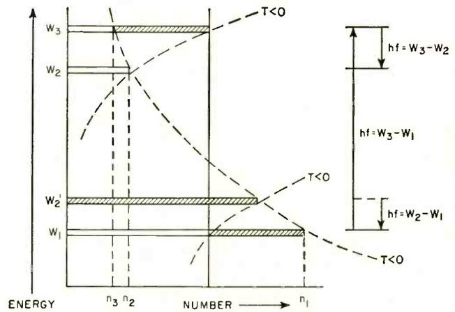
FIG. 4—Spin distribution showing two modes of maser operation
