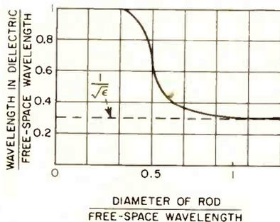
FIG. 1—Effective wavelengths plotted as function of ferrite rod diameter. Curve approaches the factor  $1/\sqrt{\epsilon}$  asymptotically as diameter increases
