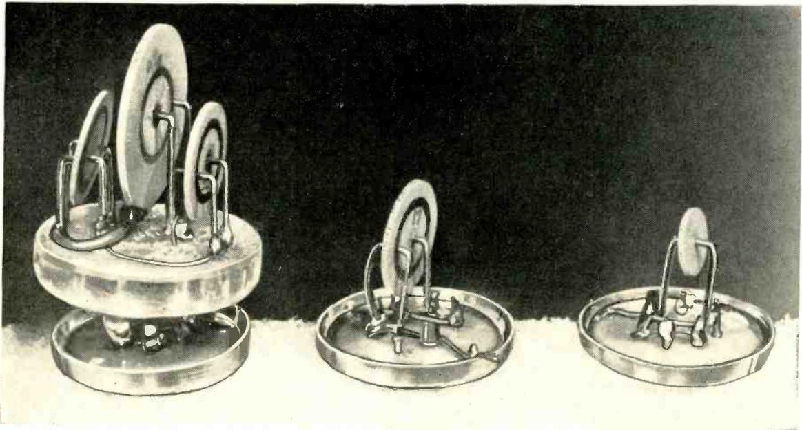
Filters, left to right, are three-disk four-terminal, single-disk four-terminal, and single-disk two-terminal types
