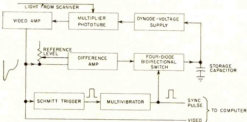
FIG. 10—Nipkow-disk scanning circuit for cytological measurements
