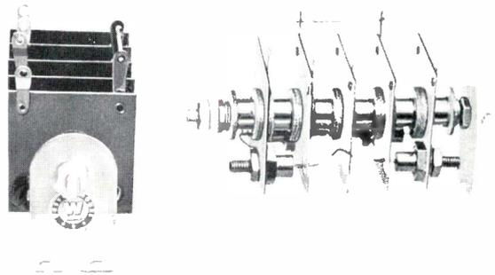
This is a 4-1-1 single-phase full-wave bridge using 305 cells on 1 1/2" x 1 1/2" copper plates. At an ambient temperature of 30° C, it will deliver up to 3.2 amperes d.c. with convection cooling. The primary applications are power supplies, relays, solenoids, mag amps, etc.
