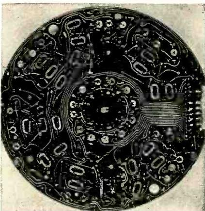
Underside of telemetering card
