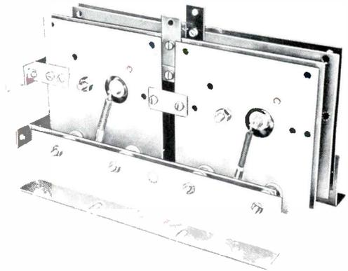
This is a 4-1-2 single-phase full-wave bridge using 302 cells on 5" x 5" copper plates. At an ambient temperature of 30° C, it will deliver up to 94 amperes d.c. with convection cooling, or 178 amperes d.c. with forced air cooling at 1000 l.f.m. The primary applications are d.c. power supplies, vibrator and magnet coil supplies, motor control, etc.
