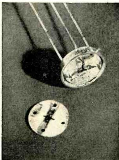
The semiconductor bar is mounted on the wafer and then the wafer is connected to the transistor leads
