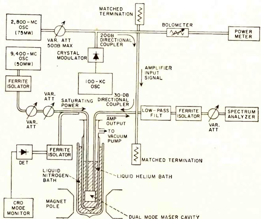
FIG. 7—Experimental arrangement for maser amplifier measurements
