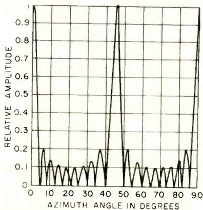
FIG. 6—Diffraction pattern for isotropic ten-element array. Half-power beam width was 3.6 deg. Elements were phased uniformly and spaced  $\lambda_0$  apart, and generated patterns of equal amplitude
