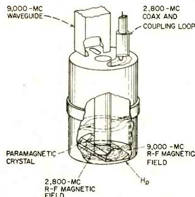
FIG. 5—Dual-frequency maser cavity with magnetic field distribution
