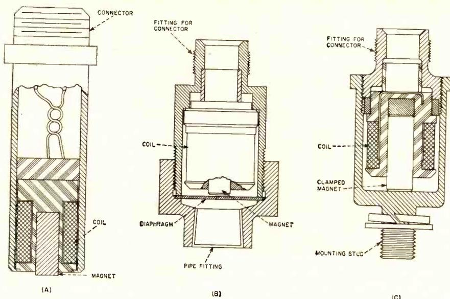
FIG. 2—Crankshaft timing pulse pickup (A) responds to magnetic discontinuities in the flywheel. Pressure pickup (B) responds to rate of change of pressure, while magnetostriction pickup (C) responds to rate of acceleration
