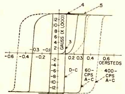
FIG. 3—Magnetization characteristics for high permeability iron
