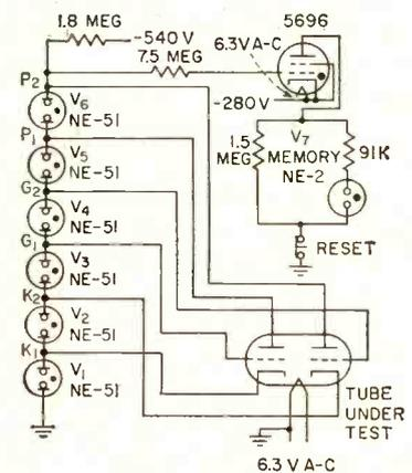
FIG. 1—Simplified short-testing circuit
