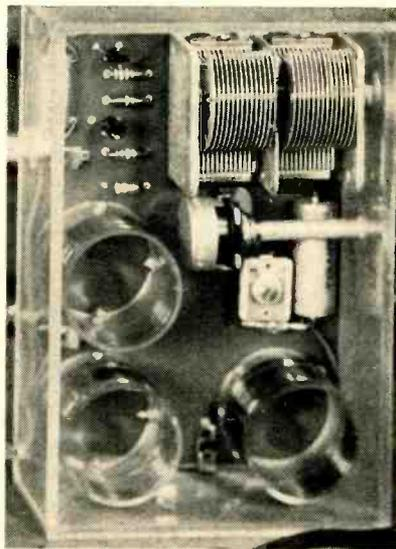
Dual-circuit receiver shown here converts radiations from strong local stations into power necessary to amplify signals from weaker or more distant stations. When both the information and power circuits are tuned to the same station, the signal is amplified by the power derived from the station's r-f carrier
