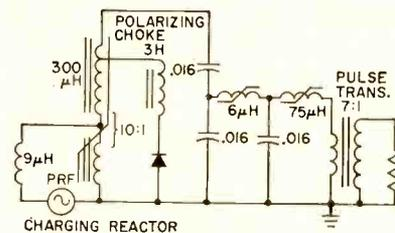
FIG. 6—Amount of polarization changes with operating level making modulator partially self-regulating
