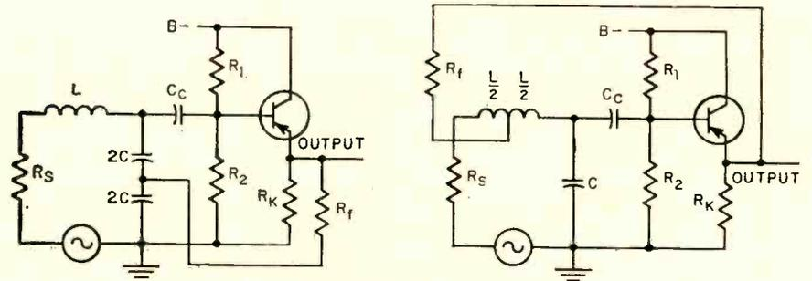
**FIG. 3—Series-tuned circuits overcome shortcomings of parallel-tuned versions**
