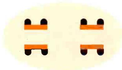
**D** Mica slots are designed with flat alignment surface and channel index to position grids with much greater precision. Closer element spacings are possible where extra Gm is required.
