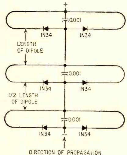
FIG. 2—Multiple dipole antenna. This combination delivered one milliwatt to a 2,500-ohm resistive load when tuned to a 189 mc, 50 kw transmitter located approximately one mile away. A similar array was capable of producing a total of 3 mw of power and charging a 2- $\mu$ f capacitor to 54 v
