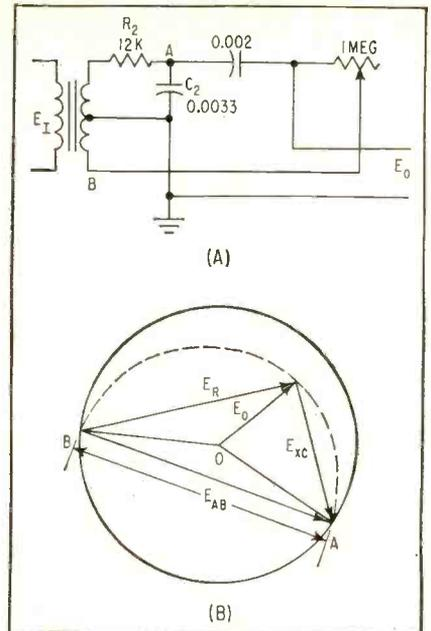
FIG. 2—Phase of output voltage can be varied more than 180 degrees but output voltage is not constant
