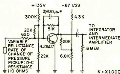
FIG. 3—Schematic of transistor pre-amplifier, the first stage in the analyzer pressure channel. This stage, stabilized by feedback, boosts the pressure pickup output by a factor of 60
