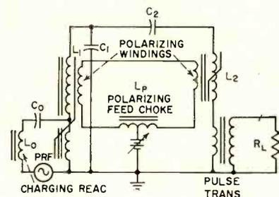
FIG. 7—Magnetic modulator with auto-transformer primary resonance and cancellation feedback
