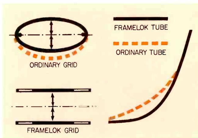
Uniform transfer characteristics of the Framelok Grid tube result largely from greater control of both major and minor dimensions of the grid. Above is a graphic representation of variations in characteristics which result from distortion of the minor dimensions in wound grids. Since both major and minor are fixed in the rigid frame grid, these variations are virtually eliminated.
