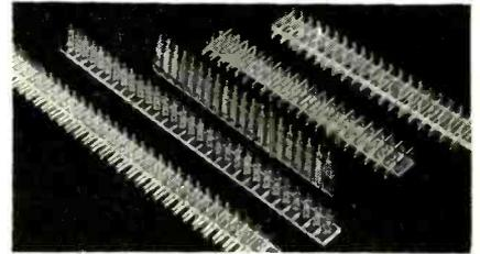
Contacts on plastic strips fit into holes in plate
