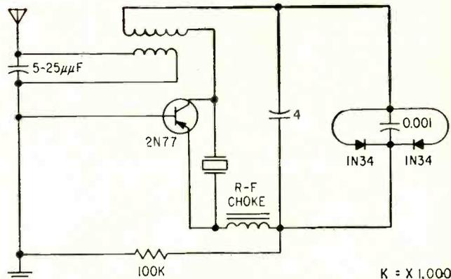
FIG. 4—Transponder. Power received at some specific frequency is used to energize the transistor oscillator at a different frequency thereby making it useful as a device for detecting position of aircraft or any other object capable of housing such a device
