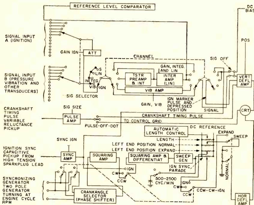
FIG. 1—Block diagram of cro engine analyzer. A sweep is driven across the crt in time with the engine. Resulting trace line displayed is responsive, in the vertical direction, to signals from ignition, cylinder vibration and cylinder pressure. Connections are made to the flywheel, ignition primary circuit, and two to a power cylinder. Timing the analyzer to the engine is done by a fifth pickup located near a mark on the flywheel
