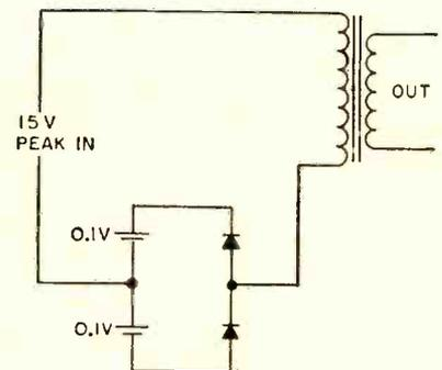
FIG. 1—Elements of biased-diode squelch
