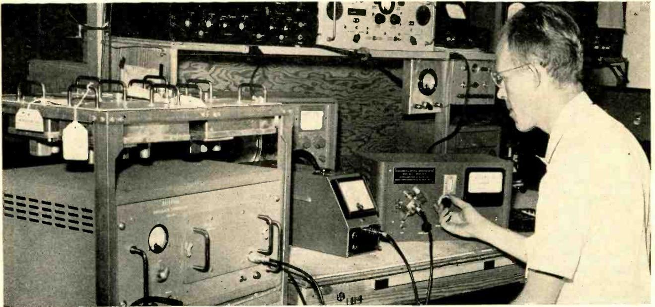
Typical test setup for checking crystals. Crystal under test and cable of electronic null-indicating meter plugged into bridge unit are next to right hand of operator. Counter-type frequency meter at left reads  $r-f$  output frequency of crystal impedance meter into which bridge is plugged. With exception of frequency measuring unit, no auxiliary equipment is required
