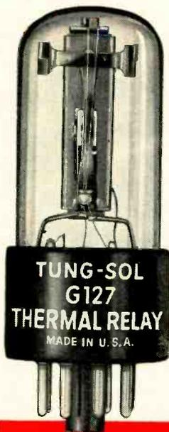
In addition, the G-127 has a calibration change of only .2 volts over a temperature range of -40° to +80° C . . . resists damage from vibration in a range of 10 to 55 cycles and from shock of 50Gs . . . employs snap action contacts for consistent operation. The G-127 is characteristic of the *precision-in-performance* of the entire line of Tung-Sol thermal relays. Whatever your relay requirement, contact Tung-Sol for complete, confidential engineering assistance.
