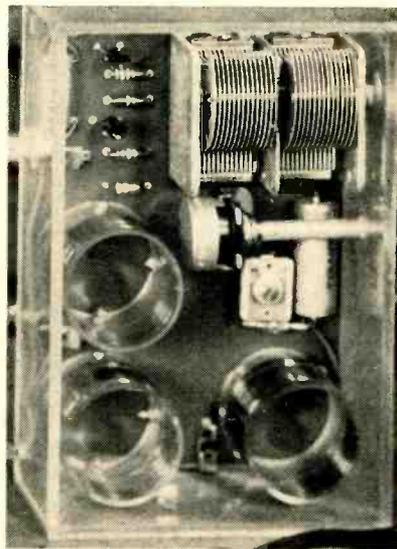
Dual-circuit receiver shown here converts radiations from strong local stations into power necessary to amplify signals from weaker or more distant stations. When both the information and power circuits are tuned to the same station, the signal is amplified by the power derived from the station's r-f carrier
