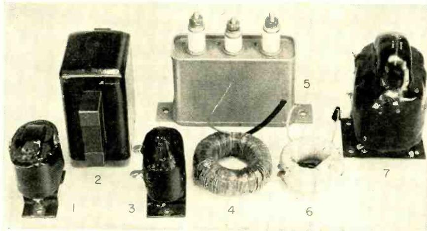
Components for a small magnetic modulator include: charging reactor (1), first saturable reactor (2), polarizing core (3), second saturable reactor (4), charging capacitors (5), third saturable reactor (6) and pulse transformer (7)
