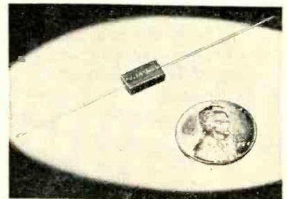
Subminiature capacitor designed to help reduce missile size and weight
