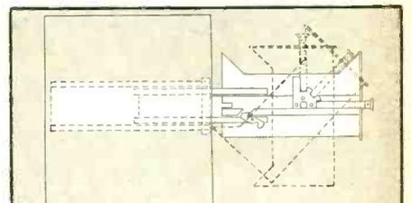
The MARK II offers tilt and locking devices as well . . . your unit can be pivoted to plus 45 and 90 degree positions for greatest accessibility. And you'll be amazed at the moderate cost of the Mark II . . . how quickly it will pay for itself by allowing your equipment to be serviced and maintained in 'jig-time instead of down-time!
