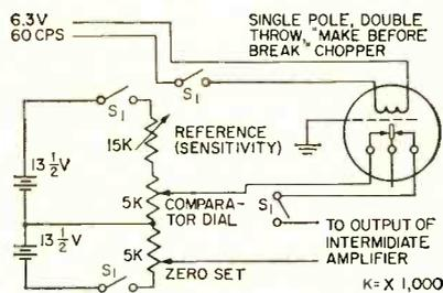
FIG. 4—Schematic of reference level comparator, used to measure relative amplitudes on crt. The comparator potentiometer and dial permit reading of deflection in terms of linear scale divisions
