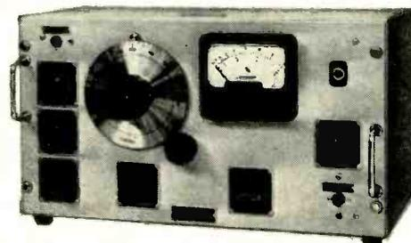
Total distortion, harmonics, and hum measured separately. Meter readings are all r.m.s. values. This instrument makes distortion measurements easy, fast and dependable.
