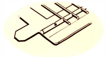
**B** Sylvania's new Framelok construction eliminates brazing and adapts the frame grid to automatic production. Grid halves are perfectly flat—free from thermal strains.
