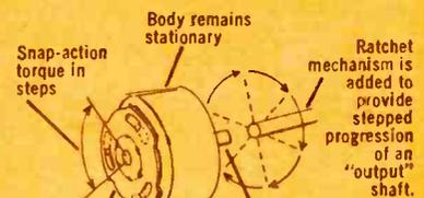
"Solenoid" shaft oscillates with armature... can be supplied at front or rear... other power take-off arrangements also possible.
