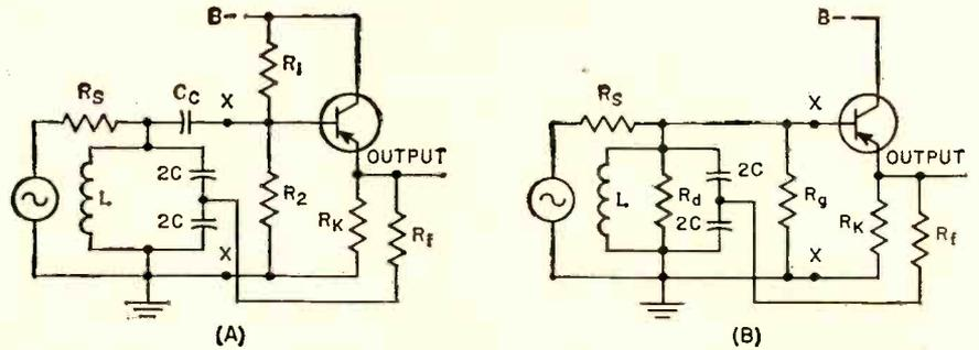
**FIG. 2—Transistor equivalent of vacuum-tube version (A) and idealized circuit (B)**
