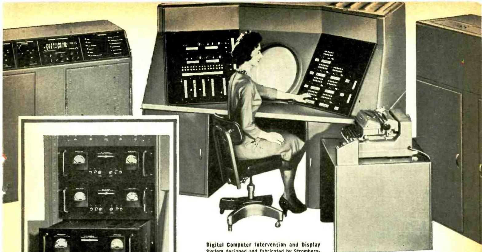
Digital Computer Intervention and Display System designed and fabricated by Stromberg-Carlson Company, a Division of General Dynamics Corporation, for the Air Proving Ground Center (ARDC) Armament Division, Eglin Air Force Base. The system is built around the CHARACTRON\* Shaped Beam Tube, designed by Stromberg-Carlson for high-speed information display and micro-film recording.
