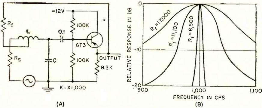
FIG. 4—Varying  $R_f$  of selective a-f amplifier (A) changes circuit Q-multiplication (B)
