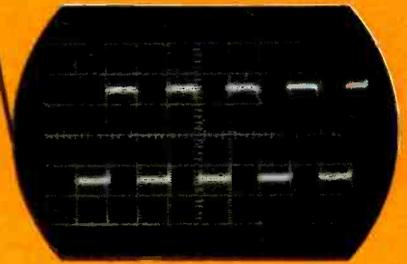
Square-Wave (2,500 Ω) Output: 0-30v peak to peak; rise time approximately 1/3 μsec; overshoot approximately 1%; hum at least 60 db below output-voltage level.
