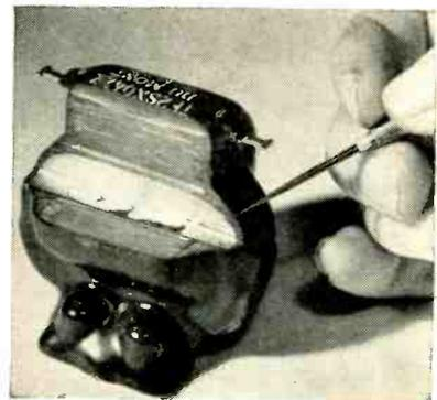
Low viscosity of epoxy encapsulation material gives exceptionally good impregnation of transformer core. Better heat transfer and moisture protection result from the deep impregnation. Thermal shock from  $-55$  to  $+85$  C will not cause encapsulation to crack
