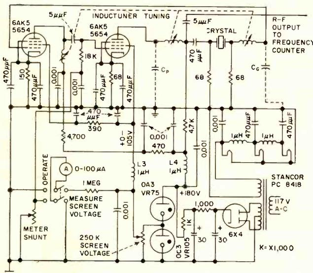
FIG. 2—Circuit of development crystal impedance meter, which may be used conventionally with test crystal in position shown, or in new method by inserting bridge in place of crystal. Rear view of instrument is shown alongside circuit
