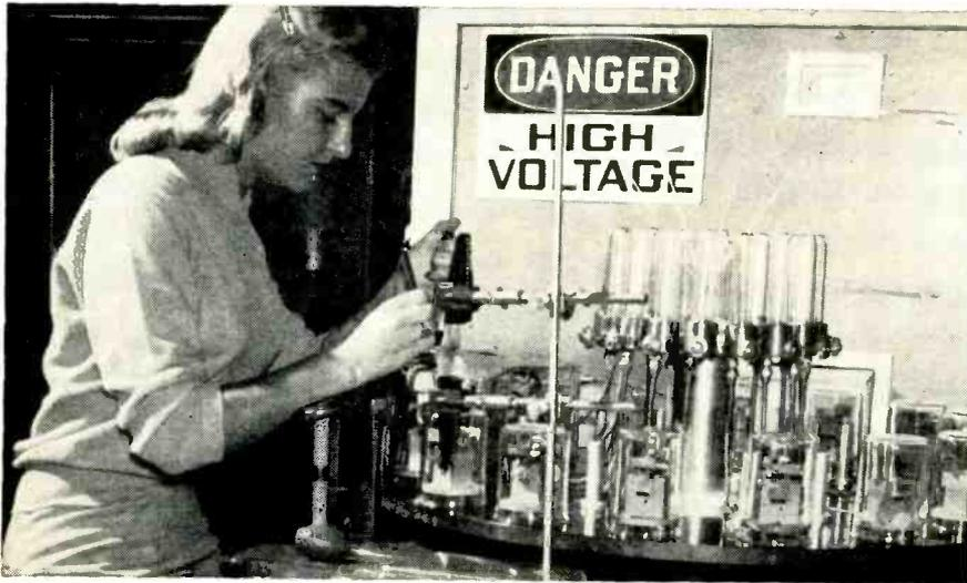
Wheel-like machine simplifies hand sealing operation. Tubes are heated at operator's left and cooled at right. Radioactive brush to clean mica windows is in foreground
