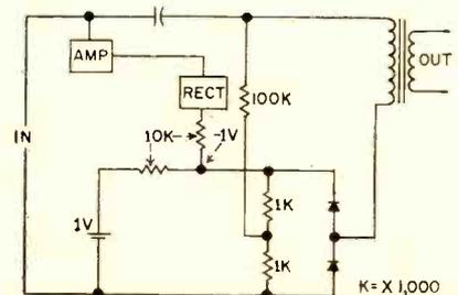
FIG. 2—Basic distortion-reduction circuit
