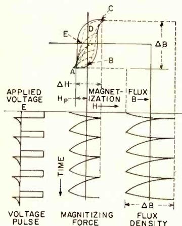
FIG. 5—Pulse permeability under the influence of a negative polarizing field
