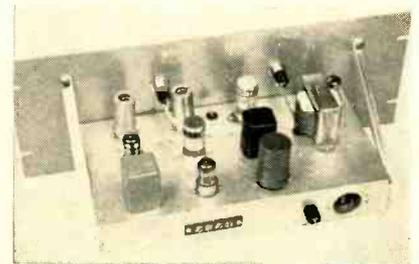
In-line mounting of plug-in components improves appearance, simplifies service
