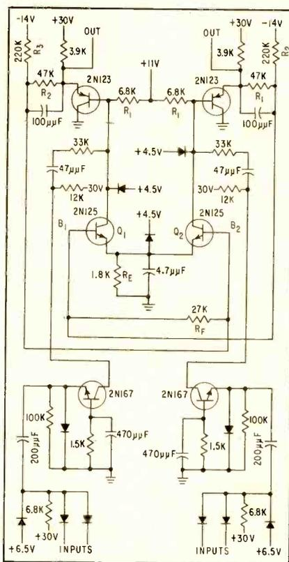
FIG. 1—Feedback resistor  $R_f$  in flip-flop makes it less sensitive to voltage variations and transistor unbalance
