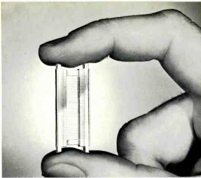
Many grids look like one! The inherent alignment capabilities of Sylvania's Framelok Grid are demonstrated by the ease with which the laterals of any number of separate grid
