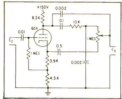
FIG. 4—Use of tube in place of transformer permits phase shifter to handle a wider band of frequencies
