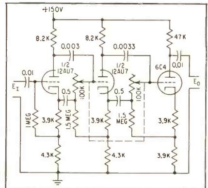
FIG. 5—More than 180 degrees of phase shift and very constant output voltage is provided by two-tube shifter
