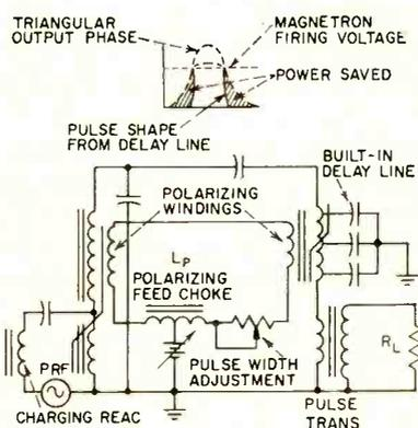
FIG. 8—Built-in delay line squares up triangular pulse normally generated in last stage of magnetic modulator
