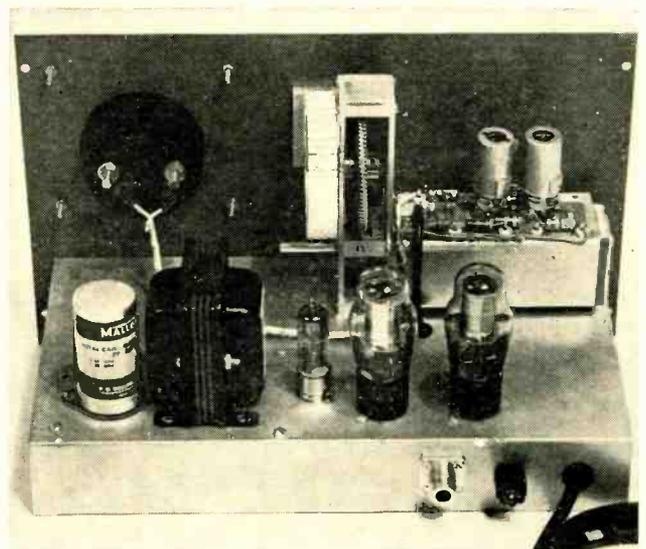
dissipated in the crystal. The frequency of the oscillator is varied by tuning through a suitable gear reduction to provide the necessary vernier adjustment. A sensitive d-c meter is provided, with a variable shunt, to indicate relative activity at high as well as at low drives. A coaxial jack provides a sample of the r-f energy for frequency-measuring purposes. The entire unit is encased in a steel cabinet for shielding and protective purposes.
