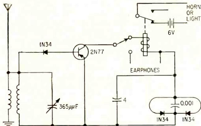
FIG. 3—Emergency receiver and alarm device. By pretuning information circuit to Conelrad's 640 or 1,240-kc emergency frequencies, civil defense broadcasts can be received regardless of availability of local power sources
