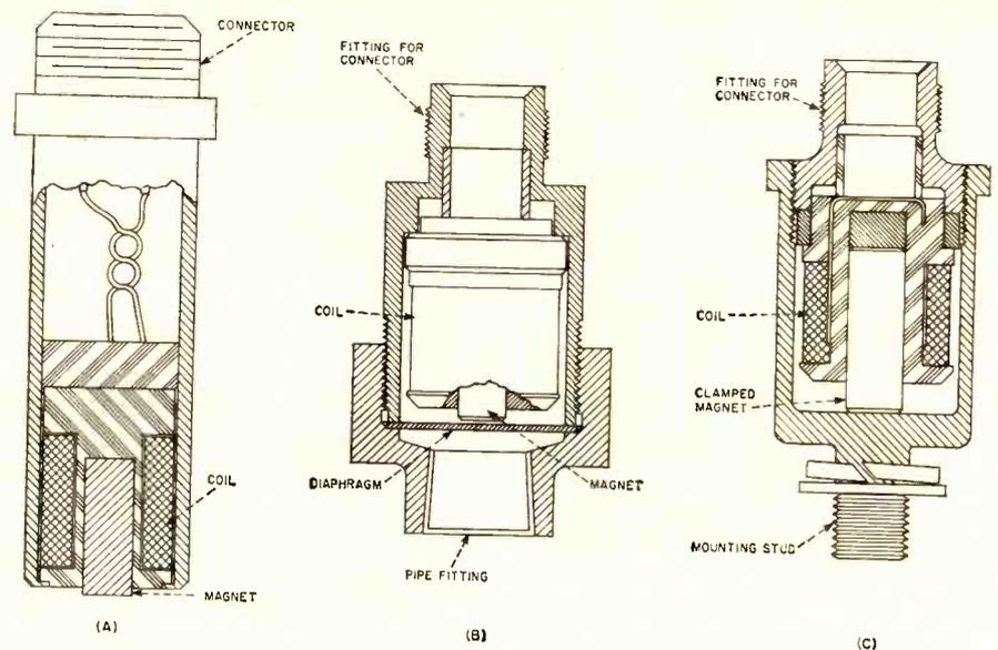
FIG. 2—Crankshaft timing pulse pickup (A) responds to magnetic discontinuities in the flywheel. Pressure pickup (B) responds to rate of change of pressure, while magnetostriction pickup (C) responds to rate of acceleration
