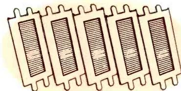
Sylvania's unique technique of frame grid construction makes it possible to duplicate grid after grid. More uniform spacings produce a more uniform electrostatic field in the tube.
