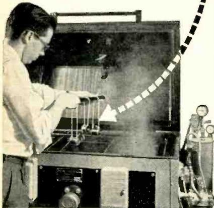
Exposure . . . to the equivalent of a stiff sea spray . . . on a hot, humid day—one more test the G-M Servos take in stride.
