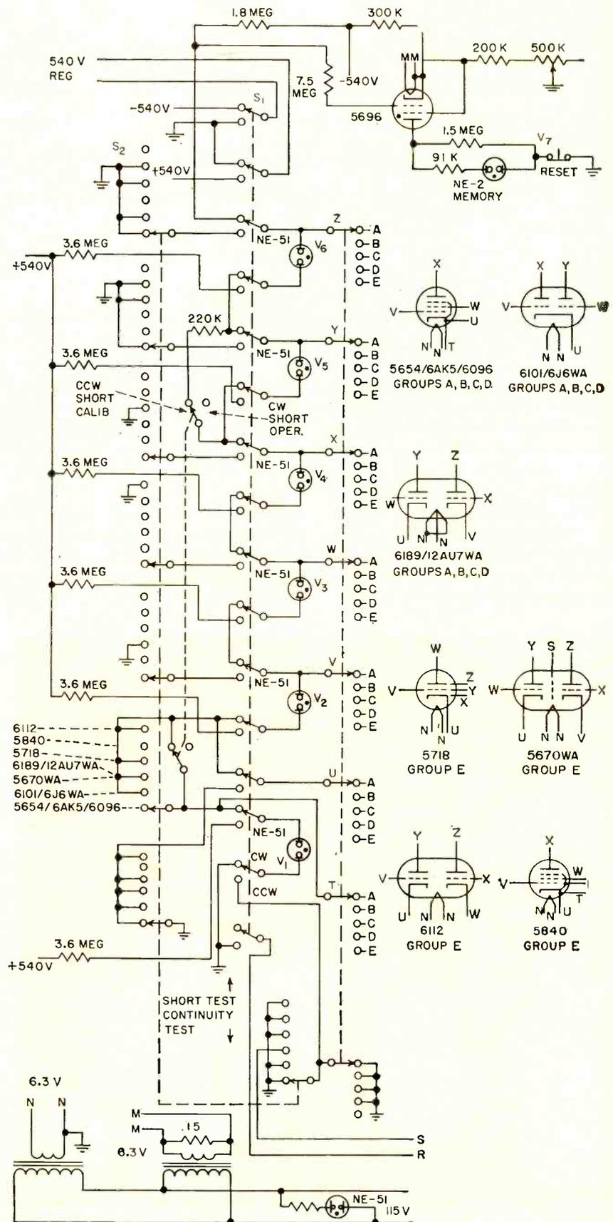
FIG. 3—Complete circuit diagram and tube connections for short and continuity tester
