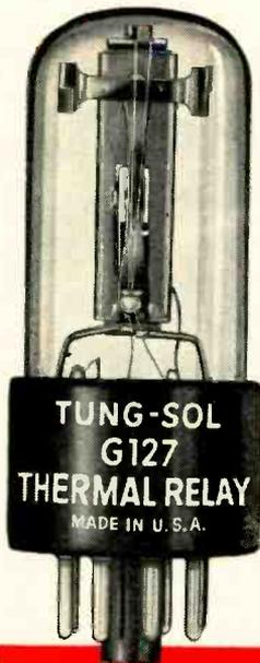
In addition, the G-127 has a calibration change of only .2 volts over a temperature range of  $-40^{\circ}$  to  $+80^{\circ}$  C . . . resists damage from vibration in a range of 10 to 55 cycles and from shock of 50Gs . . . employs snap action contacts for consistent operation. The G-127 is characteristic of the *precision-in-performance* of the entire line of Tung-Sol thermal relays. Whatever your relay requirement, contact Tung-Sol for complete, confidential engineering assistance.
