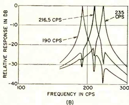
FIG. 5—Three channels of multichannel selective a-f amplifier (A) use coil and capacitor combinations in Table I for staggered resonant frequencies (B)
