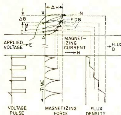
FIG. 4—Continuous plot of magnetizing force and flux density before magnetic conditions stabilize
