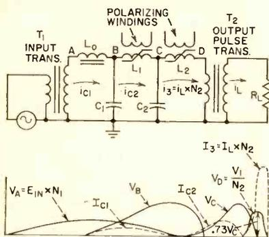
FIG. 1 — Polarized two-stage magnetic modulator with current and voltage waveforms for each reactor resonant stage
