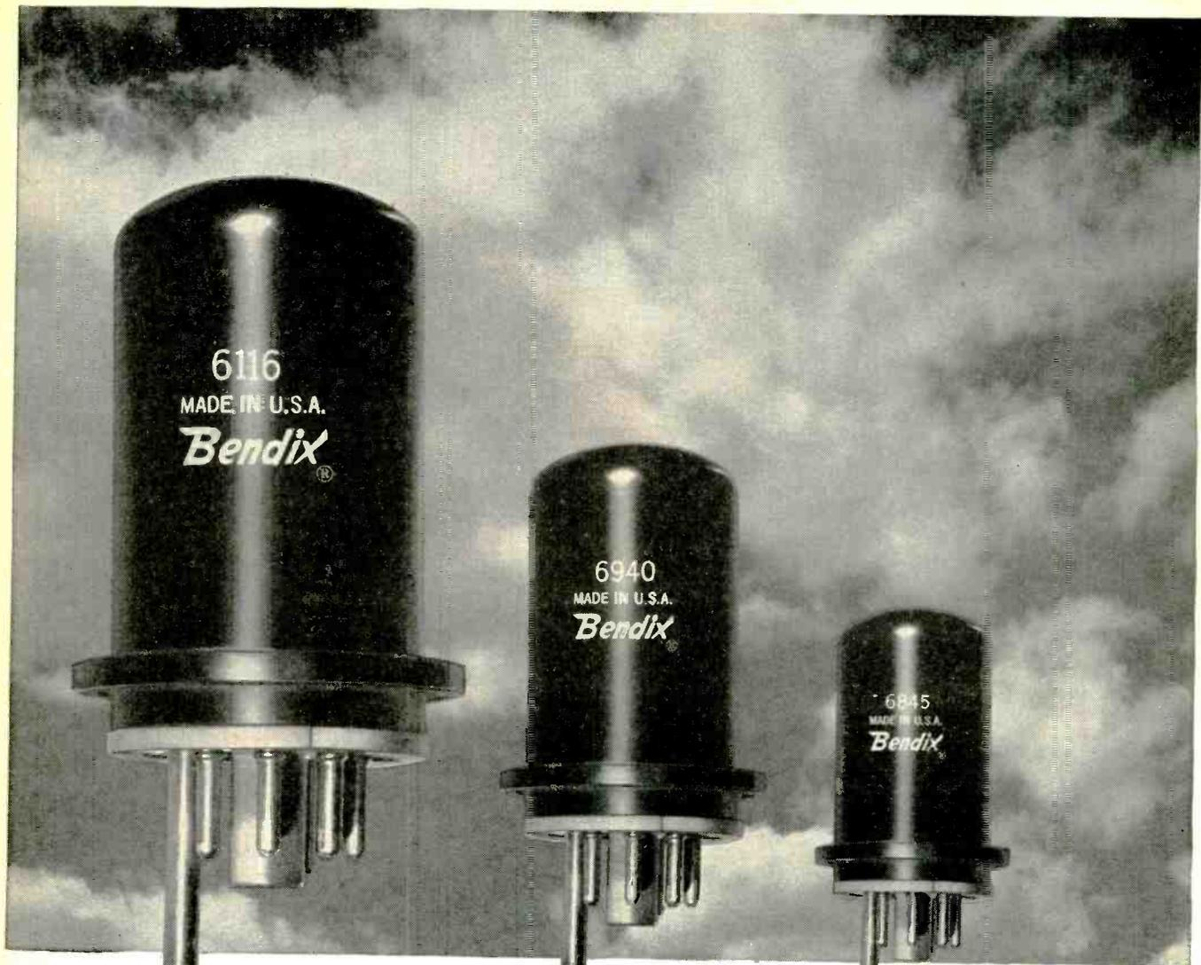
The 6116/TE-39 ruggedized Reflex Klystron thermally tunes a band of 8500 to 9660 MC by means of a diode within the vacuum envelope. Tuning speed over the required frequency range is 0.7 seconds min. to 3.0 seconds max.
