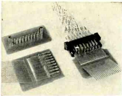
Other side of support plates, with taper tab and stand-off contacts
