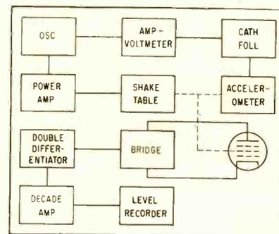
FIG. 1—Accelerometer is used as a sensing device to maintain constant acceleration of shake table as it is swept in frequency
