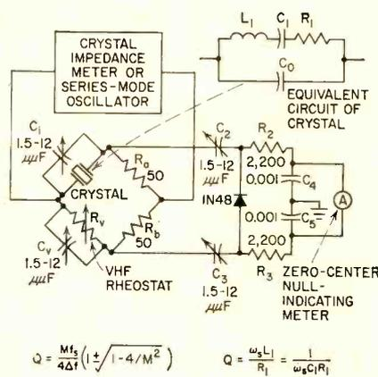
FIG. 1—Bridge circuit and equations used with test results to give desired parameters. Bridge plugs into crystal socket of impedance meter or oscillator
