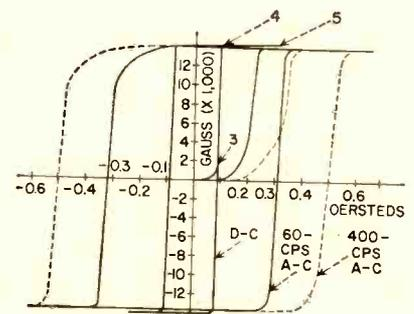
FIG. 3—Magnetization characteristics for high permeability iron
