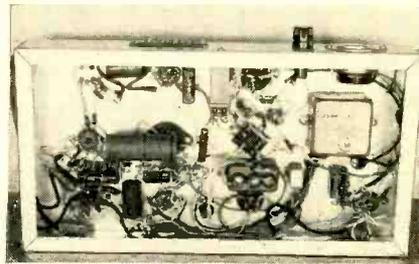
Readily-available parts are used and wiring is conventional point-to-point
