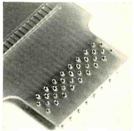
After contacts are staked and excess conductor cut off, plate is ready for solder
