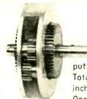
1 to 1 reverse ratio; 48 teeth on input and output gear, 1-1/32 inch diameter. Total outside diameter 1-25/32 inches. Shaft size is 1/4 inch. One shaft is 9/16" long; other
