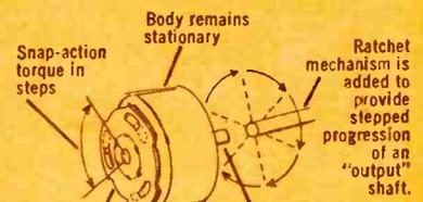
Armature plate rotates through predetermined angle then springs back to original position.
