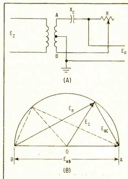
FIG. 1—Constant output voltage is produced by simple phase-shifting circuit with a theoretical range of 180 degrees
