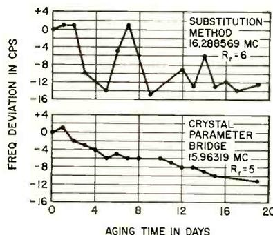
FIG. 3—Comparison of results obtained with older substitution method and new crystal parameter bridge method, when checking aging of crystals. High accuracy of new method gives smoother curve more nearly representative of true behavior of crystal
