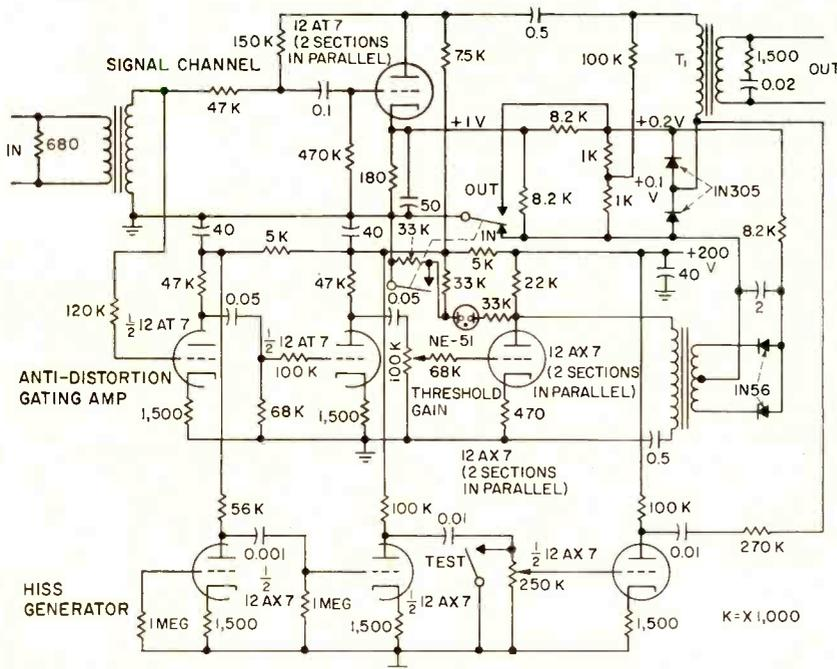
FIG. 3—Circuit of print-through suppressor. In-out switch permits operation as straight amplifier and test switch shorts output of hiss generator for A-B test
