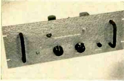
All functional controls appear on front panel except power switched in rack
