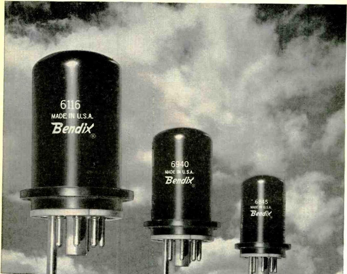
The 6116/TE-39 ruggedized Reflex Klystron thermally tunes a band of 8500 to 9660 MC by means of a diode within the vacuum envelope. Tuning speed over the required frequency range is 0.7 seconds min. to 3.0 seconds max.
