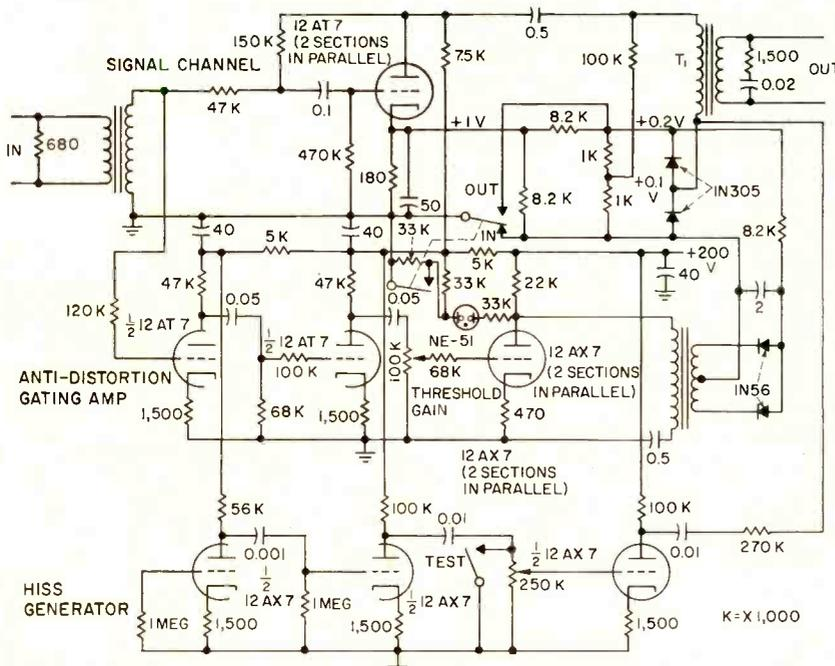
FIG. 3—Circuit of print-through suppressor. In-out switch permits operation as straight amplifier and test switch shorts output of hiss generator for A-B test
