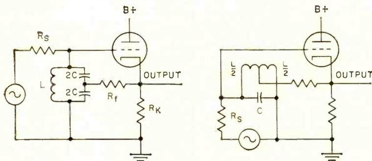
FIG. 1—Vacuum-tube Q-multiplier circuits use center-tapped coil or capacitor divider
