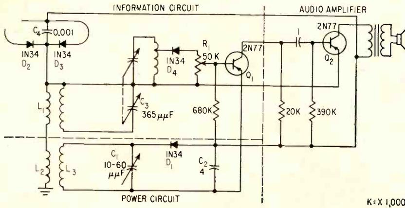
FIG. 1—Broadcast receiver. Specially constructed tuning coils are used but can be replaced by standard coils. Antenna and power circuits are designed to operate at all communications frequencies
