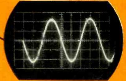
High-Impedance (12.5 KΩ) Output for Loads of 10 Kiloohms and Higher: No-load output is 0-45 v, constant to within ±1 db from 200 c to 150 kc; no-load distortion less than 5% from 200 c to 200 kc (distortion reduced under load); hum at least 50 db below maximum output level.
