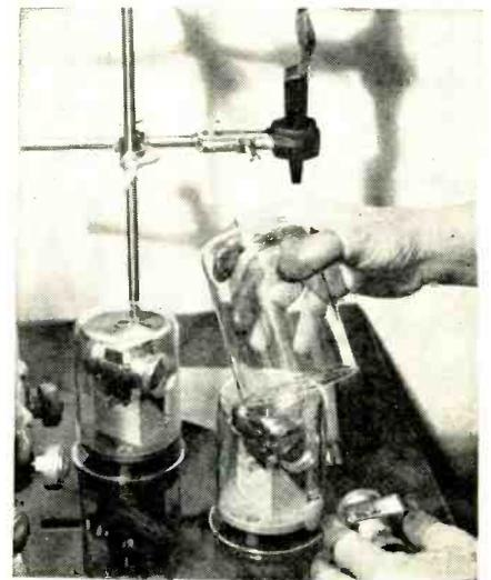
Tubes are placed in metal heat concentrators after windows are positioned
