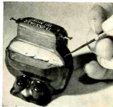
Low viscosity of epoxy encapsulation material gives exceptionally good impregnation of transformer core. Better heat transfer and moisture protection result from the deep impregnation. Thermal shock from  $-55$  to  $+85$  C will not cause encapsulation to crack
