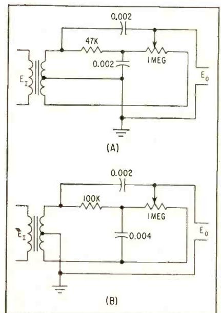
FIG. 3—Output voltage for these circuits is more nearly constant
