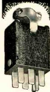
Socket contacts phosphor bronze cadmium plated. Plug contacts hard brass cadmium plated. Insulation molded bakelite. Plugs and sockets polarized. 2, 4, 6, 8, 10, 12 contacts. Steel caps with baked black crackle enamel.
