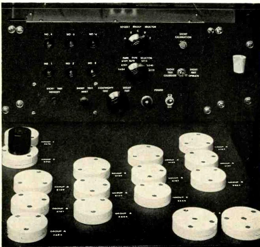
Three groups of four long-life tube sockets are used for most-required types. Octal adapter is used for subminiature types. Cork hammer aggravates tap shorts
