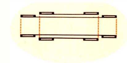
**A** Straight line geometry of grid side-rods in present grids is considerably weaker than the double-box configuration formed by frame grids. Distortion due to mount "twist" is virtually non-existent in the frame grid structure.
