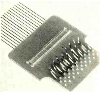
Bare conductors fed through holes of contact plate
