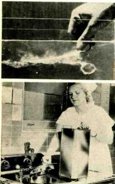
DRIED BLOOD, bits of tissue and other soils on surgical instruments are removed by cavitation caused by ultrasonic sound waves (upper photo) generated in a new medical washing machine (lower photo) manufactured by Acoustica Associates, Inc., of Mineola, N. Y.
