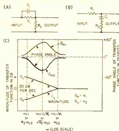
FIG. 1—Lead and lag networks at (A) and (B) result in gains shown at bottom of C and phase angles shown at top of (C)
