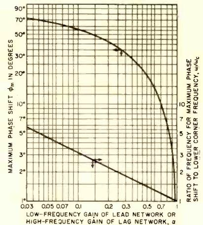
FIG. 2—Relationship of phase shift to gain enables user to determine  $\omega/\omega_c$
