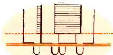
**C** Self-alignment is accomplished in the Framelok Grid through precise control of the distance between the mica and the first grid lateral wire. These tolerances in the frame grid are held in the order of one tenth of one thousandth of an inch—considerably tighter than ordinary grid tolerances.
