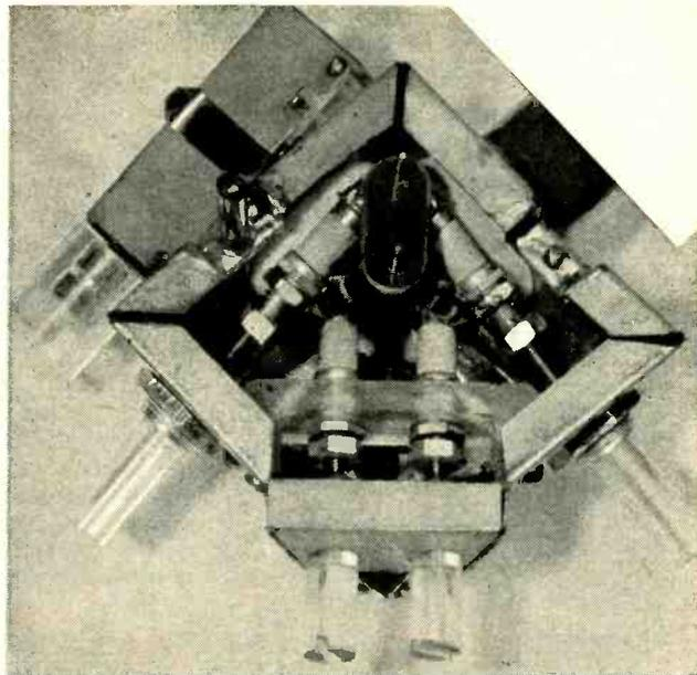
Top and bottom views of plug-in bridge unit. Slotted clear plastic rods permit adjustment of variable resistor and capacitors in bridge. Crystal is at upper right, vhf resistor at upper left,  $C_2$  and  $C_3$  adjustments at bottom center and  $C_0$  and  $C_1$  adjustments at lower left and right respectively in bottom view. Unit permits measurement of all equivalent circuit parameters of a quartz crystal
