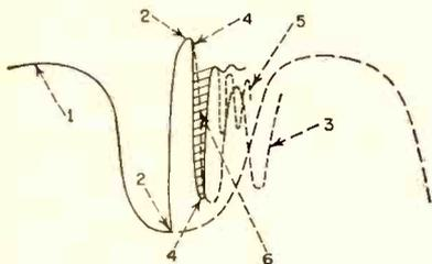
FIG. 2—Switching and ringing waveforms. Resonant input sine wave (1), flattened by polarization first switching (2), ringing which would occur due to first switching (3), second switching (4), ringing which would occur due to second switching (5), and output pulse (6)
