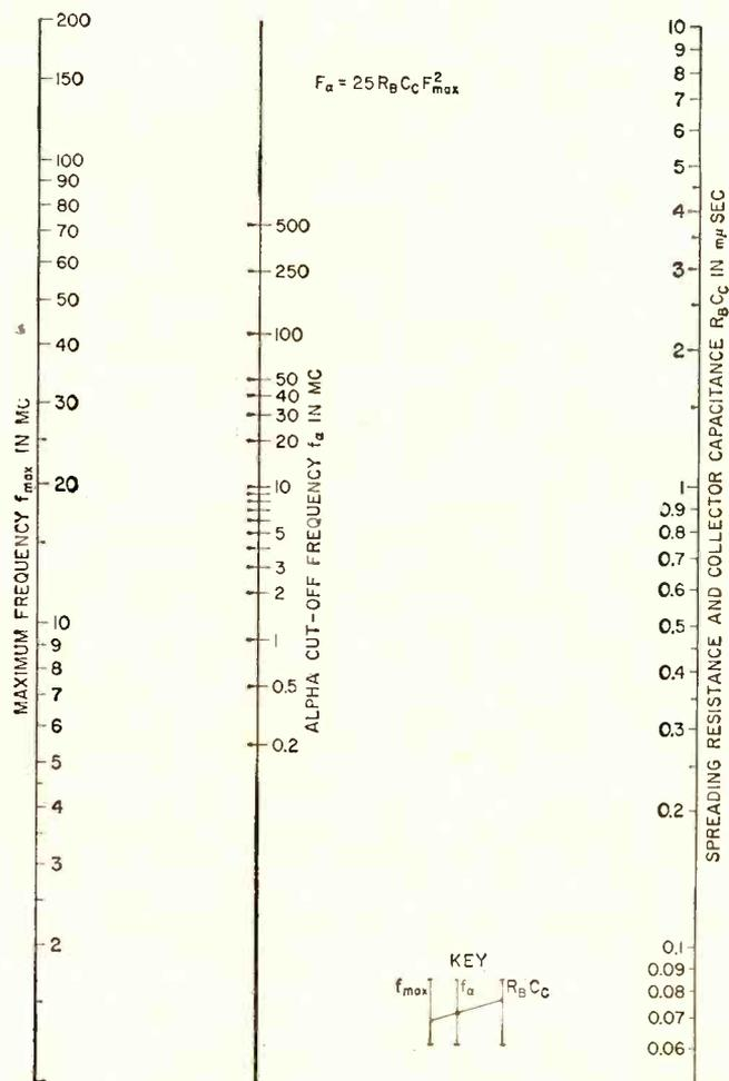
Nomograph for converting transistor high-frequency parameters
