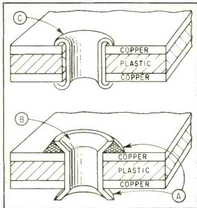
Funnel Flange eyelet permits easier component lead insertion (B); and solder fillet (A) gives a more reliable structure than rolled-head (C).
