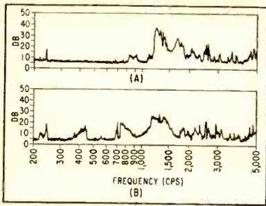
FIG. 2—Comparison of recordings with capacitance bridge between cathode and plate (A) and between cathode and screen grid (B) indicate frequencies at which cathode vibrates
