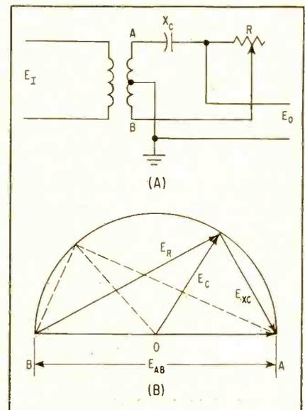
FIG. 1—Constant output voltage is produced by simple phase-shifting circuit with a theoretical range of 180 degrees
