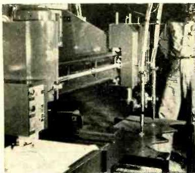
No templates are needed by electronic tracer control which scans line drawings and steers steel-cutting torches. Tracer system consists of vibrator-type scanner, phototransistor and a closed-loop servo. Unit was developed by Canadian Westinghouse, Ltd., for National Cylinder Gas Company
