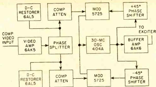
FIG. 2—Frequency deviator has feedback-controlled oscillator
