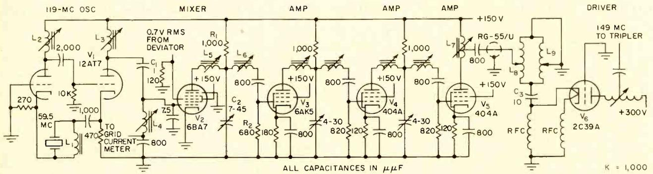
FIG. 3—Transmitter exciter consists of local oscillator, mixer, three amplifier stages and driver that provides 3-w to tripler stage
