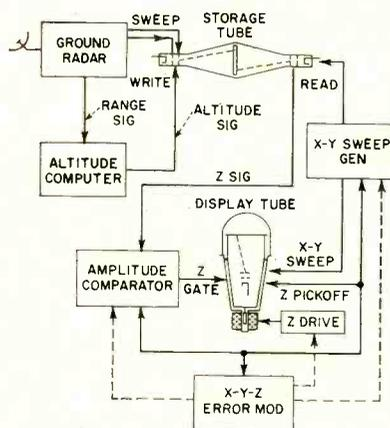
FIG. 4—One method of translating altitude and position data from the airport radar into a three-dimensional display. Error signals are shown in dashed line
