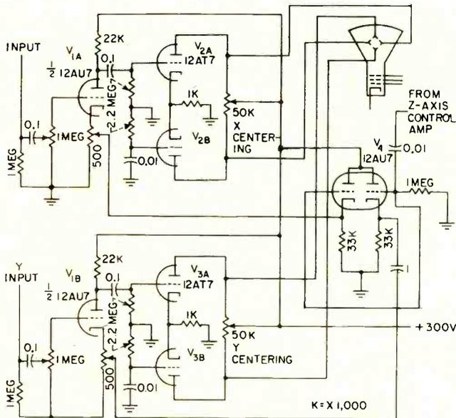
FIG. 2—Display tube and X- and Y-input amplifier portions of signal circuits used with three dimensional tubes
