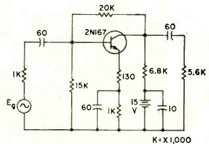
FIG. 4—Practical transistor a-c amplifier with selected component values. Use of 20,000-ohm shunt feedback resistor provides d-c and a-c voltage feedback and eliminates two components
