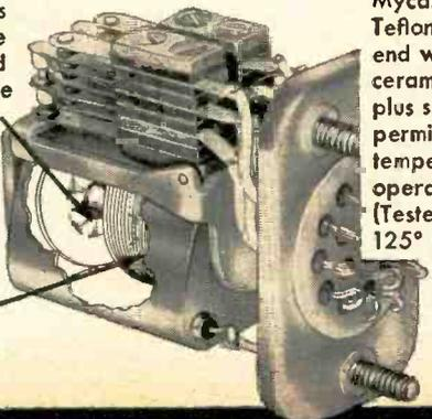
Mycalex stack, Teflon wire and end washers and ceramic pushers, plus sealed coil, permit high temperature operations. (Tested up to 125° C.)
