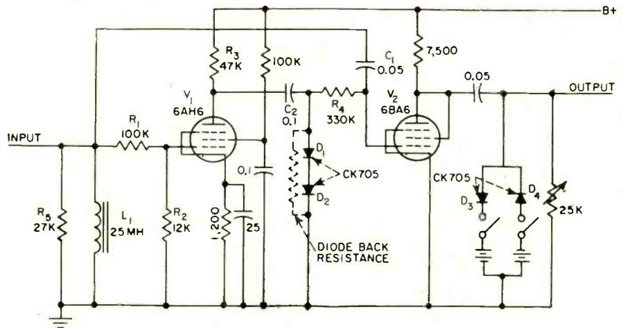
FIG. 1—Circuit of automatic amplitude control for audio section of radio transmitter
