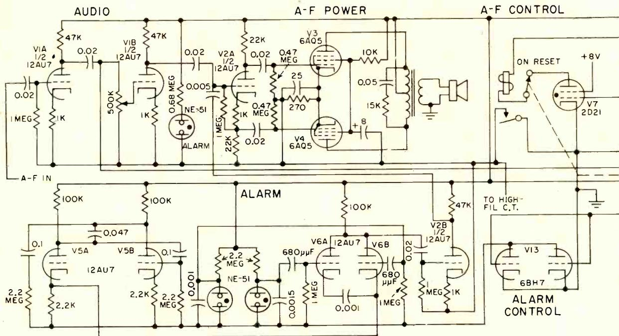
FIG. 4—Schematic of signal-selective Conelrad alarm. Fail-safe provisions are maximized when all tubes are pre-aged in non-
