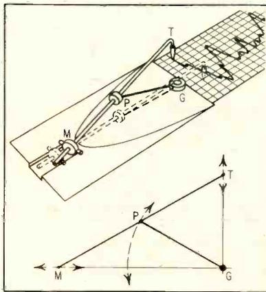
FIG. 1—Jeweled pivots convert curvilinear motion of the galvanometer movement to rectilinear motion. Rectilinear pen recordings have the same shape as a plotted graph and can be measured with a straight edge ruler.
