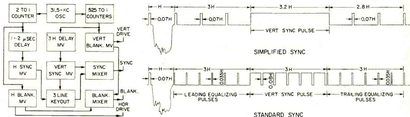
FIG. 5—Simplified-sync generator used in airborne system and its output compared to commercially used sync signals
