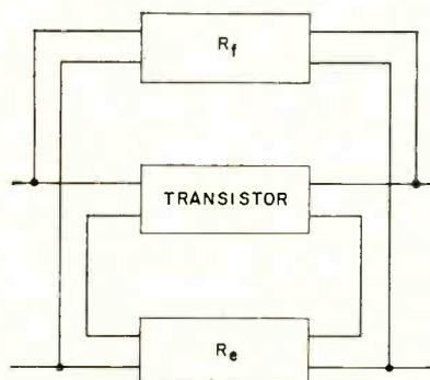
FIG. 3—Circuit shown can be used for matrix analysis technique. Matrix is derived by using equivalent a-c circuit shown in Fig. 2 and reducing transistor and feedback loops to 4-terminal networks
