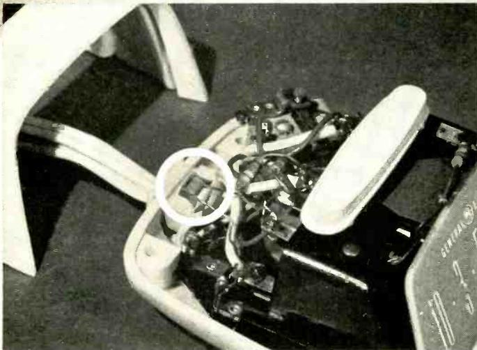
The advantages of Vac-u-Sel rectifiers lie in General Electric's precision vacuum process for obtaining a pure, more even deposition of selenium over the entire cell surface. This results in longer life—even at high operating ambients and better-than-normal rated current. Performance can be reliably predicted from unit to unit.
