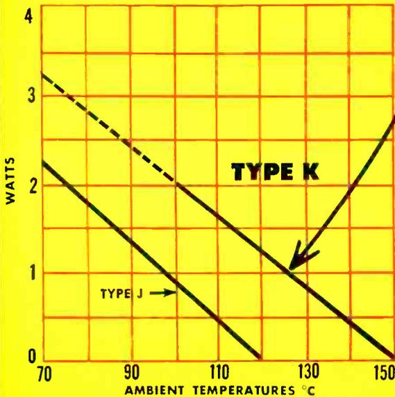
Comparison between Type K and Type J variable resistors—power ratings vs. ambient temperature. Type K far exceeds the requirements of MIL-R-94B.
