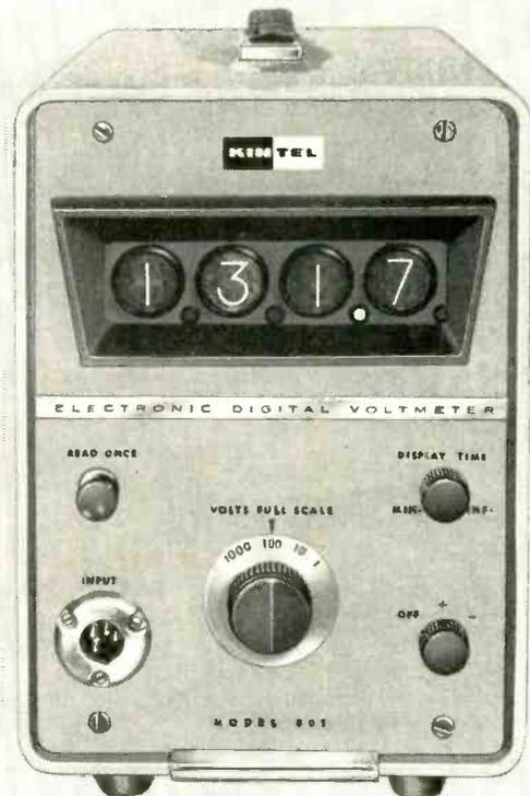
Here at last is a portable all-electronic digital voltmeter that measures DC voltages from .001 to 1000 volts with 0.1% accuracy. In less than 1/10 of a second the measured voltage is presented in clear numerical form on a digital in-line readout that even unskilled personnel can read quickly and accurately, with little possibility of error. *Direct* voltage measurement by successive approximation provides accuracy and sensitivity previously obtainable
