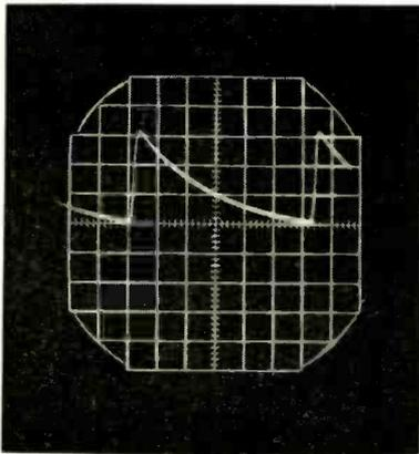
Generator output is shown with vertical scale of 5 volts per cm and horizontal scale of 2 microseconds per cm
