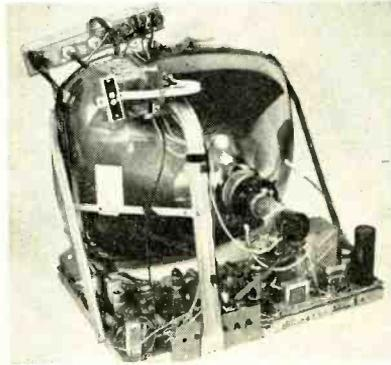
Relatively massive tv chassis (left) has been replaced by a lighter, less costly triangular chassis (right) which frames the picture tube and printed circuit board
