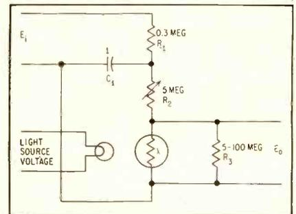
FIG. 1—Photoconductive chopper offers low noise level and resistance to vibration
