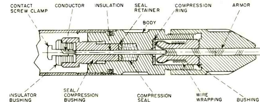
FIG. 2—Cross-section of cable-head assembly shows details of method used to seal probe against pressures which may rise as high as 2,000 psig
