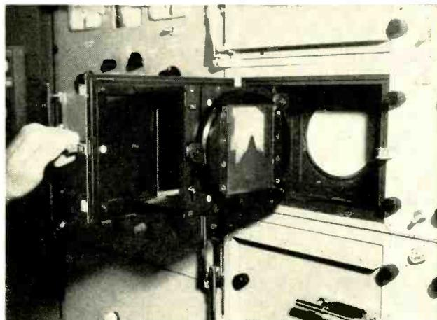
Slide chamber, which holds photoplate, is at left. Cathode ray tube is at right. Photoplate is easily accessible
