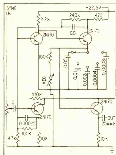
FIG. 1—Transistorized crt beam-direction marker has direct-coupled emitter follower to isolate oscillator from load
