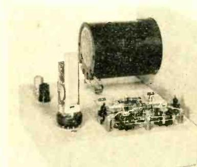
Side view of time-interval clock system shows mounting of circuit components
