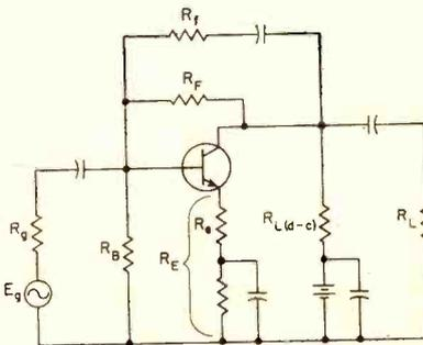
FIG. 1—Transistor a-c amplifier using both shunt and series feedback loops. Multiple loop enables circuit properties to be preselected and controlled independent of transistor parameters
