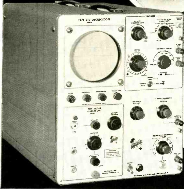
This new fast-rise oscilloscope with the Tektronix Plug-In Feature is extremely versatile and easy to operate. With a single Type 53/54 fast-rise plug-in pre-amplifier the Type 543 handles the usual applications in the DC-to-30 MC range. Many other inexpensive plug-in units are available for the more-specialized jobs, including one for transistor rise, fall, delay and storage time testing.
