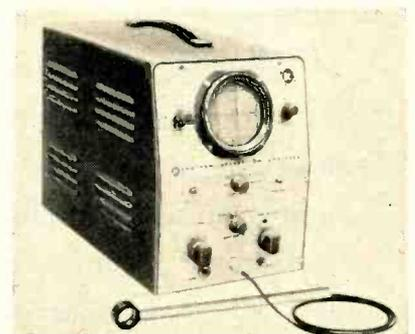
Waveform is displayed on the scope by picking up the electrostatic field around a component
