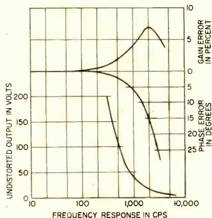
FIG. 2—Frequency response, phase error and gain error curves of photoformer. Response is flat to about 300 cps
