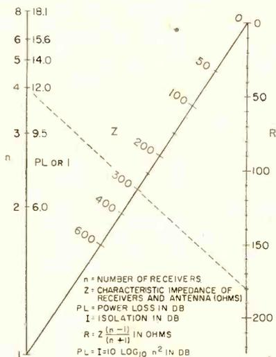
FIG. 2—Nomograph for  $n$ -set multicoupler. Since the multicoupler circuit is symmetrical, isolation between receivers is equal to power loss when both values are expressed in decibels
