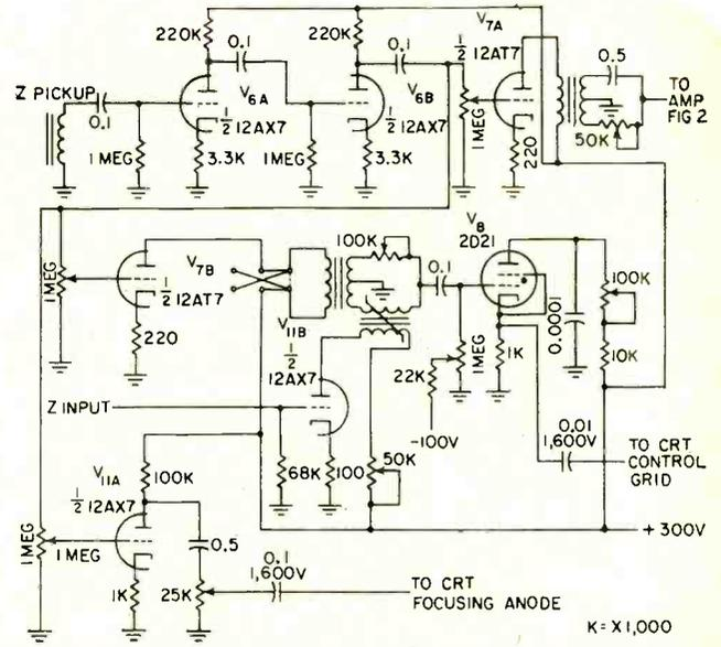
FIG. 3—Z-input amplifier and Z-axis control circuits for the display tube generate gate to produce spot on screen at right time
