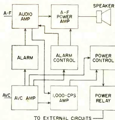
FIG. 3—Functional diagram of complete alarm system and control circuits
