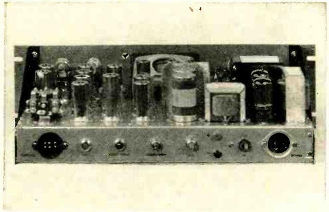
Standard relay-rack construction is used, with 3½-in. front panel Connections to rear of chassis include remote power control (left)
