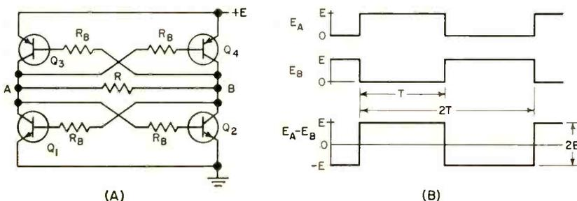
**FIG. 2—**Voltage-doubling chopper utilizes complementary symmetry feature of transistors (A) to double input voltage to that appearing across the load in (B)
