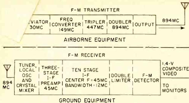
FIG. 1—Elements of airborne and ground-based tv equipment
