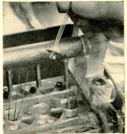
Transistor is removed from electrolyte and quickly placed in jet spray. Dried electrolyte is hard to remove
