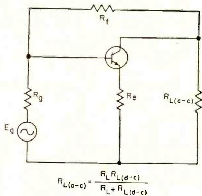
FIG. 2—Equivalent a-c circuit derived from network in Fig. 1
