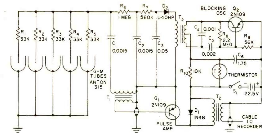
FIG. 1—Schematic of gamma-ray probe. High voltage for G-M tubes is provided by blocking oscillator  $Q_2$  and selenium rectifier  $D_2$ . Simple but effective temperature compensation is achieved through the use of a thermistor
