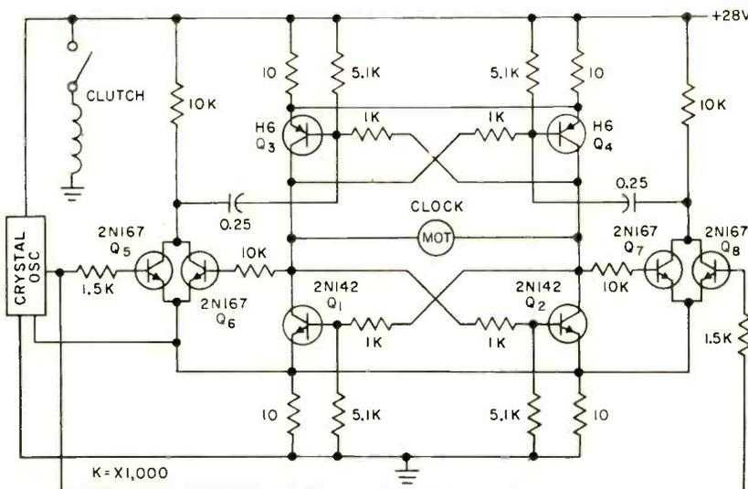
**FIG. 1—**Time-interval clock uses bistable voltage doubling chopper to provide a-c power necessary to drive synchronous clock motor with 0.02-percent accuracy
