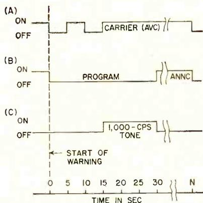
FIG. 1—Typical sequence of carrier (A), program (B) and warning-tone (C)
