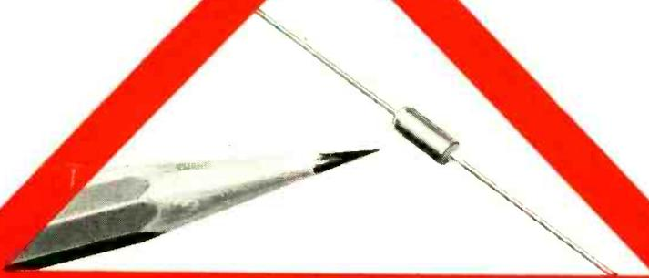
This solid-electrolyte Tantalex Capacitor (shown 1½ times actual size) is rated at 4.7  $\mu$ F, 10 volts d-c, and is only 1/8" in diameter by 1/4" long.
