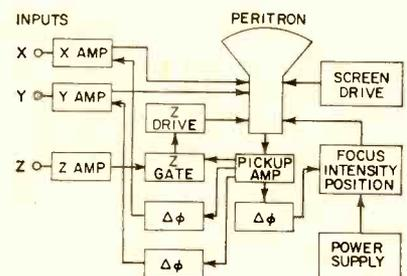
FIG. 1—Logic employed for generating three-dimensional patterns on display tube described in text
