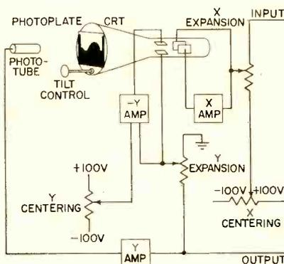
FIG. 1—Block diagram of photoformer crt deflection system. Photoplate, containing image of waveshape, is placed between phototube and crt. Closed loop deflection system enables phototube to sense crt spot-position error. Spot is then driven to the point on plate where phototube sees it
