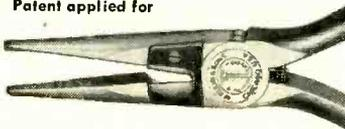
208-6C long nose shear cutting plier. A 6½-inch long nose plier with shear blades. Point of nose ⅜-inch diameter. Coil spring keeps jaws open ready for use.
