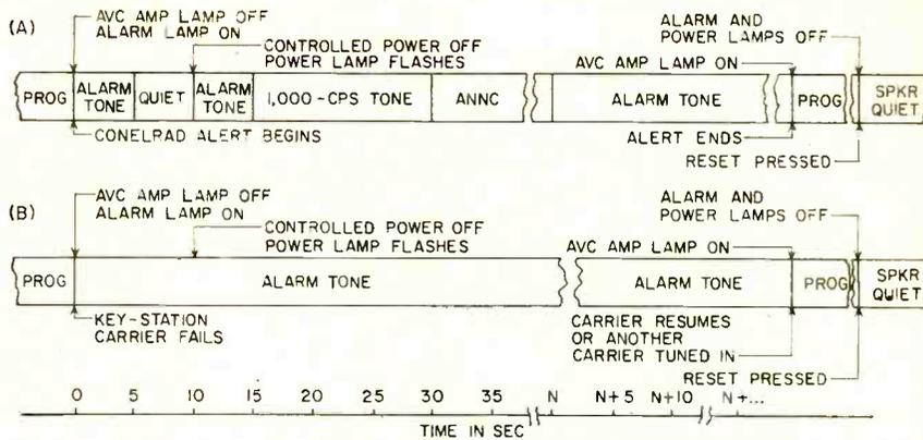
FIG. 2—System operation during Conelrad alert (A) and key-station carrier failure (B) gives indication of relative time intervals involved during possible alert
