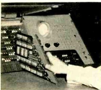
Transistors are mounted on 332 printed-circuit cards for ease of access
