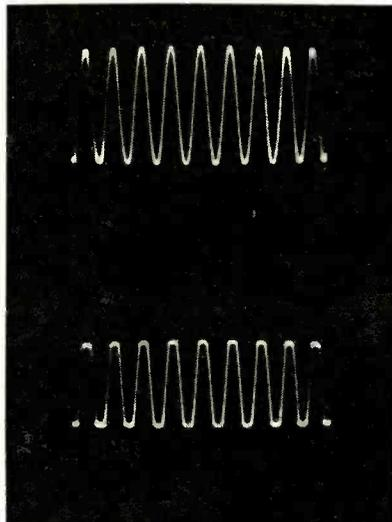
FIG. 3—Waveforms showing degree of clipping required for pure 1,000-cps sine wave (above) to limit output variations to approximately 1 db. Wave below is clipped 5.8 db
