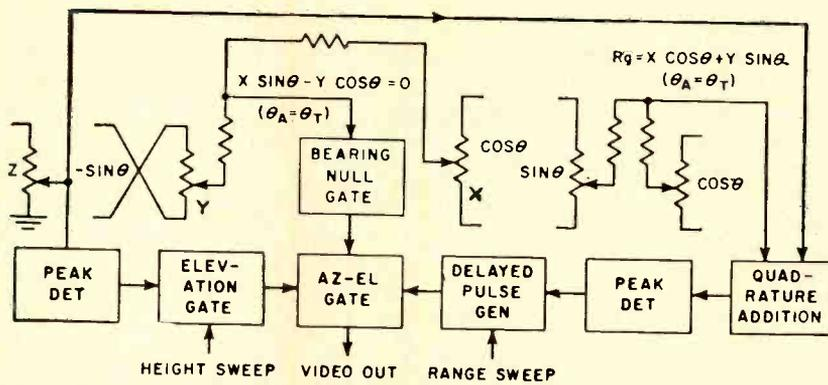
FIG. 5—Three dimensional radar target simulator uses a resolver to supply X, Y and Z potentiometers. Signal for ppi is modulated at height scan rate
