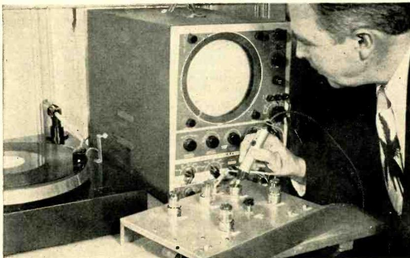
Author checks experimental setup of development model of stereo preamplifier and high-quality monaural pickup arranged for stereo disk playback. Power amplifiers are not shown
