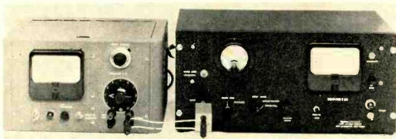
Capacitor discharge test set (left) is evaluated by discharging capacitor through mercury switch into ergmeter (right). Meter at left of ergmeter panel balances bridge and sets calibration while output indication meter is at right
