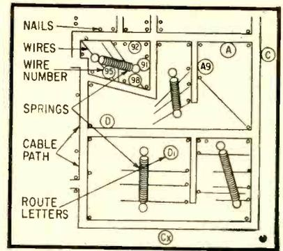
Diagram shows how a portion of the cable board is laid out
