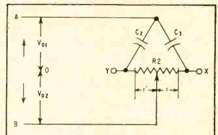
FIG. 3—Phase shift of voltage between X and O and input voltage increases as r is increased
