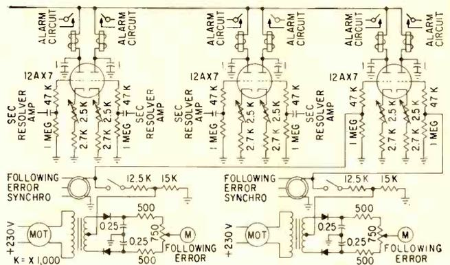
FIG. 8—Malfunction circuits. Six tube-operated relays protect coincidence telescope circuits against overload caused by component failure or against inaccuracies caused by system errors
