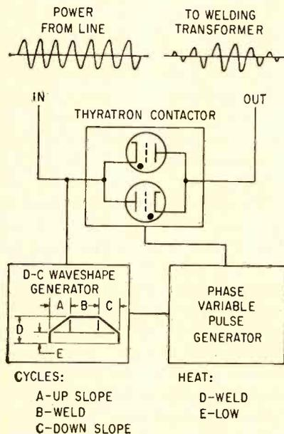
FIG. 1—Block diagram of weld timer
