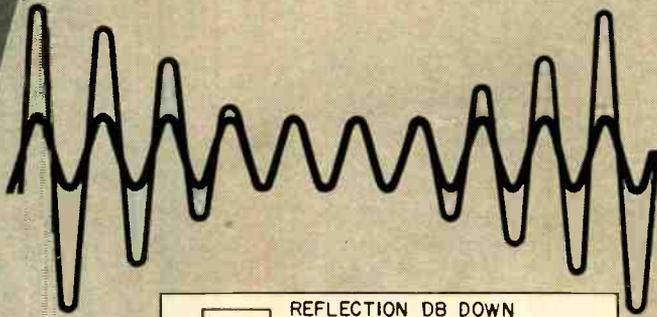
Measurement Of Voltage Standing Wave Ratio
