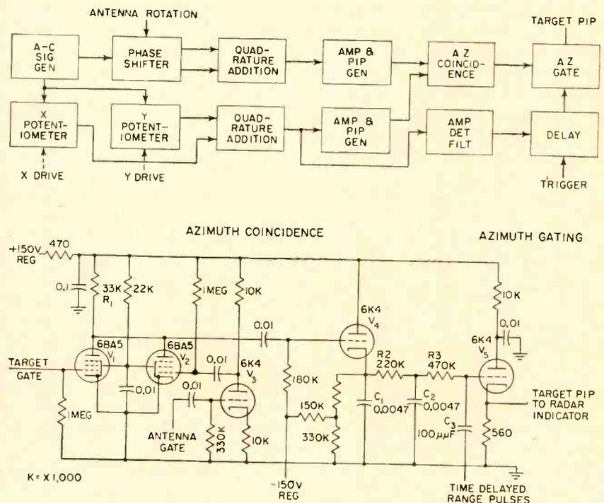
FIG. 1—Two dimensional radar target simulator supplies target pip to radar indicator
