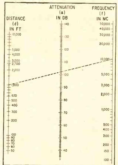
FIG. 1—Nomograph provides attenuation in db between two isotropic antennas
