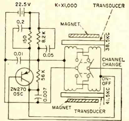
FIG. 2—Schematic of ultrasonic generator, comprising transducers and oscillator
