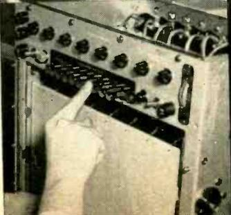
Recorder back plate holds eight plug-in Power Amplifier modules (one shown unplugged in photo), four on either side of Power Supply section. Entire back plate removable for servicing.
