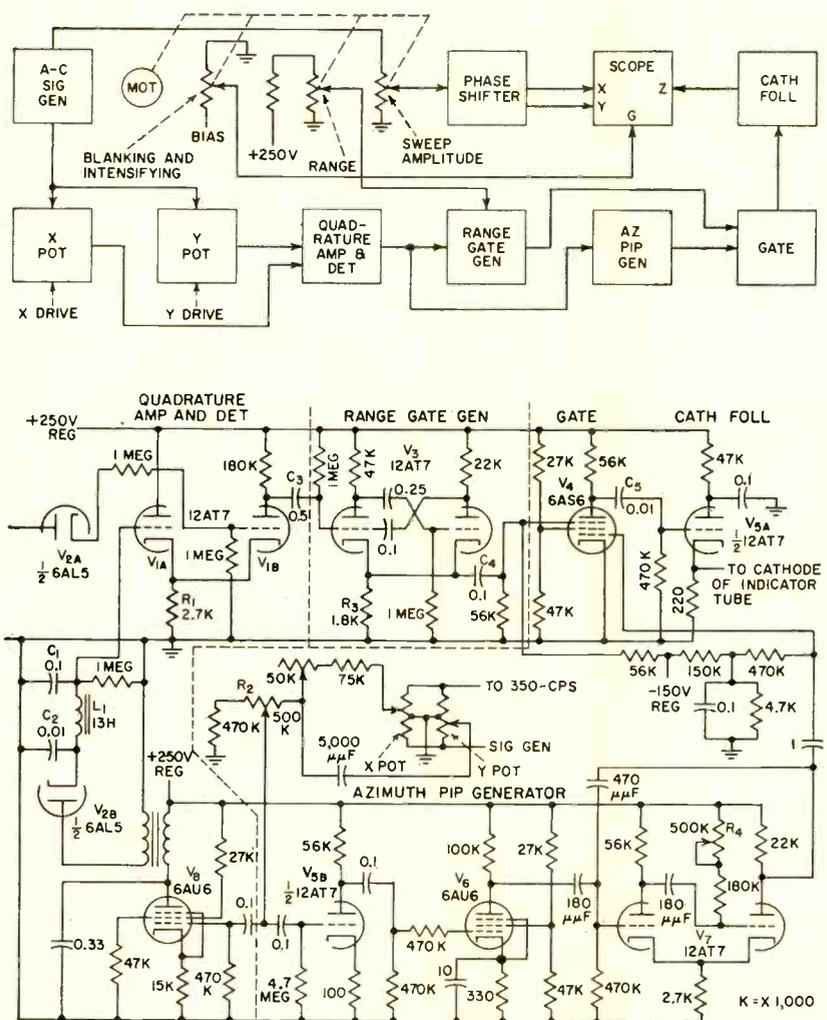
FIG. 2—Simulator does not require any operational radar equipment. Antenna signal is obtained from phase shifter and sweep amplitude potentiometer
