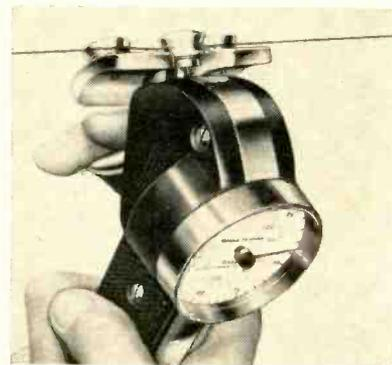
Trigger-operated tension meter
