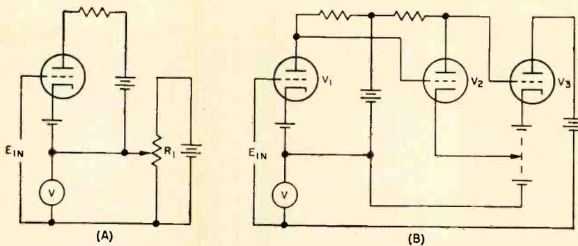
FIG. 1—Evolution of infinite input impedance d-c amplifier. Cathode-to-plate voltage in slideback voltmeter (A) is held constant by physically adjusting potentiometer  $R_1$ . In the completely automatic vacuum-tube circuit (B), the cathode-to-plate voltage of tube  $V_1$  is continuously maintained at a constant level by feedback from tubes  $V_2$  and  $V_3$ .
