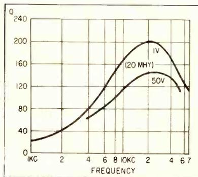
FIG. 3—Typical Q vs frequency characteristics for a 20 mh high frequency variable inductor
