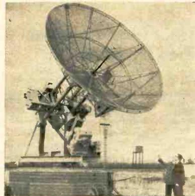
Seventeen-foot parabolic antenna follows the sun to enable Cornell scientists to pick up radio waves emitted from the solar atmosphere. Simultaneous measurements of intensities of right and left circularly polarized waves, correlation coefficient and phase difference between them and time checks are recorded by Brush oscillograph
