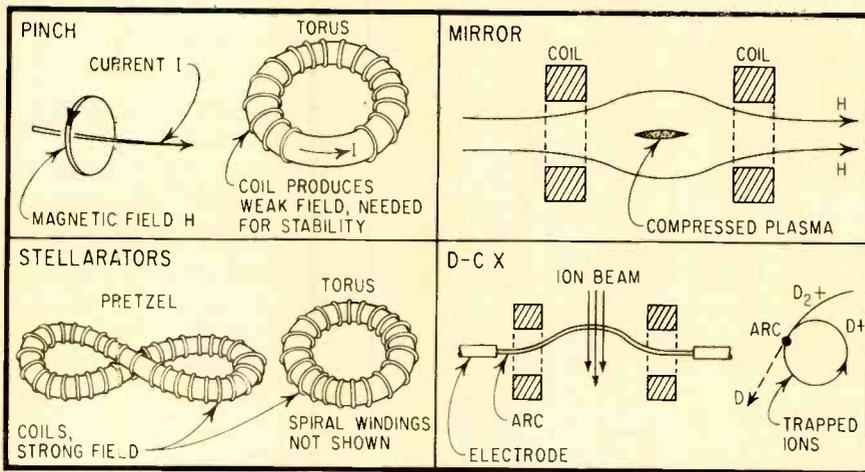
Basic designs of experimental apparatus used in controlled thermonuclear power research are shown as . . .
