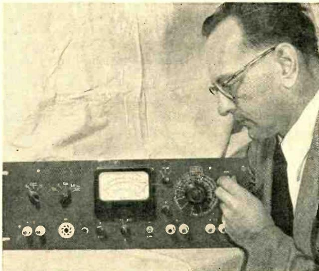
Zero adjustment of differential voltmeter containing two infinite input d-c amplifiers is made from front panel. Calibration is not needed since amplifier gains are within 0.0005 percent of unity
