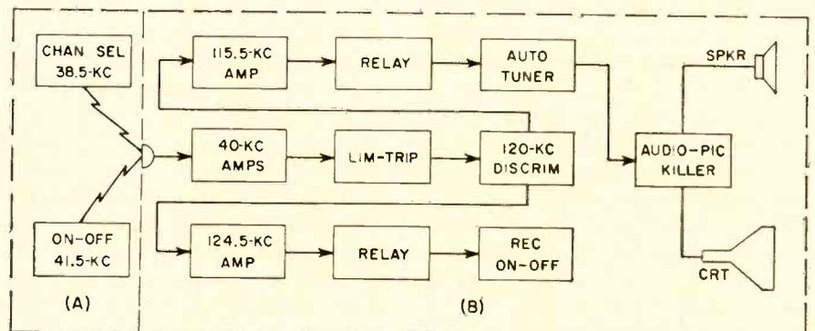
FIG. 3—Block diagram of complete control system. Box (A) comprises remote generator, while equipment in box (B) is included within the television receiver
