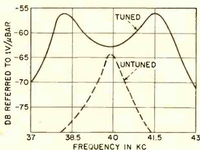
FIG. 5—Microphone characteristics with and without inductive tuning
