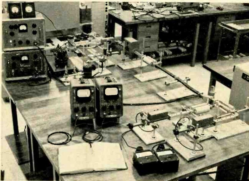
Simple operation and calibration are key features of setup for measuring losses in microwave devices
