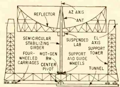
FIG. 1—Physical arrangement of antenna assembly. Twelve four-wheeled carriages support the entire antenna structure. Four carriages are used under each tower to help distribute the load and to counteract toppling effect of wind. Two driving carriages are used to move each tower around on two circular sets of railroad tracks.
