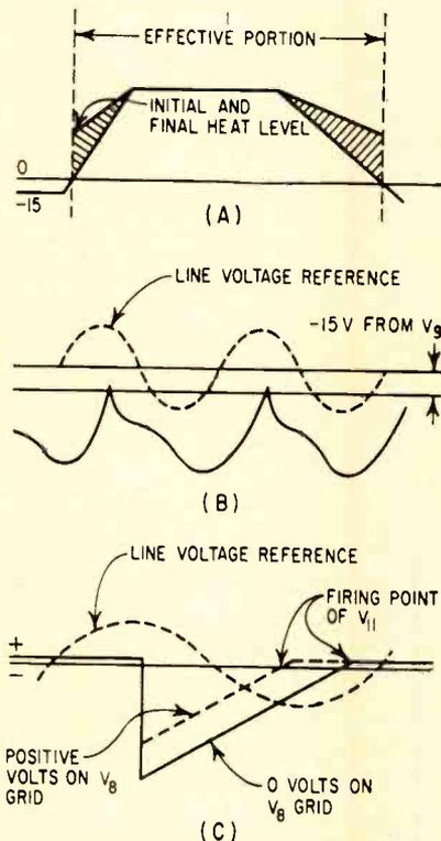
FIG. 3—Pulse-generating circuits operate in effective portion (A), with shaded section representing voltage added by low heat adjust. Triggering in (B) occurs once each cycle. The instant of start of conduction is controlled by weld heat adjust
