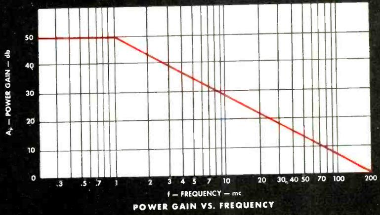
Now for your television IF's, VHF oscillators and amplifiers plus high speed computer applications... new round welded 2N623 diffused-base germanium transistors give you 200 mc typical maximum frequency of oscillation, 90 mc alpha cutoff, plus a 25 nusec typical total non-saturated switching time.
