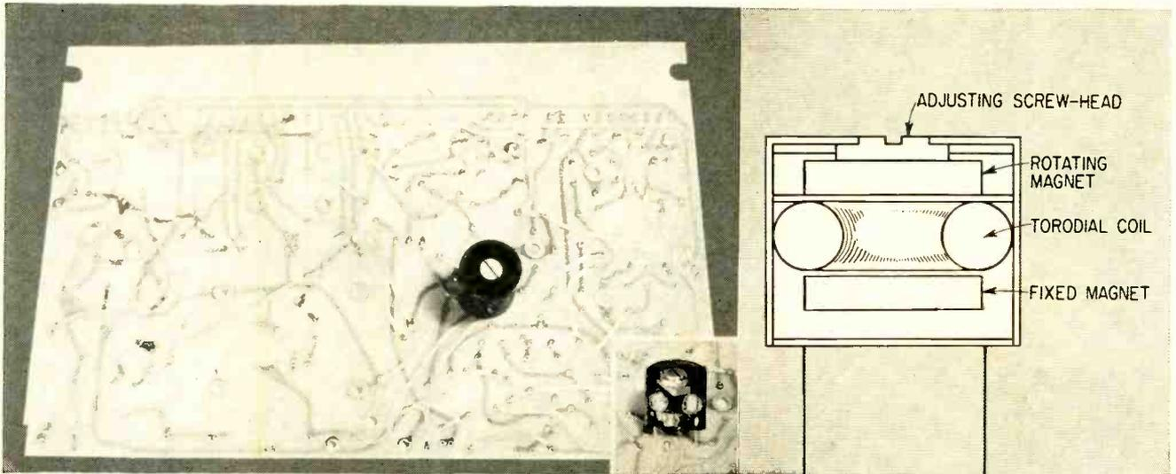
FIG. 1—Miniature variable inductor developed especially for printed circuits. Inductance is varied by rotating the top permanent magnet to change toroidal flux.
