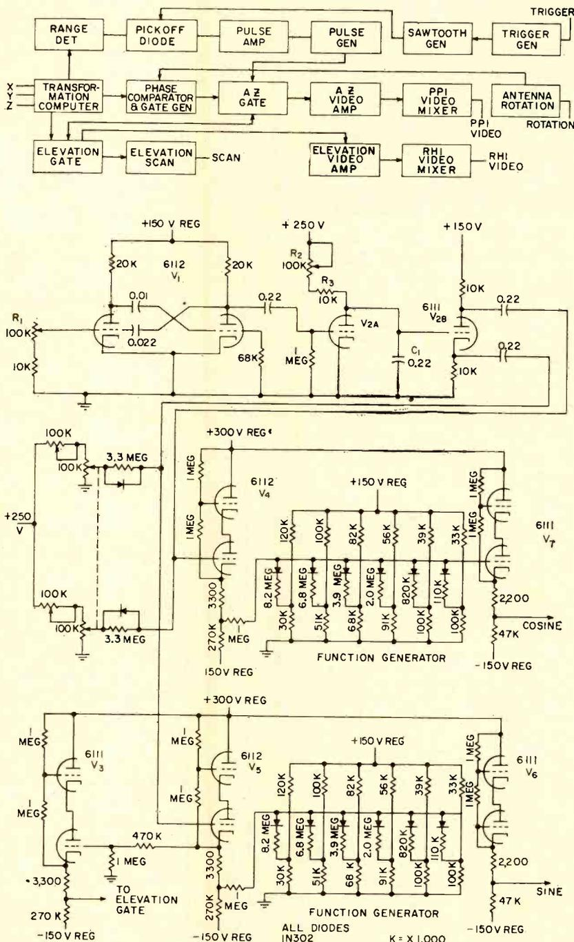
FIG. 3—Three dimensional radar target simulator uses computer approach to convert from rectangular to polar coordinates to obtain both ppi and rhi information
