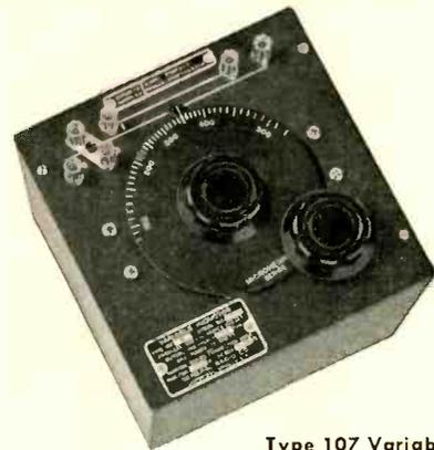
**Type 107 Variable Inductor** — two concentrically-mounted coils are used as rotor and stator, and may be connected in series or parallel. Calibration accuracy is  $\pm$ 1%. Five models available with following series-connected values: 9-50  $\mu$ h, 90-500  $\mu$ h, 0.9-5 mh, 9-50 mh, 90-500 mh. When parallel connected, inductance is one-fourth of series-connected value. Prices range from \$85 to \$95.
