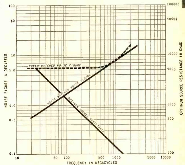
Wide range of 7077 performance, 30 to 1,000 mc, is shown by the noise figures above, under power-matched and noise-matched conditions, using an argon noise source. Noise contours are similar to those below with a diode noise source. Contours below plot noise figure and gain for 450 megacycles at various tube operating points.
