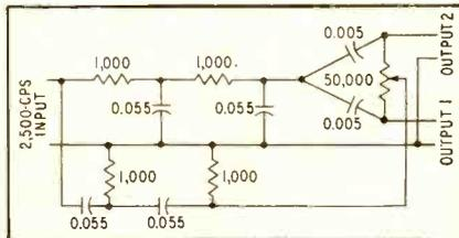
FIG. 5—Circuit produces a total phase shift between output 1 and output 2 from less than 180 degrees lagging to more than 180 degrees leading
