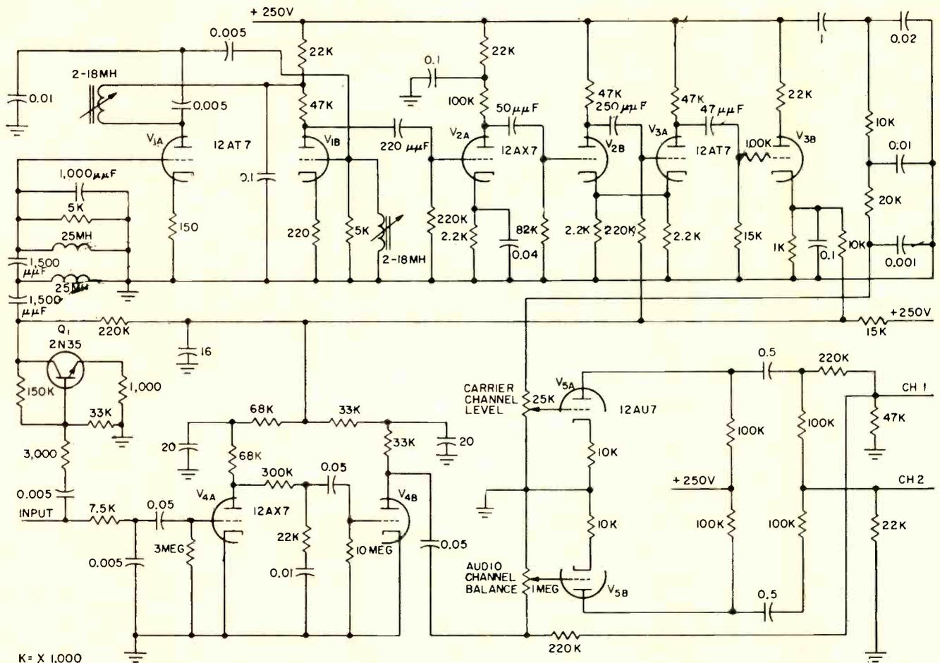
FIG. 2—Schematic diagram of auxiliary playback preamplifier. Limiting of the f-m carrier is performed by a Schmitt trigger circuit comprised of  $V_{2B}$  and  $V_{3A}$ . The detected stereo information is therefore in the form of pulse-sampled audio at the output of  $V_{3B}$ .
