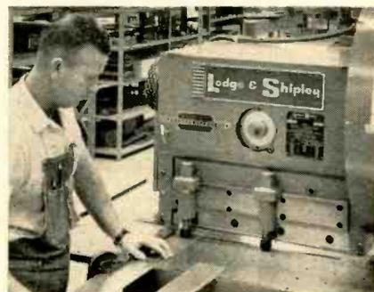
HIGH PRODUCTION rate on shearing of small component parts is obtained at Hewlett-Packard Co., Palo Alto, Calif., through use of new Lodge and Shipley 24 inch shear. Photo shows operator feeding 10-gage aluminum folding stock into shear at 400 per hour rate production of fan bracket plates for frequency counter.
