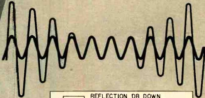
Measurement Of Voltage Standing Wave Ratio
