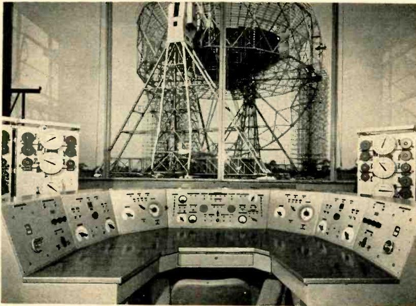
View of radio telescope looking through control room window. Antenna assembly can be operated remotely by one person sitting at the desk-type console which houses all necessary controls. A wide range of telescope movements can be selected including: automatic sidereal motion at a given right ascension and declination; motion in galactic latitude and longitude; motion in azimuth and elevation; and various automatic scanning motions with a choice of rasters
