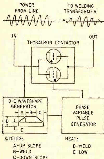
FIG. 1—Block diagram of weld timer
