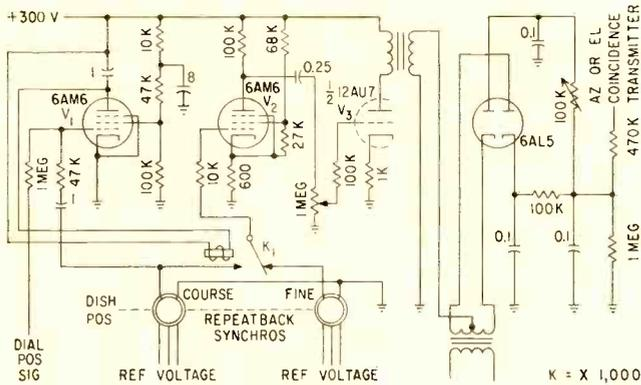
FIG. 7—This circuit amplifies signal from repeatback synchros and converts it into a d-c signal which controls the coincidence transmitters of the repeatback dials
