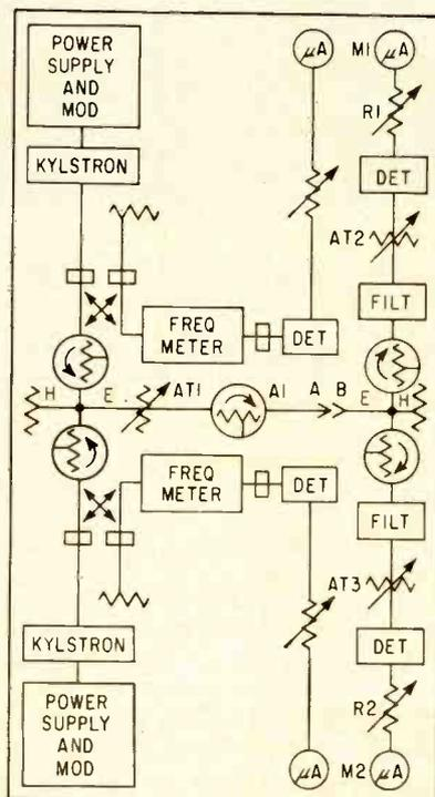
FIG. 1—Circuit measures losses in microwave components at two frequencies
