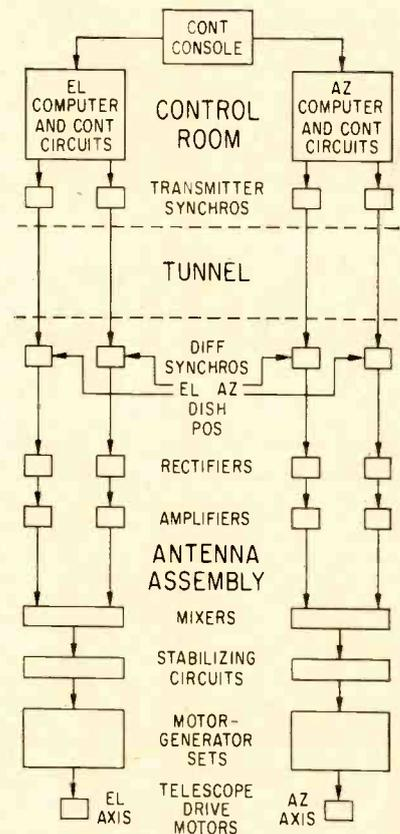
FIG. 2—Servo loop diagram of radio telescope. Command position signals from the computer and control circuits are compared with actual position signals from the reflectors. Difference, or error, signals control the exciter field of motor-generator sets. Output of the motor-generator sets drive d-c motors which compensate for the error by positioning the reflector
