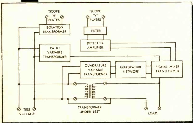
The Ratiometer consists of two precision variable transformers, a calibrated quadrature injector, a filter, and a pre-amplifier. Block diagram indicates connections of the various components within the instrument.
