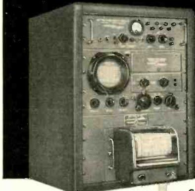
Panoramic Model PDA-1 Spectral Power Density Analyzer
