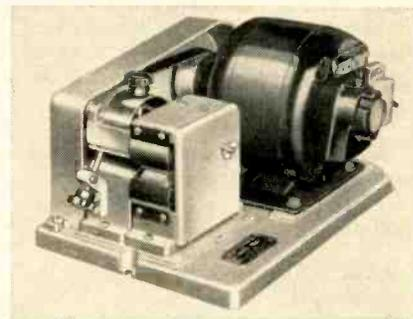
For example, using a standard wire stripper such as illustrated, we have made automatic coil lead straightening, trimming and stripping equipment for Electric Auto-Lite, Ford Motor, General Electric, Westinghouse and others. (Note: Each system was designed and built to meet the individual requirements of the user.)
