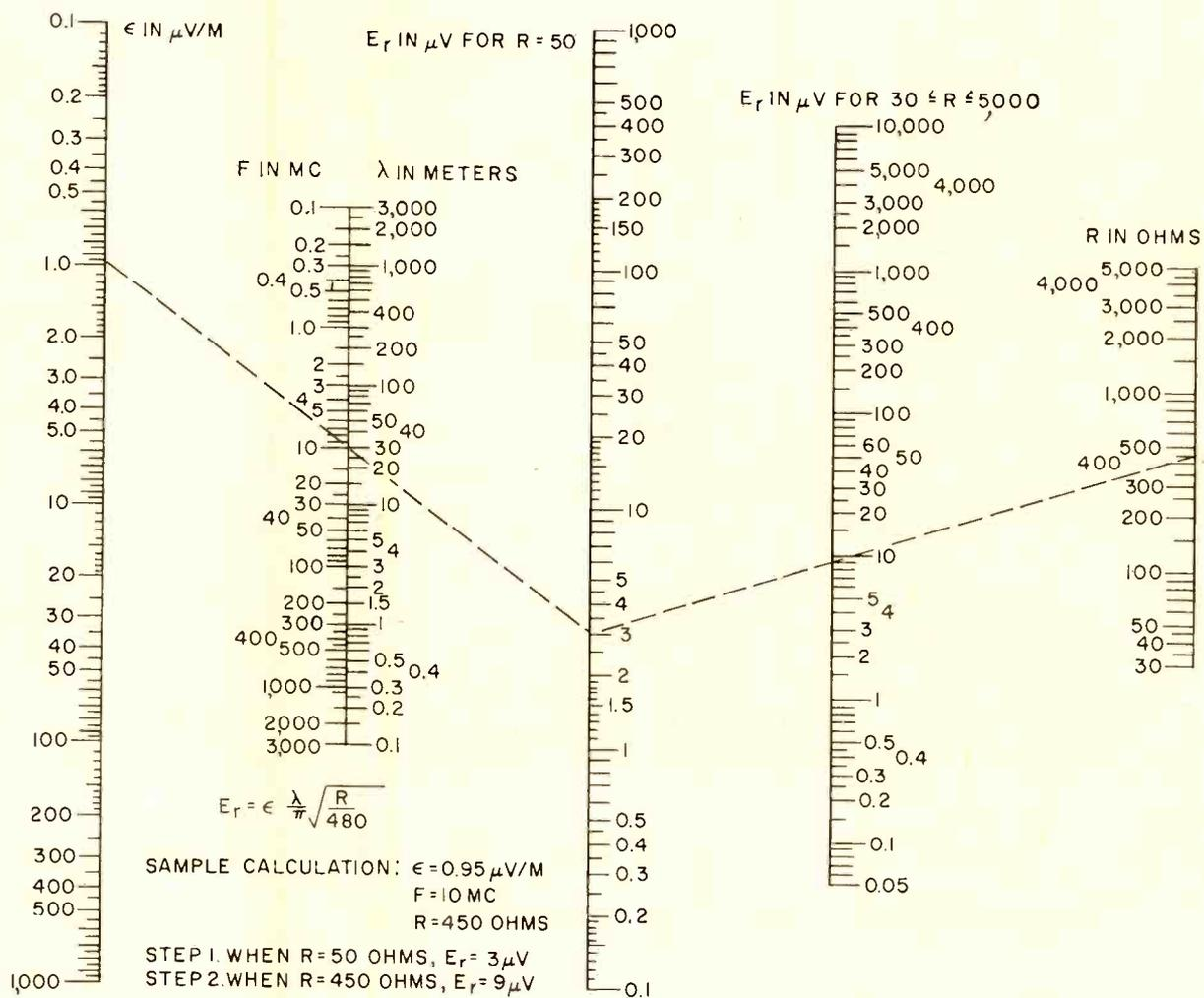
FIG. 1—Nomograph for converting field intensity to receiver input voltage
