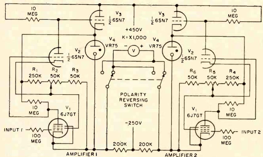
FIG. 2—High-impedance differential vtm with input range from  $-150$  to  $+150$  v. Conventional input voltage dividers are eliminated; range resistors are in output circuit. A polarity switch is provided to eliminate nuisance of transposing leads. Any simple half or full-wave unregulated voltage supply is suitable for use with this circuit.
