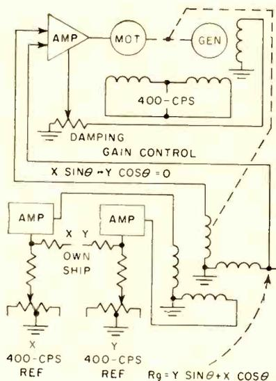
FIG. 4—Target position relative to moving own ship position can be obtained from this arctan computer circuit
