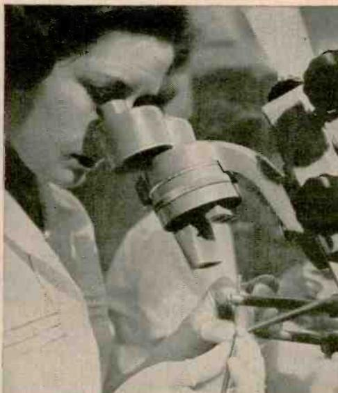
**CATHODE ASSEMBLY BY MICROSCOPE!** The G-E production worker above is welding the nickel cap on a tantalum cathode sleeve only 1/10 inch in diameter. Note the white Dacron lint-free dress and rubber finger cots! These help protect 7077's from dust and lint—the most common causes of short-circuits.
