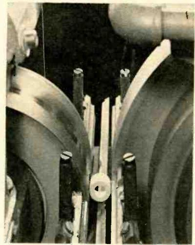
Operator positions workpiece by sliding it along lucite stick (left). As part traverses diamond wheel, grinding of another part may start
