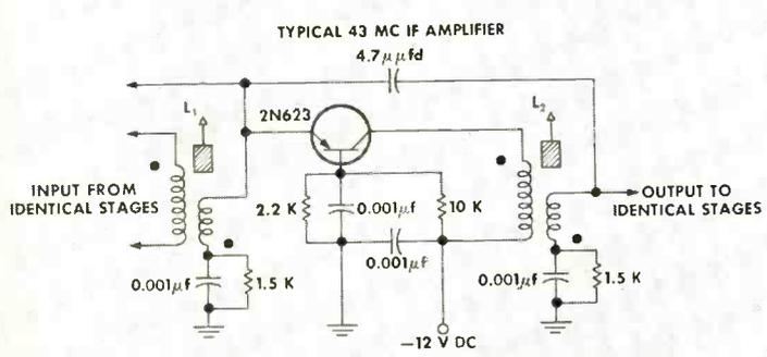
TYPICAL VALUES — AVAILABLE POWER OUTPUT 20 mW (PEAK) NOISE FIGURE 6 db • POWER GAIN 15 db • BAND WIDTH, ONE STAGE 11 mc APPROX. IMPEDANCE LOOKING INTO PRIMARY 56 Ω • LOAD ON SECONDARY 3000 Ω
