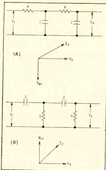
FIG. 1—Simple network at A produces 90-degree phase lag, while that at B produces 90-degree lead
