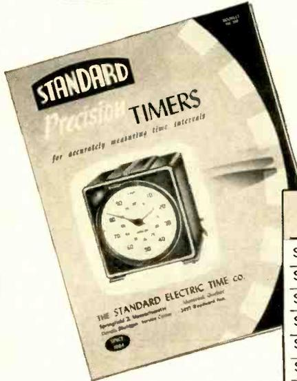
Accurate, reliable, versatile Elapsed Time Indicators. Synchronous motor drive, manual or electric zero reset. Electric clutch controlled by manual or automatic switch or output of electronic tubes. Units available for flush panel mounting or portable use.
