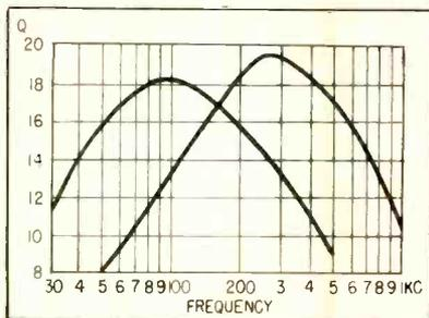
FIG. 2—Typical Q vs. Frequency characteristics for low frequency variable inductor
