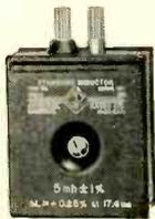
**Type 1481 Standard Inductor** — has higher Q at low frequencies than does Type 1482 Standard Inductor, although accuracy is not as high. Twelve models are available, from 1 mh to 5 h in 1-2-5 sequence (for 2-terminal measurements only). Temperature coefficient of inductance is about 25 parts in 10<sup>6</sup> per degree C, between 16° and 32°C. Accuracy is  $\pm$ 0.25% for large values,  $\pm$ 1% for smaller values. Prices from \$32.50 to \$40.00.
