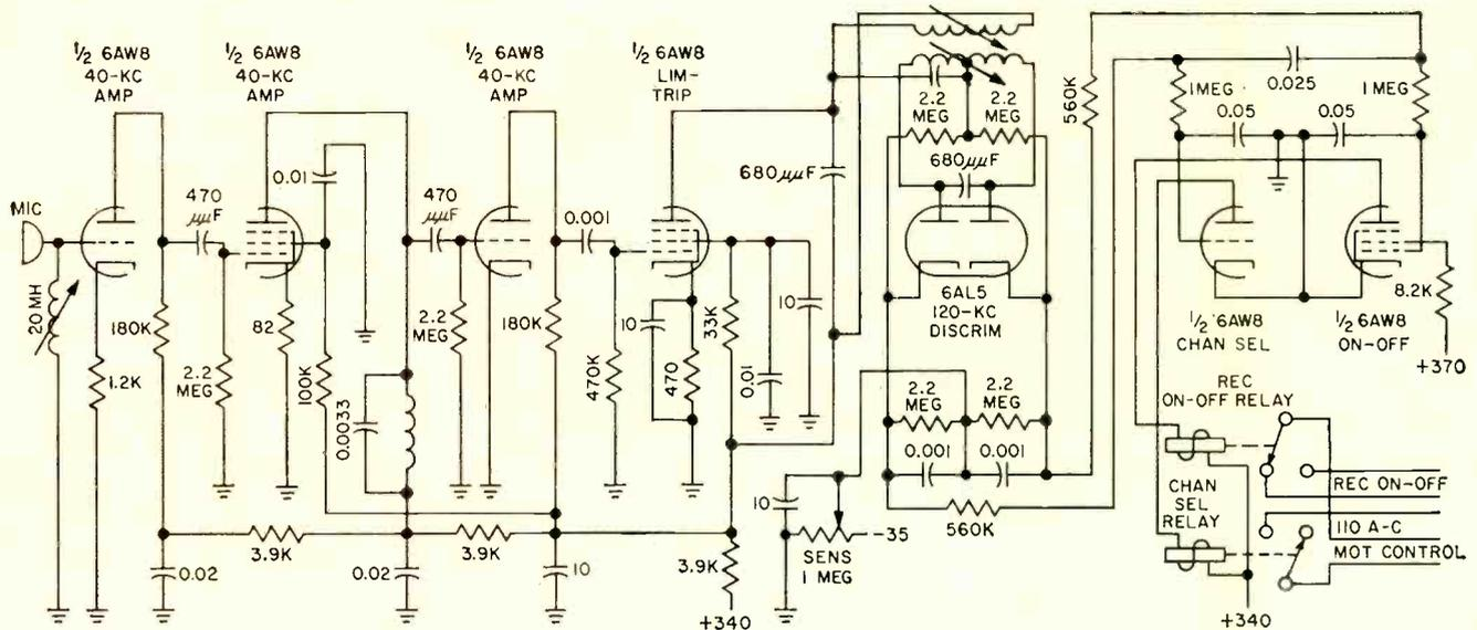
FIG. 4—Complete schematic of control receiver. On-off switches in receiver and remote unit are spdt for independent operation
