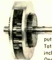
1 to 1 reverse ratio; 48 teeth on input and output gear, 1-1/32 inch diameter. Total outside diameter 1-25/32 inches. Shaft size is 1/4 inch. One shaft is 9/16" long; other **\$5.00**
