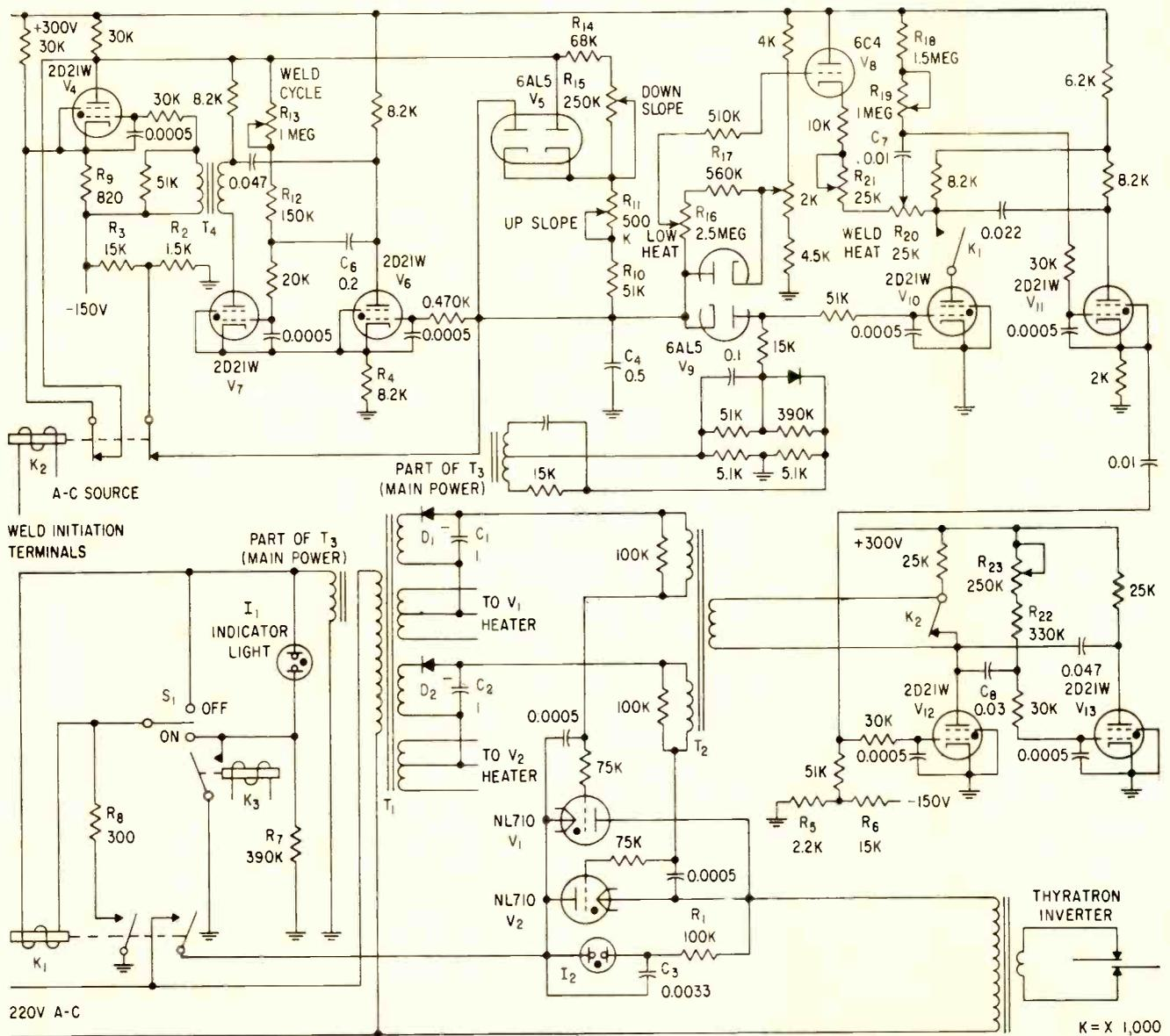
FIG. 2—Schematic of the heat program timer, showing the adjustable potentiometers that control the heat functions
