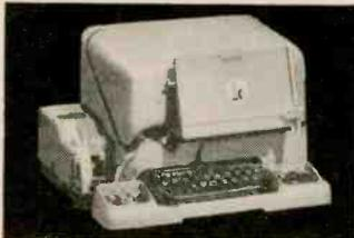
**Model 120 Typing Reperator-Tape Transmitter**
