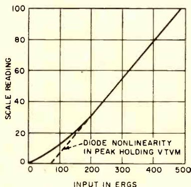
FIG. 3—Half-sine wave pulser injects energy bursts for calibration. Nonlinearity at low end of scale is caused by peak-holding voltmeter diode
