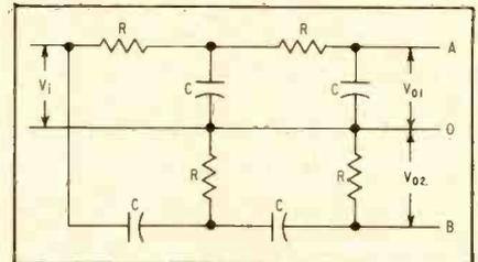
FIG. 2—Voltage across AO is 180 degrees out of phase with that across BO
