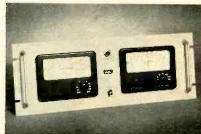
Rack-mounted electronic voltmeters are accurate over a wide range frequency range.
