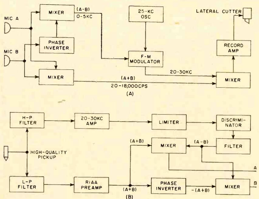
Fig. 1—Block diagram of (A) the recording system, and (B) the playback system. A monaural system could be converted to stereo by addition of (B) and a power amplifier
