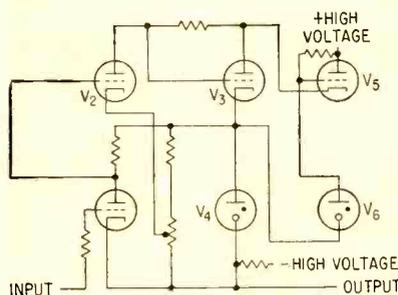
FIG. 3—D-c amplifier for high input voltages. High-voltage series regulator tube  $V_5$  maintains plate voltage of  $V_3$  at virtually constant level
