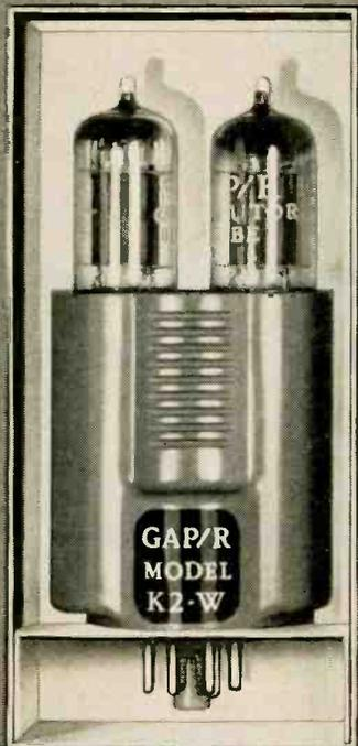
**FAST DC AMPLIFIER:** Model K2W is an efficient and foolproof high-gain operational unit for all feedback computations, fast and slow. A number of special varieties are also in quantity production. (\$24.00)
