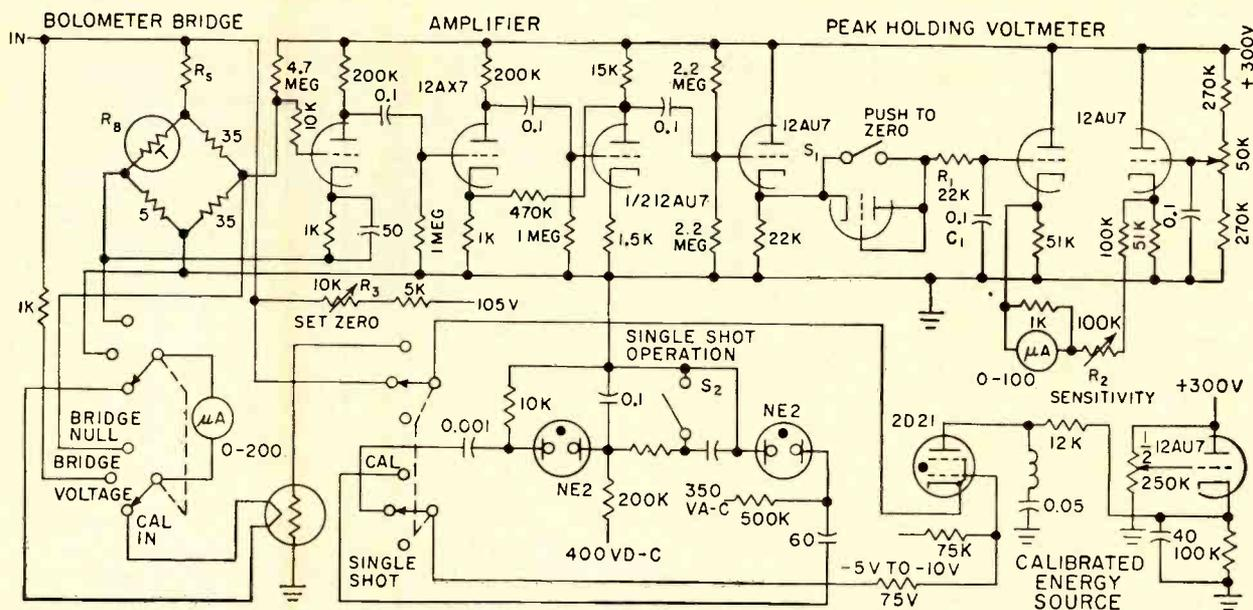
FIG. 2—Ergmeter consists of bolometer bridge, three-stage amplifier, peak-holding voltmeter and calibrated energy source
