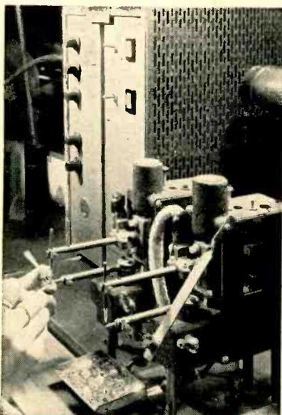
Heat program timer chassis (left) and power head (right) in operation on the electron tube assembly line
