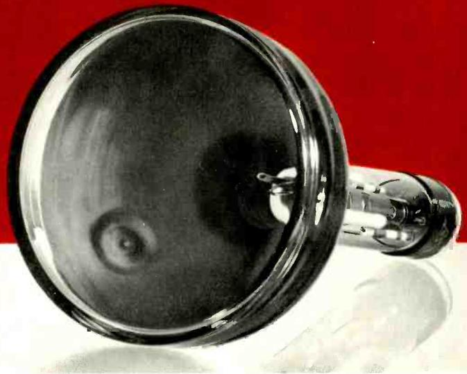
New five-inch experimental evaporated phosphor CRT
