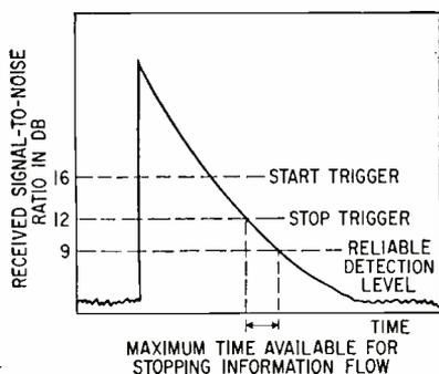
FIG. 7—Threshold levels of stop-link trigger are based on known maximum fade rate of meteor burst
