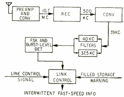
FIG. 2—Information receiver detects the presence of a usable signal during a meteor burst and demodulates the fsk signal information
