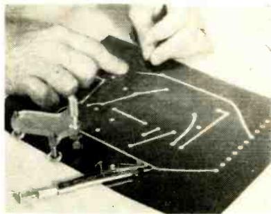
Coating is stripped from plastic film to produce photo-etch negative
