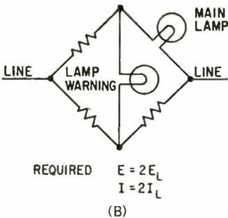
FIG. 4—Lamp failure in circuits at A and B does not stop current flow, and circuit at B also indicates lamp failure
