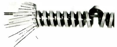
Multiconductor, multicolored retractable cable manufactured by Organic Development Corp., Garden Grove, Calif., has its winding direction reversed in the middle of its length. Technique eliminates strain at terminals and reduces inductive effect
