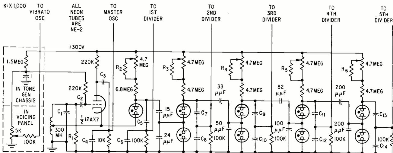
FIG. 3—Complete tone generator for one series of octavely related tones has master oscillator that provides initial sync for neon-lamp divider chain. Resistor  $R_1$  varies from unit to unit and maintains oscillator  $Q$  within common range
