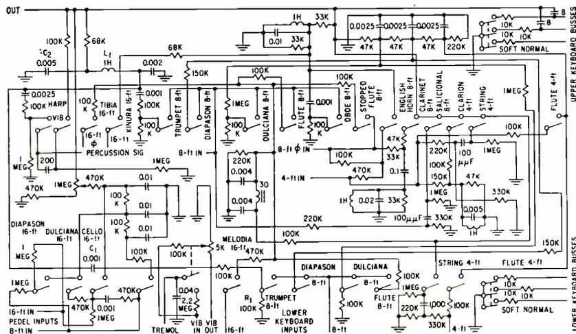
FIG. 6—Voicing panel contains formant filters which transform sawtooth-generator signals into waveforms of various instruments
