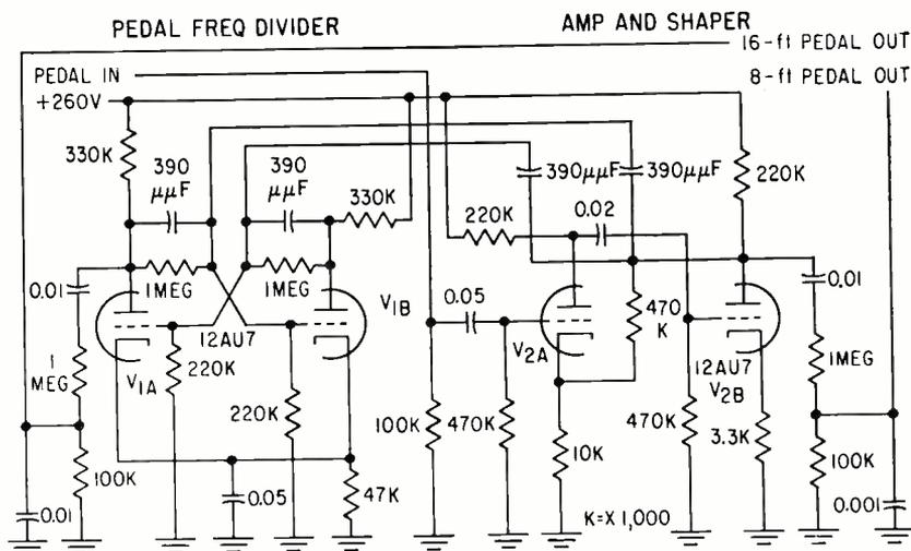
FIG. 4—Pedal generator produces notes an octave lower than main generator with the use of bistable multivibrator  $V_1$
