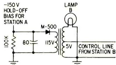
FIG. 2—Hold-off bias of -150 volts is developed to override unused station
