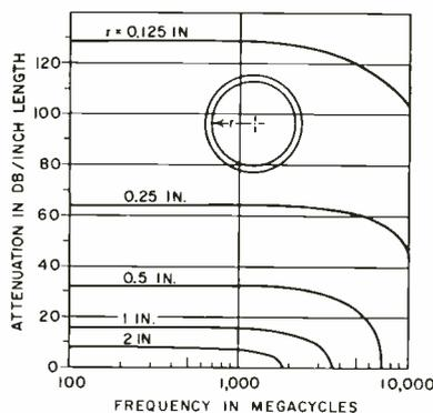
FIG. 1—Attenuation of a circular waveguide for  $TE_{11}$  mode. Curves continue horizontally down to 10 mc
