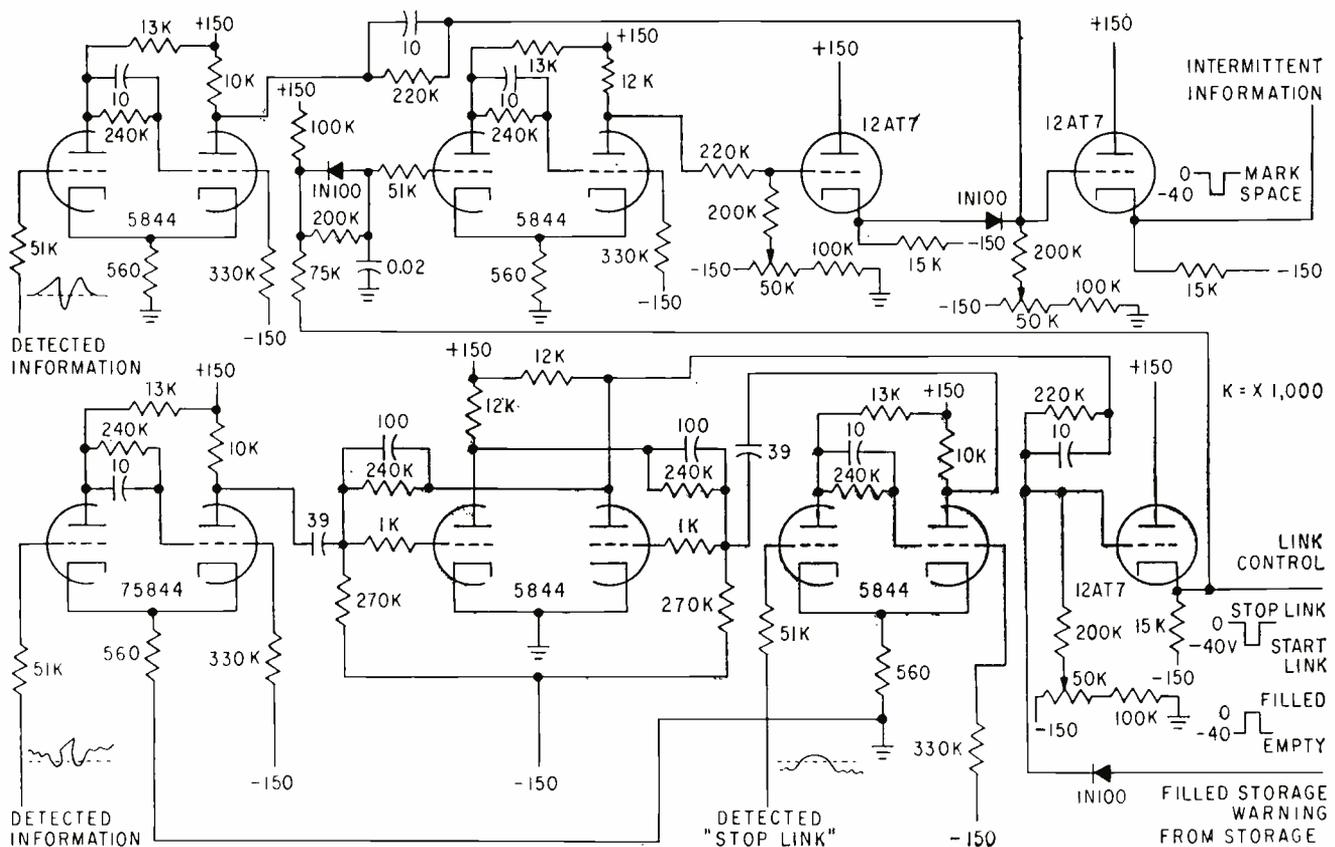
FIG. 6—Link-control schematic. Triggers are set well above ambient noise to preclude false triggering by noise spikes
