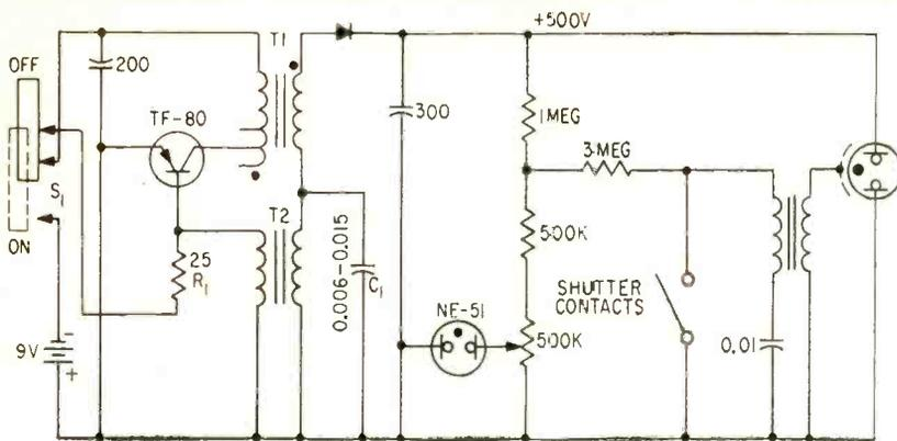
FIG. 4—Single power transistor is used in Burleigh Brooks Mecablitz 100 modified blocking-oscillator circuit. Half-wave rectifier requires higher voltage step-up by  $T_1$
