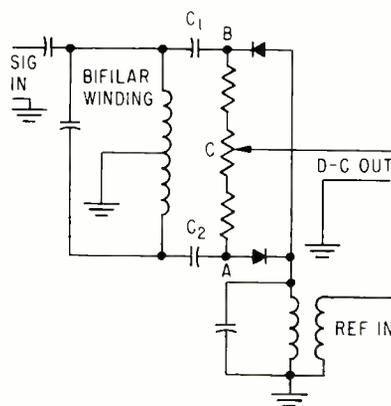
FIG. 1—Bifilar winding ensures that signal voltages applied to diodes are equal in amplitude
