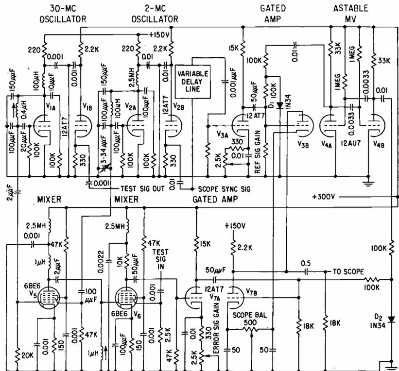
FIG. 4—Free-running multivibrator output is R-C coupled to grids of gated amplifiers  $V_{3B}$  and  $V_{7B}$ . Output of  $V_{7B}$  is a composite signal
