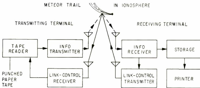
FIG. 1—Overall block diagram of meteor-burst communications system shows signal path for the detection and control of transmission, as radio waves bounce from ionized meteor trail. Information is transmitted only during meteor-burst
