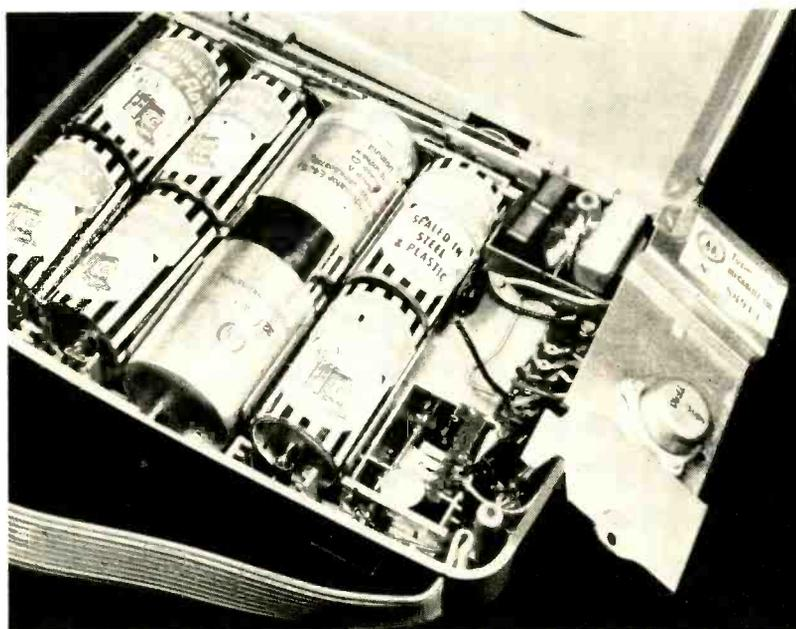
Aluminum plate provides heat sink for Mecablitz's power transistor; 4,200-cps operating frequency permits decreasing transformer sizes to those shown
