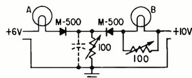
FIG. 1—Basic override circuit will operate with d-c, like-phased a-c, mixed a-c and d-c and, with a capacitor, unlike-phased a-c
