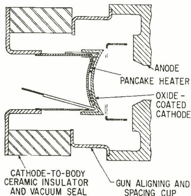
FIG. 2—Electron-gun assembly
