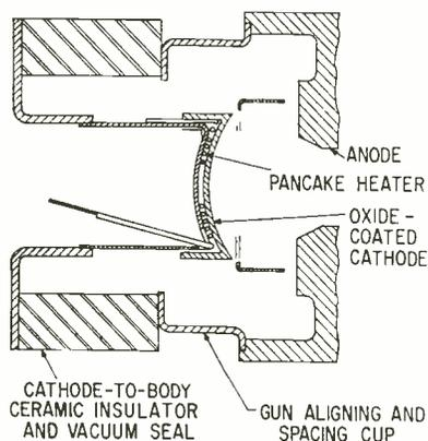
FIG. 2—Electron-gun assembly
