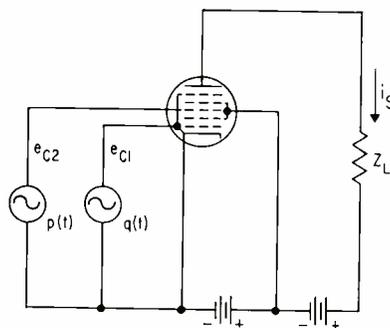
FIG. 1—Output of pentagrid mixer is a nonlinear function of its two inputs
