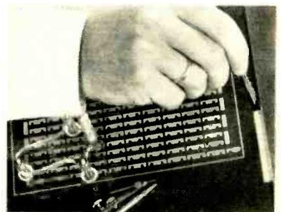
cut with the 3-legged tool shown, using a straight-edge or French curve as a guide. The tool has twin knife points held in a metal block. Adjusting knives in 3 block sizes allows conductor lines to vary from  $\frac{1}{2}$  inch to  $\frac{3}{8}$  inch. Plastic buttons on the tool legs slide over the film.
