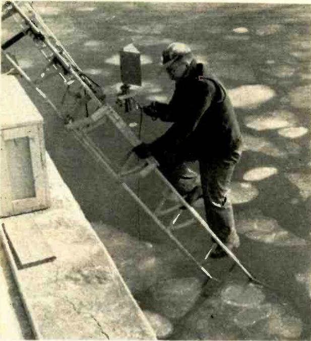
After adjustments are made on transmitting hydrophone, it is allowed to slide down track into the water to the desired depth
