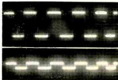
FIG. 2—Collector-to-collector (top) and base-to-base (bottom) voltage waveforms for circuit of Fig. 1
