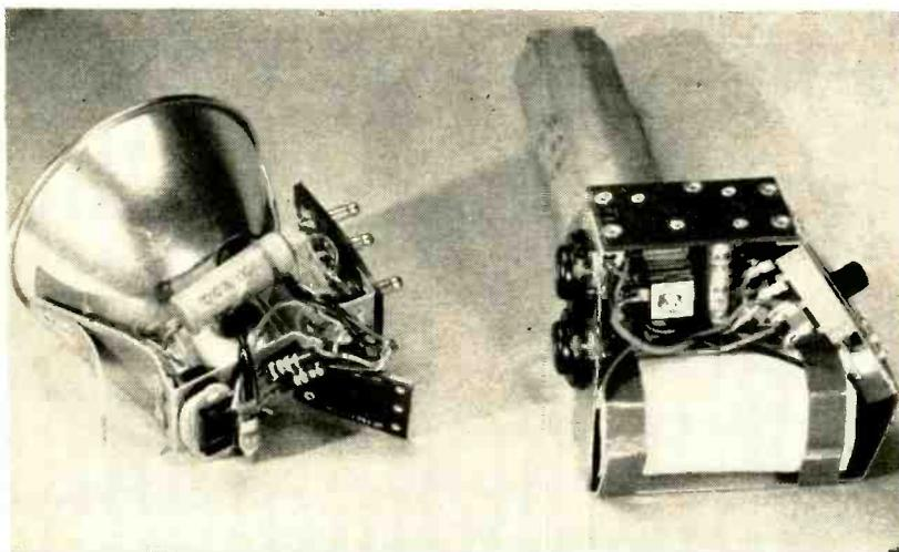
Flashtube and power supply illustrate off-chassis mounting of Vanguard's two power transistors, heat sink is not necessary because of relatively low current operation
