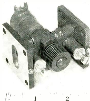
Type VA-824 klystron amplifier
