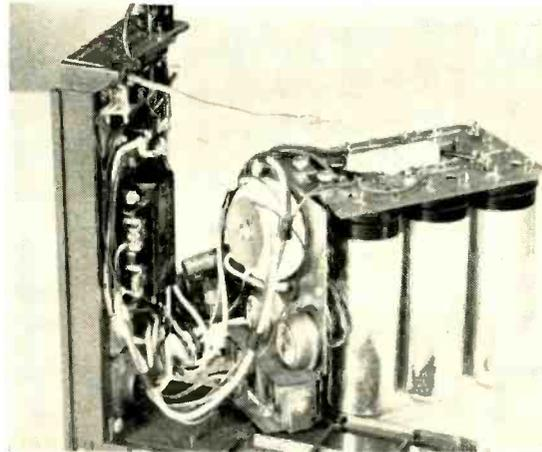
FIG. 1—Power unit by American Speedlight Ascorlight uses symmetrical inverter circuit. Thyatron trigger tube limits shutter con-
