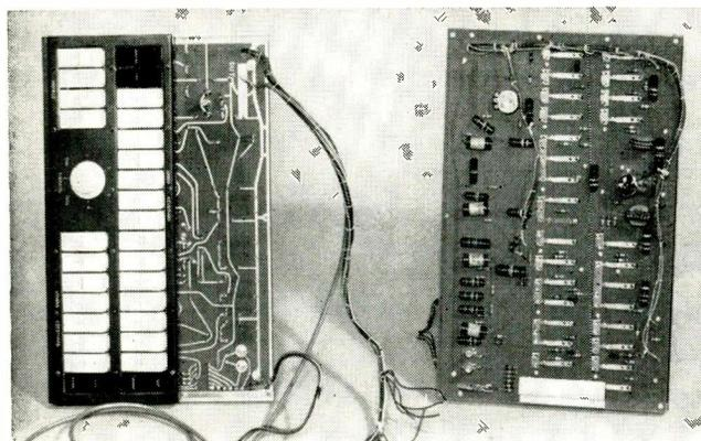
Voicing panel contains all filter components plus stop switches operated by plastic stop tablets shown at left
