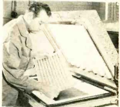
Negative of multiple artwork is placed on metal sheet in printing frame
