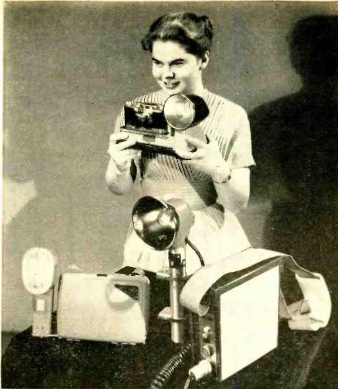
Electronic photoflash units for amateurs and professionals use transistorized power converters to increase efficiency and decrease size and weight for portability
