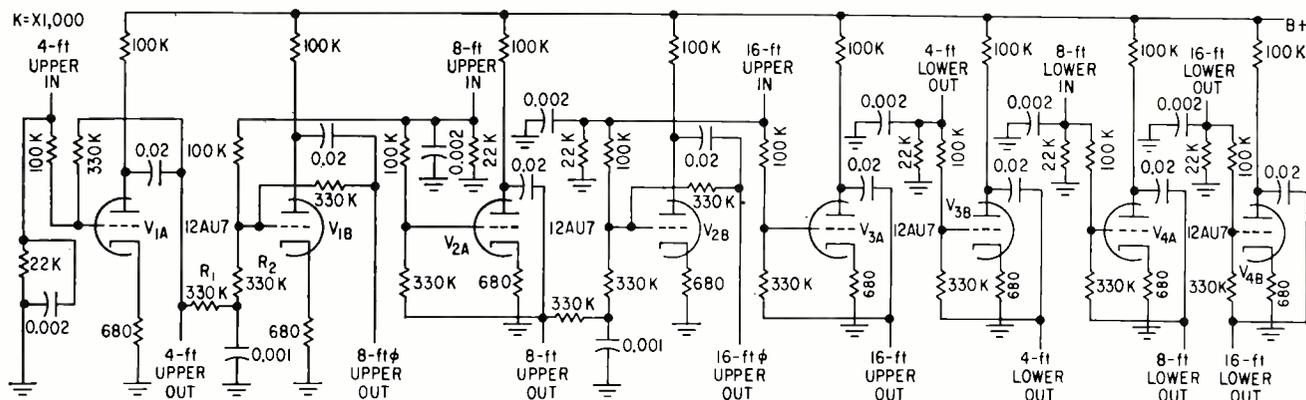
FIG. 5—Bus amplifiers located between keying-system outputs and formant filters provide outphased signals  $\phi$  that lack even-harmonic content. Combinations of these produce the tone colors called for by the voicing panel
