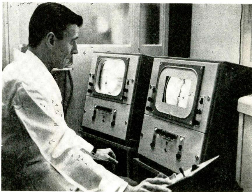
Peristaltic movement of a patient's intestine is viewed by doctors eight miles away in a Montreal hospital. Closed-circuit or transmitted tv pictures of x-ray images used with a Philips intensifier permit consultants to diagnose human ills without being on the spot
