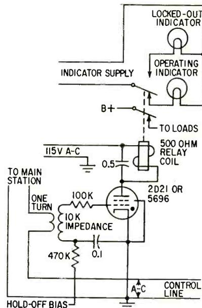
FIG. 3—Current transformer in control line locks out overridden station in system with any number of stations
