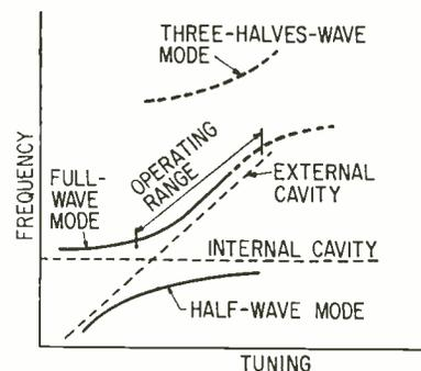
FIG. 3—Tuning curves for tightly coupled double-tuned cavity
