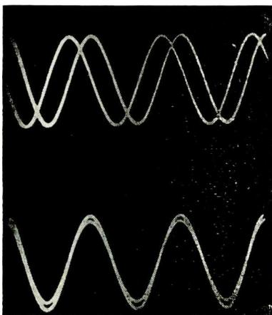
FIG. 3—Error signal shifted in phase with respect to reference signal (top) and reference signal shifted into phase with error signal by calibrated phase shifter (bottom)
