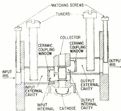
FIG. 1—Sectional view of klystron
