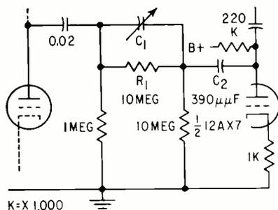
FIG. 7—Swell shoe operates capacitive volume control  $C_1$  that replaces expensive industrial-type potentiometer
