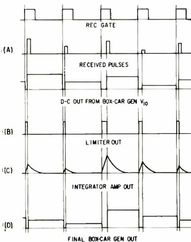
FIG. 6—Key waveforms for the ultrasonic equipment
