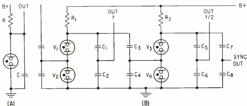
FIG. 2—Standard neon relaxation oscillator (A) is modified (B) so that series lamps have high-impedance point between lamps for sync injection
