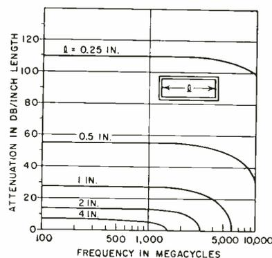
FIG. 2—Attenuation of a rectangular waveguide for  $TE_{10}$  mode. Curves continue horizontally down to 10 mc
