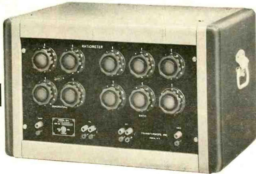
The Transformers, Inc. Model 214 A. C. Ratiometer is a precision instrument to measure any voltage ratio from 0.000001 to 1.111111. Transformer ratios can be accurately measured at "no load" or under any required load.
