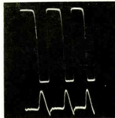
FIG. 5—Collector (top) and emitter (bottom) voltages for circuit of Fig. 4
