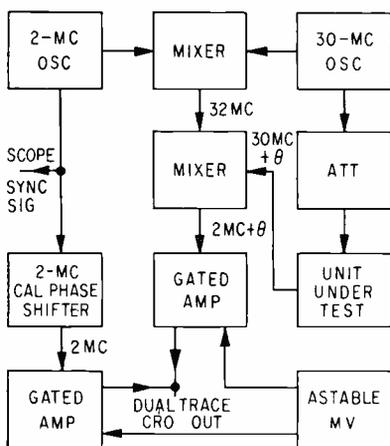
FIG. 2—Phase-measuring system has two mixers that brings 30-mc input down to 2 mc
