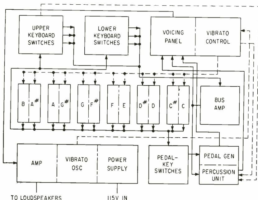
FIG. 1—Each main block in organ block diagram is a removable module with two tone generators on each of six tone modules
