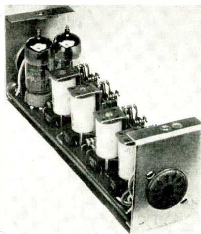
Planes of bright neon lamps form and hold easily-read 2½-inch numerals. In-line readout was designed by Computer Measurements Corp., North Hollywood, Calif., for use with electronic counters. Controller receives read-command pulses from frequency counter and operates code converters at proper moment to receive 4-line 1-2-2-4 binary decimal code from counter. Six code converters (right) translate input into 10-bit code in form of relay contact closures. Converters use unique folded relay
