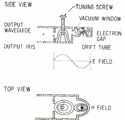
FIG. 4—Electromagnetic fields for tube
