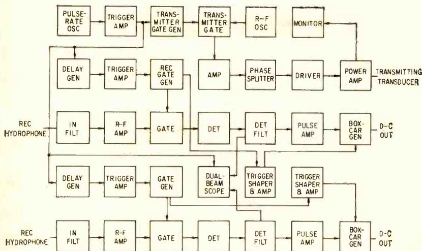
FIG. 1—Block diagram of the complete ultrasonic instrumentation system
