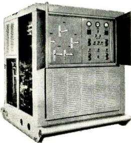
This INET 400-cycle ground power unit was tailor-made for the Atlas. In meeting all of Convair's specifications for pre-flight calibration of electrical systems, the unit operates in parallel with the missile's power system and provides remote control regulation. Frequency regulation is  $\pm 0.2\%$ .
