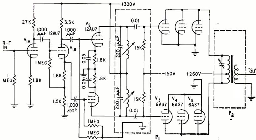
FIG. 3—Schematic diagram of the transmitter
