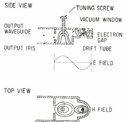
FIG. 4—Electromagnetic fields for tube
