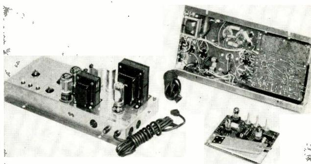
Printed-circuit section of amplifier (left and right background) contains capacitor plate operated by swell shoe (right foreground)
