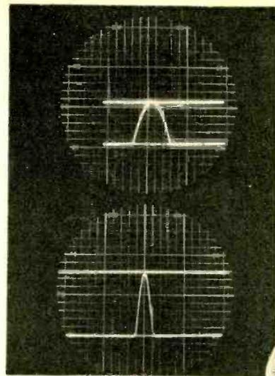
FIG. 6—Typical presentation of 5-cps signal with 0.7-volt peak is shown at top with 500 mv/in. sensitivity and at bottom with 50 mv/in. sensitivity. No bias was used for low-level signals
