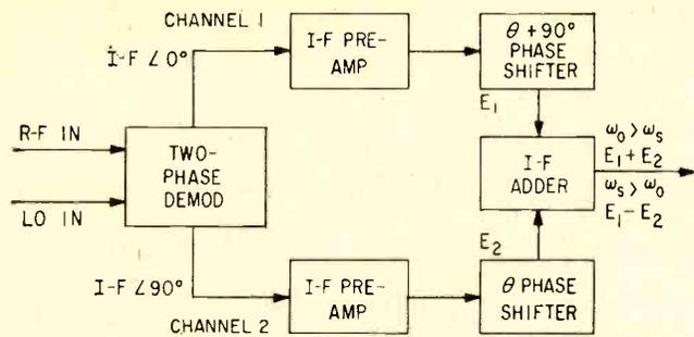
FIG. 7—Basic image-rejection receiver with phase relationships
