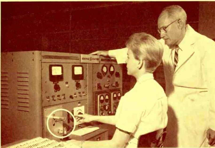
**IMPULSE-TESTING G-E SUBMINIATURES.** R. W. Field, Manager, Finished Tube Quality Control, General Electric Owensboro tube plants, watches test operator take peak and integrated output readings as 5-Star 6111's are tapped by pendulum (circle). To assure accurate readings, the meter pointers remain in indicating position until operator presses the reset button.
