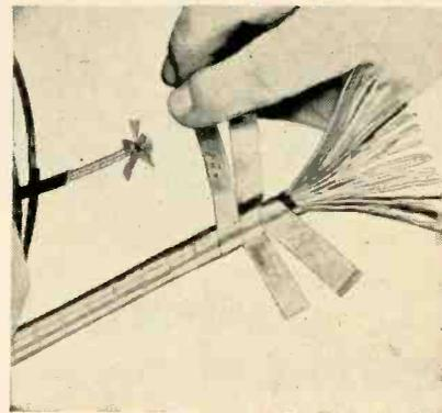
BI-DIRECTIONAL Netic Co-Netic foil strips, applied to cable in contra-spiral wraps, provide magnetic and electrostatic shielding. Cable retains flexibility and will not pickup or radiate, permitting closer positioning of components. Manufacturer, Magnetic Shield division, Perfection Mica Co., Chicago, Ill., says the shielding is not sensitive to shock, is non-retentive and does not require periodic annealing.
