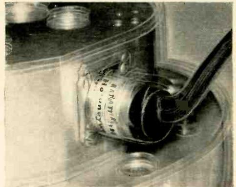
Typical M Series Gyro undergoes 20 G Linear Vibration Test with no deterioration of performance.
