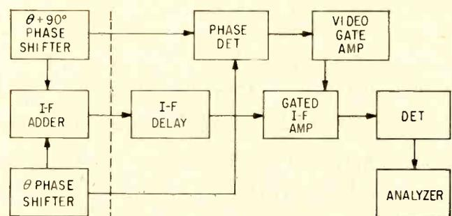
FIG. 8—Additional stages for increased image rejection
