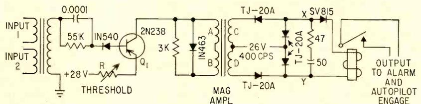
FIG. 5—Comparator-alarm circuit for system of Fig. 4 activates alarm or disengages automatic pilot if signals from dual accelerometers differ appreciably
