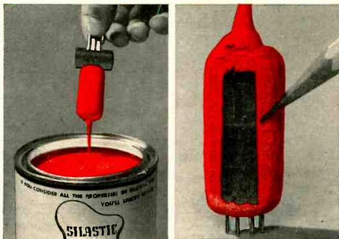
Electronic tube encapsulated with Silastic.
