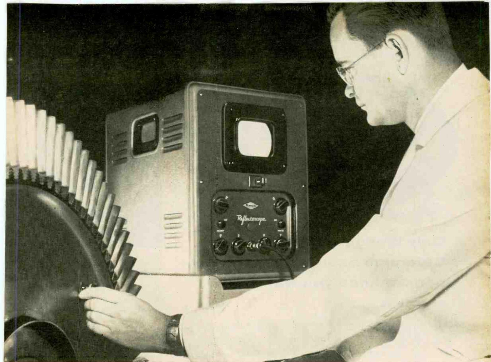
TEST ENGINEER touches Sperry Reflectoscope search unit to completed jet rotor forging in test for material flaws. A quartz crystal in the search unit converts high power pulse supplied by a Tung-Sol/Chatham 1258 hydrogen thyatron
