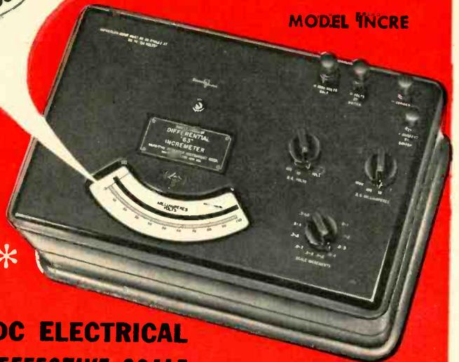
The Model INCRE essentially consists of a differential instrument of "high comparison accuracy" and a stable "high accuracy" reference source. The instrument's actual scale length is 6.3", but this represents only 10% of its total effective scale length. Each 10% of its full scale range is selected by an incremental switch in effect creating a 90% scale suppression at all times. **Ranges**—single or multirange from 200 mv. full scale (lowest reading .2 mv.)
