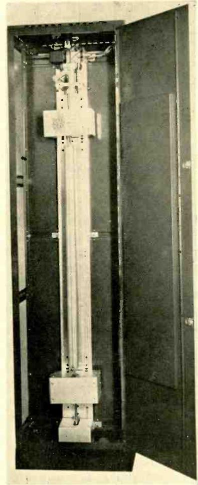
Rear view of atomic frequency standard, showing beam tube construction
