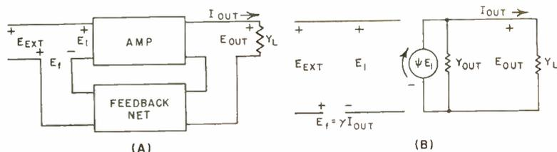
FIG. 1—Amplifier with feedback voltage in series with externally applied signal (A). Amplifier (A) can be represented by equivalent circuit (B)
