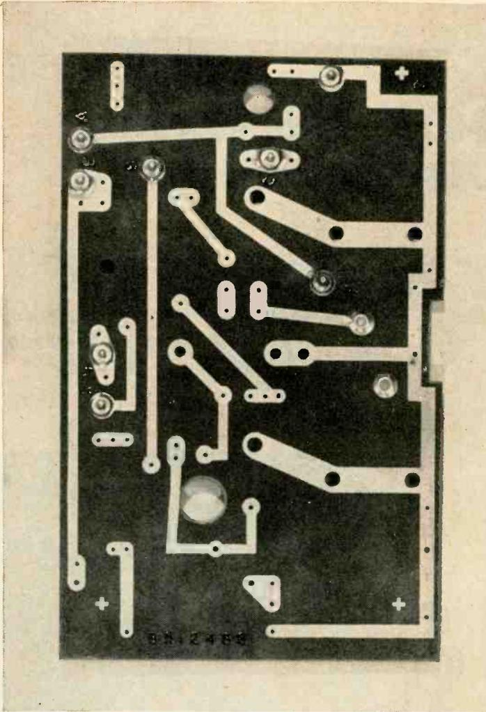
**Di-Clad 2350.** An economy paper-base phenolic grade having good tensile, flexural, compressive, and impact strength. Adequate for most non-critical printed-circuit applications. Can be cold punched and sheared up to 5/64 of an inch in thickness.
