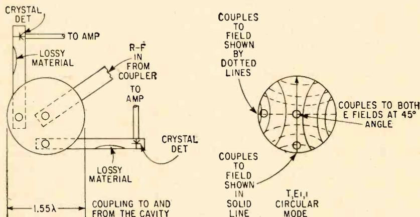
FIG. 5—Reference cavity of microwave signal source (left) and mode representation of the cavity (right)
