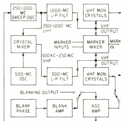
FIG. 1—Block diagram of agc and rf sections of vhf-uhf sweep generator
