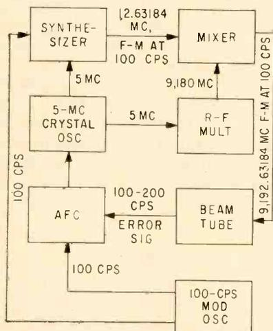
FIG. 1—System functional block diagram
