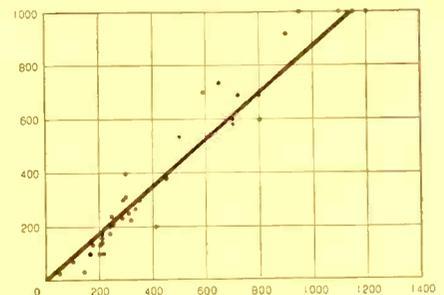
Horizontal: integrated output of impulse excitation, in microvolt-seconds. Vertical: swept-frequency vibration (100 to 10,000 CPS, 10 G peak acceleration), max output in peak-to-peak millivolts. Tube tested, Type 6021, 40 sections.  $E_f$ : 6.3 v.  $E_b$ : 100 v.  $R_k$ : 150 ohms,  $R_f$ : 10,000 ohms.
