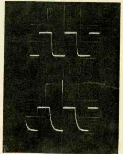
FIG. 5—Adding 200  $\mu\mu\text{f}$  capacitor in parallel with wiring capacitance at bottom shows how fall time is increased
