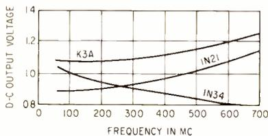
FIG. 6—Characteristics of monitoring diodes considered for use with agc circuit of Fig. 5
