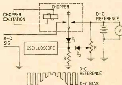
FIG. 2—Addition of biasing arrangement permits circuit to measure peaks of higher level a-c signals
