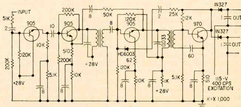
FIG. 3—Preamplifier for pitch-axis channel employs four npn silicon transistors
