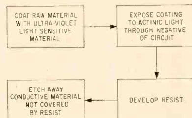
Fig. 1—Basic flow chart of photo resist printed wiring technique
