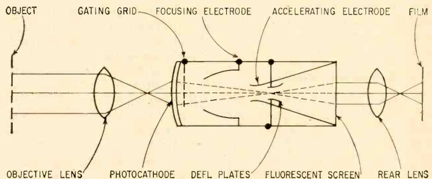
FIG. 1—Ray diagram of electronic camera shows operating principle
