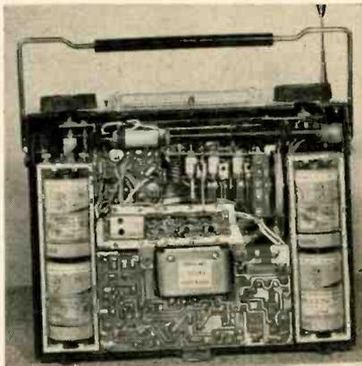
All-transistorized f-m/a-m portable radio made by Sony Corp. of Tokyo uses 15 transistors, operates on four standard flashlight batteries, weighs 5½ lb
