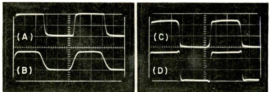
FIG. 3—100-kc input waveform (A) and resultant outputs. (B) shows output of 400-mv peak with 5-mv input. Waveforms (C) and (D) are 600-mv outputs at gains of 12 and 1.5, respectively
