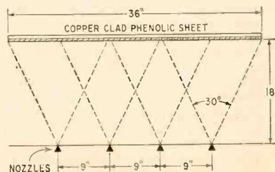
Fig. 2—Nozzle arrangement used in vapor developing operation
