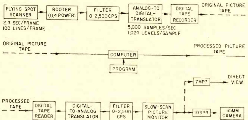
FIG. 3—Picture coding by computer simulation encompasses components shown
