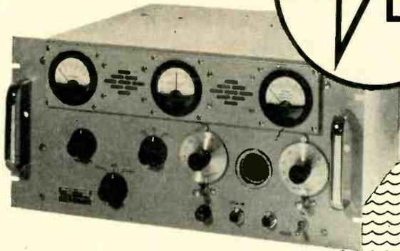
Now available in the Nems-Clarke line of telemetry receivers is the 1400 Series employing phase-lock detection. The receivers are of the double super-heterodyne type with a noise figure of less than 8 db.
