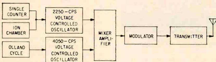
FIG. 3—Block diagram of the f-m/f-m telemetering system. Carrier frequency is 95 mc
