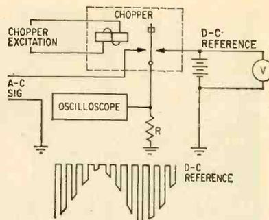
FIG. 1—Basic circuit uses chopper to compare low-level ac peaks with d-c standard. Appearance of oscilloscope presentation is shown at bottom
