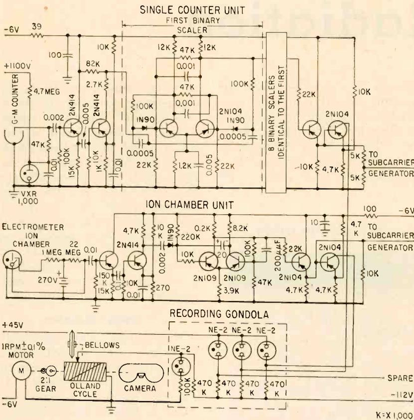
FIG. 2—Circuit schematic of the cosmic ray detection and counting circuits. Equipment is designed to operate from +30C to -40C
