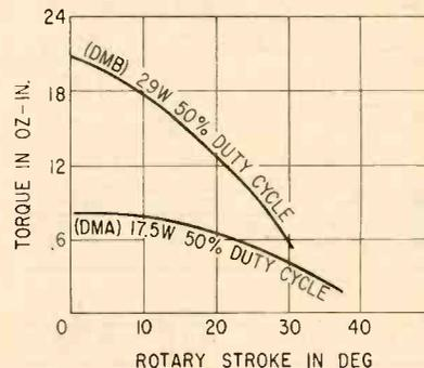
FIG. 2—Torque vs. stroke, watts and duty cycle for two models of the motor
