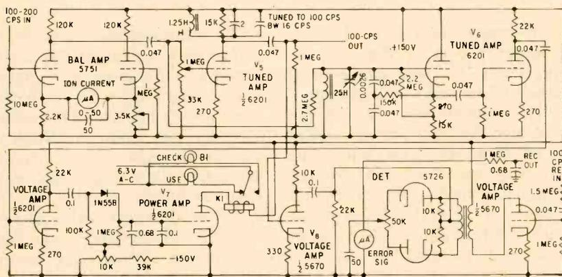
FIG. 8—Schematic of beam-tube preamplifier. Ion current meter is tuning indicator
