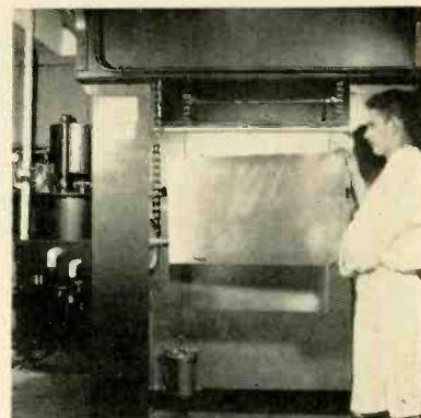
Loading vapor developing machine. Distillation unit is at left
