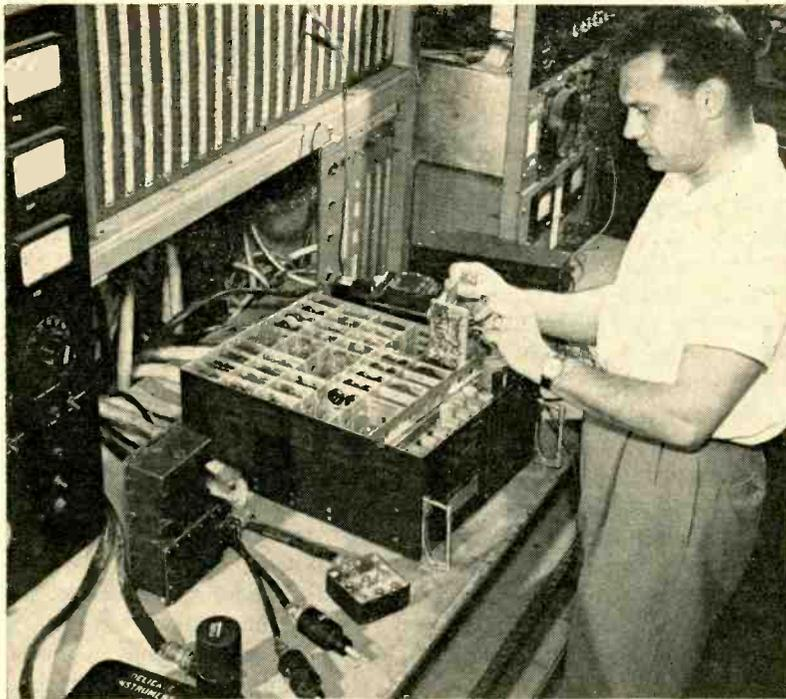
Systems engineer checks out automatic-pilot computer and amplifier as part of overall system test
