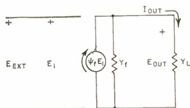
FIG. 2—Norton equivalent circuit with current feedback
