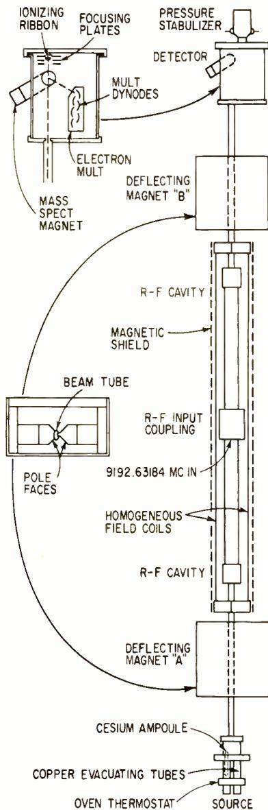
FIG. 9—Arrangement of beam tube
