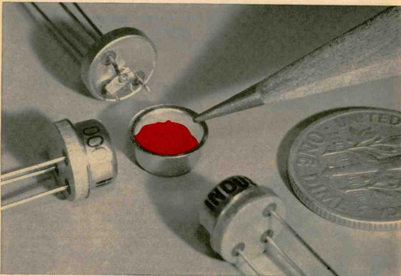
Made by Industro Transistor Corp., these miniature transistors are potted with a Dow Corning silicone compound to cushion vibration, improve heat dissipation, prevent contamination of the junction.
