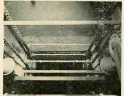
Looking down into vapor tank of developing machine
