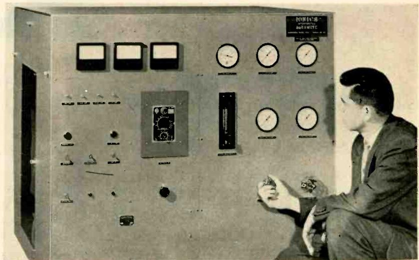
Small model of saline water conversion plant can produce 500 to 1,000 gals. per day as . . .
