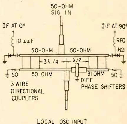
FIG. 6—Schematic representation of S-band two-phase demodulator
