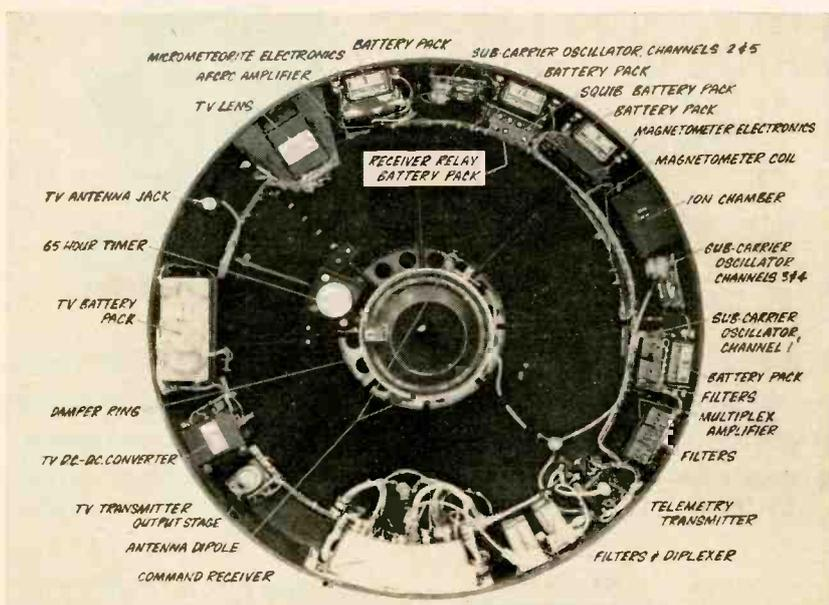
Here are inside details of Pioneer I instrumentation package Air Force sent aloft in lunar probe project directed by Space Technology Labs. Glass fiber chamber surrounds payload's 22 items
