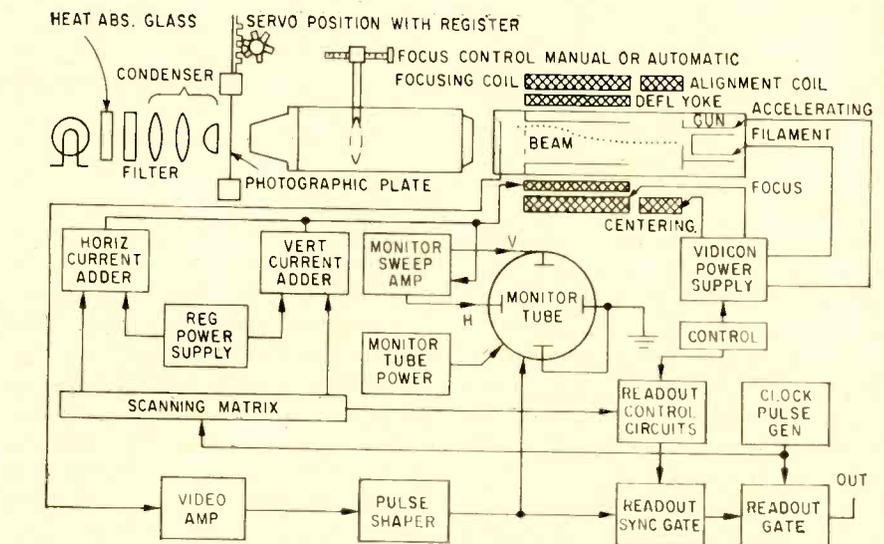
FIG. 2—Microspace storage system illustrated uses a photographic plate for storage. Information is projected onto face of vidicon
