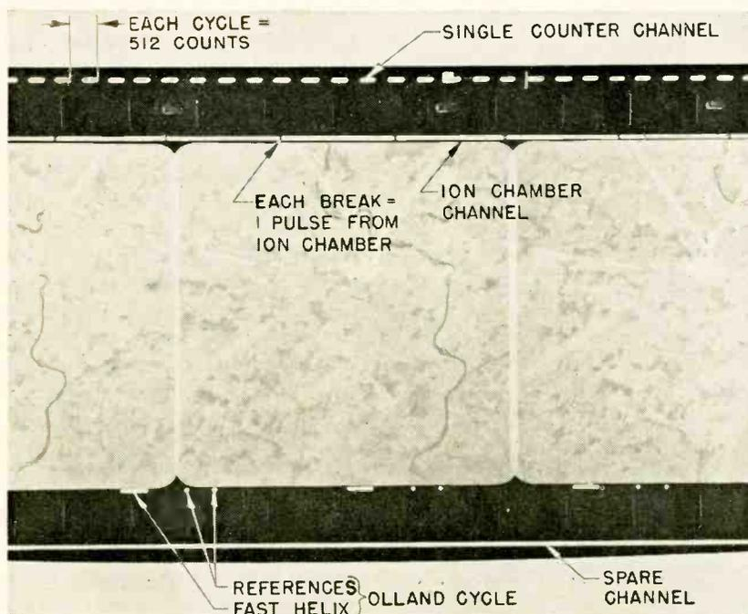
Film strip taken at a balloon height of 100,000 ft. The records are typical of the response to cosmic radiation over Minnesota during solar maximum. Each camera frame spans 100 sq mi on ground. Position of river indicates balloon drift in 3-min
