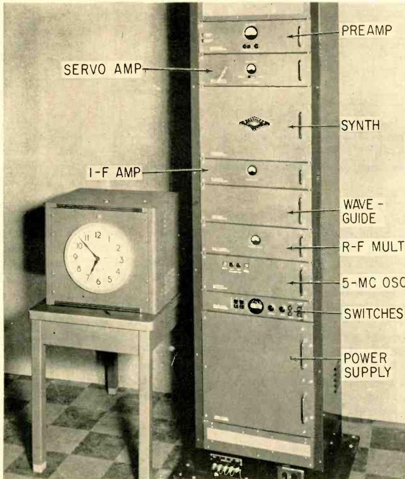
Atomic clock driving standard electric clock with built-in 100-kc to 60-cps divider. Electric clock will lose only one second in thirty years.
