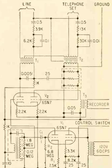
FIG. 1—Recorder connector made by Western Electric provides beeps for recording telephone conversations. Difference in level of speech from line and from studio telephone is reduced about 20 db by circuit
