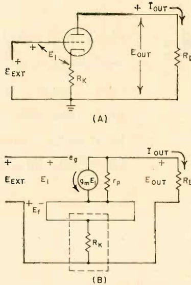
FIG. 3—Typical triode amplifier with degenerative feedback (A) can be reduced to equivalent circuit (B) for current feedback analysis
