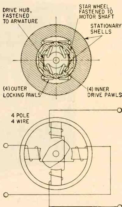
FIG. 1—Operating mechanism for digital motor (top) and schematic diagram
