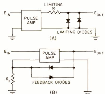
FIG. 1—Simplified schematics illustrate (A) standard limiting circuit and (B) nonlinear feedback limiting
