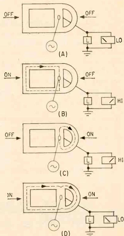
FIG. 1—Four logical states of the integrated Magnistor
