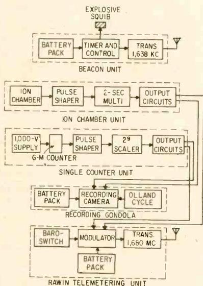
FIG. 1—Block diagram of the flight equipment using Rawin telemetering
