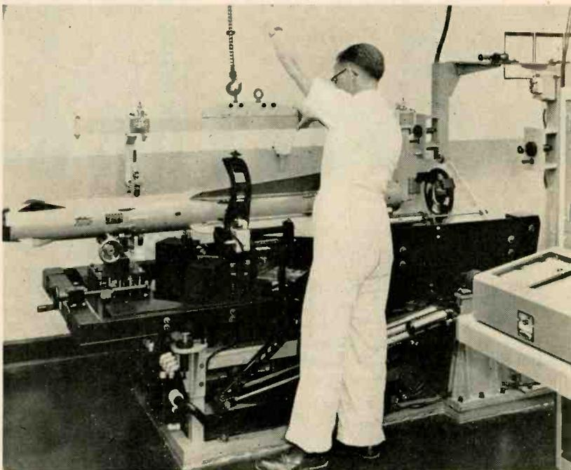
Falcon missiles are tested for balance on this aircraft missile weight and balancing system built by Baldwin-Lima-Hamilton for Hughes Aircraft. Arrangement of B-L-H SR-4 sensing elements and load cell in the stand measures missile's weight, finds longitudinal and lateral centers of gravity and thrust alignment. X-Y plotter and printer mark measurements on chart. Hoist moves missile directly from production line to platform. Missile is lined up by insertion of pin in tooling hole
