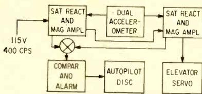
FIG. 4—Torque-modulation system has dual accelerometer that measures acceleration in pitch plane of motion. Servomotor torque is proportionately decreased with increasing acceleration
