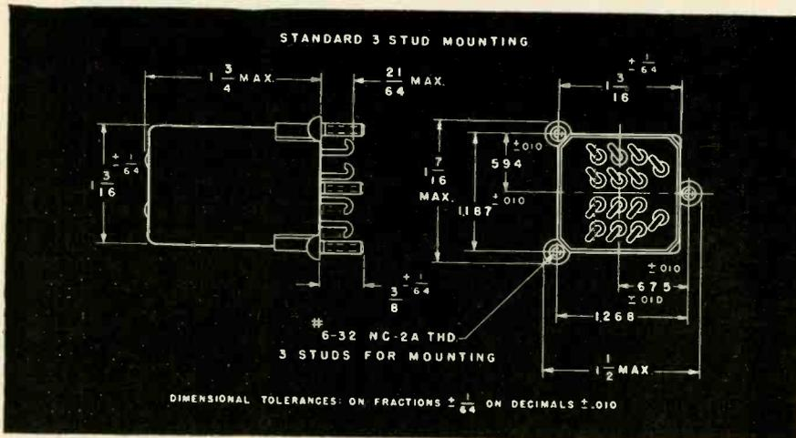
The Allied CH-12D Relay was developed to meet the more rigid requirements of vibration, shock, temperature, rupture and overload conditions of the latest MIL spec. This relay is available with other mounting arrangements for special applications, such as 4 mounting studs or brackets for Allied MHY-12D type 2 stud or 2 hole mounting. For additional information write for Bulletin CH.
