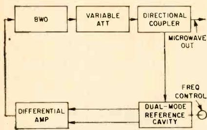
FIG. 4—Simplified block diagram of basic microwave signal source
