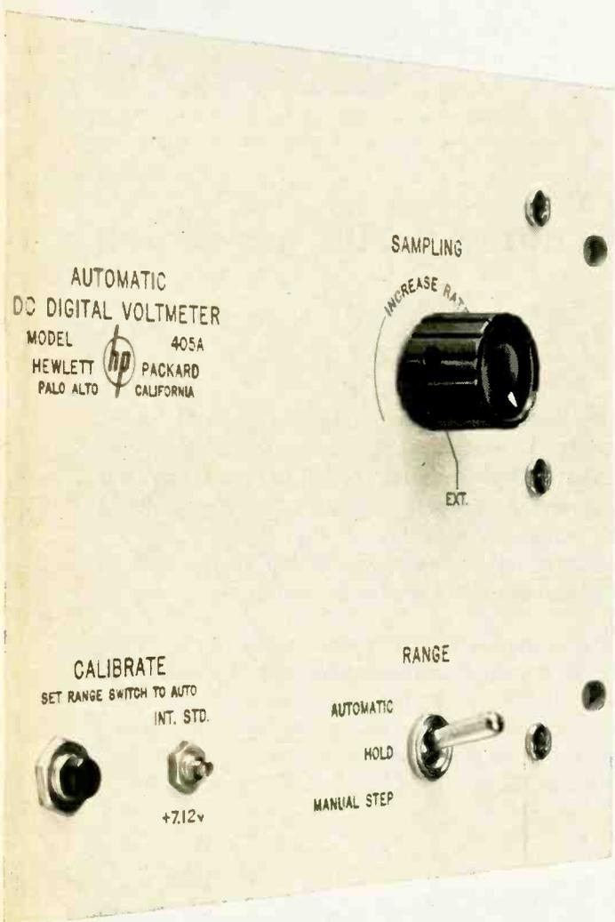
**405AR DC DIGITAL VOLTMETER** is a completely new instrument providing, literally, "touch-and-read" voltage measurements between 1 and 1,000 volts. *Range, even polarity, are automatically selected.* Readout is in-line, in bright, steady numerals.
