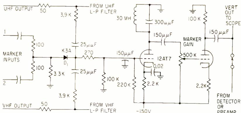
FIG. 7—Frequency-marker circuits can be used with either vhf or uhf operation
