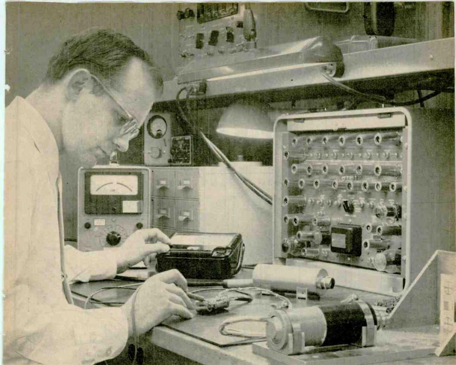
*A MISSILE AND TELEVISION INDUSTRY FIRST. Lockheed-developed, miniaturized TV cameras, designed for both government and commercial use. Only 6 inches long and 2 1/4 inches in diameter, tiny cameras extend man's vision into the unexplored. Unmanned lunar probes to the far side of the moon; lunar landings; monitoring interiors of manned spacecraft and remote TV coverage of on-the-spot happenings on a scope never before possible are some of the uses foreseen for the cameras.*
