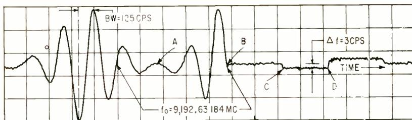
FIG. 11—Typical recording taken on atomic clock, when it goes through resonance is reversed at A and locked at B
