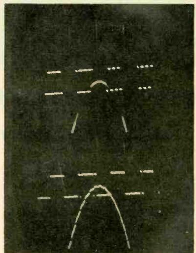
FIG. 4—A 5-cps signal at 2.5 volts is compared to upper and lower reference levels of 2.55 and 2.45 volts, respectively. Comparison chopper is driven at 400 cps in top pattern and reference chopper at 60 cps. Chopper frequencies are reversed in bottom pattern
