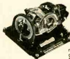
115 volts, 400 cycles, single phase, 35 watts. Pitch and roll potentiometer pick offs 890 ohms, 40 volts max. AC or DC. Speed 20,000 rpm, ang. momentum 12,500,000 gm-cm<sup>2</sup>/sec. Erection system 27 VAC, 400 cycles, time 5 min. to 1/2°. Weight 5.5 lbs.
