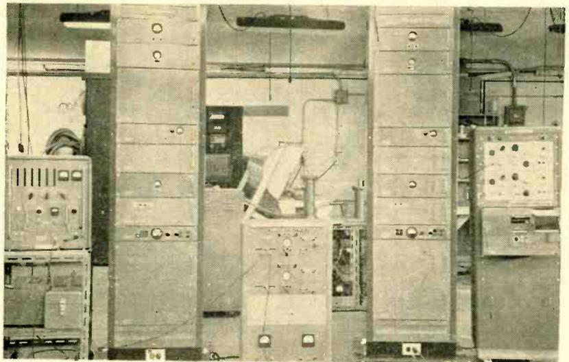
Test setup for comparing stability of one atomic frequency standard against another
