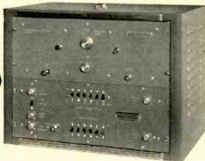
SKL's 320 mc bandwidth Model 206 distributed amplifier serves to achieve 3 mμs rise time performance with various oscilloscope models now in common use.
