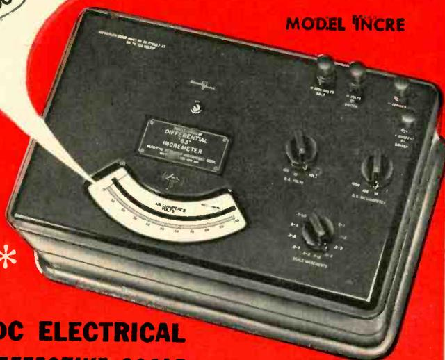
The Model INCRE essentially consists of a differential instrument of "high comparison accuracy" and a stable "high accuracy" reference source. The instrument's actual scale length is 6.3", but this represents only 10% of its total effective scale length. Each 10% of its full scale range is selected by an incremental switch in effect creating a 90% scale suppression at all times. **Ranges**—single or multirange from 200 mv. full scale (lowest reading .2 mv.)
