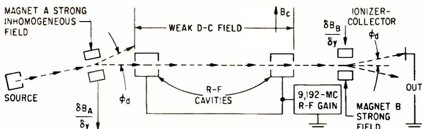
FIG. 10—Path of atoms through magnetic fields in beam tube. Deflection angle  $\phi_d$  is usually small, about 0.01 radian
