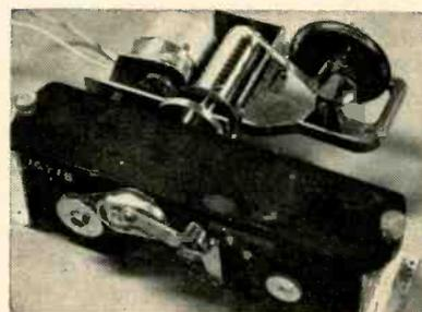
Time-lapse camera and Olland cycle pressure transducer assembly. Bellows moves contactor over rotating helix as pressure changes, varying phase of pips recorded on film
