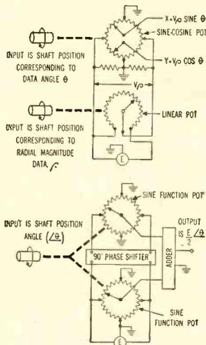
**ANGLE DATA TRANSMISSION** as used in automatic controls, directional and ranging systems, analog computers, and telemetry.
