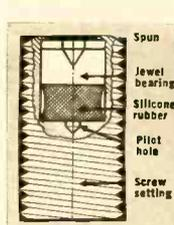
. . . add shock protection to any instrument for only pennies. Variable cushioning of silicone rubber controls movement, eliminates waste due to poor bearing adjustment in mounting.
