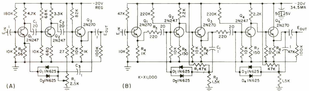
FIG. 2—Circuit diagrams of pulse amplifiers. (A) yields output variation of 8 db for input level variation of 38 db. In (B), feedback paths in two direct-coupled transistor pairs improve limiting action
