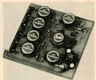
Alpha-numeric character module for storage, comparison, coincidence detection and solenoid drive
