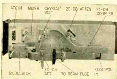
Physical arrangement of waveguide
