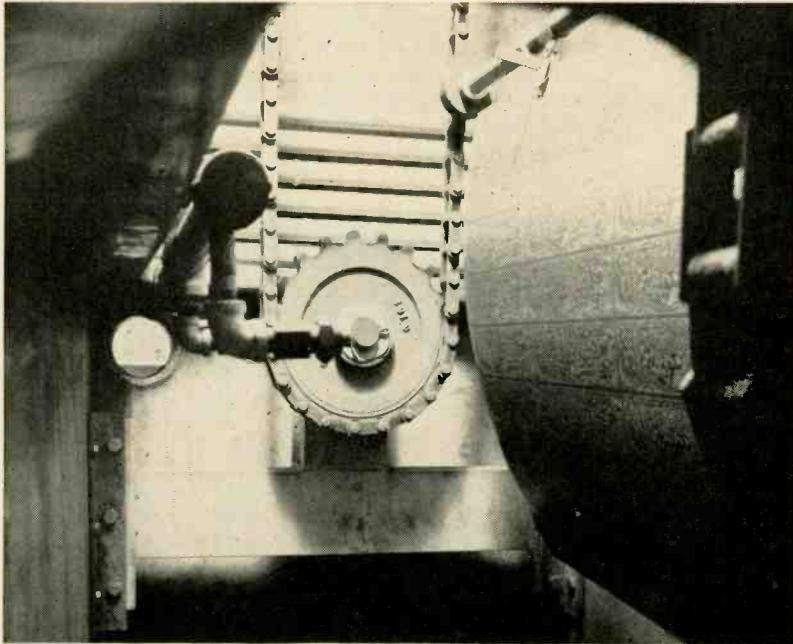
View through porthole of developing machine, showing condensation coils, mist spray nozzles and multiple sheet of printed wiring in development position
