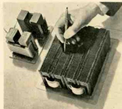
by one-quarter. Less material is used than with conventional units, cooling is easier, and lighter plates and housings are adequate. Up to 50 w per sq. in. of power can be delivered by the transducer in the range from 15 to 40 kc.
