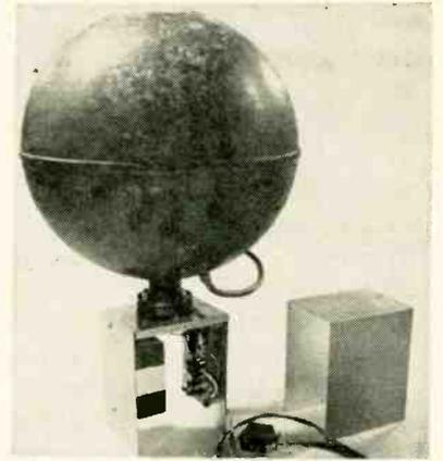
Complete ion chamber assembly. Copper-plated steel sphere is filled with pure argon at 100 psi
