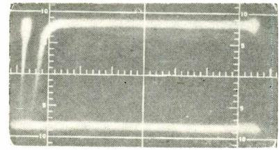
Waveform shows signal generator's output to be flat within  $\pm 0.5$  db to 250 mc at extreme right of scale
