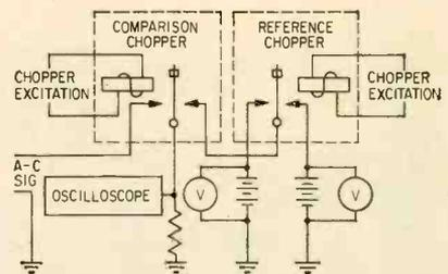
FIG. 3—Upper and lower limits can be presented by using second chopper operated at a different frequency
