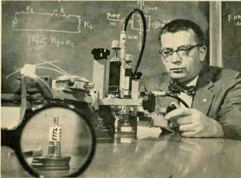
Silicon diode, shown in circle, is heart of parametric amplifier that extends 250-mile scatter link to more than 350 miles
