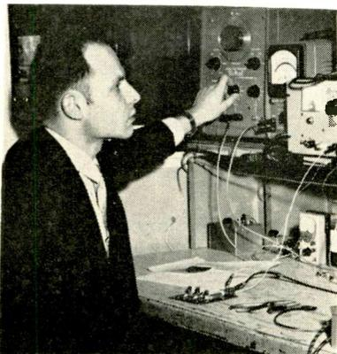
Checking the gain of amplifier-limiter
