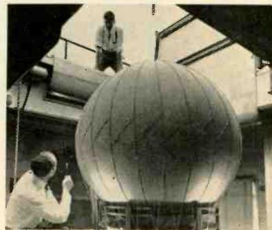
balloon is a grid of closely spaced conductors making a 45-deg angle with the perpendicular.
