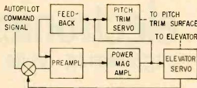
FIG. 1—Pitch-axis servo channel
