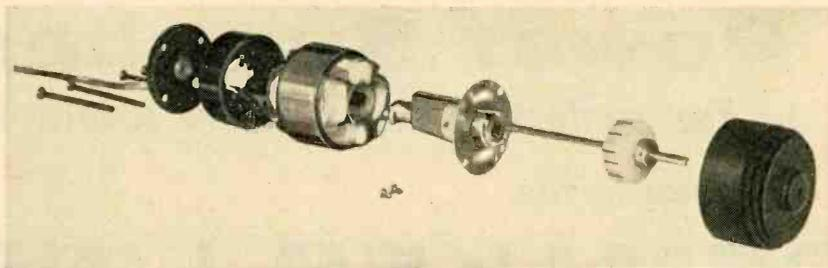
Exploded view of digital motor shows how design eliminates screws or any other type of fastener for internal assembly of parts
