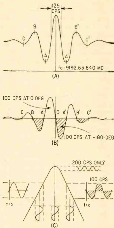
FIG. 2—Typical d-c (A) and a-c (B) resonance curves. Detection of 100-cps f-m signal is shown graphically at (C)
