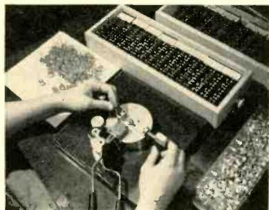
Jig bends leads of diodes into position
