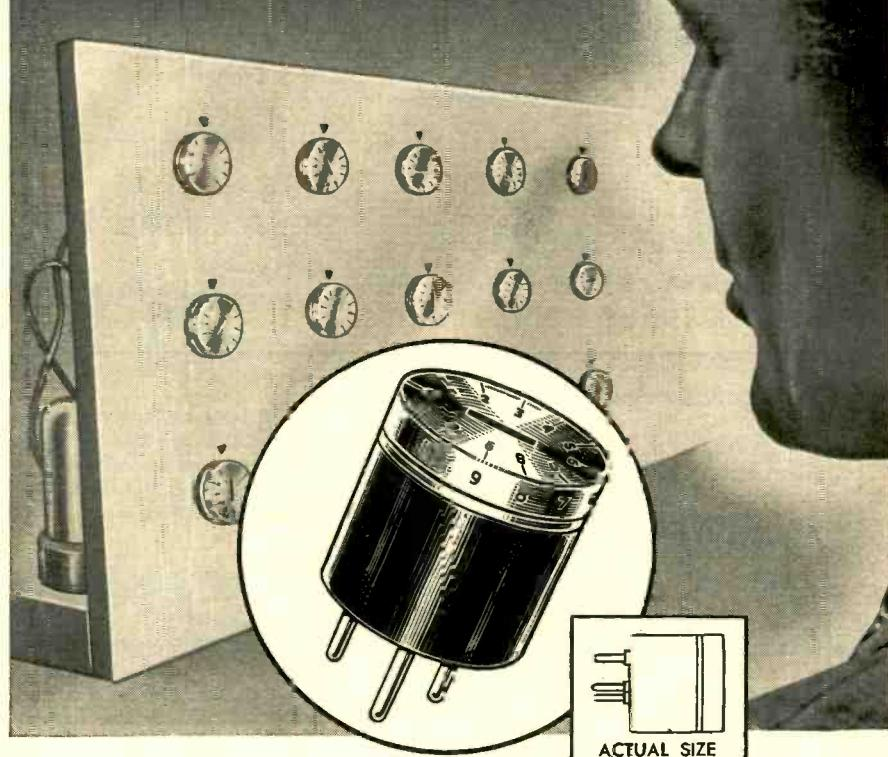
**Plugged into printed circuits or mounted on control panels**, this new  $\frac{1}{2}$ " pot speeds adjustments by letting you see what you've set. Its dual-calibrated dial tells at a glance slider location, shaft angle and voltage percentage. The  $300^\circ$  winding angle is equally graduated from 0 to 10. Zero on the dial lines up with a scribe line on the side of the pot at  $0^\circ$  rotation. Terminals are located on a standard 0.1" grid, as used in printed circuits.
