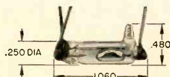
This new switch, designed for vertical gyro's, stable platforms, missiles and rockets, is the most precise mercury switch available. Differential angle—.150° max. Mass shift—.085 gm. cm. SPDT. It operates reliably at temperatures as low as -65° F. Hermetically sealed contacts. Switch is unaffected by water vapor, dust, dirt, fungus and corrosive fumes. It is rated at .225 amps., 30 vac, 400 cps resistive load. Weight—3.5 grams (including leads). Ask for data sheet No. 153.
