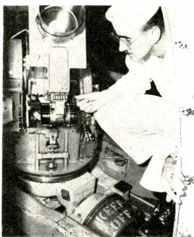
Electronics technician adjusts camera assembly of Fairand's photoelectric sextant now being evaluated on USS Compass Island. Sensing device is image orthicon tube
