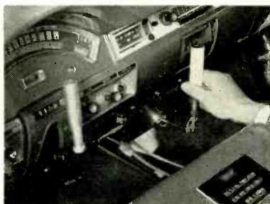
FIG. 1—Ford's control system uses two tiller sticks. Right is for steering, left controls automatic transmission
