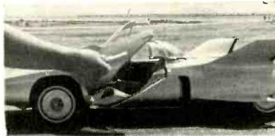
FIG. 10—Pen-shaped "ultrasonic key" opens door of GM's Firebird III from 15 feet away
