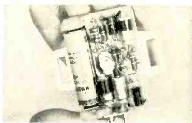
Pulse amplifier. Gain control in center of unit can be screwdriver adjusted
