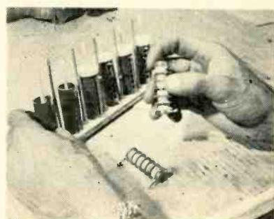
Fixture holds 6 resistors in Teflon for easy parting after cure
