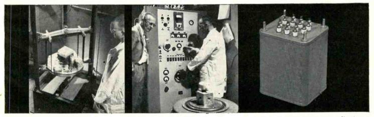
Westinghouse electronic transformers being shock-tested according to specifications of MIL-T-27A with new in-plant qualification testing equipment. P. K. Goethe, Specialty Transformer Engineering Manager at the Greenville plant, observes shake-down run of vibration test equipment in new laboratory. Particularly designed for power applications involving 60-400 cycles, the Westinghouse hermetically sealed MIL-T-27A transformers are available in the complete line of standard MIL-T-27A case sizes.
