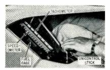
FIG. 16—Electronically controlled instrument panel in Firebird III
