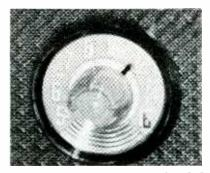
FIG. 9—Electroluminescent radio dial developed for use in American Motor's Rambler
