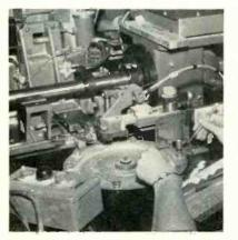
Cathode loading station. Girl drops cathode onto turntable through funnel
