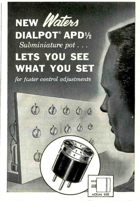
Plugged into printed circuits or mounted on control panels, this new  $\frac{1}{2}$ " pot speeds adjustments by letting you see what you've set. Its dual-calibrated dial tells at a glance slider location, shaft angle and voltage percentage. The 300° winding angle is equally graduated from 0 to 10. Zero on the dial lines up with a scribe line on the side of the pot at 0° rotation. Terminals are located on a standard 0.1" grid, as used in printed circuits.
