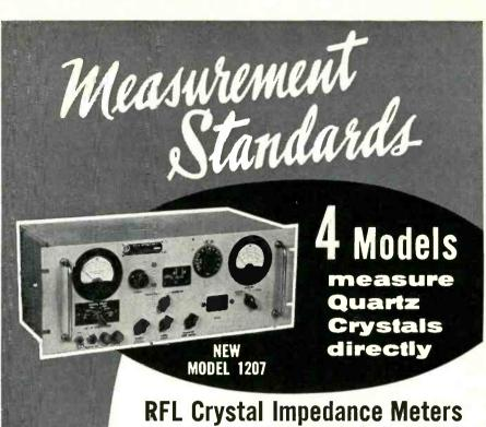
Developed under U. S. Signal Corps technical requirements for the national crystal testing standardization program. They measure resonance and anti-resonance resistance of quartz crystals, including those covered by MIL-C-3098B, for determination of capacitance, induct ance and performance index (PI).
