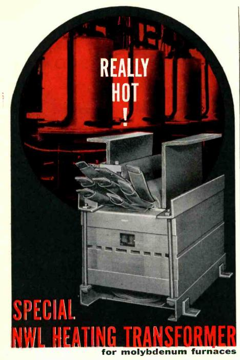
This transformer has a 10,000 Ampere secondary with a maximum of 5 volts. The primary taps are extended to reduce secondary to 0.75 volts. The secondary copper is 3/6" thick and 16" long, over which is connected and built-in a 5 Ampere current transformer. This special transformer is made for air-blast cooling as the physical size had to be kept extremely small.
