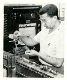
Diaphragm being inserted between compression and expansion chambers
