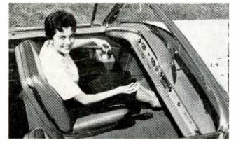
Steering, accelerating and braking operations are all done by moving single stick in GM's Unicontrol system
