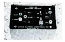
rejection at 60 cps greater than 10,000, unity gain bandwidth of approximately 500 Kc, and voltage drift less than one mv per day under laboratory conditions. It operates off two 9-v batteries, drawing a quiescent current of less than 2 ma, can deliver  $\pm 5$  volts at 10 ma. Price is \$99.50, with batteries.
