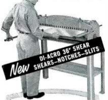
New cam-lever linkage of the Di-Acro Model 36 shear provides a greater mechanical advantage than lever actions. This makes it easier to control both machine and material so that operation is easier, faster and safer.
