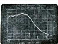
Noise spectrum analysis using internal video smoothing filter presents noise envelope aver-age versus frequency in readily appreciated form. Internal marker pips are 500kc apart.
