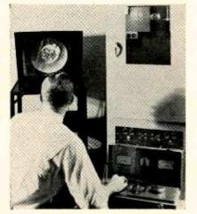
Industrial image amplifier enables x-ray inspection of devices with moving parts. Above, Picker X-Ray Corp. shows how its system would be used to inspect a gear. The television monitor permits remote viewing
