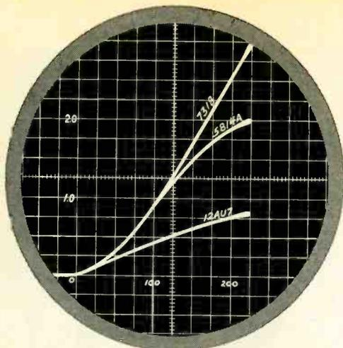
"Y" Axis Peak Cathode Current in Amperes
