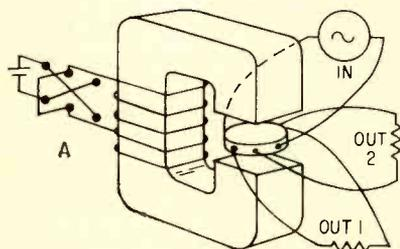
Position of switch  $A$  determines whether input is transmitted to output No. 1 or 2
