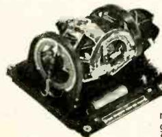
115 volts, 400 cycles, single phase, 35 watts. Pitch and roll potentiometer pickoffs 890 ohms, 40 volts max. AC or DC. Speed 20,000 rpm, ang. momentum 12,500,000 gm-cm<sup>2</sup>/sec. Erection system 27 VAC, 400 cycles, time 5 min. to 1/2°. Weight 5.5 lbs. Price **\$35.00 each**
