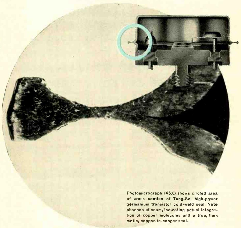
Photomicrograph (45X) shows circled area of cross section of Tung-Sol high-power germanium transistor cold-weld seal. Note absence of seam, indicating actual integration of copper molecules and a true, hermetic, copper-to-copper seal.
