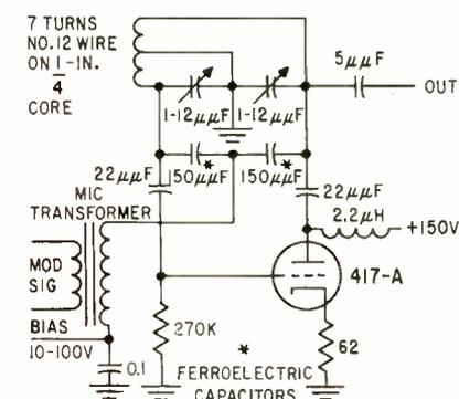
FIG. 5—F-m oscillator uses ferroelectric capacitors for tuning as well as for modulating
