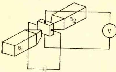
Magnetic bars  $B_1$  and  $B_2$  concentrate earth's magnetic field at sample. Bars are rotated for null reading
