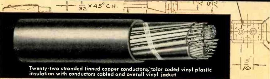
Twenty-two stranded tinned copper conductors, color coded vinyl plastic insulation with conductors cabled and overall vinyl jacket
