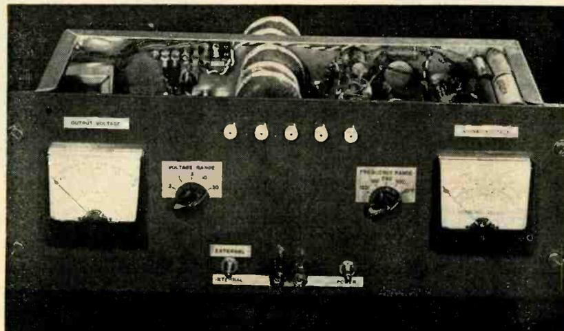
Front panel view of tuned voltmeter designed for power system analysis
