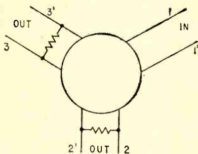
Load resistances must be of proper values for device to circulate. May be used with parallel resistances
