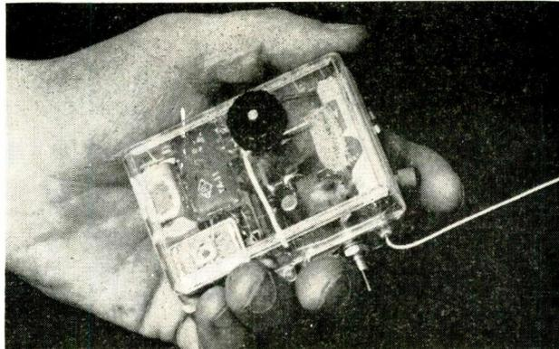
Plastic-encased miniature transmitter has electrically tuned oscillator and is powered by hearing-aid batteries
