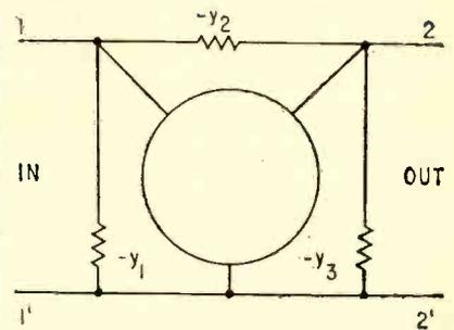
For amplifier to isolate,  $y_1$ ,  $y_2$  and  $y_3$  must have precise values
