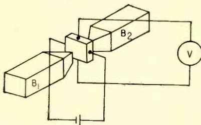
Magnetic bars  $B_1$  and  $B_2$  concentrate earth's magnetic field at sample. Bars are rotated for null reading
