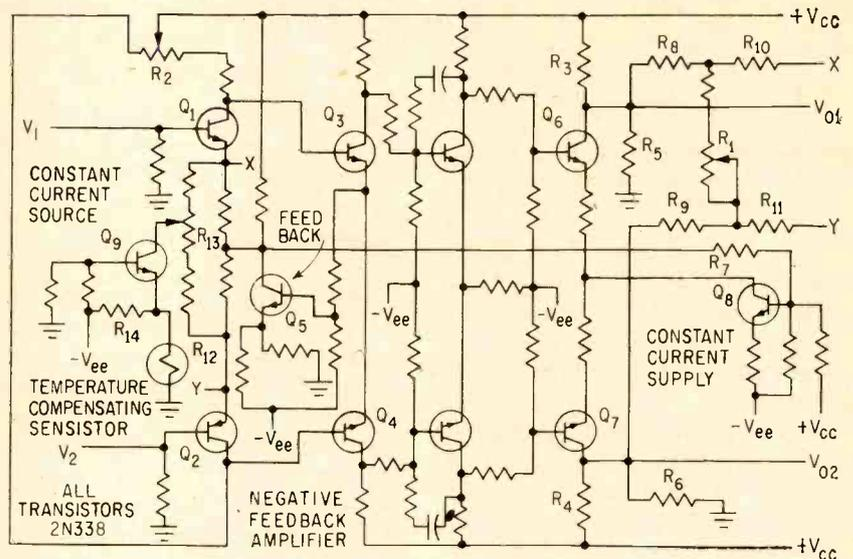
tures below 80 C, is due primarily to thermal changes of  $V_{be}$ . Since  $V_{be}$  has a predictable temperature characteristic and is stable with time, its thermal effect is reduced appreciably by the differential connection.
