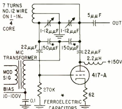
FIG. 5—F-m oscillator uses ferroelectric capacitors for tuning as well as for modulating
