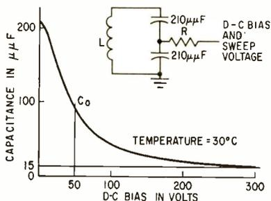
FIG. 1—Ferroelectric capacitors are connected in parallel with bias and sweep voltages but in series with r-f voltage to keep low r-f field across each capacitor. Plot shows capacitance against bias voltage with  $C_0$  the operating point
