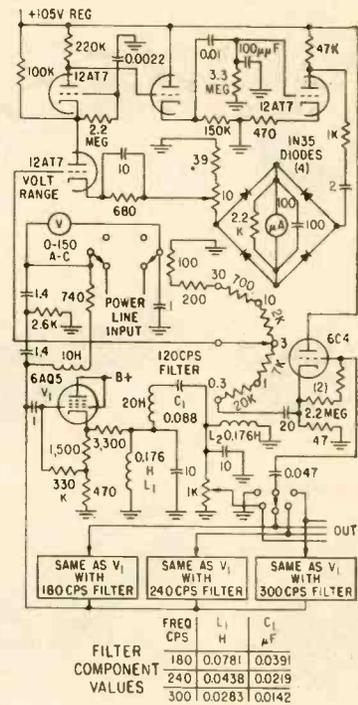
FIG. 1—Tuned voltmeter construction has five ranges of 0.3 to 30 v full scale
