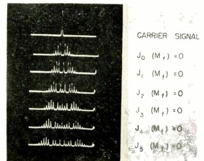
FIG. 8—Deviation of 110-kc sine-wave modulating signal is shown as a function of amplitude with 46-mc carrier and 50-volt bias
