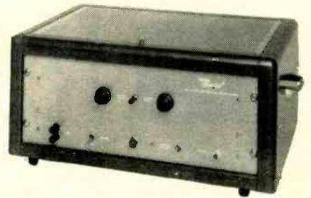
**What it does:** produces a pulsed output whose frequency is proportional to input voltage.
