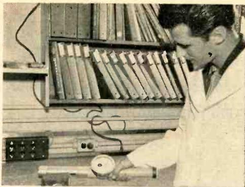
Direct-indicating logarithmic scale on meter of transistorized Geiger counter eliminates reading error resulting from incorrect positioning of range switch
