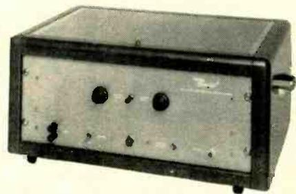
**What it does:** produces a pulsed output whose frequency is proportional to input voltage.
