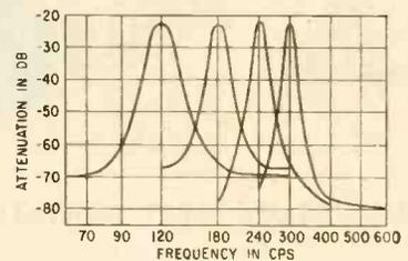
FIG. 2—Response curve of selective voltmeter filters
