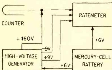
FIG. 1—Counter produces pulses whose rate of occurrence is proportional to radiation intensity of contaminated area
