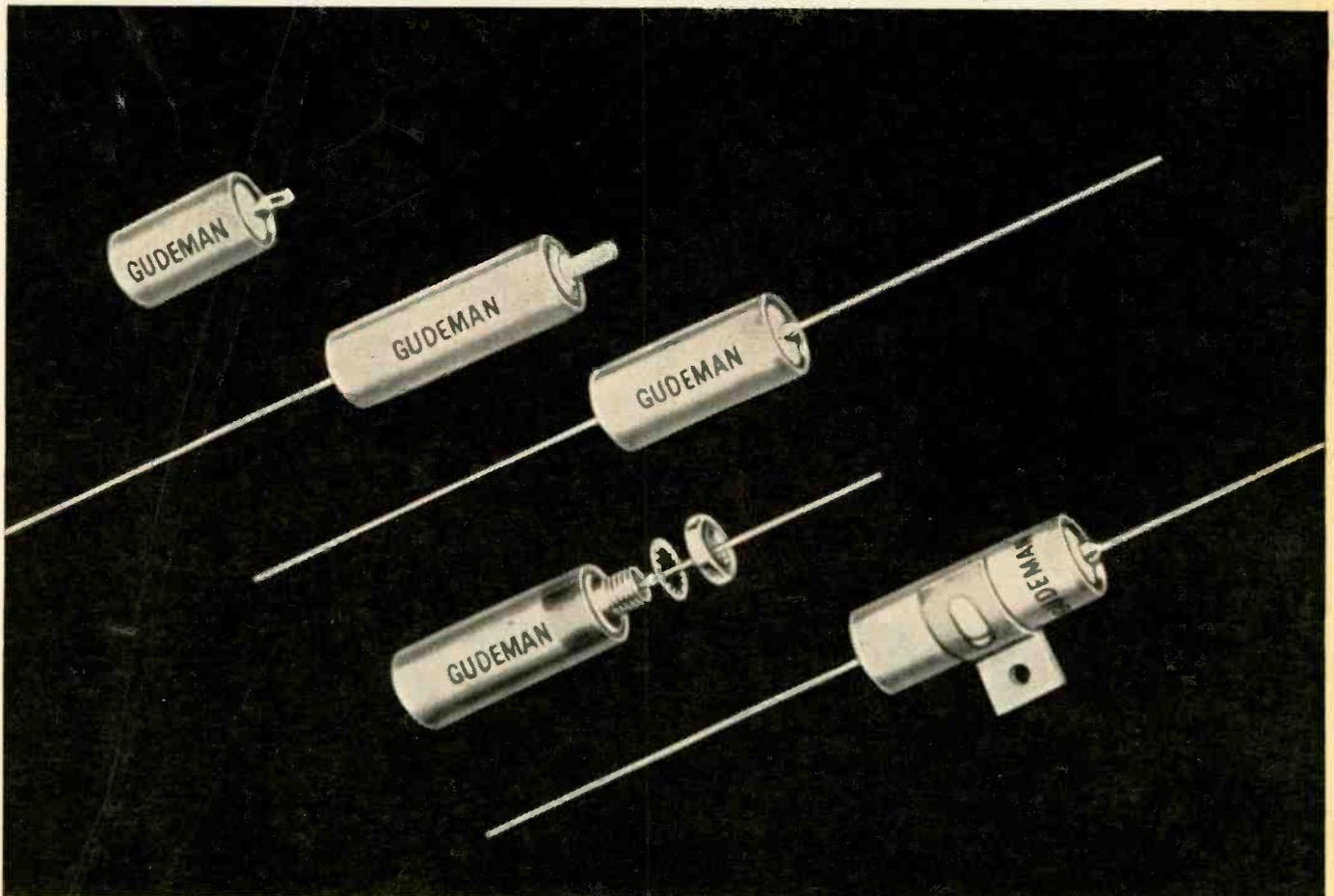
These miniature capacitors made by Gudeman Company for filter, by-pass and blocking service, are impregnated with silicone fluids to decrease electrical losses and increase permissible operating temperatures. Designed to meet all specifications of characteristic "K" MIL-C-25A, they have an operating temperature range of  $-55$  to  $125$  C.
