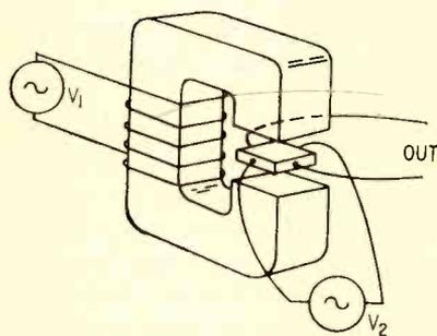
Also circuit for analog multiplier and frequency spectrum analyzer. Output is proportional to product of  $V_1$  and  $V_2$
