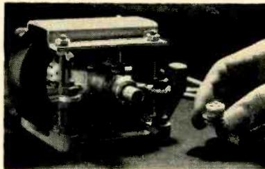
units. They are essentially high-frequency generators for the microwave bands. Tuning characteristics are linear over a 1.7 to 1.0 frequency range or greater, with changes in anode voltage. Mechanical tuning is not necessary. Circle 201 on Reader Service Card.
