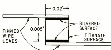
FIG. 2—Construction diagram shows silvered surfaces on which leads of capacitors are soldered
