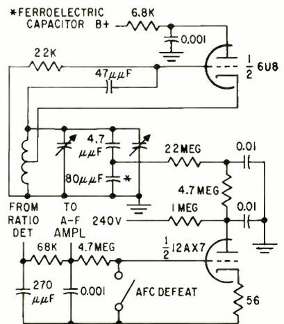
FIG. 11—Automatic frequency control is obtained in f-m tuner by amplifying change in output from ratio detector caused by local oscillator drift and applying it to ferroelectric capacitor
