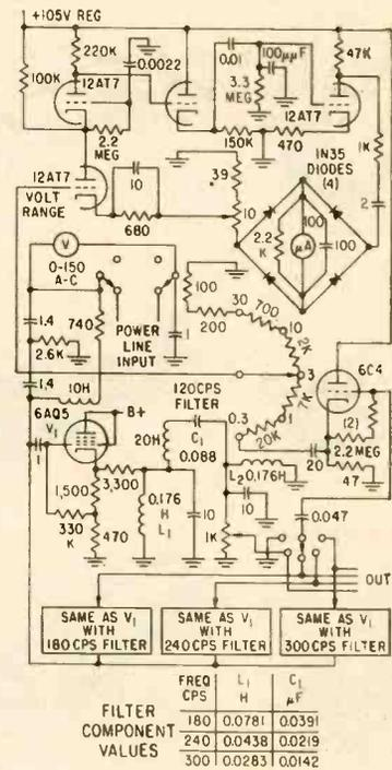
FIG. 1—Tuned voltmeter construction has five ranges of 0.3 to 30 v full scale
