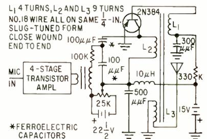
FIG. 9—Transistorized f-m oscillator operates in 50-mc range
