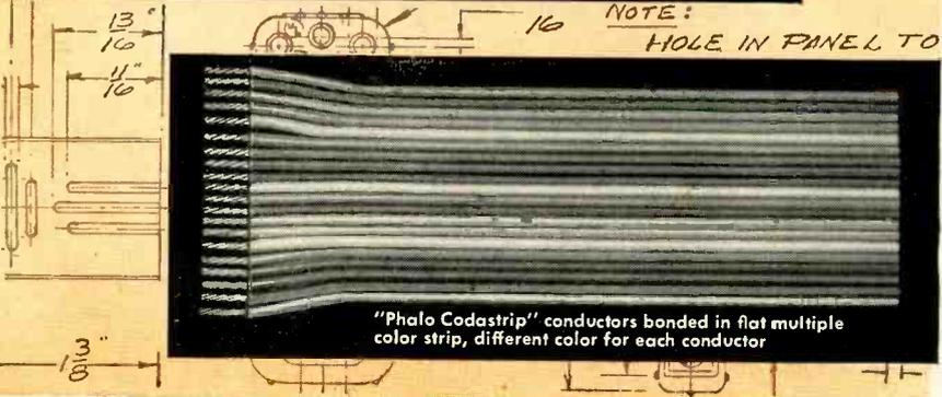
"Phalo Codastrap" conductors bonded in flat multiple color strip, different color for each conductor
