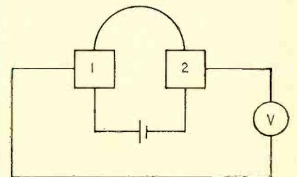
If magnetic field is different in two samples, voltmeter reads; if not, outputs cancel
