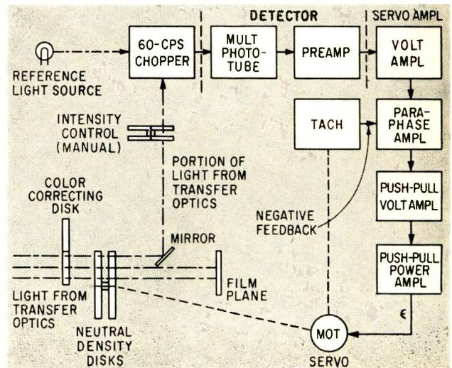
FIG. 2—ROTI automatic exposure control
