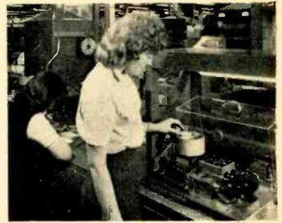
Dice measuring equipment being charged. Charging is normally done through opening in top of dust cover
