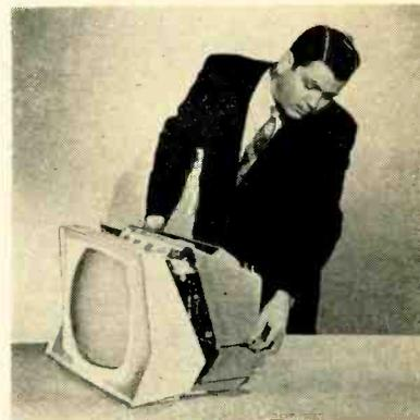
Design engineer shows modular chassis separation used in latest Sylvania portable
