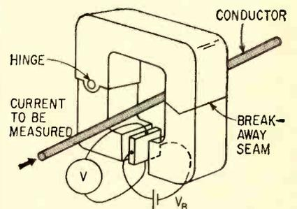
Some type of box holds sample and magnet pieces together. Device becomes wattmeter if voltage across conductors is used in place of  $V_B$
