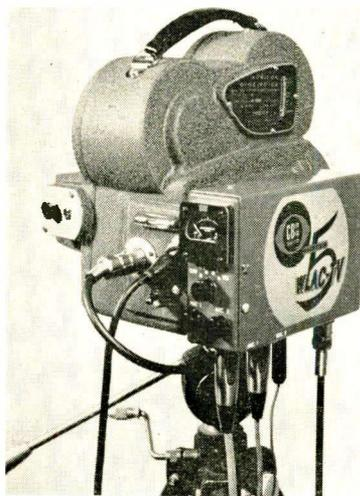
Transistor amplifier is mounted on camera
