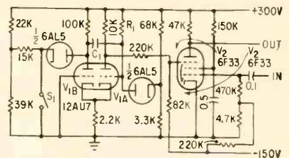
FIG. 1—When switch  $S_1$  is closed, the astable multivibrator opens the gate for period determined by the values of  $C_1$  and  $R_1$ .
