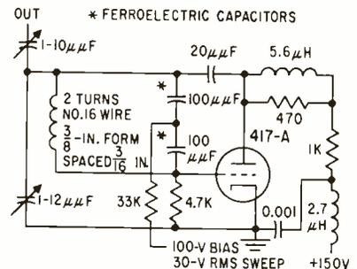
FIG. 3—Vhf swept oscillator has tuning ratio of about 2 to 1 from 20 to 250 mc and about 1.5 to 1 from 250 to 400 mc
