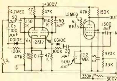
FIG. 2—When switch  $S_1$  is closed, gate is opened. Negative-going trailing edge of pulse closes gate again
