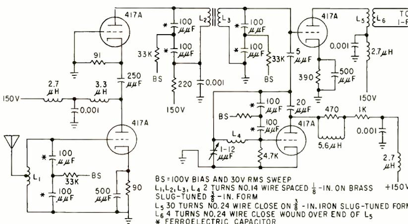
FIG. 10—Tuned stages of panoramic receiver are packaged plug-in units covering 35 to 70, 70 to 130 and 130 to 200 mc
