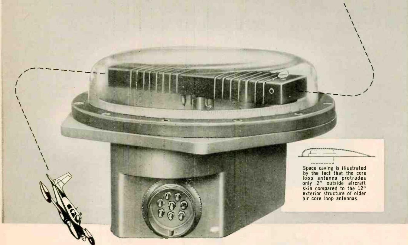
Space saving is illustrated by the fact that the core loop antenna protrudes only 2" outside aircraft skin compared to the 12" exterior structure of older air core loop antennas.
