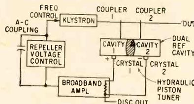
FIG. 1—Block diagram of the dual-cavity stable reference oscillator
