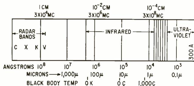
FIG. 1—Location of Infrared Spectrum
