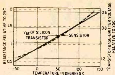
FIG. 3—Temperature characteristics of silicon resistor element, used to compensate for thermal variation due to  $V_{be}$ .
