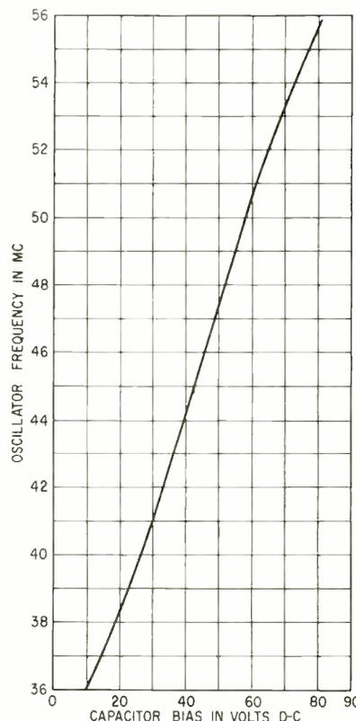
FIG. 6—Plot of frequency against bias shows linear relationship between the two in f-m oscillator shown in Fig. 5
