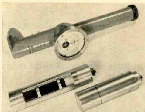
Disassembled probe handle showing case and meter (top), high-voltage generator and ratemeter circuit board (bottom, left) and battery housing (right)
