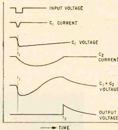
FIG. 2—Circuit produces indicated current and voltage waveforms
