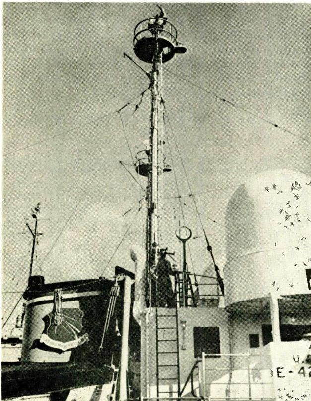
Radomes and mast-top tracking antenna on one of the six telemetry ships
