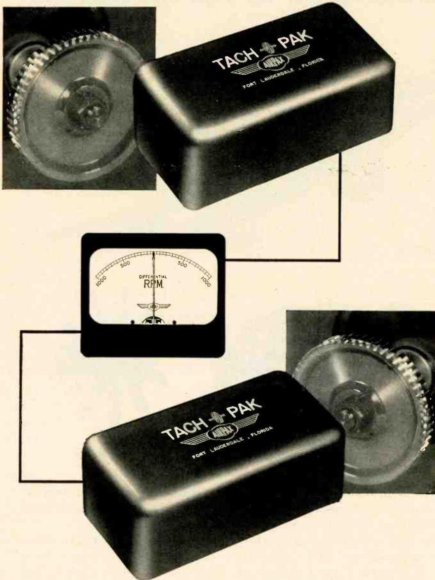
The difference in speed between two rotating shafts is accurately sensed and indicated on a center-zero meter. Even slight variations are instantly transmitted to the indicator. The proximity magnetic pickups used with the system do not impede shaft rotation. Shaft speeds may be adjusted manually or, if a closed servo loop is used, a predetermined rotational speed difference may be maintained automatically.
