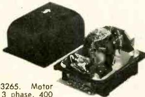
Part #653265. Motor 115 volts, 3 phase, 400 cycle, 8 watts, 20,000 RPM. 3-minute runup, synchro pickoffs, roll 360°, pitch 85°. Synchro excitation 26 volts, 400 cycle, 150 m.a. Vertical accuracy  $\pm 1/2^\circ$ . Weight 3 1/2 lbs. Approx. dim. 5 3/4" L., 4 1/2" W., 4 1/2" H. Price **\$35.00**
