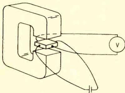
When used as a transducer (for microphone or strain gage), sample moves in and out of magnetic increasing or decreasing voltmeter reading respectively
