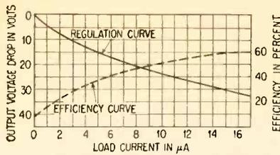
FIG. 3—Regulation and efficiency curves for high-voltage generator
