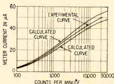
FIG. 4—Metering circuit calibration curves. Two calculated curves apply to extreme limits of the adjustment for  $R_2$ .
