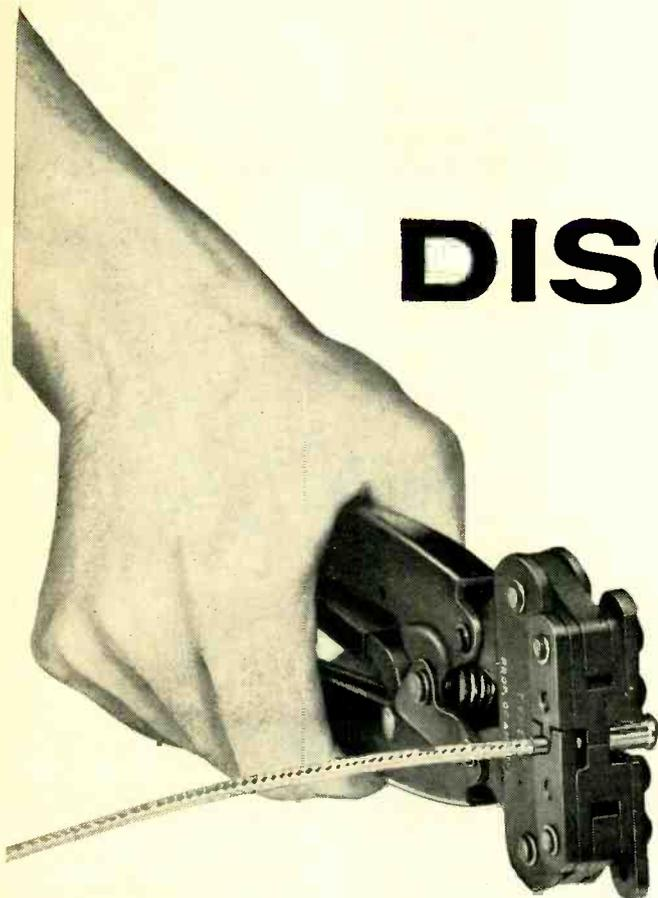
**COAXICON**—brand new. One stroke of the A-MP precision tool does it. Two strokes and you have the pin and receptacle units permanently attached to coaxial cable. For low level circuitry, either panel mounted or free hanging.
