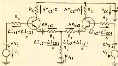
FIG. 1—Common-emitter amplifier configuration, used to pinpoint basic causes of drift sources
