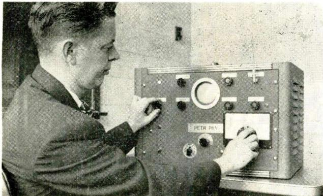
Panoramic receiver using electrically tuned capacitors sweeps between 35 and 200 mc. Frequency change with time is linear
