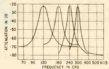
FIG. 2—Response curve of selective voltmeter filters
