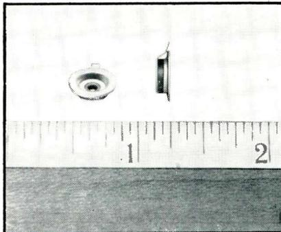
Designed for voltage tunable CW or pulsed operation over the Government X-band (8500 to 9600 Mc), the QK-684 integral magnet backward wave oscillator delivers 10 to 50 mW over delay-line voltages ranging from 215 to 325 vdc. Regulation of a special control grid facilitates pulsed or amplitude modulation to meet power and frequency requirements. Models available for coupling to standard, type "N" connectors.
