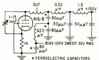
FIG. 4—Lumped-constant technique was used in designing vhf oscillator that delivers about 10 mw into 50 ohms
