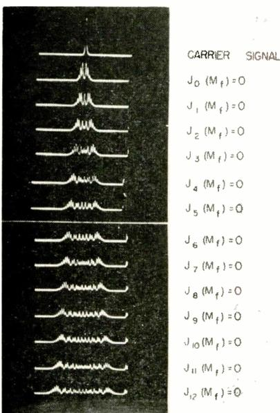
FIG. 7—Bessel function plot shows 40-kc sine-wave modulating frequency with amplitude varied to obtain indicated roots. Carrier is 46 mc and bias is 50 volts
