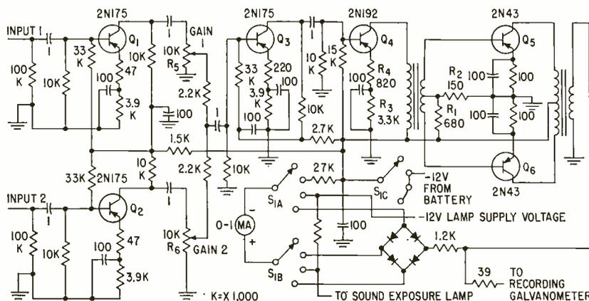
FIG. 1—Dual-input amplifier for Auricon CM-72A drives recording galvanometer
