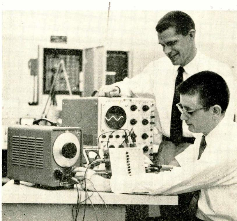
Engineers demonstrate the low-drift d-c differential amplifier. Output of amplifier is visible on the oscilloscope screen
