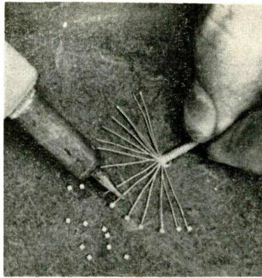
In making ferroelectric capacitors, leads are attached to silvered surface
