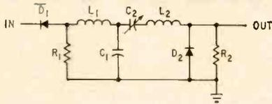
FIG. 1—Delay times from 5  $\mu$ sec to 5 millisecc are produced by circuit with stability better than 0.1 percent
