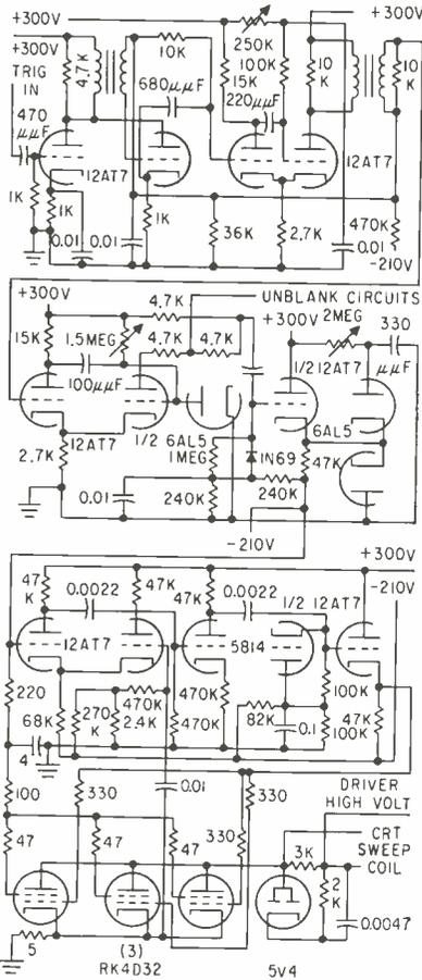
FIG. 3—Deflection yoke and sweep circuits for crt must operate at sweep lengths varying by a factor of 8 to 1
