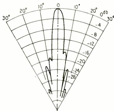
FIG. 3—Plot shows directivity of transducer
