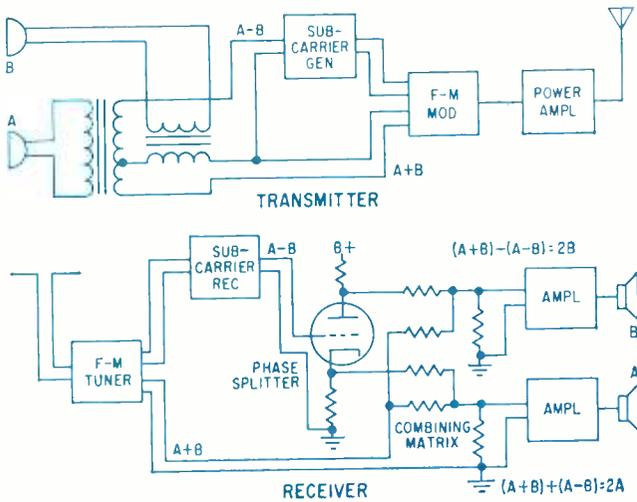
FIG. 1—Sum-and-difference f-m multiplexing arrangement used in Crosby-Harkins stereo system tests
