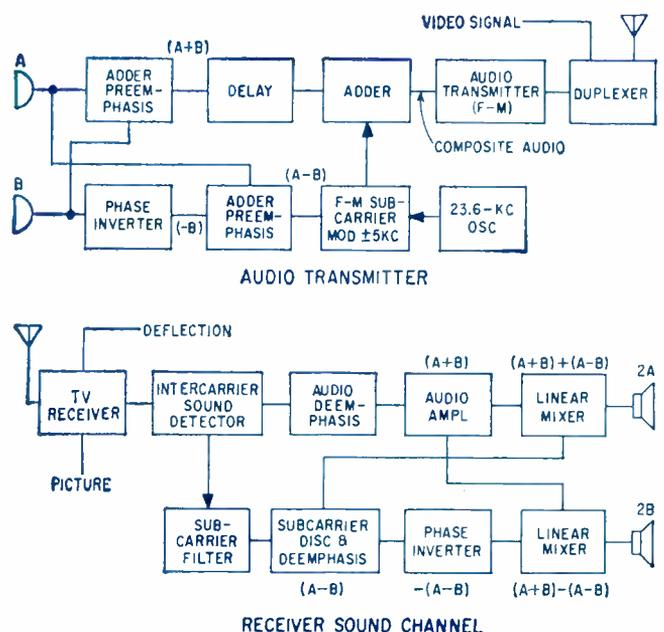
FIG. 7—Stereo setup for television sound channel as demonstrated by Motorola
