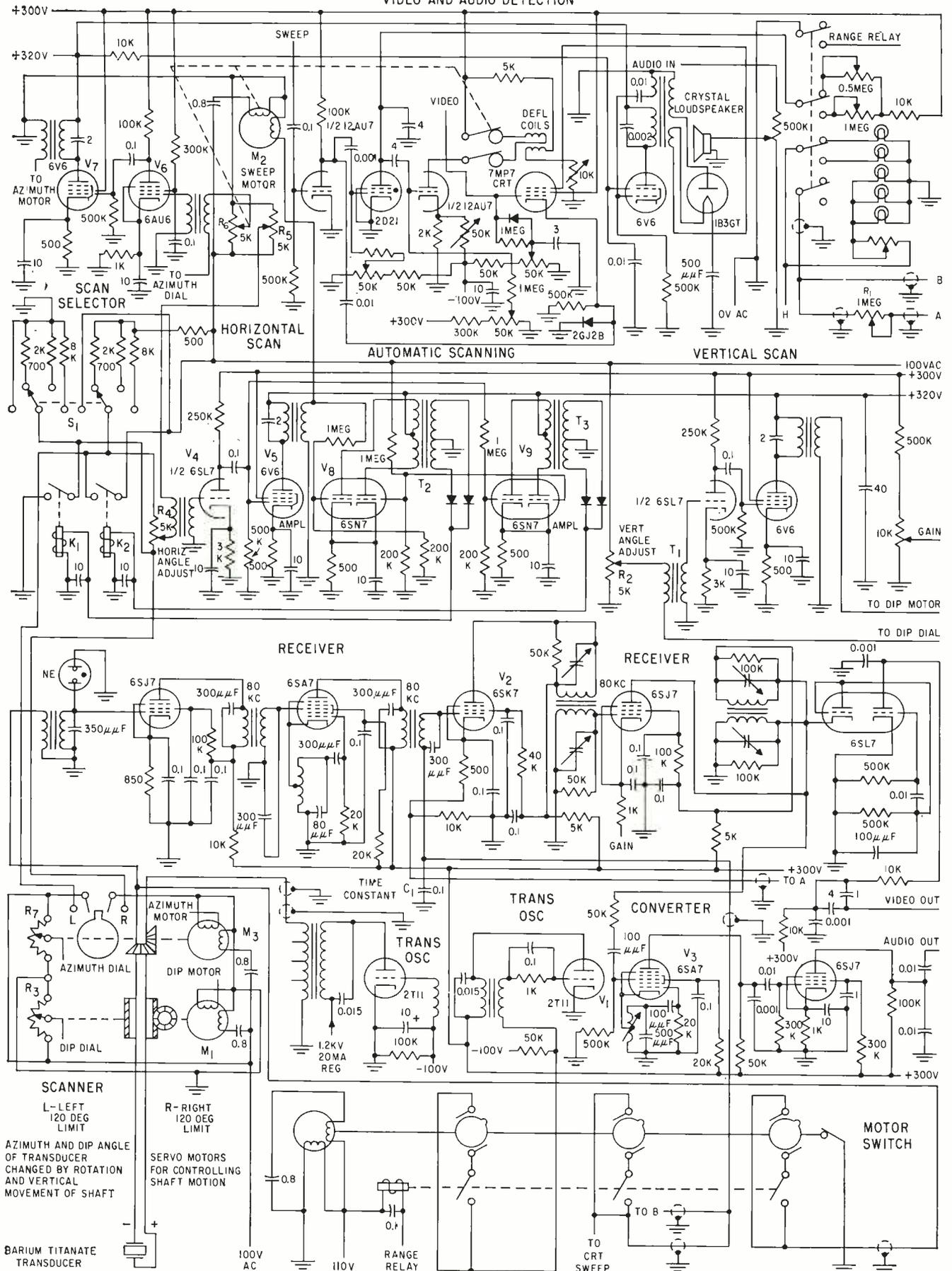
FIG. 2—Circuit diagram of sonar fish detector shows detailed circuit connections to transducer, oscillator and detection system
