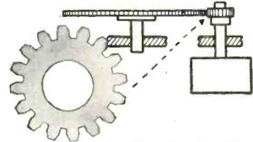
**HIGH-VOLTAGE (1800v.) RF ISOLATION** is achieved by miniature C-D-F Dilecto gears in an aircraft receiver-transmitter switch. They also had to exhibit dimensional stability through a wide temperature range, resistance to fungus growth and thermal shock.
