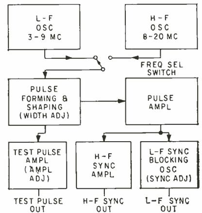
FIG. 1—Pulse generator uses two oscillators and has three outputs
