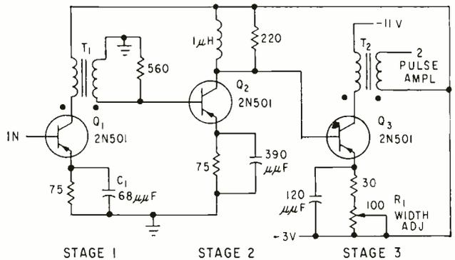
FIG. 4—Pulse former and shaper has three stages
