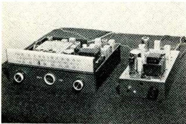
Stereo multiplex adapter, right, works with f-m/a-m set, left
