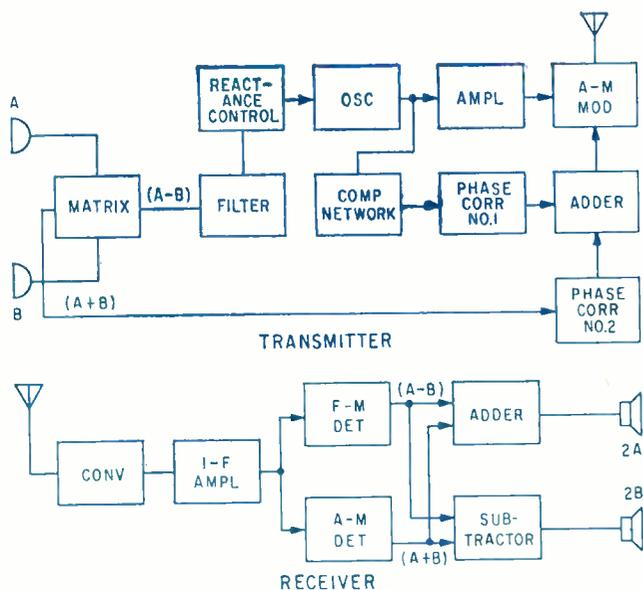
FIG. 9—Standard broadcast stereo system by Westinghouse uses a-m and narrow-band f-m
