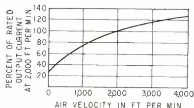
**FIG. 2—Forced air cooling rerating curve for high-current types**
