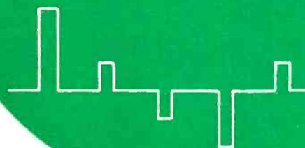
**THE QUATERNARY WAVE** combines information from trains 1 and 2, and the timing pulse regulates the width and position of the quaternary output wave. Thus, twice as much information is passed through the same bandwidth as is required for one train.
