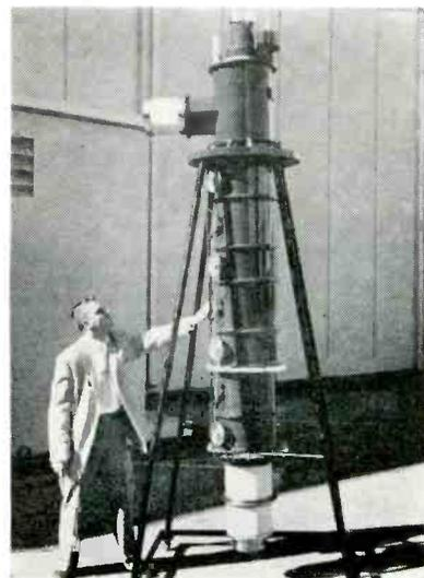
Varian Associates' VA-842 klystron is said to be the world's largest. It's 12-ft high; weighs 900 lb
