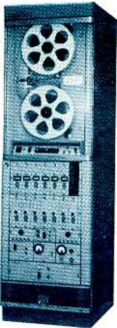
By providing a means of locally adjusting signal and bias levels, the meters are invaluable when setting up the 5-752 prior to a test run. On Analog record amplifiers, the units can be used to monitor bias signal level by means of a front panel selector switch.
