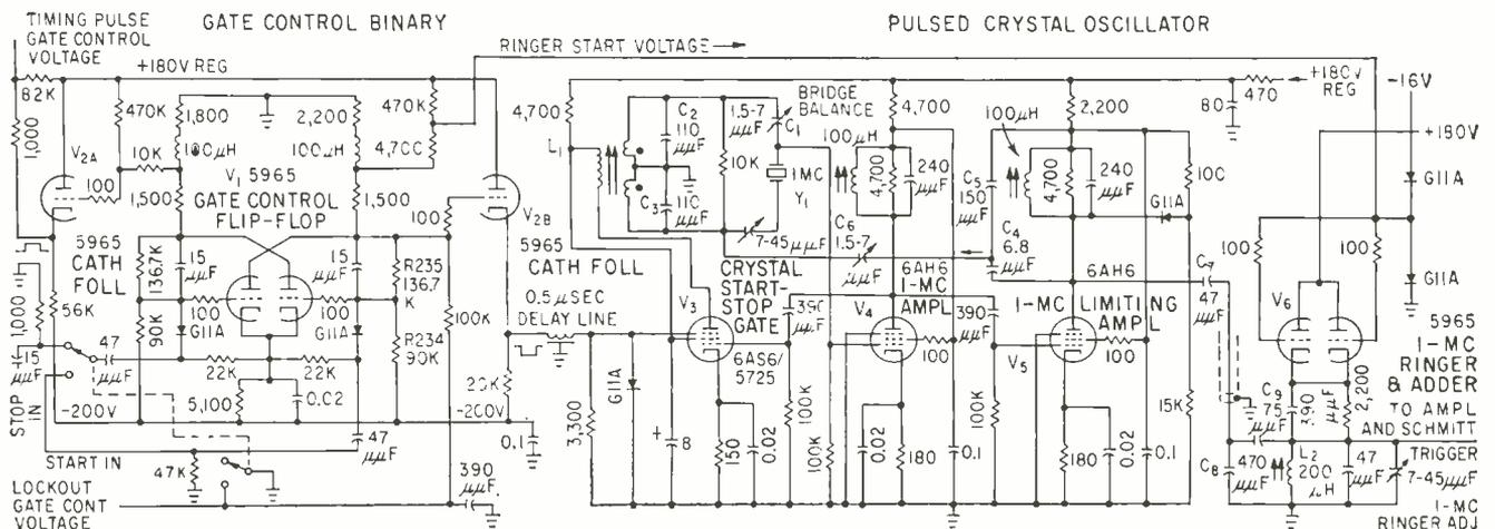
FIG. 2—Gate control flip-flop  $V_1$  gates the pulsed crystal oscillator on at  $T_0$  and off at the desired delay interval set by the digital counters timing circuit and controlled from the front panel
