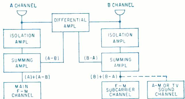
FIG. 2—Burden phantom carrier system as used with Halstead f-m multiplex plan
