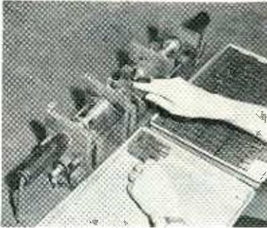
Operator places switch on mount between irons
