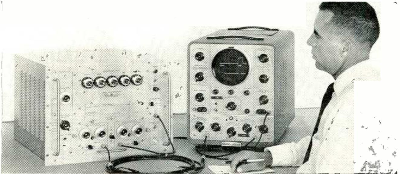
Precision delayed pulse generator with plug-in dual pulse generator unit shown in typical test setup
