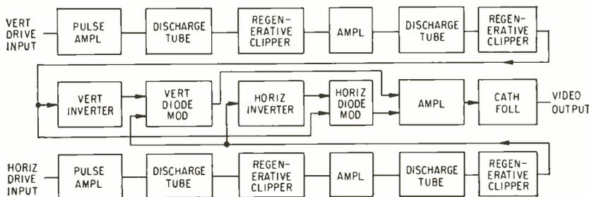
FIG. 1—Complete outline generator showing both horizontal and vertical channels
