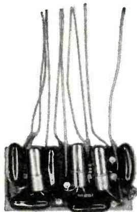
**TYPICAL MOLDED MODULE** used in Raytheon PCM equipment comprises logic circuitry required for a 2.3 mc shift register shown in the diagram. Other modules are used for repetitive and-or gates, flip-flops and binary-storage elements.
