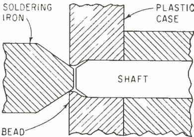
FIG. 1—Iron's heat forms plastic bead around shaped shaft end
