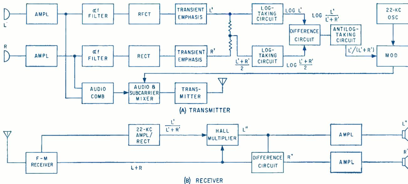
FIG. 5—Encoding (A) and decoding (B) equipment for Percival stereo system introduced by EMI of England
