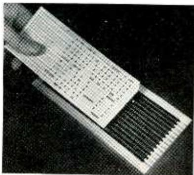
Photorectifier array ready to receive light mask behaves like complex diode array
