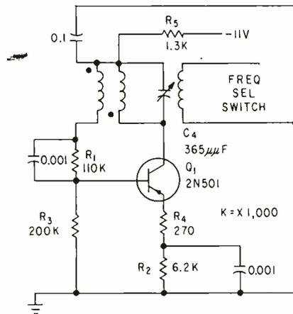
FIG. 2—Oscillator for h-f and l-f are identical with exception of coils used
