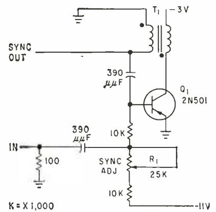
FIG. 7—Low-frequency sync blocking oscillator provides synchronizing signals for conventional oscilloscopes
