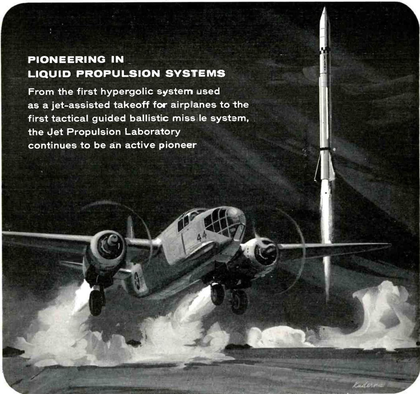
Months before Pearl Harbor, JPL had tested America's first liquid rocket engines using spontaneously igniting propellants. By April 1942, a simple nitric acid-aniline propulsion system was designed into and successfully tested in an A-20-A Bomber for a jet-assisted takeoff. For high-altitude atmosphere research purposes, JPL then used the hypergolic liquid rocket system in the WAC CORPORAL. Placed as a second stage on a V-2 rocket, this became the
