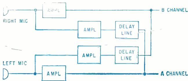
FIG. 4—Precedence-effect stereo arrangement recently demonstrated by Bell Telephone Laboratories
