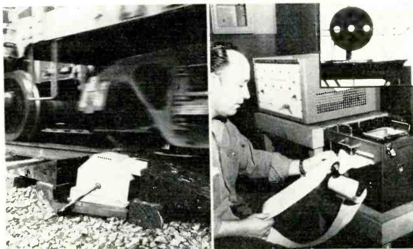
"Hot box" detector by Servo Corp. of America signals train to stop and makes a record
