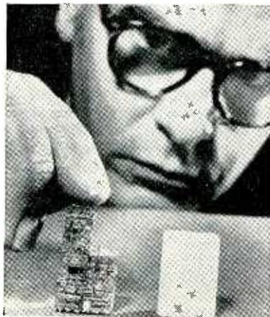
All the electronic parts of this military radio are no bigger than a sugar lump. Receiver is made of micromodules, circuit building blocks developed by Army Signal Research & Development Laboratory and RCA
