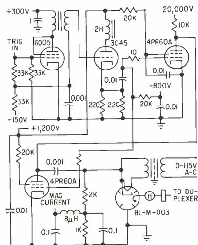
FIG. 2—Modulator supplies 0.02 $\mu$ sec pulses at a prf of 14,400 pps
