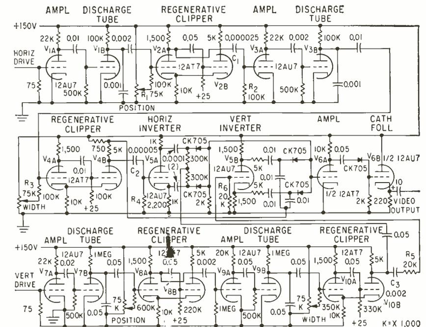
FIG. 2—Two pulse-forming channels are triggered by horizontal and vertical drive pulses. The outputs are mixed in diode modulators to produce the white outline signal
