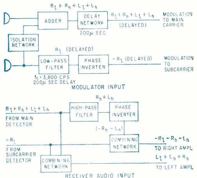
FIG. 3—Narrow-band stereo system for f-m proposed by Calbest
