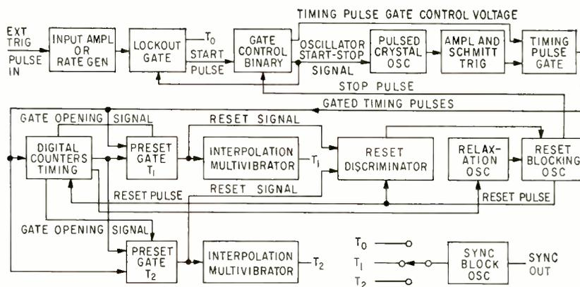
FIG. 1—Upon receiving a trigger pulse the unit generates a pulse at  $T_0$  and simultaneously starts two independent delay periods for  $T_1$  and  $T_2$ .
