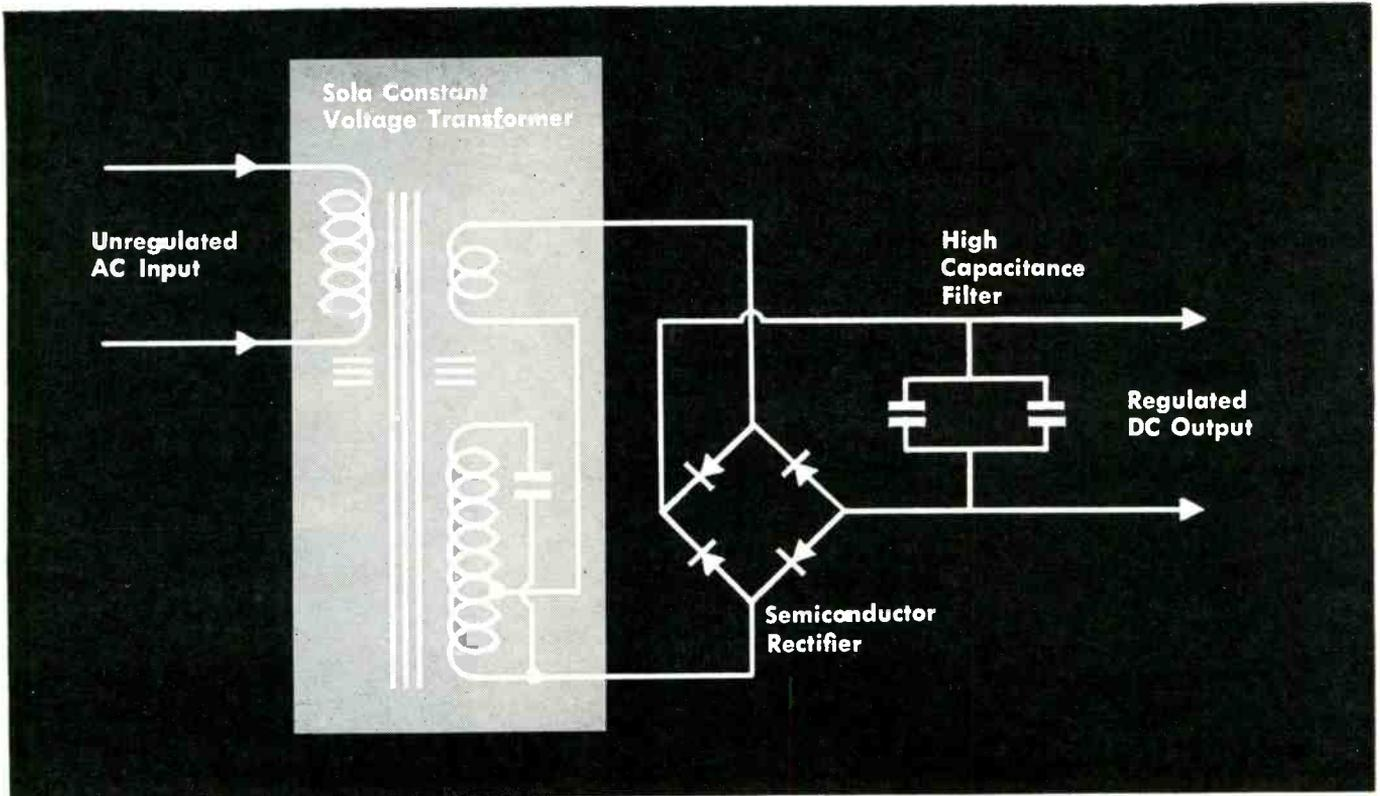
*Inherently simple design of the Sola Constant Voltage DC Power Supply is shown by this general schematic diagram. Its basic simplicity of design and its reliable components make this regulated power supply rugged and dependable, both electrically and mechanically.*
