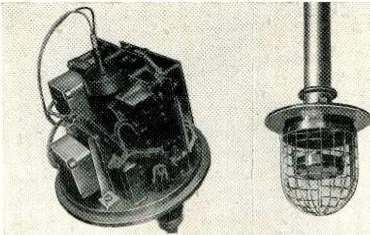
The left unit shows the servomotors that are contained in the upper part of the scanner. Unit at the right shows the lower part of the scanner which contains the transducer, inside of the wire net
