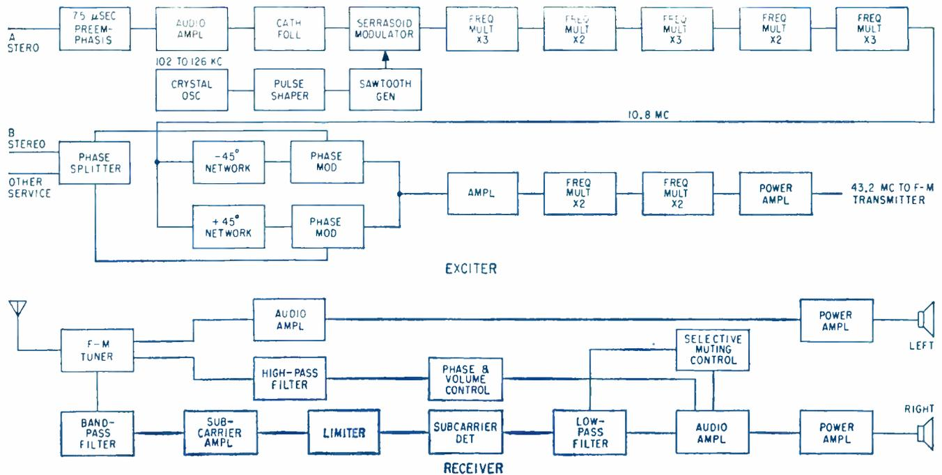
FIG. 6—Exciter and receiver used with Halstead f-m stereo system provide both stereo and private-wire service
