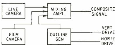
FIG. 3—Relationship of outline generator to typical video system
