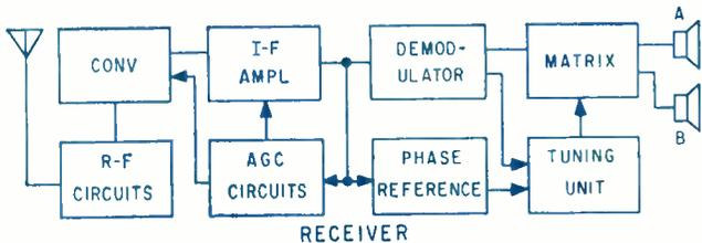
FIG. 8—Philco system for a-m stereo uses combined amplitude and phase modulation
