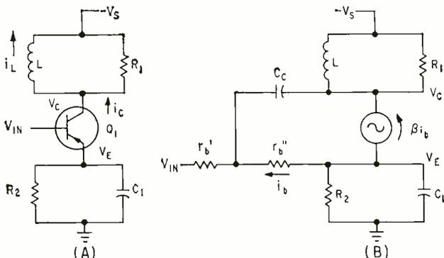
FIG. 3—Basic pulse circuit (A) and its simplified equivalent circuit (B)
