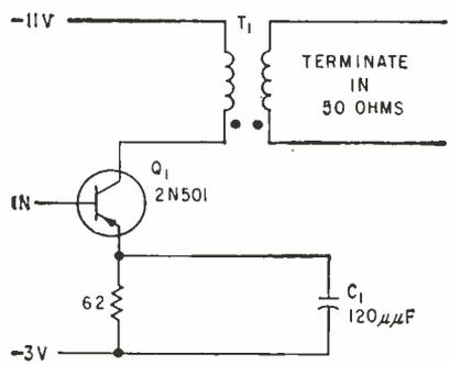
FIG. 6—Pulse amplifier uses circuit similar to last pulse former and shaper stage
