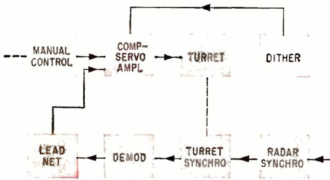
FIG. 1—Manual and radar inputs control operation of aided tracker's two channels. Only one channel is shown
