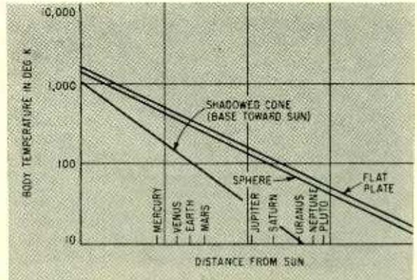
FIG. 1—Temperatures attained in space by black or gray bodies of various shapes
