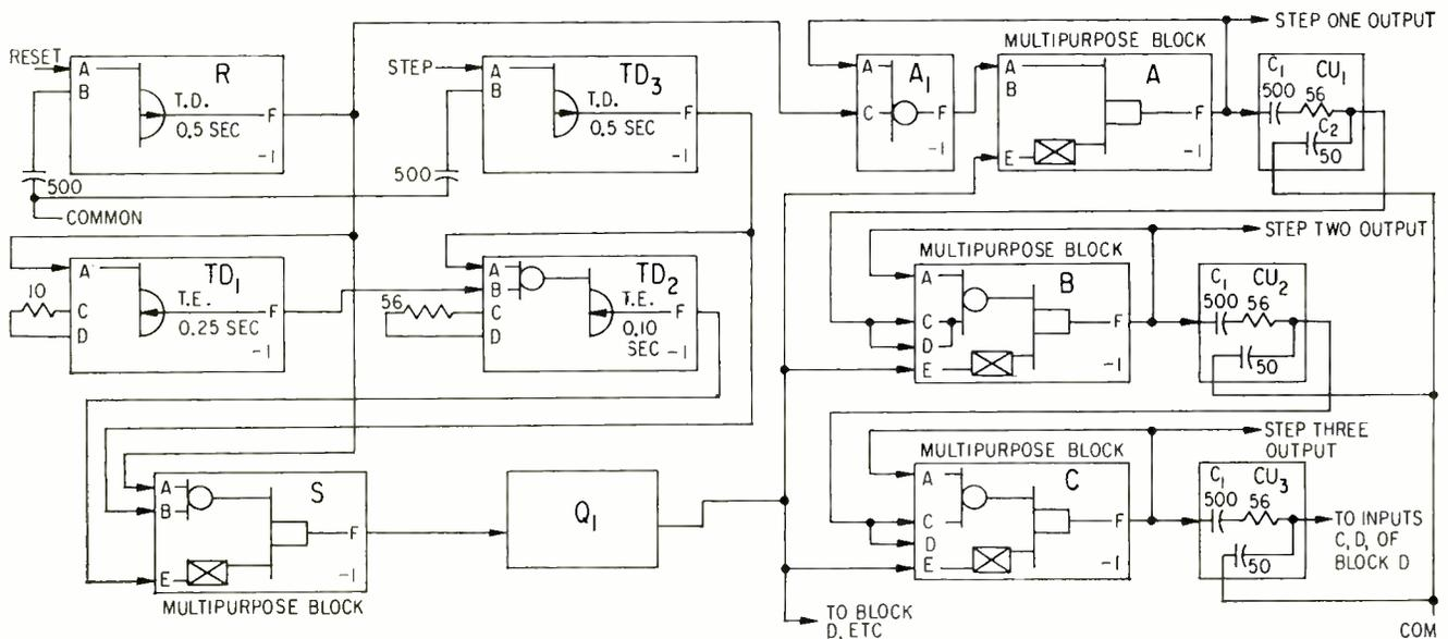
FIG. 7—Blocks *A*, *B* and *C* are switched on in sequence, in the manner of stepping-switch operation. As in previous diagrams, a number in the lower right-hand corner of a block indicates the bias of the block
