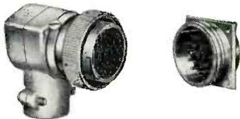
Standard K and RK...in straight and angle 90° plugs, wall mounting receptacles. Conduit and clamp entry types. 1 to 82 contacts in 213 different insert arrangements. 10-, 15-, 30-, 40-, 60-, 80-, 115-, and 200-amp. silver-plated brass contacts. High quality phenolic, melamine, and formica insulators. Cadmium-plated aluminum alloy shells. Flashover voltages: 1100 to 5000v 60cps ac rms.
