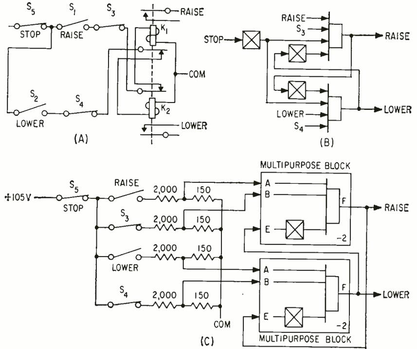
ments of the units determine their logic function. Block A is an AND gate because it requires a signal from terminal A and requires the absence of a signal from terminal E to produce a voltage at F.
