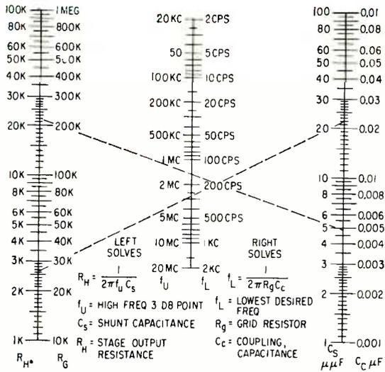
FIG. 3—Left sides of dual scales find stage output resistance. Right sides find interstage coupling capacitance
