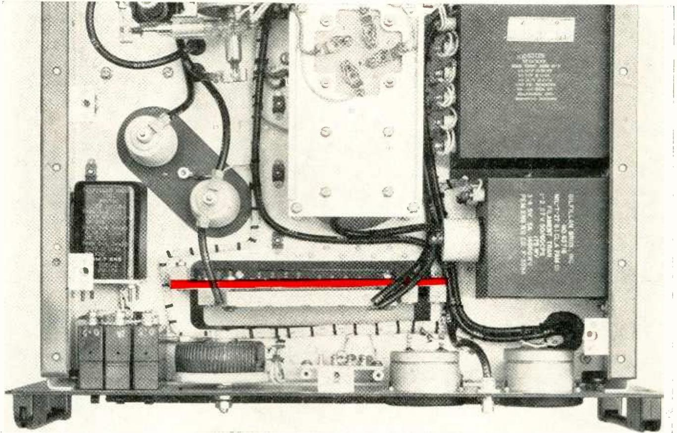
This AN/FPN-33 Quadraradar Transmitter of Gilfillan Bros., Inc., of Los Angeles, employs silicone-glass laminates to prevent recurrent arcing under high voltage and high humidity conditions. Gilfillan Bros. also use silicone laminates in their Ground Control Approach equipment.
