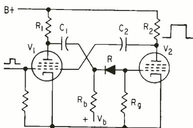
FIG. 1—Basic monostable multivibrator circuit using a nonlinear resistance
