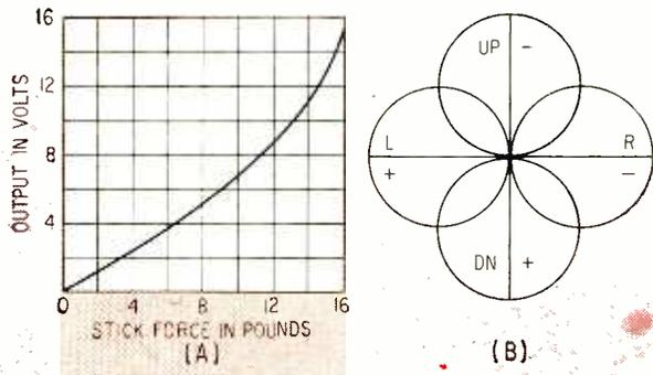
FIG. 3—The two manual control outputs are determined by the stick (A). Relative voltages produced when the stick is deflected by a constant force in a 360-deg arc (B)
