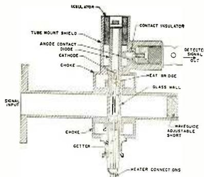
FIG 2—Crossguide diode and mount assembly
