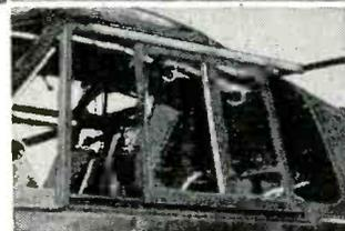
From the aluminum extrusions, to the stainless steel balls, the patented "ball retainer" the exclusive "Shok-Loks" and the precision assembling and fitting, Grant Slides are constructed with an absolute maximum of strength and serviceability. Pilot windows on the Sikorsky helicopters are mounted on Grant Slides — which operate continuously well under the most severe vibratory conditions.
