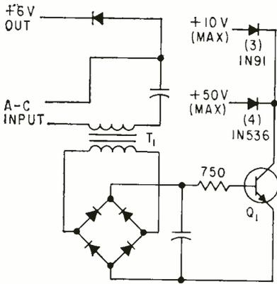
FIG. 3—Input to this switch is pulsating d-c whose average value is 6 v
