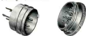
Hermetically sealed connectors... with steel shells, steel contacts, and Can-seal glass insulators, fused to shell and contacts. True hermetic sealing. Electro tin plating over cadmium plate over copper flash provides highly receptive surface for soldering and corrosion resistance.
