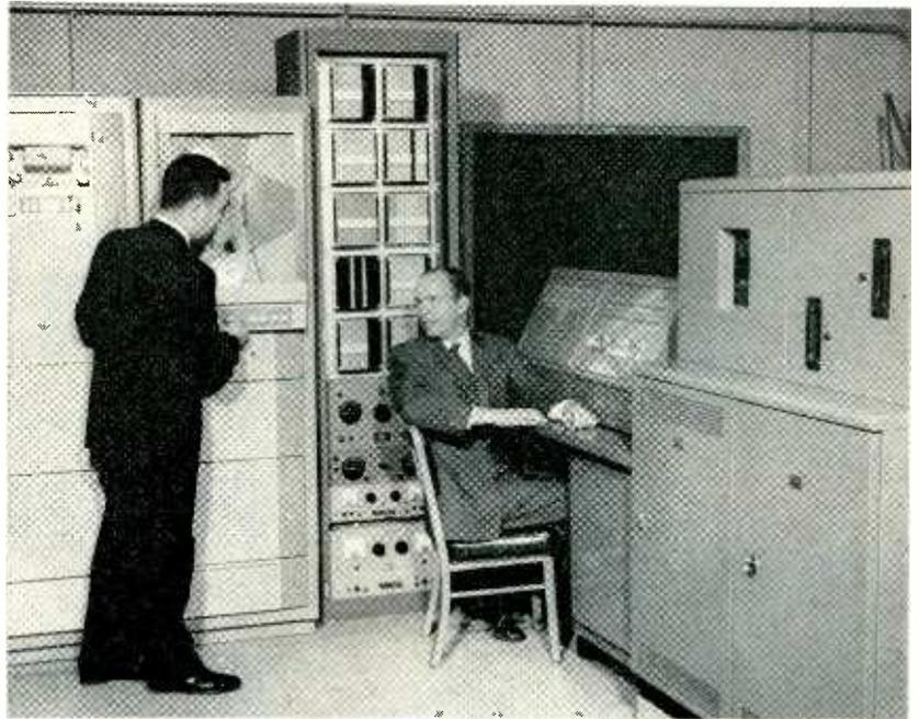
Scanner for evaluating pattern-recognition systems includes program tape machine at left, logic unit, and at right of console, flying-spot light source and pickup unit
