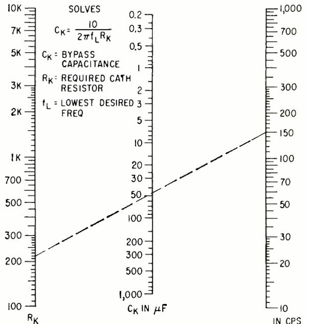
FIG. 6—Cathode bypass nomogram finds value of cathode bypass capacitance when cathode resistor and lowest frequency of interest are known
