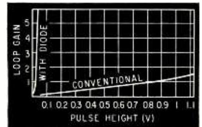
FIG. 2—Loop gain plotted as a function of input signal amplitude for conventional and modified multivibrator
