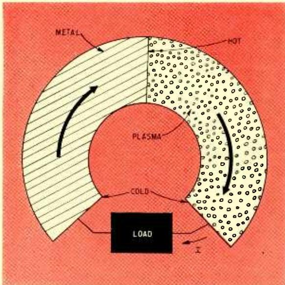
FIG. 16—Basic plasma-metallic thermocouple
