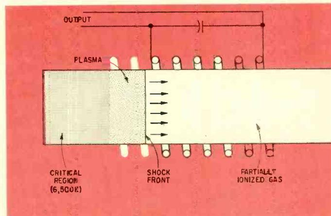
FIG. 15—Plasma-fission reactor would produce electricity directly
