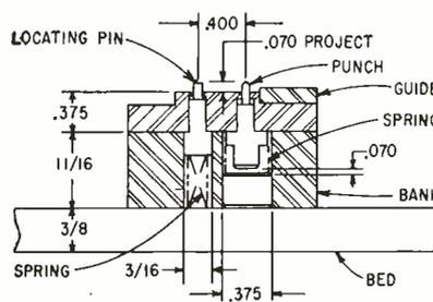
FIG. 2—Lower mechanism in loading position
