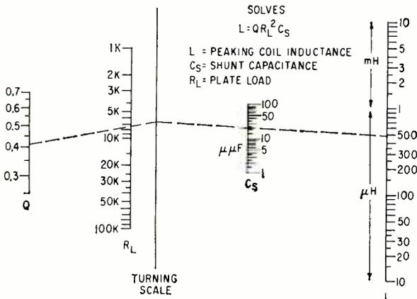
FIG. 5—Peaking coil nomogram finds value of inductance required when  $Q$ ,  $R_L$  and total shunt capacitance are known
