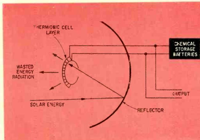
FIG. 14—Basic arrangement for thermionic-converter system
