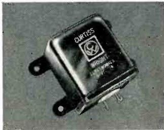
Curtiss-Wright "IR" thermal time delay relays reset the instant that they are de-energized. Variations from 22 to 32 volts will not affect the time delay specified.
