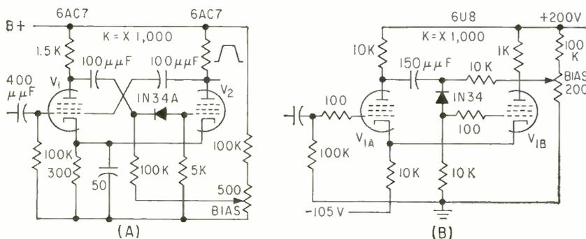
FIG. 4—Examples of sensitive multivibrator design: (A) satisfies stability criterion; (B) is a cathode-coupled version of circuit
