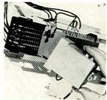
Inserting a multipurpose block in mounting bus
