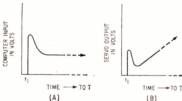
FIG. 4—Output obtained for a typical input voltage (A). During the first portion of the time constant of the computer, the output rate (B) is proportional to voltage input and stick displacement
