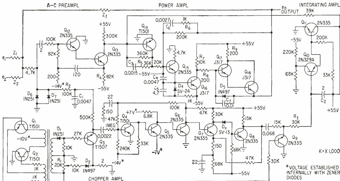
FIG. 1—Schematic of the operational amplifier. Drift compensation achieves accuracy of 0.005 percent or less in analog computers
