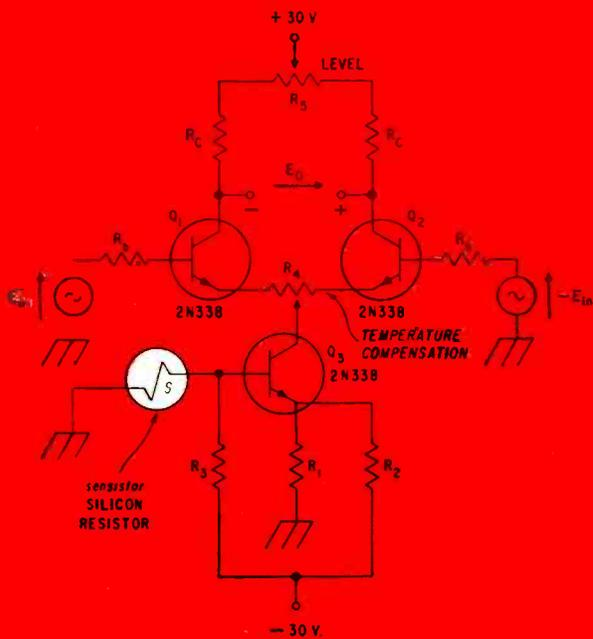
**DIFFERENTIAL DC AMPLIFIER USING SENSISTOR SILICON RESISTOR.**
