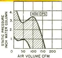
For airborne and missile cooling applications, the AXIMAX-3 when turning at 20,000 rpm will deliver 165 cfm at free delivery. This performance is possible although the fan is only 2.8" in diameter, 2.3" in length and weighs a mere 14 ounces.
