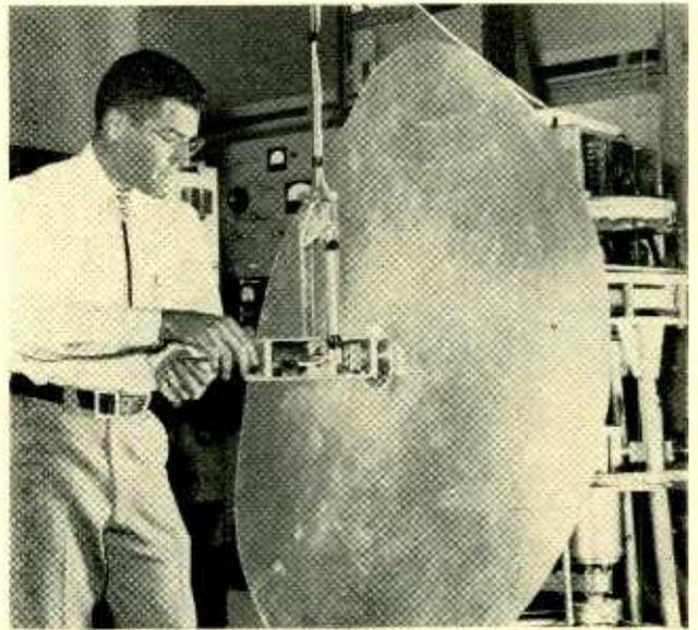
Scientist in charge of Los Alamos Laboratory's solar sail development adjusts counterweights on miniature dynamic mockup. Electric motor spins plastic sheet flat by centrifugal force
