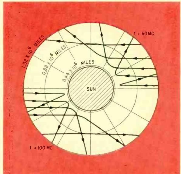
FIG. 8—Ionized field in Sun's vicinity refracts communication paths in its near vicinity
