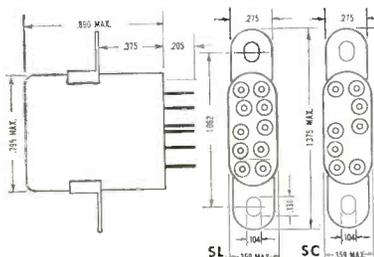
**SL**—dual coil latching relay. Operates on a 1 watt, 3 ms. pulse at nominal voltage. Permanent magnet latch locks the armature in either position.
