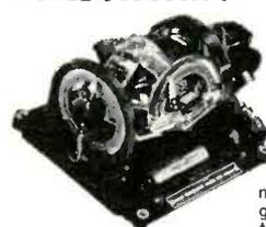
115 volts, 400 cycles, single phase, 35 watts. Pitch and roll potentiometer pickoffs 890 ohms, 40 volts max. AC or DC. Speed 20,000 rpm, ang. momentum 12,500,000 gm-cm<sup>2</sup>/sec. Erection system 27 VAC, 1/2". Weight 5.5 lbs. Price \$35.00 each
