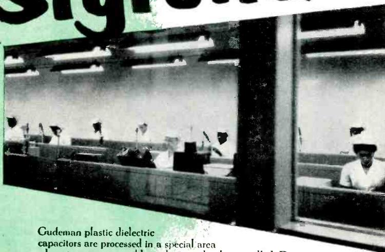
Gudeman plastic dielectric capacitors are processed in a special area where temperature and humidity are closely controlled. Dust and other contaminants are filtered out, and as an extra precaution, operators wear nylon caps, smocks, and gloves. Operators like Styroflex because it winds easily. Quality control inspectors like it because the capacitors test out "on the nose" with a minimum of rejects.
