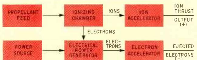
FIG. 3—Basic components of ion-drive propulsion system
