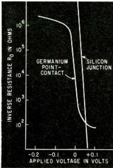
FIG. 3—Typical curves of average diode resistance as a function of applied voltage
