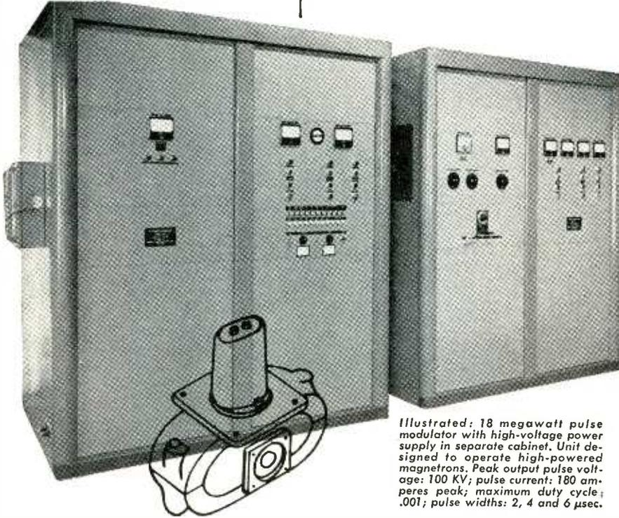
Illustrated: 18 megawatt pulse modulator with high-voltage power supply in separate cabinet. Unit designed to operate high-powered magnetrons. Peak output pulse voltage: 100 KV; pulse current: 180 amperes peak; maximum duty cycle: .001; pulse widths: 2, 4 and 6  $\mu$ sec.
