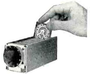
Switches are available in sizes approx. 2" x 2", 3" x 3" and 4" x 4" with lengths to accommodate up to 36 wafers. Virtually unlimited choice of switch circuit configurations. All connections are to a single bank of receptacles and are conveniently accessible from one side of the aluminum housing. Contacts are silver, gold or rhodium plated on a copper base. Wafers can be made to include printed circuitry and components in addition to their normal switching function.
