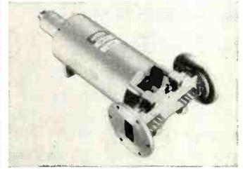
power levels results in small-signal gain of up to 35 db. To simplify replacement, the tube plugs into a waveguide coupler package which accommodates UG 344/U waveguide-type flanges. When used with coaxial output coupler, tube covers 4,000 to 8,000 Mc range.
