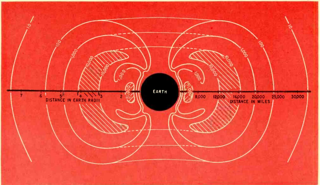
FIG. 2—Radiation in Earth's vicinity is in form of two concentric doughnut-shaped belts; contour lines of this cross-sectional representation indicate particle counts per second. Outer belt is believed to be caused by spurts of gas from Sun
