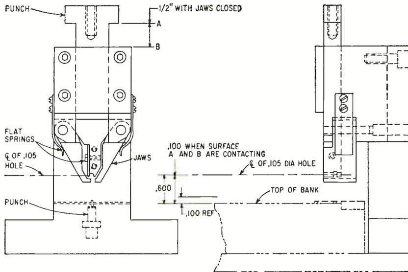
FIG. 1—Front and side views of upper punch mechanism in loading position
