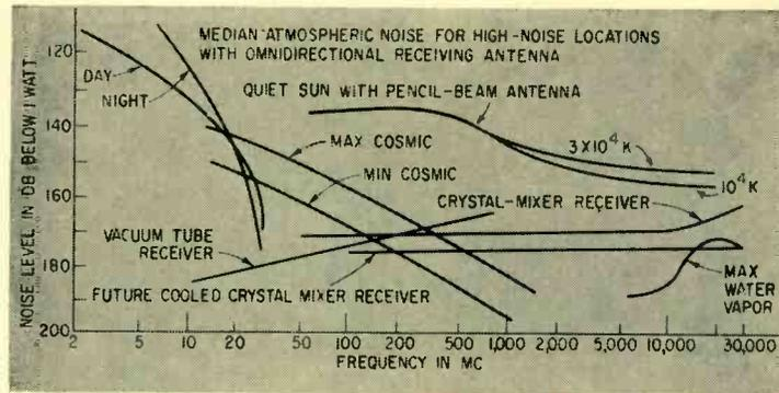
FIG. 7—Overall limitations on receiver sensitivity due to various cosmic, atmospheric and receiver noise sources
