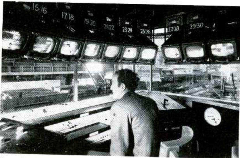
A complex, 15-camera closed-circuit tv installation helps speed output at Steel Company of Wales, Port Talbot, Wales. Marconi's Wireless Telegraph Co. Ltd. placed cameras in a line on one of rolling mill's outside walls. Operator gets composite view of 700 ft of track, far end of which is 1,000 ft away
