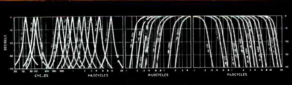
This standardized group of filters covers most popular filter applications and frequencies. Units are in compact, drawn, magnetic shielding cases... 1 1/16 x 1 1/16 base, 1 3/8 high for BMI, LMI, BML; others 2 1/2 high. There are six basic types:
