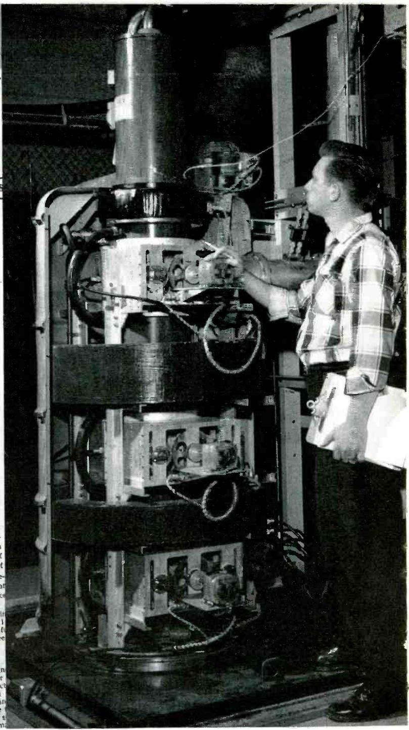
Eimac Klystron final amplifier at Millstone Hill Radar site.
