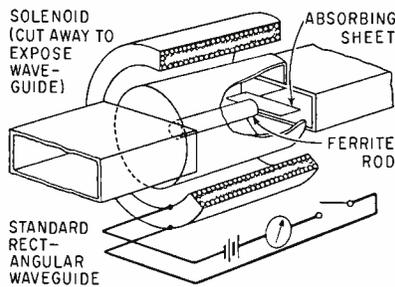
FIG. 2—Simplified Faraday rotation switch. Solenoid supplies d-c magnetic field to produce 90 deg. of rotation. Sheet of absorbing material suppresses the reflections
