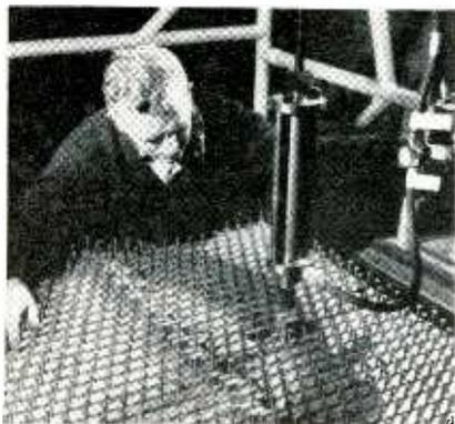
Plastic silver-coated lens developed by Sperry Gyroscope Co. for the Talos missile guidance radar is composed of 4100 cells. The lens is molded of plastic-impregnated fiber glass and coated with silver to make it electrically conductive. Aluminum cores forming the grid structure are molded into lens and then removed with a pneumatic ram
