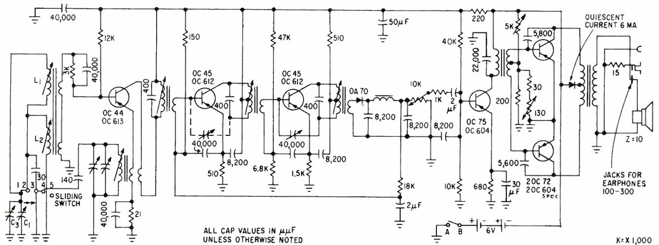
FIG. 5—Combined broadcast and long-wave receiver, developed by Braun GmbH. Sliding contacts are used for switching bands
