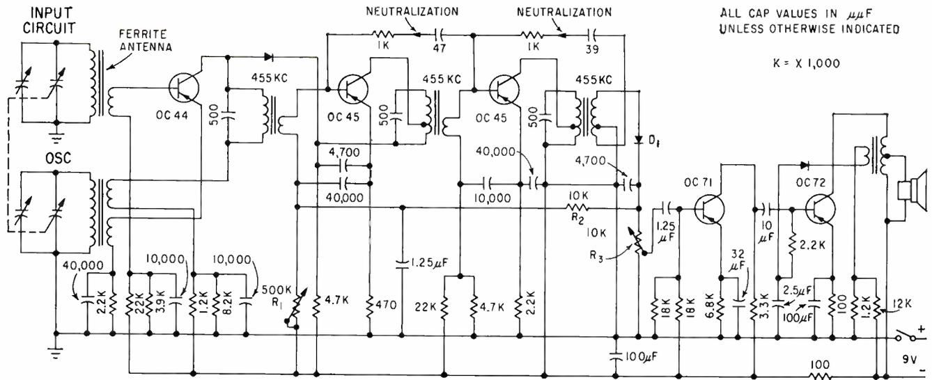
FIG. 4—Typical European broadcast-band receiver, the Peggie portable of Akkord AG
