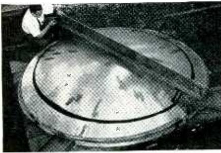
Paraboloid face mold with plastic-topped female templates
