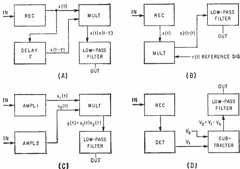
FIG. 1—Autocorrelator (A) is used in a superheterodyne. Crosscorrelator (B) is a synchronous detector using reference signal resembling expected signal. Two-receiver radiometer (C) detects aperiodic signals. Subtraction-type radiometer (D) subtracts stored noise signal from expected signal plus noise
