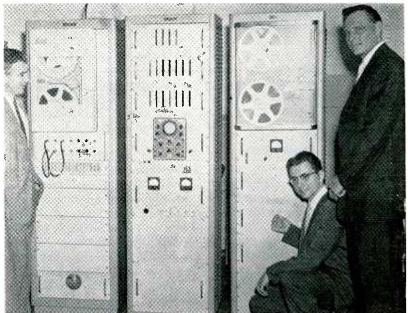
Automatic Doppler cycle counter produces magnetic tape which is fed to digital computer for processing
