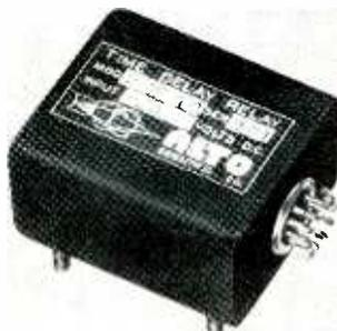
overall standard accuracy of  $\pm 5$  percent. The instrument's time delay is 0.05 sec to 60 sec, preset at the factory. Ambient temperature (operating) range is from -55 C to 71 C. Input voltage is 24 to 32 v d-c, and current drain is 50 ma at 28 v. **Circle 204 on Reader Service Card.**
