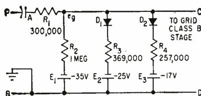
FIG. 1—Basic network used in compensator. Two are needed in amplifier
