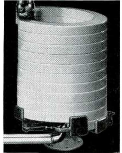
For carrying cooling water which must undergo a change in potential, use of Lapp porcelain eliminates trouble arising from water contamination and conductivity, sludging and electrolytic attack of fittings. Permanent cleanness and high resistance of cooling water is assured with the completely vitrified, non-absorbent Lapp porcelain.
