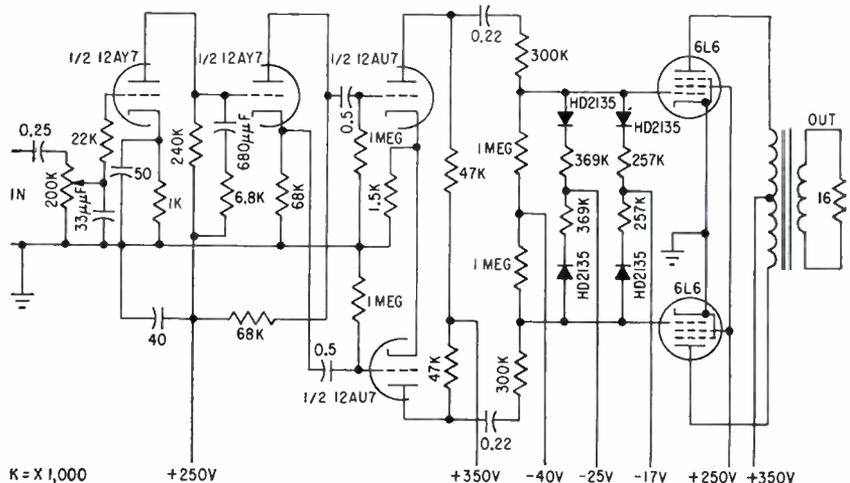
FIG. 4—Compensated amplifier delivers 16 w with 2.6 percent total distortion at 47.6-percent efficiency
