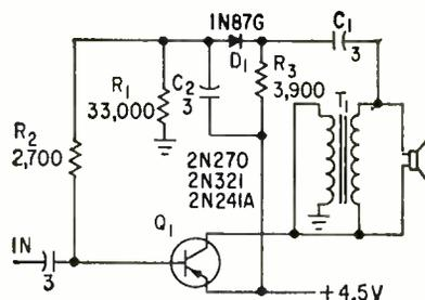
FIG. 2—Sliding class-A output has one transistor and no input transformer
