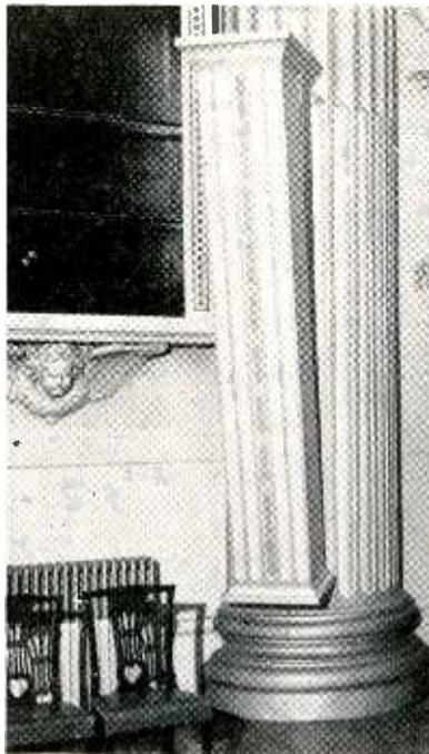
Column loudspeaker designed to blend into design of surrounding area
