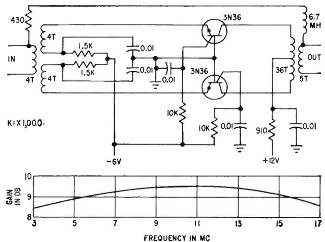
FIG. 7—Receiving amplifier and response
