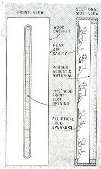
FIG. 2—A typical slotted column loudspeaker showing construction details
