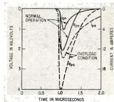
FIG. 3—Voltage and current relationships across clipper diodes
