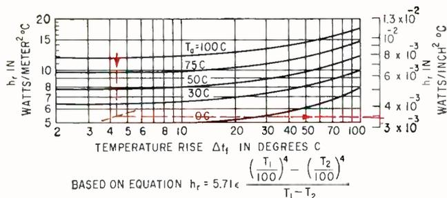
FIG. 5—Radiation heat transfer coefficient ( $h_r$ ) for unobstructed radiation and an emissivity of 1
