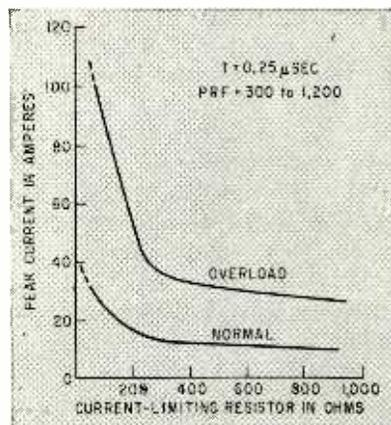
FIG. 9—Effect on diode peak current of varying value of current-limiting resistor
