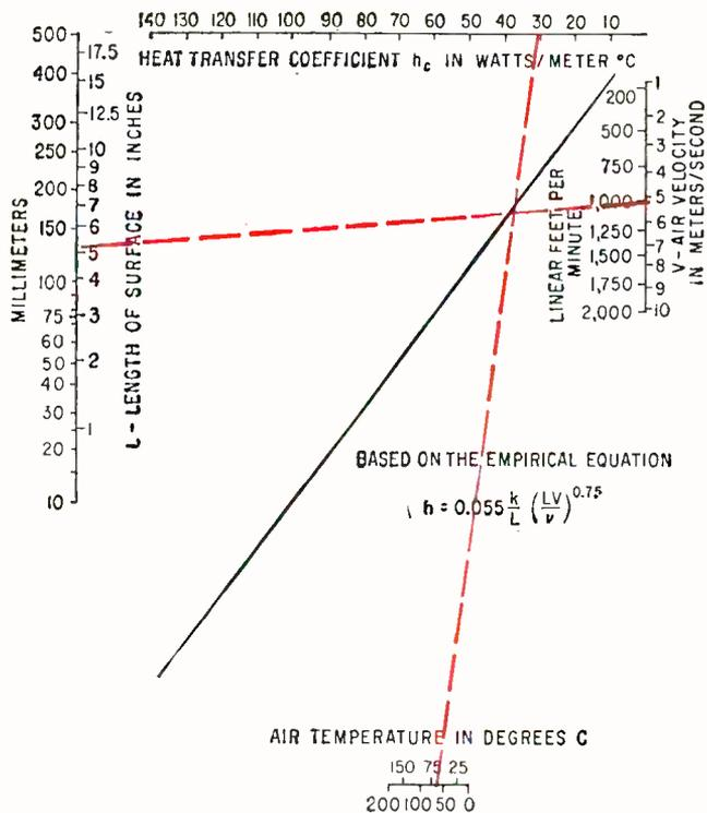
FIG. 4—Nomogram for obtaining heat transfer coefficient for forced convection cooling of plane surfaces in air at sea level with turbulent flow. Dashed lines show sample solution
