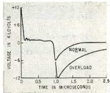
FIG. 2—Thyratron plate voltage
