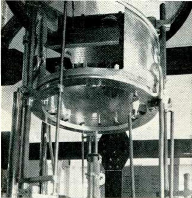
View of bell jar setup, looking up through ring source to mask
