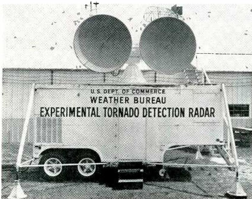
Weather Bureau at Wichita Falls, Texas, tests experimental Doppler radar by Radiation, Inc. Project, in existence for three years, detected a tornado 23 miles away last year. Modifications are being made to increase receiver sensitivity and reduce transmitter noise
