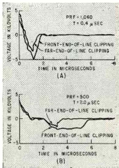
FIG. 8—Inverse voltage at pulse-forming network for 0.4- $\mu$ sec network (A) and 2- $\mu$ sec network (B)
