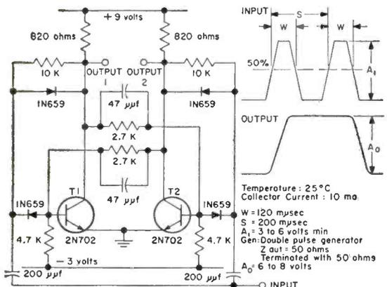
TYPICAL CIRCUITRY FOR OBTAINING 5-MC REP RATE
