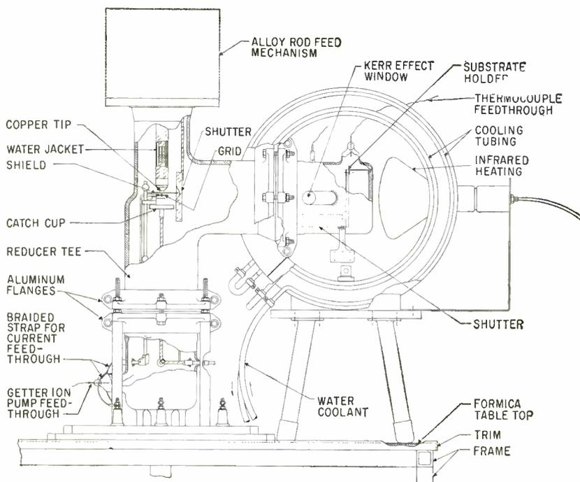
FIG. 2—Arrangement of principal parts of electron bombardment vacuum evaporator
