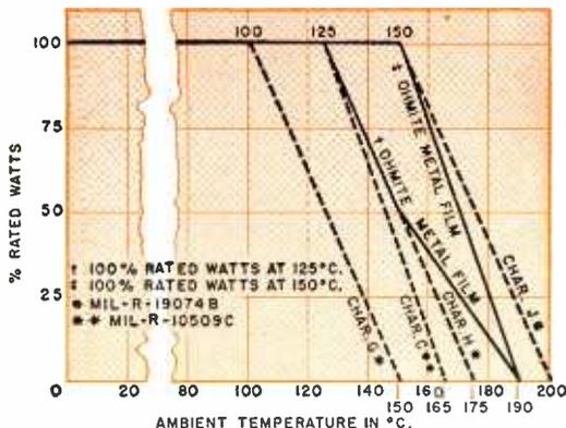
Watt rating chart. These curves indicate percentage of rated wattage that can be applied at temperatures higher than 125°C and 150°C. However, at no time shall the applied voltage exceed the maximum for each style.
