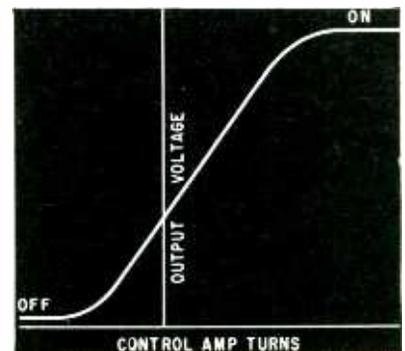
FIG. 3—Transfer characteristic of power-unit magnetic amplifier
