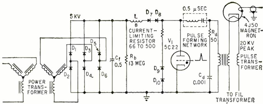
FIG. 1—Radar modulator uses ten silicon diodes to replace five vacuum tubes
