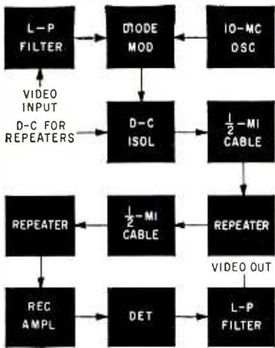
FIG. 1—Basic transmission system
