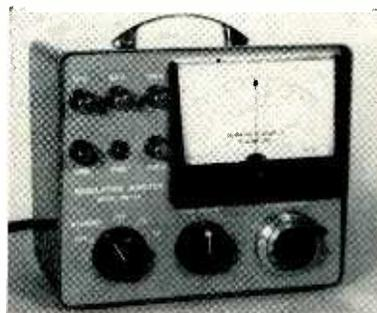
ation and is calibrated at the factory. Drift is less than 0.005 percent for an 8 hr day and short term drift is less than 0.002 percent. At maximum sensitivity the meter gives full scale deflection for a deviation of  $\pm 0.1$  percent.
