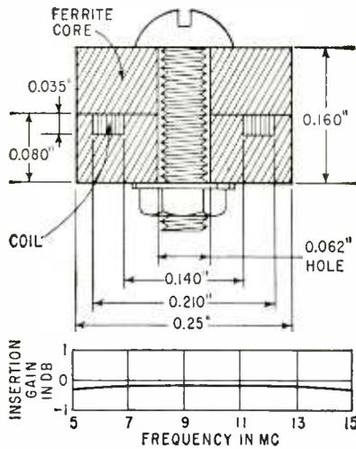
FIG. 2—Transformer and response
