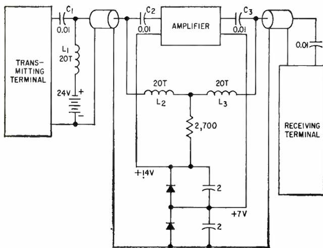
FIG. 6—Repeater d-c power supply
