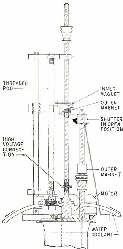
FIG. 4—Alloy feed rod mechanism
