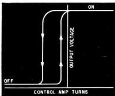
FIG. 4—Transfer characteristic of hold-unit magnetic amplifier
