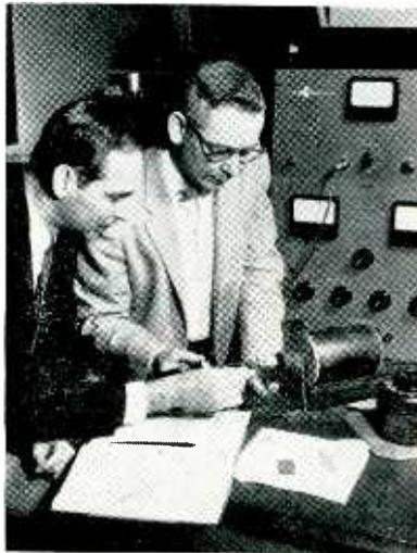
A strip of metal, coated with a fluoride film, is inspected by S. S. Flaschen (left) and P. D. Garn of Bell Labs, who developed an insulating technique that may solve problems in space electronics.
