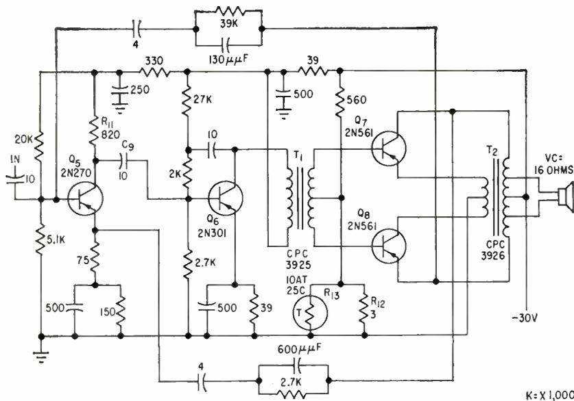
FIG. 2--Power amplifier uses balanced negative feedback and operates class-B. Output stage has emitter degeneration as further improvement
