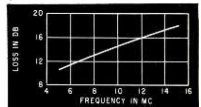
FIG. 4—Transmission characteristic of 0.5-mi cable
