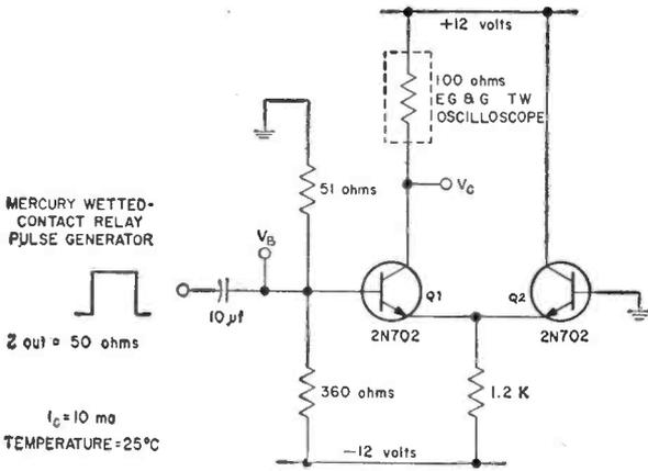
TYPICAL NON-SATURATED LOGIC SWITCHING CIRCUIT
