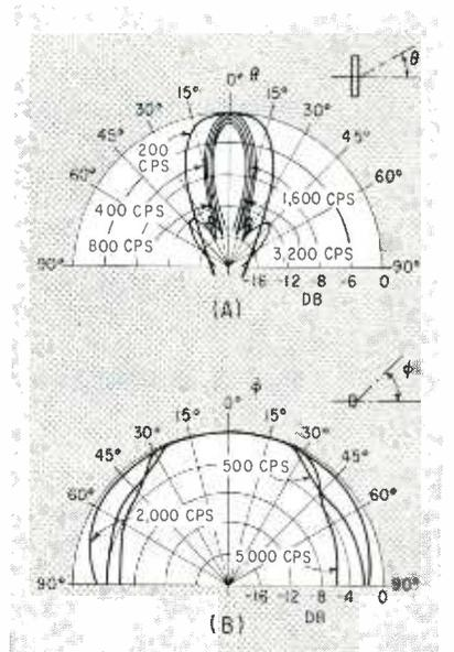
FIG. 4—Polar responses of a typical column loudspeaker in the vertical plane (A), and in the horizontal plane (B)
