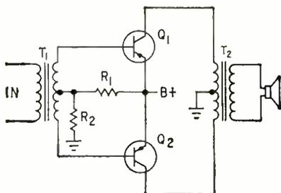
FIG. 1—Conventional push-pull class-B output uses two transistors
