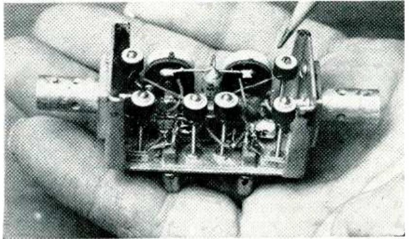
Closeup of terminal repeater amplifier shows ferrite core transformers
