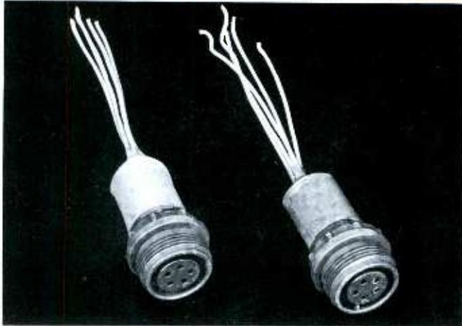
**POTTED CONNECTIONS** subjected to pressure tests clearly show the superiority of wires which have undergone bonding treatment (see results of tests in table below).
