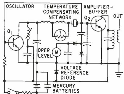
FIG. 1—Portable frequency standard provides accuracy of one part/million and can operate at frequencies from 5 to 50 mc
