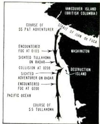
Misreading radar data resulted in collision of cargoship P & T Adventurer with tanker Tullahoma in August 1951. In this typical case, both vessels were attempting to open up distance between them, actually closed on collision course
