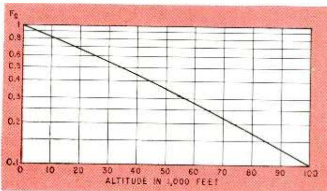
FIG. 3—Altitude correction factor ( $F_a$ ) for convective heat transfer coefficient
