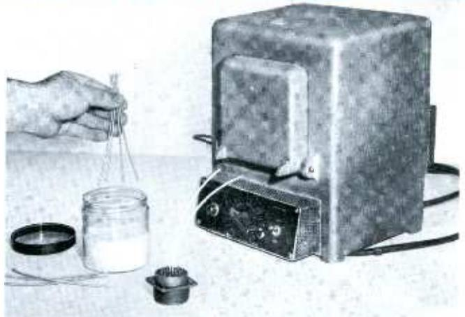
**PRIMER** is applied to unstripped wire ends preparatory to sintering of coating onto the surface of insulation of TEFLON TFE-fluorocarbon resins.
