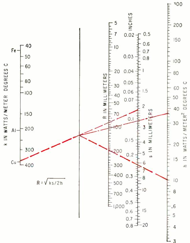
FIG. 9—Nomogram for obtaining fin thickness
