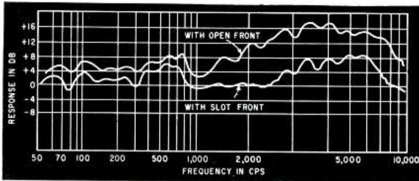
FIG. 1—Frequency response of a moving coil 10-in. cone loudspeaker with conventional open front and with 1½-in. wide slotted front
