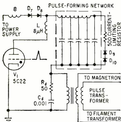
FIG. 7—Clipper is shown in optimum location at far end of line
