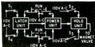
FIG. 2—When *run* pushbuttons are depressed, power unit energizes magnetic valve. Hold unit takes over from power unit later on
