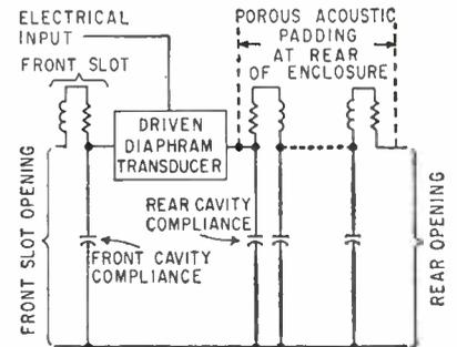
FIG. 3—Approximate electrical analogy circuit representing phase shift of elements of a slotted column loudspeaker at low frequencies
