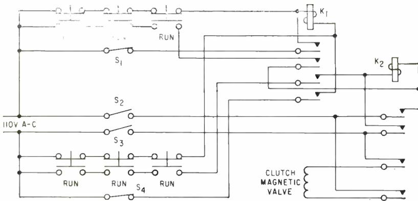
FIG. 1—Relay-circuit start conditions shown assume that 110 v is not present
