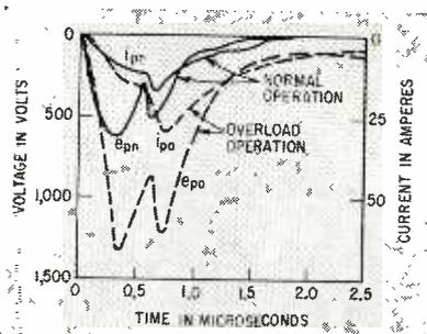
FIG. 4—Voltage and current with inductance in thyatron plate circuit
