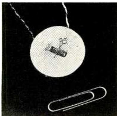
DEVELOPED FOR THE U. S. NAVY Bureau of Ships by Armour Research Foundation, compact magnetic field detector uses a Hall-effect probe as the basic pickup. The probe is made of indium antimonide and is responsive directly to the magnetic field rather than to its time rate of change as in a conventional loop pickup.
