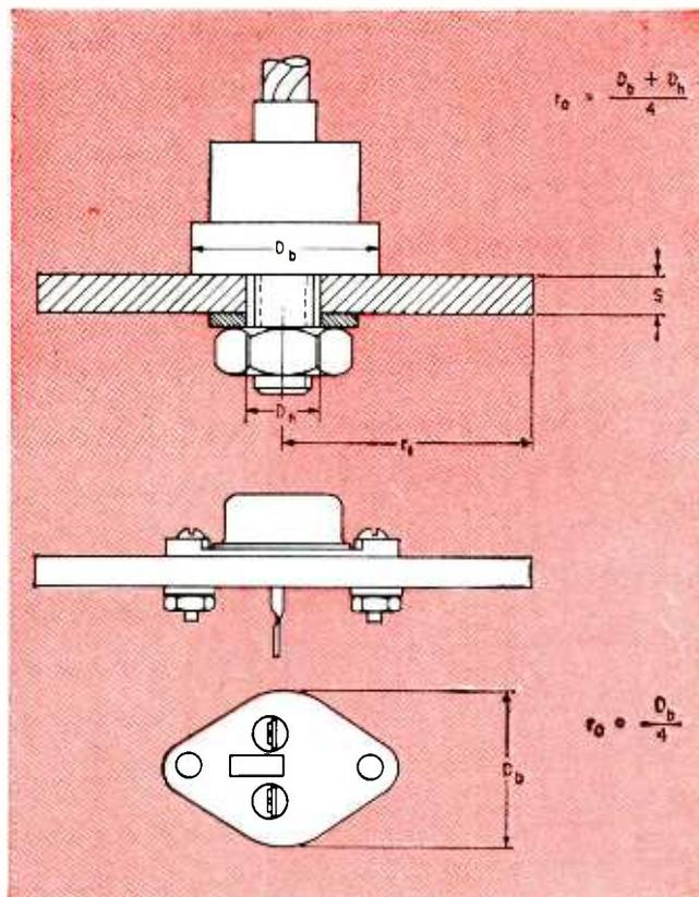
FIG. 7—Relation of device dimensions to heat input radius
