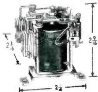
**LM SERIES:** Plate circuit relays similar to the MR. All sp and dp contact arrangements shown above are available. Coils are wound to specified resistances up to 58,000 ohms max. Sensitivity ranges from 15 mw min. (single pole) to 70 mw min. (double pole).
