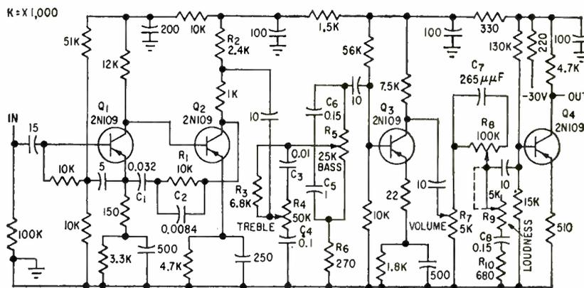
FIG. 1—Preamplifier accepts variable reluctance cartridge signal and contains bass, treble, volume and loudness controls. Four alloy junction transistors are used
