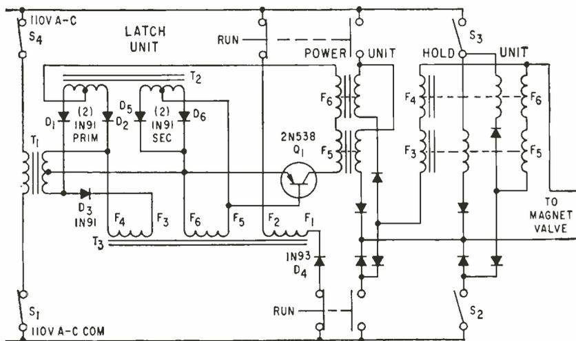
FIG. 5—Bias connections of static switching control are not shown. Control switches are in positions they occupy before start of cycle. Operators begin cycle by depressing both *run* pushbuttons
