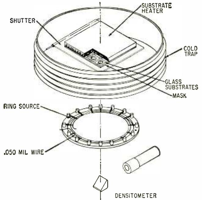
FIG. 1—Isometric view of experimental setup employing ring source
