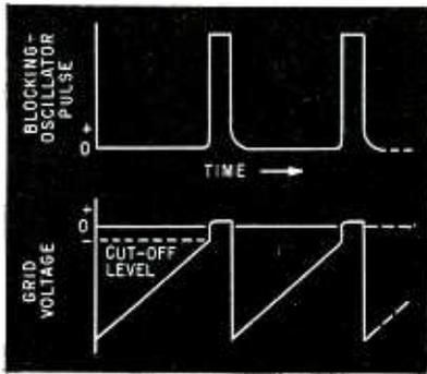
FIG. 3—Blocking-oscillator pulses and grid voltage are shown on a common time scale
