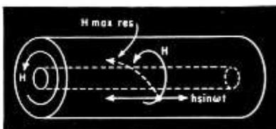
FIG. 3—Method of inducing torsional vibrations
