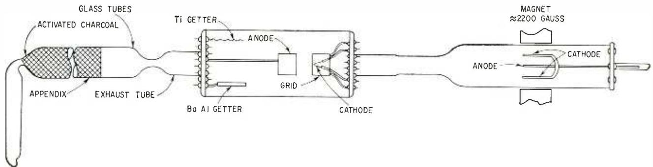
FIG. 1—Prototype vacuum tube uses adsorption principle for exhausting
