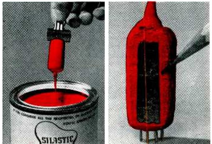
Electronic tube encapsulated with Silastic.
