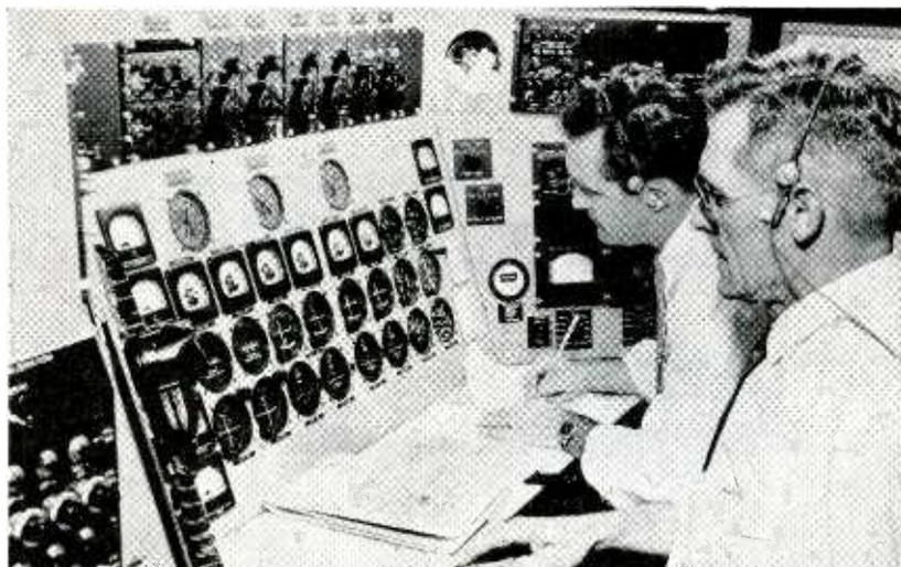
Federal Aviation Agency technicians check out new direction-finding gear made by Topp Industries to work into VOR (vhf omnirange) system. Topp gear reduces angular tolerance of VOR measurement to half a degree; present systems vary as much as 5.4 deg
