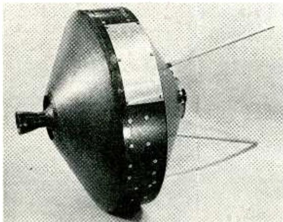
Pioneer lunar probe vehicle. Retro rocket to place the vehicle in lunar orbit protrudes from shell. Antenna is at rear
