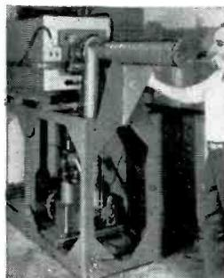
Two-zone 5" diameter muffle vacuum heat treating furnace. For annealing semiconductors and electronic parts.
