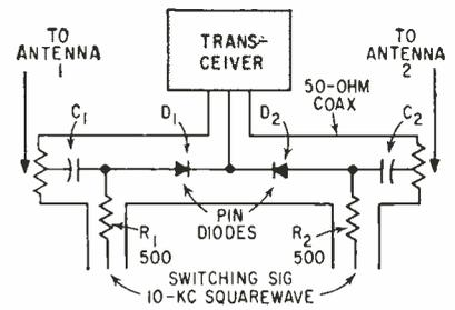
FIG. 1—Antenna switching system, using Sarkes Tarzian M-600 silicon diodes in coaxial cables
