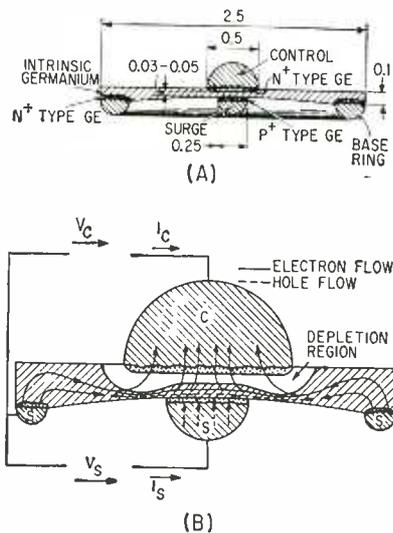
FIG. 1—Cross section of Deplistor (A) gives the dimensions in mm. The current-flow pattern in the on condition is shown in (B)
