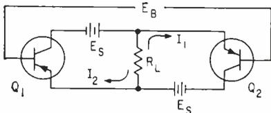
FIG. 1—Emitter currents in basic diagonally symmetrical circuit flow in opposite directions through load
