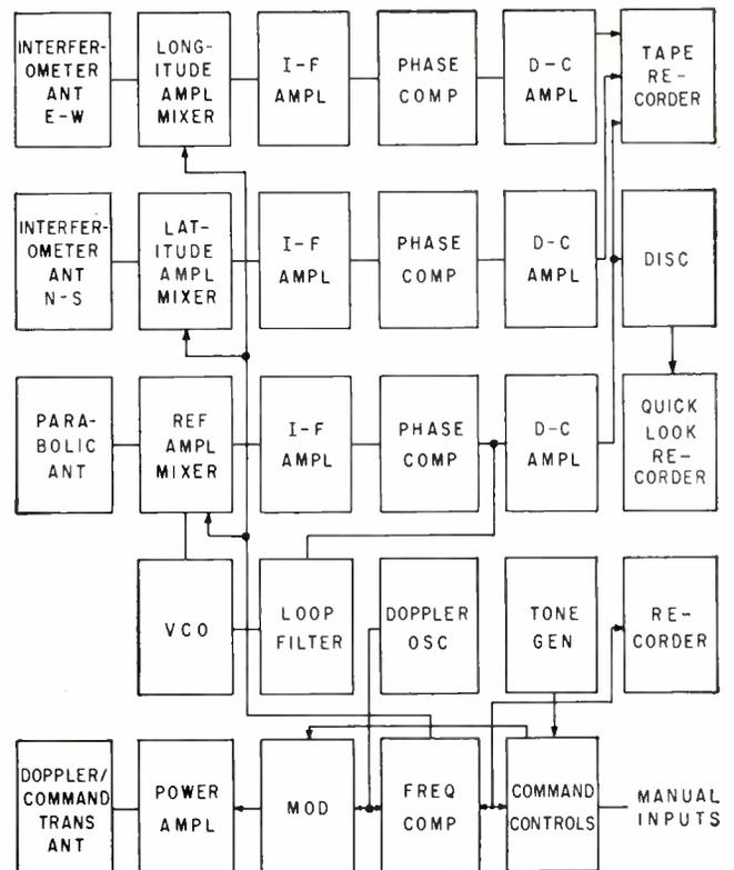
FIG. 4—Main elements of the Hawaii tracking station showing the microlock receiving system and the command transmitter
