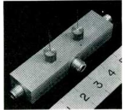
Model of diode switch was developed by the Communications Laboratory of the McDonnell Aircraft Corp.
