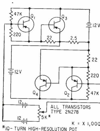
FIG. 2—Automotive storage batteries are used for 12-v transistor supplies in practical circuit although rectifier supplies could be used. Maximum current drain from two 12-v dry cells in control voltage circuit is 7 ma
