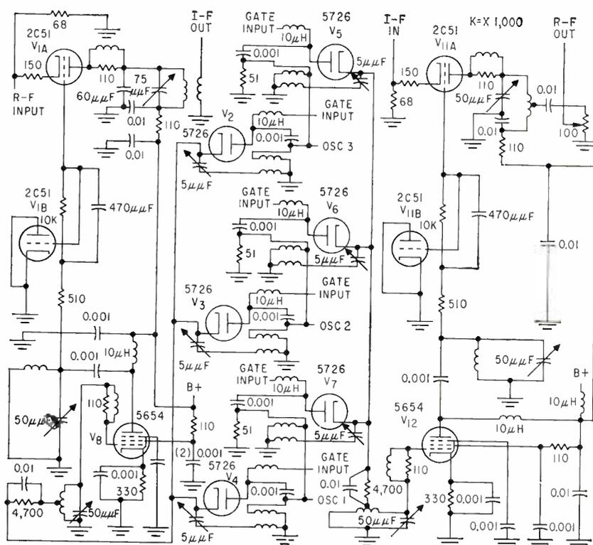
FIG. 6—First mixer, gates and second mixer of transmitter. Output of first mixer passes through two i-f amplifiers, which are not shown, before entering the second mixer
