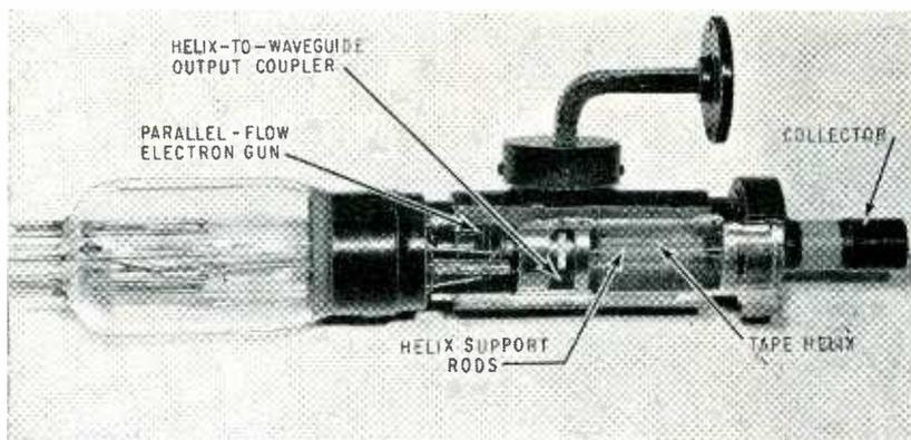
Cut-away section exposes electron gun, r-f output coupler and helix of millimeter oscillator
