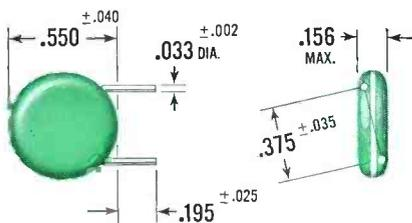
Allen-Bradley Type A capacitors are available in the most frequently used types and capacitance values.
