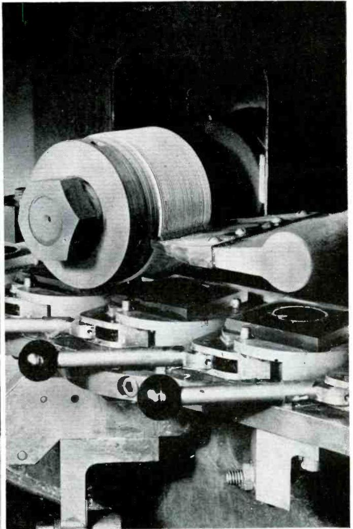
Slicing and dicing operations are both performed by Norton diamond cut-off wheels. An ingot of pure silicon, cemented to a ceramic block is sliced by a single wheel. In dicing, wafers are also mounted on ceramic blocks. Ganged wheels first cut in one direction; then the blocks supporting
