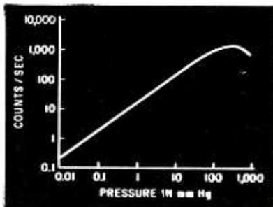
FIG. 4—Reversal of near-atmospheric pressures is due to ion recombinations
