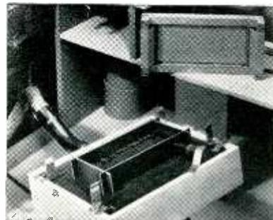
Vibration-vacuum fixture to align cores. Tape transfer fixture is above
