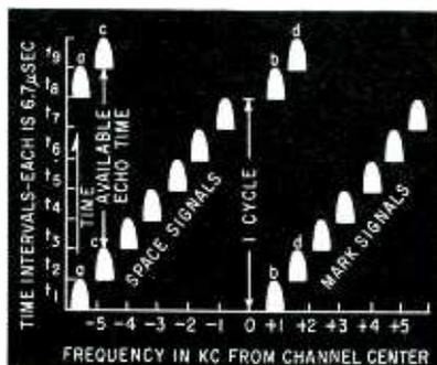
FIG. 2—At any time  $t$ , channel frequency is shifted either right or left of center, depending on keying information
