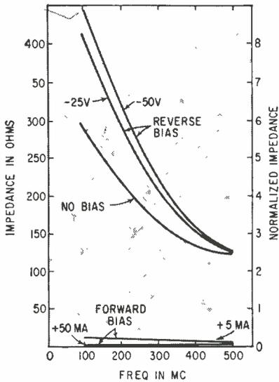
FIG. 3—Impedance of a pin diode plotted as a function of frequency for varying bias conditions
