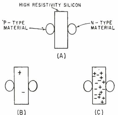
FIG. 2—Sketch of pin diode (A) shows distribution of conduction carriers when reverse-biased (B) and when forward-biased (C)
