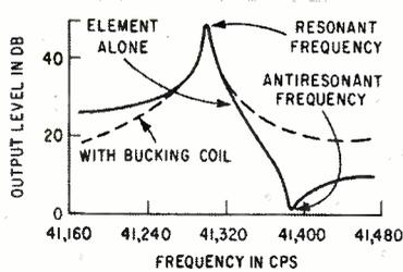
FIG. 4—Frequency response of typical element, with and without bucking coil
