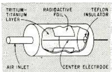
FIG. 1—Although radiation is not detectable outside the radiological transducer, its external surface bears a warning symbol
