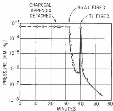
FIG. 4—Pressure is plotted against time for prototype vacuum tube
