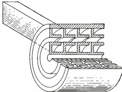
FIG. 3—Proposed coiled ridge waveguide structures for higher power output
