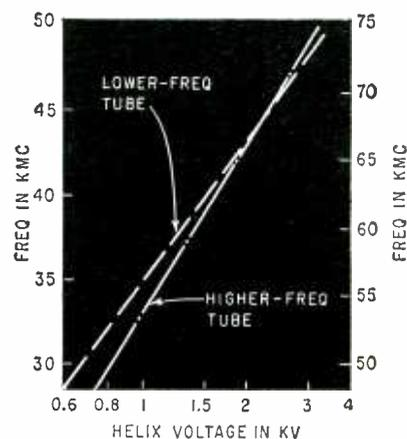
FIG. 1—Helix voltages control operating frequencies of oscillators
