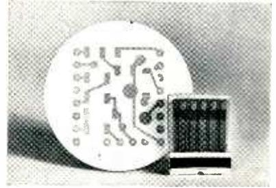
Folder of matches indicates size of ceramic circuit board
