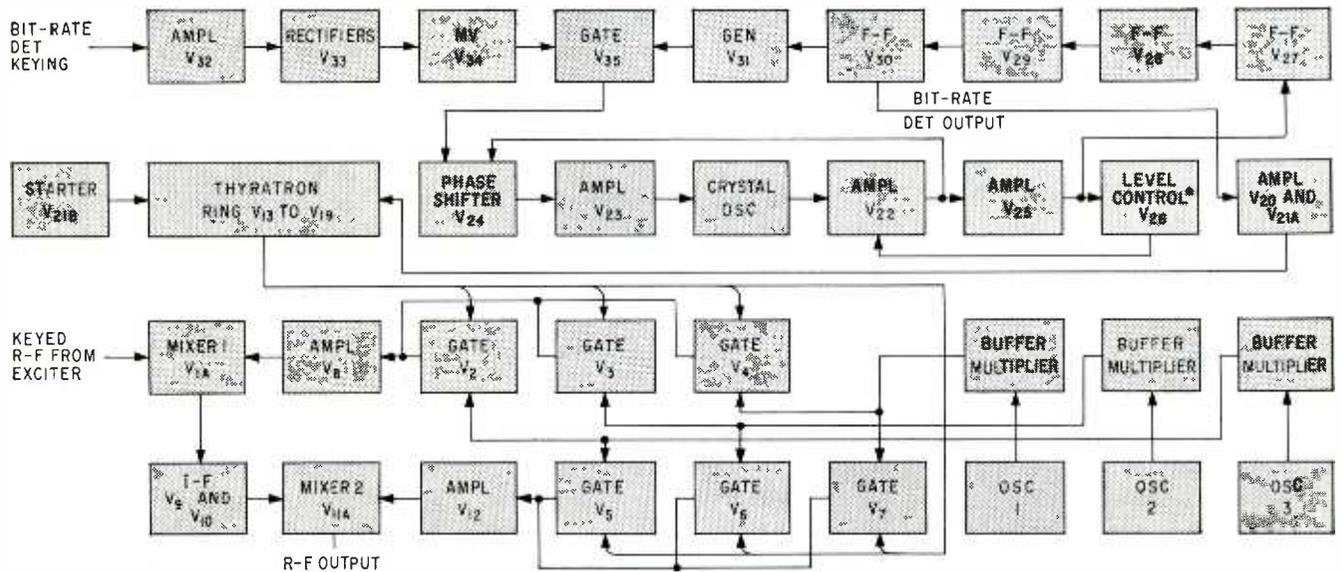
FIG. 4—Transmitter frequency translator. Bit-rate detector consists of all blocks in the upper-two rows, except the thyatron block
