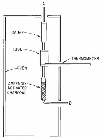
FIG. 2—Simple arrangement for baking tube requires home-made oven
