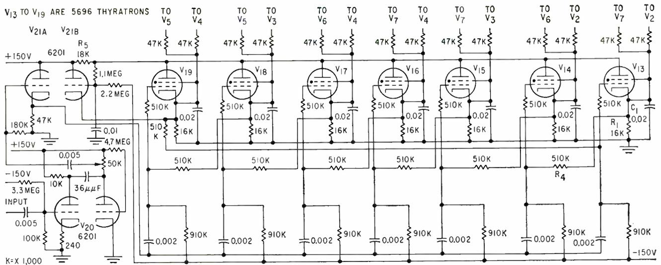
FIG. 7—The bit-rate detector supplies the input to  $V_{20}$ , which is an input amplifier of the thyatron ring comprising tubes  $V_{13}$  to  $V_{19}$
