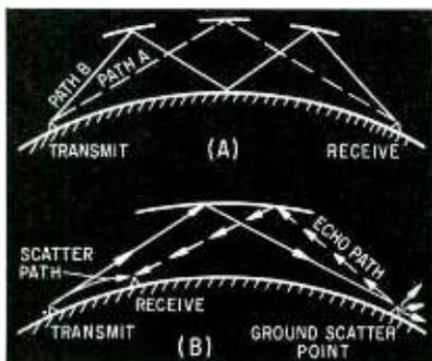
FIG. 1—Path B (A) is the longer of the two paths. Direct-scatter path (B) is much shorter than the indirect paths
