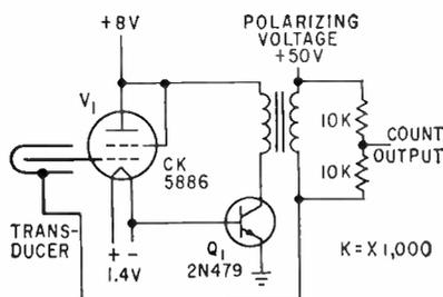
FIG. 2—Transformer is an audio type with large step-up ratio. Polarizing voltage supplies less than a  $\mu$  amp
