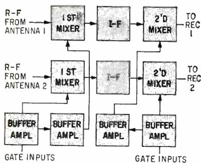
FIG. 5—These blocks compose portion of receiver frequency translator that differs from transmitter frequency translator
