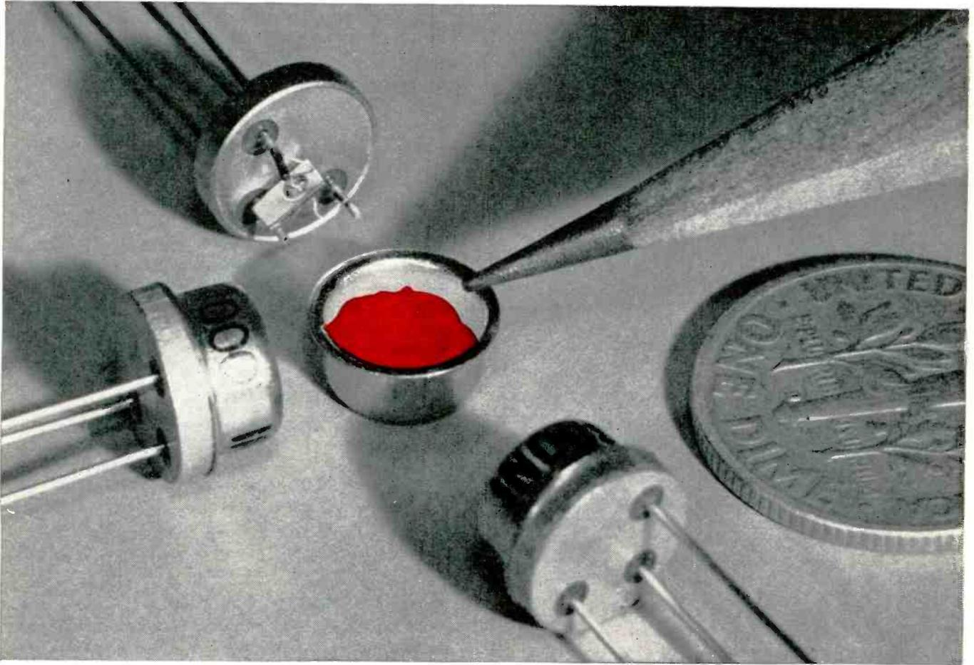
Made by Industro Transistor Corp., these miniature transistors are potted with a Dow Corning silicone compound to cushion vibration, improve heat dissipation, prevent contamination of the junction.
