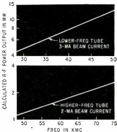
FIG. 2—Power outputs of oscillators vary with operating frequencies
