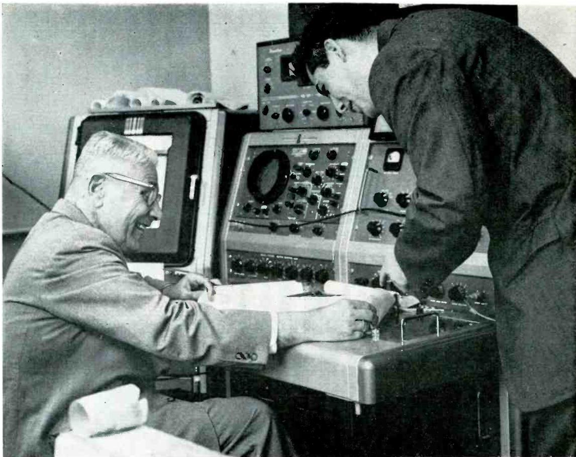
NYU physics professor Hartmut P. Kallman and a graduate student use an electron paramagnetic resonance spectrometer to detect and measure the concentration of unpaired electrons in inorganic phosphors
