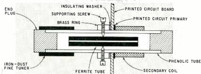
FIG. 2—Construction details of a torsional mode magnetostriction filter element
