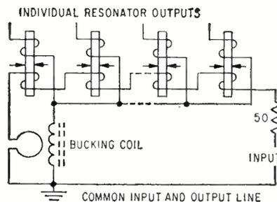
FIG. 6—Circuit for typical comb filter
