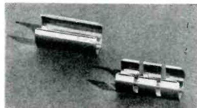
Hughes Aircraft found shock mounting clip at right compensates for variations in tube envelope dimensions
