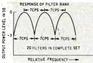
FIG. 1—Frequency response of a narrow-band filter bank
