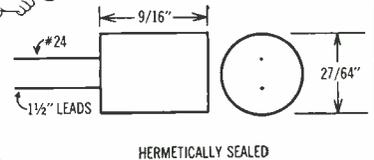
You can choose Micro-Stats from over 50 designs, each with Pulse Engineering's singular clamped core construction. Pulse constructs these units on an armite form for precise winding geometry to control leakage inductance and distributed capacity. Voltage breakdown and insulation resistance are improved over conventional toroid and cup core construction. Available for immediate delivery—many types in stock.
