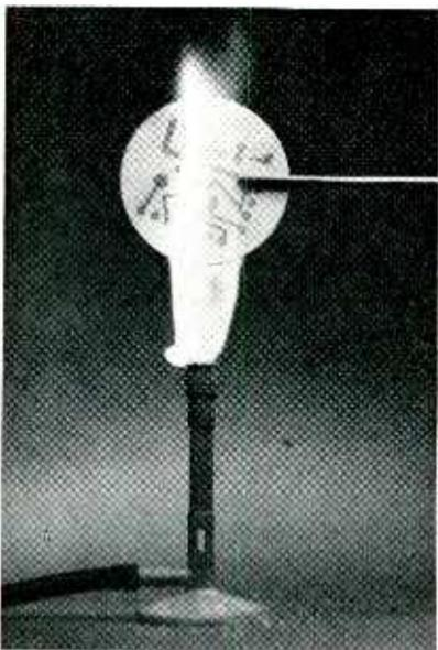
Molybdenum printed circuit subjected to heat of a Bunsen burner
