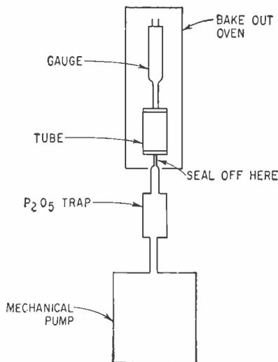
FIG. 3—Mechanical fare-pump is used in this approach to exhausting
