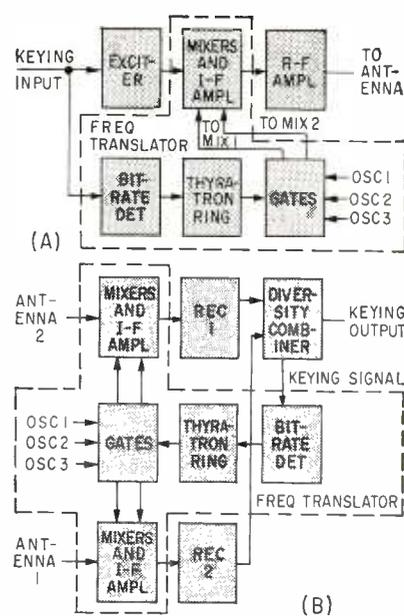
FIG. 3—Section enclosed by the broken lines is the frequency translator of the transmitter (A) or the receiver (B)
