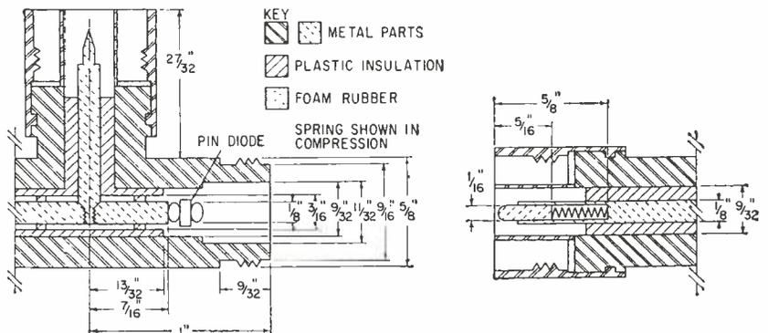
FIG. 5—Mechanical arrangement of diode, showing details of the semiconductor switch. The diodes are positioned inside a coaxial tee connector with a spring-loaded plug for making contact to the diode
