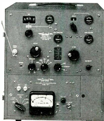
As optional equipment the FM-7 may be combined with the new DM-3 Deviation Meter as illustrated. The DM-3 is a new Dual-Range Deviation Meter with 15 kc and 7.5 kc full scales.
