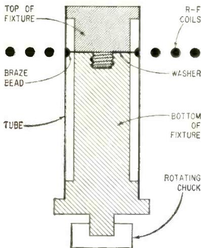
FIG. 1—Cross section of setup, showing how take-apart fixture positions internally-brazed part
