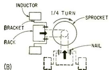
FIG. 3—Rack dips 9 assemblies into encapsulant with 1 motion
