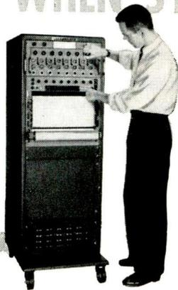
Additional features of the 950-1500 include: common power supply, built-in MOPA, front and rear inputs, easily serviced plug-in circuit cards, adaptability for use with other readout devices. When many channels are constantly in use for floating or grounded high gain inputs the simplified 950-1500 design assures dependable operation, yet at much lower "per channel" cost.
