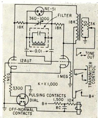
FIG. 6—Dial code sender circuit used in mobile units to unlock repeater station
