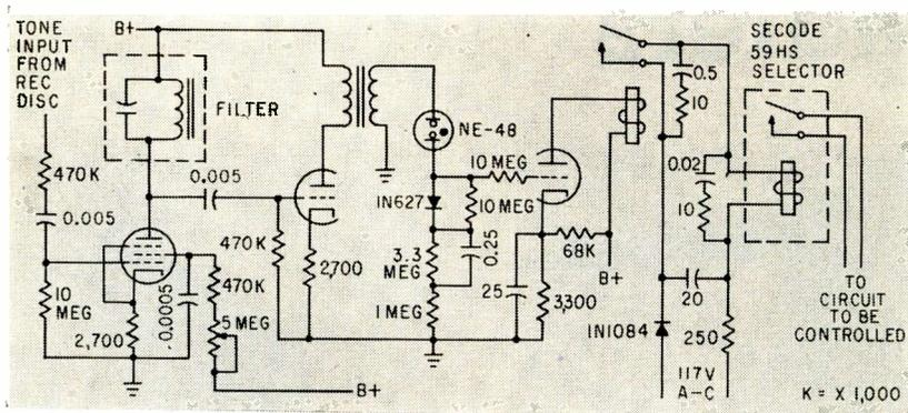
FIG. 5—Decoder circuit used in repeater station with dial lock out
