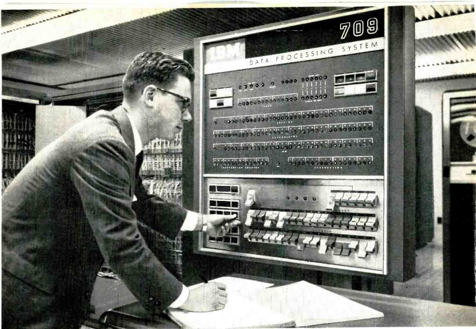
Programmer makes operational check from "driver's seat" of IBM 709 Data Processing System — the most up-to-date system utilizing electron tubes.
