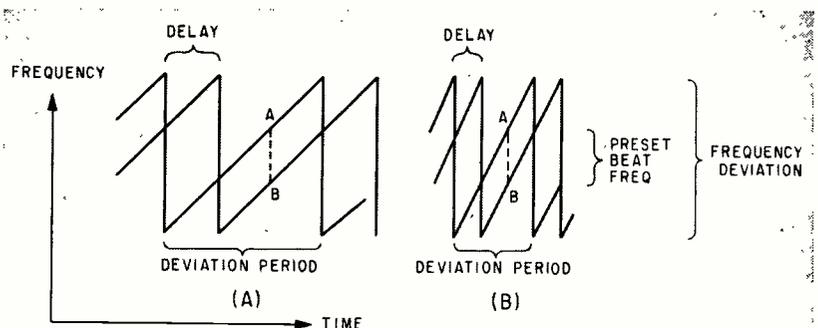
FIG. 2—Transmitter sweep rate is shown for a missile at two distances. For A, the missile is farther away than at B
