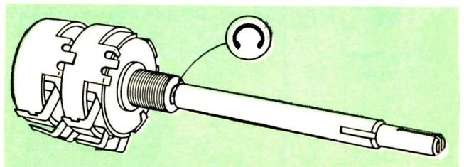
**FIG. 2**—Radially-assembled crescent ring locks threaded ferrule on potentiometer shaft. Low shoulder, uniformly concentric with shaft, provides clearance necessary for assembly of panel locknut. Ring may be removed easily and reused
