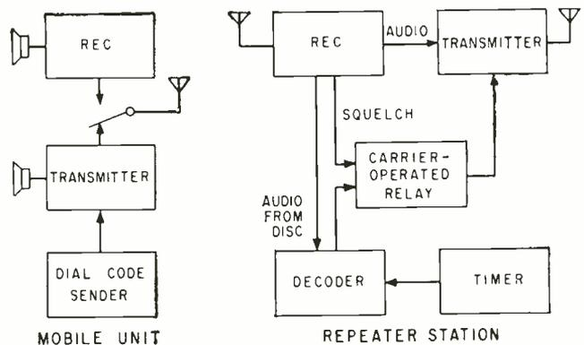
FIG. 4—With dial lock out, mobile operator dials to gain access to repeater. Decoder cuts in the carrier-operated relay so that the presence of carrier will turn on transmitter
