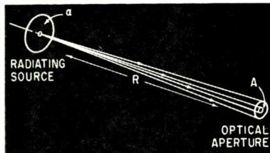
FIG. 1—Power radiated from source is a function of wavelength and temperature
