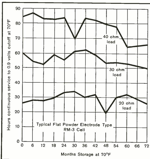
An extensive series of storage tests, now well past the six-year mark, proves that Mallory Mercury Batteries can take extremely long storage far past the point where ordinary batteries become useless.
