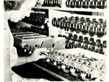
Assembling Increductors. Completed units are in storage racks
