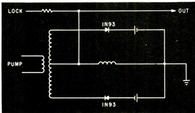
FIG. 5—Phase-locked subharmonic oscillator using lumped parameters. Oscillating parameter is nonlinear capacitance of the two 1N93 diodes
