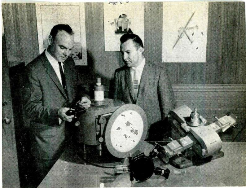
Early Amplitron tube, left, shown beside wooden mockup of new microwave tube 20 to 50 times more powerful
