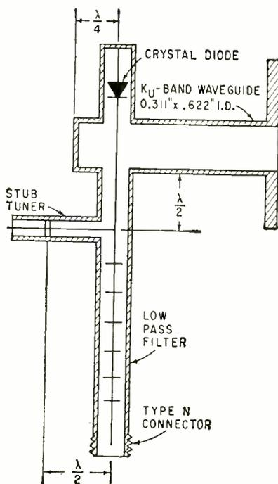
FIG. 1—Multiplier mount dimensions in Ku-band wavelengths
