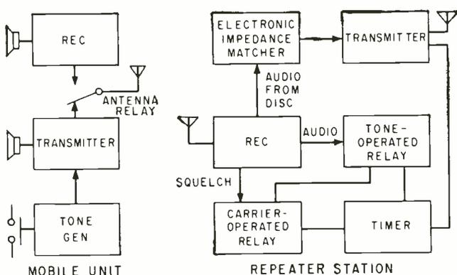
FIG. 3—With tone-gated lock out, mobile unit uses repeater station by transmitting a tone burst which actuates the tone-operated relay allowing carrier control of repeater transmitter
