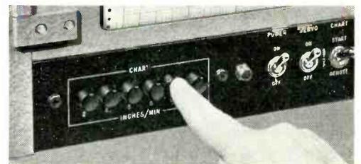
Six chart speeds, 2, 4, 6, 8, 15 and 60 in/min selected instantly by front panel push buttons.
