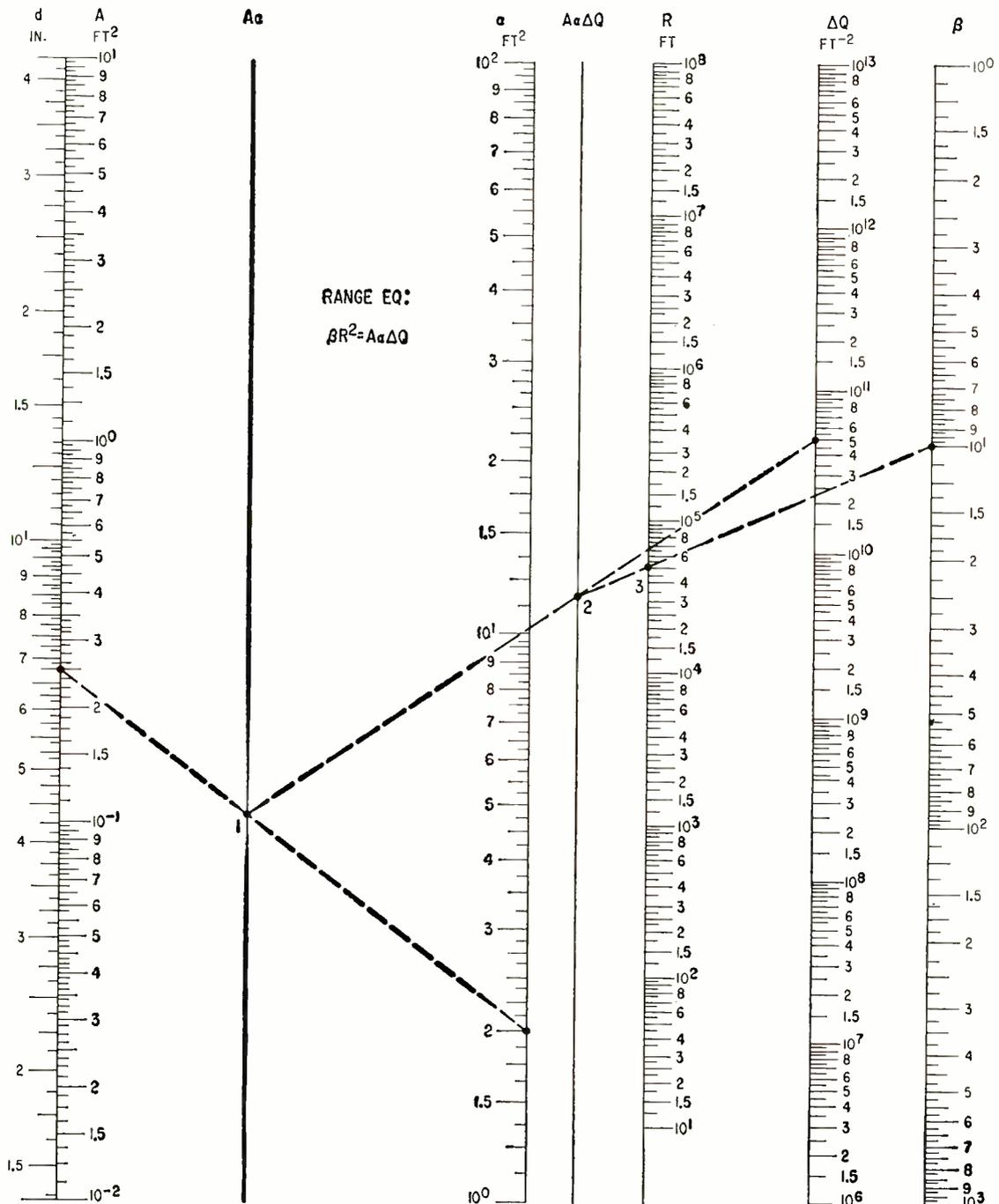
FIG. 3—Using this nomograph and Table II makes it possible to solve for unknowns in range equation. Column labeled  $d$  gives diameter in inches of lens having area  $A$
