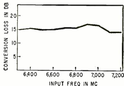
FIG. 2—Second harmonic conversion loss using a 1N78 diode in the mount. Fundamental peak power is equal to  $19 \pm 3$  db above one milliwatt
