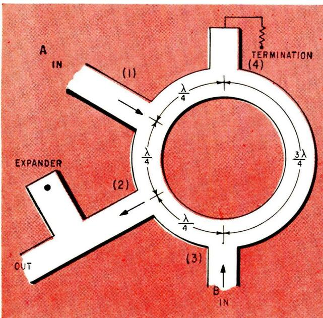
FIG. 2—Logical AND circuit using hybrid ring. Expander (diode in quarter-wave stub) gates output when both input signals are present. Removal of stub termination at (4) changes circuit to primitive half-adder
