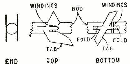
FIG. 2—Rubber bands and cement keep tabs of top rod in place until dipping
