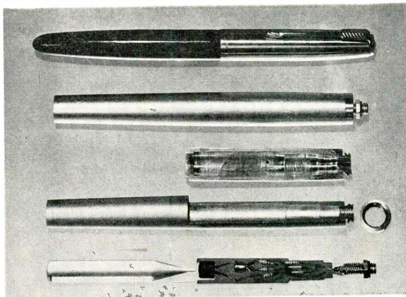
Disassembled pen with light-pipe lens and preamplifier mounting board removed is shown at bottom. Above is assembled light pen, at top fountain pen for size comparison
