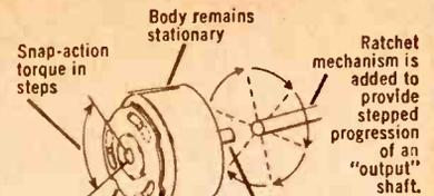
Armature plate rotates through predetermined angle then springs back to original position.
