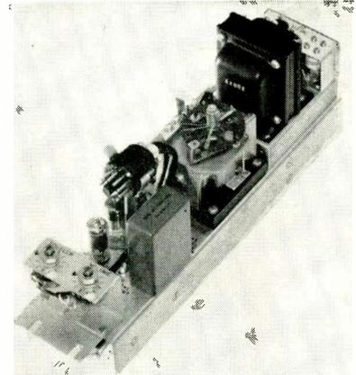
Dial pulse decoder shows escapement wheel selector. Some selector types can be set to any of 20,000,000 different code combinations
