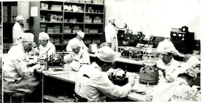
**COMPLETE FACILITIES** include dust-free rooms for precision production . . . environmental testing equipment . . . compass-testing devices that simulate ship's pitch, yaw and roll. Plant is fully air-conditioned.
