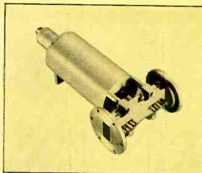
Ideal for linear accelerators and high-power radar systems. The QK-783 and QK-622 Amplitrons operate over the 2,700-2,900 mc and 2,900-3,100 mc bands, respectively, at a peak power of 3 megawatts and a typical efficiency of 75%. Because no heater is required, these tubes are capable of exceptionally long life. RF gain is 8 db under rated conditions, and as high as 12 db at lower peak power outputs. Phase pushing figure is less than 0.5 degrees for a 1% variation of anode current.
