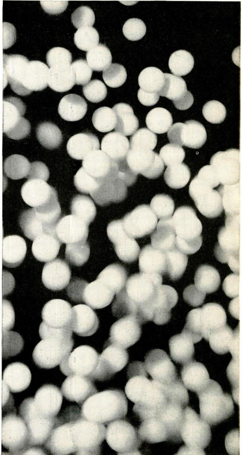
Large-scale dynamical model of gas in operation
