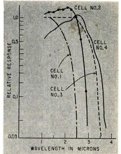
FIG. 2—Typical spectral response curves
