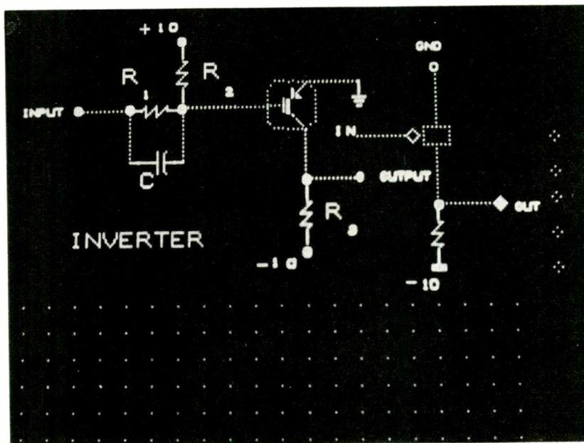
Sample cathode-ray-tube pattern drawn using control link
