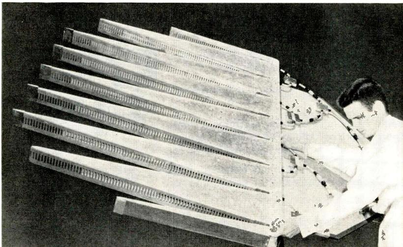
Retarded wave surface antenna with high gain and low silhouette was developed by Chance Vought Electronics Division for use in airborne early warning radar as well as ground based and shipboard radars. One-sixth scale model of 35-ft retarded surface wave antenna is shown
