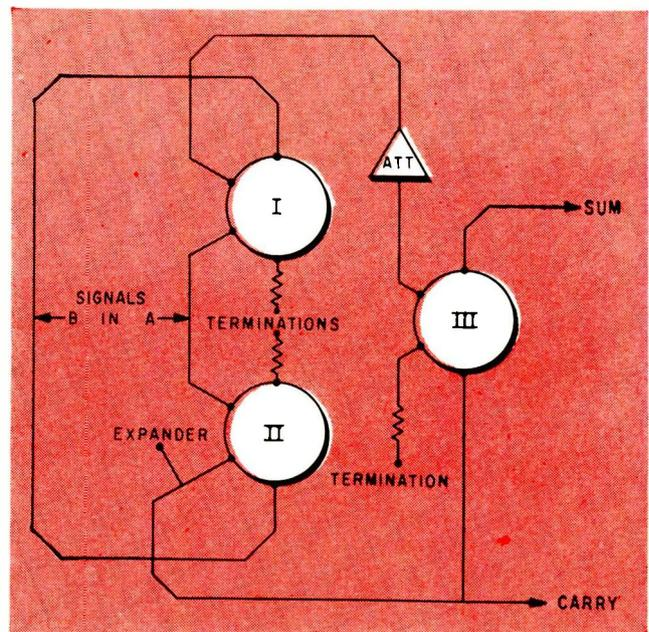
FIG. 3—Phase-determined half-adder using hybrid ring. Ring I combines signals; ring II serves as logical AND circuit to produce carry; ring III is logical NOT circuit to suppress sum when carry is present
