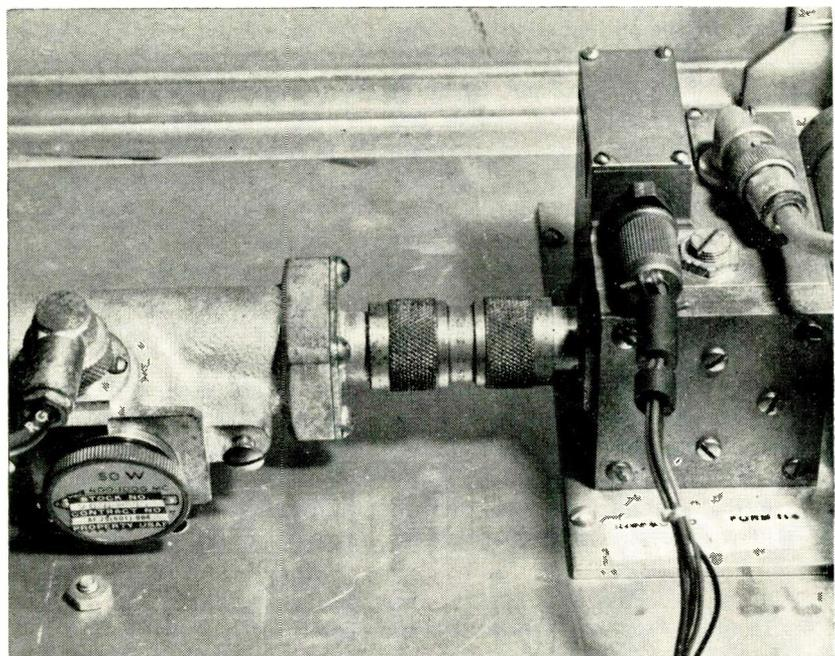
The f-m/c-w radar transmitter operates from 800 to 1,000 mc. The actual transmitter is at the right side of photo
