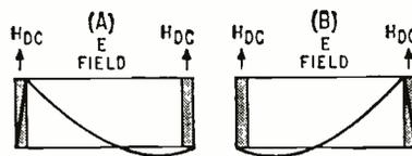
FIG. 4—Graphs of E and H-field distributions along two cross sections of waveguide in positive (A) and negative (B) directions
