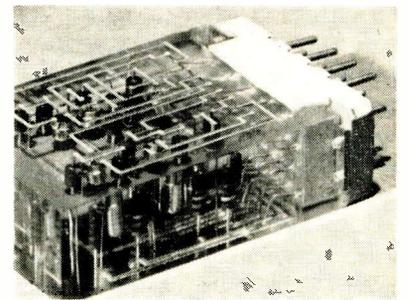
Transistor inverter package with deposited wiring and plated connections
