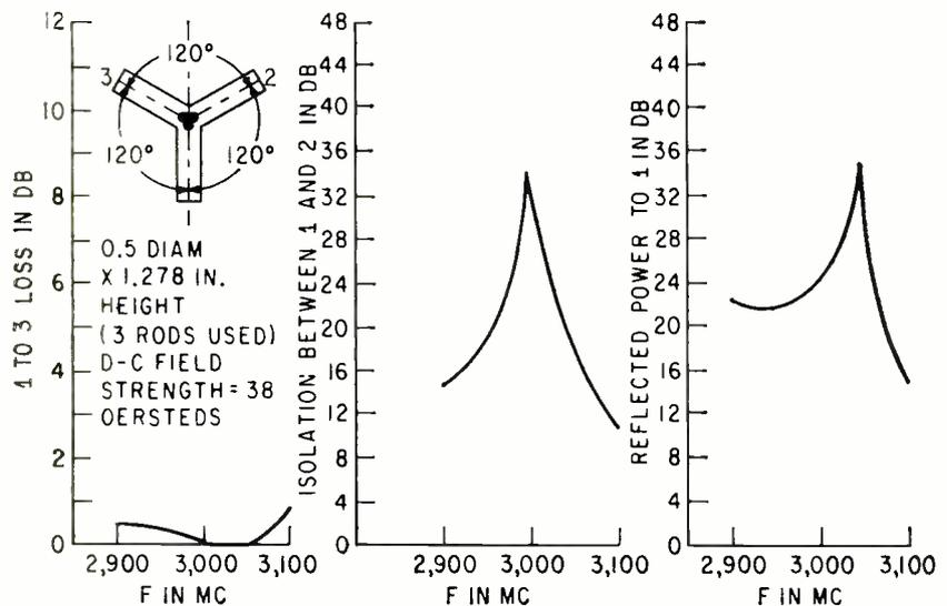
FIG. 8—Test data for S-band circulator whose wave-travel direction is from 1 to 3
