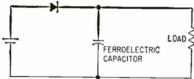
FIG. 1—Holding diode prevents capacitor from losing initial battery charge. Increase in charge results only from temperature change
