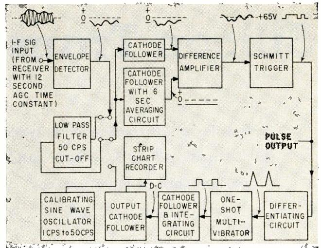
FIG. 1—This recorder diagram shows progressive transformations of i-f signal input
