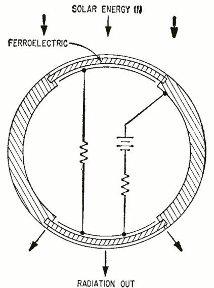
FIG. 5—Solar energy could be converted into a-c voltage with this arrangement
