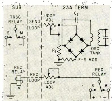
FIG. 3—Modulation arrangement for two-path polar loop uses diode bridge. Similar bridges are used for other types of loop operation
