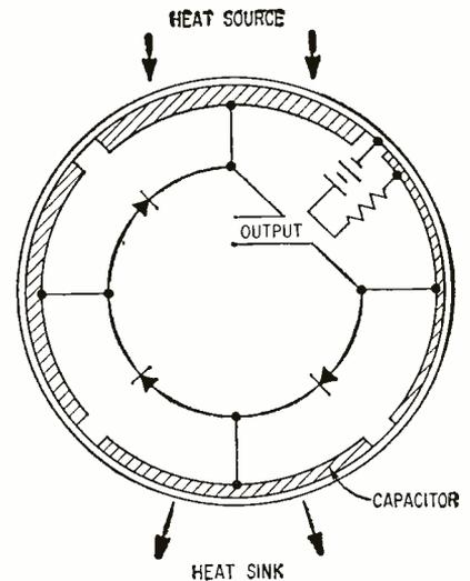
energy also increases by  $K_c/K_b$ . Permittivity in Fig. 2 depends on field strength, which changes during a temperature cycle, and the curve is applicable only with low applied field. Practical converters operate at higher field strength and permittivity does not drop below Curie temperature. They are therefore cycled between Curie point and a higher temperature.
