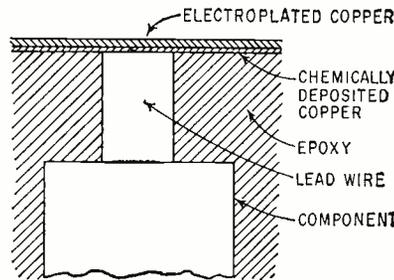
FIG. 1—Detail of plated connection
