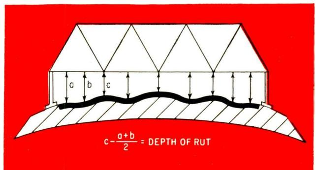
FIG. 7—To measure depth of rut, outputs of probes a and b are averaged then subtracted from output of probe c
