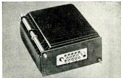
This is a compact, modular electronic control amplifier that boosts small error signals to power electro-mechanical components, providing a gain factor of 500. Hermetically sealed in nitrogen and hydrogen. Latest design techniques result in direct 115-volt, 400-cps excitation with lower power consumption than on conventional bridge-type amplifiers. Meets a wide range of applications due to low power consumption, high gain, load capacity, and compactness. Ask for full details.
