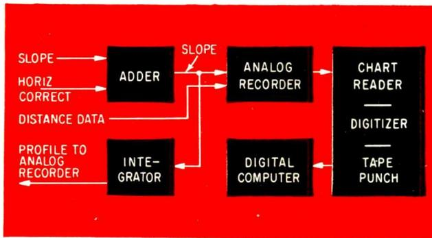
FIG. 5—Analog recorder accepts pavement slope signal which is digitized for summation purposes. Distance data and start and finish signals are also supplied
