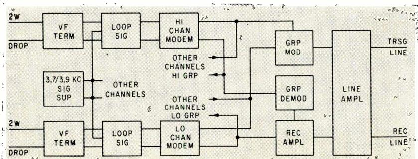
FIG. 6—Terminal of telephone carrier system. Four terminals can be mounted in one 11-ft, 6-in. bay
