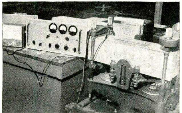
FIG. 1—Test setup checks strain gage by bending concrete beam in beam breaker that determines flexural strength
