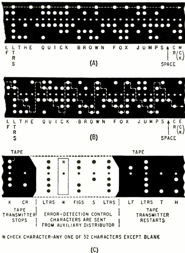
FIG. 4—Horizontal check line (A), spiral check line (B) and error-detection control characters (C) used in odd-even count error detection system
