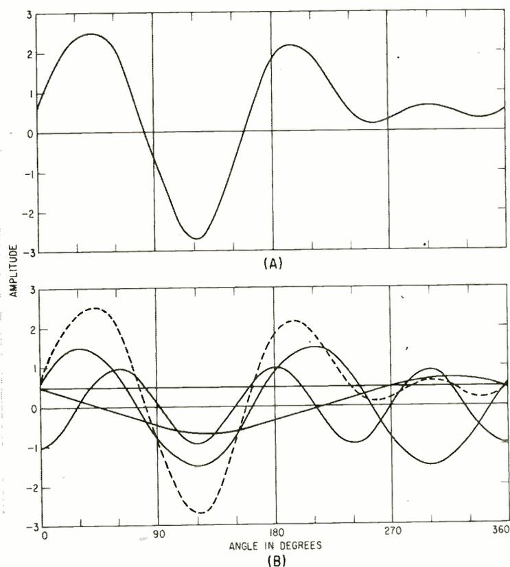
FIG. 1—Complex wave (A) is broken into its harmonics and baseline (B) by using form shown in Fig. 2. Dotted line shows check obtained by adding harmonics and baseline at each point
