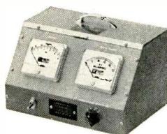
**VTP TC-43-1 THERMOCOUPLE GAUGE CONTROL** Dual meter control. Indicating meters for heater current and system pressure. Rotary switch permits selective measurement of pressure at any one of four separate measuring points.
