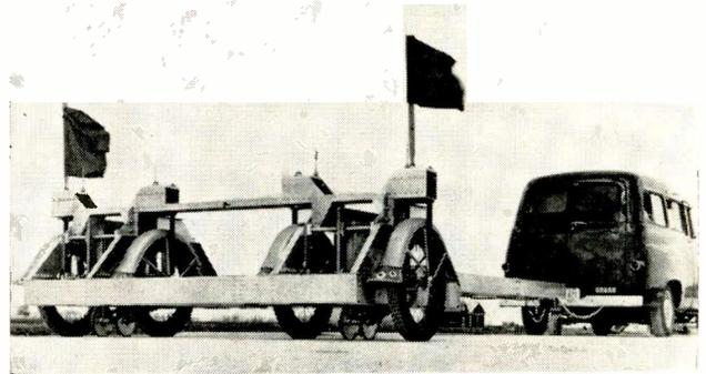
FIG. 4—Longitudinal profile of road is highly correlated with road performance. Slope-detecting wheels are located between the two pairs of large riding wheels
