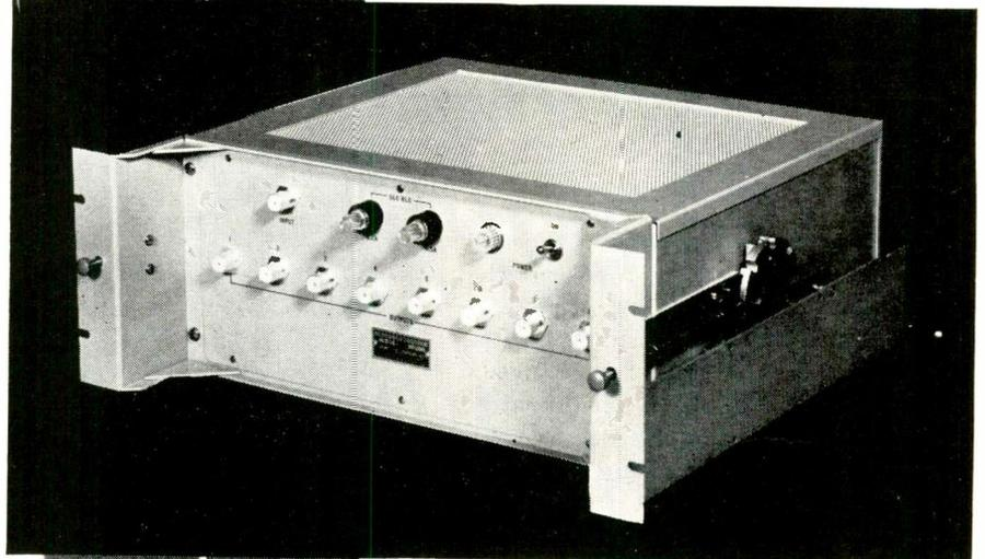
**T**HE PM-406 is a combination instrument comprised of a preamplifier and multicoupler located on a single chassis for rack mounting. This unit permits the coupling of eight receivers to a single antenna and is designed for use where short runs of cable from the antenna are employed. These units are of the "bath tub" chassis design having a 3-inch recessed front panel to permit patching cables to hang without protruding. Modifications of this design are available on special order.
