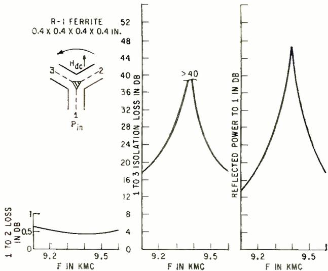
FIG. 6—Data for Y-type circulator. Wave travel is from port 1 to 2
