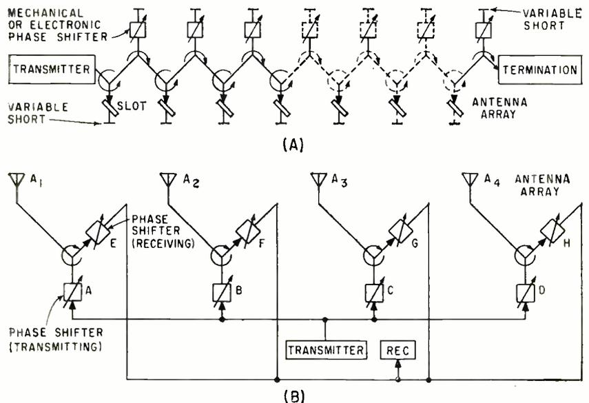
FIG. 9—Series-fed antenna array (A); parallel-fed antenna array (B)
