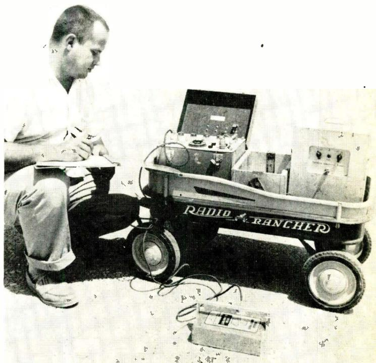
FIG. 8—Crushed stone base material density measured by backscatter from  $Cs^{137}$  source and indicated on wagon-mounted scaler
