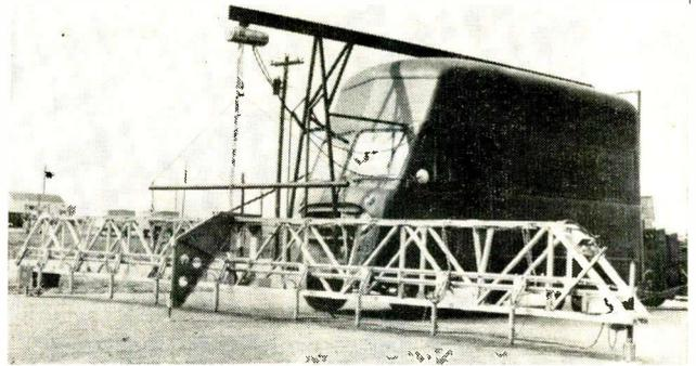
FIG. 6—Transverse profilometer truss can be quickly leveled and probes activated by equipment in truck. Motor-driven carriage (left bottom of truss) records analog of profile
