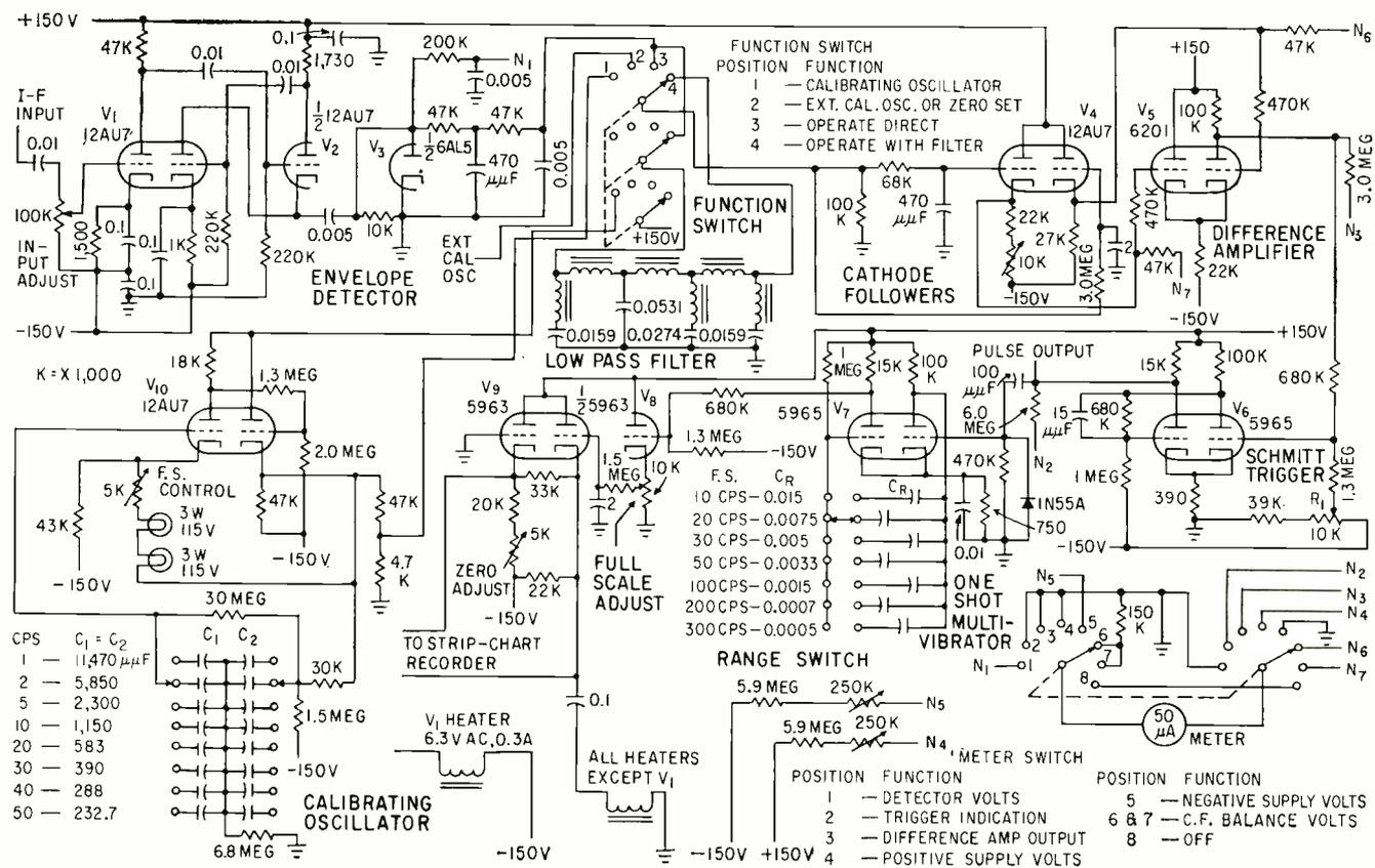
FIG. 2—Complete schematic of fading rate recorder. This unit records fading rates from less than 0.5 cps to 300 cps at receiver i-f frequencies from 100 kc to 455 kc
