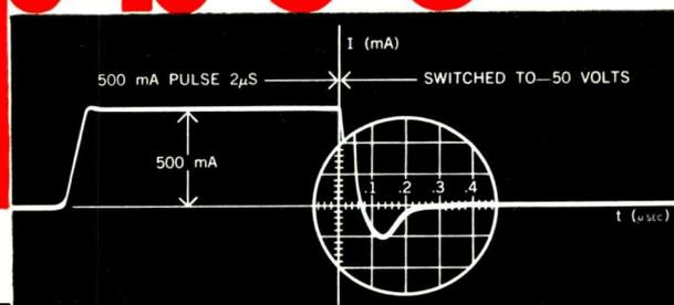
... in a high-current silicon switching diode. The 1N920-1N923 series is the latest result of Sperry Semiconductor's unique developments for the computer field.
