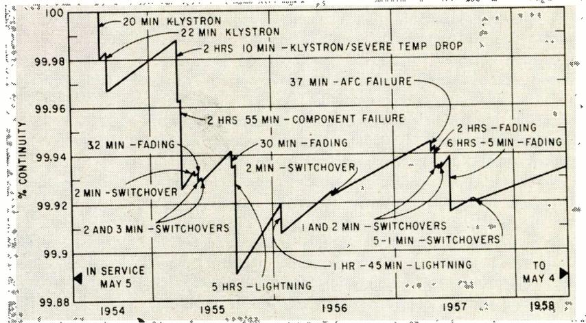
FIG. 1—Typical microwave system (Canton-Philo) provides reliable operation. Records show a continuity about 99.88 percent for the system or 99.97 percent per hop
