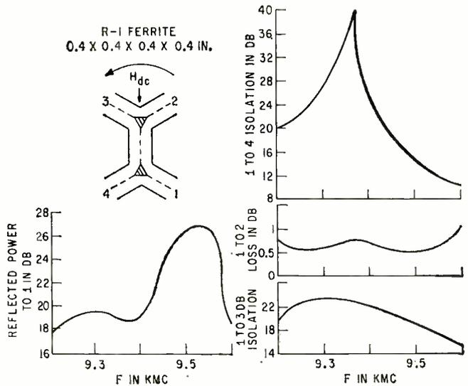
FIG. 7—Data for 4-port circulator. Wave travel is from port 1 to 2
