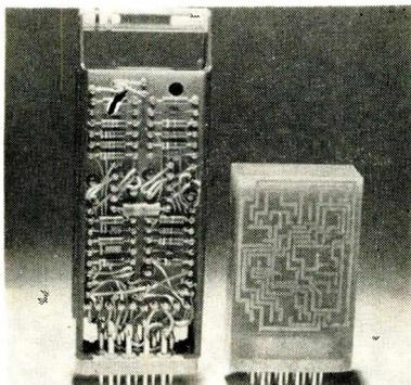
Flip-flop with deposited wiring and plated connections (right) contains components identical to those in the conventional package
