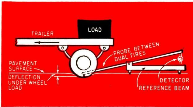
FIG. 3—Benkelman beam used to measure road distortion due to applied load as truck passes probe at creep speed. Road deflection is indicated on detector
