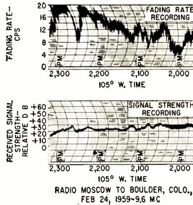
FIG. 3—Typical recording of fading rate and average signal strength
