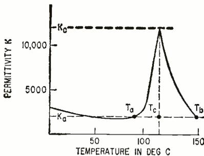
FIG. 2—Permittivity curve of barium titanate as temperature is varied around Curie point,  $T_c$ , applies only with low field strength
