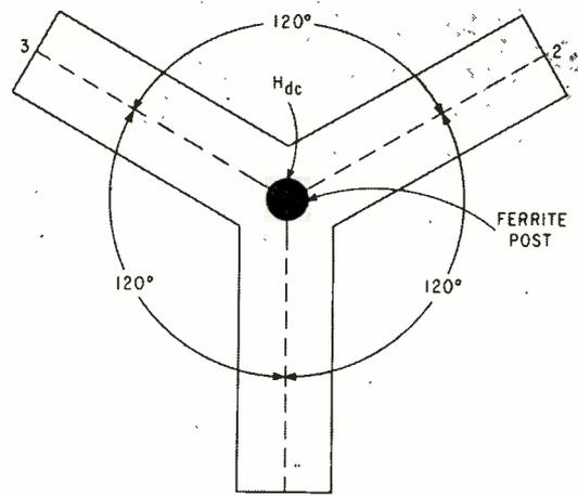
FIG. 1—Circulator's cylindrical ferrite produces transverse d-c field
