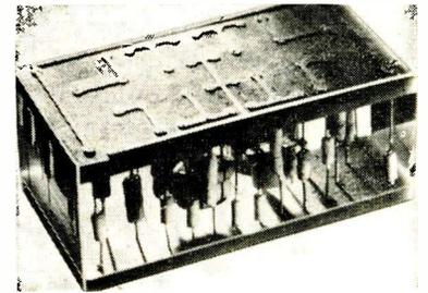
Encapsulated dual flip-flop with plated connections and etched wiring. Unit is 2 inches long
