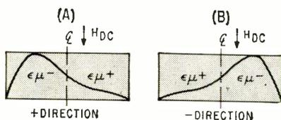
FIG. 2—R-f fields in positive (A) and negative (B) directions of wave travel
