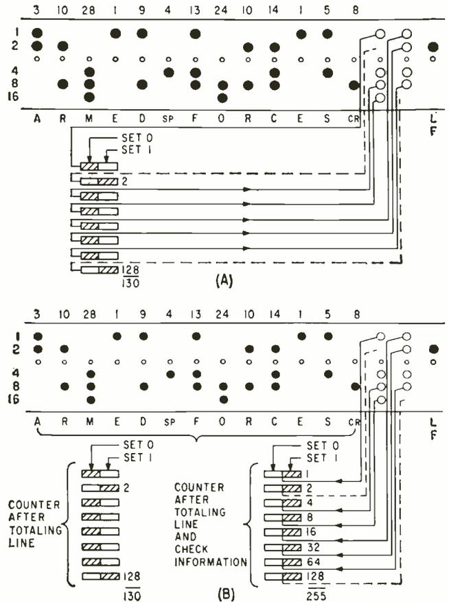
FIG. 5—Method of preparing tape at sending station (A) and checking tape at receiving station (B) in binary totaling error detection system shows how characters are totaled
