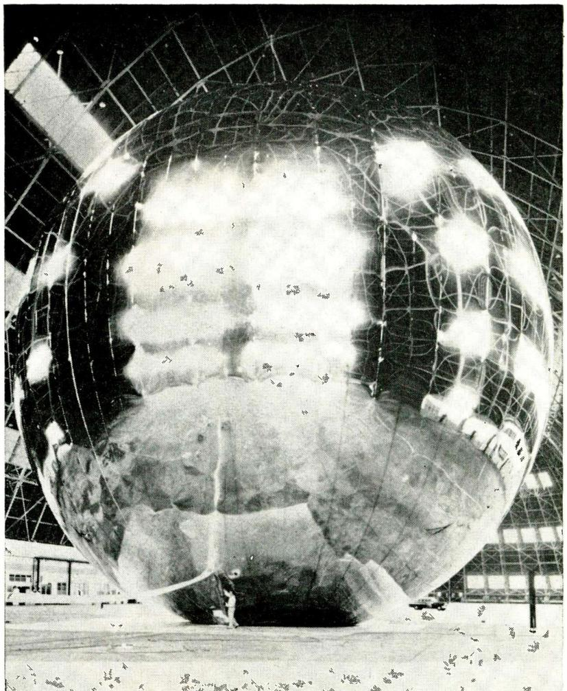
NASA's 100-ft aluminumized polyester film sphere will fold inside a 28-in. diameter container at launching of passive balloon satellite
