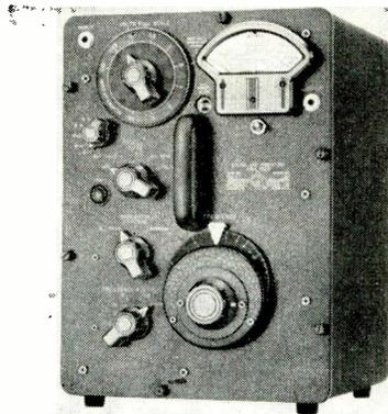
frequency) components, but also continuous (noise) components. The instrument's narrow bandwidth is wide enough to embrace the small frequency fluctuations (or wow) arising from normal variations in speeds of engines, machines and appliances; 40-db discrimination obtains at one octave from selected frequency. The alternate,  $\frac{1}{3}$ -octave bandwidth is available at low vibration frequencies.
