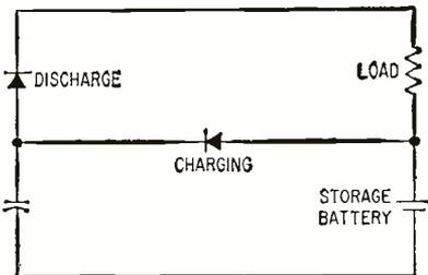
FIG. 3—Increased voltage across capacitor as temperature increases recharges storage battery through discharge diode
