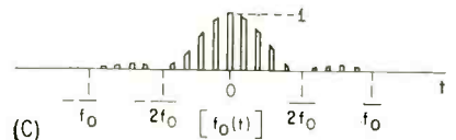
FIG. 3—Radar return from search-lighted target (A); dynamic antenna pattern (B); and return from scanned target for which spectrum is desired (C)
