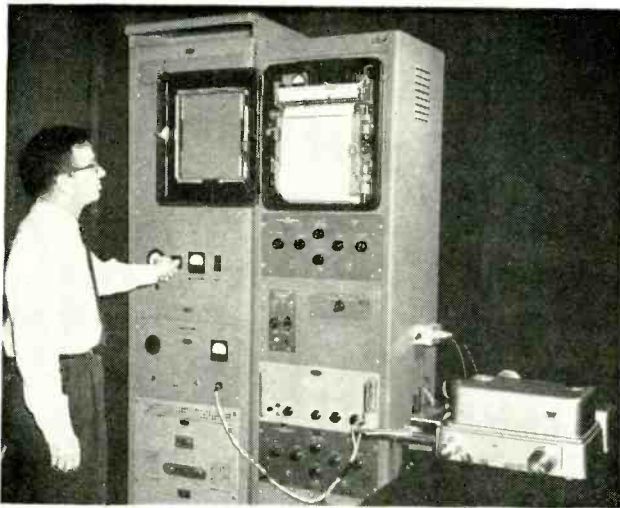
Monochromator is at right in the photo; at left are power supplies for the lamps; recorder and amplifier are in the center
