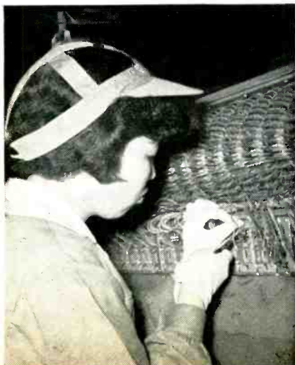
Tatsuko performs an intricate series of wiring jobs on automatic switchboard assembly line
