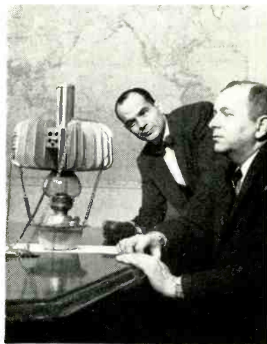
Martin Co. vice president J. D. Rauth, (right) and nuclear division head M. E. Talaat study Russian-built device for converting heat of kerosene lamp into electricity for radios in remote Asian-USSR provinces
