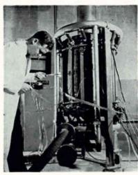
Testing of one of two 2,500-w subgenerators making up thermoelectric power plant developed for Bureau of Ships, U. S. Navy
