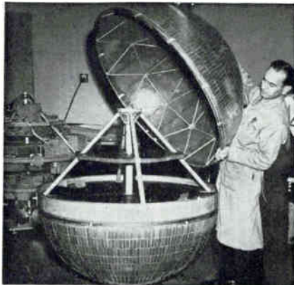
Epoxy glass fiber shells are put on dummy form to check fit of parts
