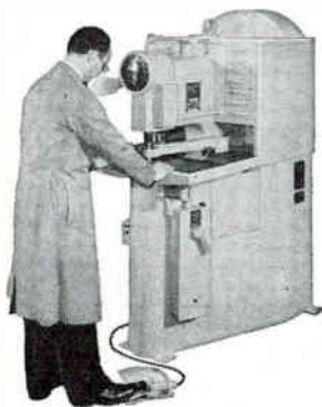
STRIPPIT Model 15A contains the new STRIPPIT Electro-Hydranatic Head. Simplified design completely eliminates the need for pressurized air.
