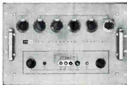
This is a KIN TEL 601A AC voltage standard, the nearest AC equivalent
