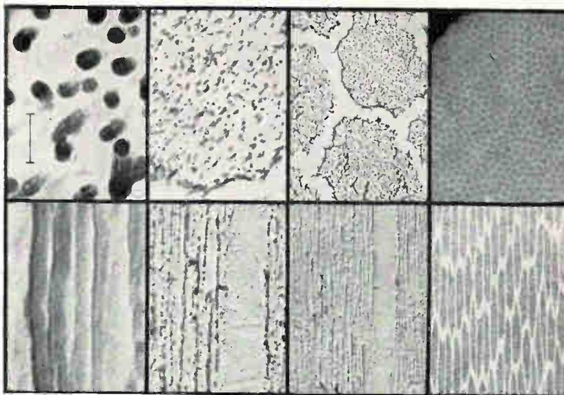
**MAGNETICS.** These are micrographs of longitudinal (bottom) and cross section of iron wires in a copper alloy matrix made by wire drawing. This technique is used to prepare elongated iron particles with diameters less than 1,000 angstroms. Work was recently described by F. E. Luborsky of General Electric Research Laboratory at the Sixth Annual Conference on Magnetism and Magnetic Materials. For other conference highlights, see Assistant Editor Lindgren's article (p 81).
