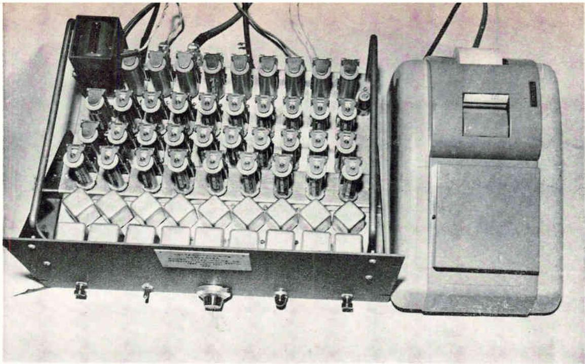
*Top view of analog-to-digital converter, with solenoid-operated printer*
