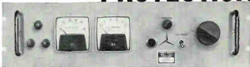
Prevents damage to power supply load under any conditions. Unique electronic circuitry monitors output voltage at all times and reduces output voltage and current to nominal zero if output attempts to rise above operating voltage. Of course turn-on and turn-off transients are also eliminated.
