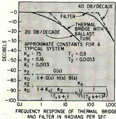
FIG. 3—Transfer function and frequency response
