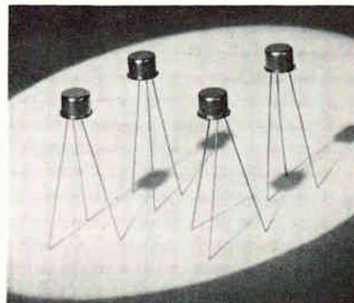
for general purpose, medium power, fast-switching applications. They have low input impedance, low collector capacitance (typically 14 pf), with operating range from 10 µa to 500 ma, and 4 watt power dissipation. (Continued on page 122)
