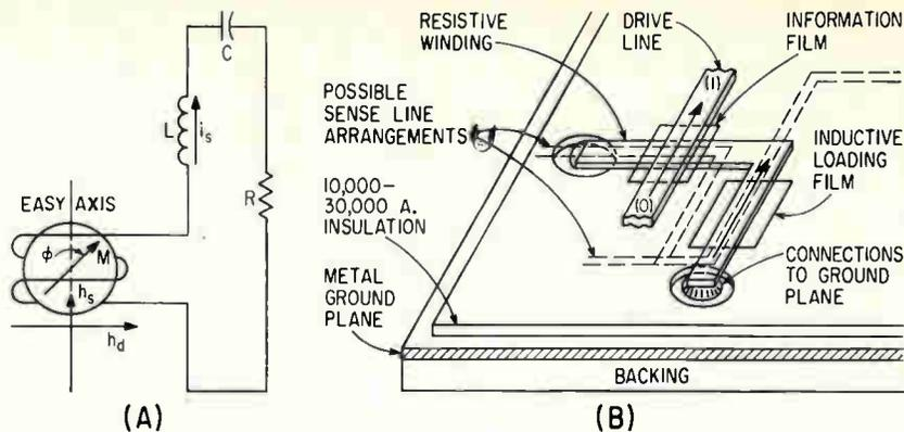
FIG. 2—With proper film and circuit parameters, this circuit (A) may be used as a flip-flop in which the magnetization  $M$  in the film is switched from either one of its rest orientations to the other by successive drive field pulses,  $h_d$ . Reliability of magnetic-film memory can be increased by passive  $R$ - $L$  loading (B)
