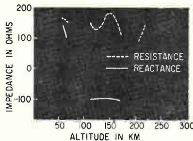
FIG. 8—Antenna impedance curves at 7.2 Mc (curves are shown where conditions permitted data reduction)
