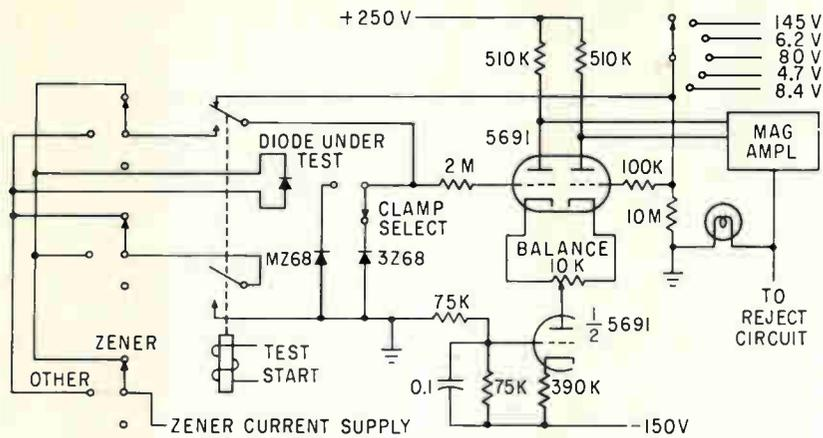
FIG. 3—Typical test circuit uses difference amplifier to trigger magnetic amplifier to signal reject
