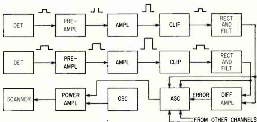
FIG. 2—Unequal length pulses from each detector of pair are converted to d-c voltages and applied to differential amplifier to produce off-axis error signal
