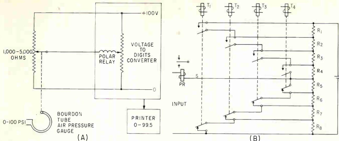
FIG. 1—Digital air-pressure recording system (A), with converter shown in simplified form. In an elaboration of the basic system (B) the  $T$  relays operate in combinations to include or short out various resistances in the voltage divider chain. For example, if relays  $T_1$  and  $T_2$  are operated, resistances  $R_1$ ,  $R_2$ ,  $R_3$  and  $R_4$  are shorted out, and the others remain in the circuit. The converter uses 9  $T$  relays and 18 divider resistors
