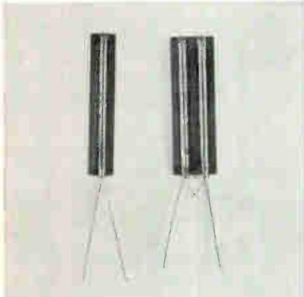
Weldable strain gages, one-piece, etched wire filaments in swaged stainless steel tubes, are suitable for use from cryogenic to elevated temperatures. Photo shows typical gages in actual size.
