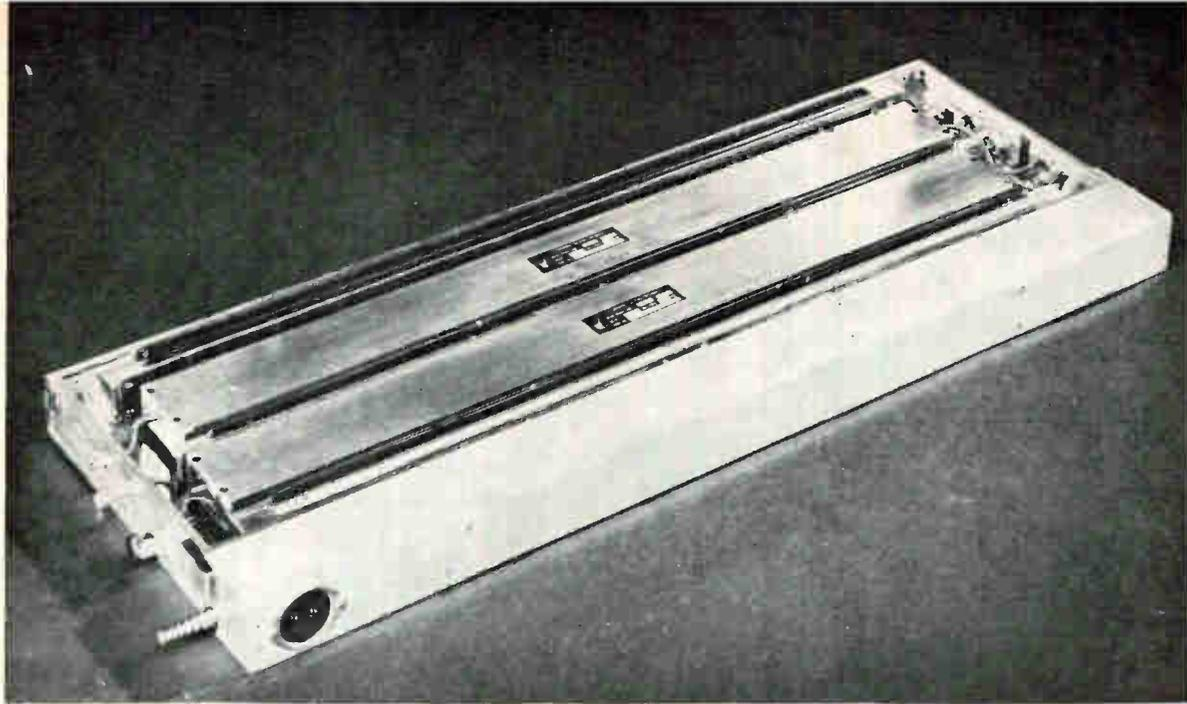
Delay line with optics package, but shown without the photoelectric readout equipment
