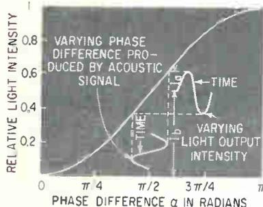
Fig. 2—Relationship between optical phase retardation and intensity of light reaching the multiplier phototube
