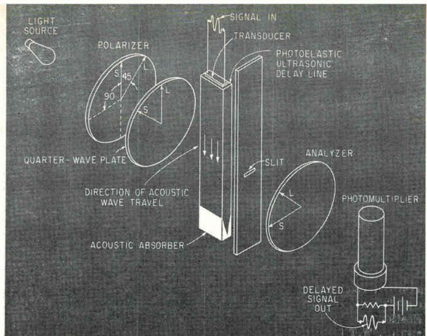
Fig. 1—Schematic arrangement for reading out the acoustic wave data as it passes down the glass delay line
