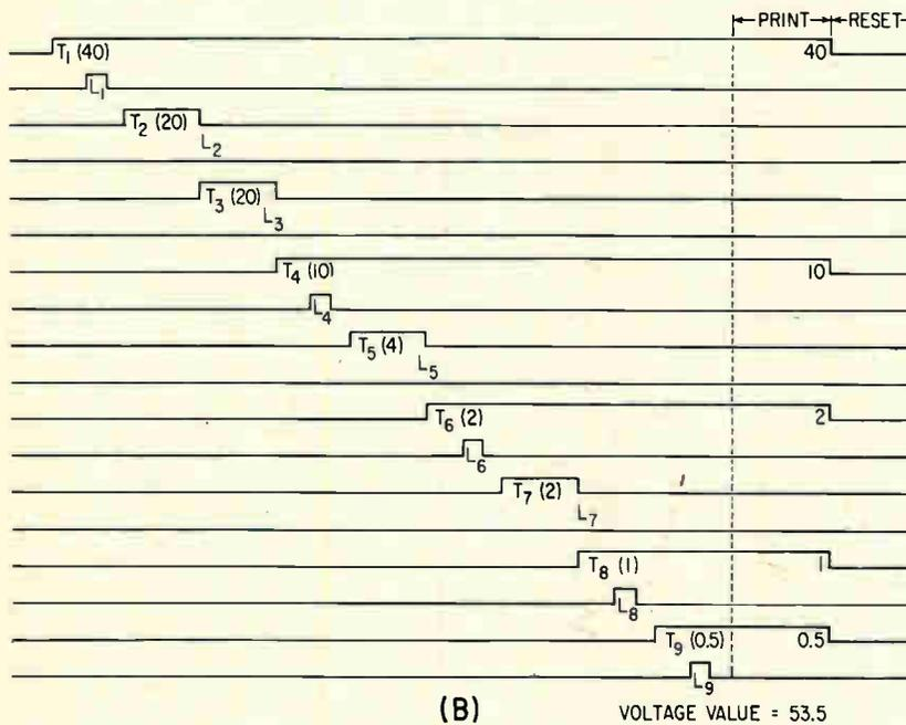
FIG. 2—The partial schematic (A) shows the first two of the nine sets of relays in the converter. The combination of locked  $T$  relays in the comparison sequence (B) determines the voltage value to be printed out
