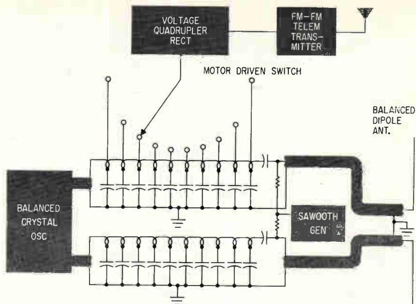
FIG. 1—Impedance measuring system consists of an r-f oscillator, dipole antenna and two artificial transmission lines
