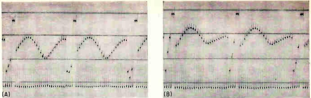
FIG. 7—Record at 7.2 Mc (Aerobee 150 IGC No. AA3.183C): normal standing wave (A) taken at 65 seconds, and abnormal standing wave (B) taken two seconds later. Fig. 8 shows corresponding impedance changes
