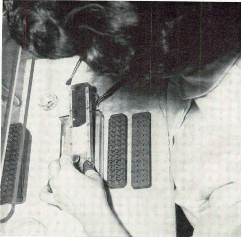
*Alloy pellets being loaded into top of squeeze plate. Pellets fill holes as they roll down plate behind sliding metal block*
