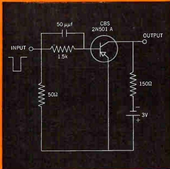
IN THIS NEW CIRCUIT, CBS 2N501 and 2N501A transistors achieve delay, rise, storage and fall times of 2.0, 3.7, 3.2, and 2.3 ns respectively.
