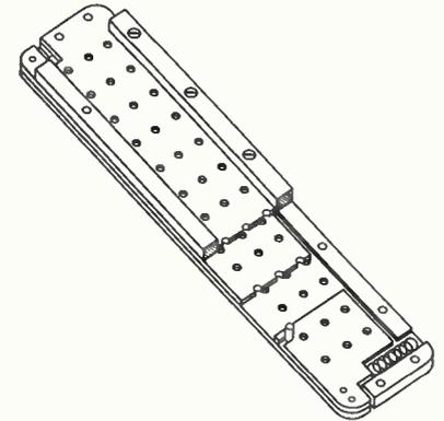
*Cutaway sketch of pellet loader. Holes in the three plates line up when fixture is squeezed*
