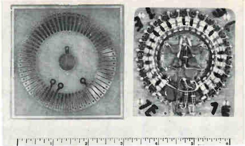
FIG. 3—Twenty-four section commutated line (right) is constructed on a sixty-section printed circuit commutator plate (left)
