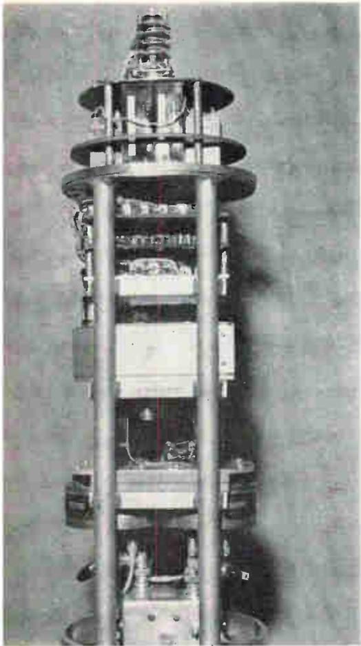
Impedance probe instrumentation for Nike Cajun rocket (Air Force Cambridge Research Center)
