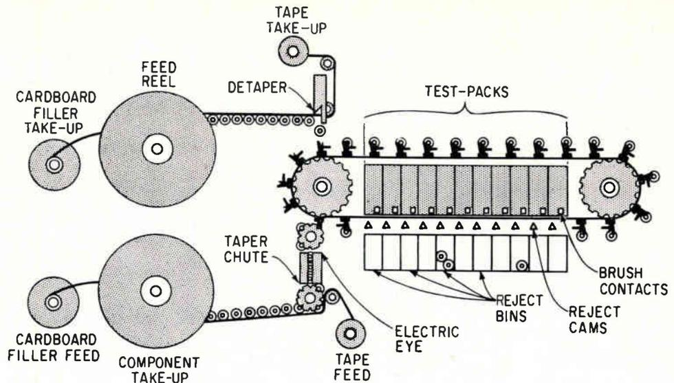
designed for in-line movement by a nylon conveyor belt. The conveyor is indexed in 3-in. increments by an 8-stop roller-gear indexing unit. The conveyor is driven by a 1-hp variable-speed drive coupled by a clutch and brake to the index unit.
