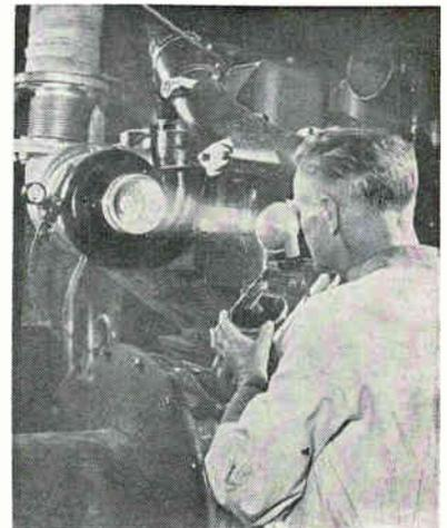
General Radio Strobotac checks running speed of turbo supercharger on diesel engine at Atlas Polar Co., Toronto. Twelve-blade turbo fan rotates at 42,000 rpm. Using Strobotac at 21,000 rpm, a stationary pattern is obtained
