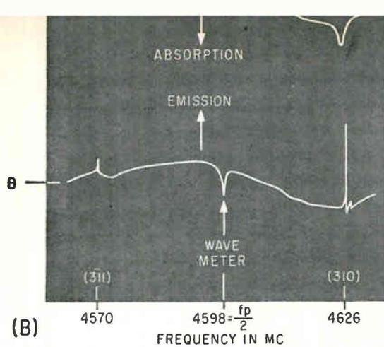
FIG. 3—Developmental design of ferromagnetic parametric amplifier (A), and the effect of longitudinal pumping on a pair of magnetostatic modes (B). Curve A is without pumping; curve B is with pumping
