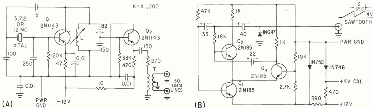
**FIG. 2**—Circuits used in standing-wave detector: oscillator (A) develops an r-f signal of one volt rms into two balanced transmission lines; generator (B) develops the linear sawtooth signal (shown) that is applied to antenna elements
