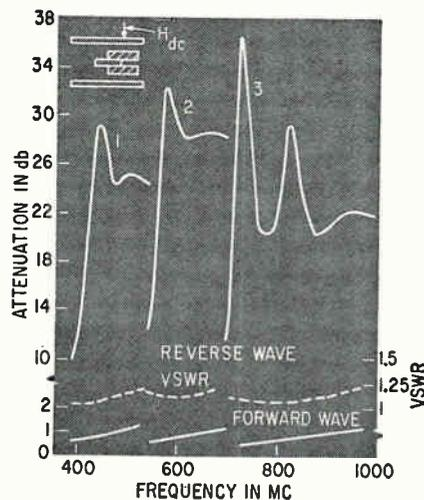
FIG. 5—In the isolator depicted, upper left, curves 2 and 3 resulted from a small change in position of the same YIG slab; for curve 1, slab was in the same position as for curve 3, but was thicker by a factor of 1.5
