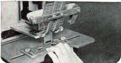
With Dynasert machines, components may be loaded into a self-feeding raceway from card-type packages or fed from a reel. It is no longer necessary to handle components manually.
