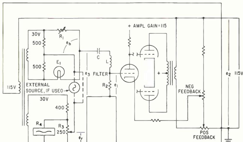
FIG. 1—Thermal regulating bridge using ballast tube operates in power oscillator to maintain output voltage constant
