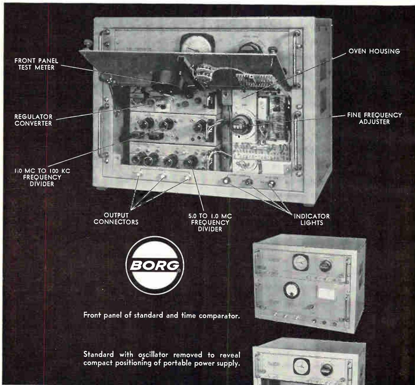
Front panel of standard and time comparator.
