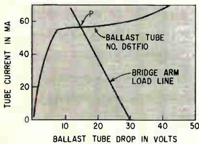
FIG. 2—Ballast tube has required characteristic for application
