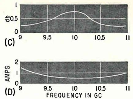
FIG. 4—Tetrahedral junction switch (A) from Caswell Electronics. When nonenergized, insertion loss is high at all points of the normal waveguide operating band (B); minimum insertion loss with current optimized (C); and current required to minimize insertion loss (D). In this switch, energy not transmitted is reflected rather than absorbed
