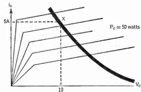
Suppose that we desire to measure the DC current gain at point X. A steady state voltage of 10V and a current of 5A would be required. If conventional DC biases were used, 50W of input power would have to be dissipated by a very large heat sink or auxiliary cooling, such as forced air.
