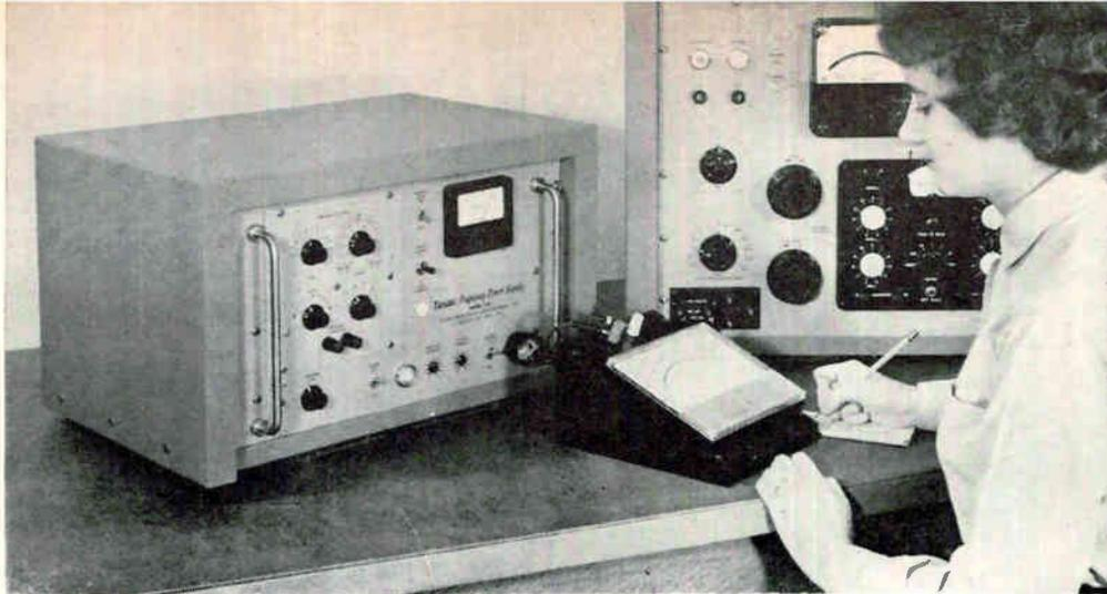
Operator calibrates instrument using precision variable frequency power supply
