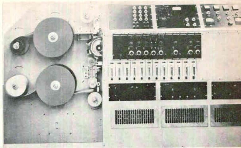
Manual diode tester (left) checks 1,200 diodes per day while automatic tester (right) checks up to 18,000 diodes per day
