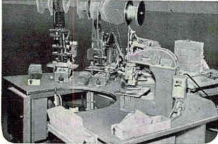
Long or short runs, Dynasert saves. Automatically feeds component, trims, bends leads, inserts, and clinches without damage to component body. Speeds model changeover. Improves board dependability.
