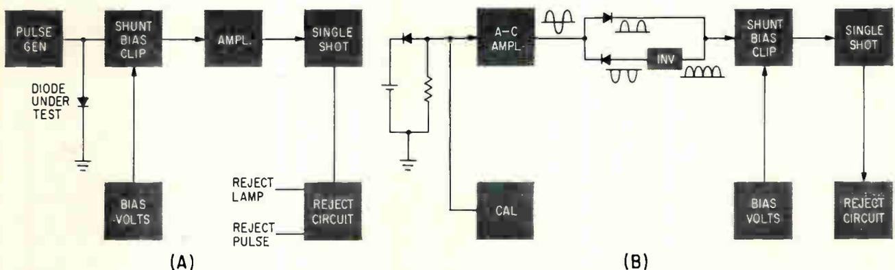
FIG. 4—Forward recovery circuit (A) compares pulse voltage drop across diode with preset reject voltage. Flutter tester (B) measures a-c component of fluctuating d-c produced by diode and battery in series
