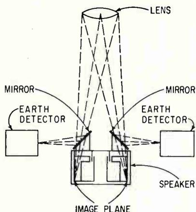
FIG. 1—Relative pulse durations from oppositely located indium antimonide detectors depend on earth's position with respect to optical axis
