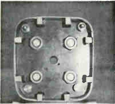
Parts located in welding fixture (top view)
