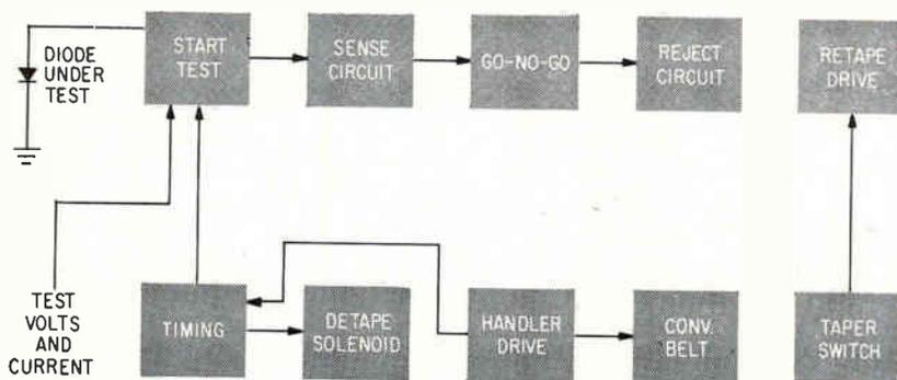
FIG. 2—Start test, sense and go no-go circuits are elements of a typical test pack. Remainder of circuits are used in all tests
