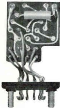
**TIME DELAY RELAYS.** This optional output, off-the-shelf line is made with precision printed circuit construction. Includes time delays on release and time delays on operate—in a timing range of 100 milliseconds to 60 seconds. Available with fixed or adjustable timing to meet your most critical requirements. And they're all 100% inspected during manufacture to insure highest reliability! Bulletin TD-200.
