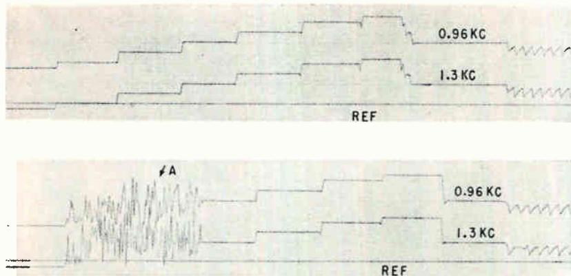
FIG. 3—Recordings of performance tests for water depth of 1,200 feet, with projector at 14-foot depth. Range 1,200 yards, hydrophone at 85 feet depth (top); range 1,300 yards, hydrophone at 130 feet (bottom)
