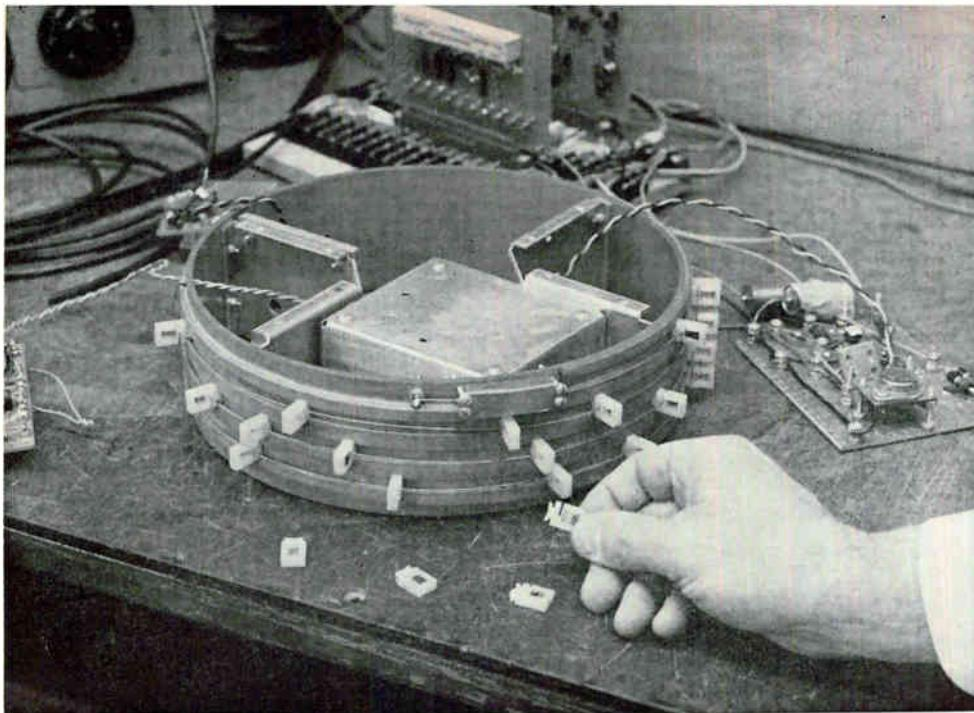
*Prototype of digital function generator showing magnet attachment*
