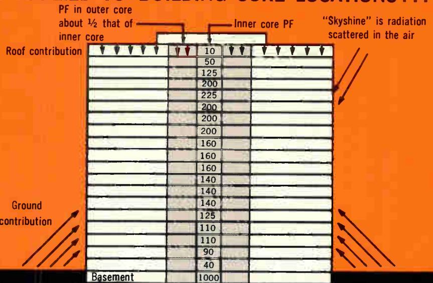
RADIATION SOURCES that must be considered are roof, ground and "skyshine". Don't overlook contribution from adjacent roofs and building setbacks. Note high PF areas in office building shown are within core on upper floors and basement. Structure studied has a steel-frame, concrete floor arches, masonry exterior walls, having 50% openings
