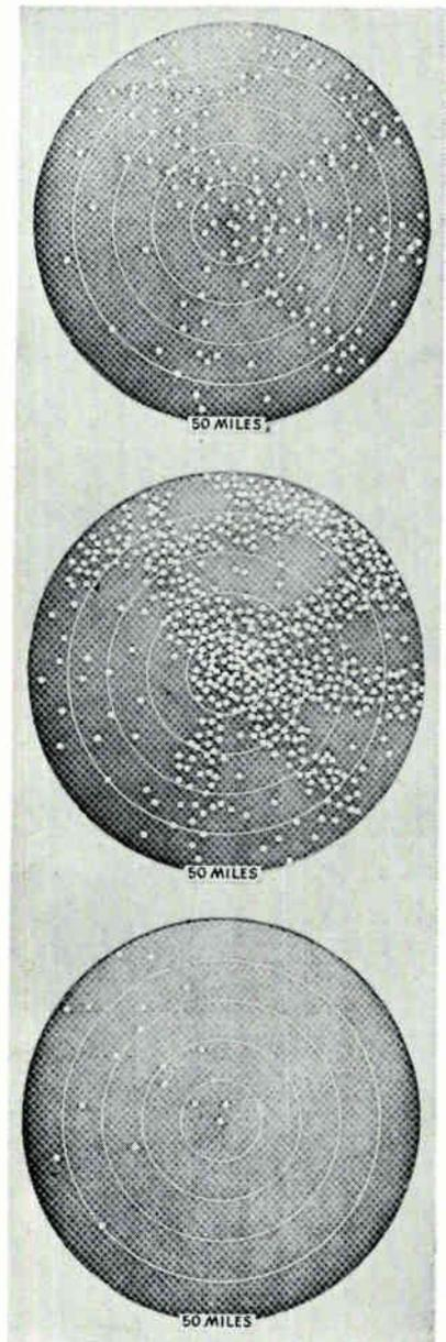
*Congested air traffic now clutters radar displays (top). Scopes will be filled with targets by 1975 (center) unless some method like separating targets into altitude layers is used (bottom), as is done by stacked-beam operation of proposed system*
