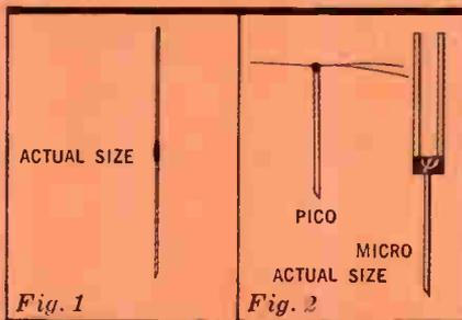
The solid-state packaging employed for protection from extreme environments used for the micro-diode was also employed for the pico and micro-transistor. Until recently, few steps had been taken by the industry to standardize on microminiature semiconductor package outlines. The smallest diode outline is still the DO-7 outline. Progress has been
