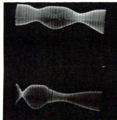
FIG. 4—Amplitude modulation of the 40-Kc carrier, which is extensive at close ranges (100 to 300 yards)
