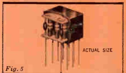
Micro-diodes and micro-transistors were designed for use in this type of packaging. Three leaded components with leads all coming out one side or radially are not particularly suited for this type of assembly, since the leads are usually used to support the structure.
