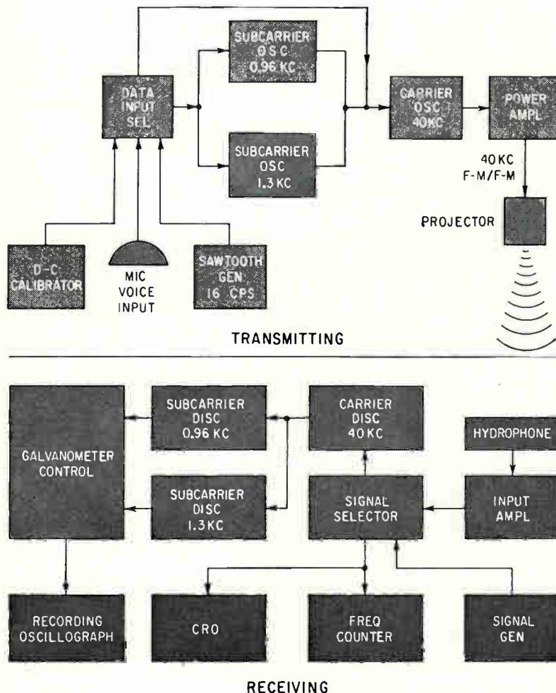
FIG. 2—Block diagram of f-m/f-m underwater telemetry system
