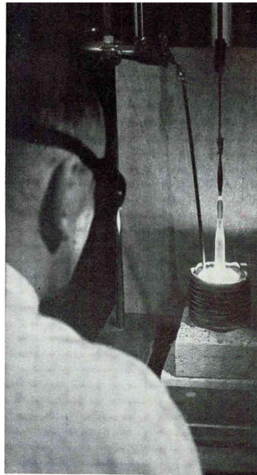
*Crystal was grown by Czochralski technique. It is composed of calcium tungstate with trivalent neodymium*
