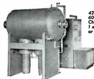
42" Dia. x 60" Long Chamber for  $1 \times 10^{-6}$  Torr or Lower
