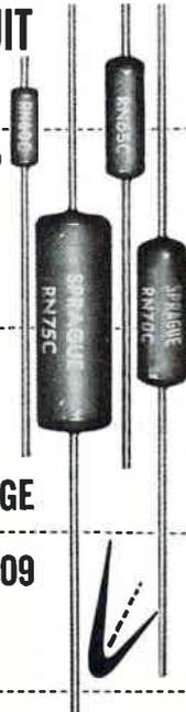
Providing close accuracy, reliability and stability with low controlled temperature coefficients, these molded case metal-film resistors outperform precision wirewound and carbon film resistors. Prime characteristics include minimum inherent noise level, negligible voltage coefficient of resistance and excellent long-time stability under rated load as well as under severe conditions of humidity.
