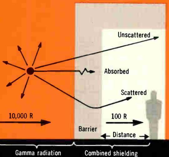
PENETRATING POWER of gamma radiation through a barrier depends on energy level of fallout components, density and thickness of barrier. No material, regardless of density and thickness, completely blocks radiation
