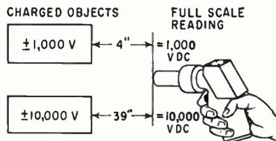
FIG. 2—Static gun indicates voltage of charged objects
