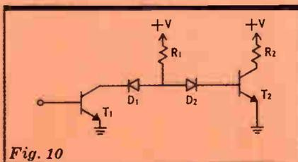
$T_1$  is initially "on" and current through  $R_1$  is steered through  $D_1$ . When  $T_1$  is turned off the current is steered through  $D_2$  to the base of  $T_2$  turning  $T_2$  "on".
