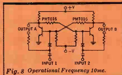
Fig. 8 Operational Frequency 10mc.
