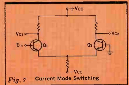
Fig. 7 Current Mode Switching
