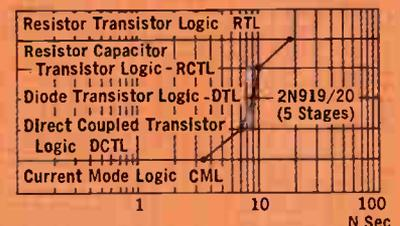
Propagation Delay Time vs Circuit Configuration Fig. 8
