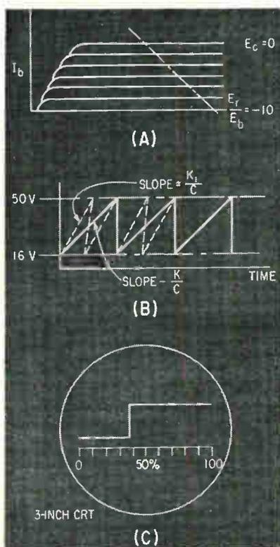
Pentode tube operates on flat portion of characteristic to provide constant current (A); linear voltage rise achieved with gas triode (B); presentation of the LDR data on face of 3-inch crt (C)
