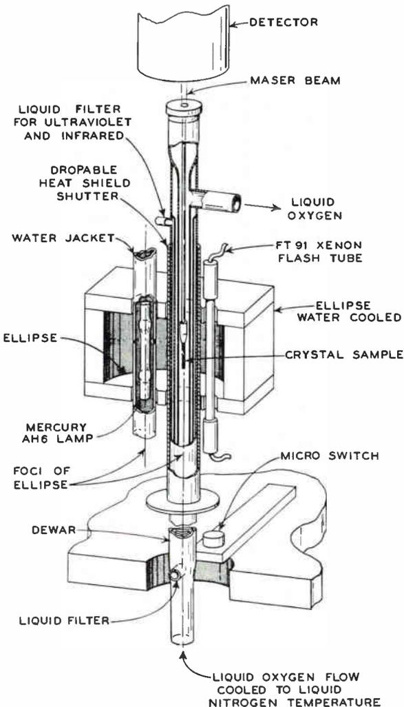
*Liquid coolant and optical filter surround crystal rod. Ultraviolet light is useless and tends to degrade the crystal*
