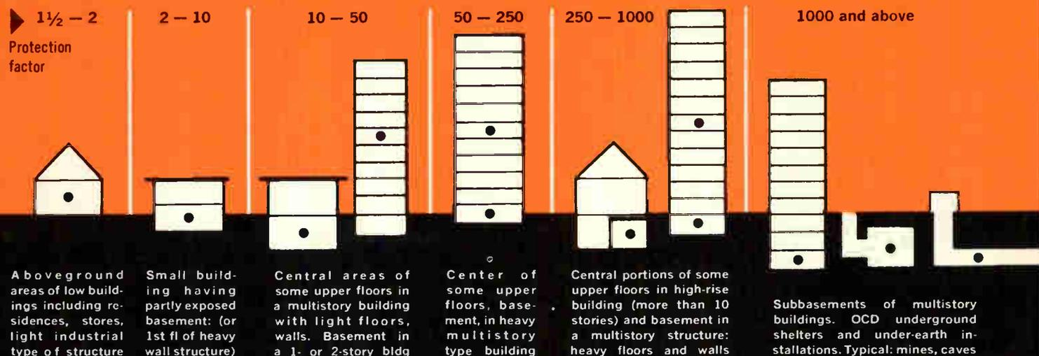
rial and few windows and doors. Some degree of safety would be available, for example, in sub-basements, basements, centers of masonry buildings. You could thicken existing walls if necessary, and concrete baffles could be placed a few feet or so in front of windows and doors to screen out radiation while leaving them in service. To further guard, primarily against roof fallout, you could erect false ceilings using supported concrete planks.
