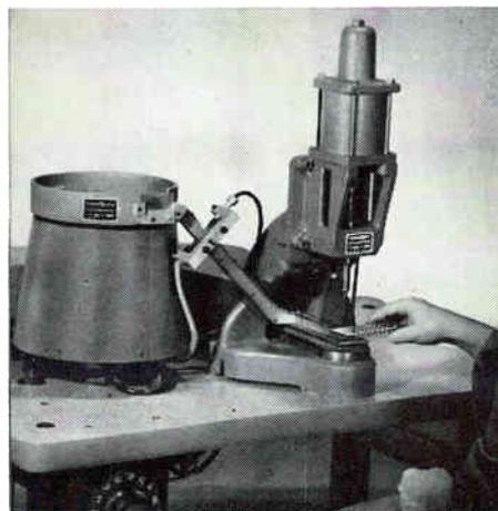
**LONG RUNS: Model FST-1** — raceway-fed, for split-lug, feedthrough, and other terminals. Up to 4200 per hour. All electric. (Model FST Automatic Terminal Setter, not shown, a tube-fed model, achieves even faster production rates.)
