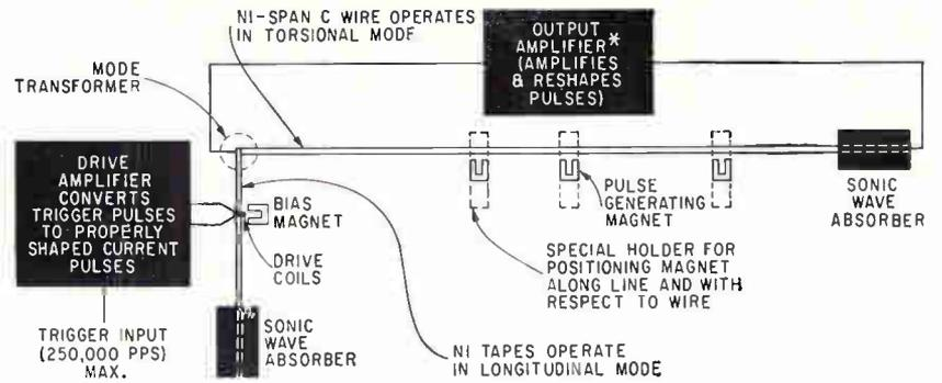
Variation of torsional magnetostriction delay line uses small magnets to replace control taps. Because of nonloading by the magnets, a large number of taps equivalent to one bit may be used with one common output
