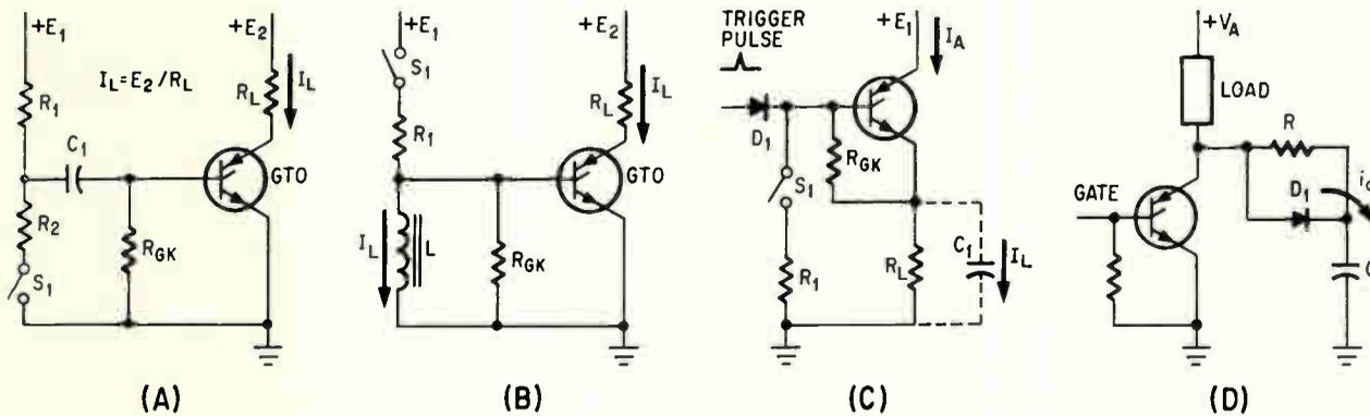
Four turn-off methods for controlling the GTO. Device may be turned on and off by charging and discharging a capacitor in series with gate lead (A). Turn-off is achieved by interrupting d-c current in inductor between gate and cathode (B). Load impedance is connected between the GTO's cathode terminal and ground (C). Use of capacitor C allows higher anode current switching by diverting part of the anode current (D)
