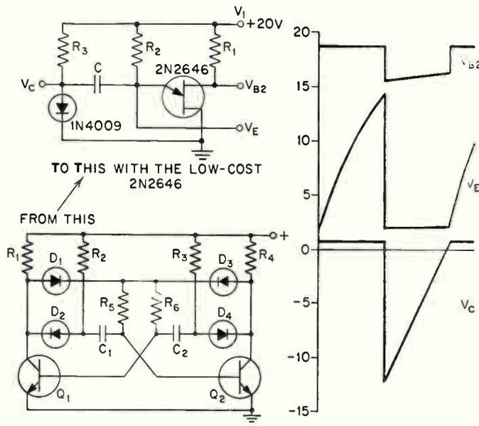
LOW-COST MULTIVIBRATOR WITH OUTPUT WAVEFORMS
