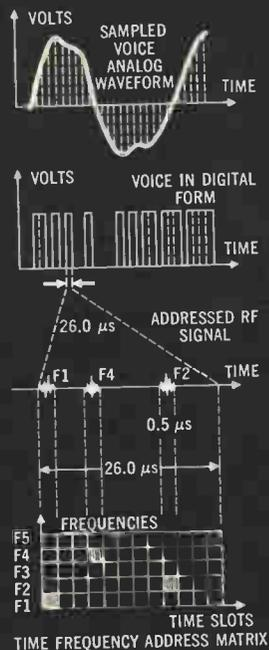
\*RADEM (Random Access Delta Modulation) principle diagramed above is the result of 5 years of independent Motorola research.
