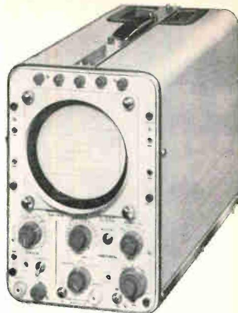
The type 247-A oscilloscope fully qualifies as a universal instrument because its performances and the size (13 cm (5") dia.) of its C.R. Tube authorize accurate measurements and tests in all fields of low-frequency instrumentation. Also, because of its simplicity of operation, the 247 A is ideally suited for practical laboratory work of an educational nature.
