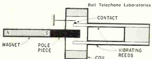
How the tuned relay works
