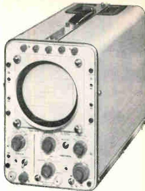
The type 247-A oscilloscope fully qualifies as a universal instrument because its performances and the size (13 cm (5") dia.) of its C.R. Tube authorize accurate measurements and tests in all fields of low-frequency instrumentation. Also, because of its simplicity of operation, the 247 A is ideally suited for practical laboratory work of an educational nature.
