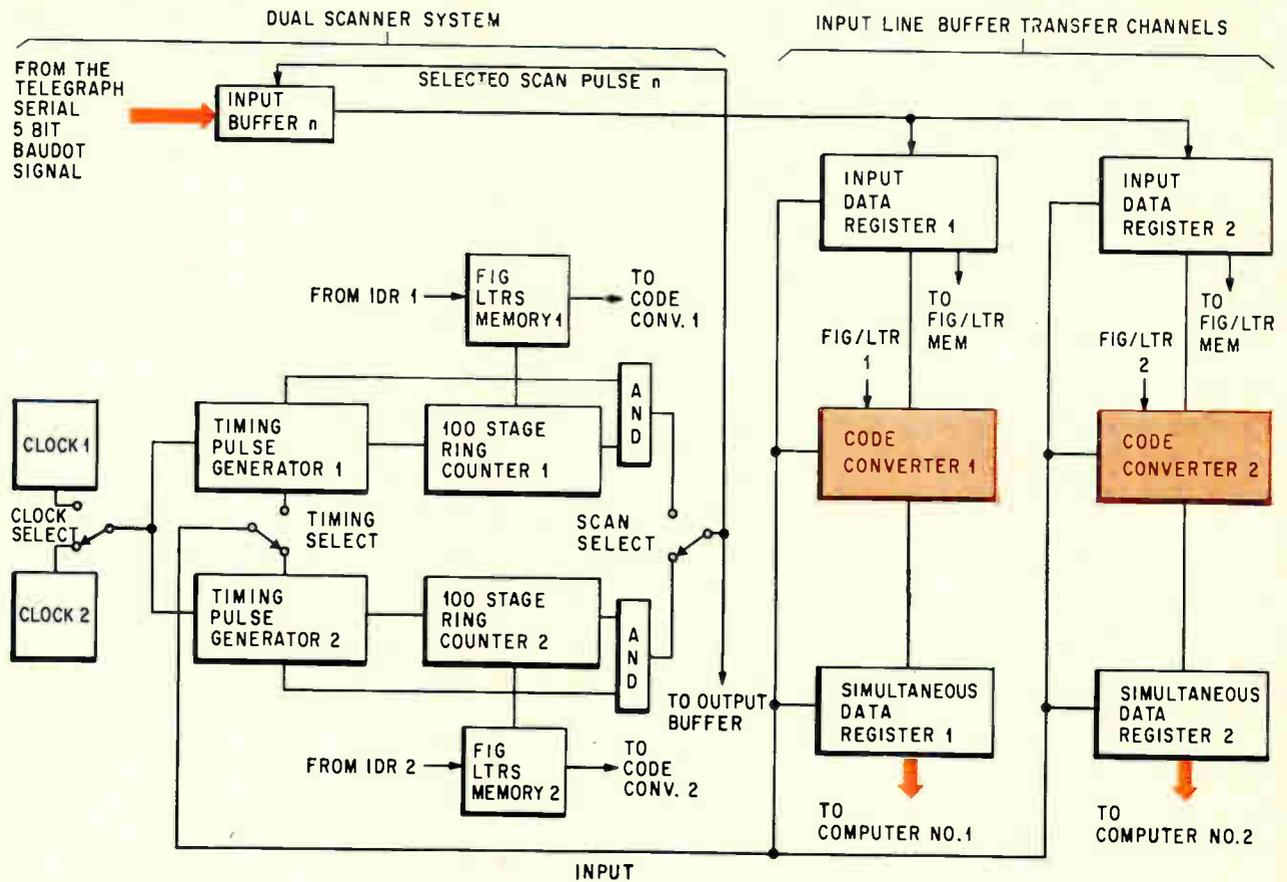
Input block diagram (left) shows special features of the electronic telegraph system front-end design. Incompatibility between conventional teleprinter signaling code and
