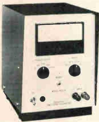
will be read out and registered on the 4½-in. rectangular panel meter. The registered transient will be displayed indefinitely until manually reset or until a higher amplitude transient is registered. There is no threshold nor preset voltage level to be exceeded before a transient will be registered and a one-shot transient can be measured.
