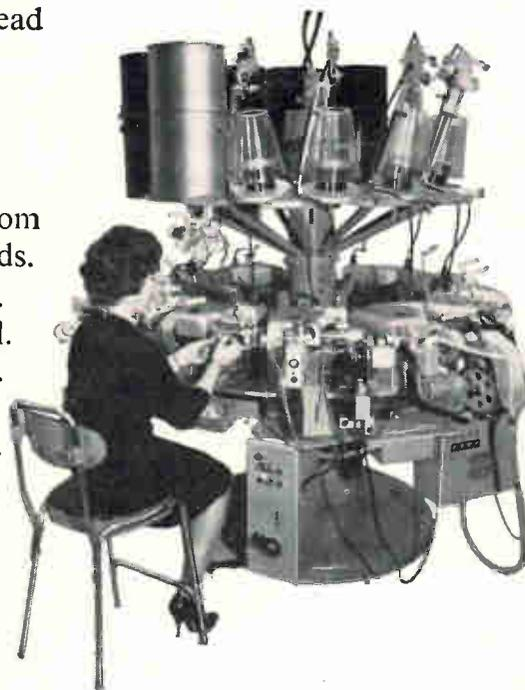
At 7250 turns, No. 39 single formex wire, 585 coils per hour is a typical production rate reported by prominent manufacturers who use the No. 116. Operator merely loads bobbin on arbor of individual head as table rotates, and clips starting lead. Production can be cycled to operator's loading time by controlling clockwise table rotation from  $\frac{1}{4}$  to 2 rpm. Winding speed of each head can be set according to number of turns desired. Write Leesona Corporation, Warwick, Rhode Island.
