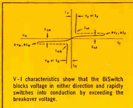
V-I characteristics show that the BiSwitch blocks voltage in either direction and rapidly switches into conduction by exceeding the breakover voltage.
