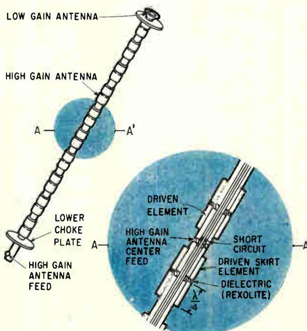
High-gain antenna is 10-element series fed collinear array of stacked dipoles; low gain antenna is a discone type fed by a coaxial line through the center of the high gain antenna
