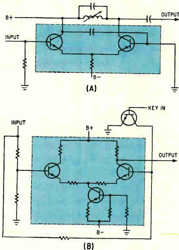
Receiver requires external adaptive circuits (A) for the 30-Mc amplifier stage. The suppressed carrier double-balanced modulator (B) has achieved a carrier rejection of 40 db. MICs are in color
