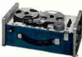
Shown above with the Model 14 rechargeable Power Pack, the Model 110 offers standard 2-speed drive over a range of 1 1/2 to 30 ips, with 3-speed ac and 4-speed dc available. With optional converter, the model 110 easily operates from 12v dc, in addition to the standard 28v dc or 117v ac. 1/4", 1/2" or 1" tape widths accommodate 2, 7 or 14 standard IRIG channels respectively. Inter-
