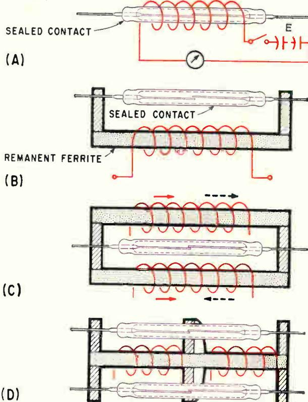
Four ways to operate a high speed miniaturized reed relay
