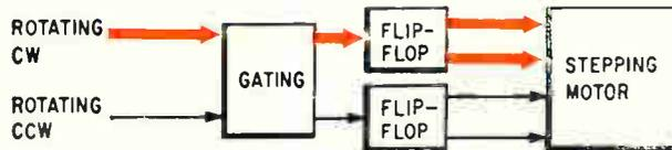
Output actuators which are actually digital, such as this stepping motor control, need no memories as do analog pneumatic valve actuators
