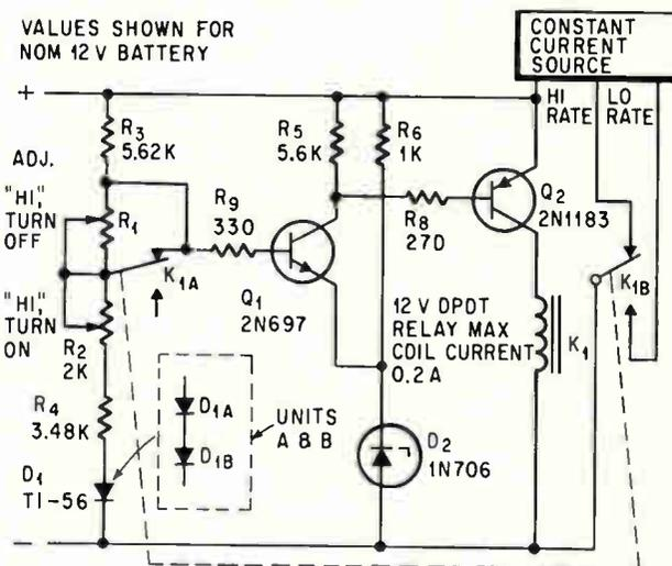
After system primary power is restored, this controller recharges batteries in 20 hours, provides trickle charge
