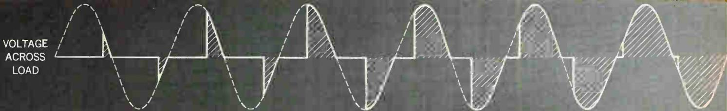
The newest member of Transistron's BiSwitch family, the 11/16" stud-mounted TBS40AS, handles up to 20 amperes at 125 volts. It gives direct full-wave AC phase control of 2.5 KW. And no AC to DC converters or variacs are needed. It permits high power control circuitry that is simpler, more reliable and more economical than ever before possible.
