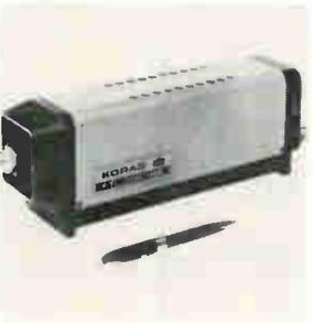
Yttrium aluminum garnet laser K-Y1 has a c-w output of 3 w. Emission is at 1.06 microns with a half-angle beam divergence of 2.5 milliradians at threshold. Power supply is housed in a  $10 \times 10 \times 20$  in. cabinet. The laser head is  $4 \times 4 \times 12$  in. Applications include trimming of resistors, real-time data display. Korad Corp., 2520 Colorado Ave., Santa Monica, Calif. [385]
