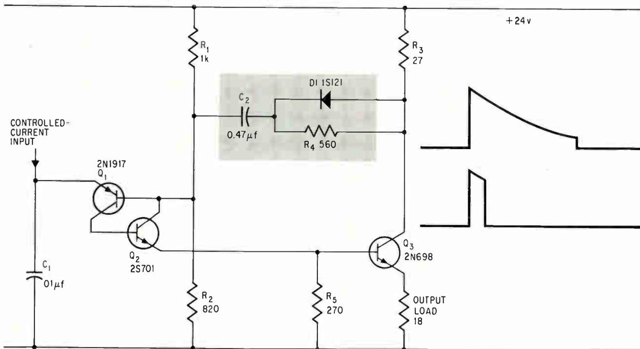
**Pulse generator.** Feedback network between pulse-circuit output and avalanche-switching input, formed by Q<sub>1</sub> and Q<sub>2</sub>, permits trailing edge of output pulse to be shaped. Exponential decay in the trailing edge of pulse output is unwanted. With a sharp decay the trailing edge triggers or controls other circuits.
