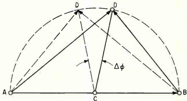
Vectors. Voltage that is proportional to the source-drain resistance of the FET is represented by vector  $DB$ . Output of network is a vector that is constant in amplitude and represented by  $CD$ .
