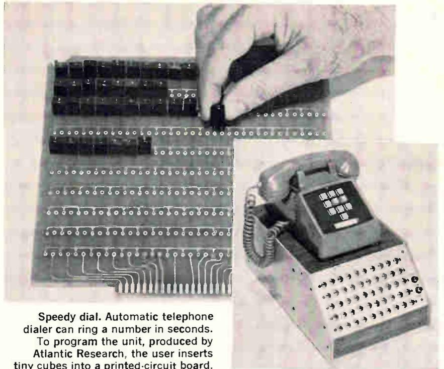
Speedy dial. Automatic telephone dialer can ring a number in seconds. To program the unit, produced by Atlantic Research, the user inserts tiny cubes into a printed-circuit board.
