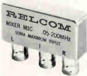
Double-balanced mixer M1C is for critical circuit functions of a-m with suppressed carrier, pcm, ppm, phase detection, and frequency converting in communications and test equipment. It has a noise figure of 5.5 db (ssb) at 50 Mhz, 45-db isolation between ports at 200 Mhz, and conversion loss of 5 db (ssb) at 50 Mhz. Relcom, 2329 Charleston Rd., Mountain View, Calif. [405]
