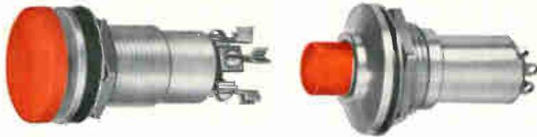
Four models, one with wide button. Choice of two and four circuit momentary, plus DPDT push-push. Ratings of 1 to 10 amps at 28 vdc; 1 amp at 120 vac.
