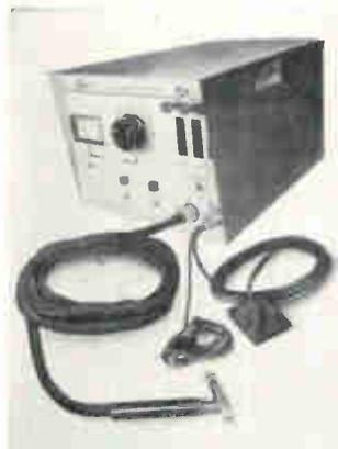
LINDE PWM-4 plasma needle arc welder—a complete package, including power supply/control unit designed for bench mounting. Uses conventional power and water supplies. Foot switch provides on-off arc control; 10-ft. service line connects torch to control unit.
