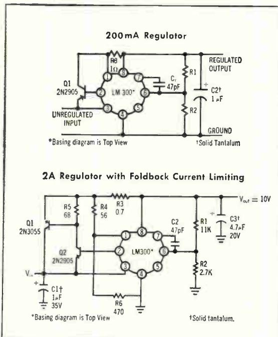
For \$3.60 in 1000 lots you can now simplify your power distribution problems with our new LM-300. It's a plastic TO-5 version of the LM-100. It operates over a temperature range of 0°C to 70°C with output voltage adjustable between 2 and 20 volts.
