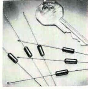
Hermetically sealed, glass-case silicon rectifiers series G have avalanche characteristics for protection from reverse voltage transients. Rated at 1 amp at 55°C, they have piv ratings from 200 to 1,000 v. Max. operating temperature is 175°C. Size is 1/8 X 1/4 in. Prices range from 20 to 46 cents in quantities. Sarkes Tarzian Inc., 415 N. College Ave., Bloomington, Ind. [442]
