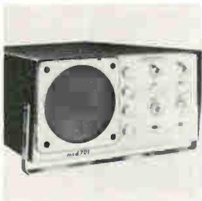
An X-Y monitor, Transi-Scope 701, uses solid state components and IC's. Specifications for the vertical and horizontal amplifiers include: deflection sensitivity of 10 kilohms, 1 kilohm, 100, 10 and 1 mv/major division with a vernier adjustment of X1 to X10 minimum; amplifier response of d-c to 1 Mhz ( $-3$  db). Measurement Control Devices Inc., 2445 Emerald St., Philadelphia, Pa. [369]
