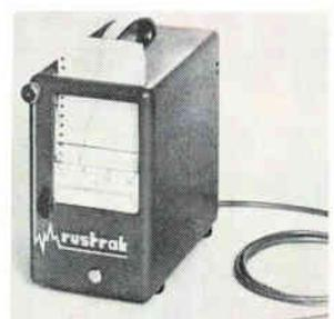
Environmental monitor model 166 uses a dry-writing method for a continuous, permanent record of temperature across  $-50^\circ$  to  $+100^\circ$  C range, with an accuracy of  $\pm 1.5^\circ$  C. The chart speed of 1 in/hr provides a 31-day record with standard 63-ft, style B, 75-division paper. The unit measures  $5\frac{3}{8} \times 3\frac{3}{8} \times 5\frac{7}{8}$  in. Rustrak Instrument Co., Municipal Airport, Manchester, N.H. [368]
