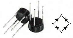
1 amp EBR. For printed circuit board mounting.
