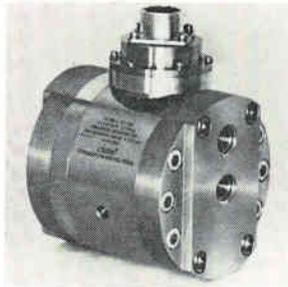
Unidirectional differential-pressure transducer PL385TC is capable of direct exposure to either gas or fluid corrosive pressure media on active or reference ports. Typical pressure ranges are from 0-5 to 0-50 psig. Differential overload is 5,000 psig. and max. allowable internal pressure is 6,000 psig. Price is \$500. Statham Instruments Inc., 12401 West Olympic Blvd., Los Angeles 90064. [362]
