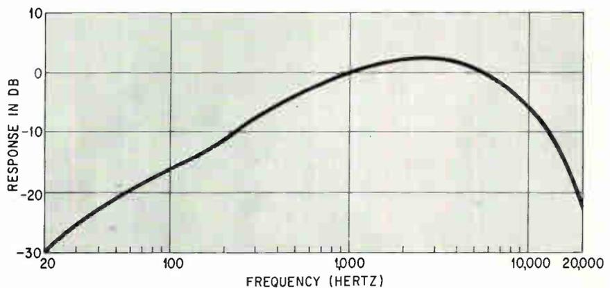
**Impressive performance.** Frequency response of new head is 10 kilohertz at -6db, with a playback speed of 3¾ inches per second. In addition, crosstalk rejection, which is even a more critical parameter in auto recorders than in home units, is greatly improved, to 80 db.
