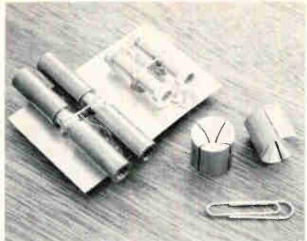
**Tuning slugs.** Applications versatility is indicated by the pair of resonators on the board at the left. Device with large tuning sleeves resonates at 300 hz, the lower end of the voice band. An identical device, but with small tuning collars, operates at 3,000 hz, the upper end of the band. Cylindrical objects are acoustic resonators; transducers haven't yet been placed on their webs.
