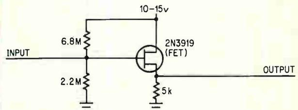
**Matching circuit.** Piezoelectric transducers are high-impedance devices. Field effect circuits like this will match Twintron outputs to low-impedance loads.
