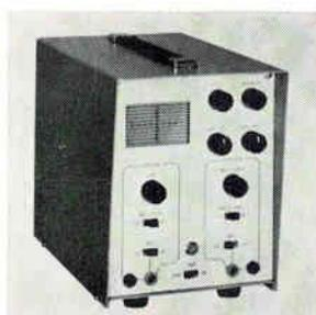
Solid state oscilloscope DM-4 is designed for the communications field. With the FM-9 frequency meter/deviation meter/signal generator, the unit presents the complete deviation picture. Alone, it serves to trouble-shoot audio circuits and to compare frequencies. Unit measures  $6\frac{1}{4} \times 8\frac{1}{2} \times 10$  in. Price is \$295. Gertsch Division, Singer Co., 3211 S. La Cienega Blvd., Los Angeles. [367]
