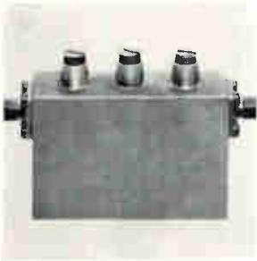
Tunable, coaxial bandpass filters series FBM span 960 Mhz through 6 Ghz in 2, 3, and 4-section combinations. They can be used as preselectors; to provide rejection for image frequencies in receiver front ends; and to eliminate harmonic or spurious signals from an oscillator multiplier chain. Prices start at \$150. Applied Microwave Dynamics Corp., 287 Sherman Ave., Newark, N.J. [401]
