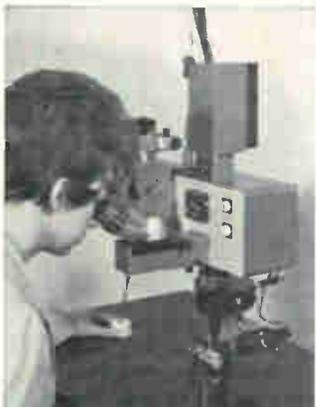
The LINDE LWM-1 is easy to use. The 25:1 ratio micro-manipulator makes precise positioning a simple operation. The binocular viewer in combination with a turret arrangement of three objective lenses gives a continuous view of the weld area at 20, 40 and 100 power of magnification. A shutter protects the operator at the moment the weld is made. LWM-1 adapts readily to automated welding and digital tape controls.
