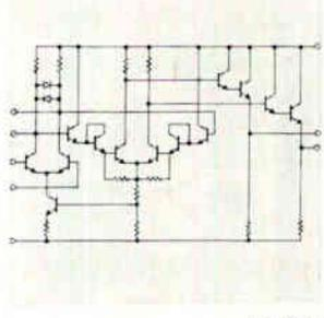
Differential amplifier model SE515 is a linear IC featuring differential input and output, an input-offset voltage of 0.5 mv, and compatibility with commonly used logic-circuit power supplies. It is offered in two operating ranges; -55° to +125°C, and 0° to +70°C. The former costs \$15 for 100 and up; the latter, \$4.75. Signetics Corp., 811 E. Arques Ave., Sunnyvale, Calif. [443]
