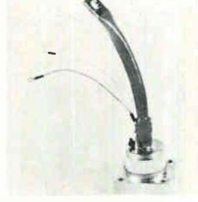
Thyristors in the CR7K series offer surge ratings of 7,000 amps and rms current of 770 amps from a pair in inverse parallel. These cells will replace ignitrons as the SCR is smaller and can be mounted in any position. Arc volt drop and triggering time are reduced by a factor of 20, and power requirement of the gate is 5 w peak. Calvert Electronics International Inc., 220 E. 23d St., N.Y. [438]
