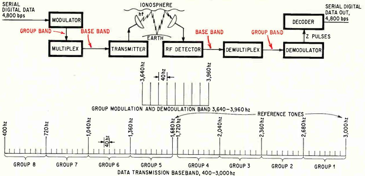
**Multiplexing.** Each group of eight data characters is first modulated in the groupband, 3,640 to 3,960 hz, and then multiplexed down to the voice, or baseband. The process is reversed at the receiver.
