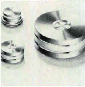
Three series of fast-recovery silicon rectifiers are in flat-button form. The TR series is rated for 20 amps at 100°C case temperature. The RU series handle 40 amps and the RD units 200 amps. Both TR and RU have 500-nsec recovery times; the RD, 700-nsec recovery time. Piv ratings are from 50 to 1,000 v. Electronic Devices Inc., 21 Gray Oaks Ave., Yonkers, N.Y. 10710. [436]
