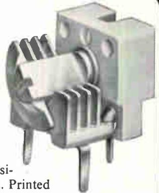
2. Cut costs with new, Johnson RIB-LOC™ Tip Jacks that save production line time with *press-in* design. No mounting hardware to assemble or handle. Simple insertion tool presses Tip Jack into pre-drilled chassis hole for a secure mount that resists loosening and turning. Jack accepts 0.080" tip plug in a recessed, closed-entry type contact. Insulating body is molded of low-loss polyamide. Brass solder terminal is silver-plated and Iridited. Low cost.
