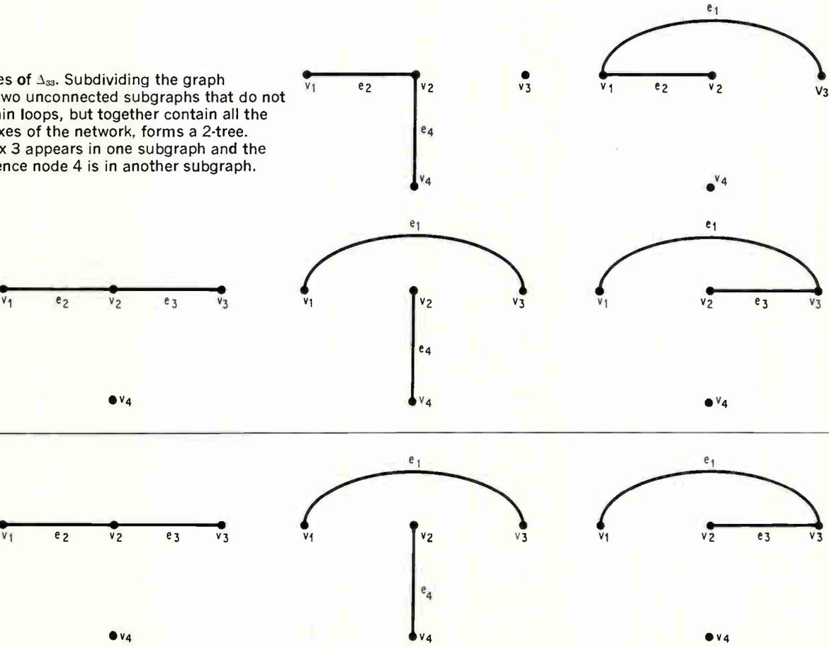
a two-part subgraph containing nodes  $i$  and  $j$  in one connected subgraph and the reference node in the other.
