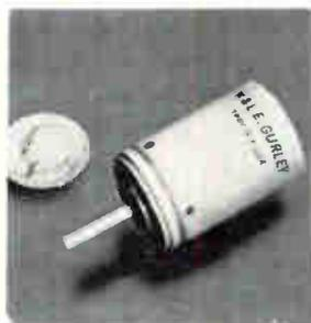
Incremental, photoelectric rotary encoder 8610 is housed in a synchro size 11 package. It is suited for use in computer and process control equipment, and aerospace guidance systems. The unit incorporates GaAs light sources for maximum reliability from  $-55^\circ$  to  $+100^\circ\text{C}$  and shock in excess of 50 g. Accuracy is  $\pm 1$  minute. W.&L.E. Gurley, Troy, N.Y. 12181. [382]
