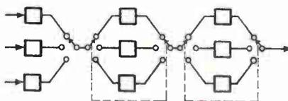
the system fails. Furthermore, the switches can also be arranged to permit any three of the nine to perform the system's function.
