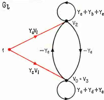
**2** Flow graph. By writing the network equations and arbitrarily labeling each with a different unknown the analyst forms the flow graph. Loop sets are then drawn by following the procedure outlined on page 85.
