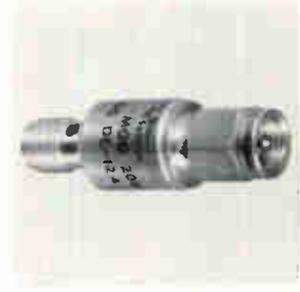
Fixed attenuators series 20600 operate from d-c to 12.4 Ghz. Standard models are available in values of 3, 6, 10, and 20 db with tolerances of  $\pm 5\%$  for attenuation values of 6 db or greater. All models are 3/8 x 1 1/4 in. Vswr is 1.20 max from d-c to 4 Ghz and 1.35 max from 4 to 12.4 Ghz. Price is \$80 each. Omni-Spectra Inc., Hallwood Ct., Farmington, Mich. [404]
