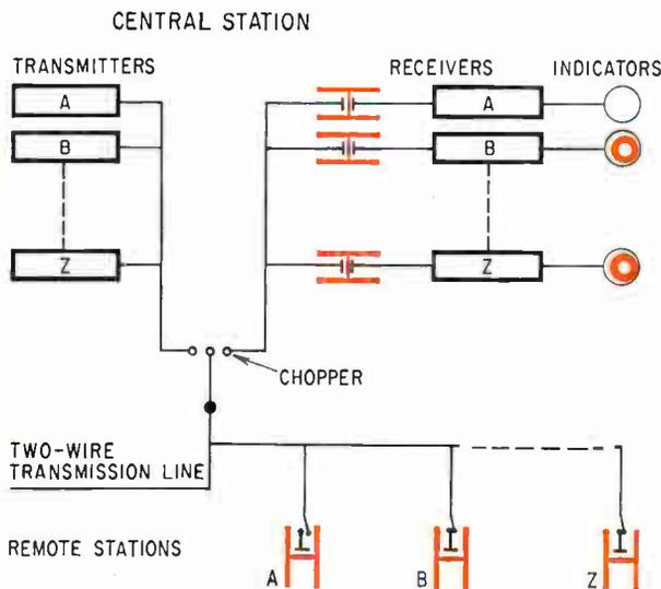
**Echo system.** Basic passive monitoring setup echoes the transmitted tone when the switch is closed at a remote station.
