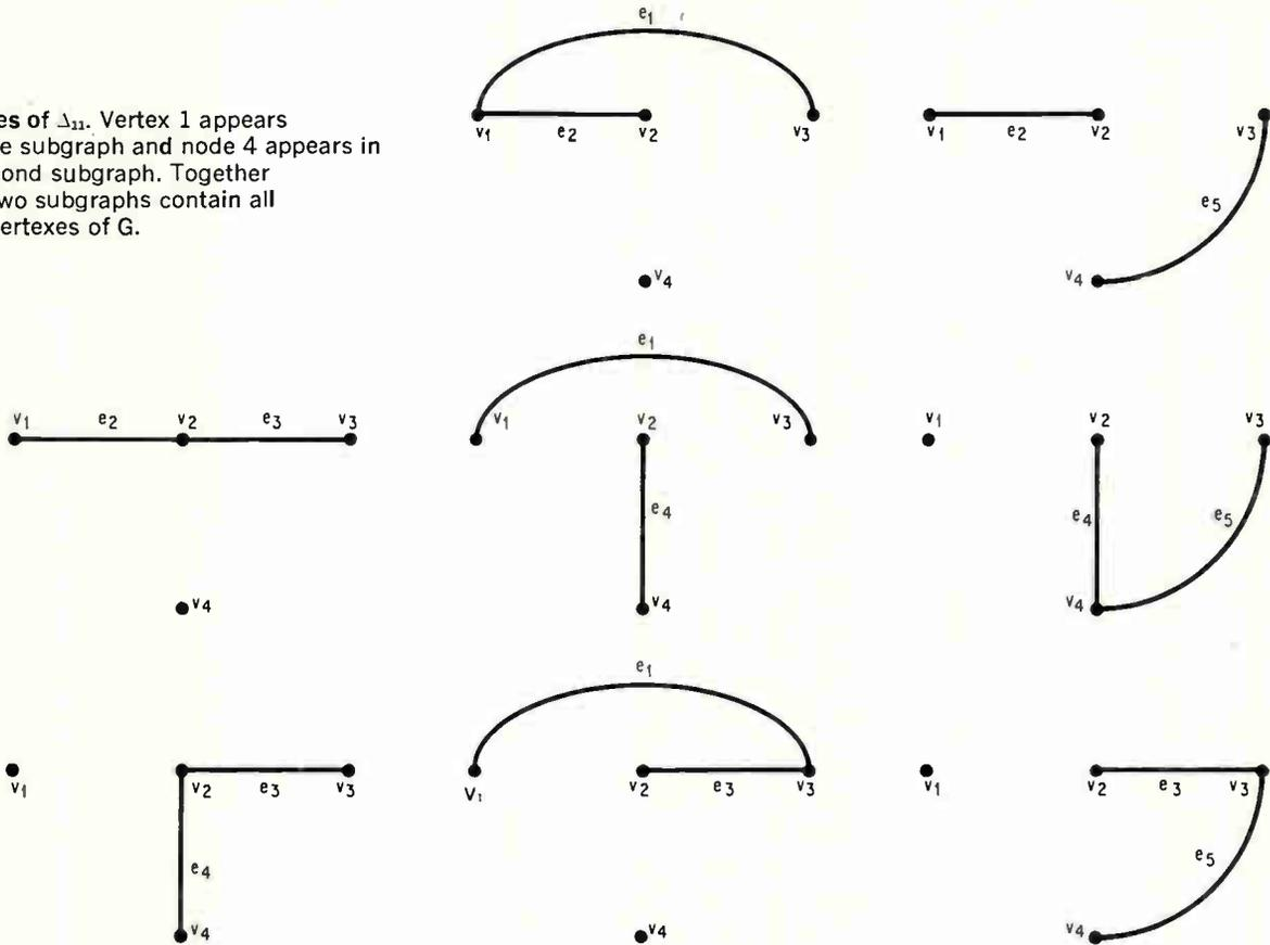
2-trees of  $\Delta_{33}$ . Subdividing the graph into two unconnected subgraphs that do not contain loops, but together contain all the vertices of the network, forms a 2-tree. Vertex 3 appears in one subgraph and the reference node 4 is in another subgraph.
