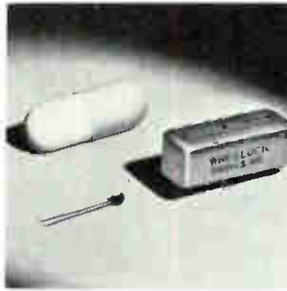
Reed relay series 442SS with built-in solid state driver occupies only 0.05 cu in. Typically, 40 2-pole relays with their driver stages can be mounted on a 4½ x 5½ in. p-c board with adequate spacing between boards. Height is only 0.25 in. Contact is rated at a full 7 w. Units are available in 1-to 4-pole models. Wheelock signals Inc., 273 Branchport Ave., Long Branch, N.J. [350]
