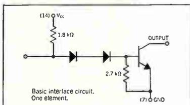
Radiation's Monolithic Diode Matrices and Interface Circuits form a compatible family of integrated circuits to implement any logic design. These circuits perform the AND, OR, and INVERT logic functions. In combination they provide the AND/OR, NAND/NOR and expandable NAND/NOR logic functions. These circuits are compatible to all logic families, RTL, DTL, T<sup>2</sup>L and CML.
