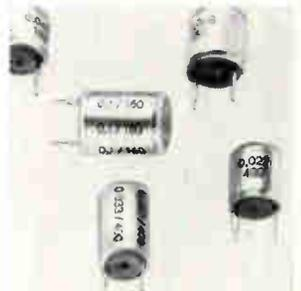
Miniature capacitors type V170 are constructed by wrapping the film dielectric with a synthetic film and thermally sealing the end. They may be subjected to 100% relative humidity for 72 hours at 75°C and suffer not more than 1/3 loss in insulation after exposure and subsequent drying. Capacitances range from 0.01 to 0.1 µf. Aerovox Corp., New Bedford, Mass. [356]
