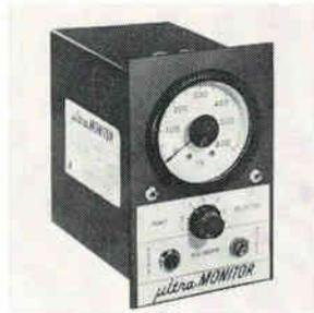
The ultraMonitor reads out any temperature point that can be sensed by a thermocouple. Used with standard thermocouples, the unit, with a  $5\frac{1}{2}$ -in. meter scale, is better than 2% accurate. It may be used with a thermocouple in parallel with other equipment because of its high input impedance that almost eliminates additional loading. Airborne Accessories Corp., Hillside, N.J. [363]
