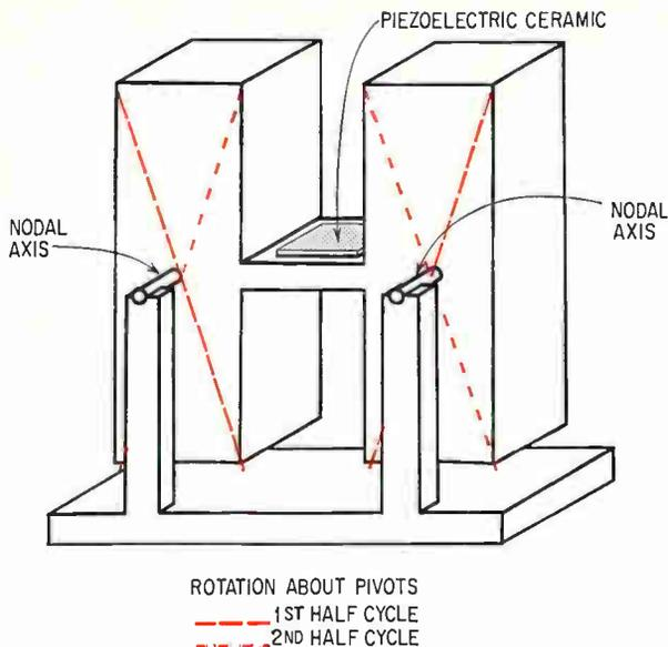
**Push-pull.** As the piezoelectric input transducer contracts and expands, the web flexes and the bars oscillate in opposing directions. The resonance signal can be picked off by a coil near a bar or by another piezoelectric transducer underneath the web.
