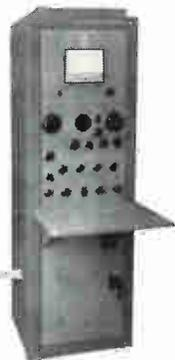
Used to measure dissipation and capacitance of electric insulating material while subjected to high-voltage stress. From these two measured values and the dimensions of the sample and test electrodes, dielectric constant, loss factor, and other values may be calculated.
