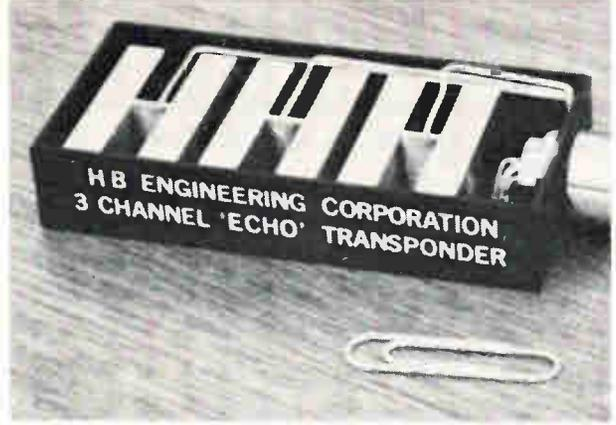
**Close quarters.** Their immunity to vibration enables several resonators to share a housing. The photo above shows a three-channel transponder for the echo system; at the left is a four-channel transponder for the passive remote telemetry system.
