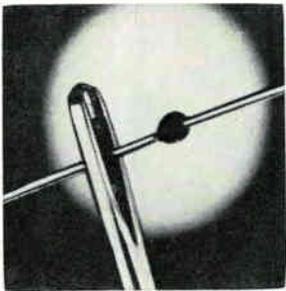
Microminiature zener diodes are electrically interchangeable with standard Jeced types. Measuring 0.075 in. in diameter and 0.125 in. long, the MTC series are encapsulated in high-temperature epoxy. Standard units cover the voltage range of 5 to 12 v. They have either silver leads or gold plated, weld ribbon type. Computer Diode Corp., Pollitt Dr. South, Fair Lawn, N.J. [440]
