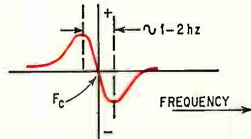
**Discriminator.** Out-of-phase transducers help f-m discriminator produce a large change in output when a small shift in frequency occurs.
