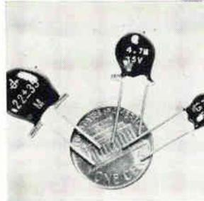
Dipped epoxy, solid tantalum capacitors series G come in 3 case sizes ranging from 0.47  $\mu$ f/50 v to 150  $\mu$ f/6 v. Maximum moisture protection is offered without costly hermetic sealing. The stand-off lead functions as a stress relief during handling. Prices range from \$1.65 to 32 cents in quantities of 1 to 999. Dickson Electronics Corp., Box 1390, Scottsdale, Ariz. [347]
