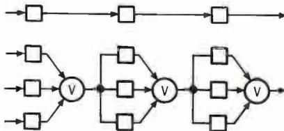
tical modules in series. One well-known method, called triple modular redundancy, or TMR, extends
