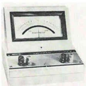
Power factor meter model 83 measures input frequencies ranging from 50 to 2,500 hz. It has an accuracy rating of  $\pm 1\%$  of total span with sine-wave inputs of 120 v and currents ranging from 1 to 5 amps. The meter is self-energized from the voltage input and produces direct readings for leads or lags of up to  $90^\circ$ . Weston Instruments Inc., 614 Frelinghuysen Ave., Newark, N.J. [366]
