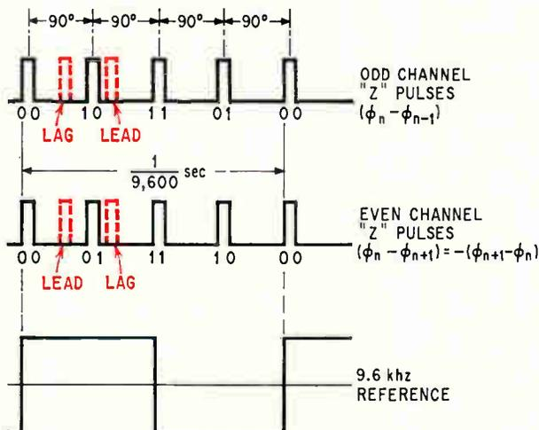
**Pulse decoding.** The phases of the output "Z" pulses correspond to the original data characters. The pulses, however, may be shifted from their undisturbed positions due to transmission delays. Shifts are in color.
