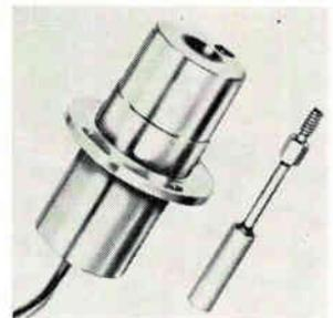
Linear position transducers series 230 are 60-hz units that provide infinite resolution. They are available in 20 different models with range of travel from  $\pm 0.010$  to  $\pm 4$  in. Units feature sensitivity to 100 mv/mil and linearity to 0.05%. A wide variety of standard mounting options simplifies installation of core and case. Robinson-Halpern Co., 5 Union Hill Rd., West Conshohocken, Pa. [364]
