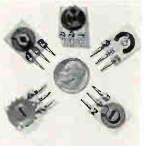
Trimmer resistor named Slim-Trim is useful in consumer, military and industrial equipment. Rated at ¼ w per section at 70°C, it has resistance values ranging from 100 ohms to 15 megohms. Maximum voltage is 350 v. The unit is built upon a base plate of alumina for heat dissipation. Centralab Electronics Div., Globe-Union Inc., 5757 N. Green Bay Ave., Milwaukee, Wis. [353]
