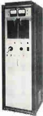
Type PA variable high voltage AC breakdown testers are designed to meet the requirements of ASTM specification D-149, and Federal specification LP-406, Method 4031, as well as all general purpose breakdown testing. Provided with motor-driven control of output voltage with any desired rise of secondary voltage. Available with wide variety of testing jigs.
