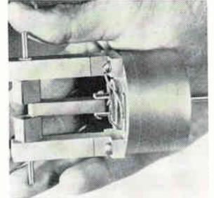
A d-c reciprocating motor consists of a copper-wound piston operating in an annular permanent air gap. The piston connects to a rotating shaft through a push rod and crank, and connects directly to an axial linear shaft. The motor is brushless, and commutated by an electronic circuit. Operating voltage is from 1.25 to 26 v. Mathews Electronics Corp., 312 S. Broad St., Mobile, Ala. [348]
