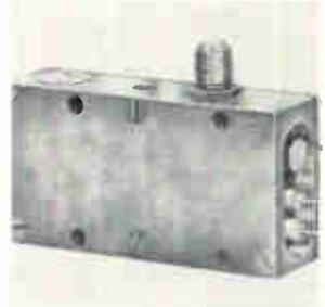
Local oscillator 6009-1100 covers 1.1 to 1.3 Ghz with a manual tuning range of 200 Mhz. Frequency stability vs temperature is 20 ppm/°C at  $-54^\circ$  to  $+71^\circ$ C. Power input requirements are  $-28$  v d-c at 25 ma nominal. Power output is 10 mw minimum. Shock is 100 g, 11 msec, 3 axes; vibration, 20 g peak, 20 to 2,000 hz, 3 axes. Trak Microwave Corp., 4726 Kennedy Rd., Tampa, Fla. [408]
