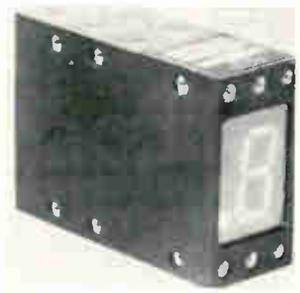
Decade counter model F1850E combines a bright segmented display with a 5-Mhz IC counter. It requires only a single supply voltage of 5 v d-c. Input voltage swing is  $\pm 1$  v. Two outputs are provided to drive other counters. The unit is  $7\frac{1}{8} \times 1\frac{3}{4} \times 2\frac{3}{8}$  in., and weighs 2 oz. Price is \$90 in production quantities. United Computer Co., 930 W. 23d St., Tempe, Ariz. 85281. [388]
