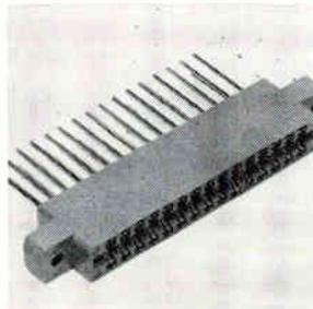
Card-edge receptacle series 6021 has 30 dual-readout or 15 single-readout wire-wrap contacts spaced on 0.156-in. centers. It accommodates a 1/16-in. p-c card. The unit is available with simple-cantilever or double-cantilever bifurcated-nose contacts, both rated at 5 amps and made of phosphor bronze with a gold flash over a nickel underplate. Elco Corp., Wil-low Grove, Pa. 19090. [346]
