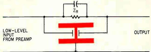
**Rejection filter.** Only the resonant frequency is blocked by this filter. All other frequencies are detoured through the resistor.
