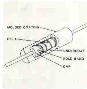
Metal film resistors in the MAF60 series are made by depositing a stable resistive film alloy on a ceramic substrate through a vacuum evaporation process. Units are rated at ¼ w at 70°C and ⅛ w at 125°C. Change in resistance after 1,000 hours load life is less than ±0.5%. Standard temperature coefficient is 100 ppm/°C. Mallory Controls Co., 100 S Parker Ave., Indianapolis. [351]
