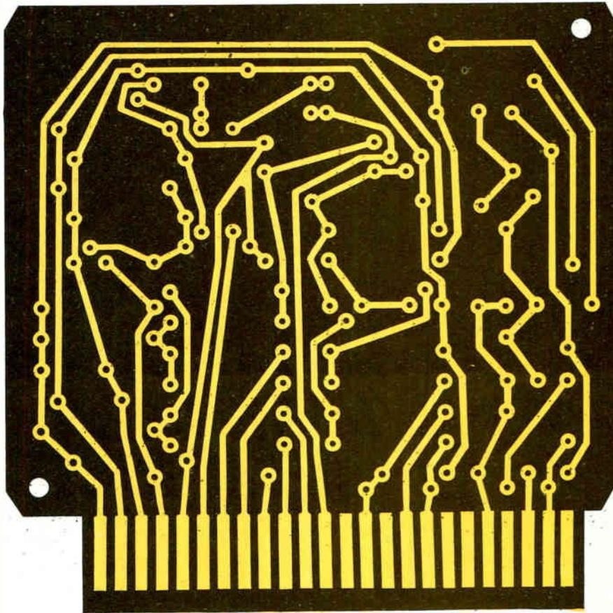
Logic modules are built on printed circuit cards. Hole location and front-to-back registration must be very accurate for machine assembly. **Hand assembly is costly.** Plated thru-holes must provide positive continuity. **Rejects are costly.** Circuit boards for logic modules must be easily solderable. **Poor solderability is costly.** Printed circuit cards must be delivered in volume quantity for large-scale logic module production. **Time delays are costly.**
