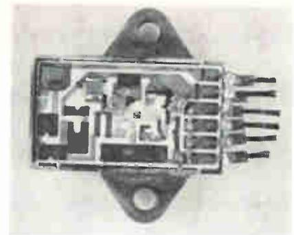
Looking down. Top view of regulator circuit showing hybrid IC configuration.
