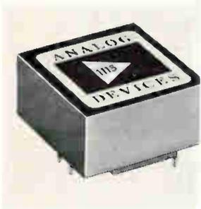
D-c differential operational amplifier model 1115 develops 5 ma output at  $\pm 10$  v. Specifications include 15,000 open-loop d-c gain at full load, 20  $\mu\text{v}/^\circ\text{C}$  max. voltage drift from  $-25^\circ$  to  $+85^\circ\text{C}$ , 200 na max. initial bias current drift, and 1.5 Mhz small-signal bandwidth. It measures  $\frac{1}{2} \times 1 \times 1$  in. Price is \$13 (\$9.75 in lots of 1,000). Analog Devices Inc., 221 5th St., Cambridge, Mass. [381]
