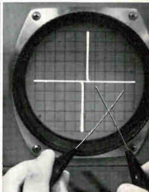
Simplest Switch ever made by man is an active thin film of OVONIC semiconductor material vacuum deposited between two wires. Oscilloscope trace shows inherently symmetrical E-I characteristic. Switching speed is less than 150 picoseconds.
