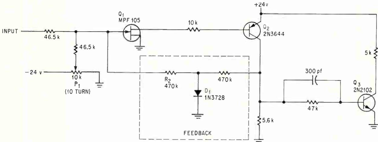
Versatile feedback. Changing the level detector's feedback causes the circuit to behave as an astable, monostable, bistable, or gated oscillator because  $Q_1$ 's gate has a high input impedance, allowing signals to be summed at that point.
