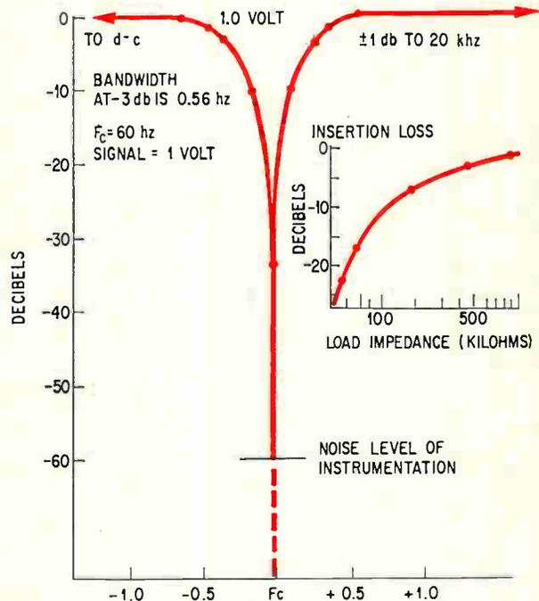
**Hum stopper.** Characteristics of a filter designed for applications requiring the rejection of 60-hz line frequency—the source of 60-cycle hum.
