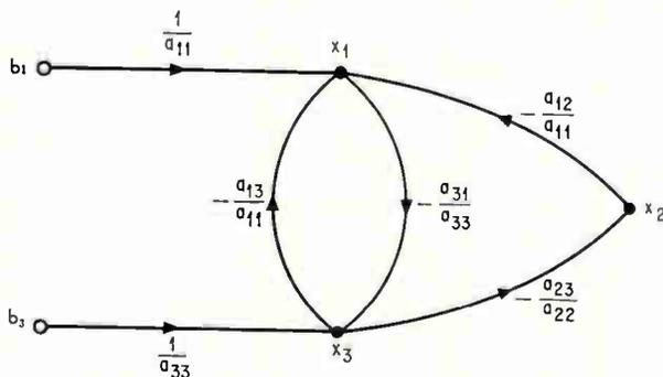
**Superposition.** Because more than one input is applied, the solution for  $x_2$  using signal-flow graphs requires superposition.
