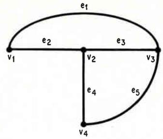
**Trees.** To form the trees of the T-network all nodes are marked and the edges are drawn between the nodes without forming any closed loops.
