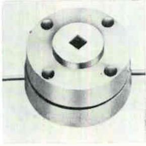
Infrared detector QKN1227 is a mercury-doped germanium unit that responds in less than 100 nsec and is sensitive from 2 to 15 microns. Designed for laboratory, industrial, and airborne use, it detects radiation from carbon-dioxide lasers emitting light at 10.6 microns. The unit measures about 1/2 X 3/4 in. Price is \$2,900. Raytheon Co., Foundry Ave., Waltham, Mass. [441]
