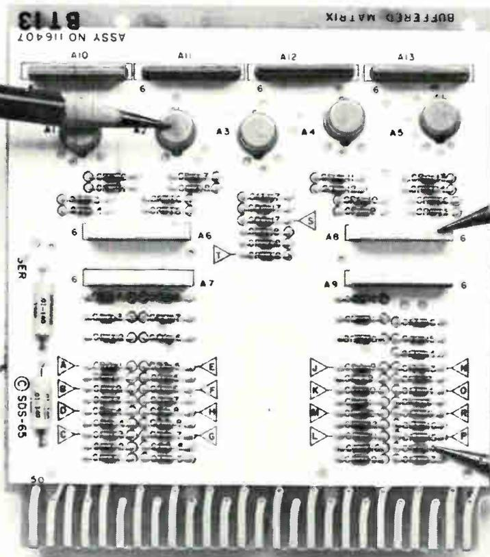
T Series input and load resistors, made to much tighter tolerances than can be attained with integrated components, are mounted outside the integrated circuit containers, eliminating power dissipation problems.
