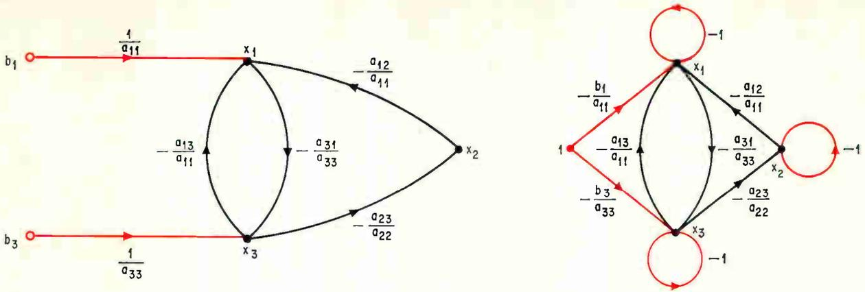
**Graph transformation.** Graph  $G_i$ , right, is formed from  $G_m$ , left, by first adding a self-loop with a gain of  $-1$  to each branch devoid of a self-loop. Then the gain of the branch at source nodes 1 and 3 are multiplied by  $-b_1$  and  $-b_3$  respectively. These are then combined into one source node, labeled 1.
