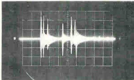
**Multipath.** A single transmitted pulse may be received as a sequence of pulses due to multipath effects.
