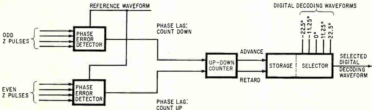
Correcting errors. Time lags in odd-channel pulses are used to sense phase retardation; lags in even-channel pulses are used to sense advances. The counter measures phase error and sets up the digital gating waveform that best accommodates the error.
