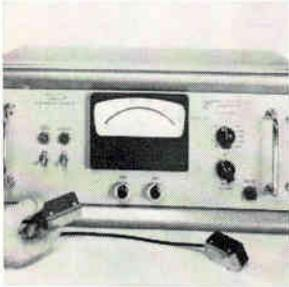
Electrostatic voltmeter model 144 Isoprobe uses a noncontacting  $1\frac{1}{8} \times 1\frac{1}{4} \times 2\frac{3}{16}$ -in. probe to permit drift-free measurement with 0.1% accuracy. Range of  $\pm 1$  to  $\pm 2,000$  v full scale at greater than  $10^{18}$  ohms input impedance allows for many potential applications in general materials research and evaluation. Monroe Electronics Inc., 5 Vernon St., Middleport, N.Y. [361]
