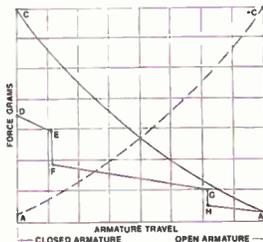
Curve CA—Balanced-Force Relay normally closed contacts.
