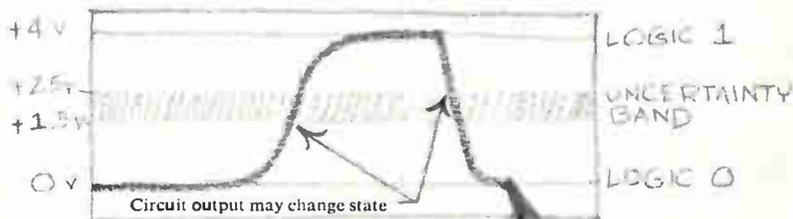
T Series logic levels are 0 and +4 volts, and noise rejection is 1.5 volts minimum, leaving a maximum uncertainty band only one volt wide within which noise can trigger the circuit output. This uncertainty band of 25% is far narrower than those of other I.C. modules on the market.
