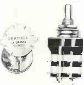
Shorting-contact series 44 rotary switch is available in a 45° angle of throw. It has 1 or 2 poles per deck. The 1-pole unit has up to 6 decks; the 2-pole type, up to 3 decks. Initial contact resistance is 0.005 ohm, rising to 0.020 ohm max after 25,000 cycles of operation. Price is from \$7.70 to \$17.50, depending on poles and decks. Grayhill Inc., 523 Hillgrove Ave., LaGrange, Ill. [354]
