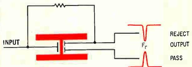
**Both ways.** Two output transducers give a circuit designer the choice of filtering out the resonant frequency, passing it, or both.
