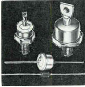
Fast-recovery rectifiers feature 7 current ratings, from 3/4 to 30 amps, and 6 voltage ranges, from 50 to 600 v. More than 50 rectifiers in the series offer 2 reverse recovery speeds of 200 nsec max and 1 μsec max thus providing 2 frequency ranges of 50 khz and 250 khz. Prices (1,000 and up) are 40 cents to \$40.50. Motorola Semiconductor Products Inc., Box 955, Phoenix, Ariz. [437]
