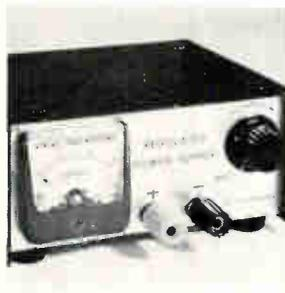
Zener reference, regulated power supply model PZ-131 delivers stable, continuously variable outputs from 0.5 to 25 v at currents to 200 ma. The compact ( $4\frac{1}{2} \times 2\frac{1}{2} \times 4$  in.) unit provides load regulation better than 100 mv, line regulation of  $\pm 30$  mv, and a-c ripple and noise of less than 2 mv at full load. Price is \$34.95. Viking of Minneapolis Inc., P.O. Box 9507, Minneapolis. [387]
