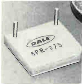
Model SPR-275 is a 21-w resistor designed to isolate line drive impulses and terminate lines within the demanding space requirements of a computer. It has a resistance range of 0.025 ohm to 1 kilohm, within 5% tolerance. Mounted to a heat sink maintained within the computer at 70°C, its maximum temperature on the other side is 100°C at 21 w. Dale Electronics Inc., Columbus, Neb. [349]
