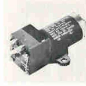
Miniature pressure transducer series P2-5000 combines a precision variable reluctance, twisted Bourdon tube pressure sensor with an integral carrier-demodulator. The series includes models for measurement of gauge, differential, and absolute pressure in ranges from 0-1 to 0-5,000 psi, with  $\pm 0.50\%$  accuracy. Whittaker Corp., 12838 Satcoy St., N. Hollywood, Calif. 91605. [372]
