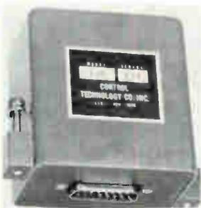
Miniature preamplifier-demodulator-quadrature rejector model 324 accepts 400-hz a-c input signals and converts them to phase-sensitive d-c signals for use in instrumentation systems. Maximum output is  $\pm 20$  v d-c. Effective quadrature rejection ratio is 30:1 minimum. Input impedance is 10,000 ohms. Control Technology Co., 41-46 29th St., Long Island City, N.Y. [386]
