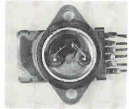
Looking up. Bottom view showing output power transistor in a TO-3.
