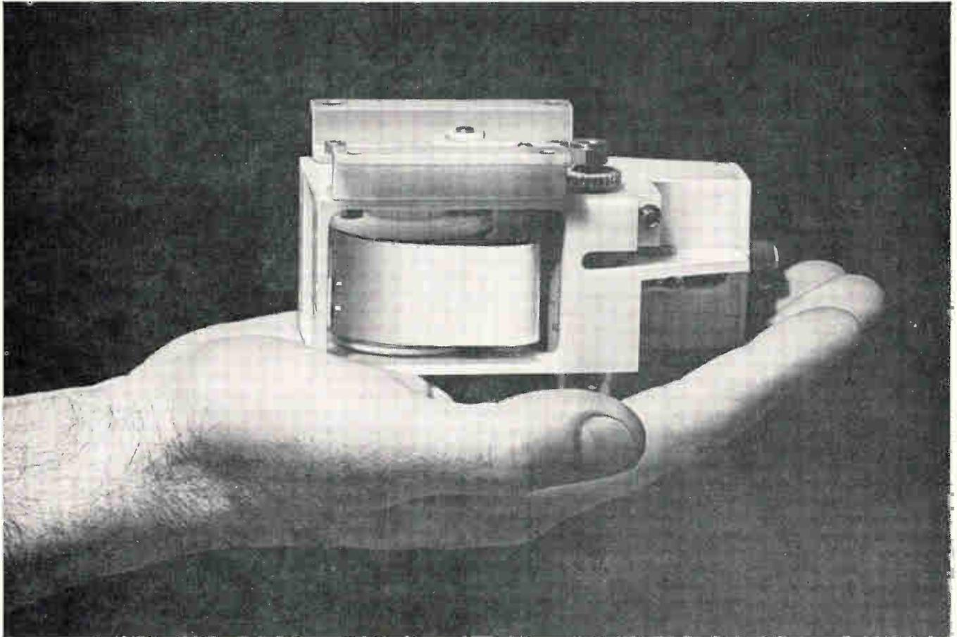
Like the other STEM (Storable Tubular Extendible Member) devices we have developed, it's a strip of specially tempered metal rolled onto a drum.
