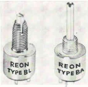
Half-inch-diameter variable resistors with conductive plastic element feature infinite resolution over a 50-ohm to 5-megohm range in sealed units with either standard (type BA) or locking (BL) bushings. Dust-, moisture-, and water-proof to 15 psi, they have an end resistance of less than 5 ohms each end. Reon Resistor Corp., 155 Saw Mill River Rd., Yonkers, N.Y. [345]
