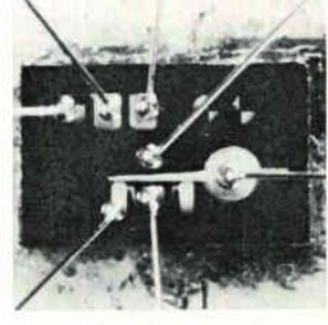
A solid state device called a resonant gate transistor (RGT) is available in evaluation quantities. It is a frequency-selective unit capable of Q's from 20 to 200, and helps solve the problem of building tuned circuits without inductors. Frequency range is presently limited to about 3 to 30 khz. Price is \$67. Molecular Electronics Div., Westinghouse Electric Corp., Elkridge, Md. [439]
