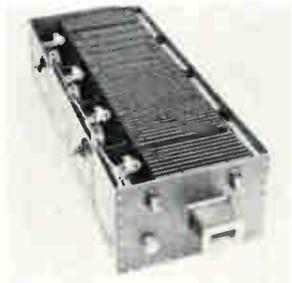
S-band dummy load model WI-A03 can handle 20 kw average power without the use of liquid cooling. It features a built-in forced-air cooling system equipped with an air-flow safety interlock switch. It operates from 2.7 to 3.3 Ghz, and has a max. vswr of 1.20. The unit can withstand an internal pressure of 45 psig. Microlab/FXR, Ten Microlab Rd., Livingston, N.J. 07039. [406]
