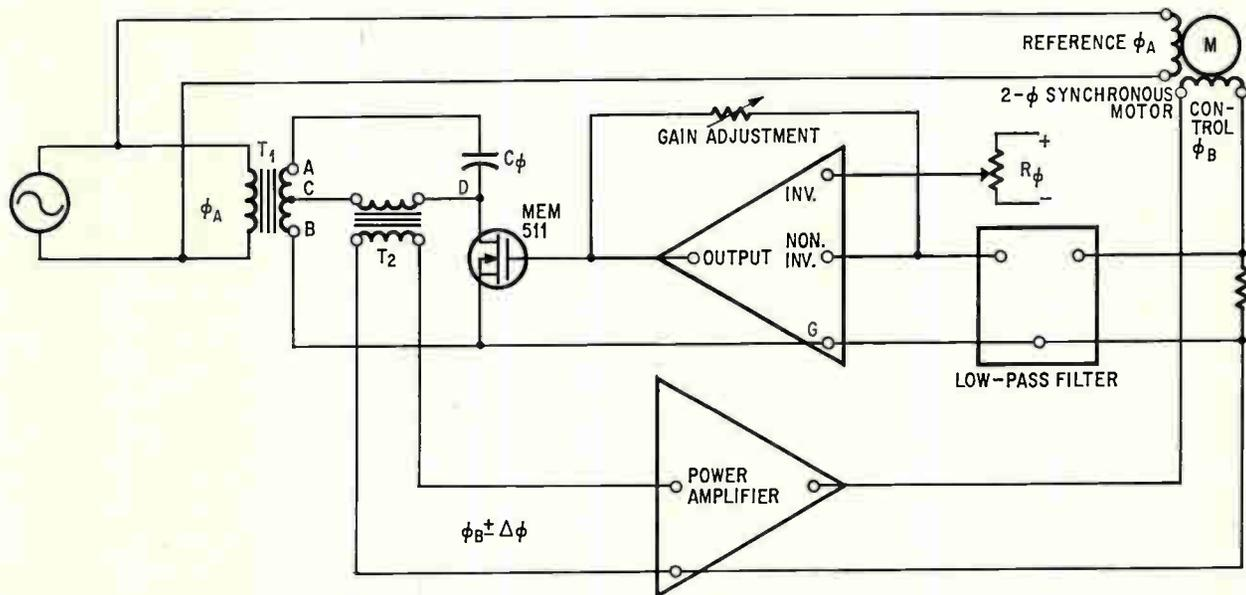
Servo loop. MOS field effect transistor serves as variable resistor in phase-shift network. Output is fed to motor winding to reduce hunting.
