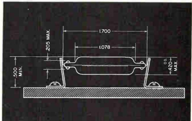
Automobile dome lamps have long employed the cartridge lamp shown at the top. It was a good lamp but it was bulky and had cemented-on end caps for contacts. Also the fuse-clip type mount was comparatively expensive to make.
