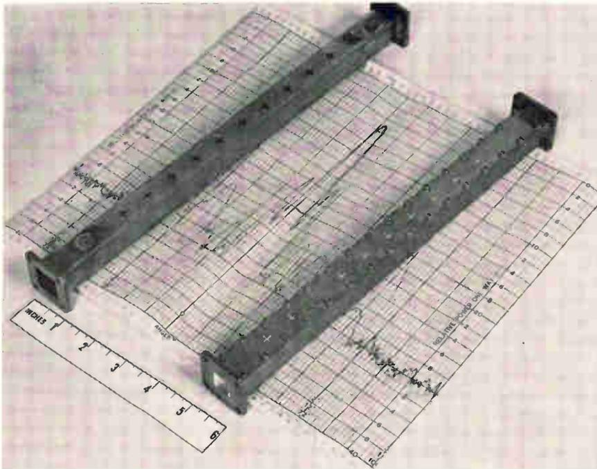
**Broad look.** Waveguides for Aeronutronic's new side-looking radar, developed for the Army, may be used by the space agency. Strip chart shows typical antenna spike pattern—decibels compared with radiated beam width.
