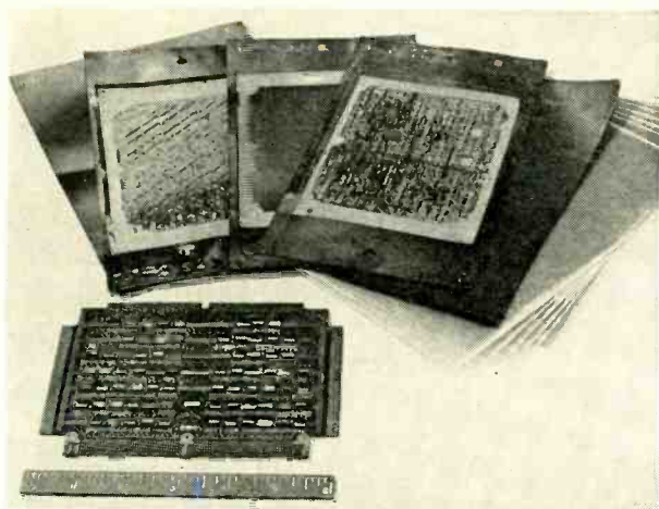
Multilayer boards raise interconnection density by increasing the amount of wiring in a given volume. This board was made by Autonetics for use in aerospace computers. The flatpacks are mounted on conduction-cooling strips.
