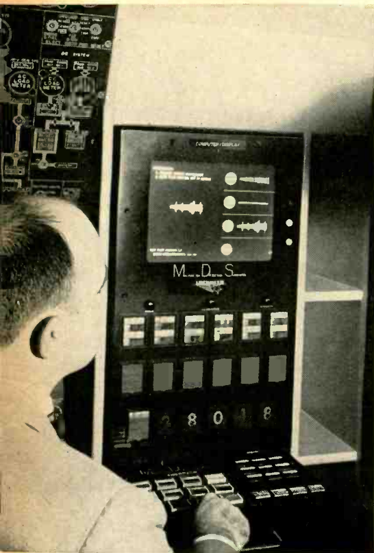
Malfunction detection and recording system will warn the flight engineer when a component fails and tell him if a replacement is aboard.
