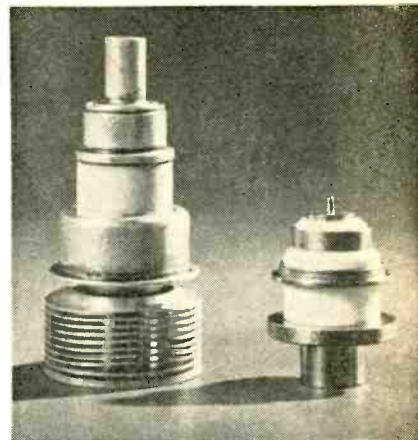
Experimental triode type L65/Y1430, right, supplies c-w power levels 20 times greater than the widely used 2C39 triode. Design improvements have also resulted in unusually high gain-bandwidth products for the L-65.
