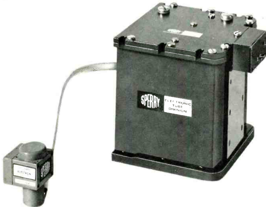
A V band Sperry klystron with matching solid-state power supply.
