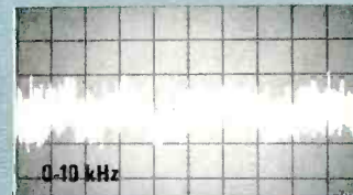
Typical Flutter. Vertical sensitivity is 0.2% p-p/cm.
