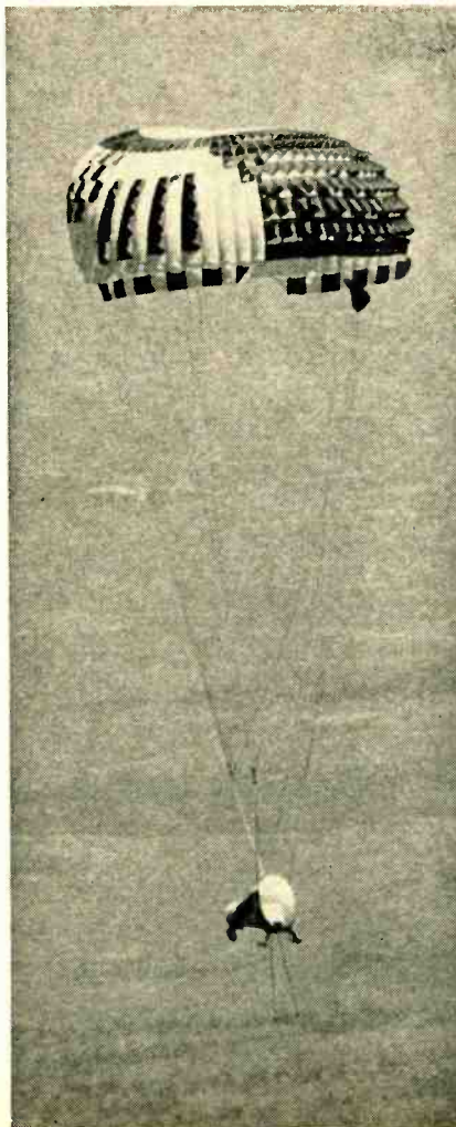
Dummy spacecraft floats to the ground supported by its steerable parachute.
