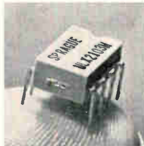
Integrated-circuit broadband amplifier ULN2103M having a 60 Mhz bandwidth with a 30 db typical voltage gain over the temperature range of 0° to +85°C comes in an 8-lead plastic dual in-line package. The IC provides a current gain of 10. The amplifier is suited for current amplification since input impedance is about 10 ohms. Sprague Electric Co., North Adams, Mass. [438]
