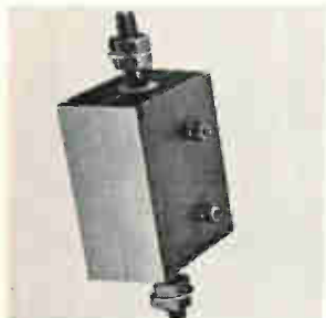
Power resistor SPR-390 has a range of from 0.001 ohm to 0.005 ohm with a temperature coefficient of \pm 50 ppm/ ^{\circ} C from +25^{\circ} to +125^{\circ} C. Standard tolerance is 1%. Inductance properties are as low as 10 nh. The unit can dissipate 50 w when mounted on a 7 \times 5 \times 2 \times 0.040 in. thick aluminum chassis. Size is 3.50 \times 2.00 \times 1.405 in. Dale Electronics Inc., Columbus, Neb. [345]
