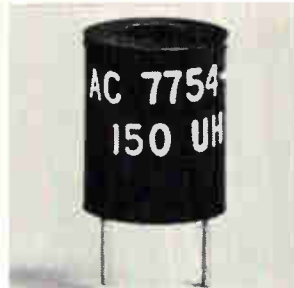
High Q miniature variable inductors AC7754 are offered in nominal inductances ranging from 0.1 \mu h to 4,700 \mu h. Designed for p-c application, the units measure 13/32 \times 1/2 in. Two mounting terminals are spaced 9/32 in. on center for vertical mount. Tuning access is from either end. Approximate price is $1.50 in quantities. Automatic Coil Co., 76 E. 2nd St., Mineola, N.Y. [343]
