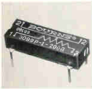
Dual in-line cermet potentiometer model 3099 measures 0.20 x 0.25 x 0.75 in. It has a standard resistance range of 10 ohms to 1 megohm, an operating temperature range of -55^{\circ} to +125^{\circ} C, and a power rating of 0.75 w at 25^{\circ} C. Resistance tolerance is \pm 10\% . It is sealed to meet or exceed immersion requirements of MIL-R-22097. Bourns Inc., 1200 Columbia Ave., Riverside, Calif. [341]
