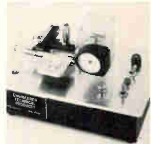
Electrical connections to IC's can be tested for reliability with the Microbond Tester, which determines the gram-range rupture force required to break these bonded interconnects. The unit is furnished with an angular dynamometer and substrate positioning stage. Six gauges are available from 0.5-5 to 15-150 grams. Engineered Technical Products, Box 1465, Plainfield, N.J. [428]
