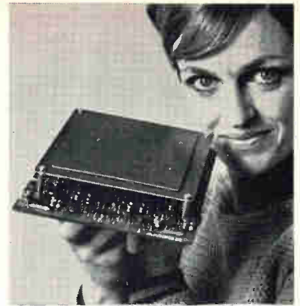
Minimem. Core storage unit is suited for jobs in displays and terminals.
