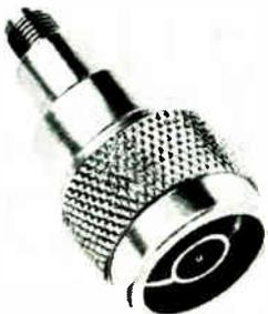
Attenuating adapter model AH-E01 is essentially an adapter from type N to 3 mm with a built-in 10 db attenuator. It reduces hardware in a circuit by combining two elements, thus eliminating a source of error or instability. Unit operates from d-c to 4 Ghz and is available in attenuation values to 20 db. Price is \$50. Microlab/FXR, Ten Microlab Road, Livingston, N.J. [405]
