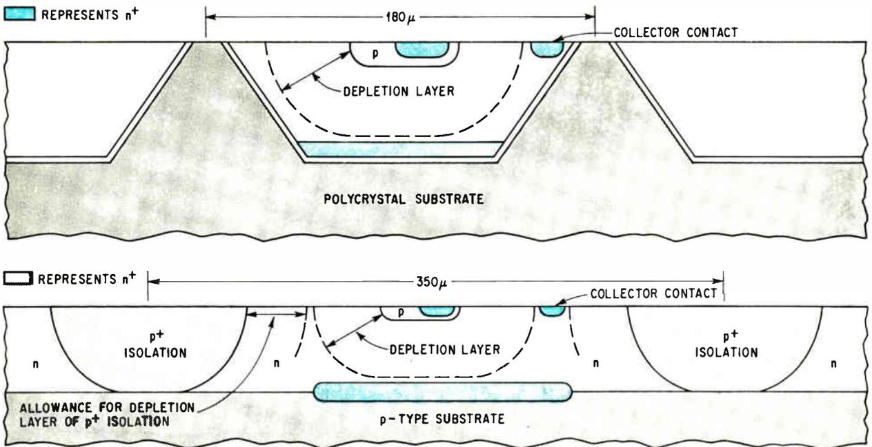
**Making room.** Big advantage of dielectric isolation with anisotropic etch is that many components can be packed on IC. Dielectrically isolated device (above) and p-n junction isolated device (below) are contrasted.
