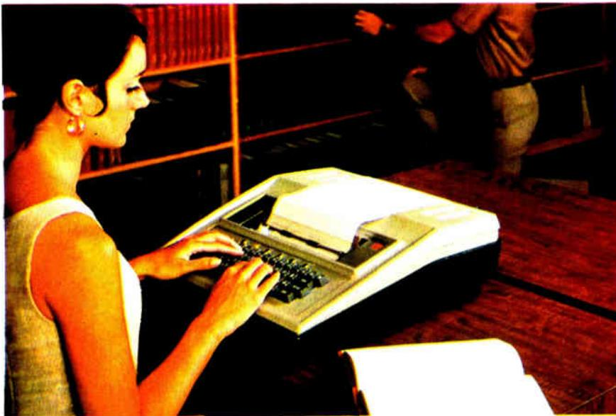
**Hot printer.** New data terminal from Texas Instruments has matrix of silicon heating elements that develop characters on heat-sensitive paper.
