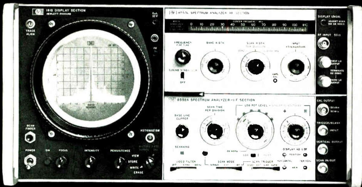
Forget all equipment limitations that used to plague signal analysis in the 1 kHz to 110 MHz range. The HP 8552A/8553L Spectrum Analyzer has all the characteristics—absolute calibration, high stability, freedom from internal distortion and spurious responses—that make it an indispensable tool for virtually every frequency domain measurement.
