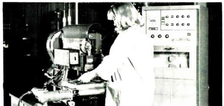
**SLO-SYN N/C WIRE TERMINATING MACHINE** provides fast, accurate positioning of back plane connector assemblies for semi-automatic wire wrapping. Accommodates all standard wire wrap guns plus AMP Termi-Point clip-on connections. Work precisely positioned beneath gun... no operator search. Up to 500 error-free wire terminations per hour. Automatic selector lights for up to 30 wire choices.
