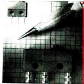
Precision, snap-action switches measure only  $0.3 \times 0.2 \times 0.1$  in. exclusive of terminals. They are rated at 1 amp resistive at 28 v d-c or 115/250v a-c, with an electrical life of 100,000 cycles and a mechanical life of 500,000 cycles minimum. Operating temperature range is from  $-100^{\circ}$  to  $+250^{\circ}$  F. Hi-Tek Corp., 2220 S. Anne St., Santa Ana, Calif. 92704. [343]
