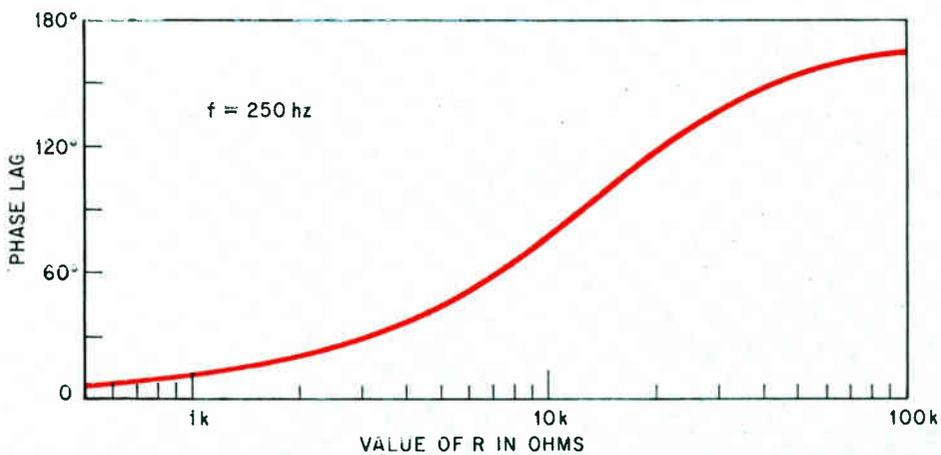
**Lagging.** This circuit's continuously variable phase shift, constant output voltage, and low output impedance makes it useful in analog computers. The phase lag of  $R_1C_1$  combined with the phase lead of  $R_2C_2$  provides a constant output voltage.
