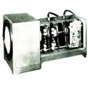
Crt mount is precisely fabricated to accomplish the accurate alignment required in high resolution work with 10 in. flat face crt's. For maximum rigidity, the mount is constructed of heavy-duty cast aluminum. Complete magnetic shielding of crt and magnetic components is achieved by a 3-layer shield assembly. Syntronic Instruments Inc., Industrial Road, Addison, Ill. [346]
