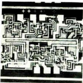
Hex 1-input inverters have been added to the SUHL I and II IC lines. The SG370 circuits operate at 12 nsec typical propagation delay and 22 mw power dissipation per gate function. The SG380's are rated at 6 nsec delay and 22 mw power dissipation. Units come in 14-lead hermetic flatpack or dual-in line ceramic packages. Sylvania Electric Products Inc., Woburn, Mass. [436]
