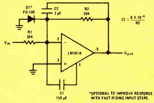
FIGURE 2. Feedforward Frequency Compensation
