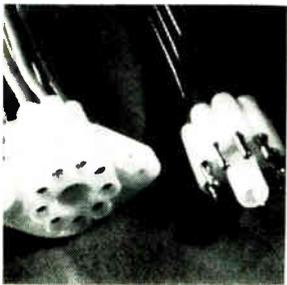
Type 1664-9 plug, used with the 1412 socket, makes a dependable circular connector. Male terminals snap-lock into their nylon housing but can be easily removed with a simple tool. The socket housing can be screw mounted or can be provided with integrally-molded mounting ears for fast snap-in chassis assembly. Molex Products Co., Downers Grove, Ill. [341]
