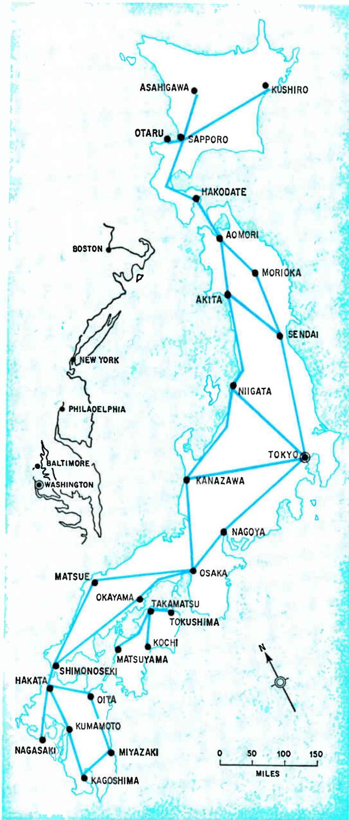
**Training ground.** The Japanese National Railways system has been operating high-speed trains through a 320-mile corridor linking Tokyo and Osaka since 1964; a westward extension from Osaka to Hakata is scheduled for service by 1975. Both lines are part of a long-range master plan to tie all of Japan's major industrial and population centers together in a 2,500-mile high-speed rail grid. Inset of Northeast corridor in U.S. is to scale.
