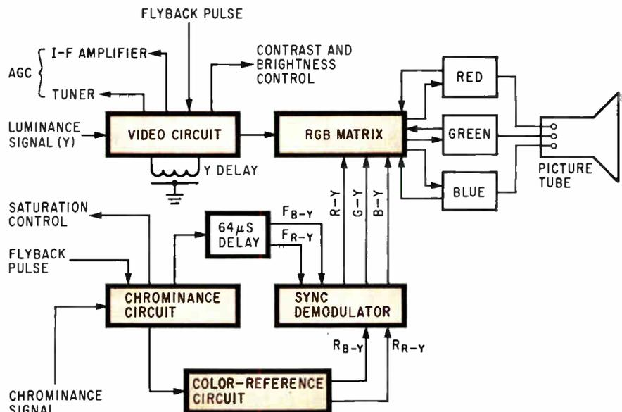
**Colorful quintet.** Color-tv signals from video i-f amplifier are processed by five IC's and two delay lines. Sync demodulator and matrix are in mass production. The other three should be in production next year.
