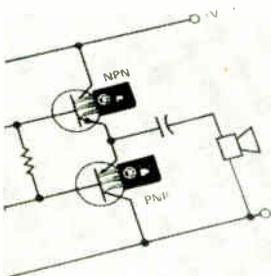
Plastic transistors for 20 and 35 w complementary audio amplifiers measure  $\frac{5}{8} \times \frac{1}{2} \times \frac{1}{8}$  in. The npn MJE205 and pnp MJE105 are 5 amp units with a  $V_{CE0}$  of 50 v, power dissipation of 65 w. The npn MJE2801 and pnp MJE2901 are 10 amp units with a  $V_{CE0}$  of 60 v,  $P_D$  of 90 w. Prices range from \$1.25 to \$1.95. Motorola Semiconductor Products Inc., Box 20924, Phoenix 85036. [440]
