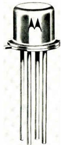
Four leads. N-channel MOS FET switch has external connections for gate, source, drain, and substrate.
