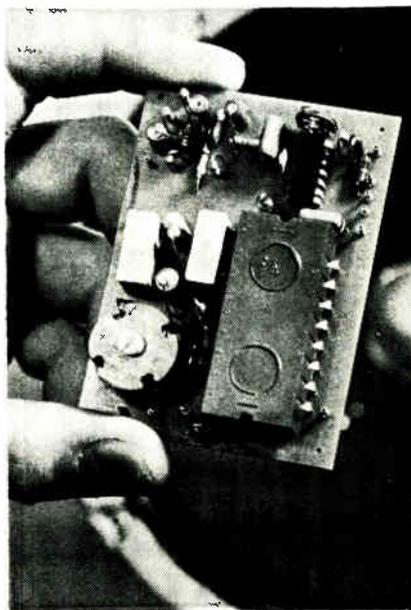
**Cool.** Mullard's experimental pdm circuit (black dual in-line package at top) and the power pack paired with it switch so efficiently that this 30-watt audio amplifier needs no heat sink.
