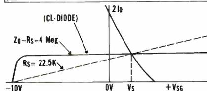
In a balanced circuit the common-mode gain is decreased in approximate proportion to the ratio of source resistances. By substituting the Siliconix CL4710 for the 22.5K source resistance,  $R_s$  is raised to 4 megohms. Common-mode gain is decreased by a factor of over 100. For further information and immediate applications assistance, call the number below. Ask for extension 19.
