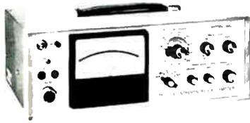
**Model 640** A high performance incremental gaussmeter with precalibrated and interchangeable probes. Center zero meter for direct readout for small incremental variations in both  $\pm$  direction. 1.0% accuracy to 30 kG (0.5% to 10 kG). One volt FS calibrated output.
