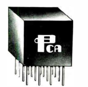
Broad-band transformers are designed for low impedance operation on transmission lines, balanced to unbalanced. Only 0.650 in. long, 0.500 in. wide and 0.700 in. high, these balun transformers have an open circuit inductance of 350  $\mu\text{h}$  minimum, and a low leakage inductance of 0.5  $\mu\text{h}$  max. PCA Electronics Inc., 16799 Schoenborn St., Sepulveda, Calif. 91343. [348]
