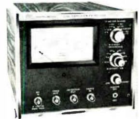
Log amplifier model 6001 accepts any r-f input from 400 khz to 130 Mhz with a power range of -70 dbm to +20 dbm. It provides a linear detected output for oscilloscope, voltmeter, or graphic recorder presentation. The output is accurate to  $\pm 3$  db. Packaged in a half-rack cabinet, the unit measures 8½ 7 x 12¼ in. Telonic Instruments, 60 N. First Ave., Beech Grove, Ind. [364]
