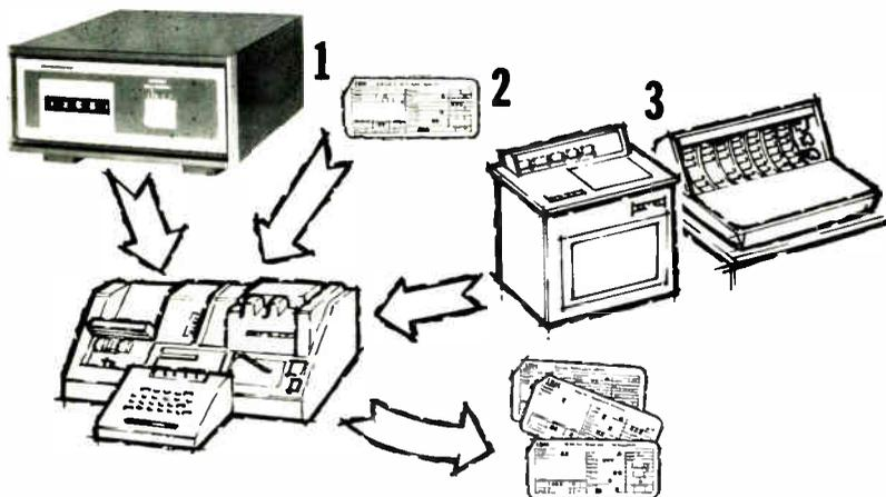
In a typical Digital Clock application, automatic keypunch assembles information from these sources: 1. Time, day and year from Durant Digital Clock. 2. Job and routing from prepunched worker's time card. 3. Production count for time period from worker, using input station. Simultaneously, instantly, keypunch enters this total input on a single computer card for EDP use.
