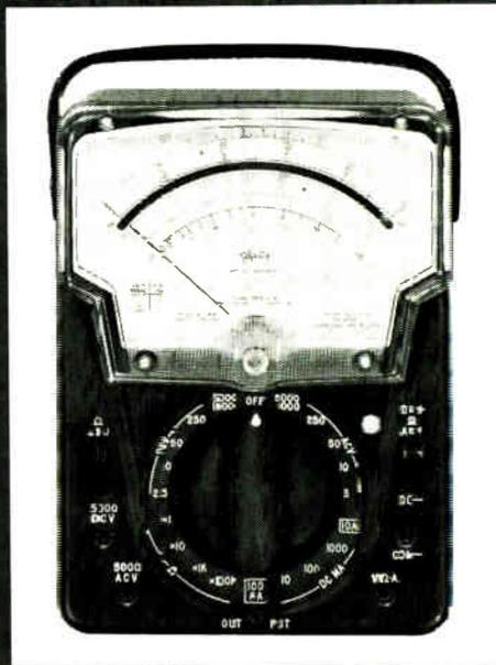
Triplett Electrical Instrument Company needed a case for its new portable volt-ohm-milliammeter that could stand up under the rugged bumps of portable use and protect the user against shock.
