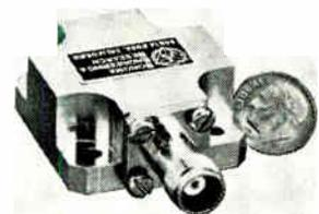
Waveguide-to-coaxial adapter called Flatback is available in ranges from 1.12 to 40 Ghz, with a maximum vswr of 1.25 for frequencies up to 18 Ghz. Miniature, subminiature, and type N coax connectors are standard. Depth of the 12.40 to 18 Ghz unit is only  $\frac{1}{2}$  in. All units meet MIL-E-16400E. Sonoma Engineering and Research Inc., 760 Montecito Center, Santa Rosa, Calif. [408]
