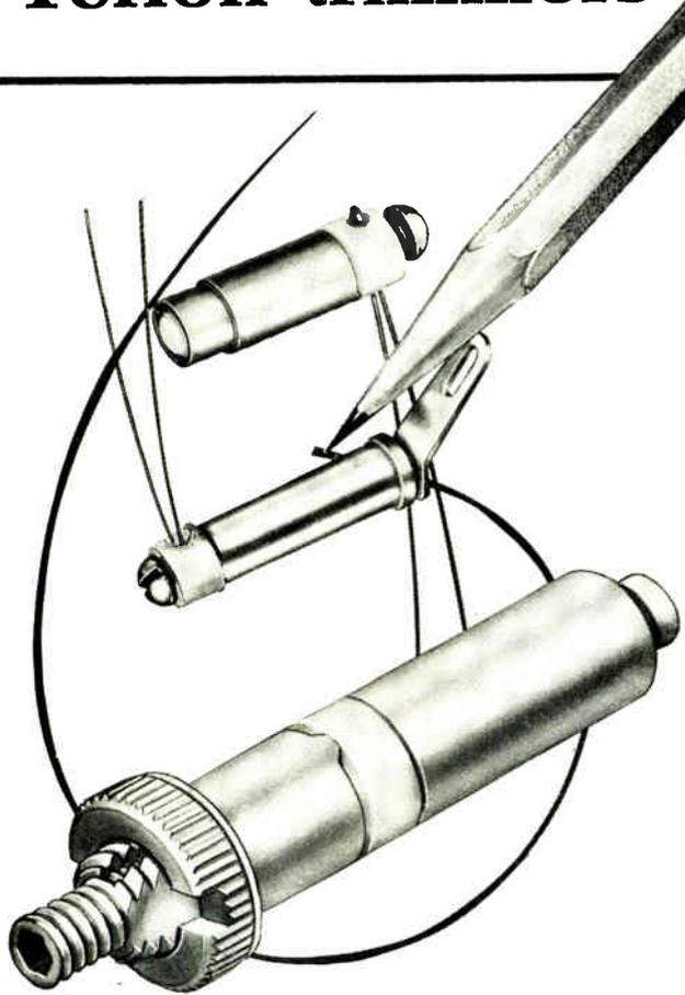
These new trimming capacitors are ideally suited for VHF and UHF applications requiring low minimum capacity and delta C. They provide high resolution and are electrically stable. Tuning is linear. High Q (2000 at 1 MHz typical). Insulation resistance  $10^6$  megohms. Temperature range— $-55^\circ$  to  $+150^\circ\text{C}$ . Voltage breakdown 2000 VDC. Part numbers 273-1-1 and 273-1-2 nominal capacity .25 pf min., 1.5 pf max.; part 273-15-1 nominal .30 pf min., 2.9 pf max.
