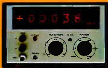
Model 7000A—Dual Slope Integrating 4-full Digit Multimeter. 0.01% accuracy. Measures DC volts, DC millivolts ( $10\mu\text{v}$  resolution), AC volts, ohms, current, BCD. Price: \$1175.00.
