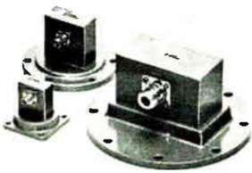
Waveguide-to-coaxial adapters series WCA feature zero transition loss from rectangular to coaxial connectors of "N" to 3 mm (SMA) types. Also featured is low vswr of 1.25 over the waveguide frequency ranges of 2.60 to 18.0 Ghz. The series is available in 18 different models covering 6 frequency ranges and 3 connector types. I-Tel Inc., 10504 Wheatley St., Kensington, Md. [401]
