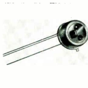
Silicon photodiodes come in 2 types. Type 720, for industrial control use, offers a minimum light current of 90  $\mu$ a at 500 footcandles 2800°K, maximum reverse dark current of 1  $\mu$ a at -1 v. The 820 is for low noise and faster response uses. Both have a peak spectral response at 8,500 A. Price ranges from 69 cents to \$2. National Semiconductors Ltd., Plattsburgh, N.Y. [438]
