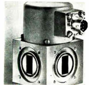
Ku-band, 3-port waveguide switch model NMC-5071 offers greater than 90 db isolation and measures only 2.75 in. in height. The unit has a low insertion loss of 0.2 db, and a low vswr of 1.10. It is available in 2-, 3-, and 4-port design. The switch measures 1.750 x 1.750 x 2.75 in. and weighs 14 oz maximum. Neico Microwave Co., 211 Second Ave., Waltham, Mass. 02154. [404]
