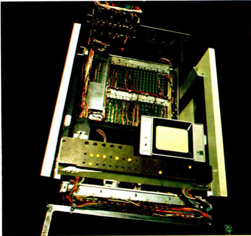
**Modular.** The electronics needed to exercise specific types of core memory is contained in plug-in modules for the test station. The basic system includes circuitry that controls the testing process and displays faults. The CMA 101 requires a minimum of "tuning" and is suited to high-volume operations.
