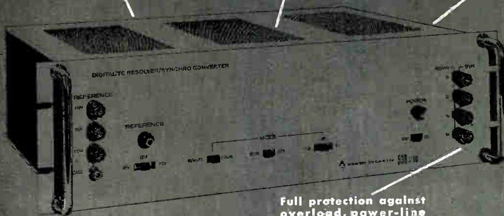
Full protection against overload, power-line transients, frequency changes or improper reference frequency, or short circuit of output terminals.
