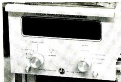
Over the range. The ratiometer measures up to 350 volts, a-c and d-c, and up to 12 megohms.
