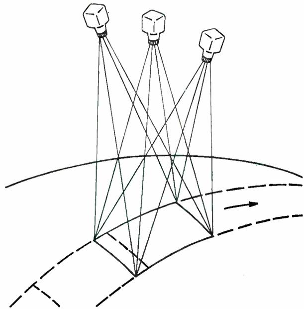
**Ground sweep.** The return-beam vidicons would focus on the same part of the ground track beneath this spacecraft, but Hughes' multispectral camera would scan across the track with an oscillating mirror.
