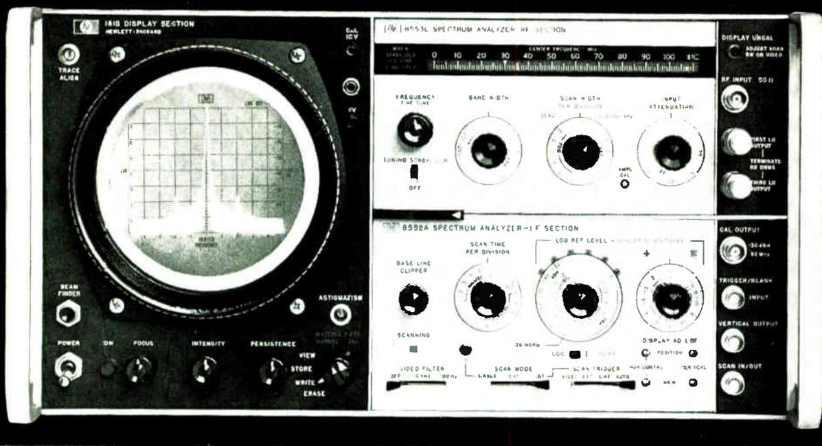
Forget all equipment limitations that used to plague signal analysis in the 1 kHz to 110 MHz range. The HP 8552A/8553L Spectrum Analyzer has all the characteristics—absolute calibration, high stability, freedom from internal distortion and spurious responses—that make it an indispensable tool for virtually every frequency domain measurement.
