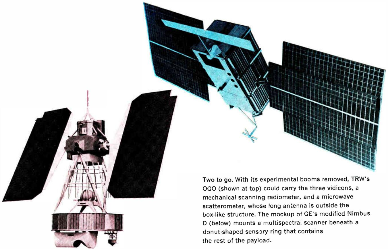
Two to go. With its experimental booms removed, TRW's OGO (shown at top) could carry the three vidicons, a mechanical scanning radiometer, and a microwave scatterometer, whose long antenna is outside the box-like structure. The mockup of GE's modified Nimbus D (below) mounts a multispectral scanner beneath a donut-shaped sensory ring that contains the rest of the payload.
