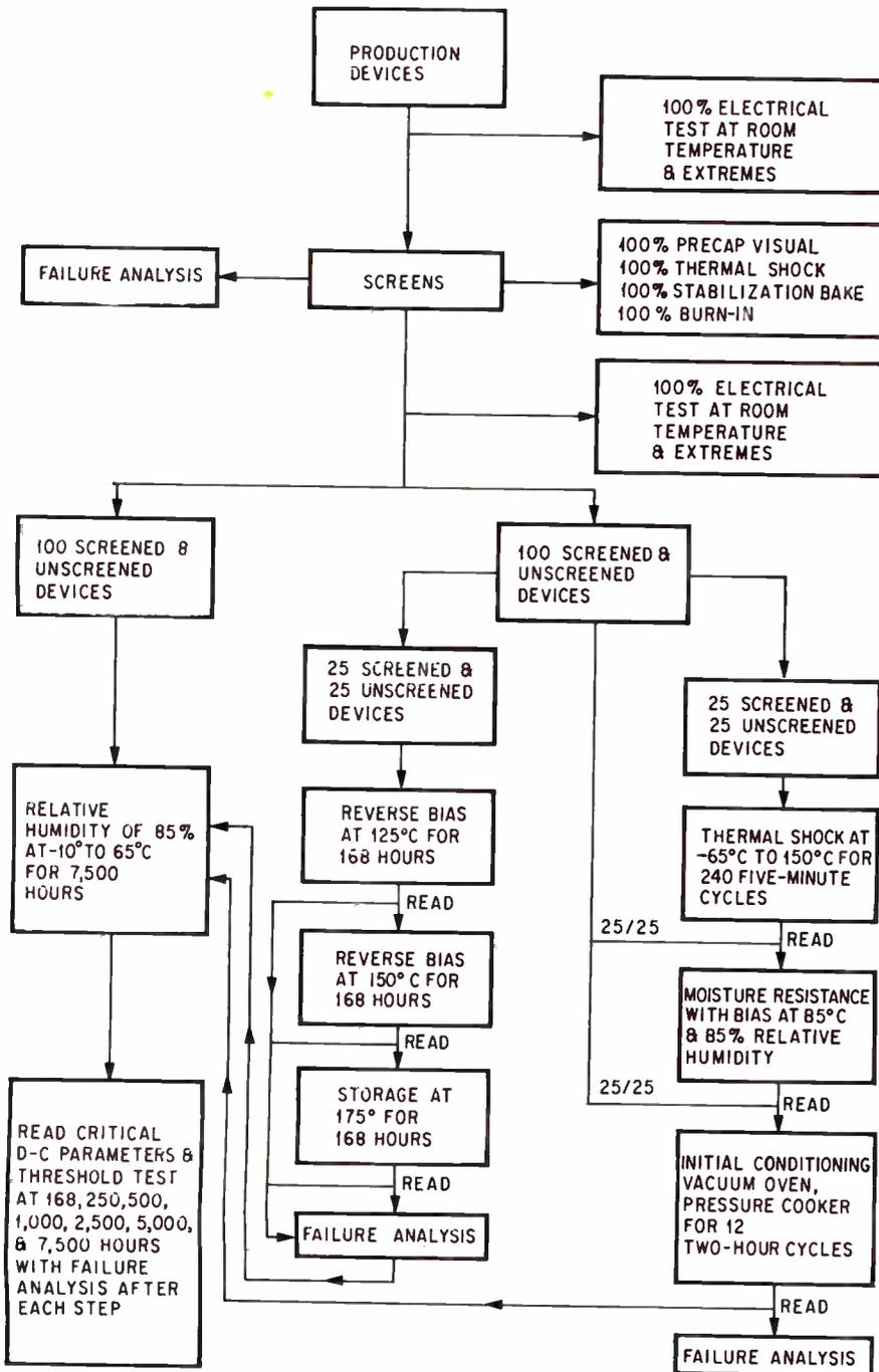
**Proposition.** The test program proposed to makers of plastic-encapsulated IC's by the Rome Air Development Center is designed to produce data on failure modes for such devices. Assemblies will be put through four screens before they're run through the program, which is sequential. The way the checks are set up, a total of 100 screened and unscreened parts, stressed three ways, are subjected to a final 7,500-hour series of tests.
