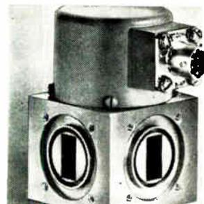
Ku-band, 3-port waveguide switch model NMC-5071 offers greater than 90 db isolation and measures only 2.75 in. in height. The unit has a low insertion loss of 0.2 db, and a low vswr of 1.10. It is available in 2-, 3-, and 4-port design. The switch measures 1.750 x 1.750 x 2.75 in. and weighs 14 oz maximum. Neico Microwave Co., 211 Second Ave., Waltham, Mass. 02154. [404]
