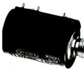
Ten-turn wirewound precision pot model 532 is  $\frac{7}{8}$  inch in diameter. It features a molded housing and lid, with a  $\frac{1}{4}$ -in.-diameter passivated stainless steel shaft, and dual slip-ring contacts. Resistance range is 15 ohms to 180 kilohms, with resistance tolerance  $\pm 5\%$ . Independent linearity is  $\pm 0.25\%$ . Spectrol Electronics Corp., 17070 E. Gale Ave., City of Industry, Calif. [342]
