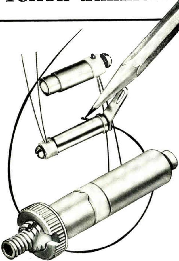
These new trimming capacitors are ideally suited for VHF and UHF applications requiring low minimum capacity and delta C. They provide high resolution and are electrically stable. Tuning is linear. High Q (2000 at 1 MHz typical). Insulation resistance  $10^6$  megohms. Temperature range— $-55^\circ$  to  $+150^\circ\text{C}$ . Voltage breakdown 2000 VDC. Part numbers 273-1-1 and 273-1-2 nominal capacity .25 pf min., 1.5 pf max.; part 273-15-1 nominal .30 pf min., 2.9 pf max.
