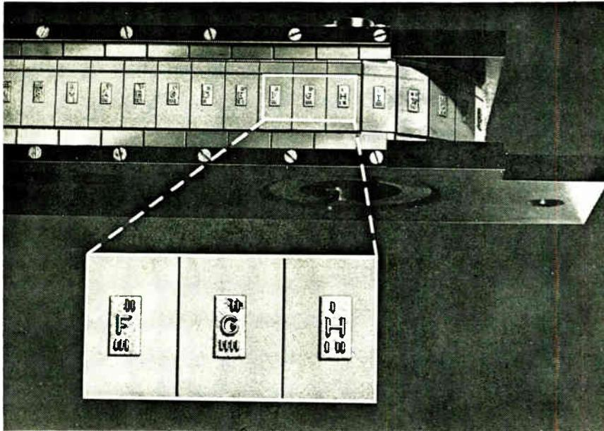
**Hole filler.** Chain module with magnetic character font for Potter printer. System replaces punched cards with man-readable letters.
