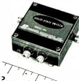
Solid state switch model DS-982 is capable of switching 3.5 kw of peak power at speeds of 50 nsec with less than 2 db loss in the operating range of 1 to 6 Ghz. Featuring a 25 db minimum isolation and a typical vswr of 2.5:1, its operating range is  $-55^{\circ}$  to  $100^{\circ}$  C. The unit weighs 80 grams and measures  $1\frac{3}{4}$  x  $1\frac{3}{4}$  x  $\frac{3}{4}$  in. Sanders Associates Inc., Ledge St., Nashua, N.H. 03060. [406]
