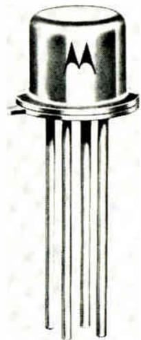
Four leads. N-channel MOS FET switch has external connections for gate, source, drain, and substrate.
