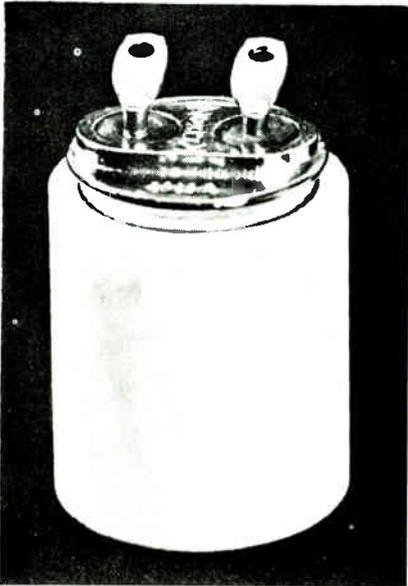
**Safeguard.** Switch is mounted in a container made of beryllia—a heat-conductive electrical insulator.
