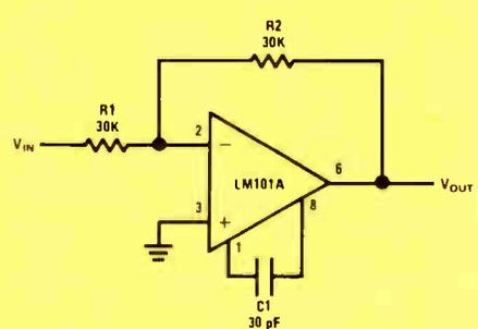
FIGURE 1. Standard Frequency Compensation
