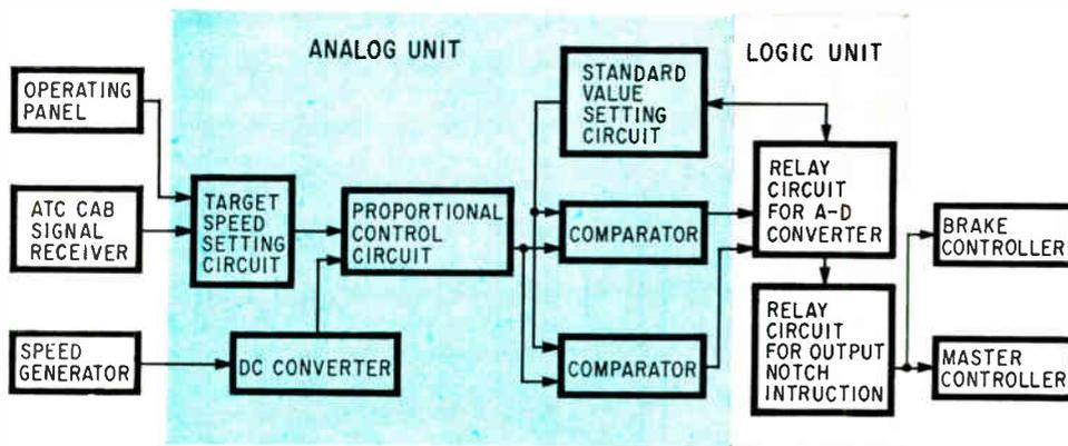
**Autopilot.** This block diagram outlines a proportional control system for automatic constant train speed proposed for new links in Japan's growing chain of high-speed railroads.
