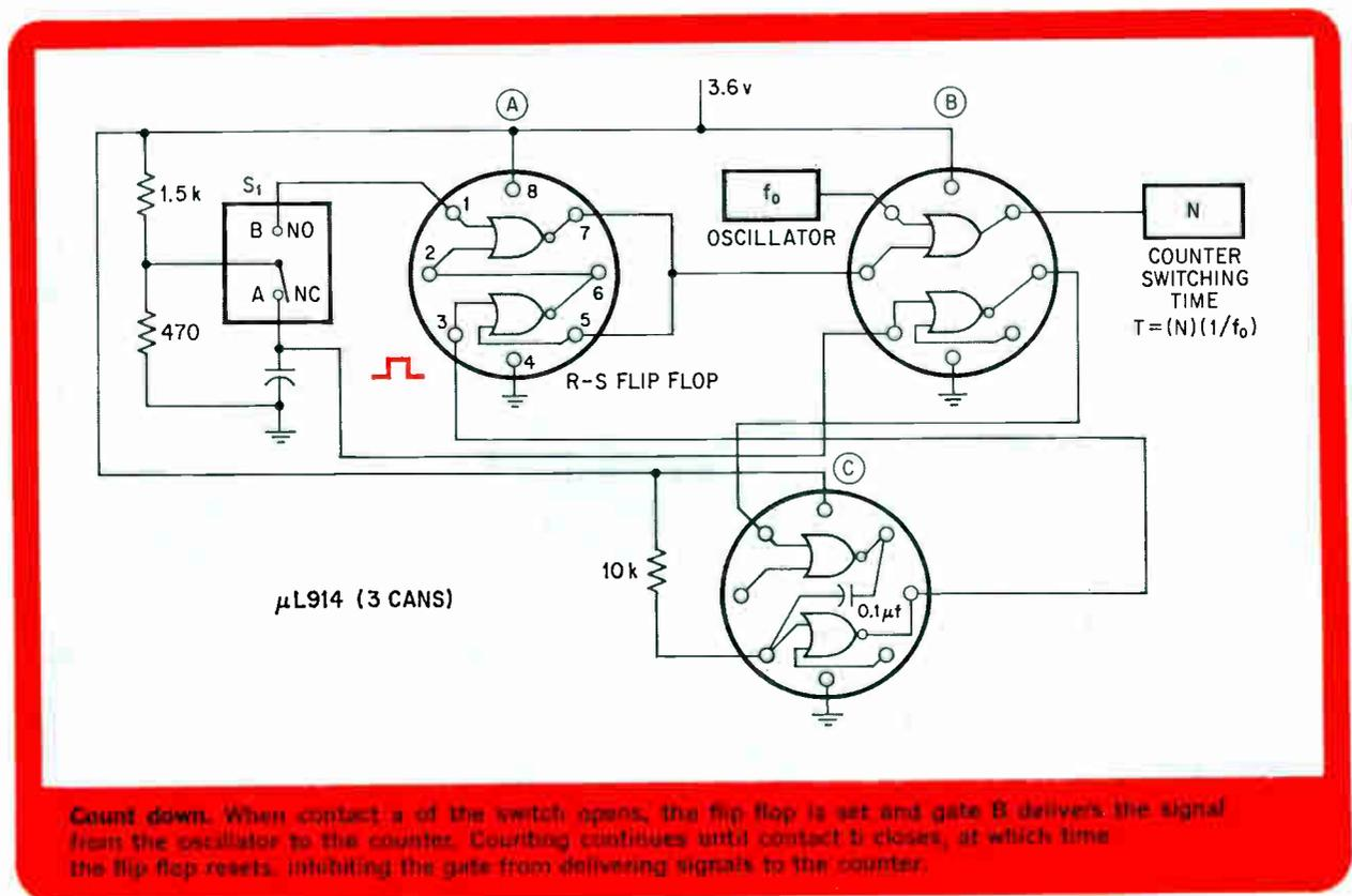
Count down. When contact a of the switch opens, the flip flop is set and gate B delivers the signal from the oscillator to the counter. Counting continues until contact b closes, at which time the flip flop resets, inhibiting the gate from delivering signals to the counter.
