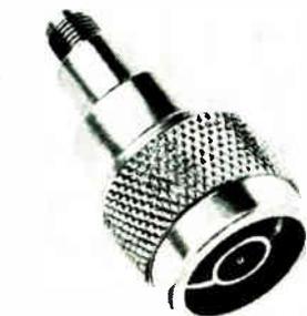
Attenuating adapter model AH-E01 is essentially an adapter from type N to 3 mm with a built-in 10 db attenuator. It reduces hardware in a circuit by combining two elements, thus eliminating a source of error or instability. Unit operates from d-c to 4 Ghz and is available in attenuation values to 20 db. Price is \$50. Microlab/FXR, Ten Microlab Road, Livingston, N.J. [405]
