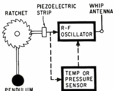
**Powerful strip.** Piezoelectric strip, activated by ratchet, supplies enough power to drive radio transmitter.
