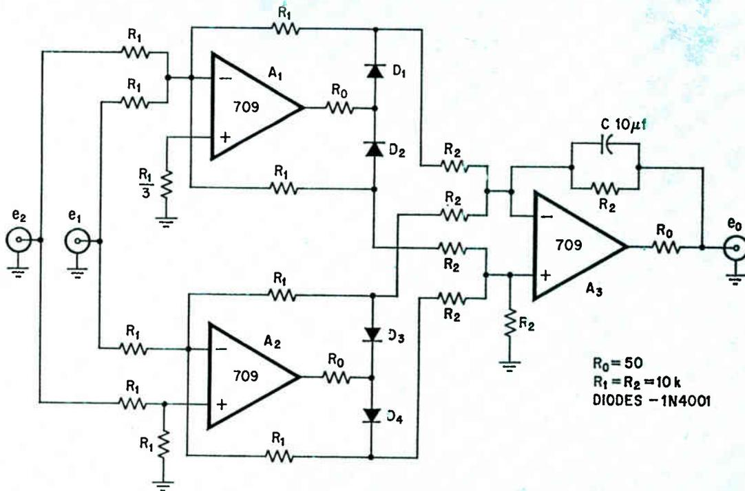
**Wideband.** The wideband, phase sensitive, synchronous detector uses operational amplifiers to increase the bandwidth over that of conventional detectors which use transformers. Op amp  $A_1$  and  $A_2$  function as small signal rectifiers while the third amplifier is used as a lowpass filter.
