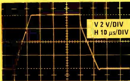
FIGURE 6. Large Signal Transient Response with Standard Compensation
