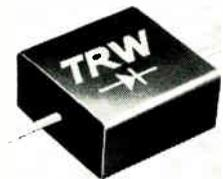
Varicap diodes are designed for use in low-frequency circuits. Type PQ2150 has a capacitance of 150 pf; type PQ2300, 300 pf, and type PQ2500, 500 pf. The single chip devices have less than 1  $\mu$ a leakage, Q factor greater than 150 and 90 v breakdown. The flat encapsulated package measures 0.320 in. sq. x 0.165 in. TRW Inc., 1100 Glendon Ave., Los Angeles 90024. [439]
