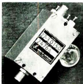
Octave band tunable, solid state source model 67-30150 is suited for wideband receiver, transmitter and test equipment applications. Frequency range is 1 to 2 Ghz; output power, 100 mw minimum; tuning voltage, 0 to  $-50$  v d-c; primary power,  $-20$  v d-c at 200 ma maximum. Size is 1 x 1 x  $1\frac{3}{4}$  in. Addington Laboratories Inc., 1043 DiGiulio Ave., Santa Clara, Calif. 95050. [407]
