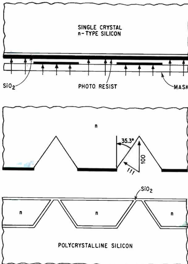
**Isolation steps.** Pattern is exposed to back side of silicon slice during dielectric isolation. Then unexposed regions are etched with anisotropic etchant, which forms v-shaped groove. SiO<sub>2</sub> dielectric coats single crystal; polycrystalline silicon backfills grooves, and silicon is lapped from top to expose grooves.
