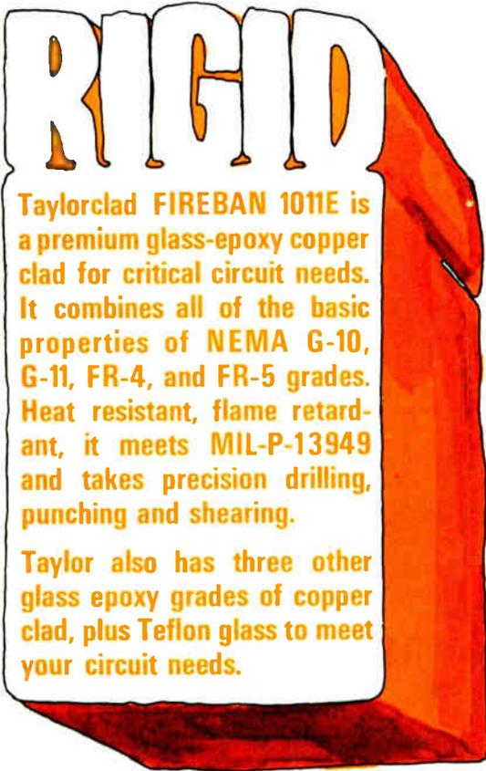
**Taylorclad FIREBAN 1011E is a premium glass-epoxy copper clad for critical circuit needs. It combines all of the basic properties of NEMA G-10, G-11, FR-4, and FR-5 grades. Heat resistant, flame retardant, it meets MIL-P-13949 and takes precision drilling, punching and shearing.**
