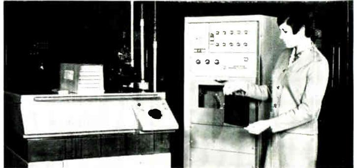
**SLO-SYN N/C DRILLING MACHINE** provides precise multiple drilling of printed circuit boards and panels. All four heads operate simultaneously from same taped program for greater accuracy and uniformity free of human error. Precise drill heads accommodate bits from 1/64 to 1/4 inch. Spindle speed adjustable to 45,000 rpm; drilling rate up to 80 cycles per minute.
