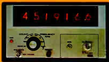
Model 8220 — 500MHz Direct Reading Frequency Counter. 7-digit display with memory. Price: \$1795.00.
