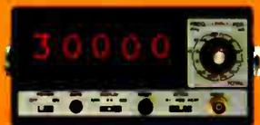
Model 8050—30MHz Frequency/period meter (with 8051 pre-scaler, capability extended to 300MHz). Also measures multiple period average and totalizes. Price: \$650.00.
