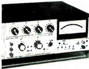
Frequency response analyzer 911A measures phase and amplitude vs frequency over the range of 0.01 to 10,000 hz with a high rejection of noise and harmonics in the return signal. It performs with an over-all accuracy of  $\pm 1^\circ$  in phase measurement, and  $\pm 1\%$  in amplitude, with greater than 40 db of harmonic and noise rejection. Bafco Inc., 80 Second St. Pike, Southampton, Pa. [362]
