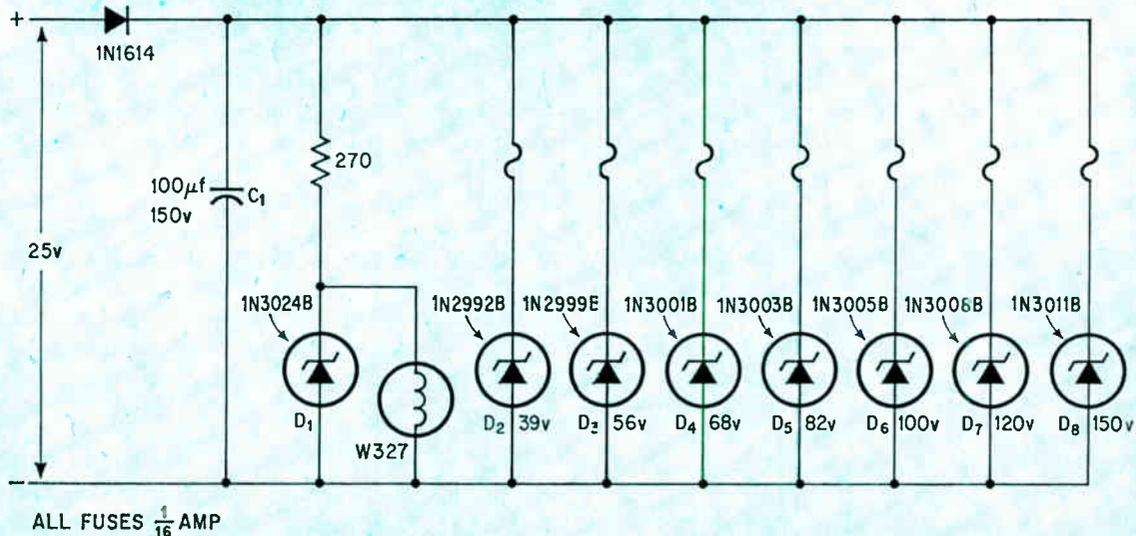
**Continuous surveillance.** To determine whether any dangerous transient voltage spikes exist on a power bus, this detector is connected in series with the supply line. Determining which fuse has blown yields an estimate of the amplitude of the spike.
