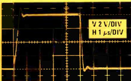
FIGURE 5. Large Signal Transient Response with Feedforward Compensation
