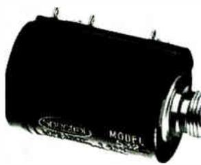
Ten-turn wirewound precision pot model 532 is  $\frac{7}{8}$  inch in diameter. It features a molded housing and lid, with a  $\frac{1}{4}$ -in.-diameter passivated stainless steel shaft, and dual slip-ring contacts. Resistance range is 15 ohms to 180 kilohms, with resistance tolerance  $\pm 5\%$ . Independent linearity is  $\pm 0.25\%$ . Spectrol Electronics Corp., 17070 E. Gale Ave., City of Industry, Calif. [342]
