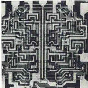
Quad 2-input NOR gate IC's series SG330 and SG340 have been added to the SUHL TTL family. The SG330 operates at 12 nsec typical propagation delay and 20 mw average power dissipation per gate function. The SG340 is rated at 6 nsec typical propagation delay and 20 mw average power dissipation per gate function. Sylvania Electric Products Inc., Woburn, Mass. [440]
