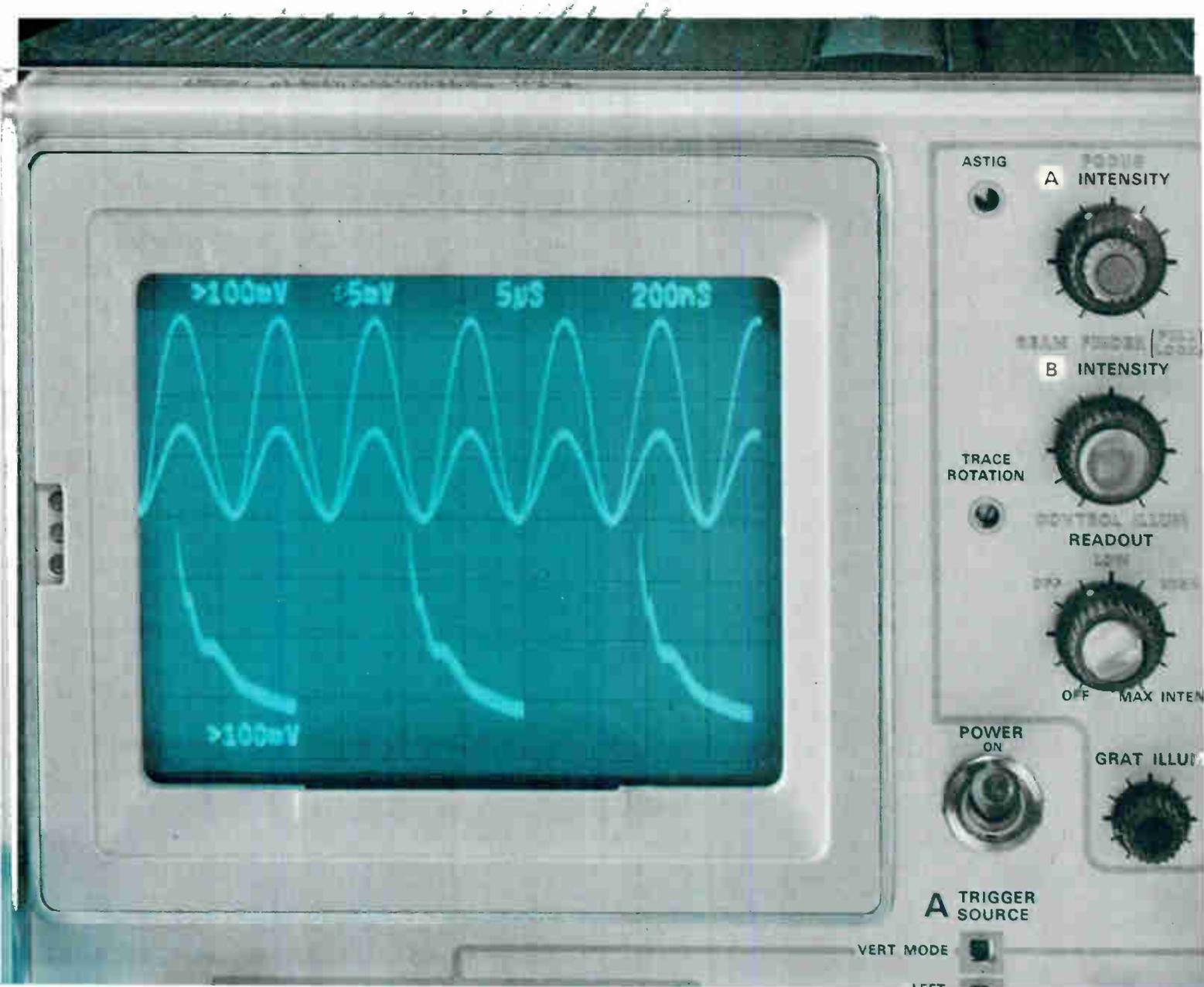
larly difficult with “fixed” readout devices). The display isn’t limited to alphanumeric; such things as arrows, limit markers, and pictorial symbols can be included. And external information, not from the plug-in, can be mixed into the display.
