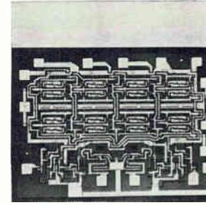
MSI memory TMC 3262 is for high-speed computer scratch pad memory applications where low power is a critical requirement. Power dissipation for the memory is typically 175 mw at a nominal operating voltage of 5 v compared to 250 mw for high power memories. Also, maximum address line select current is only 6.5 ma. Transiltron Electronic Corp., Wakefield, Mass. [442]
