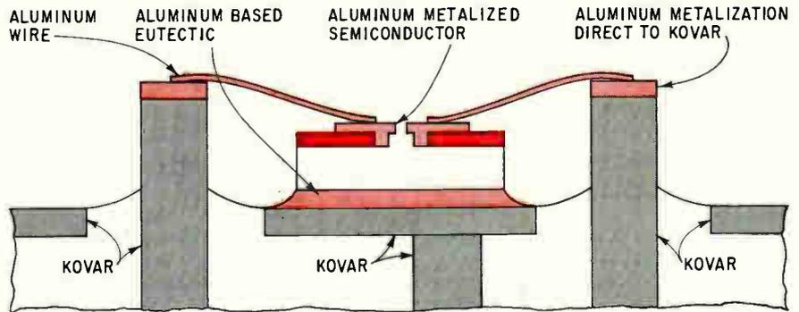
**Nothing glitters.** Gold, which is prone to catastrophic failure in harsh radiation environments, is replaced by aluminum in top posts, the lead wires bonded to those posts, transistor metalization itself, and eutectic bonding material. Latter is aluminum-germanium.
