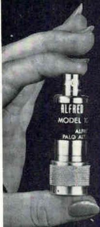
With flat frequency response and low SWR, Alfred broadband crystal detectors, Models 1001, 1002, and 1003 provide top performance in your leveling, power measurement, broadband RF detection and reflectometer requirements.
