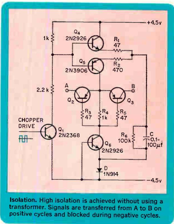
**Isolation.** High isolation is achieved without using a transformer. Signals are transferred from A to B on positive cycles and blocked during negative cycles.
