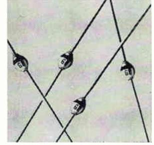
Axial lead fast recovery rectifier series A114 is for use in high frequency applications. It is rated at 1 amp in 50 to 600 v versions, with a 200 nsec maximum reverse recovery time. Unit has dual heat sink construction which provides rigid mechanical support for the pellet and excellent thermal characteristics. General Electric Co., 1 River Rd., Schenectady, N.Y. 13205 [443]
