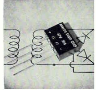
Full wave bridge rectifiers series AFW are pre-packaged silicon rectifier circuits for commercial and industrial applications. They directly replace individual units in multirectifier circuits. Units come in the following prv ranges: 50, 100, 200, 300, 400, 500, 600, 800, 1,000 v all with d-c output of 2 amps at 50°C ambient. Analog Equipment Corp., 18 Granite St., Haverhill, Mass. [439]
