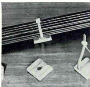
Adhesive backed mount ABMS-A secures wiring harnesses to virtually any smooth surface for light duty applications. Inclusion of a countersunk hole permits the mount to be used with a No. 6 flat-head screw or a ⅜ in. flat-head rivet. The result is a one-hole mount which will not rotate. Mount measures 1⅜ in. sq. Panduit Corp., 17301 Ridgeland Ave., Tinley Park, Ill. [345]
