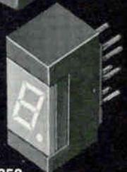
ALCO's RK numeric and symbol readouts have a unique in-line design to provide clear displays without focusing problems. The precision machined 1-piece aluminum case also serves as a heat sink.
