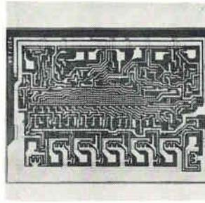
Seven-segment decoder/driver MSI 9317 offers a medium scale complexity that can convert 4 inputs in 8421 BCD format. It is for any military, computer, or industrial system employing seven-segment incandescent lamp displays or light emitting diode indicators. Prices are from \$9.40 to \$30.80 depending on quantity and temperature. Fairchild Semiconductor, Mtn. View, Calif. [441]
