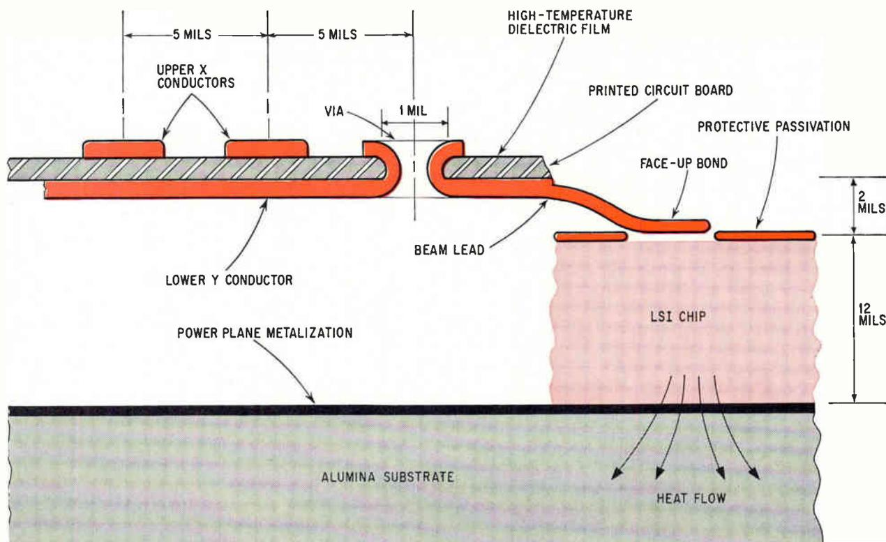
**Cross-section.** In one electroplating cycle, the beam leads are integrally formed with the upper and lower conductors and anchored by means of the vias. The beam lead, which contains a 2-mil offset for strain relief, is bonded face-up to the LSI chip. Thermal conductivity is through the alumina substrate base rather than the contacts. Power is delivered to the chip by a metalization layer on the substrate.
