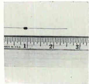
Microminiature, magnetically shielded axial lead inductor series designated the Pee-Wee Ductor is designed to meet MIL-C-15305C Class 5 requirements. It has minimum Q values of 34 to 55 at r-f frequency, with a standard inductance tolerance of ±10%. Current capabilities range from 43 ma to 1½ amps. Nytronics Inc., 550 Springfield Ave., Berkeley Heights, N.J. 07922 [344]
