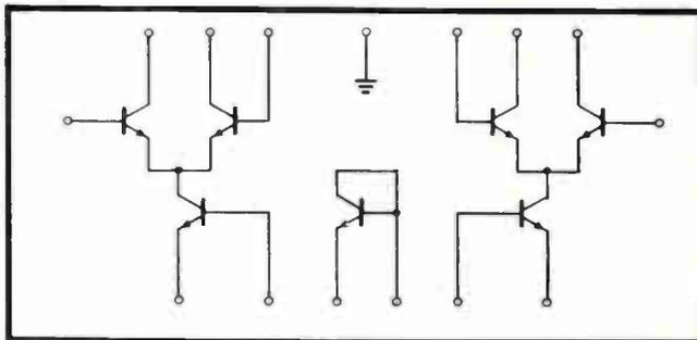
**3.** Improve your computer's memory with Linear Circuit 526—the high-speed comparator that's beyond compare! (Do you know of another comparator with a propagation delay of 30 ns?) Other features to remember: 1) operates from  $\pm 5\text{V}$  supplies; 2) overdrive recovery, 20 ns; 3) fanout of 10; 4) high gain operation; 5) output compatible with DCL, DTL and TTL.
