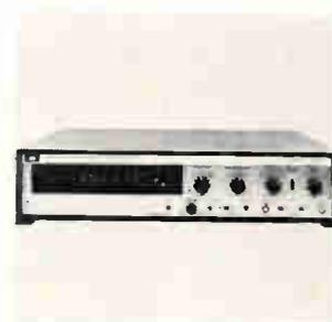
Programable universal counter/timer 110C is a 150 Mhz unit featuring light-emitting numeric display. It totalizes from 0 to  $10^8$  and is prescaled from 10 to  $10^{-16}$ . Frequency ratio is measured from  $10^{-3}$  to  $10^8$ . Period average is from 0.1  $\mu\text{sec}$  to 1 sec and period is measured from 1  $\mu\text{sec}$  to  $10^{-8}$  sec. Monsanto Electronic Instruments, W. Caldwell, N.J. [364]
