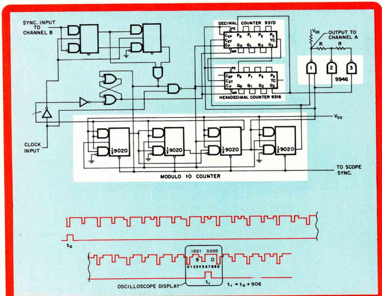
**Timely.** An alternative to the delayed sweep of an oscilloscope is the digitally-encoded reference waveform generator. A clock drives two binary counters connected as a shift register whose contents move circularly once for each clock pulse. The waveform's period is equal to the period of the input clock.
