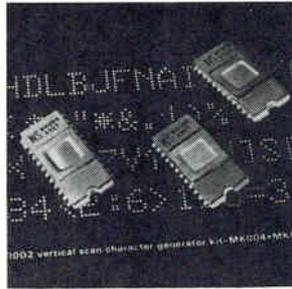
Two MOS read only memory kits generate control signals for digital data displays. The three 1,024-bit memories in each kit are preprogrammed to convert standard communications code words into raster scan or vertical scan control signals. Displays can be operated at high speed by TTL integrated circuits. National Semiconductor Corp., 2975 San Ysidro Way, Santa Clara, Calif. [437]
