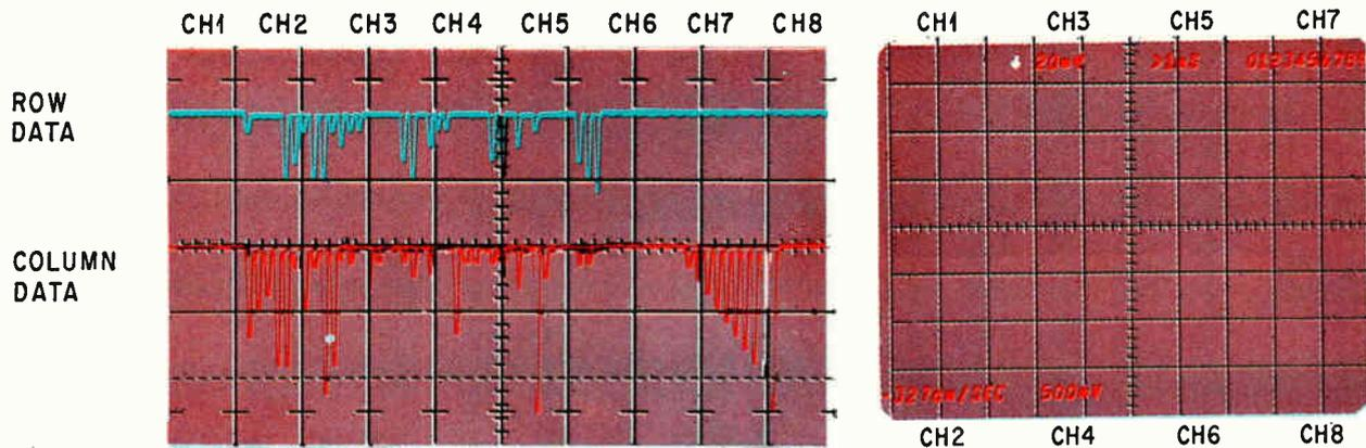
**Analogs and digits.** Multilevel analog pulses, top, built up in increments of  $-100$  microamperes, represent dial or probe setting for each channel displayed on scope screen (right). With analog code, fewer connections are needed between plug-in and main frame than if binary digital code were used.
