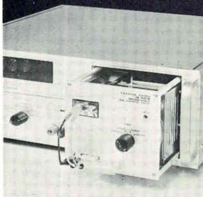
**-TR-6018** Microvolt DC Range Unit permits DC voltage measurements at a resolution of 10 nanovolts. Input circuit employs a floating and guarded system. Input cable features a special conductor having an extremely small thermoelectric force. Main unit: **-TR-6515** autoranging, integrating digital voltmeter.
