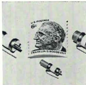
Vertical mount series of high Q variable air capacitors are for p-c applications. They feature 4 basic models with both single and double leads. Model 8051 has a capacitance range of 0.5 to 3 pf; 8052 ranges from 1 to 10 pf; 8053, from 1 to 14 pf; and 8054, from 1.2 to 20 pf. Johanson Mfg. Corp., 400 Rockaway Valley Rd., Boonton, N.J. 07005 [342]
