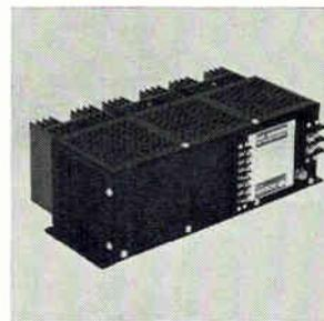
Modular power supplies series SR come in 64 models ranging in voltage from 3.6 to 48 v, and currents up to 35 amps. Typical specifications include 0.075% regulation (load and line), ripple less than 5 mv peak to peak, transient response 20 to 50  $\mu\text{sec}$ . Prices start at \$89 for a 5 v, 5 amp unit. Powertec Division of Airtronics Inc., 9168 DeSoto Ave., Chatsworth, Calif. [384]
