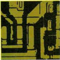
Fairchild's new MSI 9314 Quad Latch is a versatile, high-speed device that can be used in any application requiring a single-input D-type latch or an R/S-type latch. It has no undefined states in the R/S mode. Its unique multi-function capabilities make it useful in a number of applications:
