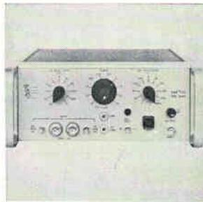
Pre-amplifier model 113 provides amplification of signals from d-c to 300 khz. Typical noise figures are 0.3 db maximum at 10 hz with a 2 megohm source impedance; 0.2 db maximum at 1 khz with a 1 megohm source impedance. Gain is from 10 to  $10^4$  in 1-2-5 sequence, continuously variable. Princeton Applied Research Corp., Box 565, Princeton, N.J. [387]
