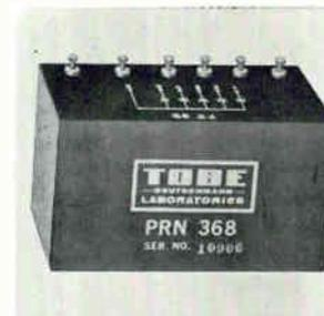
Solid dielectric pulse capacitor PRN-368 features high reliability, low dissipation factor (less than 0.2% at 1 khz), close tolerance between sections, and high energy density. It is a 5-section capacitor with 0.0225 µf capacitance per section, with less than 450 pf difference between adjacent sections. Tobe Deutschmann Laboratories, 550 Turnpike St., Canton, Mass. [346]
