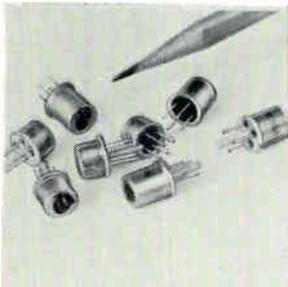
Ultraminiature power dividers feature high isolation (30 db) and low insertion loss (0.5 db) for the broadband of 10 khz to 10 Mhz. Available in 2 models, these 3-port hybrid junctions will divide a signal input into 2-phase stable equal amplitude outputs, or resolve 2 independent inputs into their algebraic sum. Olektron Corp., 6 Chase Ave., Dudley, Mass. 01570 [341]
