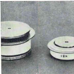
Flat disk scr's from 115 to 470 amps average offer high surge current handling capability, low forward drop and  $dv/dt$  of 200  $\mu$ sec to 1,300 v. Applications include choppers, welders, and regulated power supplies. In 24-99 lots, prices range from \$66 for the 115PA, 500 v to \$210 for the 470 PA, 500 v. International Rectifier, 233 Kansas St., El Segundo, Calif. [436]
