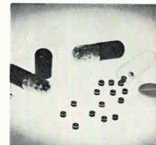
Microminiature pellet resistors are suited for use in flatpacks, microwave loads and attenuators, temperature compensated transistor circuits, etc. Pellets are available in three models measuring 0.100 x 0.062 in. Tolerances are attainable to ±1%, resistance range is 10 ohms to 500 kilohms. Pyrofilm Corp., 60 S. Jefferson Road, Whippany, N.J. 07981 [348]
