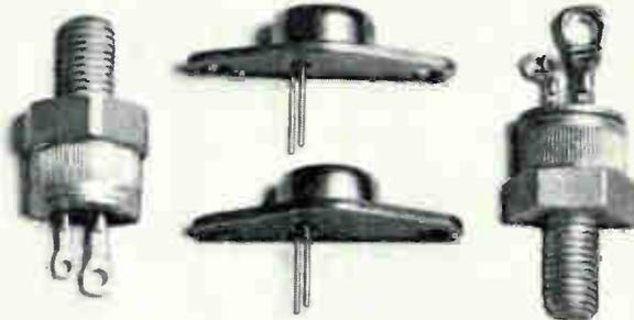
Shock most SCR's with a 400 A/ $\mu$ s pulse and they're destroyed—they can't turn off fast enough. Slam the developmental RCA-TA7395 with the same kind of pulse, and it keeps working . . . and working . . . and working. (It literally breaches the current barrier!) That's because RCA SCR's turn off in 10  $\mu$ s and spread forward current faster—so switching losses are low—and less heat is dissipated internally.
