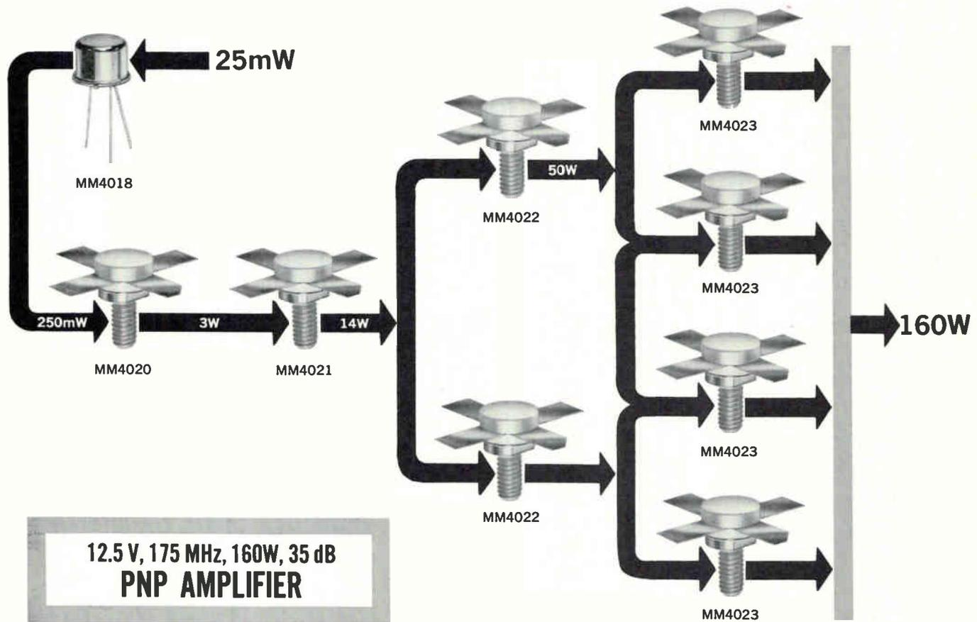
Six new types in Motorola's exclusive line-up of PNP silicon RF Power transistors now give you the advantages of the inherently higher saturated power and superior power output stability vs. temperature of PNP polarity in applications such as VHF large signal amplifiers.
