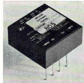
Four lightweight power amplifiers identified as the C70 3722 series are designed to drive either resistive or reactive loads in synchro driver or voltage follower applications. They meet the environmental requirements of MIL-E-5400. Rated output volts range from  $\pm 11$  to  $\pm 18.5$  v; rated output current, 135 to 500 ma. Singer-General Precision Inc., Little Falls, N.J. 07424 [388]
