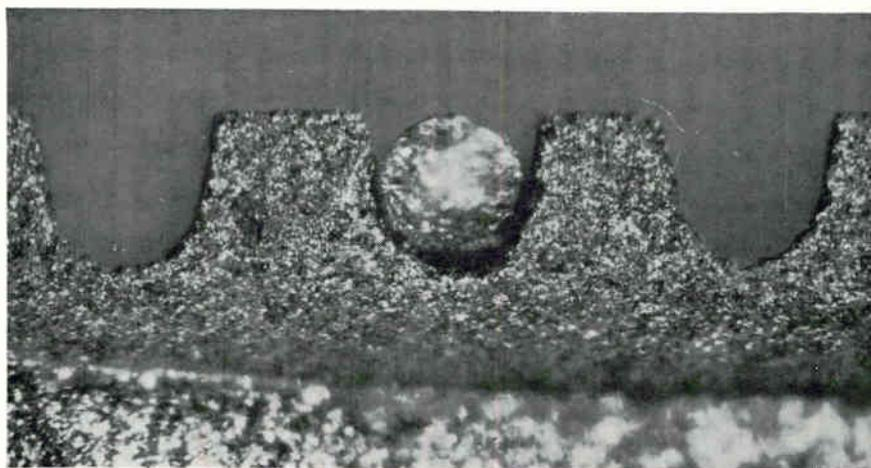
Imbedded. Bit lines of 0.13-mm copper wire with magnetic plating rest in shallow grooves. At right angles run 0.07-mm insulated copper wires, nestled in grooves cut deeper in ferrite keeper sheet.
