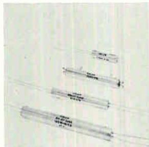
Precision series lumped constant delay lines are designed to meet the extreme requirements of sophisticated military and airborne applications. They offer delay time accuracy of ±3% or better. Temperature range is -50° to +125° C, while test voltage is 500 v d-c, and working voltage is 200 v d-c. Valor Electronics Inc., 3100 Pullman Ave., Costa Mesa, Calif. 92626 [343]
