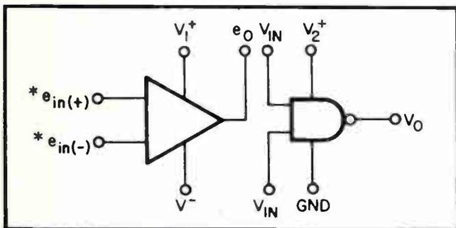
**4. Improve your computer's memory with Linear Circuit 5733.** It's the video amplifier that operates over— are you ready?— 120 MHz band width! Differential in/differential out with minimal phase distortion, too. And as a pre-amp in computer applications, don't forget: 1) 10 ns rise time; 2) fixed gains of 10, 100, 400 available (variable between 10 and 400 with a single, external resistor); 3) internally compensated (no external frequency compensation components required.)
