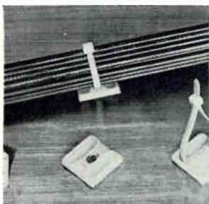
Adhesive backed mount ABMS-A secures wiring harnesses to virtually any smooth surface for light duty applications. Inclusion of a countersunk hole permits the mount to be used with a No. 6 flat-head screw or a ⅜ in. flat-head rivet. The result is a one-hole mount which will not rotate. Mount measures 1⅞ in. sq. Pandult Corp., 17301 Ridgeland Ave., Tinley Park, Ill. [345]
