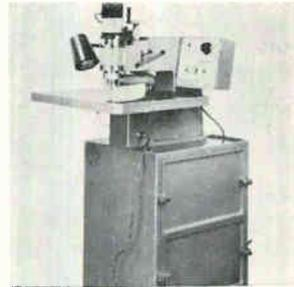
Precision pin router, the Acro-Router, for circuit board profiling and inside routing, features a constant torque spindle, features a constant torque spindle. Spindle speed is infinitely variable to 40,000 rpm max. Peak power is 0.6 h-p at 24,000 rpm. An integral dust collector sucks up chips and dust, keeps work and table surface clean. Aetna Mfg. Co., 245 Park Ave., Bensenville, Ill. [426]
