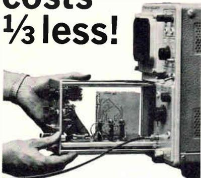
With U-Tech's plug-in and console units, any X-Y oscilloscope becomes a curve tracer displaying the dynamic characteristics of both NPN and PNP transistors, N Channel and P Channel junctions, FET's, MOS-FET's, bipolars, unijunctions, diodes, tunnel diodes and SCR's. You have curve tracer capabilities, without buying a complete curve tracer unit. In so doing you pay up to:
