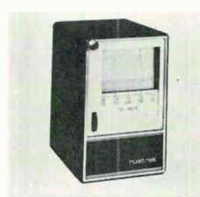
Voltage recorder model 2186 for high resolution line monitoring is an expanded scale recording voltmeter with low end of scales suppressed. Scales centered on nominal commercial line voltages have a resolution of 0.5 v per division on the basic range and 2 v per division in the 460 v a-c range. Rustrak Instrument Division of Gulton Industries Inc., Manchester, N.H. 02103 [368]
