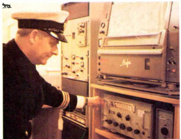
**Shooting the satellites.** A navigator checks weather map reproduced on a Muirhead facsimile machine from a radio transmission on shore. On his left is ITT Aerospace's satellite navigation system, which contains its own PDP-8/1 computer made by Digital Equipment Corp. The ITT/DEC combination contacts one of several Navy navigation satellites for an hourly position fix. The fixes are accurate to a tenth of a nautical mile—about 600 feet. That's within the ship's length—963 feet.
