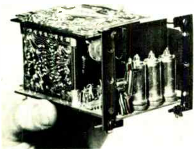
Uncased. Low-priced digital panel meter is offered in unipolar and bipolar versions.
