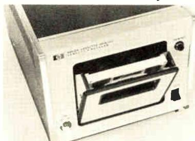
different lengths and are located by address without rewinding. The ability to find a file by number also lets the user recall data from that file, modify it, then restore it to the same file without rewriting on a second cassette. Search speed is 130 feet per minute in either direction. Price is \$1,750.
