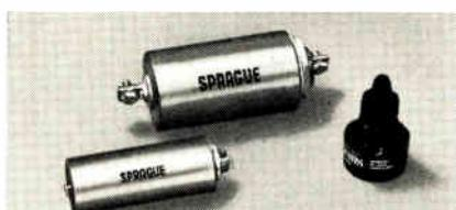
**U.L. LISTED FILTERS.** Series JX5000 for EDP equipment and general-purpose use. Rated 125/250 VAC, 0-60 Hz, 1 thru 50 amps. 60 db @ 150 kHz, 80 db from .5 MHz thru 1 GHz. Special designs and rectangular multi-circuit units also available. Write for Engineering Bulletin 8210 or;
