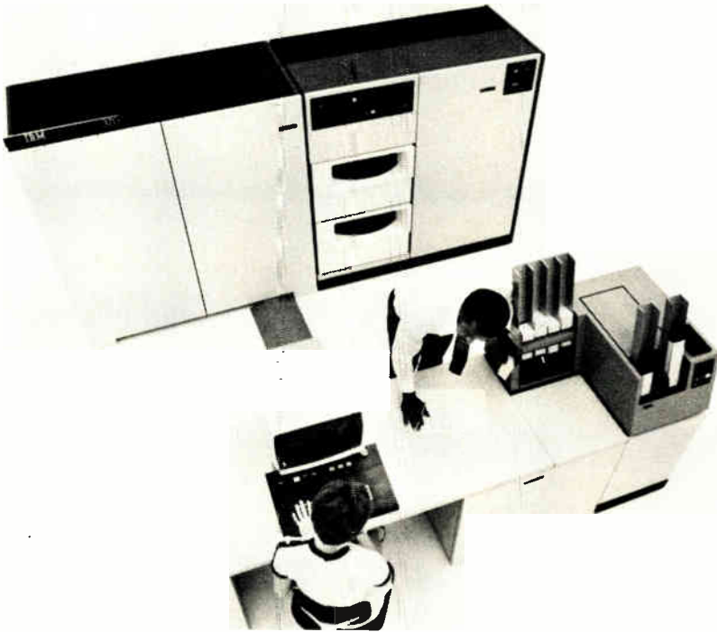
New baby. The addition to the low end of IBM's 370 line, the model 125, incorporates virtual memory and offers large on-line disk storage capacity. The total can be 400 million.
