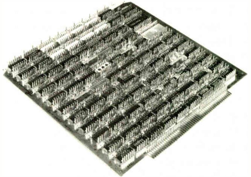
**5. Workhorse.** The model LV7015 (a) is one of the first convolution coder/decoders to have become commercially available. It reduces signal-to-noise level requirements in a communications-satellite data link by over 5 dB—a reduction otherwise attainable only by tripling the area of the receiving earth station's antenna. Most of the ICs used in the single printed-circuit board (b) in the LV7015 are devoted to decoding the test functions.
