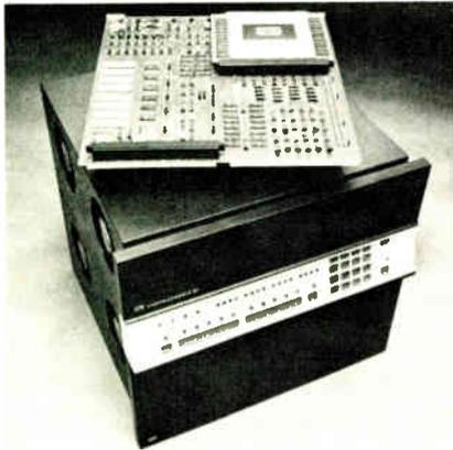
standards two years ago, now has a full 16-bit minicomputer on a single plug-in 15-by-16-inch circuit board for under \$1,000.
