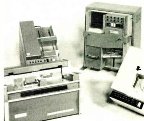
allows accurate single selection of cards even when the cards are worn or damaged. A finger-like device brings a vacuum to the leading corner of the card, drawing it down to meet the friction transport system for positively controlled, constant-velocity travel past the read station. Electronic Associates Inc., West Long Branch, N.J. 07764 [365]
