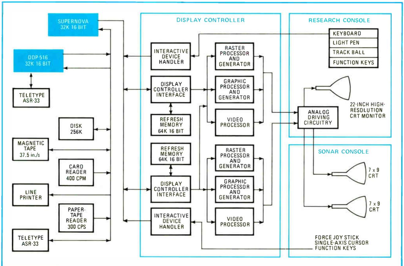
faces and the interaction tools became clear. To the system they appear as standard peripherals with high priority; they are controlled by a modification of the basic disk-operating system supplied by the manufacturers. The resulting monitor system is called an integrated disk-operating system, IDOS (Fig. 6).
