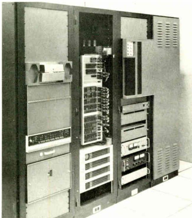
**1. Sonar simulator.** One minicomputer, the two display-control channels, and additional memory are all housed in these four racks. Central computer, a Supernova, is visible in the middle of the nearest rack; the second computer, containing a model of the ocean, stands alone and is not visible here.
