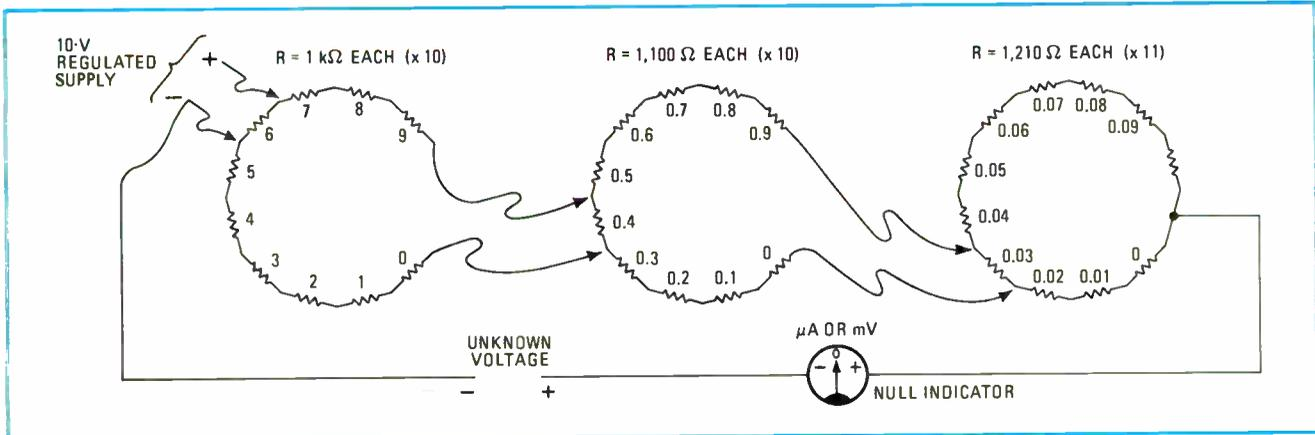
**Dial a voltage.** Circular resistor arrangement trims resistor count without sacrificing precision. The output voltage of this bridge can be set from 0 to 10 volts, to within 0.01 V. All resistors in the same ring have the same value, which is 1.1 times larger than the value of the resistors in the preceding ring. Resistors in the first ring must be able to withstand the full supply voltage. Just 31 resistors are used here.
