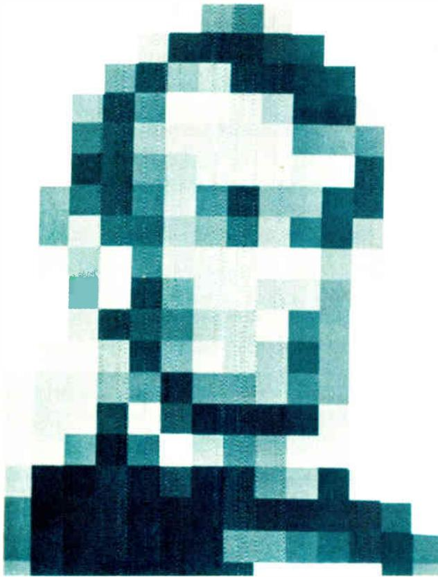
**3. Computer cubism.** To learn what is the least amount of visual information a picture may contain and still be recognizable, researchers at Bell Labs, with the help of a computer, processed this picture of Lincoln. The picture contains about 800 bits of information (about 200 picture elements, each containing four bits of gray-shade information). With conventional teletypewriter codes, only about 12 to 15 words could be transmitted using the same 800 bits.
