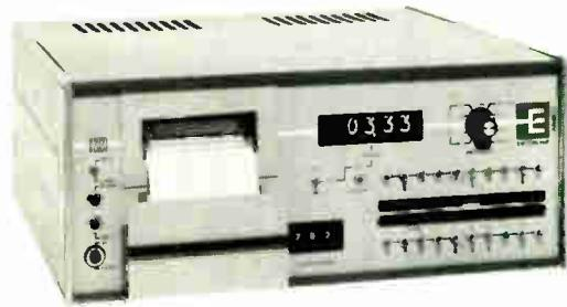
Esterline Angus D-2020 P.D.A.S. (programmable data acquisition systems) give you 5 to 200 channels, 0.1% accuracy, a hard copy record, computer compatibility—and a cost per hundred channels comparable to multi-point analog recorders. Ours is second-generation, with more than 100 in use—many repeat customers.
