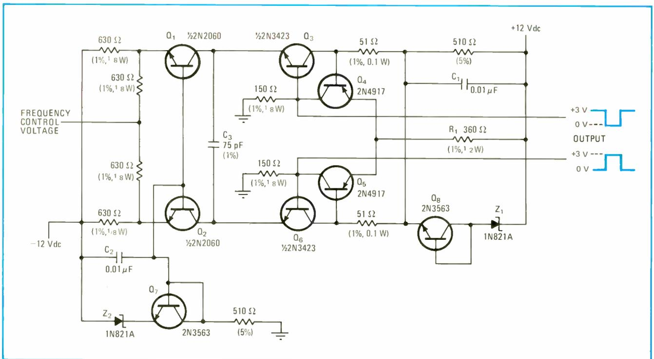
**Simplified design.** Square-wave generator supplies complementary outputs whose frequency is determined by an input control voltage. This control voltage determines the current provided by transistors  $Q_1$  and  $Q_2$  to charge capacitor  $C_3$ . The charge rate of this capacitor sets the switching frequency of the two Schmitt triggers, which are formed by transistors  $Q_3$  and  $Q_4$  and transistors  $Q_5$  and  $Q_6$ .
