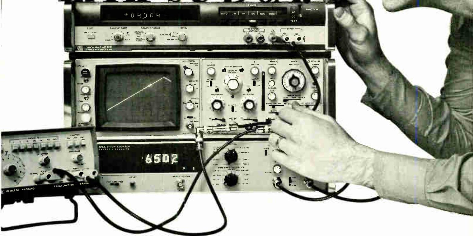
By adding a Sample and Hold option to our Self-Test 3490A, we've made a good DMM even better. And more accurate. Now, you'll be equipped to test ramp linearity; and pulse droop; and hysteresis; and peak amplitude — all at 0.01% resolution.
