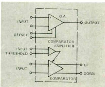
verter race isn't on one chip, but it is a building block that, combined with a d-a converter and a counter, forms a complete, high-speed tracking eight-bit a-d converter for under \$20 in 100-unit orders. Complete a-d converter modules are considerably higher in price.
