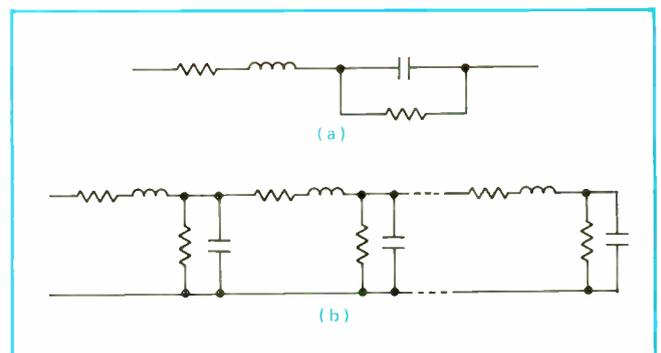
1. **A look inside.** Lumped-parameter equivalent circuit (a) can be used to model the capacitor at very high frequencies. But in the microwave region, a distributed-parameter configuration (b) must be used instead. Capacitance increases with rising frequency.
