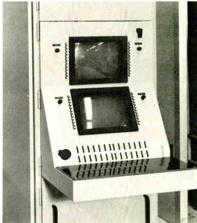
**2. Simulated sonar console.** Vertical rows of switches beside the two screens are programmable function switches; labels for them appear alongside on the screen, as in Figs. 3 and 4.
