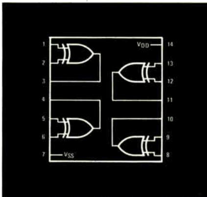
Pin for pin compatible with CD-4030A.
