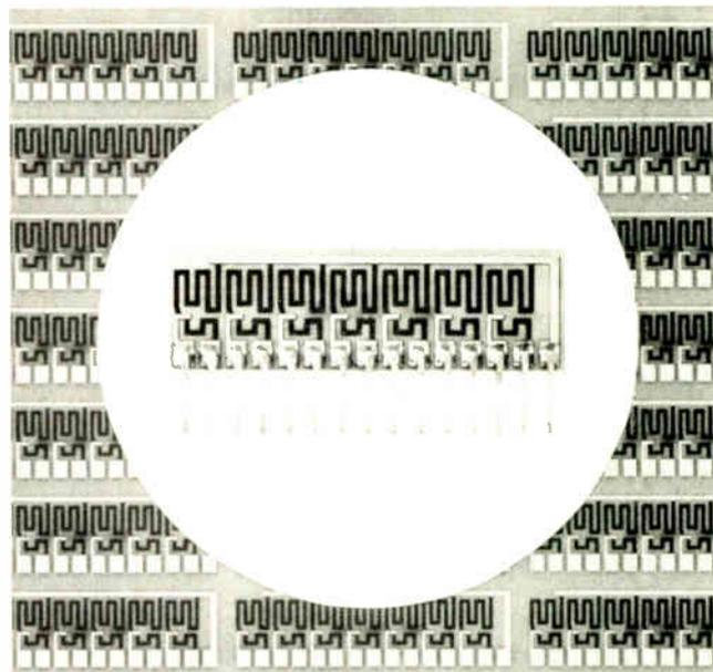
**3. Mass production.** Dark regions are the thin-film resistors and light regions are the conductors on this desk calculator plug-in resistor board. Printed-circuit techniques etch both conductors and resistors of 95 such circuits prior to their separation.
