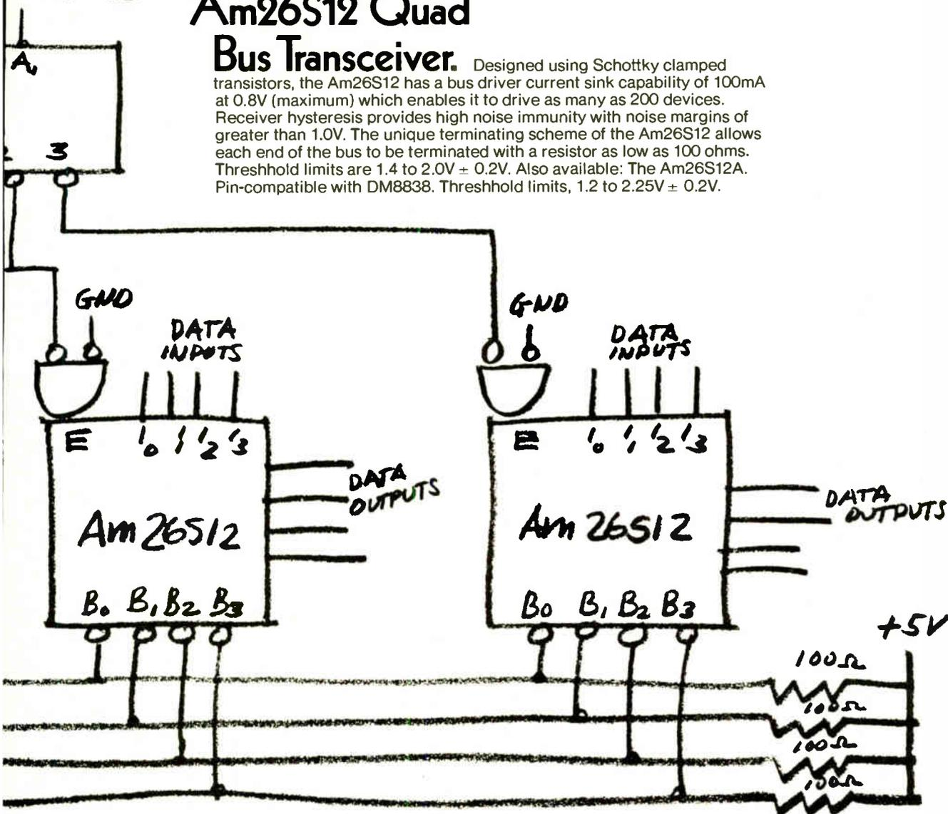
It's a bus driver with the world's highest drive capability and a bus receiver with unbelievably high noise immunity together in a single package.
