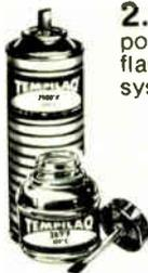
**2. TEMPILAQ<sup>®</sup>:** materials of calibrated melting points suspended in an inert, volatile non-flammable vehicle. Available in over 100 systematically spaced temperature ratings from 100° to 2500°F. Tempilaq<sup>®</sup> indicates its temperature rating by liquefying within  $\pm 1\%$  of its rating. Available in bottles or spray cans.
