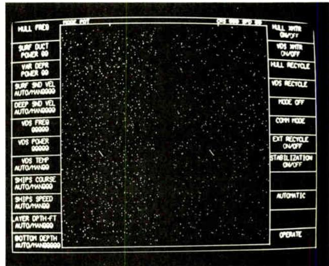
**4. Variable depression search.** The pips in this simulated display, apparently random, actually lie along vertical lines. One line shows echoes along a single beam, with range increasing from bottom to top; six such adjacent lines produce data history for a beam. Several beams make up one half display. Two halves of screen show echoes from two kinds of pings separately generated and processed. Short lines identify an area to be expanded on another screen.
