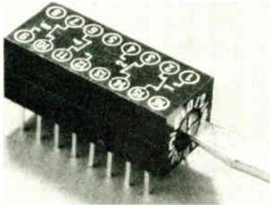
tion. A slot in the end of the switch housing provides screwdriver access to rotate the cam. Settings are indicated by a pointer and associated legend, while the contacts provide positive detent action to eliminate off-center stopping. A minimum of 2-oz.-in. torque is required to release the detent.
