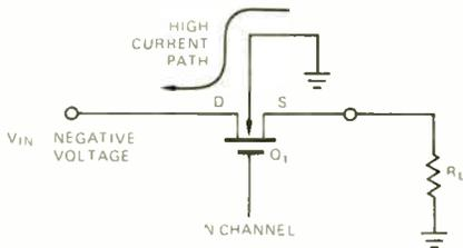
Figure 2. Intersil's Floating Body Process eliminates latch-up with a diode between the N-channel FET body and the positive supply.
