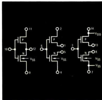
Pin for pin compatible with CD-4007A.
