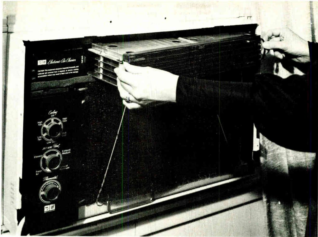
**5. Clean air.** An electrostatic precipitator, which attaches to a residential room air conditioner, has been developed by Frigidaire to provide an air-cleaner feature. Electrically charged dirt particles drawn into the room are attracted to a collection plate of opposite charge.
