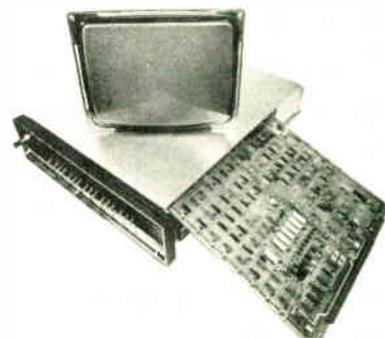
features a 2,000-character MOS random-access memory that is organized to give an 80-column-by-25-row format. Use of the RAM eliminates latency time and the need for interrupt programing. The unit also includes a keyboard control, the operation of which does not require a teletypewriter interface. Price is \$1,585.
