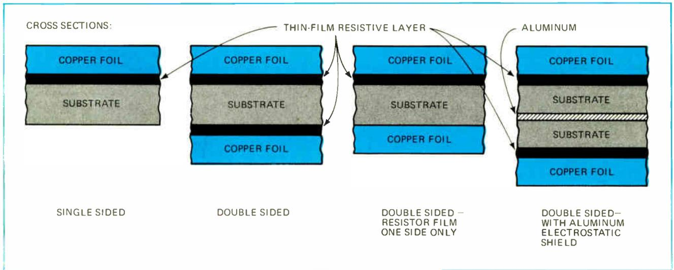
**1. Resistor-filled sandwiches.** Copper-resistor printed-circuit-board laminate can be fabricated in single- and double-sided variations. Copper foils can serve as conductors or as heat sinks to soak up power dissipated by planar resistors.
