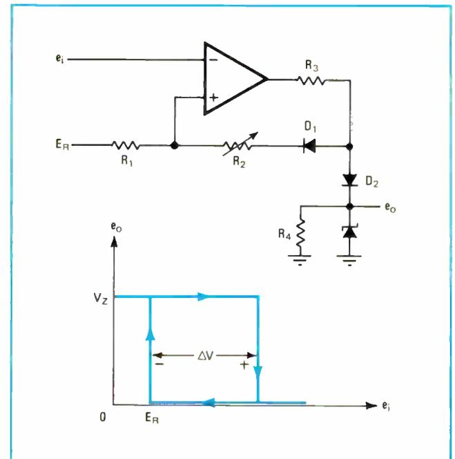
**Controllable hysteresis.** Positive feedback circuit for analog op-amp comparator does not shift the initial reference trip point while introducing hysteresis in the second trip point. The voltage difference,  $\Delta V$ , between the trip points can be adjusted by varying resistor  $R_2$ . When the output voltage is taken from the zener diode, as shown, it switches between zero and  $V_Z$ , the zener voltage.
