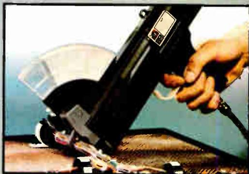
Our other new production tool, the high speed TR-300, automatically positions a TY-RAP tie around bundle, cinches to a preset tension, locks tie securely and trims evenly... all in 8/10 of a second... and on bundle diameters ranging from 1/32" to 5/8".
