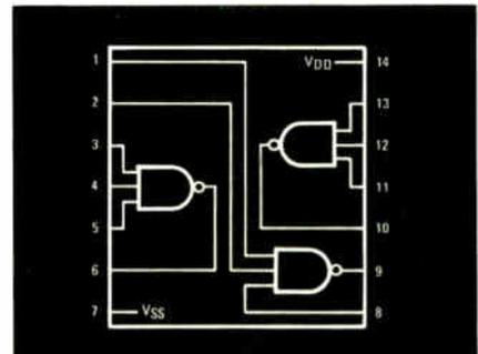
Pin for pin compatible with CD-4023A.
