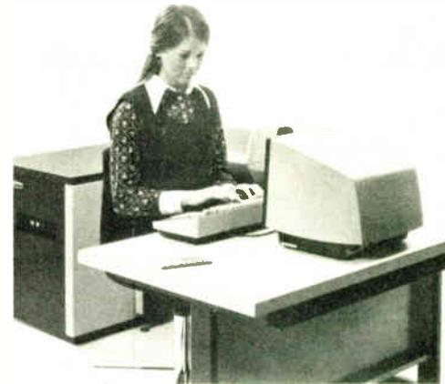
video terminals at a remote site and can be expanded to handle up to 16 video terminals and 16 printers. The unit is communications-compatible with IBM computers. The IV/40 may additionally be used with a central data base for real-time data entry and retrieval.
