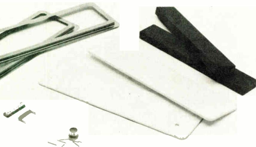
**Piece offering.** These are the parts of the pc-board TWT built by Varian for the military. Two thin-film circuits replace helix winding as well as other parts of conventional tubes.
