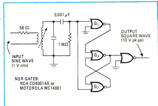
**Squaring circuit.** Link-coupled tuned circuit provides transformer-like action, stepping up the low-level drive signal supplied by most standard oscillators. This permits complementary-MOS gates, the threshold voltages of which are generally 5 to 7 volts, to be used without adding extra active devices. With this squaring circuit, a 1-v sine wave is converted to a 10-v square wave at megahertz rates.
