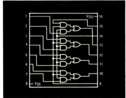
Pin for pin compatible with CD-4019A.
