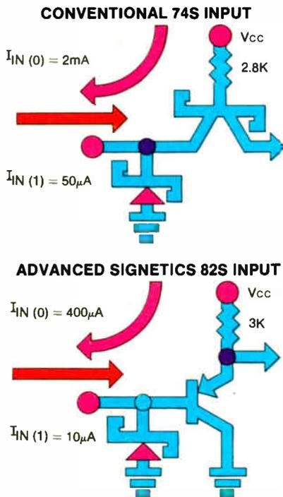
The growing line of 82S includes ultra high speed pin-for-pin replacements for the popular 8200 series MSI. In addition, the 82S90/91 100 MHz counter will replace the 74196/197, and the 82S70/71 70 MHz shift register will replace the 74178/179 in systems requiring improved speed performance.
