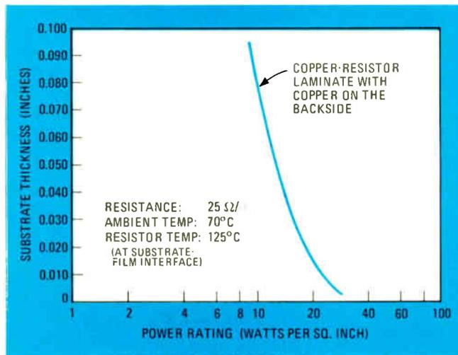
**2. The path out.** Negative slope of the curve indicates that the thinner the board, the higher the dissipation capability of the laminate. Higher dissipation for the thinner board is due to the shortened thermal path from the resistive film to the foil on the back.
