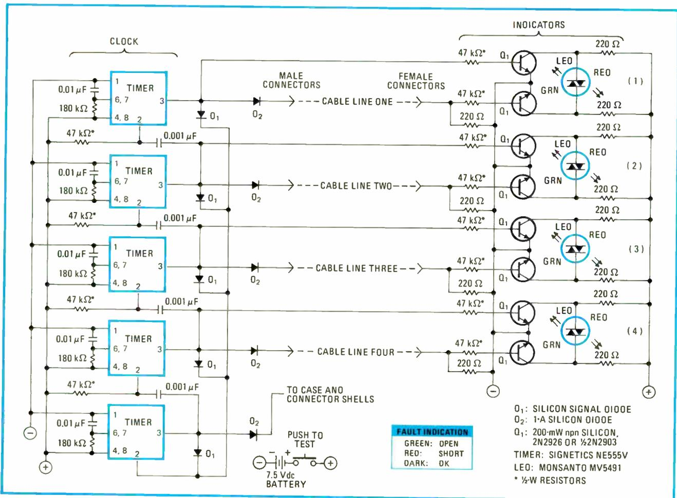
**Finding cable faults.** Compact tester checks cables for open-circuit or short-circuit conditions. A differential transistor pair at one end of each cable line remains balanced as long as the same clock pulse—generated by the timer ICs—appears at both ends of the line. A clock pulse just at the clock end of the line lights a green light-emitting diode, and a clock pulse only at the other end lights a red LED.
