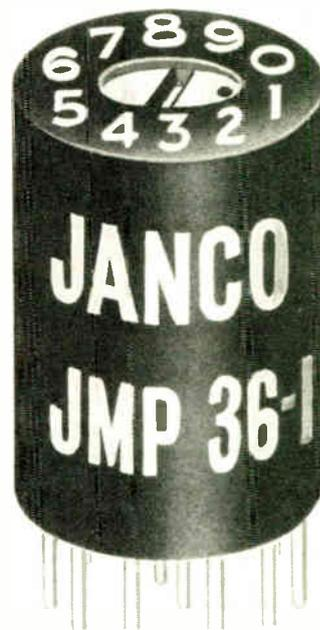
discrete components normally used on pc boards. The switch pin terminals are set to fit a TO-100 grid pattern. The unit has a 36° angle of throw, 10 positions, and one or two poles, in addition to bridging functions. Voltage breakdown is 500 v ac minimum between mutually insulated parts, and electrical rating is 2 A continuous.
