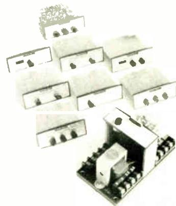
applications for photoelectric controls. Functions offered include on-off, time delay, and impulse types for registration. Other functions are planned for future additions.
